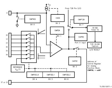
FIGURE 1. COP888EK Analog Function Block
