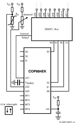
FIGURE 3. Expansion of A/D Channels
