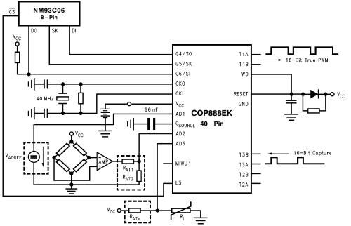
FIGURE 2. COP888EK with Strain Gauge Transducer
