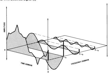
FIGURE 3. Combined Time Domain and Frequency Domain Plots
