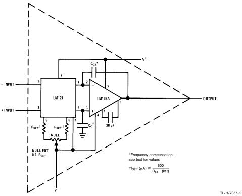
FIGURE 9. General Purpose Amplifier Using the LM121
