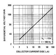
FIGURE 5. Gain vs Set Current
