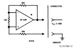
\*Op amp shown in Figure 9. **FIGURE 3. Drift Measurement Circuit**
