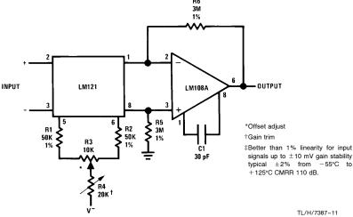
FIGURE 11. Gain of 1000 Instrumentation Amplifier
