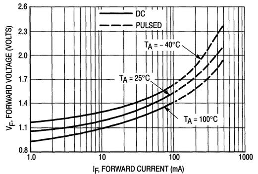
Figure 2. LED Forward Voltage versus Forward Current
