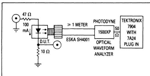
**Figure 2. Optical Turn-On and Turn-Off Test Setup**
