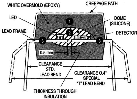
The DOME package is a manufacturing/quality improvement in that it represents a significant reduction in the complexity of the assembly steps. This is consistent with Motorola's goal of continual quality improvement by reduction in process variations (in this case through assembly simplification).
