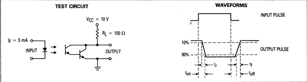
Figure 9. Switching Times
