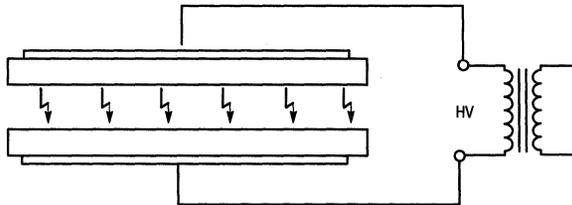
Figure 1b. Corona Discharge Between Two Glass Plates
