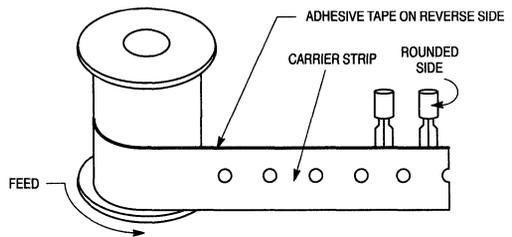
Rounded side of transistor and carrier strip visible
