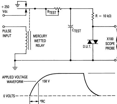
1. The mercury wetted relay provides a high speed repeated pulse to the D.U.T.
