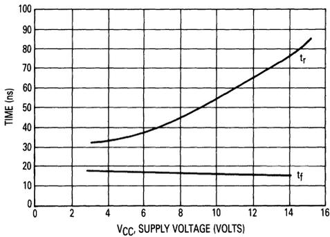
Figure 8. Pulse Response Time versus Supply Voltage
