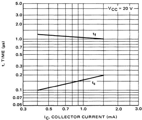
FIGURE 22 – Switching Storage and Fall Times for MRD300
