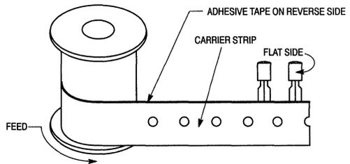
Flat side of transistor and carrier strip visible
