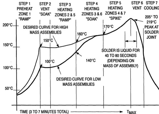
Figure 1. Typical Solder Heating Profile
