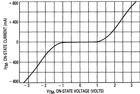
Figure 2. On-State Characteristics
