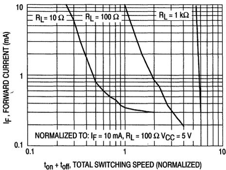
Figure 6. Input Current versus Total Switching Speed
