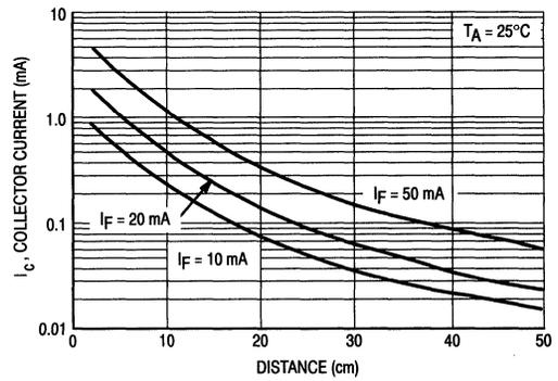
Figure 6. Current Transfer with Devices Optically Coupled
