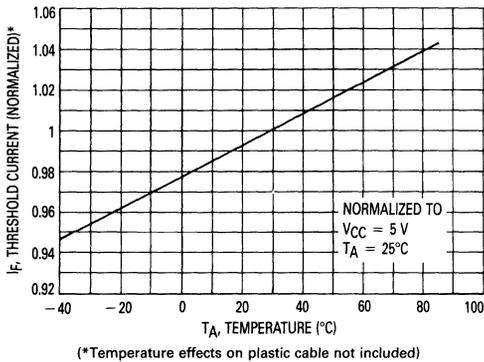
Figure 10. Threshold Current versus Temperature
