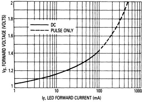
Figure 1. LED Forward Voltage versus Forward Current
