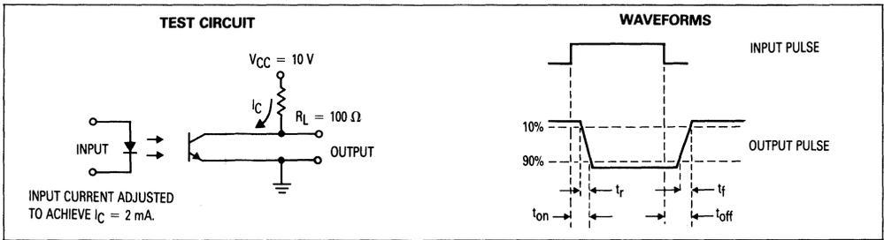
Figure 11. Switching Times
