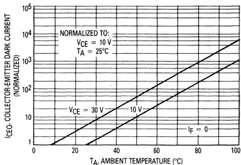
Figure 4. Collector-Emitter Dark Current versus Ambient Temperature
