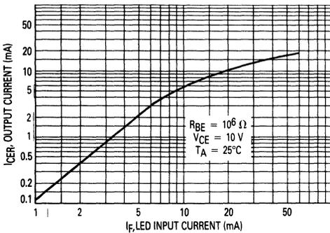
Figure 1. Output Current versus LED Input Current
