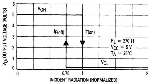
Figure 2. Transfer Characteristics
