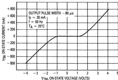
Figure 1. On-State Characteristics
