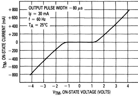
Figure 1. On-State Characteristics
