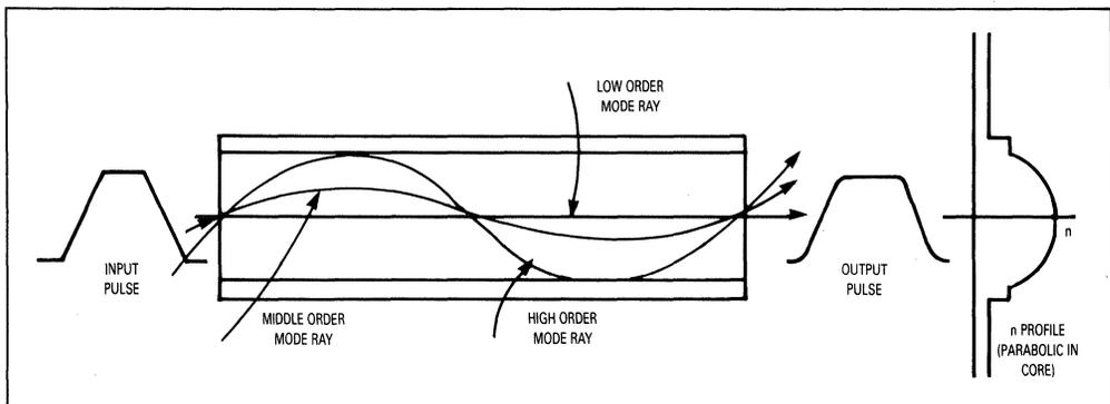
Figure 16. Propagation Along A Multimode Graded Index Fiber
