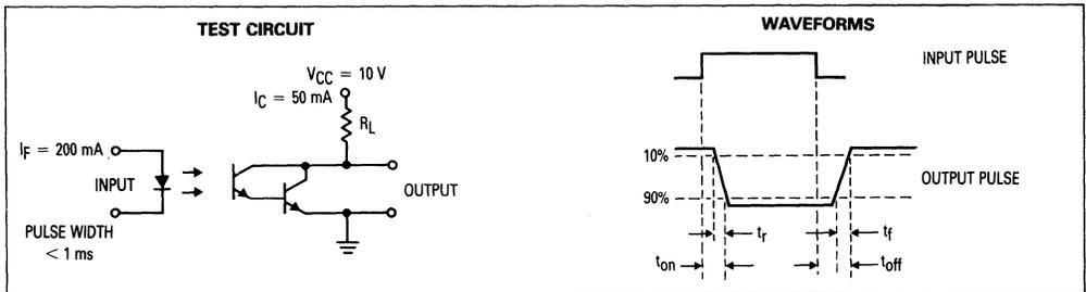
Figure 11. Switching Times
