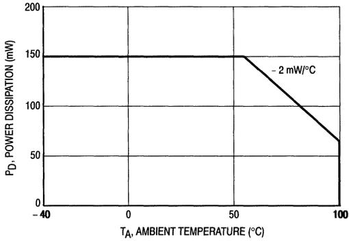
Figure 1. Power Dissipation
