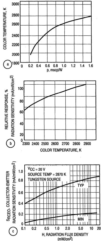
1. To predict light-sensing system performance, an incandescent source description is obtained from curve "a". Once this is done, the phototransistor relative response is obtained from "b". After calculating the radiation flux intensity, H, on the basis of data from "a" and "b", you can read the actual phototransistor radiation sensitivity from "c".
