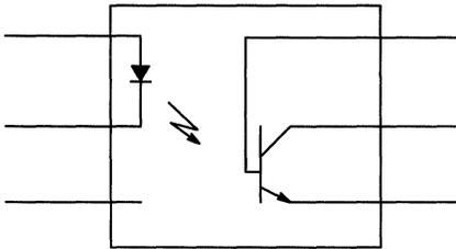
Figure 3. Transistor Optocoupler
