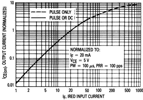
Figure 1. Typical Output Current versus Input Current
