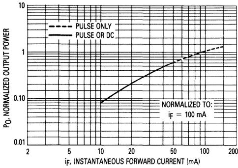
Figure 1. Normalized Output Power versus Forward Current
