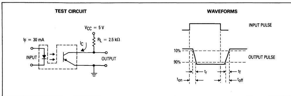
Figure 9. Switching Times
