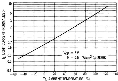
Figure 2. Normalized Light Current versus Temperature
