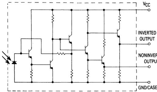
Figure 1. Equivalent Schematic
