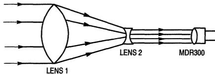
2. Photocurrent can be increased by collecting more light from the source. The radius of lens 2 is equal to the radius of the lens built into the phototransistor.
