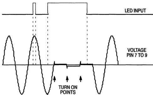
Figure 12. Operating Waveforms
