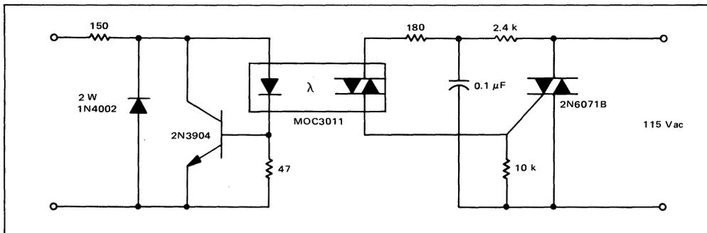
FIGURE 10 – Solid-State Relay
