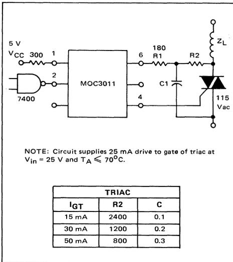
NOTE: Circuit supplies 25 mA drive to gate of triac at  $V_{in} = 25 \text{ V}$  and  $T_A \leq 70^\circ\text{C}$ .
