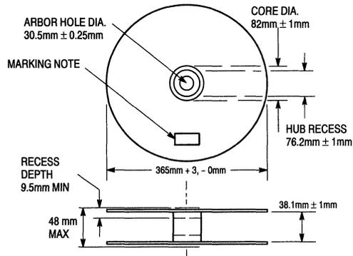
Material used must not cause deterioration of components or degrade lead solderability
