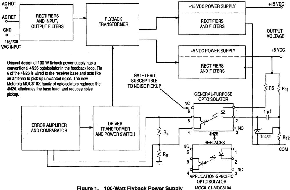
Noise is further reduced by coplanar die placement of the LED and phototransistor. This reduces the internal capacitance to 0.2 pF and minimizes the coupled noise injected by the optoisolator.
