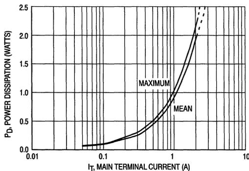
Figure 7. Power Dissipation versus Main Terminal Current
