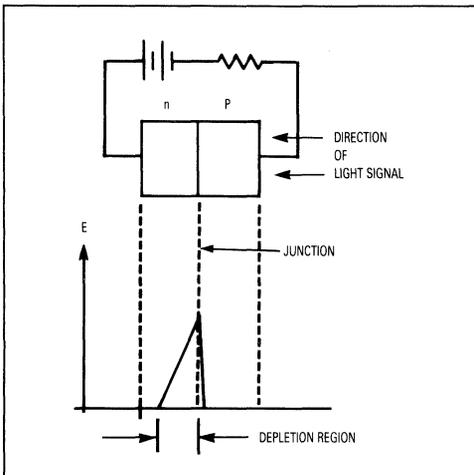
Figure 29. Electric Field In A Reverse-Biased PN Photodiode
