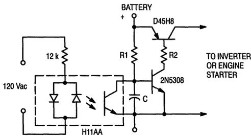
Figure 3. UPS Solid State Turn-On Switch
