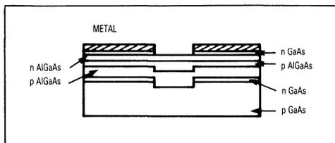
Figure 22. Section AA Of Planar Heterojunction LED
