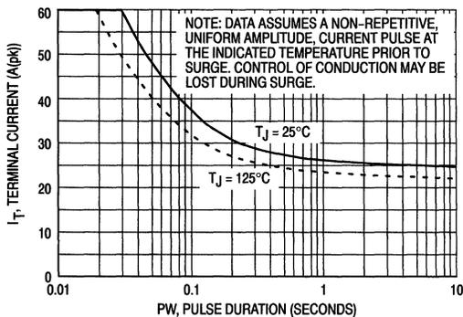
Figure 5. Maximum Allowable Surge Current versus Pulse Duration
