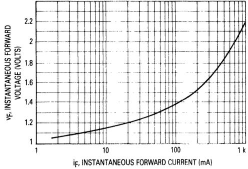
Figure 2. Forward Characteristics
