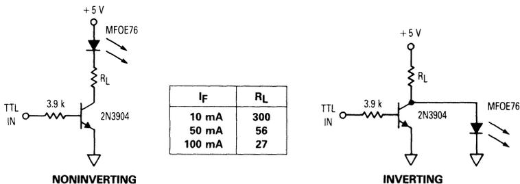
Figure 6. TTL Transmitters
