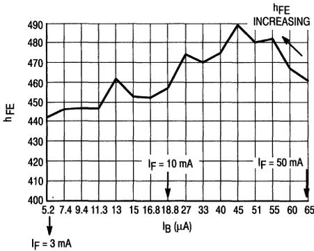
Figure 5.  $h_{FE}$  versus Photo Generated Current ( $I_B$ )
