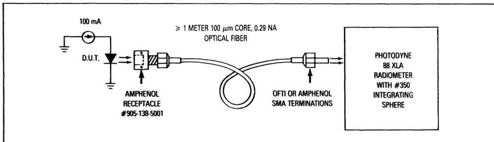
Figure 4. Launched Power (P<sub>L</sub>) Test Set
