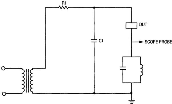
Figure 3. Narrowband Partial Discharge Test Circuit
