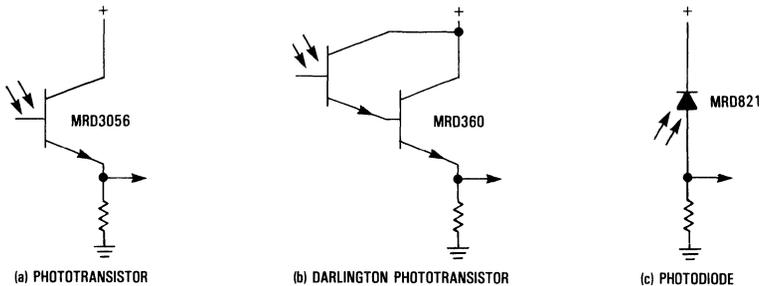
Figure 2. The Basic Detectors for IR Photosensing
