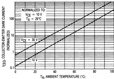
Figure 4. Dark Current versus Ambient Temperature
