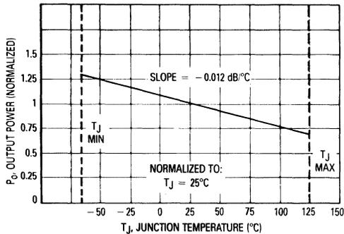
Figure 2. Power Output versus Junction Temperature
