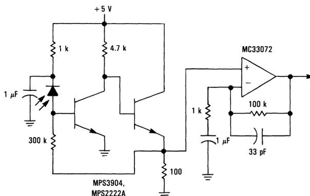
Figure 7. Simple Discrete Front End with Op Amp
