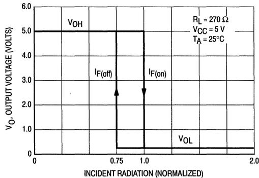
Figure 1. Transfer Characteristics
