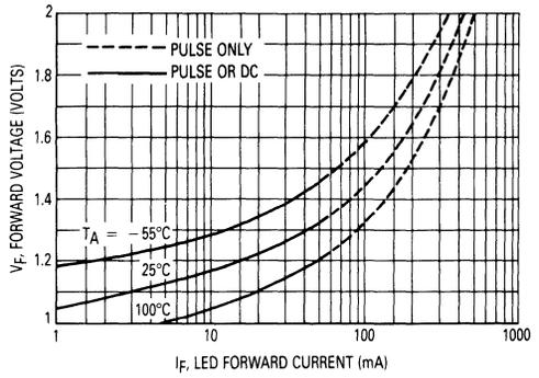
Figure 4. Forward Characteristics
