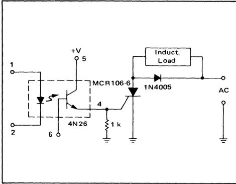
FIGURE 11 – Coupler-Driven SCR
