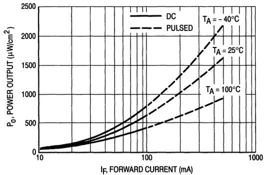
Figure 2. Power Output versus Forward Current
