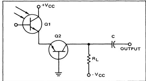
FIGURE 32 – Improved Speed Configuration for Phototransistor
