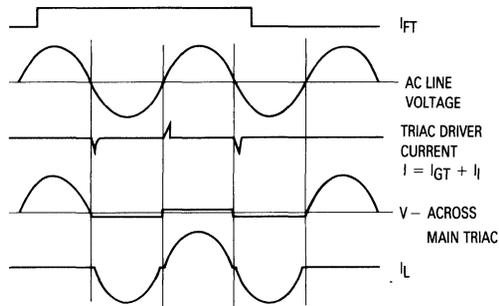
Figure 8. Waveforms of a Basic Driving Circuit
