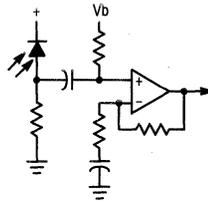
(b) DIRECT-COUPLED DIODE FRONT END
