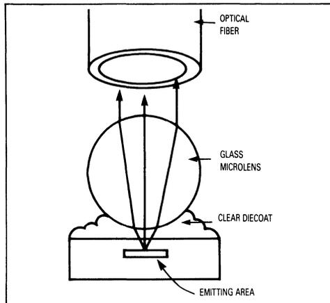
Figure 23. Increasing Light Coupling With A Microsphere
