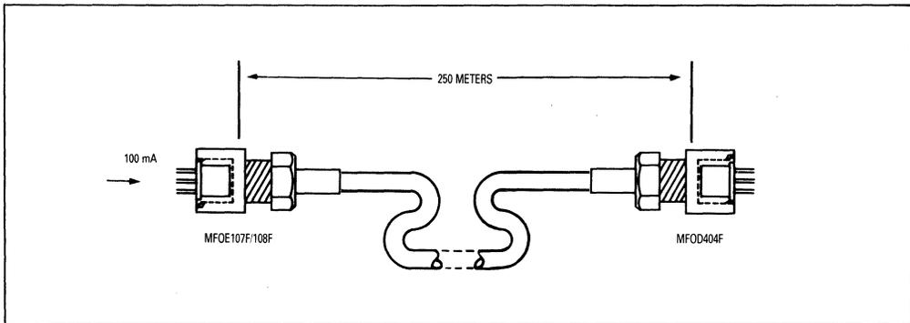
Figure 38. Simplex Fiber Optic Point To Point Link
