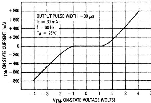
Figure 1. On-State Characteristics
