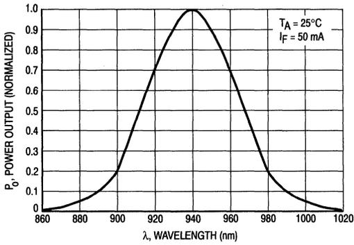
Figure 3. LED Relative Power Output versus Wavelength
