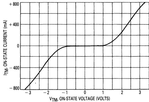
Figure 2. On-State Characteristics
