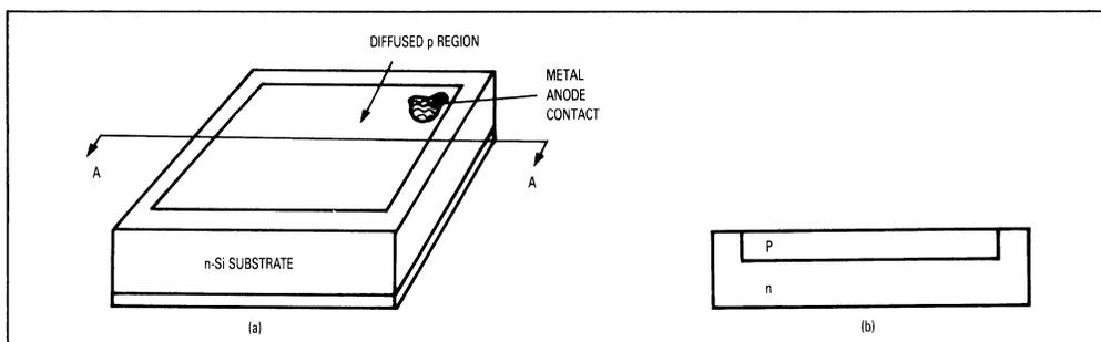
**Figure 27. PN Photodiode:**
