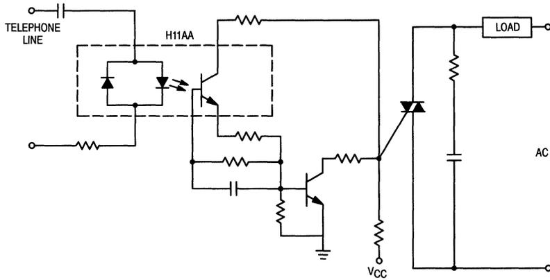
**Figure 4. Power Control by Bell Signal Circuit**
