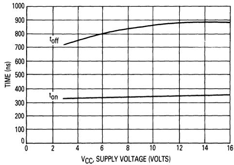
Figure 9. Total Switching Time versus Supply Voltage
