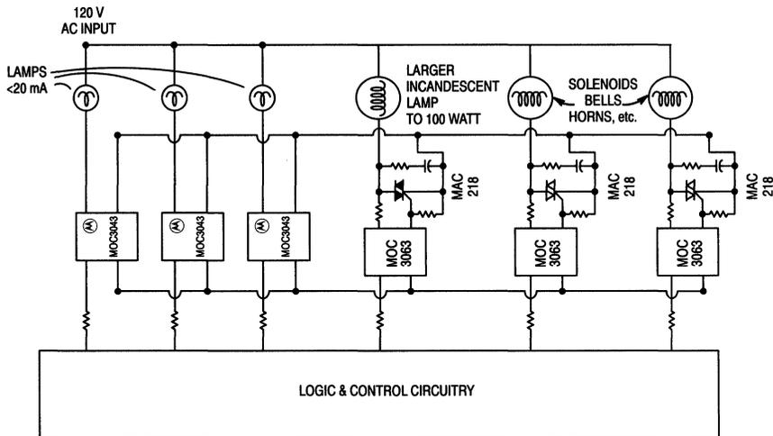
**Figure 3. Gaming Machine or Lamp Control Application**
