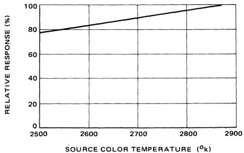
FIGURE 12 – Relative Response of MRD300 versus Color Temperature
