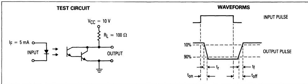
Figure 11. Switching Times
