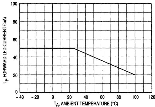
**Figure 1. Maximum Allowable Forward Current versus Ambient Temperature**
