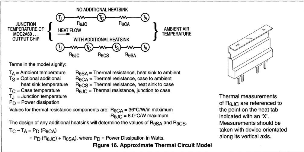
Thermal measurements of  $R_{\theta JC}$  are referenced to the point on the heat tab indicated with an 'X'. Measurements should be taken with device orientated along its vertical axis.
