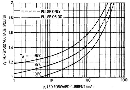
Figure 4. Forward Characteristics
