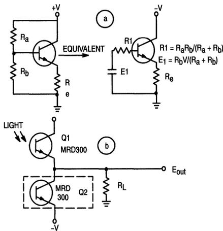
7. Temperature-compensation methods for a three-lead phototransistor are quite similar to a classical bias-stabilization approach (a). In the case of a two lead device, a matched pair of phototransistors can be used, one to receive the normal light input, while the other is masked (b).
