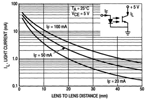
Figure 6. Coupled Characteristics of MLED91 and MRD901
