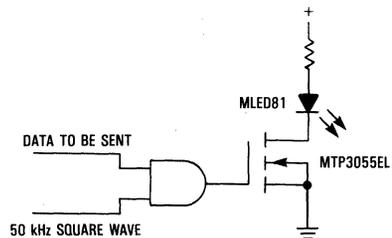
Figure 3. Basic IR Source Drive for CW Operation
