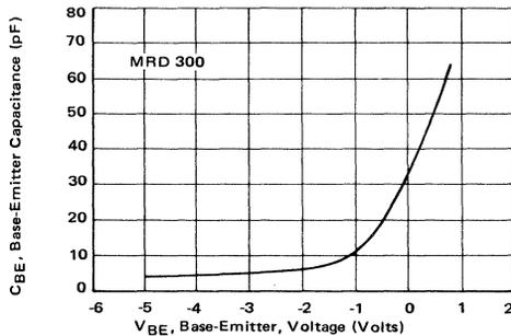
FIGURE 30 – MRD300 Base-Emitter Junction Capacitance versus Voltage
