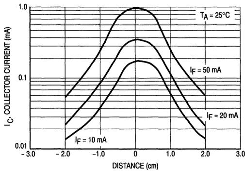
Figure 7. Translational Optical Coupling at 5 mm Separation (Lens to Lens)
