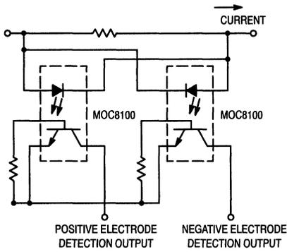
**Figure 7. Telephone Line Polarity Detection Circuit**
