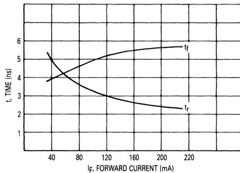
Figure 12. Rise and Fall Time versus Forward Current
