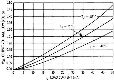
Figure 3. Output Voltage, Low versus Load Current
