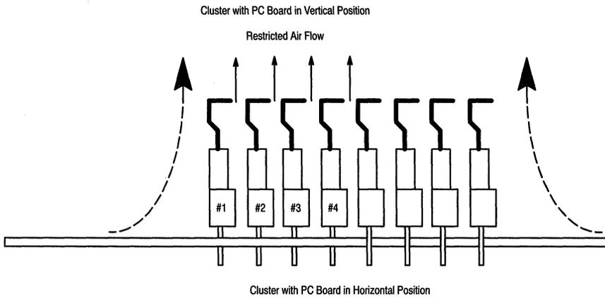
Figure 13. Clusters of Devices on a PC Board
