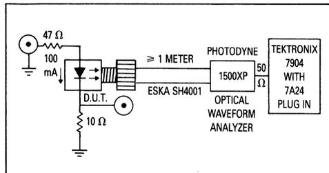
Figure 5. Optical Rise and Fall Time Test Set (10%-90%)
