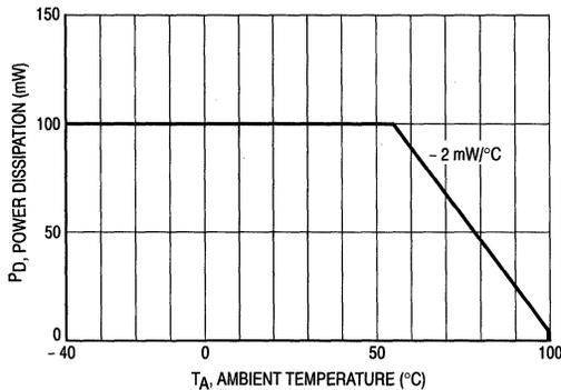
Figure 1. Power Dissipation
