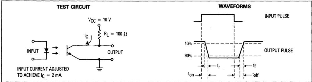
Figure 11. Switching Times
