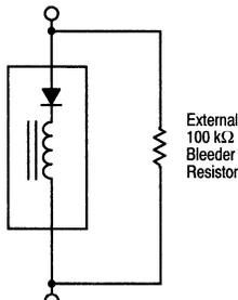
Figure 9. AC-DC Solenoid with Integral Diode
