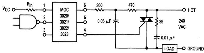
\*This optoisolator should not be used to drive a load directly. It is intended to be a trigger device only. Additional information on the use of optically coupled triac drivers is available in Application Note AN-780A.
