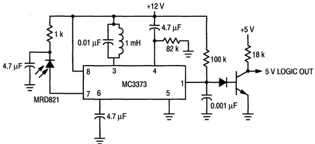
IR Receiver Using the Integrated MC3373, for Ranges of 10–30 Meters
