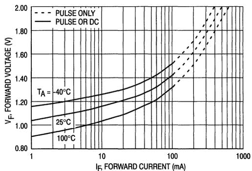
Figure 2. LED Forward Voltage versus LED Forward Current
