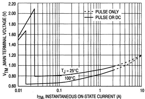
Figure 6. On-State Voltage Drop versus Output Terminal Current
