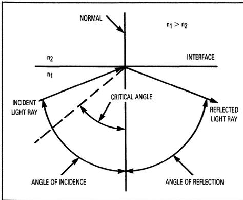
Figure 5. Light Incident At Greater Than Critical Angle
