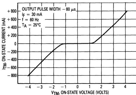
Figure 1. On-State Characteristics
