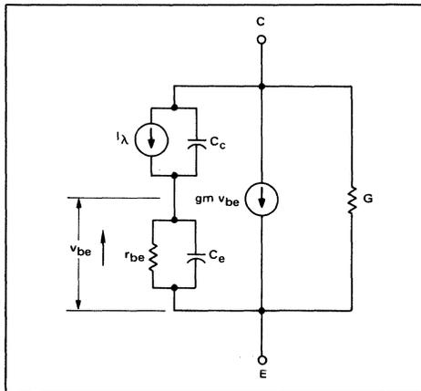
FIGURE 8 - Floating Base Approximate Model of Phototransistor
