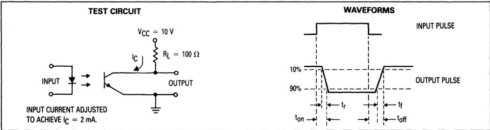
Figure 10. Switching Times
