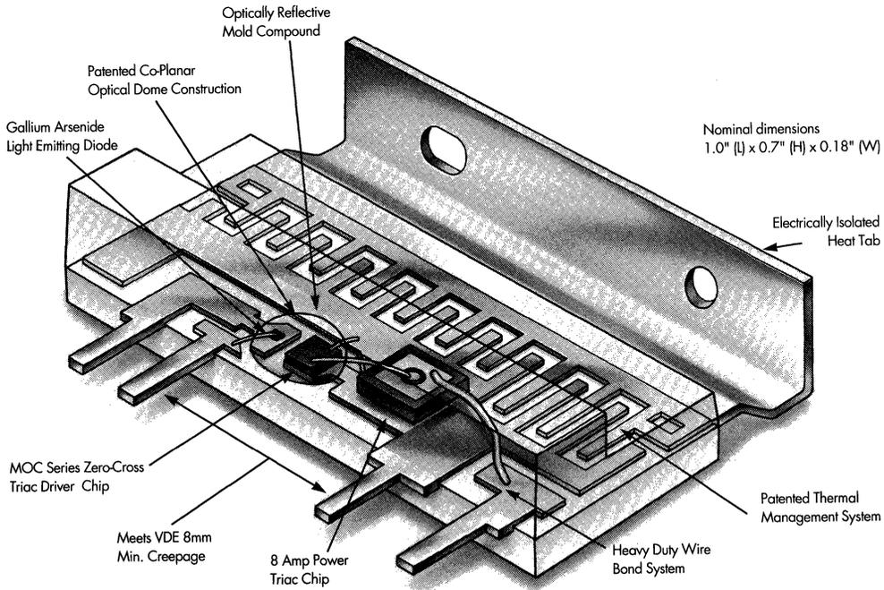
Figure 1. Internal Construction of the POWER OPTO Isolator
