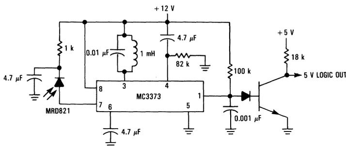
Figure 8. IR Receiver Using the Integrated MC3373
