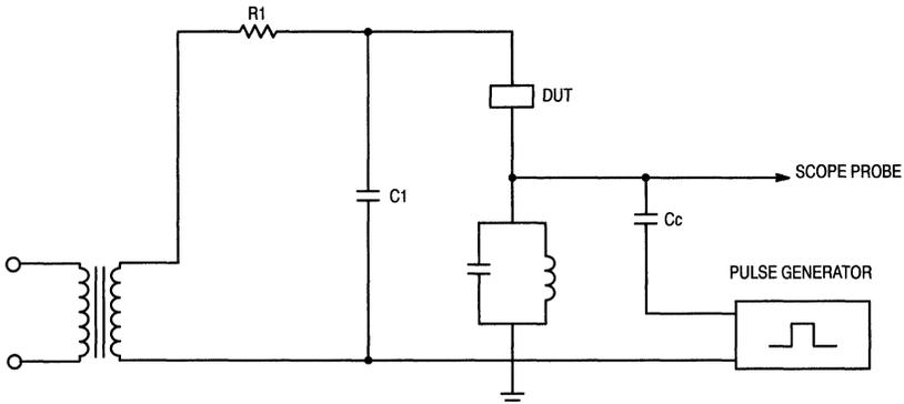
Figure 4. Narrowband Partial Discharge Test Circuit with Calibrator
