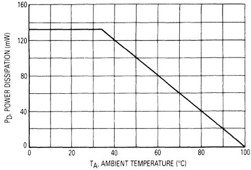
**Figure 8. Power Dissipation**
