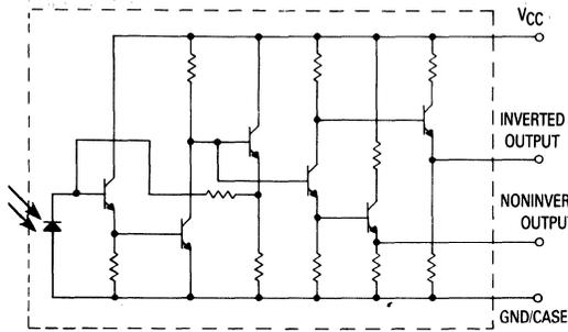
Figure 1. Equivalent Schematic
