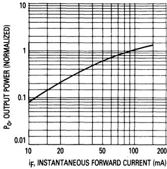
**Figure 3. Normalized Output Power versus Forward Current**
