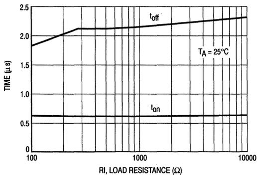
Figure 9. MRD950 Switching Time versus Load Resistance
