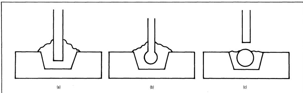
**Figure 25. Fiber Coupling To A Burrus Diode:**
