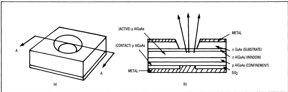
**Figure 24. Burrus, Or Etched Well, LED:**
