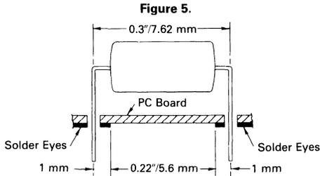
Input/Output Leads —  $L = 0.3"/7.62 \text{ mm}$
