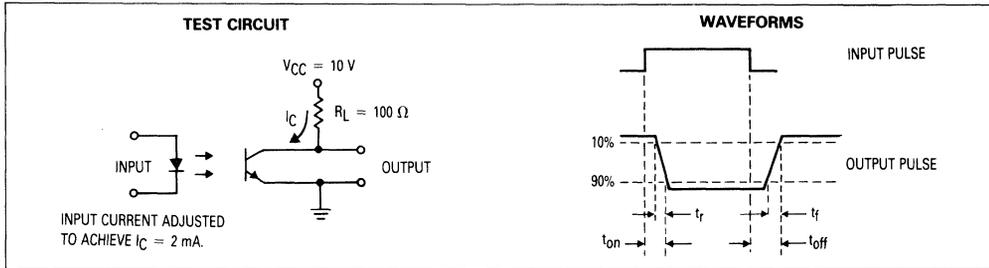
Figure 11. Switching Times
