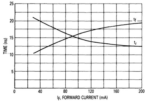
Figure 11. Rise and Fall Time versus Forward Current
