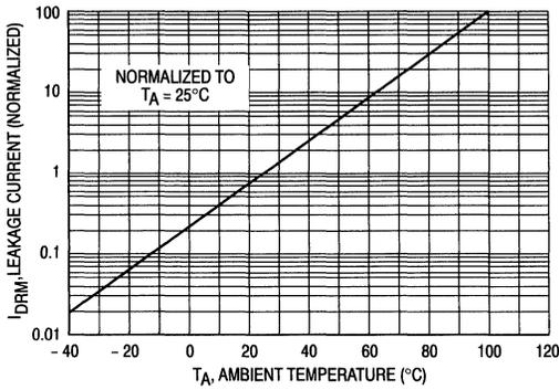
Figure 9. Leakage With LED Off versus Ambient Temperature
