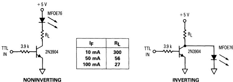
Figure 6. TTL Transmitters
