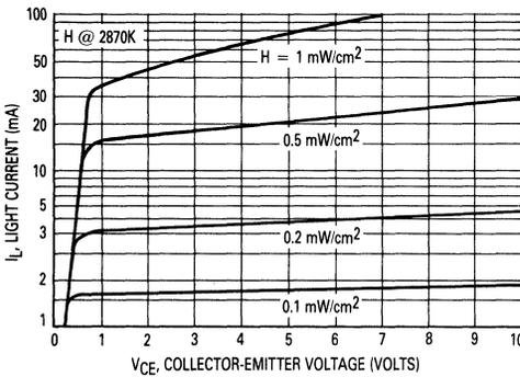
Figure 3. Collector Characteristics
