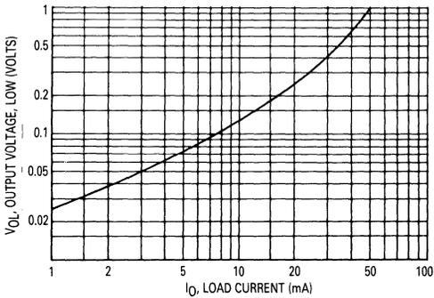
Figure 5. Output Voltage, Low versus Load Current
