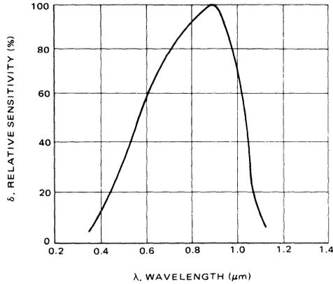
FIGURE 4 – Spectral Response of Silicon Photodiode
