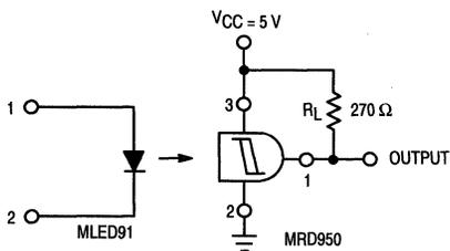
Figure 11. Test Circuit for Threshold Current Measurements
