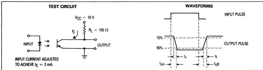
Figure 11. Switching Times
