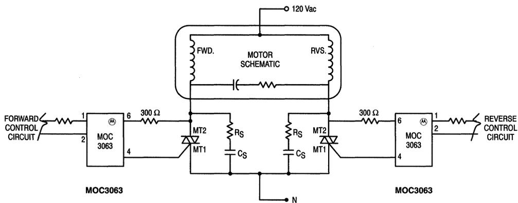
Figure 4. Reversing Motor Application
