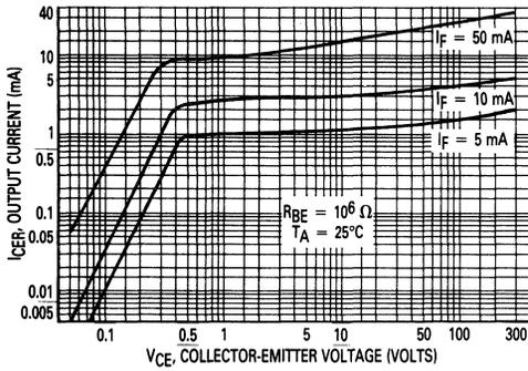
Figure 3. Output Characteristics
