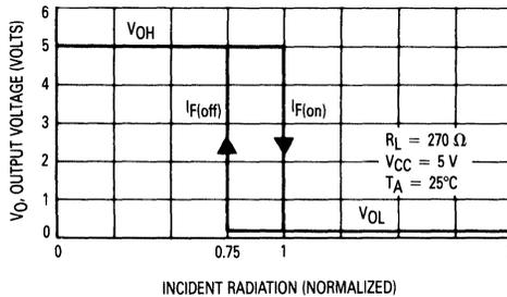
Figure 1. Transfer Characteristics
