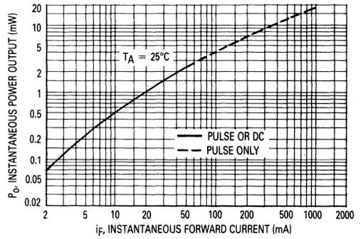
Figure 4. Instantaneous Power Output versus Forward Current
