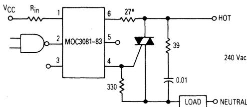
Typical circuit for use when hot line switching is required. In this circuit the "hot" side of the line is switched and the load connected to the cold or neutral side. The load may be connected to either the neutral or hot line.
