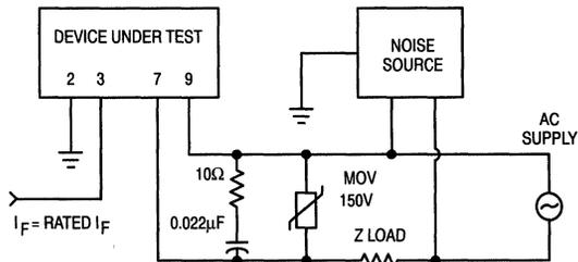
Figure 15. Test Circuit for Conducted Noise Tests
