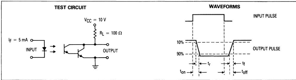
Figure 9. Switching Times
