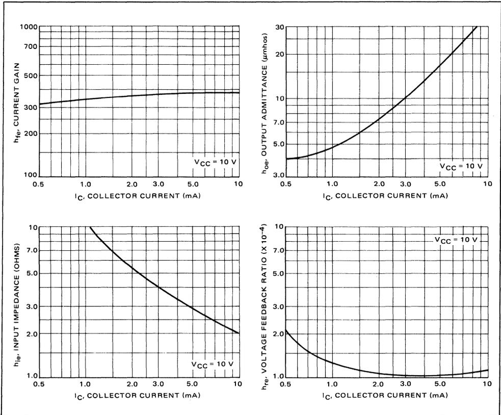
FIGURE 19 – 1 kHz h-Parameters versus Collector Current for MRD300
