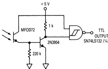
Figure 7. 5 kHz Transistor Receiver
