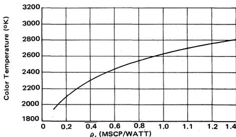
FIGURE 22 – Color Temperature versus Candle Power/Power Ratio
