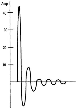
Figure 7. Size No. 4 Contactor Inrush Current
