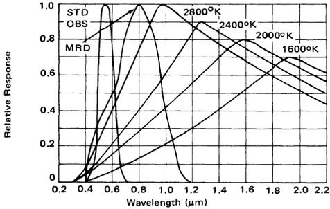
FIGURE 17 – Radiant Spectral Distribution of Tungsten Lamp
