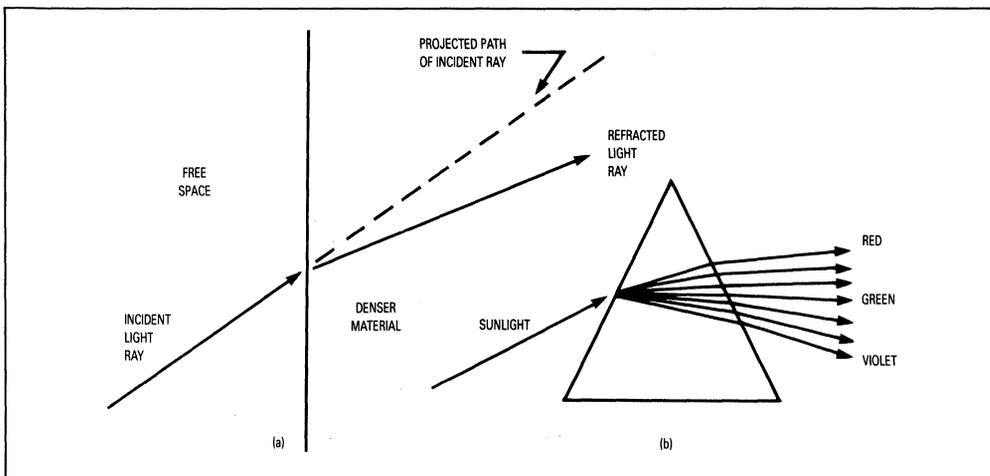
Figure 2. Refraction Of Light:
