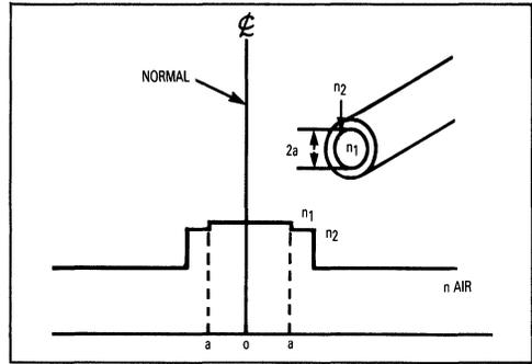
Figure 7. Index Profile For A Step Index Fiber
