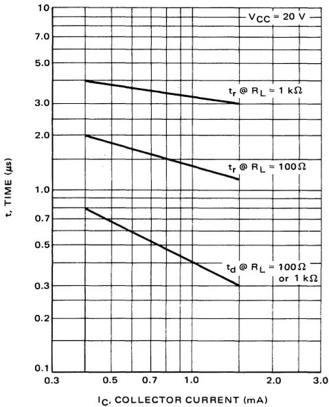
FIGURE 21 – Switching Delay and Rise Times for MRD300
