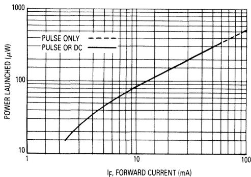
Figure 5. Power Launched versus LED Forward Current
