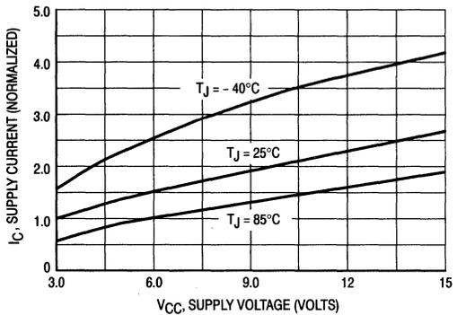
Figure 4. Supply Current versus Supply Voltage — Output High
