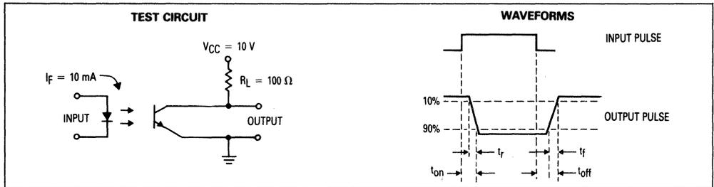
Figure 11. Switching Times
