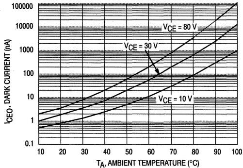
Figure 4. Collector-Emitter Dark Current versus Temperature
