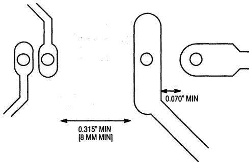
Figure 14. PC Board Layout Recommendations
