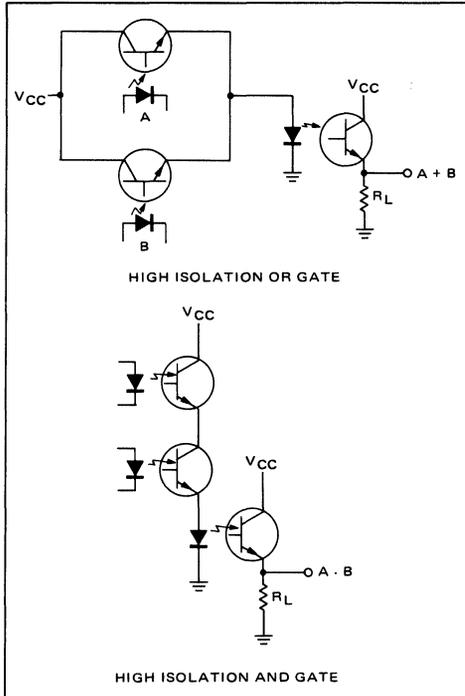
FIGURE 25 – Logic Circuits Using the MRD300 and LEDs
