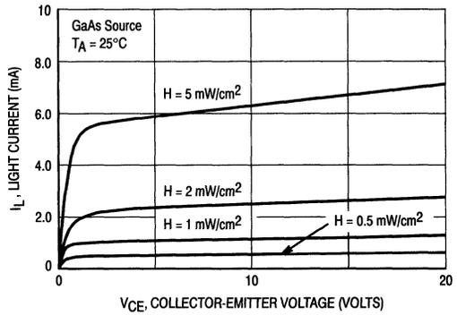
Figure 4. Transistor Collector Current versus Collector-Emitter Voltage
