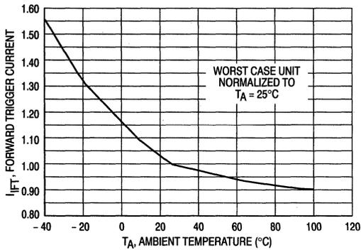
Figure 3. Forward LED Trigger Current versus Ambient Temperature
