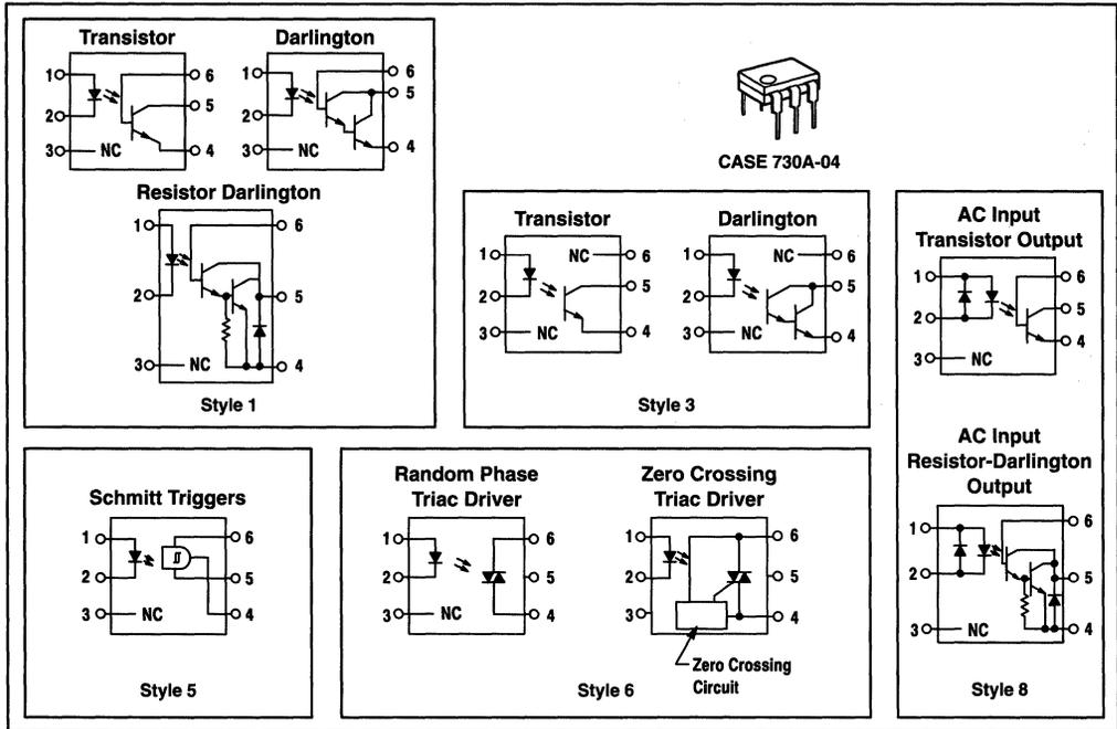
An optoisolator consists of a gallium arsenide infrared emitting diode, IRED, optically coupled to a monolithic silicon photodetector in a wide array of standard devices and encourages the use of special designs and selections for special applications. All Motorola optoisolators have  $V_{ISO}$  rating of 7500 Vac(pk), exceeding all other industry standard ratings.
