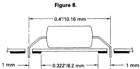
Where the equipment norms demand a clearance and creepage path of 8 mm Min, the coupler input and output leads should be bent to  $0.4"/10.16 \text{ mm}$  and the printboard layout should be as shown.
