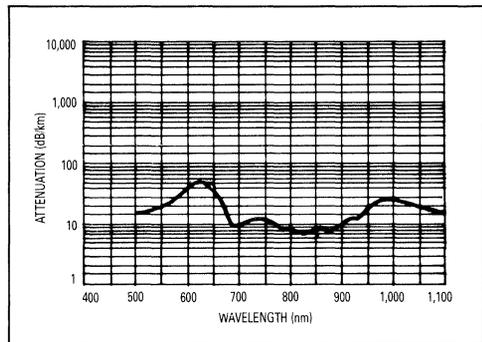
Figure 19. Attenuation versus Wavelength For A Sample Fiber
