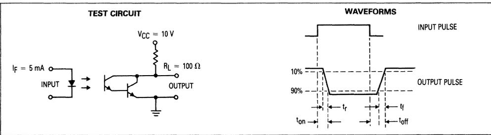
Figure 11. Switching Times
