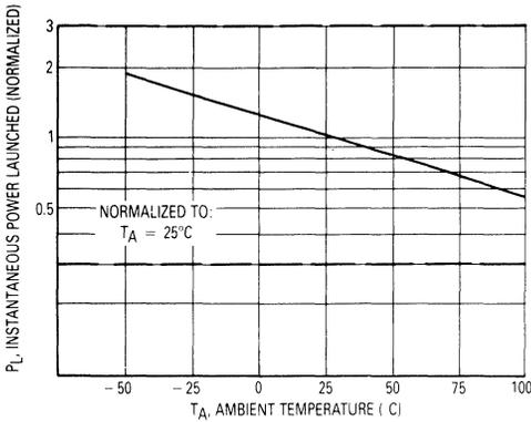
**Figure 7. Instantaneous Power Output versus Ambient Temperature**
