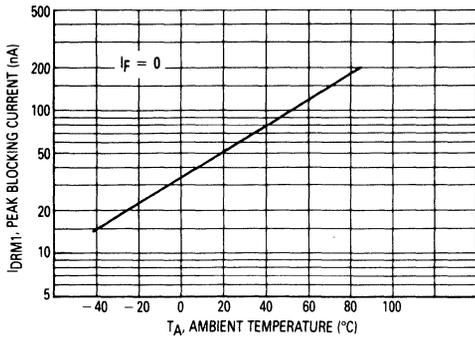
Figure 3. IDRM1, Peak Blocking Current versus Temperature
