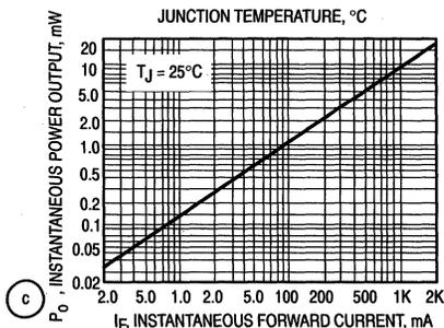
5. In predicting a phototransistor response to a LED, first determine the instantaneous power dissipation of the LED from "a", which is needed for calculating the corresponding junction temperature. With these data, you can determine the LED's power output by using curves "b" and "c" and a few simple calculations.
