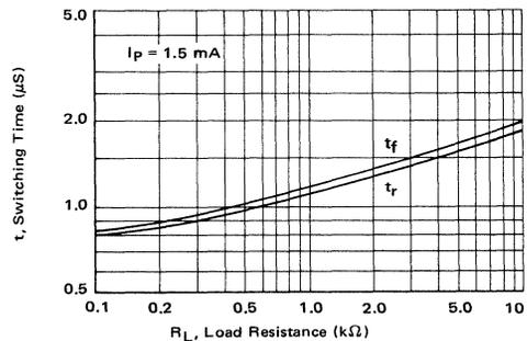
FIGURE 34 – Switching Times with Speed-up Circuit
