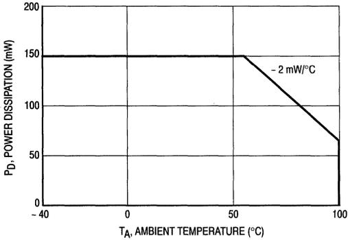
Figure 1. Power Dissipation
