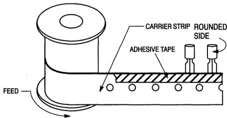
Rounded side of transistor and adhesive tape visible.
