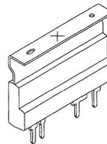
Thermal measurements of  $R_{\theta JC}$  are referenced to the point on the heat tab indicated with an 'X'. Measurements should be taken with device orientated along its vertical axis.
