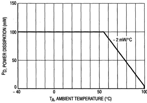
Figure 1. Power Dissipation
