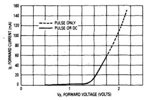
Figure 4. Forward Current versus Forward Voltage
