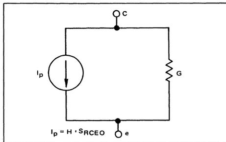
FIGURE 6 — Low-Frequency and Steady-State Model for Floating-Base Phototransistor
