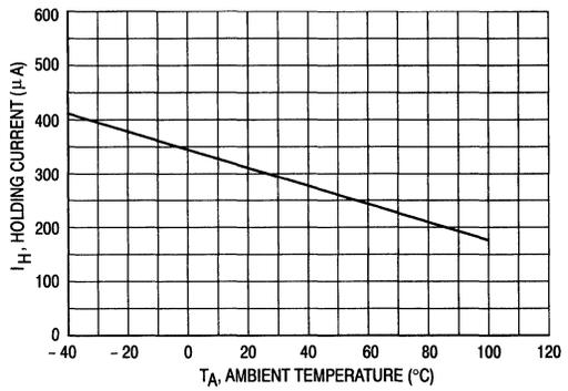
Figure 10. Holding Current versus Ambient Temperature
