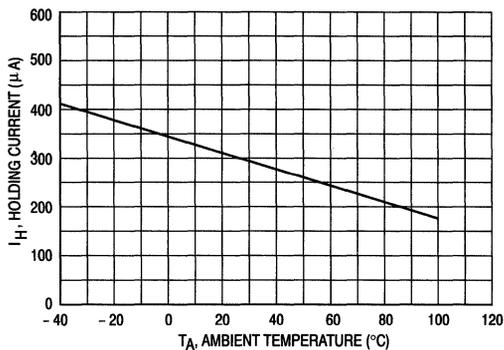
Figure 10. Holding Current versus Ambient Temperature
