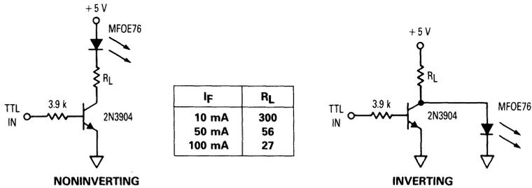
Figure 6. TTL Transmitters
