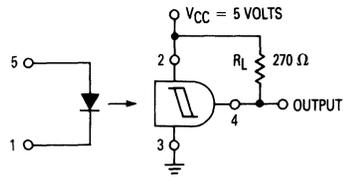
**Figure 6. Test Circuit for Threshold Current Measurements**
