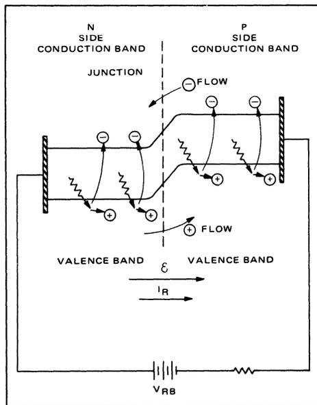
FIGURE 3 — Photo Effect in a Reverse-Biased PN Junction
