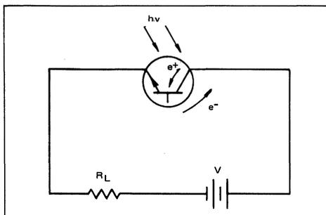
FIGURE 1 - Photo-Generated Carrier Movement in a Phototransistor
