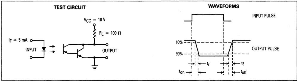
Figure 9. Switching Times
