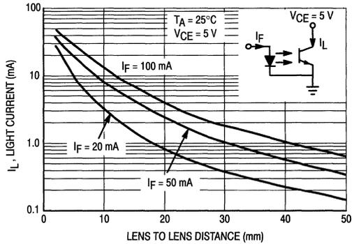
Figure 4. Coupled Characteristics of MLED91 and MRD901
