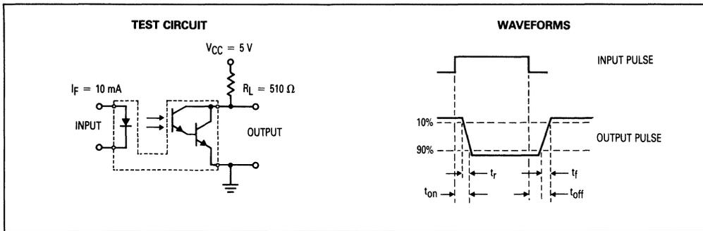
Figure 9. Switching Times
