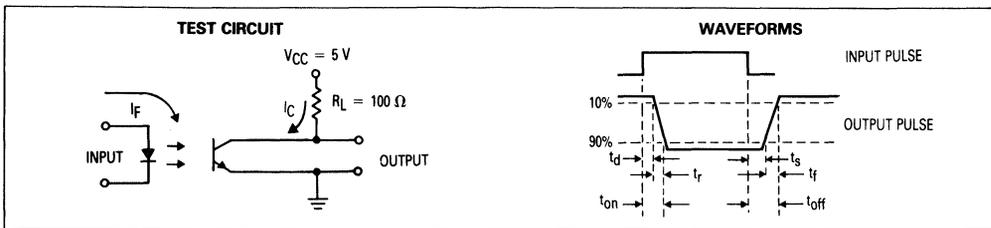
Figure 11. Switching Times
