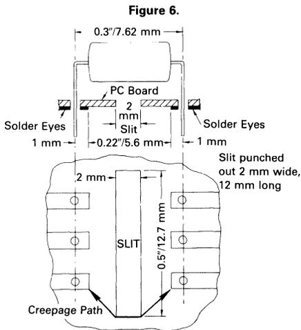
VDE equipment norms demanding longer creepage path than  $0.22"/5.6 \text{ mm}$  can be accomplished by a slit in the PC board between the coupler input and output solder eyes of 2 mm width.
