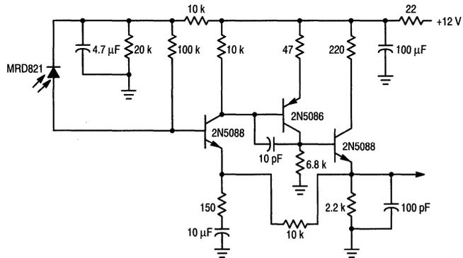
High-Performance Discrete Front-End Amplifier with Special Attention Paid to Noise for Range of up to 100 Meters
