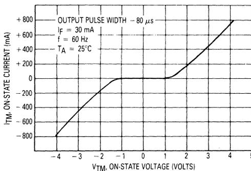
Figure 1. On-State Characteristics
