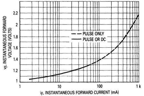
Figure 2. Forward Characteristics
