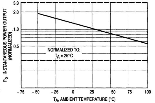
Figure 2. Instantaneous Power Output versus Ambient Temperature
