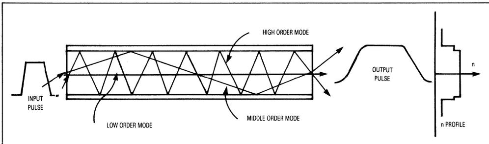
Figure 14. Propagation Along A Multimode Step Index Fiber
