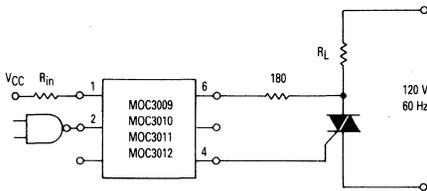
**Figure 8. Resistive Load**
