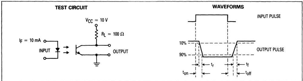
Figure 11. Switching Times
