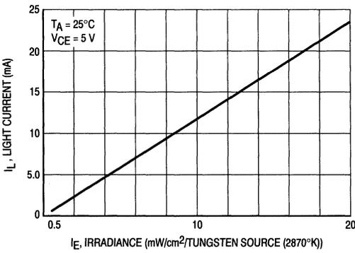
Figure 5. Transistor Collector Current versus Irradiance
