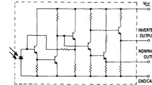
Figure 1. Equivalent Schematic
