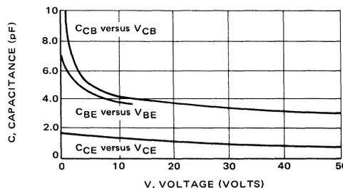
FIGURE 16 – Junction Capacitances versus Voltage for MRD300
