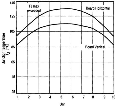
**Figure 14. Cluster T<sub>J</sub> Junction Temperature Distribution in a Cluster of 10 T<sub>A</sub> = 25°C, All Devices on with I = 1 Arms**
