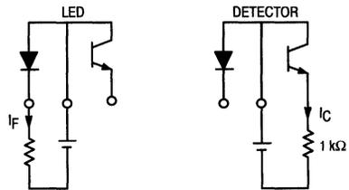
Figure 8. Test Circuit for Figures 6 and 7
