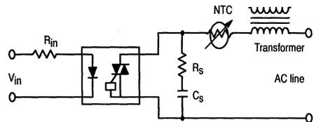
Figure 8. Thermistor Limits Excessive Inrush Current
