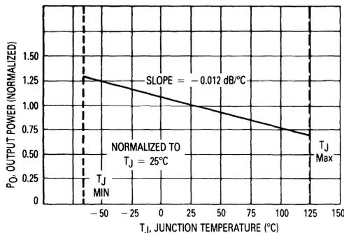
Figure 2. Power Output versus Junction Temperature
