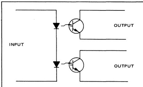
FIGURE 27 – DPST Relay Using MRD300s and LEDs
