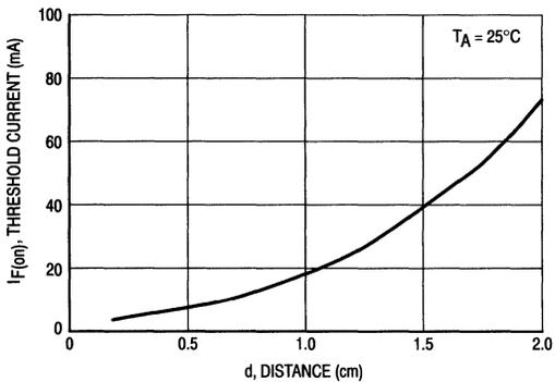
Figure 8. Threshold Current versus Lens to Lens Separation Distance at 25°C
