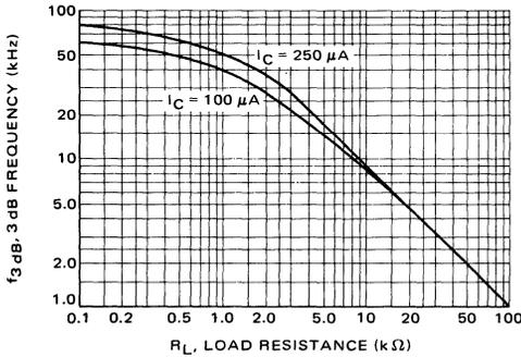
FIGURE 17 — 3 dB Frequency versus Load Resistance for MRD300
