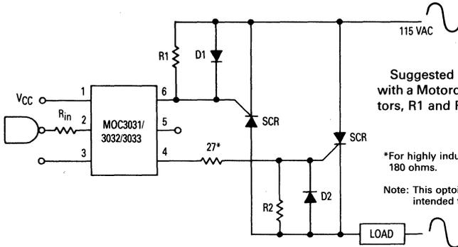
Suggested method of firing two, back-to-back SCR's, with a Motorola triac driver. Diodes can be 1N4001; resistors, R1 and R2, are optional 1 k ohm.
