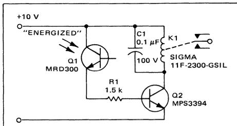
FIGURE 25 – Light-Operated Relay
