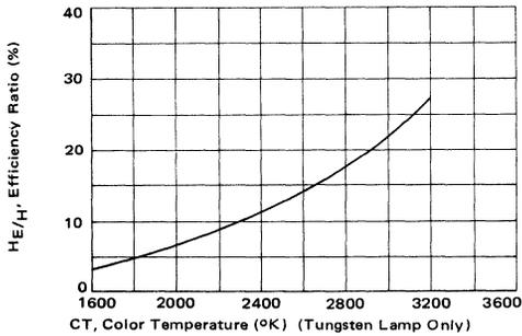
FIGURE 18 – MRD Irradiance Ratio versus Color Temperature
