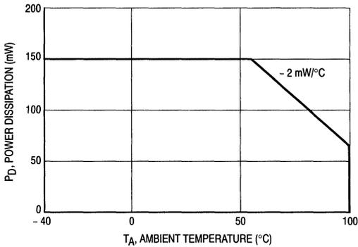
Figure 1. Power Dissipation
