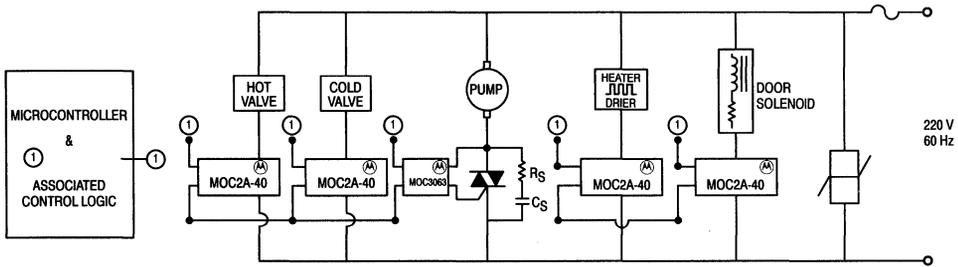
**Figure 2. Commercial Appliance Control (Dishwasher/Washing Machine/Dryer) Application**
