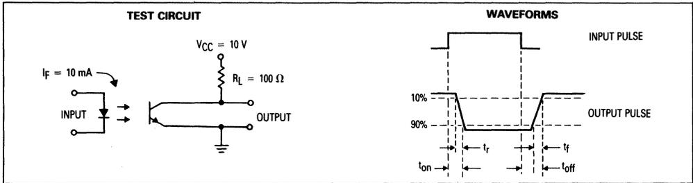
Figure 11. Switching Times
