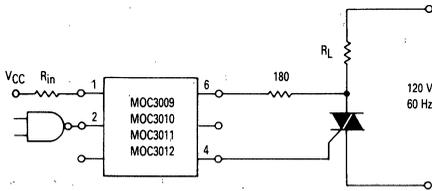
Figure 8. Resistive Load
