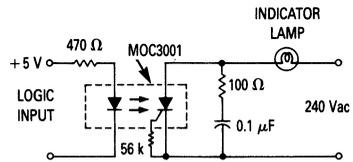
The high surge capability and non-reactive input characteristics of the MOC3001 allow it to directly couple, without buffers, T<sup>2</sup>L and DTL logic to indicator and alarm devices, without danger of introducing noise and logic glitches.
