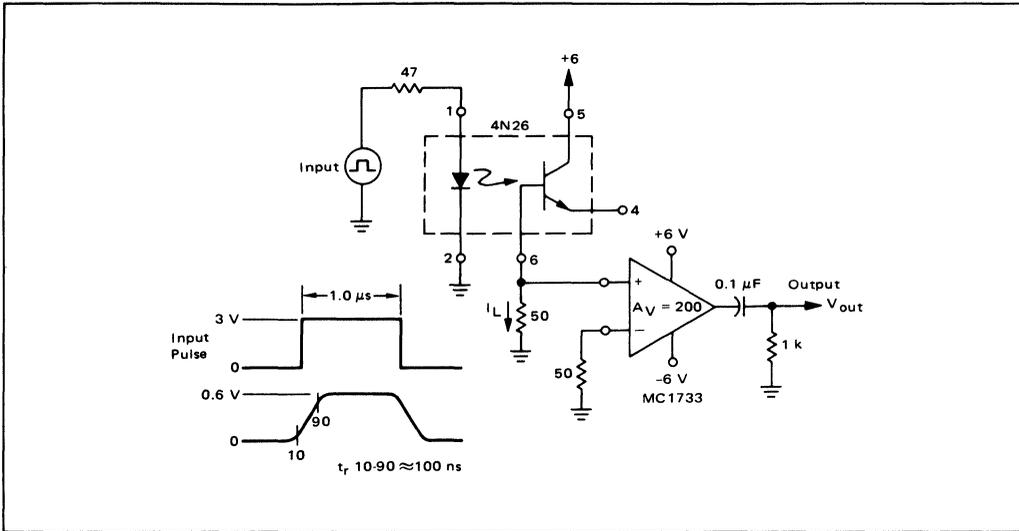
FIGURE 14 — Using the 4N26 as a Diode-Diode Coupler
