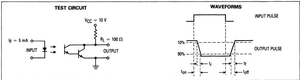
Figure 11. Switching Times
