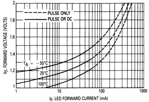
Figure 4. Forward Characteristics
