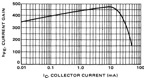
FIGURE 11 – DC Current Gain versus Collector Current
