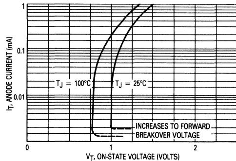
Figure 2. On-State Characteristics
