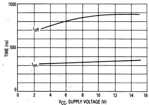
Figure 10. Total Switching Time versus Supply Voltage
