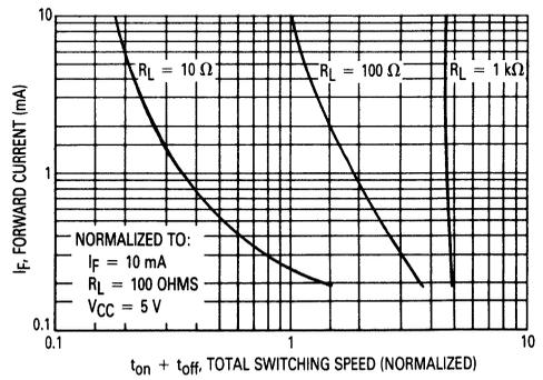
**Figure 6. Input Current versus Total Switching Speed**
