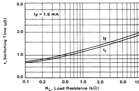
FIGURE 34 – Switching Times with Speed-up Circuit
