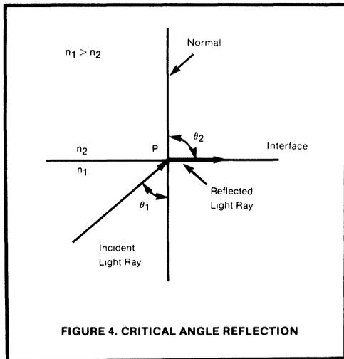
The angle,  $\theta_c$ , is known as the critical angle and defines the angle at which incident rays will not pass through the interface. For angles greater than  $\theta_c$ , 100 percent of the light rays are reflected (as shown in Figure 5), and the angle of incidence equals the angle of reflection.
