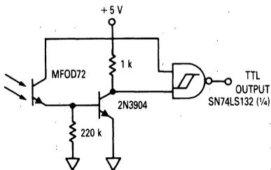
Figure 7. 5 kHz Transistor Receiver
