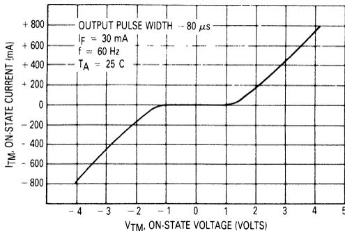
Figure 1. On-State Characteristics
