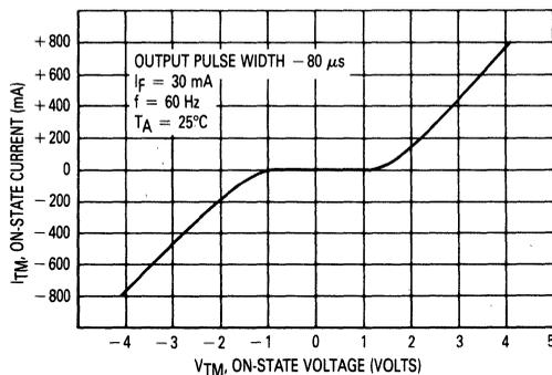
Figure 1. On-State Characteristics
