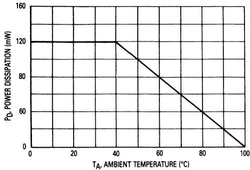
Figure 1. Power Dissipation
