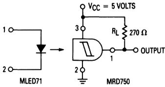
**Figure 9. Test Circuit for Threshold Current Measurements**
