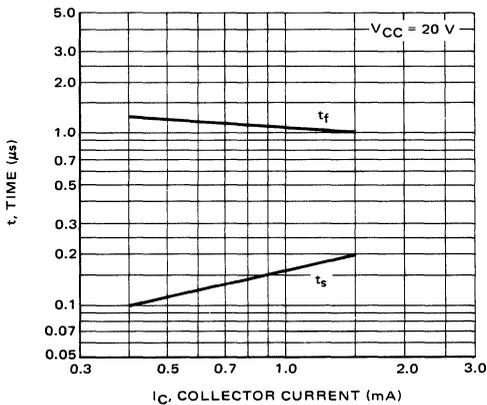
FIGURE 22 – Switching Storage and Fall Times for MRD300
