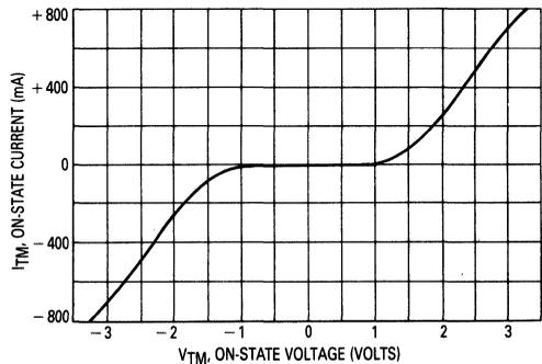
Figure 2. On-State Characteristics
