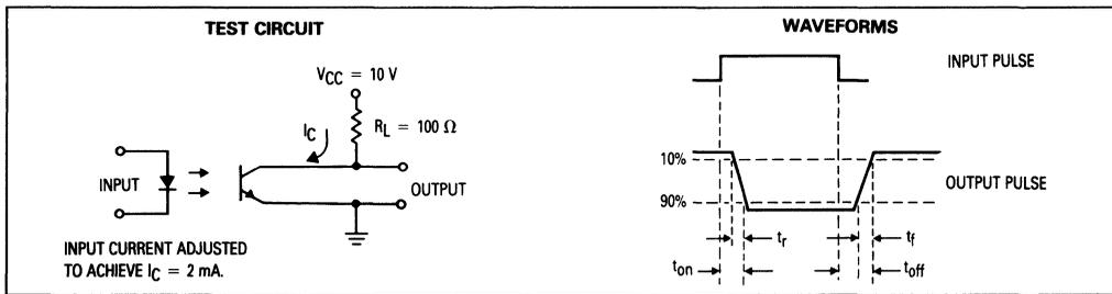
Figure 11. Switching Times
