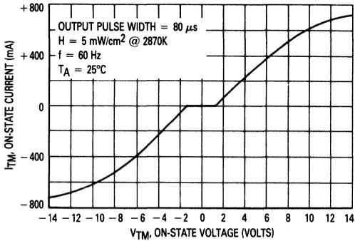
Figure 2. On-State Characteristics
