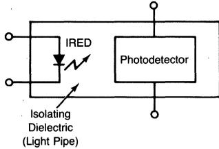
Figure 4. Block Diagram of Optoisolator
