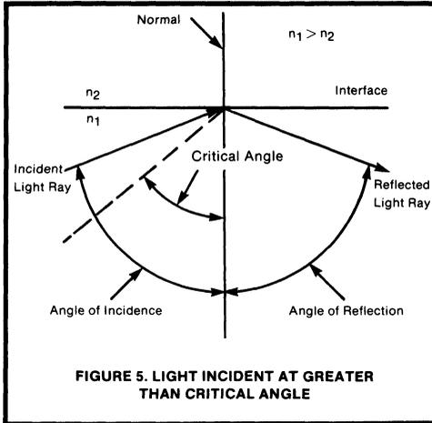
FIGURE 5. LIGHT INCIDENT AT GREATER THAN CRITICAL ANGLE
