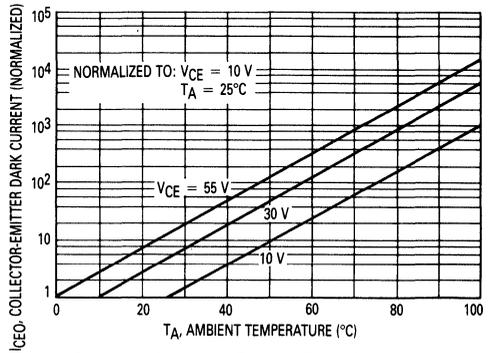
Figure 6. Collector-Emitter Dark Current versus Ambient Temperature
