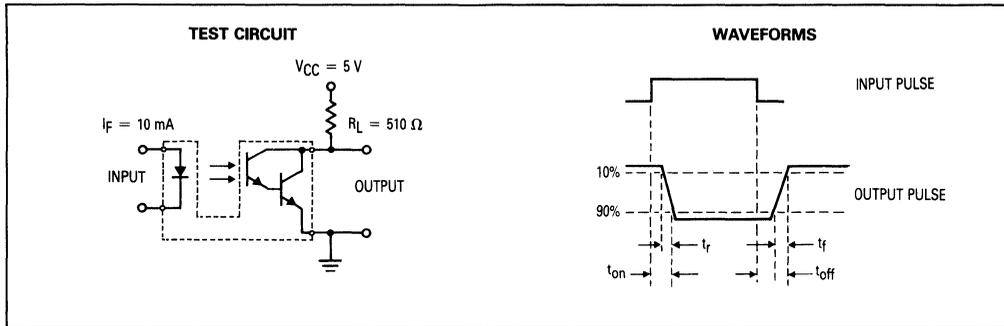
Figure 9. Switching Times
