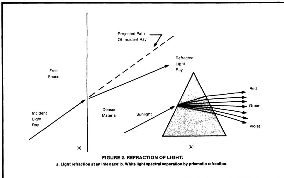
stated, the light ray is bent at the interface. This is shown in Figure 2a. In fact, the reduction of the speed of light is different for different wavelengths; and, therefore, the degree of bending is different for each wavelength. It is this variation in effect for different wavelengths that results in rainbows. Water droplets in the air act like small prisms (Figure 2b) to split white sunlight into the visible spectrum of colors.
