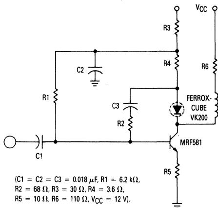
**Figure 11. LED Drive Circuit to 100 MHz**
