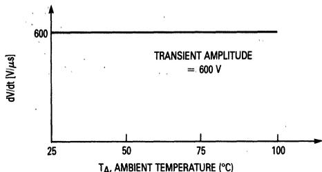
Figure 5. Static dV/dt versus Temperature
