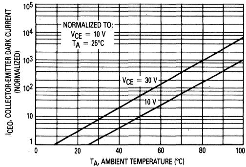
Figure 6. Collector-Emitter Dark Current versus Ambient Temperature
