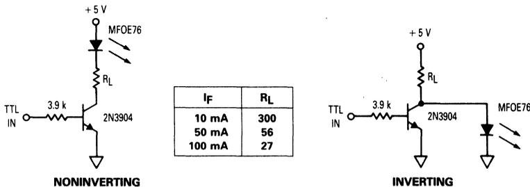
Figure 6. TTL Transmitters
