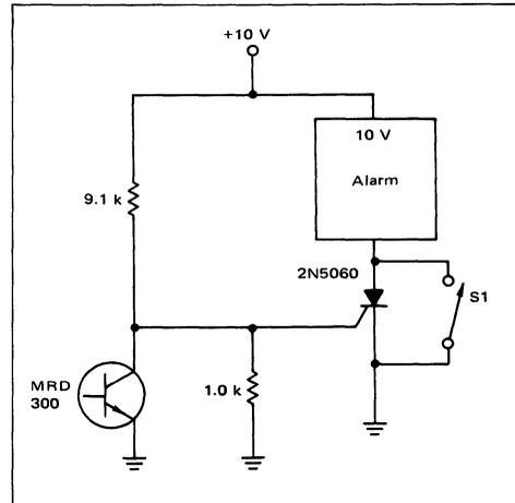
FIGURE 28 – Light Operated SCR Alarm Using Sensitive-Gate SCR
