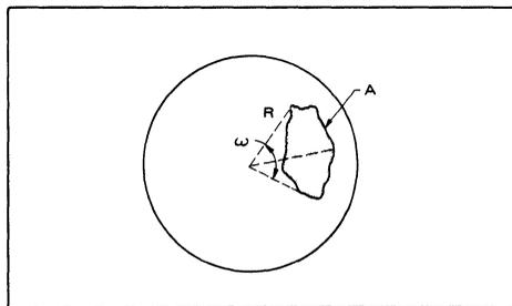
FIGURE 1-3 - Solid Angle,  $\omega$
