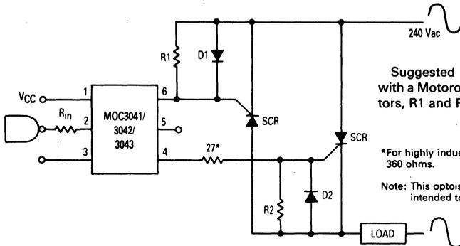
Suggested method of firing two, back-to-back SCR's, with a Motorola triac driver. Diodes can be 1N4001; resistors, R1 and R2, are optional 330 ohms.
