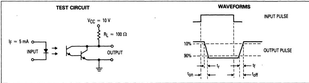
Figure 11. Switching Times
