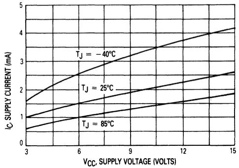
Figure 5. Supply Current versus Supply Voltage — Output High
