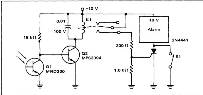
FIGURE 27 – Light-Relay Operated SCR Alarm Circuit
