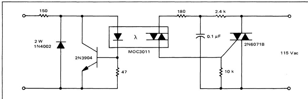
FIGURE 10 — Solid-State Relay
