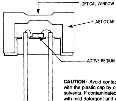
Figure 4. Package Cross Section
