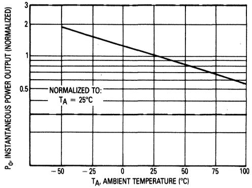
Figure 2. Instantaneous Power Output versus Ambient Temperature
