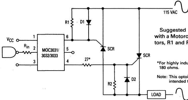
Suggested method of firing two, back-to-back SCR's, with a Motorola triac driver. Diodes can be 1N4001; resistors, R1 and R2, are optional 1 k ohm.
