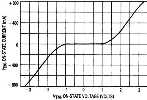
Figure 1. On-State Characteristics
