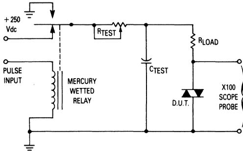
1. The mercury wetted relay provides a high speed repeated pulse to the D.U.T.
