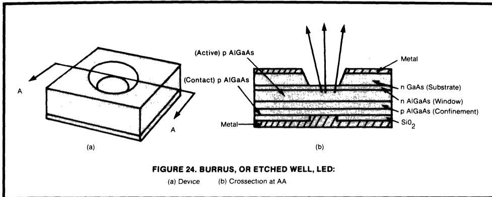
etched wells are aligned over the active areas defined by the  $\text{SiO}_2$  openings on the underside of the wafer and remove the heavily-photon-absorptive substrate down to the window layer. As an indication of the delicacy of this operation, it requires double-sided alignment on a wafer about 0.1 mm thick with a final thickness in the opening of about 0.025 mm.
