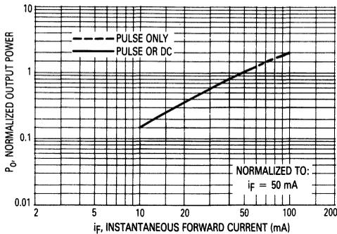
Figure 2. Normalized Output Power versus Forward Current
