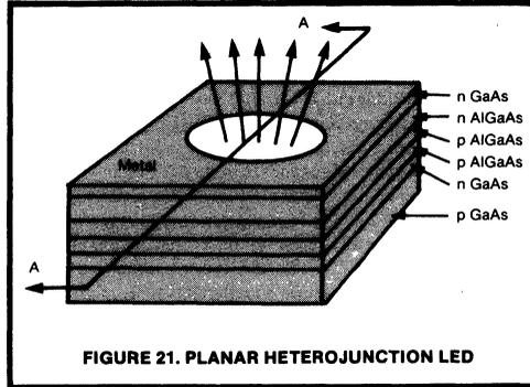
The emission pattern is lambertian, similar to the grown junction LED above.
