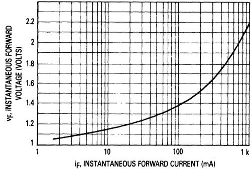
Figure 2. Forward Characteristics
