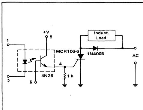
FIGURE 11 – Coupler-Driven SCR
