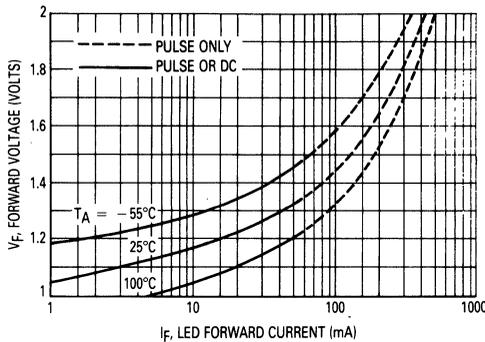
Figure 1. LED Forward Voltage versus Forward Current
