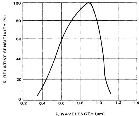
FIGURE 4 – Spectral Response of Silicon Photodiode
