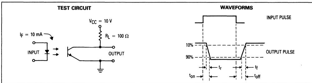
Figure 11. Switching Times
