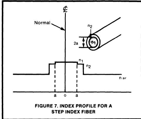
FIGURE 7. INDEX PROFILE FOR A STEP INDEX FIBER
