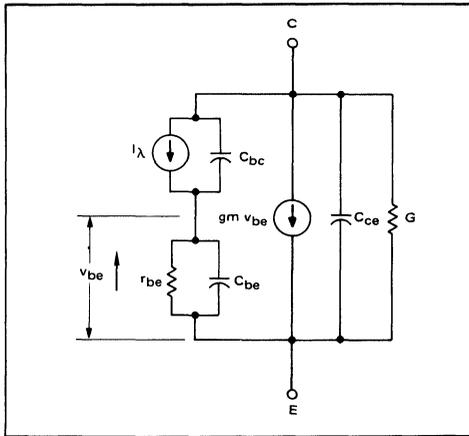
FIGURE 3 — Floating Base Approximate Model of Phototransistor
