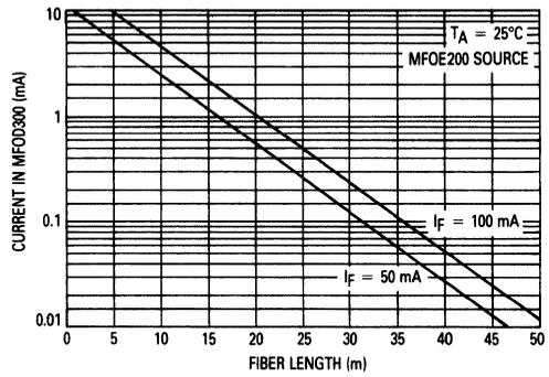
Figure 2. Coupled System Performance versus Fiber Length
