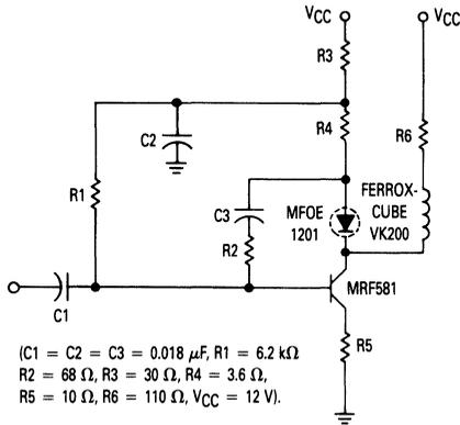
Figure 11. LED Drive Circuit to 100 MHz
