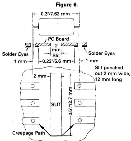
VDE equipment norms demanding longer creepage path than  $0.22"/5.6 \text{ mm}$  can be accomplished by a slit in the PC board between the coupler input and output solder eyes of 2 mm width.
