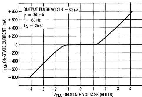
Figure 1. On-State Characteristics
