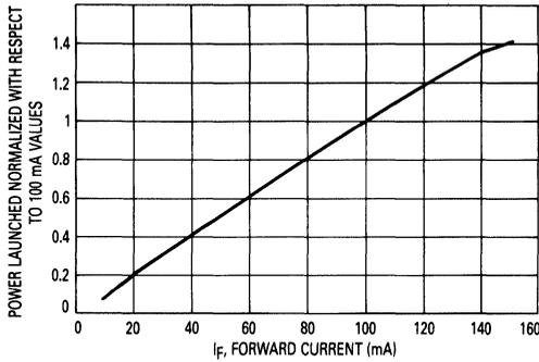
**Figure 1. Normalized Power Launched versus Forward Current**
