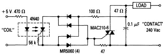
Use of the 4N40 for high sensitivity, 7500 V isolation capability, provides this highly reliable solid state relay design. This design is compatible with 74, 74S and 74H series T<sup>2</sup>L logic systems inputs and 240 Vac loads up to 10 A.
