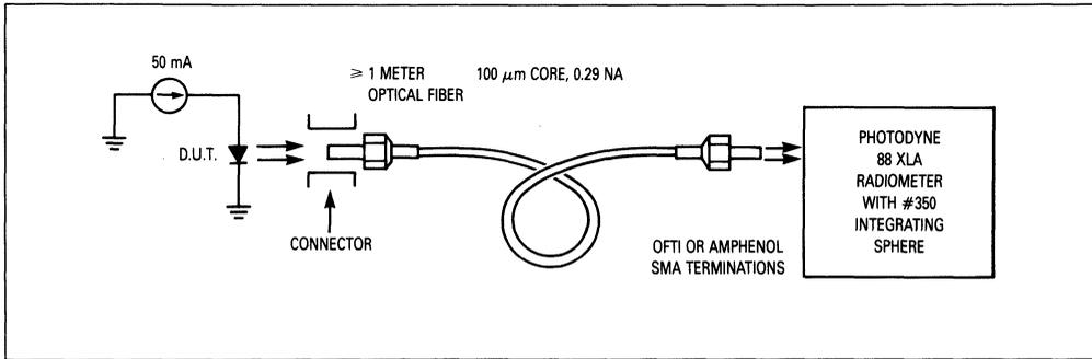
Figure 6. Coupling Efficiency
