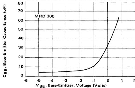
FIGURE 30 – MRD300 Base-Emitter Junction Capacitance versus Voltage
