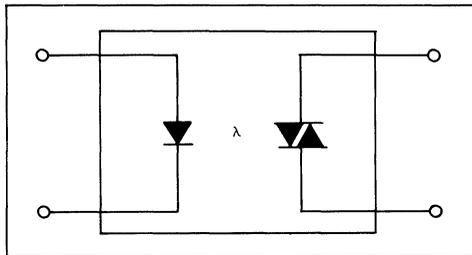
FIGURE 2 – Schematic Representation of MOC3011 and MOC3010
