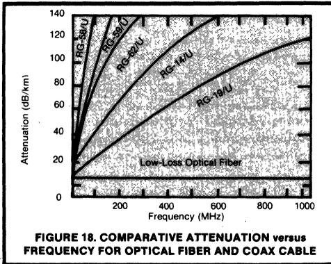
FIGURE 18. COMPARATIVE ATTENUATION VERSUS FREQUENCY FOR OPTICAL FIBER AND COAX CABLE
