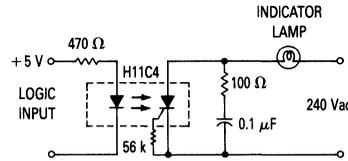
The high surge capability and non-reactive input characteristics of the H11C allow it to directly couple, without buffers, T<sup>2</sup>L and DTL logic to indicator and alarm devices, without danger of introducing noise and logic glitches.
