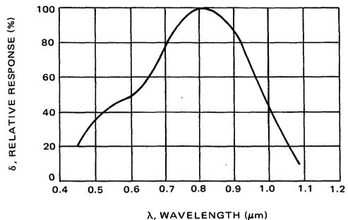
FIGURE 9 – Constant Energy Spectral Response for MRD300
