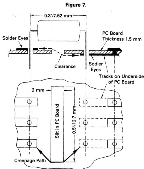
If a clearance of  $0.23"/6 \text{ mm}$  and a creepage path of minimum 8 mm is required, this is a possible solution.
