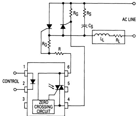
Figure 15. A Circuit Using Inverse Parallel SCRs
