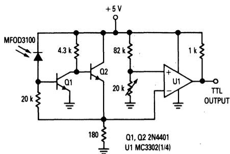
**Figure 14. 1 MHz Pin Receiver**
