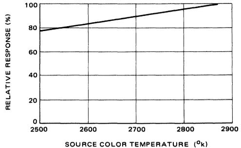
FIGURE 12 – Relative Response of MRD300 versus Color Temperature
