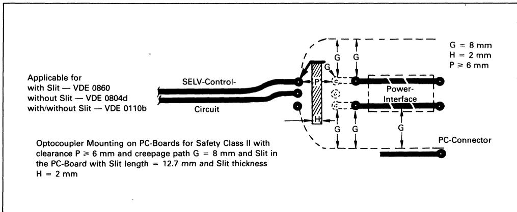
**COUPLER MOUNTING ON A CIRCUIT BOARD**
