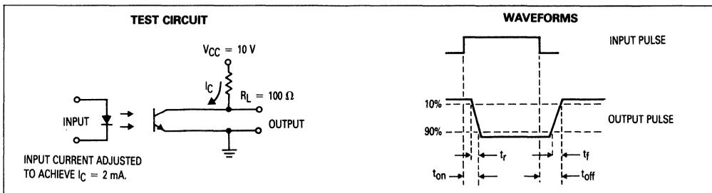
Figure 11. Switching Times
