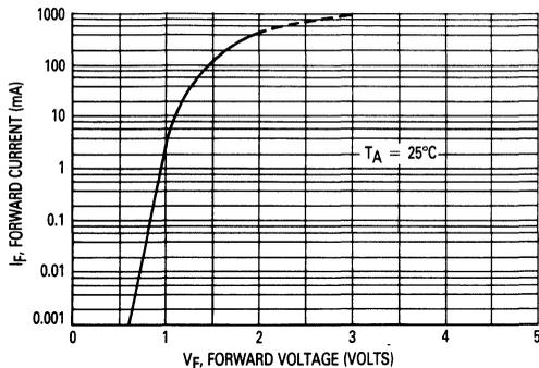
Figure 1. Forward Current versus LED Forward Voltage
