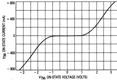
Figure 2. On-State Characteristics
