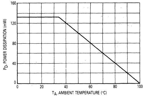
**Figure 8. Power Dissipation**
