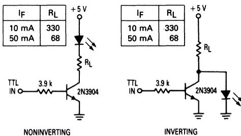
**Figure 13. TTL Transmitters**
