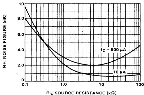
FIGURE 18 — MRD300 Noise Figure versus Source Resistance
