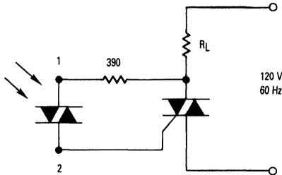
Figure 7. Resistive Load
