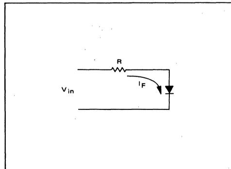
FIGURE 2 - Simple Drive Circuit For An LED
