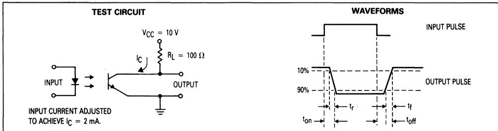
Figure 10. Switching Times
