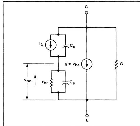
FIGURE 8 – Floating Base Approximate Model of Phototransistor
