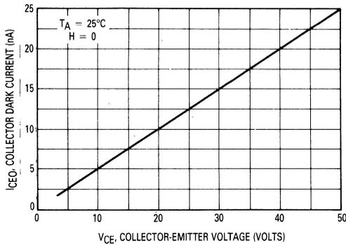
Figure 5. Dark Current versus Voltage
