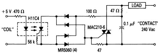
Use of the H11C4 for high sensitivity, 7500 V isolation capability, provides this highly reliable solid state relay design. This design is compatible with 74, 74S and 74H series T<sup>2</sup>L logic systems inputs and 240 Vac loads up to 10 A.
