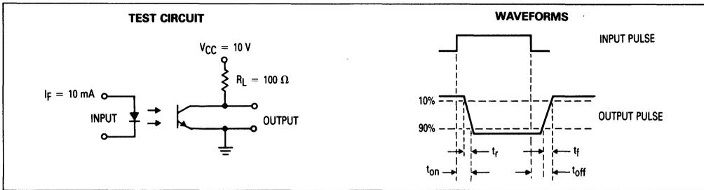
Figure 11. Switching Times
