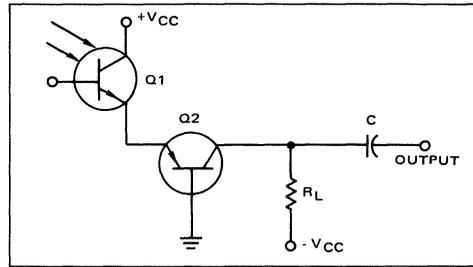
FIGURE 32 – Improved Speed Configuration for Phototransistor
