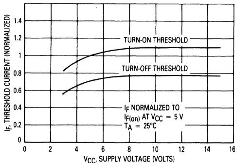
Figure 1. Normalized Threshold Current versus Supply Voltage
