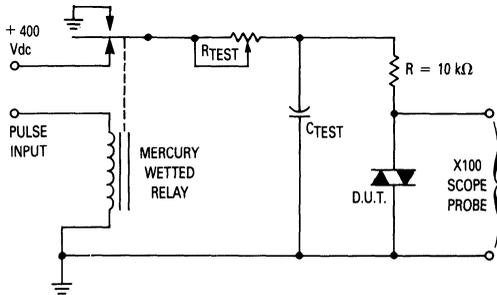
1. The mercury wetted relay provides a high speed repeated pulse to the D.U.T.
