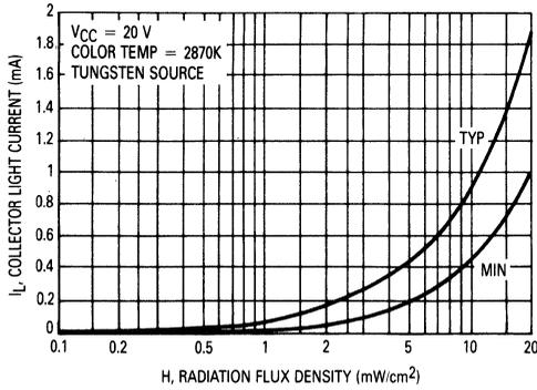
Figure 1. Collector-Emitter Sensitivity
