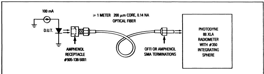
Figure 4. Launched Power (P<sub>L</sub>) Test Set
