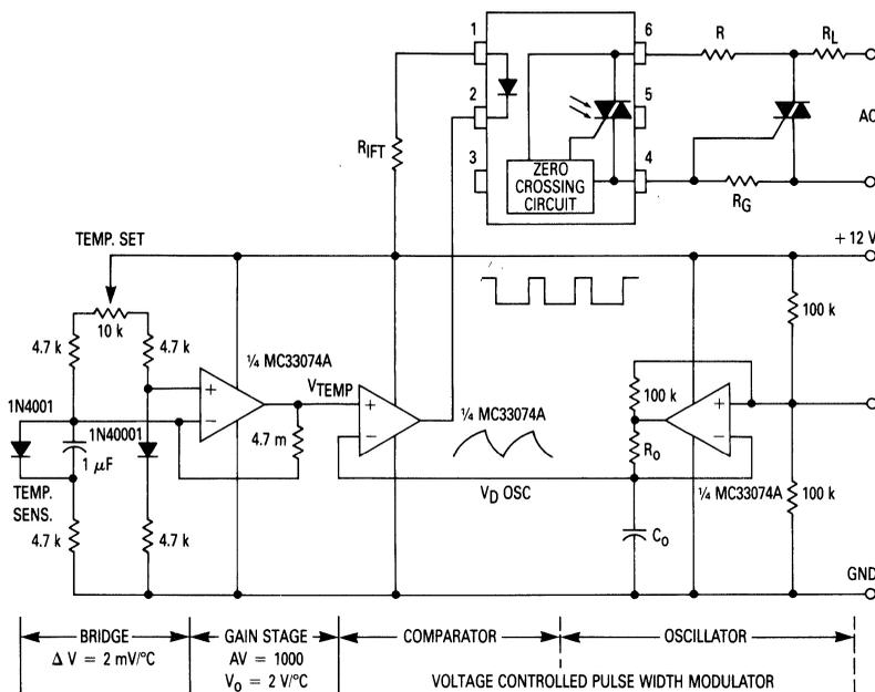
Figure 17. Proportional Zero Voltage Switching Temperature Controller
