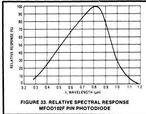
FIGURE 33. RELATIVE SPECTRAL RESPONSE MFOD102F PIN PHOTODIODE
