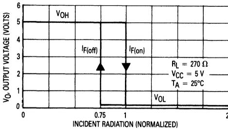
Figure 2. Transfer Characteristics
