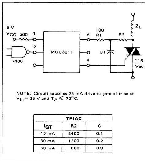
FIGURE 4 – Logic to Inductive Load Interface
