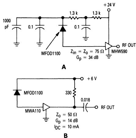
**Figure 12. Receiver Circuits**
