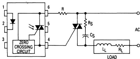
Figure 13. Triac Driving Circuit — with Snubber
