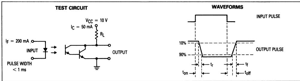
Figure 11. Switching Times
