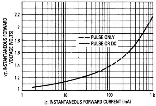
Figure 2. Forward Characteristics
