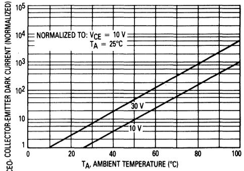
**Figure 6. Collector-Emitter Dark Current versus Ambient Temperature**
