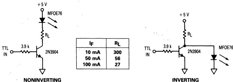
Figure 6. TTL Transmitters
