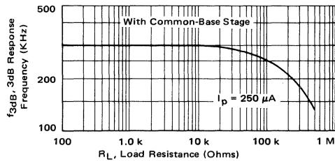
FIGURE 33 – 3dB Frequency Response for Speed-up Circuit
