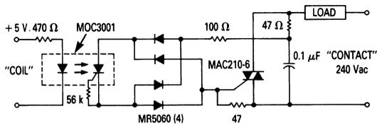
Use of the MOC3001 for high sensitivity, 7500 V isolation capability, provides this highly reliable solid state relay design. This design is compatible with 74, 74S and 74H series T<sup>2</sup>L logic systems inputs and 240 Vac loads up to 10 A.
