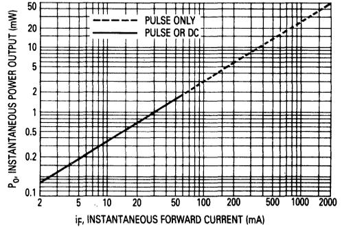
Figure 2. Instantaneous Power Output versus Forward Current
