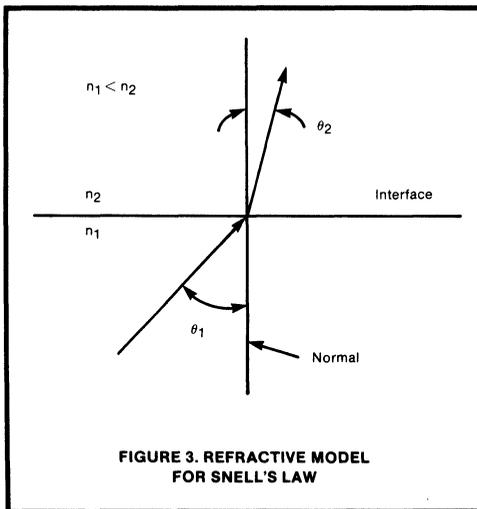
The angle of refraction,  $\theta_2$ , can be determined:
