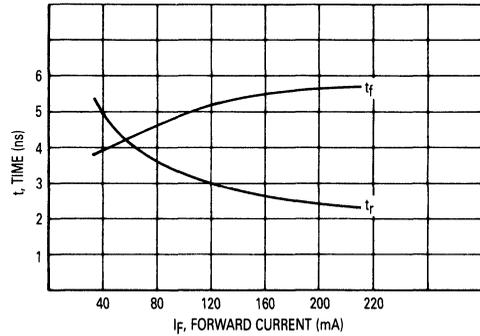
Figure 12. Rise and Fall Time versus Forward Current
