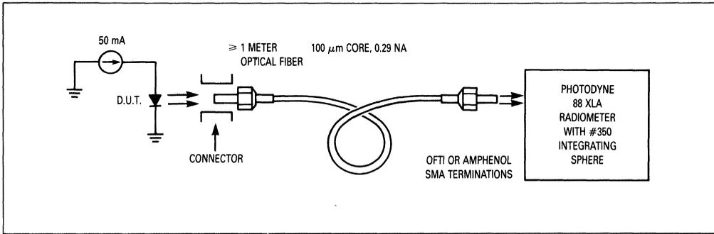
Figure 6. Coupling Efficiency
