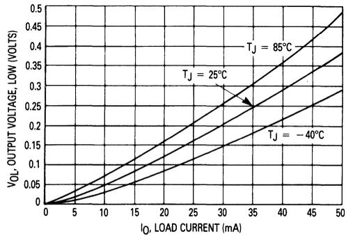
Figure 3. Output Voltage, Low versus Load Current
