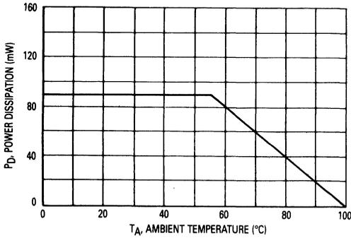
Figure 1. Power Dissipation
