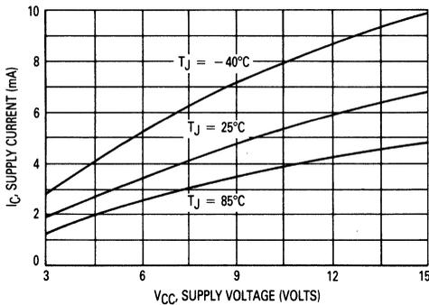
Figure 5. Supply Current versus Supply Voltage — Output Low
