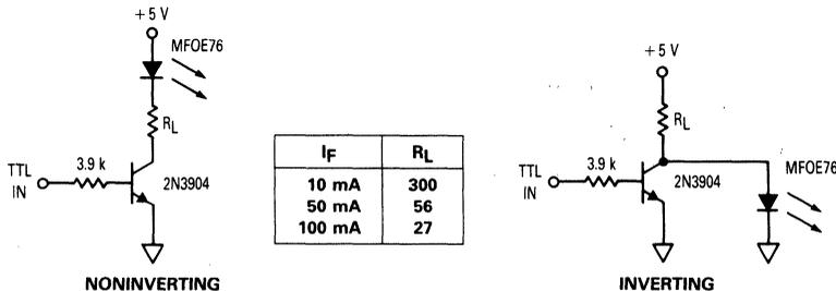
Figure 6. TTL Transmitters
