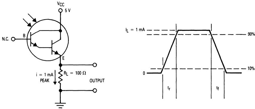
Figure 8. Pulse Response Test Circuit and Waveform
