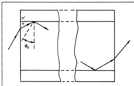
FIGURE 16 – Refraction in an Optical Fiber
