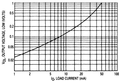
Figure 5. Output Voltage, Low versus Load Current
