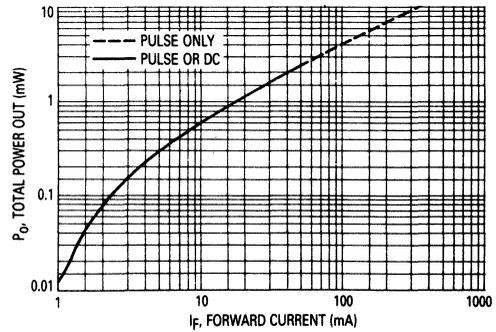
Figure 6. Instantaneous Power Output versus Forward Current
