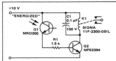
FIGURE 25 — Light-Operated Relay
