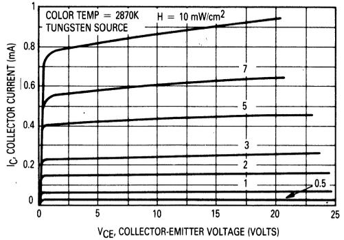
Figure 2. Collector-Emitter Characteristics
