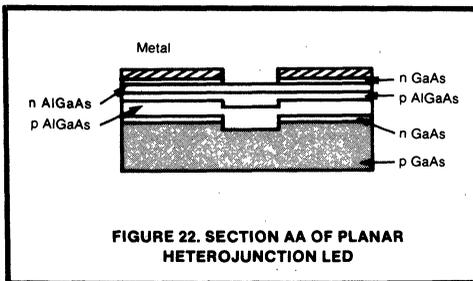
FIGURE 22. SECTION AA OF PLANAR HETEROJUNCTION LED
