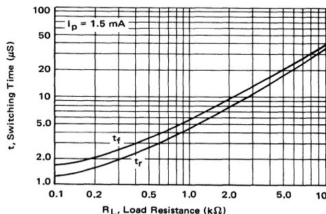
FIGURE 31 – MRD300 Switching Times versus Load Resistance
