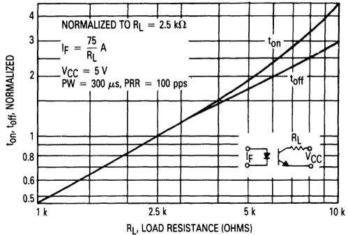
Figure 2. Typical  $t_{on}$ ,  $t_{off}$  versus Load Resistance
