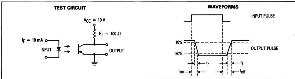
Figure 11. Switching Times
