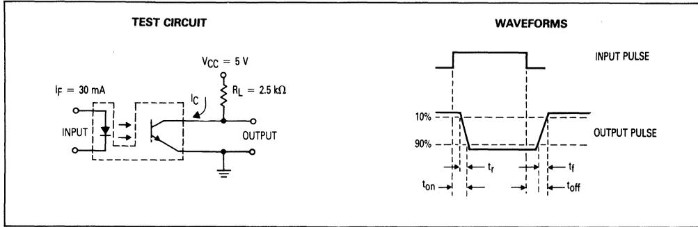
Figure 9. Switching Times
