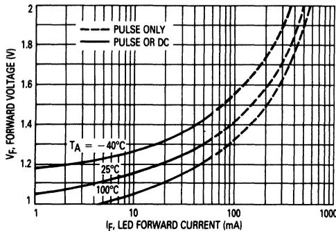
Figure 1. LED Forward Voltage versus Forward Current
