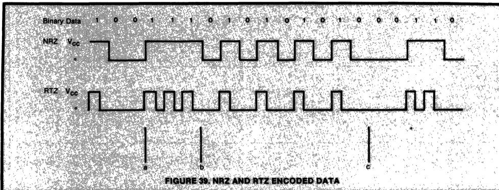
or "0's" for RTZ will prevent the receiver from recovering any clock signal.
