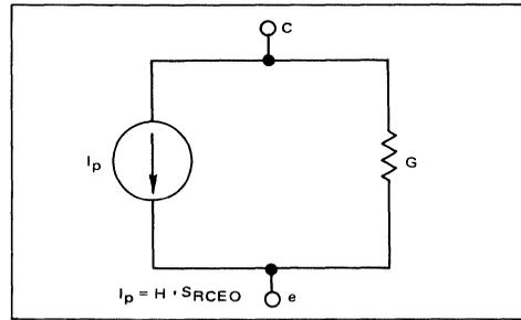
FIGURE 6 – Low-Frequency and Steady-State Model for Floating-Base Phototransistor
