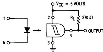
Figure 6. Test Circuit for Threshold Current Measurements
