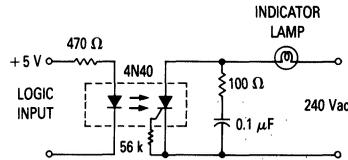
The high surge capability and non-reactive input characteristics of the 4N40 allow it to directly couple, without buffers, T<sup>2</sup>L and DTL logic to indicator and alarm devices, without danger of introducing noise and logic glitches.
