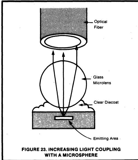
FIGURE 23. INCREASING LIGHT COUPLING WITH A MICROSPHERE
