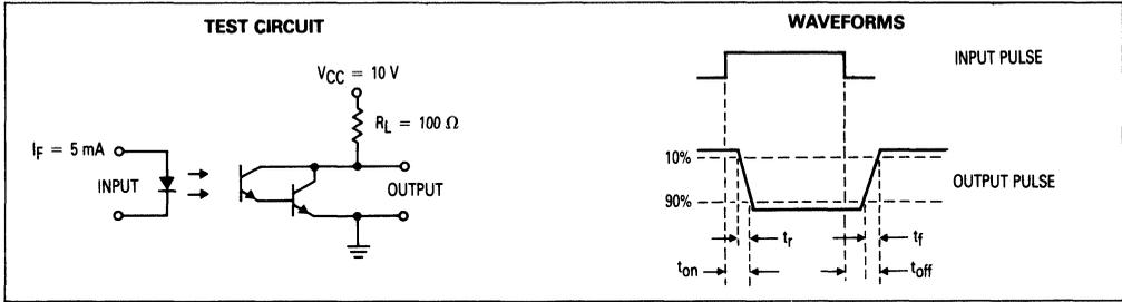
Figure 9. Switching Times
