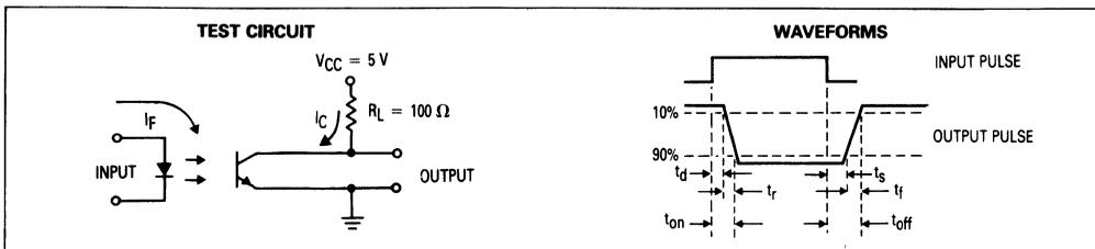
Figure 11. Switching Times
