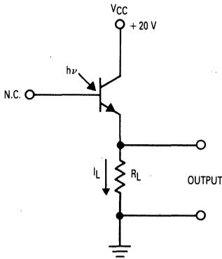
Figure 9. Pulse Response Test Circuit and Waveform
