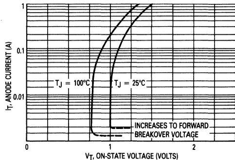
Figure 2. On-State Characteristics
