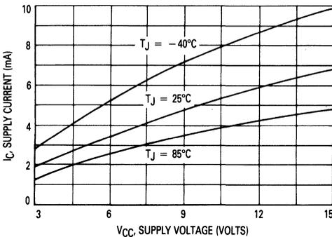
Figure 4. Supply Current versus Supply Voltage — Output Low
