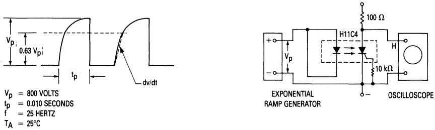
Figure 8. Coupled dv/dt — Test Circuit
