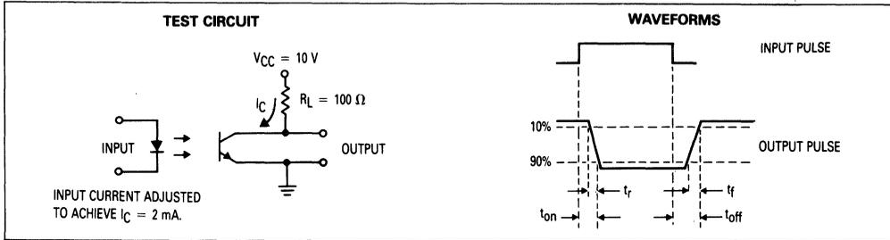
Figure 11. Switching Times
