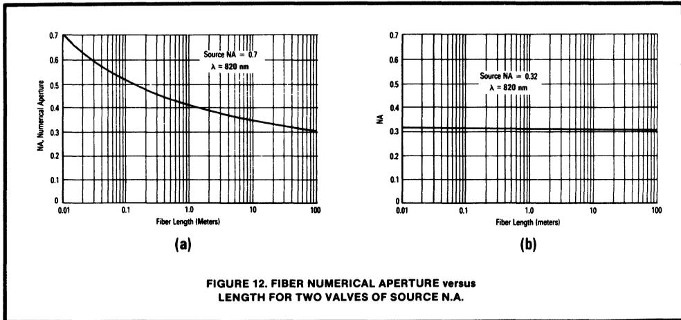
FIGURE 12. FIBER NUMERICAL APERTURE versus LENGTH FOR TWO VALUES OF SOURCE N.A.
