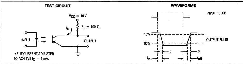
Figure 11. Switching Times
