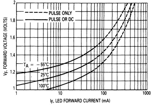
Figure 4. Forward Characteristics
