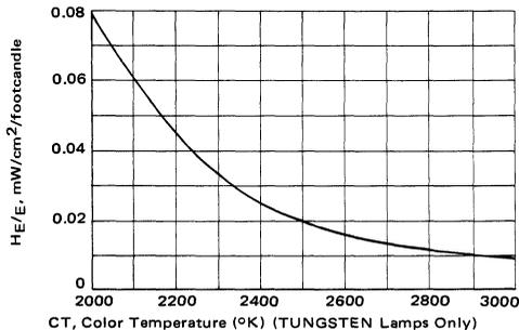
FIGURE 19 – MRD Irradiance/Illuminance Ratio versus Color Temperature
