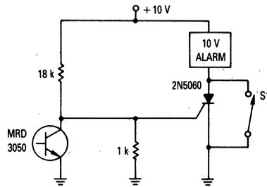
Figure 7. Light Operated SCR Alarm Using Sensitive-Gate SCR
