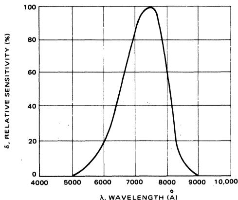
FIGURE 2 - Spectral Response of Cadmium Selenide
