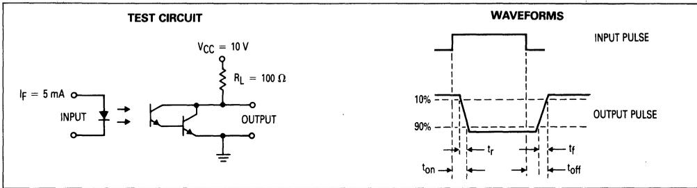
Figure 9. Switching Times
