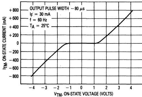
Figure 1. On-State Characteristics
