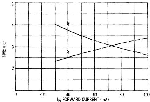
Figure 7. Rise Time ( $t_r$ ) and Fall Time ( $t_f$ ) versus Forward Current ( $I_f$ )
