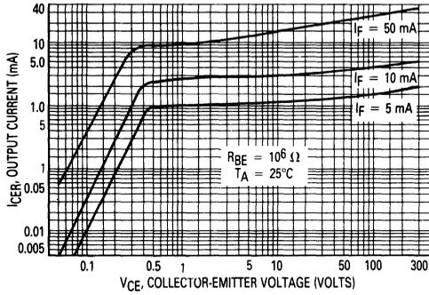
Figure 3. Output Characteristics
