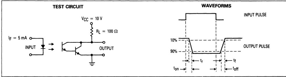
Figure 9. Switching Times
