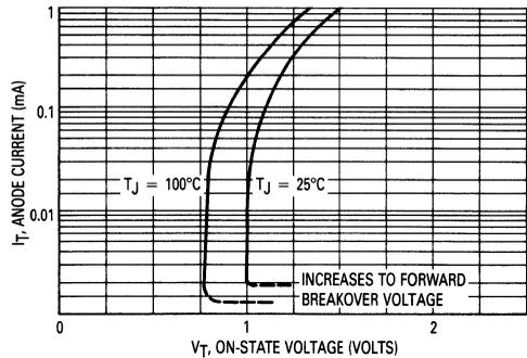
Figure 2. On-State Characteristics
