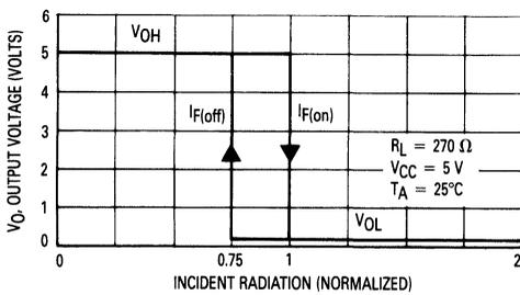
Figure 2. Transfer Characteristics
