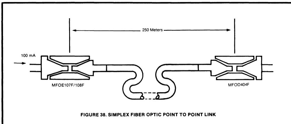
$$P_R = 10 \log \frac{0.00043 \text{ mW}}{1.0 \text{ mW}} = -34 \text{ dBm} \quad (23)$$
