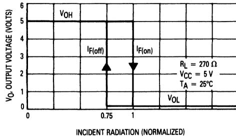
Figure 1. Transfer Characteristics
