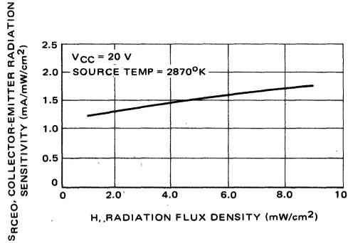
FIGURE 14 – Open Base Sensitivity versus Radiation for MRD300
