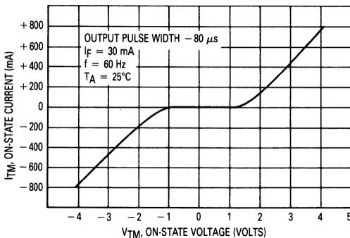
Figure 1. On-State Characteristics
