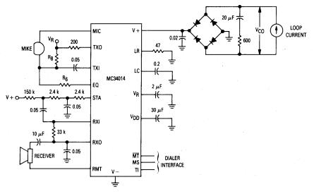
For Primo EM-95A microphone Rg = 500  $\Omega$ , R<sub>6</sub> = 10 k For Hosiden KUC2123 microphone Rg = 1.5 k, R<sub>6</sub> = 30 k
