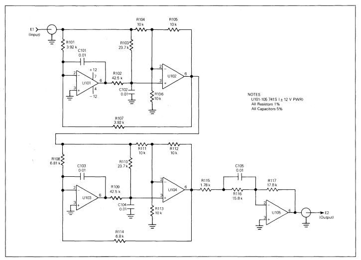
FIGURE 6 - 2400 BPS Modem System Equalizer Sub-Board
