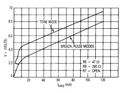
through the VR series pass transistor to V+, modulating the loop current. The voltage signal at V+ is out of phase with the signal at TXI.
