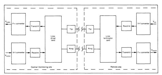
1. The maximum range of an RS-232 or RS-422 communications link can be extended to over 4 miles of uncompensated 24 AWG wires by a line-driver card based on a single-chip subscriber-loop interface circuit.
