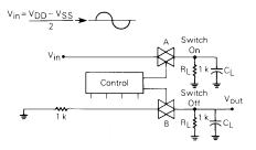
FIGURE 5 - CROSSTALK CONTROL TO OUTPUT
