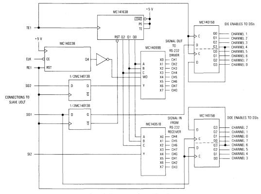
Figure 8. Slave Sequencing and Signalling
