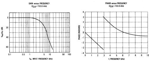
NOTES: 1. Break frequency is equal to the clock frequency + 64.2. Figure 1 illustrates Filter B performance.Filter A would be 18 dB higher.
