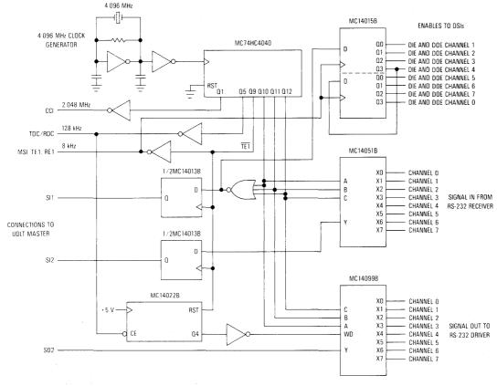
Figure 7. Master Sequencing and Signalling
