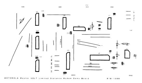
Figure 10. Photostat of LDM Demonstration Board - Front
