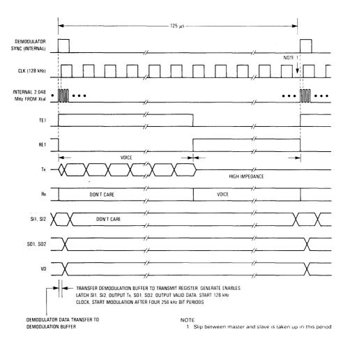
Figure 13. Slave DLT Timing
