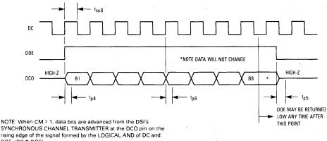
SYNCHRONOUS CHANNEL TRANSMITTER at the DCO pin on the rising edge of the signal formed by the LOGICAL AND of DC and DOE (DC
