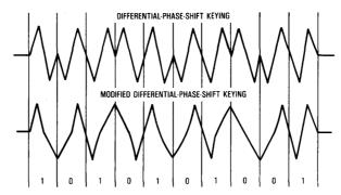
Figure 12. Modified Differential Phase Shift Keying
