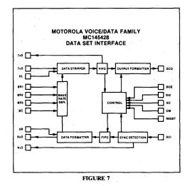
The MC145428 was designed in Si-gate CMOS technology and utilized in a 20 pin package. This IC will lend itself to a variety of data communication applications.
