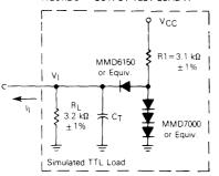
$C_{T}=20\ pF=total parasitic capacitance, which includes$ probe, wiring, and load capacitances.
