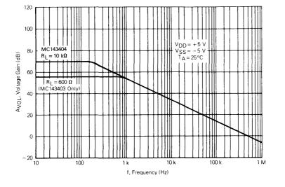
FIGURE 1 - TYPICAL OPEN LOOP FREQUENCY RESPONSE
