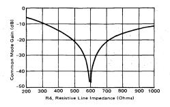
FIGURE 6 - Common Mode Gain versus Line Impedance
