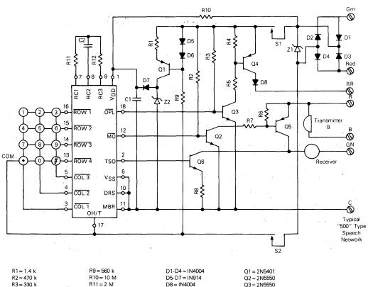
R3 = 330 kD8 = IN4004 Q3 = 2N5550 R12 = 220 k R4 = 100 kQ4 = 2N5401 R5 = 3 kZ1 = 120 V, IW Q5 = 2N5401  $C1 = 68 \ \mu F$  low leakage R6=100 k Z2=5 V, 500 mW Q6 = 2N5550 R7 = 3 k C2 = 390 pFR8=20 k
