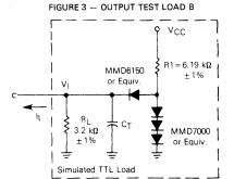
$C_T = 20 \text{ pF} = \text{total parasitic capacitance, which includes}$ probe, wiring, and load capacitances.
