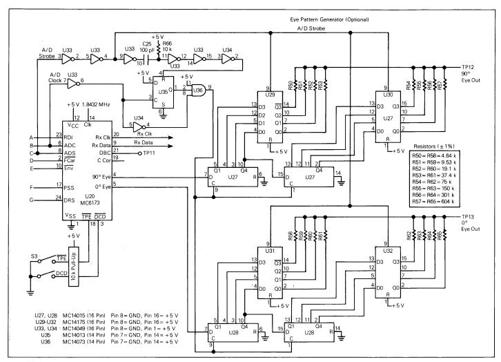
FIGURE 5 - 2400 BPS DPSK Demodulator System (2 of 2)
