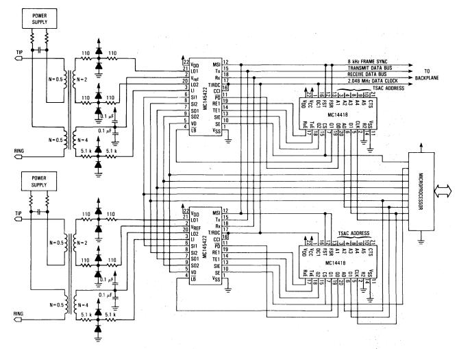
Figure 15. Typical Multichannel Digital Line Card
