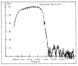
The switched-capacitor low-pass filter limits both input and output frequencies to about 3.7 kHz, as reflected by the system frequency response curve. Input frequencies are limited to prevent aliasing; filtering the output smooths it out.
