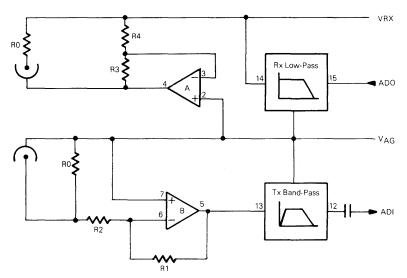
FIGURE 13 - TYPICAL 4-WIRE PORT INTERFACE USING MC14413
