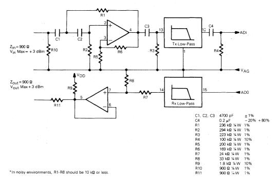
FIGURE 11 -- FILTER SCHEMATIC FOR MC14414-1, -2 WITH 60 Hz REJECTION AND 900 TERMINATION
