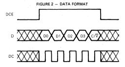
When  $C/\overline{V}$  is "1", D0-D3 are loaded into the configuration register. The four configuration register bits then address a ROM which has outputs to control the analog subsystem elements, enable the appropriate volume register, select the appropriate volume register for the speaker/ringer volume control, and provide the SAE output.
