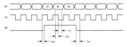
NOTE: When CM = 0, data bits are read into the DSI's SYNCHRONOUS CHANNEL RECEIVER at the DCI pin on the falling edge of the signal formed by the LOGICAL NAND of DC and DIE.
