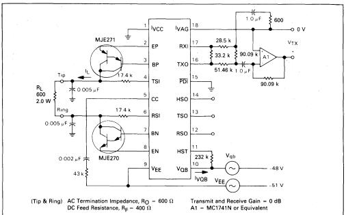
FIGURE 3 --- SUPPLY NOISE REJECTION TEST CIRCUIT
