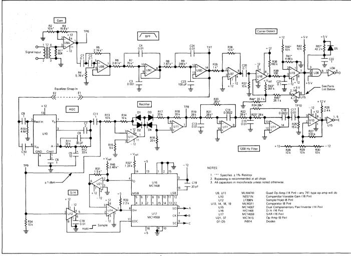
FIGURE 5 - 2400 BPS DPSK Demodulator (1 of 2)
