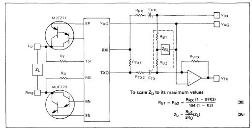
When the 2-wire port has a parallel R and C load, then (see Figure 12):
