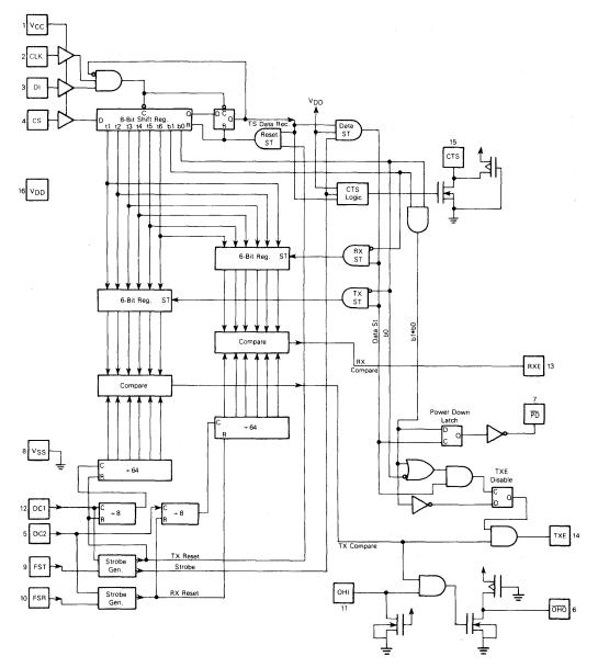
The MC14416 and MC14418 TSACs are microprocessor peripherals intended to be used to control and supervise per channel codec subscriber channel units. The TSACs consist of three basic functions.
