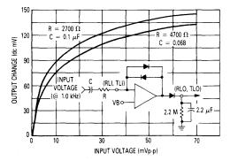
FIGURE 7 — LOG AMP TRANSFER CHARACTERISTICS
