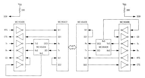
Figure 1. Limited Distance Modem Block Diagram
