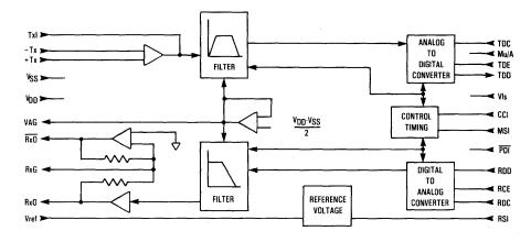
Figure 1. Block Diagram of the Mono-circuits
