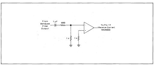
FIGURE 11 - Limiter Schematic
