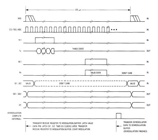
Figure 12. Master DLT Timing
