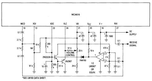
Figure 1. Receive-Idle Circuit
