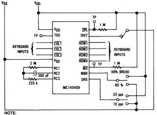
This circuit demonstrates operation of the device. Outputs can be observed at testpoints.
