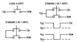
Figure 1. Keyboard Configurations
