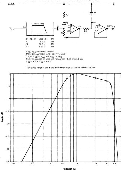
FIGURE 17 - TELEPHONY C-MESSAGE FILTER USING MC14414-1, -2 FILTER
