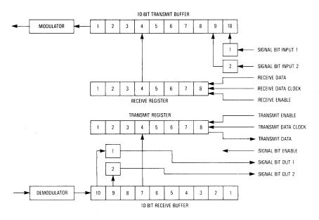
Figure 3. UDLT Receive and Transmit Registers
