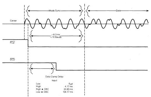
FIGURE 4 -- DEMODULATOR SYNC TIMING DIAGRAM
