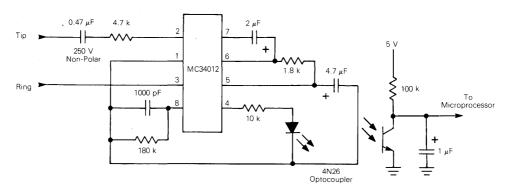
FIGURE 1 - Ring Detector Schematic
