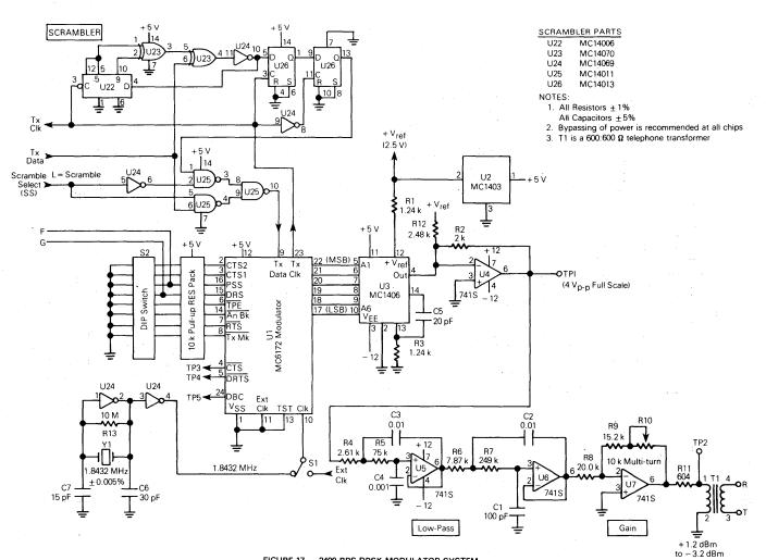
FIGURE 17 - 2400 BPS DPSK MODULATOR SYSTEM
