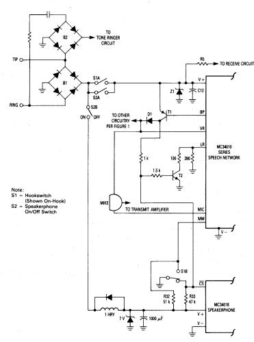
Figure 6. Microphone Muting - MC34010 Series
