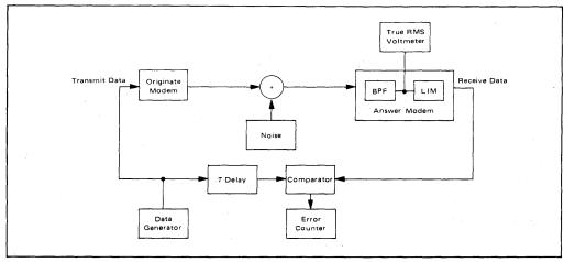
FIGURE 16 - Modem Test Equipment Configuration
