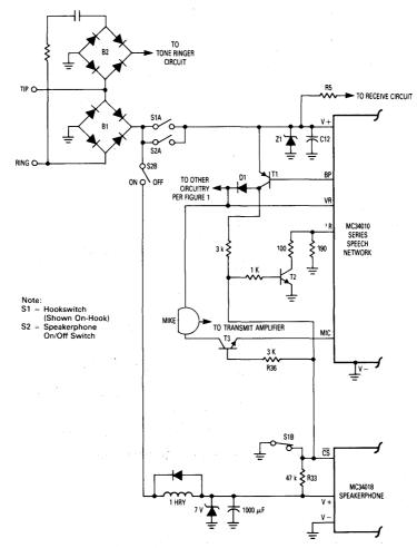
Figure 7. Microphone Muting — MC34010A Series
