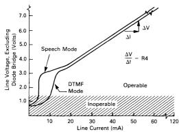
FIGURE 4 - DC V-I CHARACTERISTIC OF THE ETC
