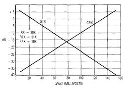
FIGURE 8 — LOG AMP TRANSFER CHARACTERISTICS
