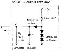
$C_T = 20 \text{ pF} = \text{total parasitic capacitance, which includes probe, wiring, and load capacitances.}$
