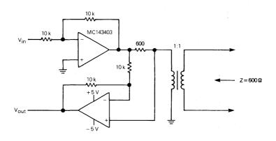
FIGURE 3 - GENERAL PURPOSE DUPLEXER (2-Wire to 4-Wire Converter)
