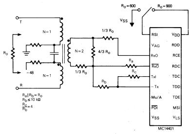
"T" Padded Transformer Hybrid Using MC14401
