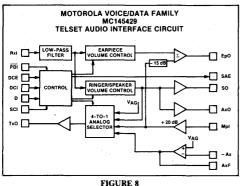
The MC145429 is designed in Si-gate CMOS technology and is implemented in a 18 pin package. This device adds ease of analog signal adjustment with software, in lieu of hardware.
