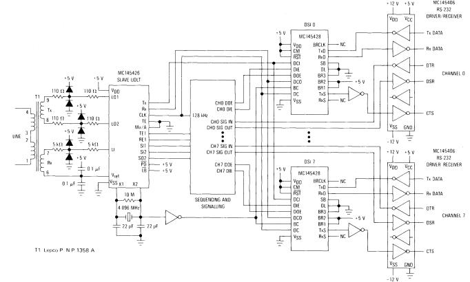
Figure 6. Multiplexing Eight RS-232 Telset Ports Into 64 Kilobits/Second Channel of MC145426
