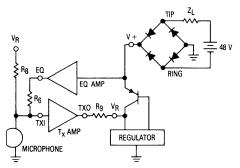
Figure 1. MC34014 Transmit Section
