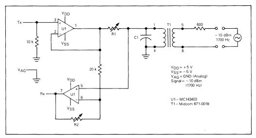
FIGURE 1 - Duplexer Circuit
