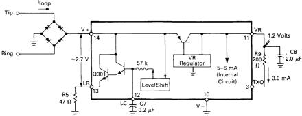
FIGURE 6 — INTERNAL CURRENT versus VOLTAGE
