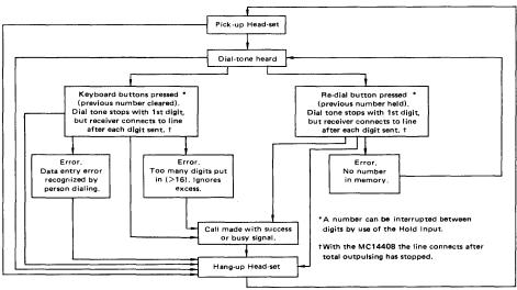
FIGURE 8 - KEYPAD TO PULSE DIALER FLOW DIAGRAM
