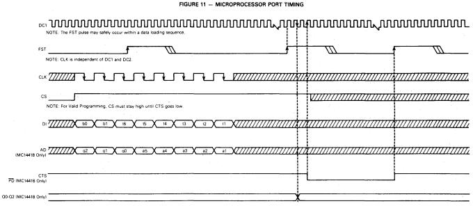
NOTE: For the MC14416, the CTS line is pulled low by the device selected by the CS pin.
