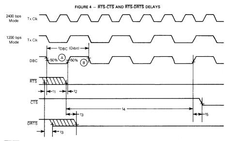
$\overline{RTS}\cdot\overline{CTS}$  delay options are selected by the CTS1 and CTS2 inputs, and are stated as time delay interval t<u>a</u>. An  $\overline{RTS}$  input signal synchronized about point A will synchronize CTS with the positive transition of DBC (Dibit Clock). Delay ta is measured with respect to the negative transition of  $\overline{RTS}$ .
