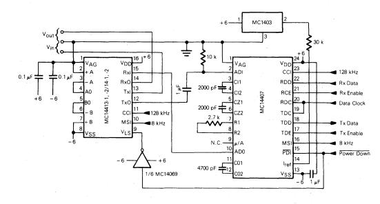
FIGURE 7 — TYPICAL CIRCUIT CONFIGURATION USING THE MC14407 CODEC AND MC14413-1, -2 FILTER (SPLIT SUPPLY)
