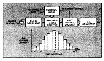
Fig. 2 The DTMF frequency synthesis technique.
