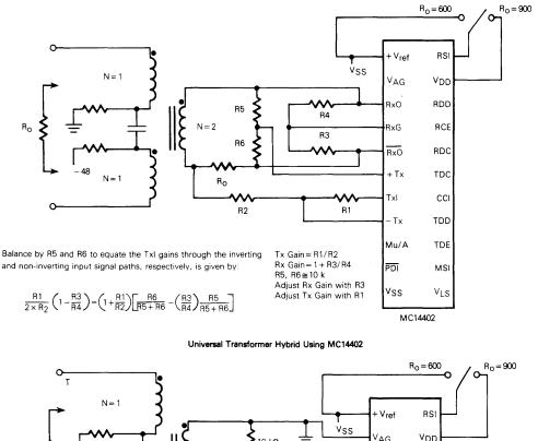
HYBRID INTERFACES TO THE MC14402 PCM CODEC/FILTER MONO-CIRCUIT
