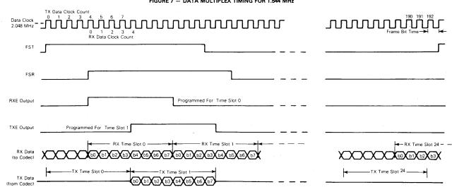
FIGURE 7 -- DATA MULTIPLEX TIMING FOR 1.544 MHz
