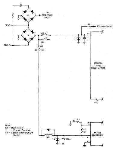
Figure 3. Handset/Speakerphone Power Switching
