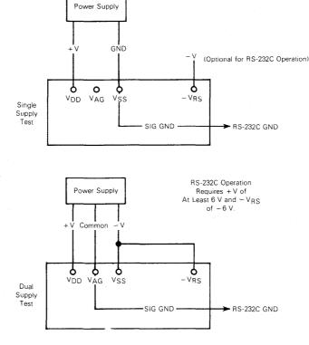
FIGURE 5 - Power Supply Set-Up
