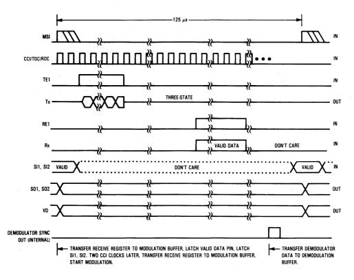
Figure 10. Master UDLT Timing
