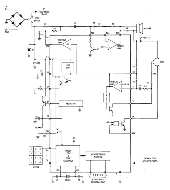
Figure 1. Basic MC34010 Type Telephone
