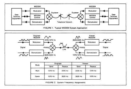
the data terminal receiving this call is the answer MODEM, (transmitting tones of 2025 Hz and 2225 Hz).
