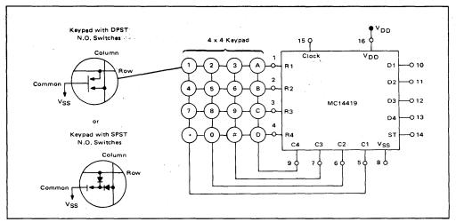
FIGURE 4 - TYPICAL KEYPAD INTERFACE APPLICATION
