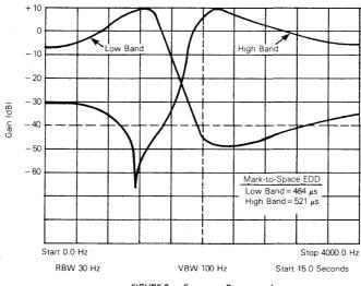
FIGURE 2 — Frequency Response of High Band and Low Band of MC145440
