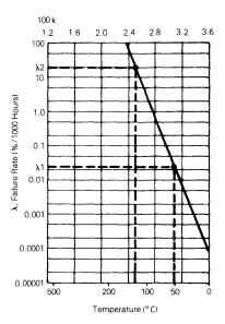
must be applied to the devices until they reach room temperature at the completion of the test. Temperature, time and voltage levels must be specified. Accelerated failure mechanisms are inversion, channeling, surface contamination, design.
