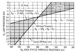
Figure 11 shows such a graph using 17.4  $k\Omega$  as the values for  $R_{\rm R}$  and  $R_{\rm T}$ . Note the oscillatory condition to the right of the crossing point. Selection of  $R_{\rm H}$  in this region is usually not a problem since the majority of telephone lines do not fall into this resistance range.  $R_{\rm H}$  always ties to  $V_{OB}$  and HST and will give reliable hook status information regardless of power supply voltages and PDI.
