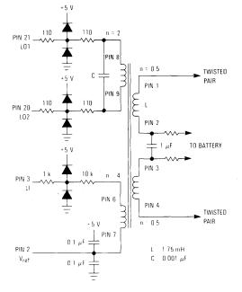
Figure 9. Battery Feed Transformer Configuration
