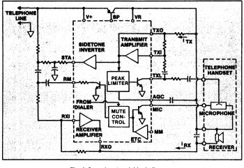
Fig. 4 Speech network block diagram.
