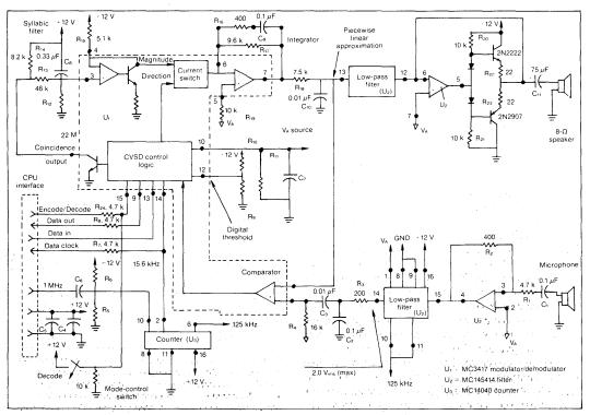
3. A continuously variable slope gives the MC3417 the accuracy to reproduce analog signals. When necessary, does be the syllabic filter changes the rate of integration and with it the slope. The three basic chips, a simple audio amplifier, and a microprocessor interface complete the speech peripheral circuit.
