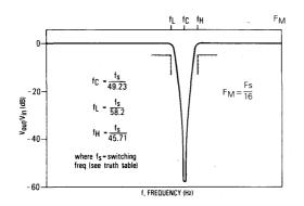
fl fc fh 0 fc 49.23 57.9 - 20fe Vout/Vin (dB) 42.8 fs 3db BW 1295 0 ≈ 26 - 40where fs = switching freq (see truth table) -60f, FREQUENCY (Hz)
