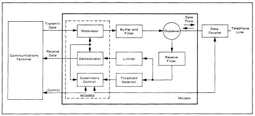
FIGURE 1 - Low-Speed Modem and Interconnections
