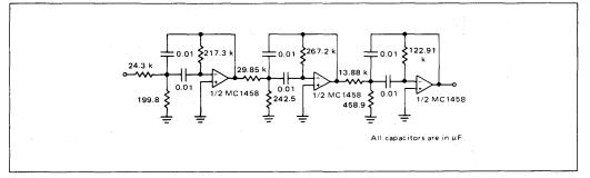
FIGURE 14a - Originate Filter Component Values
