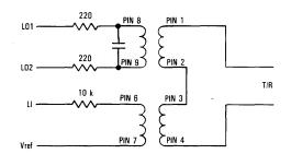
Figure 3. Transformer Configuration
