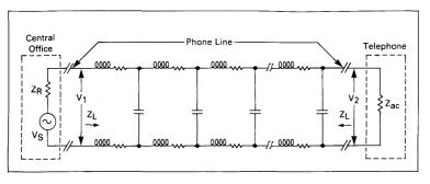
Figure 16 depicts the situation in the transmit mode. In this mode, the MC34014 is an ac current source, with a finite output impedance, modulating the loop current. The voltage signal V<sub>1</sub> is therefore equal to the ac signal current acting on Z<sub>ac</sub> in parallel with the characteristic
