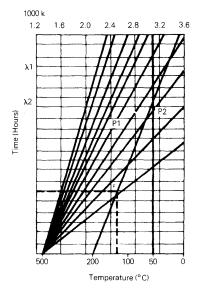
For increased flexibility in working with a broad range of device hours, the time-temperature regression lines have been normalized to  $500^{\circ}$ C and the time scale omitted, permitting the user to define the scale based on his own requirements.
