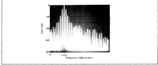
FIGURE 4 -- Modulation Spectrum for Alternate Mark/Space
