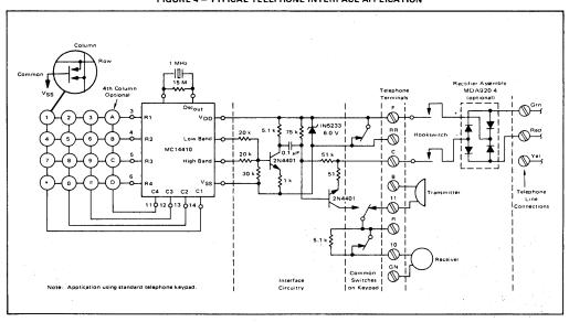
FIGURE 4 - TYPICAL TELEPHONE INTERFACE APPLICATION
