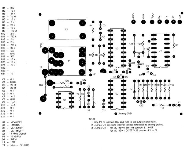
FIGURE 9 - Modem 1 Board MC145440/MC14412
