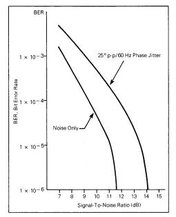
FIGURE 10 - B Mod 2400 BPS Back-To-Back 511 Test Pattern
