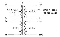
Figure 3. DLT Coupling Transformer
