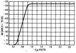
Figure 1. Equalization Amplifier Gain
