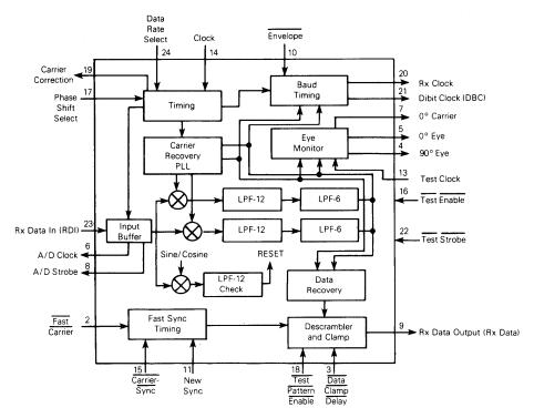
FIGURE 2 - DEMODULATOR BLOCK DIAGRAM
