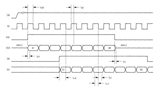
Figure 3B. Synchronous 1/O, Eight Bit, Clock Mode High
