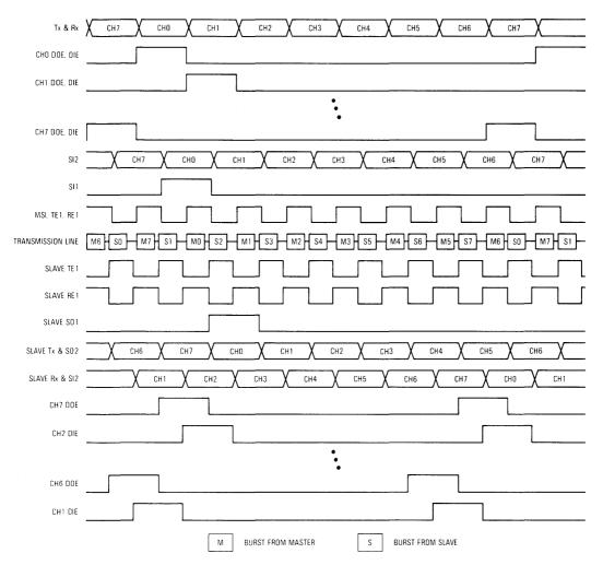
Figure 9. System Timing
