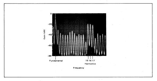
FIGURE 3 - Frequency Spectrum of MOS Sine Wave
