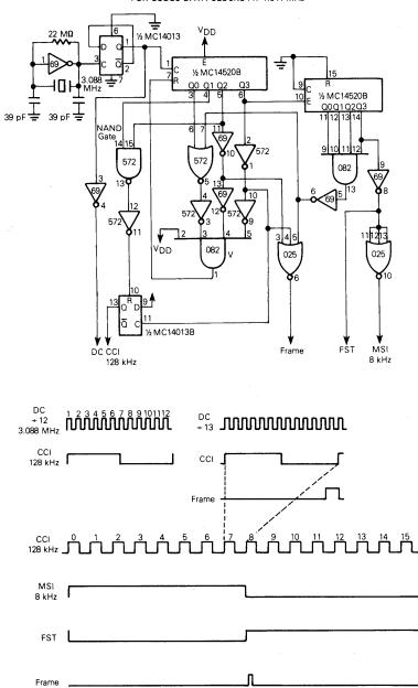
FIGURE 15 – CLOCK CIRCUIT AND TIMING FOR CODEC DATA CLOCKS AT 1.544 MHz
