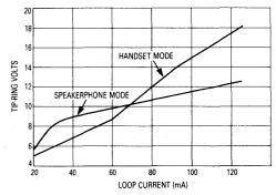
Figure 5. Tip-Ring Voltage versus Loop Current
