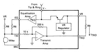
If a variation in  $Z_{ac}$  of less than 3:1 is desired, the circuit configuration of Figure 18 may be used. The ac impedance is the parallel combination of  $R_x$  and the
