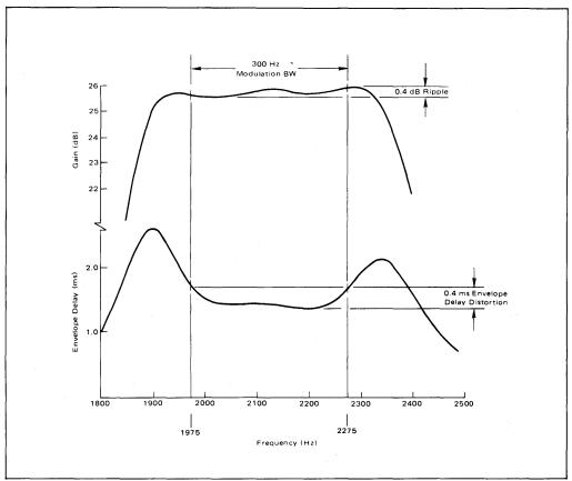
FIGURE 10 - Originate Bandpass Filter Characteristics
