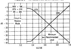
FIGURE 6 — ATTENUATOR GAIN versus ΔVacf
