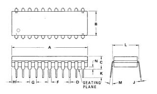
NOTES: 1. LEADS TRUE POSITIONED WITHIN 0.25 mm (0.010) DIA AT SEATING PLANE AT MAXIMUM MATERIAL CONDITION (DIM "D"). 2. DIM "L" TO CENTER OF LEADS WHEN FORMED PARALLEL.
