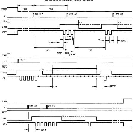
FIGURE 3 PHONE DIALER SYSTEM TIMING DIAGRAM
