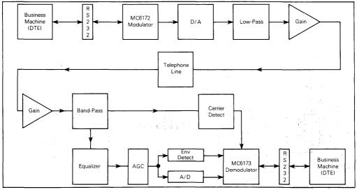
FIGURE 3—MC6172/6173 Modem Block Diagram
