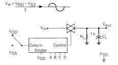
FIGURE 4 – CROSSTALK BETWEEN ANY TWO SWITCHES
