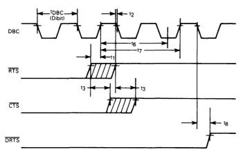
A positive transition of  $\overline{\text{RTS}}$  after  $\overline{\text{CTS}}$  has become active can result in different functional characteristics of the  $\overline{\text{CTS}}$  and  $\overline{\text{DRTS}}$  output signals, depending on the time duration that  $\overline{\text{RTS}}$  remains inactive.
