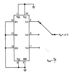
Figure 1. Power-Off Source Resistance (Drivers)
