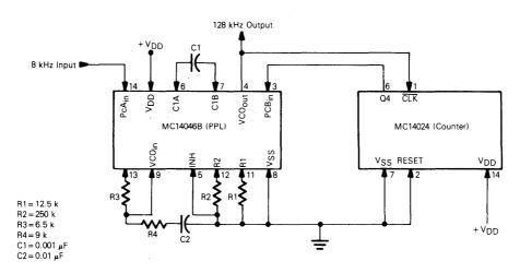
FIGURE 15 - 128 kHz FREQUENCY SYNTHESIZER USING 8 kHz INPUT
