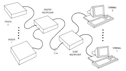
Figure 1. Typical Multiplexer Application
