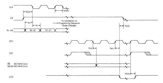
NOTE: tPCH is measured from the rising edge of the latter of FST or DC1.
