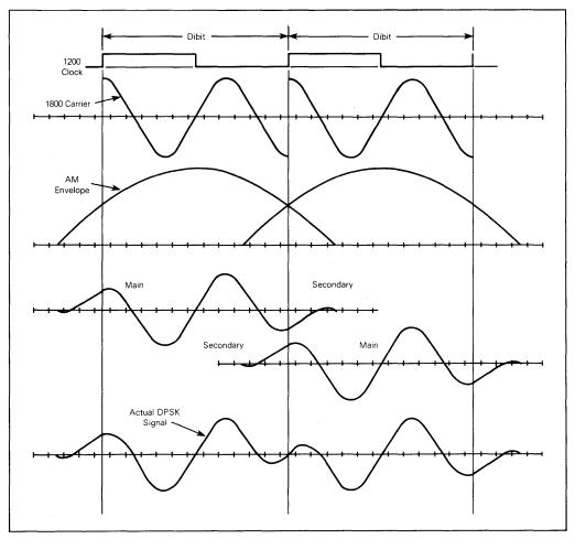
FIGURE 2-DPSK Waveforms
