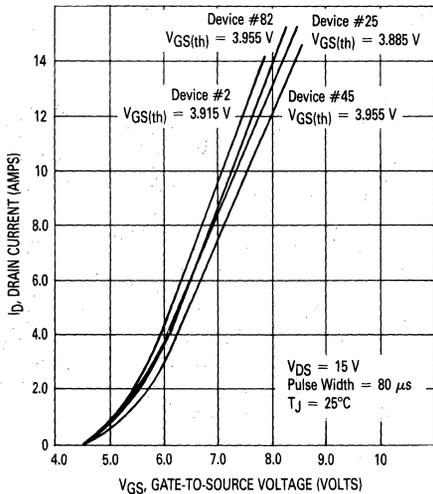
FIGURE 6-8 — TRANSCONDUCTANCE CURVES OF MTP8N18s WITH MATCHED THRESHOLD VOLTAGES
