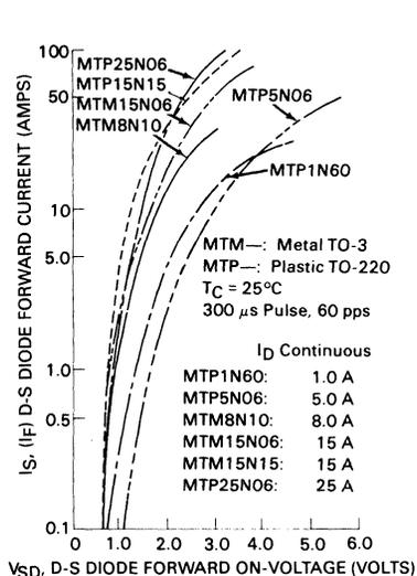
FIGURE 11-22 — FORWARD CHARACTERISTICS OF POWER MOSFETS D-S DIODES
