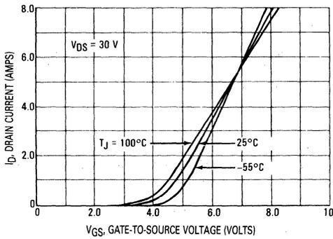
FIGURE 2-3 — TRANSFER CHARACTERISTICS OF MTP4N50
