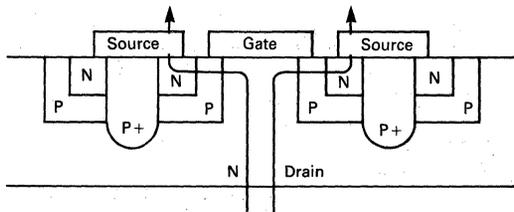
FIGURE 11-6a — TYPICAL CURRENT FLOW IN T MOS POWER MOSFET
