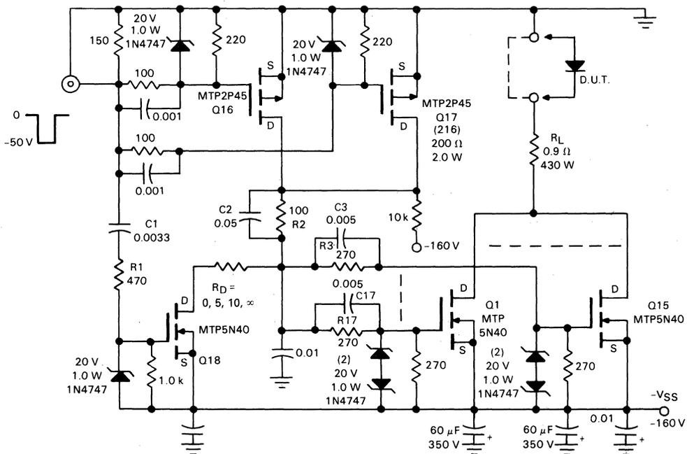
**FIGURE 6-38 — PARALLELED POWER MOSFETS 150 A SWITCH**
