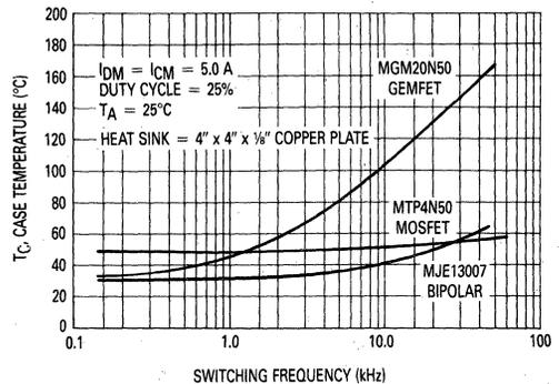
FIGURE 8-11 — COMPARISON OF CASE TEMPERATURE versus FREQUENCY FOR A GEMFET, MOSFET AND BIPOLAR
