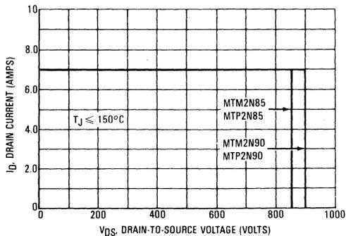
FIGURE 7-11b — MAXIMUM RATED SWITCHING SAFE OPERATING AREA
