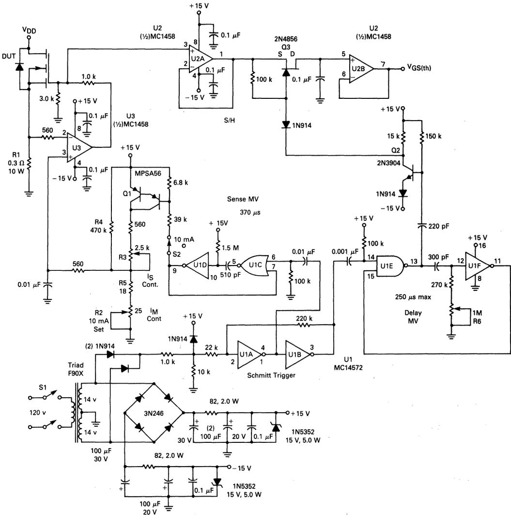
FIGURE 11-28 — POWER MOSFET  $V_{GS(th)}$  THERMAL FIXTURE
