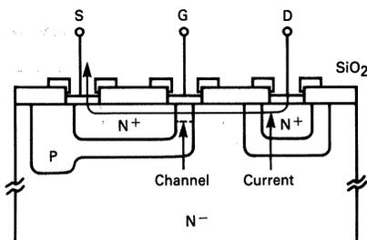
FIGURE 1-4 — LATERAL DOUBLE DIFFUSED MOSFET STRUCTURE FEATURING SHORT CHANNEL LENGTHS AND HIGH PACKING DENSITIES FOR LOWER ON RESISTANCE.
