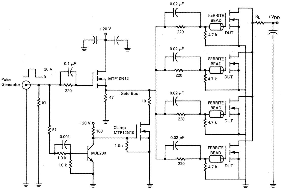
FIGURE 6-5 — DYNAMIC CURRENT SHARING TEST CIRCUIT
