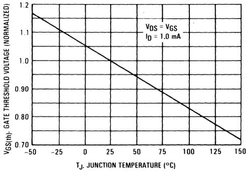
FIGURE 6 — TRANSFER CHARACTERISTICS
