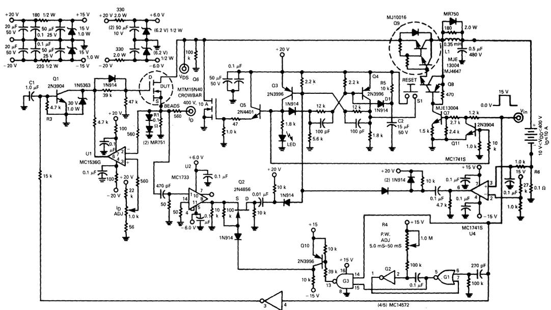
FIGURE 11-1 — N-CHANNEL POWER MOSFET NON-DESTRUCT FBSOA TESTER
