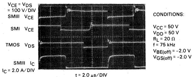
FIGURE 9-3 — RESISTIVE LOAD SWITCHING OF DUTs AT 75 kHz
