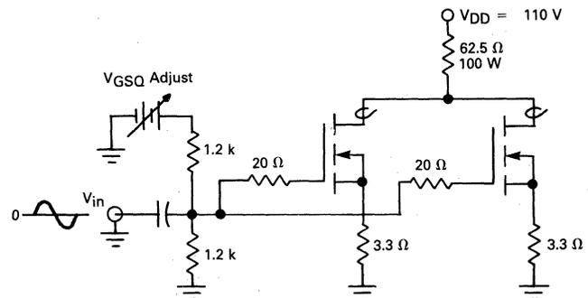
FIGURE 6-29 — CIRCUIT TO TEST CURRENT SHARING IN PARALLELED MOSFETs OPERATING IN THE LINEAR MODE
