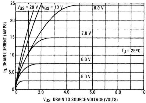
FIGURE 3 — TRANSFER CHARACTERISTICS
