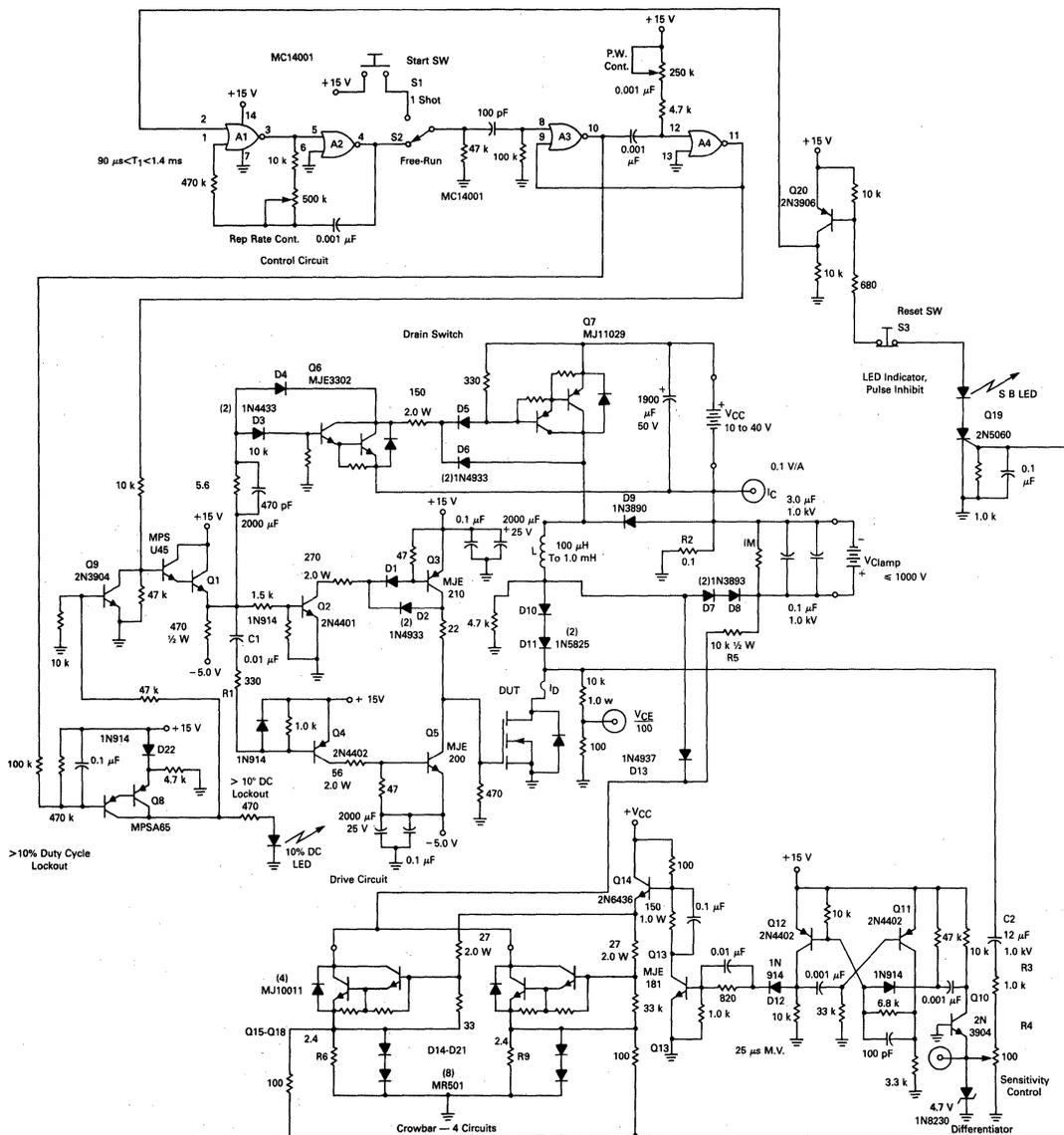
FIGURE 11-11 — N-CHANNEL POWER MOSFET NON-DESTRUCT TURN-OFF SWITCHING SOA TESTER 1000 V, 50 A
