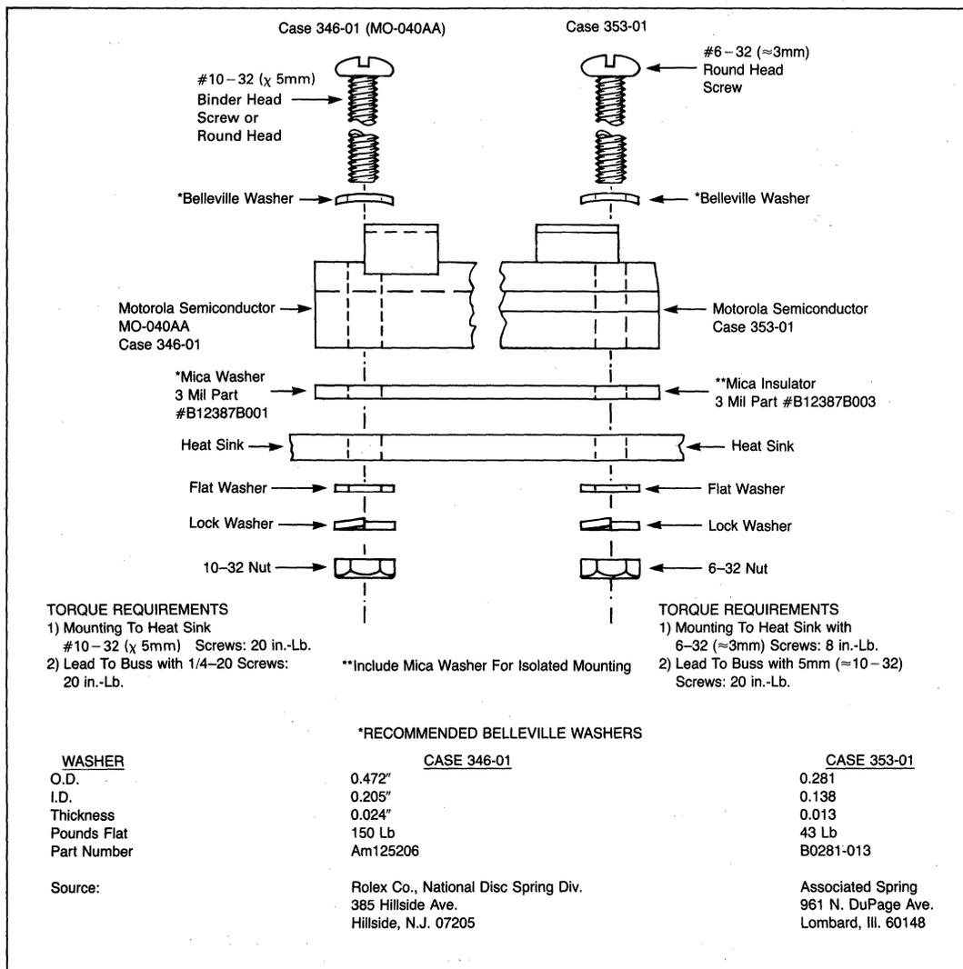
FIGURE 13-10 — MOUNTING OF ENERGY MANAGEMENT SERIES CASE 346-01 AND CASE 353-01
