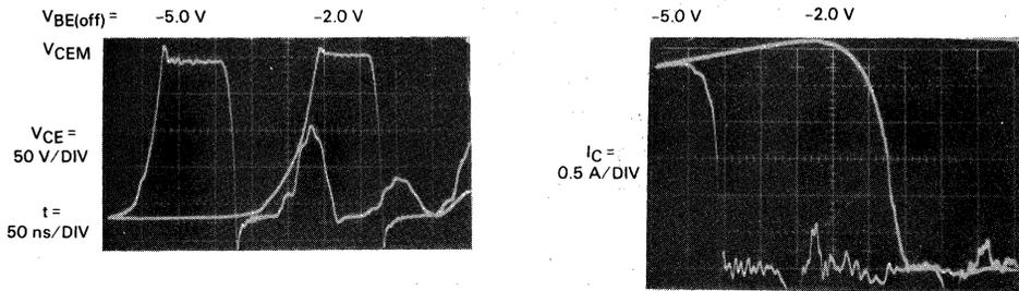
FIGURE 9-7 — CLAMPED INDUCTIVE LOAD TURN-OFF TIMES OF SWITCHMODE I 2N6545 WITH TWO OFF-BIAS VOLTAGES
