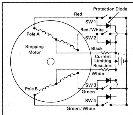
FIGURE 7-17 — SIMPLIFIED STEPPING MOTOR AND CONTROL BLOCK DIAGRAM\*
