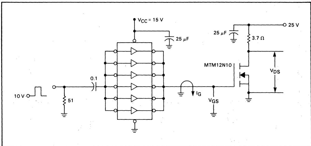
FIGURE 5-12 — MC14050CL HEX BUFFER AS A DRIVER FOR POWER MOSFET
