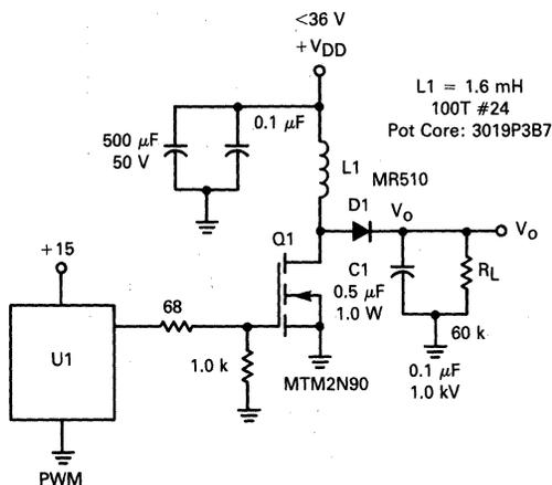
FIGURE 7-10a — SINGLE MOSFET OUTPUT
