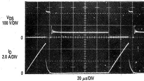
FIGURE 8-10a — CLAMPED INDUCTIVE SWITCHING WAVEFORMS AT 7.0 kHz — GEMFET
