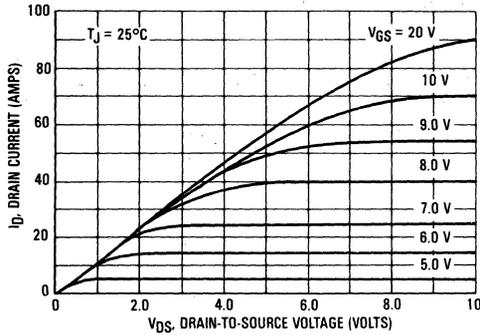
FIGURE 3 — TRANSFER CHARACTERISTICS
