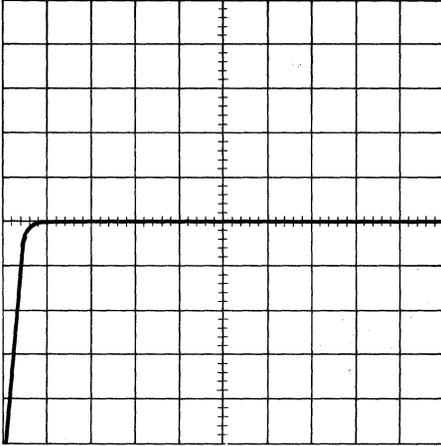
FIGURE 11-30 — CURVE TRACER PRESENTATION FOR  $V_{GS(th)}$  — MTP12N10
