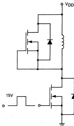
FIGURE 6-33 — INTRINSIC D-S DIODE CLAMPING AN INDUCTIVE LOAD
