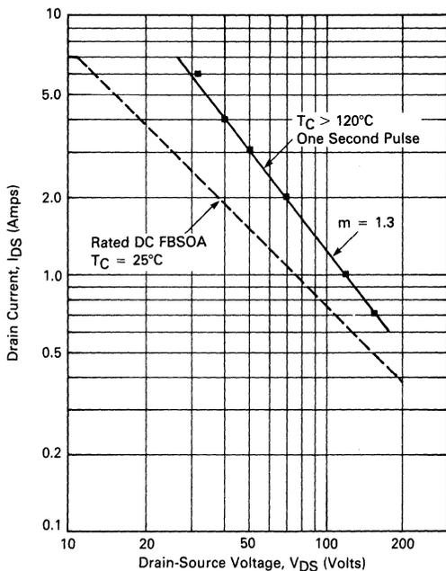
FIGURE 11-4 — DC FBSOA TEST ON MTP7N20
