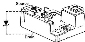
FIGURE 10-3 — OPTIMUM PLACEMENT OF  $V_{DS}$  CLAMP
