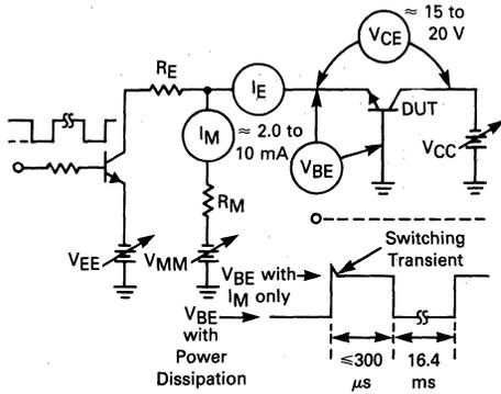
FIGURE 11-24 — BASIC BLOCK DIAGRAM OF STEADY STATE THERMAL RESISTANCE TEST CIRCUIT FOR BIPOLAR TRANSISTORS
