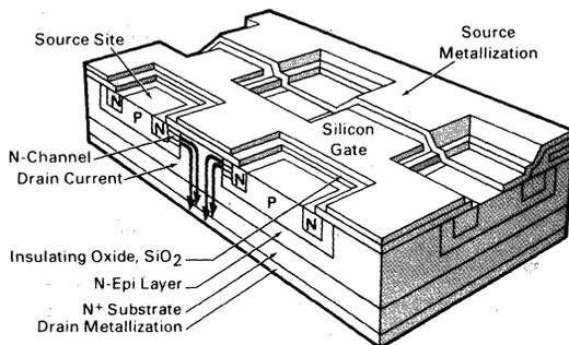
FIGURE 2-17 — CROSS SECTION OF TMOS CELL
