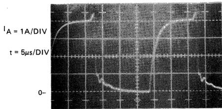
FIGURE 9-12a — GTO ANODE CURRENT
