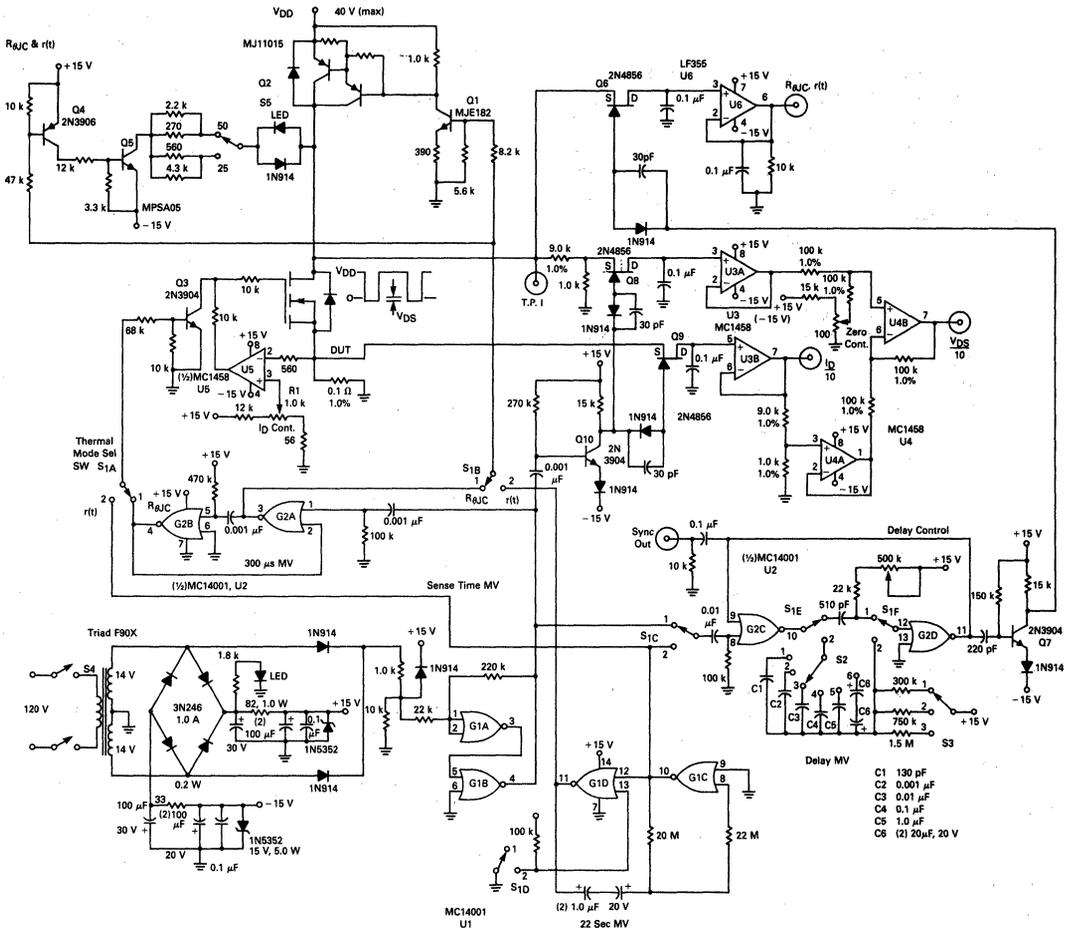
FIGURE 11-27 — POWER MOSFET THERMAL FIXTURE
