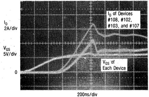
FIGURE 6-17b — SLOW TURN-ON SUPPLYING REVERSE RECOVERY CURRENT OF FREEWHEELING DIODE
