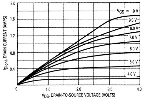
FIGURE 5 — OUTPUT CHARACTERISTICS
