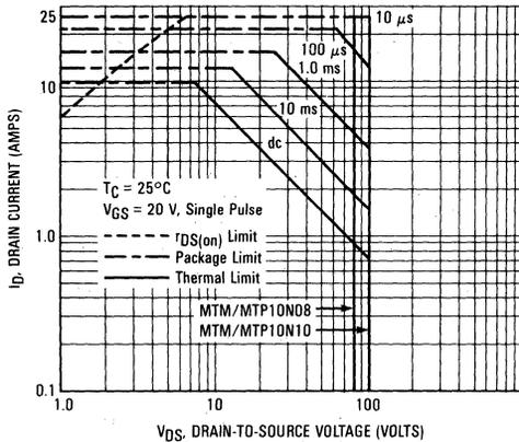
FIGURE 10 — MAXIMUM RATED SWITCHING SAFE OPERATING AREA
