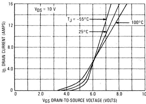
FIGURE 6 — GATE THRESHOLD VOLTAGE VARIATION
