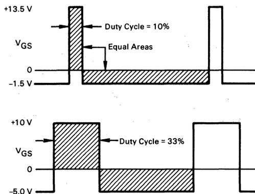
FIGURE 5-9 — VARIATION OF  $V_{GS}$  WITH DUTY CYCLE IN PULSE TRANSFORMER GATE-DRIVE
