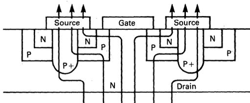
FIGURE 11-6c — CURRENT FLOW DURING NEGATIVE RESISTANCE BREAKDOWN
