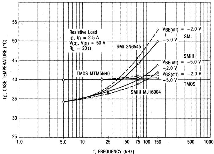
FIGURE 9-5 — TEMPERATURE RISE OF SWITCHMODE DEVICES AS A FUNCTION OF FREQUENCY
