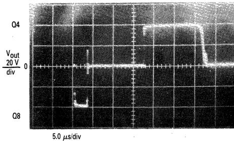
FIGURE 6-43b — FAST TRAILING EDGE, NEG. VOLTAGE, TURN-OFF CLAMP Q10 "ON"
