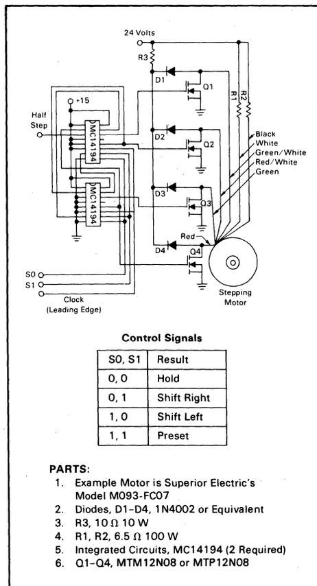
FIGURE 7-20 — HALF- OR FULL-STEP DRIVE FOR CENTER-TAPPED STEPPING MOTORS
