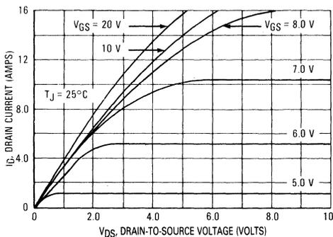
FIGURE 6-24 — TYPICAL OUTPUT CHARACTERISTICS OF AN MTP8N20
