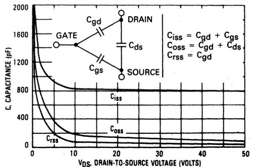
FIGURE 2-9 — TMOS INTERELECTRODE CAPACITANCES
