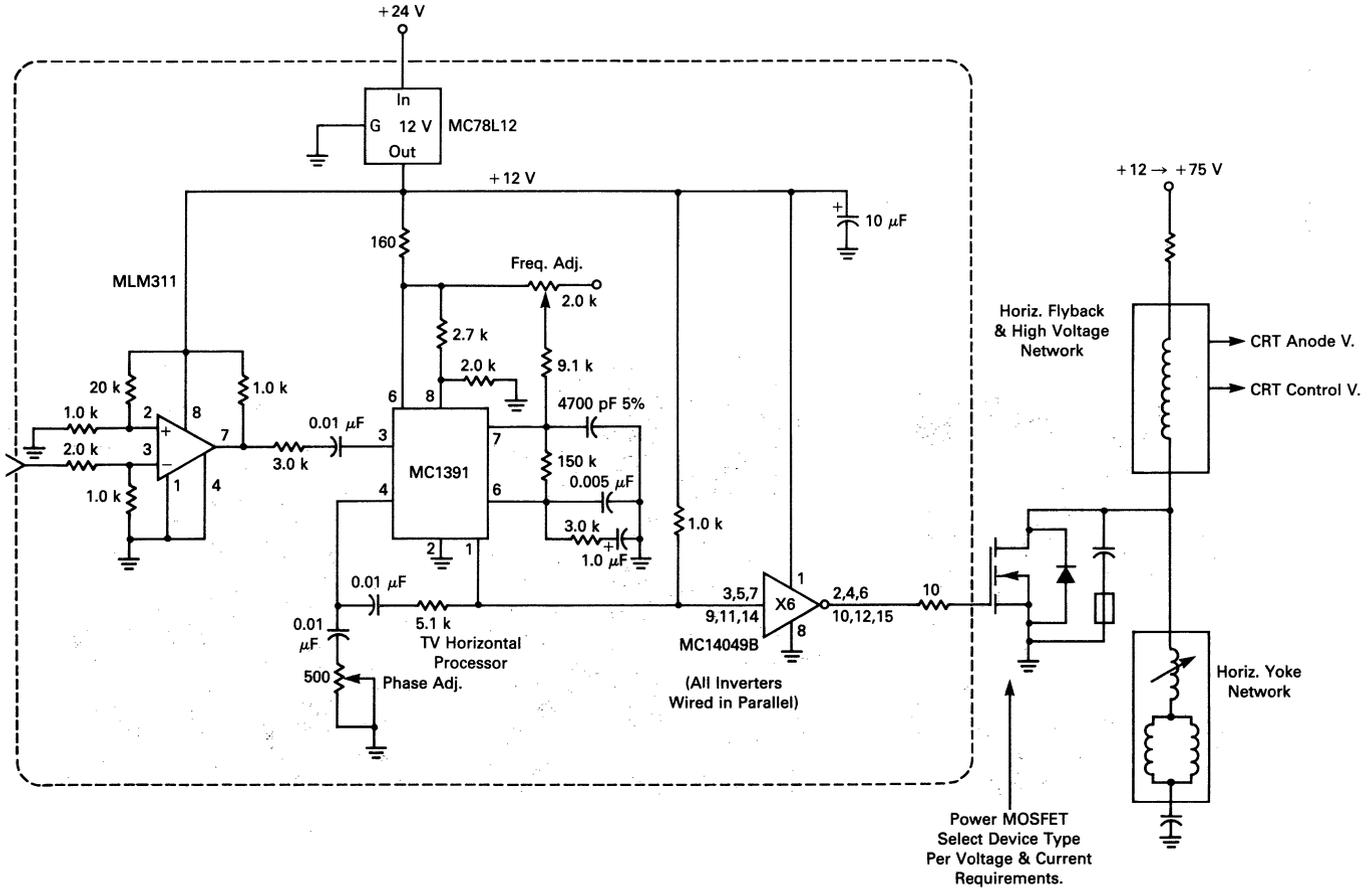
FIGURE 7-34 — POWER MOSFET HORIZONTAL SWEEP DESIGN
