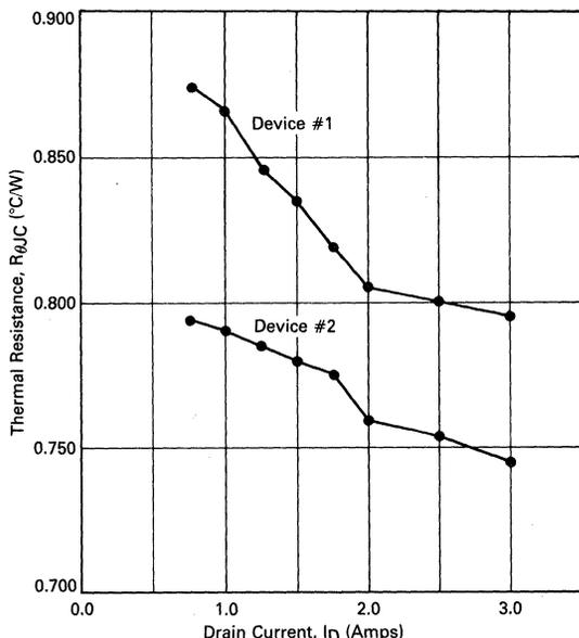
FIGURE 11-7 — THERMAL RESISTANCE OF MTM12N10 versus DRAIN CURRENT AT  $P_D = 50$  W
