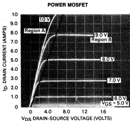
FIGURE 2-1 —  $I_D$ - $V_{DS}$  TRANSFER CHARACTERISTICS OF MTP8N15. REGION A IS CALLED THE OHMIC, ON, CONSTANT RESISTANCE OR LINEAR REGION. REGION B IS CALLED THE ACTIVE, CONSTANT CURRENT, OR SATURATION REGION.
