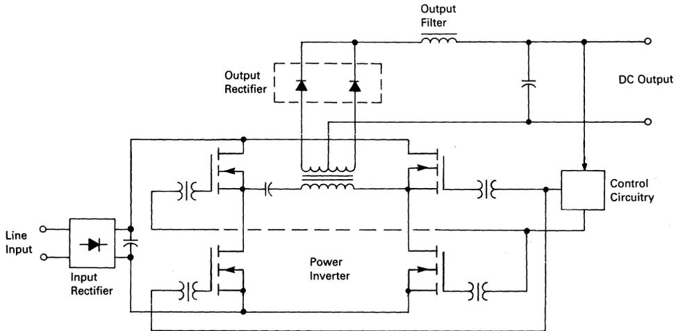
**FIGURE 7-14 — BASIC FULL-BRIDGE CONFIGURATION**
