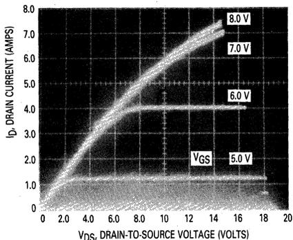
FIGURE 8-3a — OUTPUT CHARACTERISTICS OF POWER MOSFET (MTP4N50)
