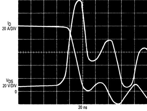
FIGURE 10-6b — DRAIN CURRENT AND DRAIN-SOURCE VOLTAGE APPEARING NEAR CHIPS — MTE60N20 — OFF BIAS = -4.0 VOLTS
