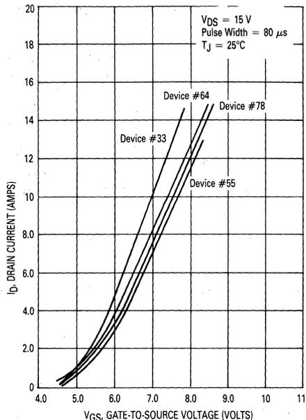
FIGURE 6-4 — WIDEST VARIATION IN TRANSCONDUCTANCE CURVES FOUND IN WAFER LOT I
