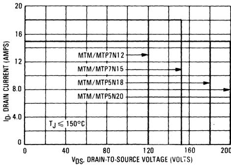
FIGURE 11-8 — MAXIMUM RATED SWITCHING SAFE OPERATING AREA
