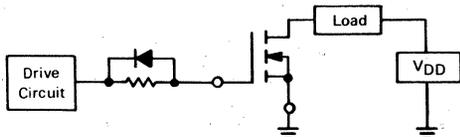
conversely, to minimize problems associated with very rapid turn-off, such as large flyback voltages, the arrangement below will increase turn-off time without affecting turn-on time:
