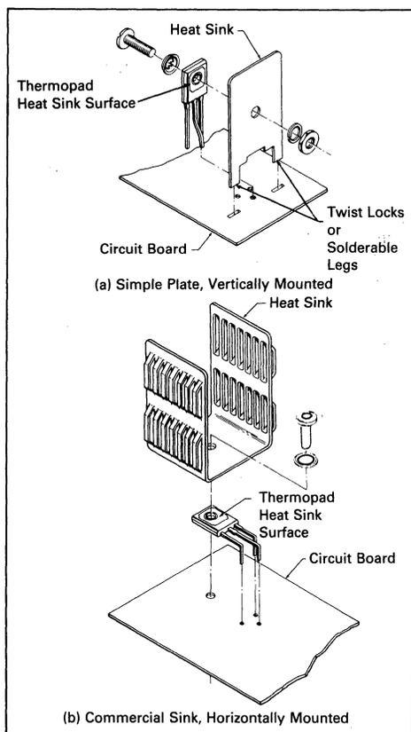
**FIGURE 13-11 — METHODS OF USING SMALL HEAT SINKS WITH PLASTIC SEMICONDUCTOR PACKAGES**
