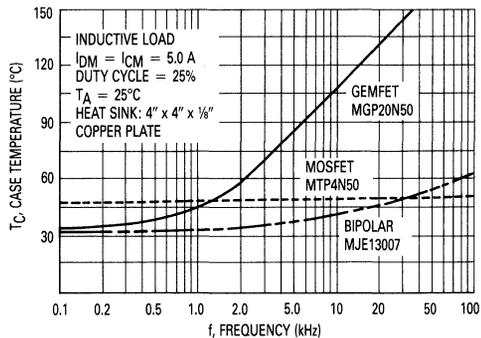
FIGURE 9-14 — COMPARISON OF CASE TEMPERATURE versus FREQUENCY FOR A GEMFET, MOSFET AND BIPOLAR TRANSISTOR
