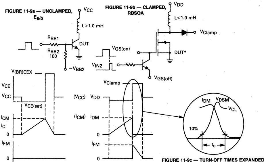
\*Waveforms shown for MOSFET DUT. Bipolar Terms in Parentheses.
