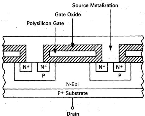
FIGURE 8-1b — CROSS SECTION OF GEMFET CELL
