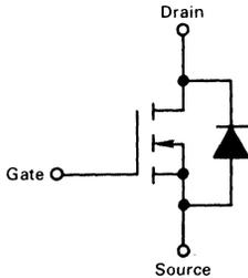
FIGURE 2-18 — COMPLETE N-CHANNEL POWER MOSFET SYMBOL INCLUDING DRAIN-SOURCE DIODE
