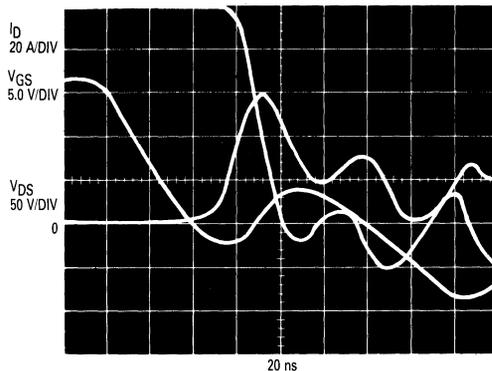
FIGURE 10-15 —  $V_{GS} - I_D$  Delay Due to Gate Suppression Resistors
