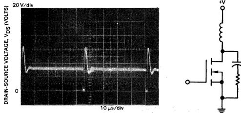
FIGURE 4-10 —  $V_{DS}$  TRANSIENT WITH RC SNUBBER
