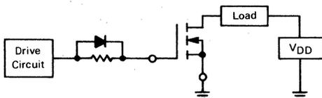
Just as they govern the turn-on process, the parasitic capacitances and gate-drive impedance also dictate turn-off speeds. At faster switching speeds, turn-off waveforms are particularly interesting because  $di/dt$ 's are not limited by load or wiring inductance.
