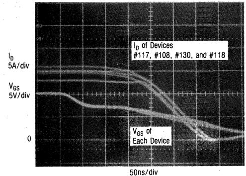
FIGURE 6-9a — PARALLELED TURN-ON
