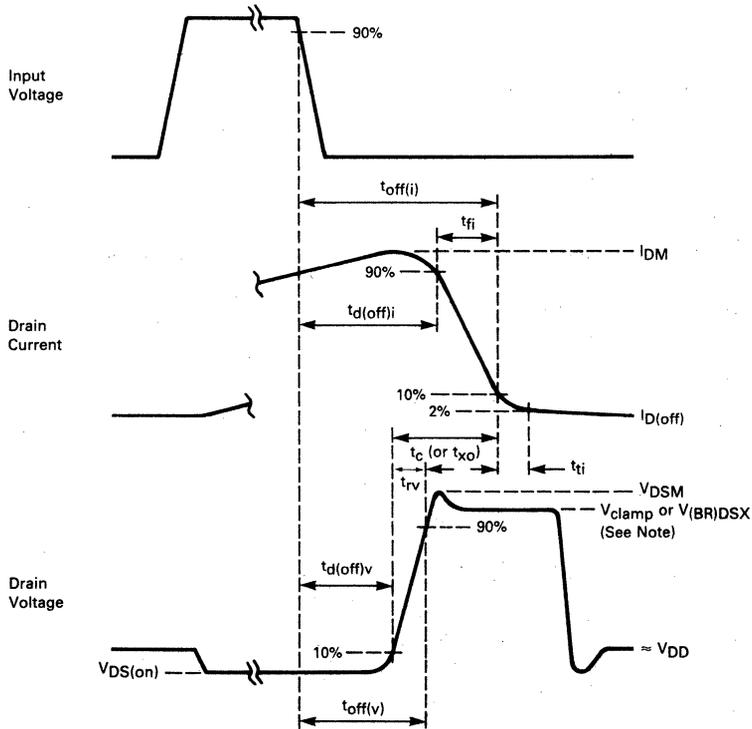
NOTE:  $V_{clamp}$  (in a clamped inductive-load switching circuit) or  $V_{(BR)DSX}$  (in an unclamped circuit) is the peak off-state voltage excluding spikes.
