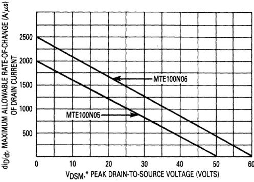
FIGURE 10-7 — MAXIMUM ALLOWABLE  $di/dt$  PEAK DRAIN-SOURCE VOLTAGE FOR MTE100N06
