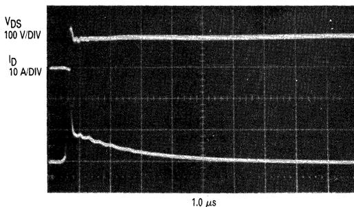
FIGURE 8-16a — CLAMPED INDUCTIVE TURN-OFF WAVEFORMS OF MGM20N50 —  $R_{GS} = 51 \Omega$
