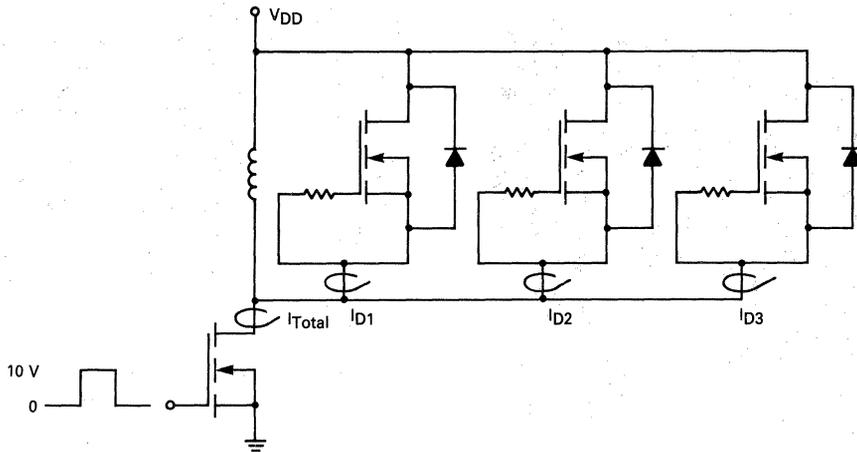
FIGURE 6-34 — TEST CIRCUIT TO OBSERVE CURRENT SHARING OF PARALLELED D-S DIODES
