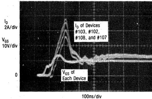
FIGURE 6-17a — RAPID TURN-ON SUPPLYING REVERSE RECOVERY CURRENT OF FREEWHEELING DIODE
