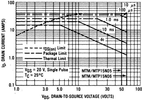
FIGURE 13 — MAXIMUM RATED SWITCHING SAFE OPERATING AREA
