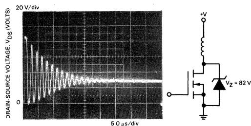
FIGURE 4-8 —  $V_{DS}$  TRANSIENT WITH ZENER CLAMP
