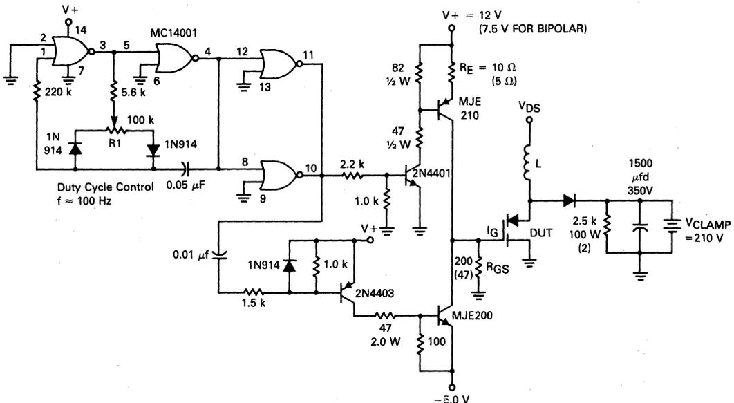
FIGURE 8-9 — CIRCUIT TO COMPARE SWITCHING EFFICIENCIES OF GEMFET, MOSFET AND BIPOLAR
