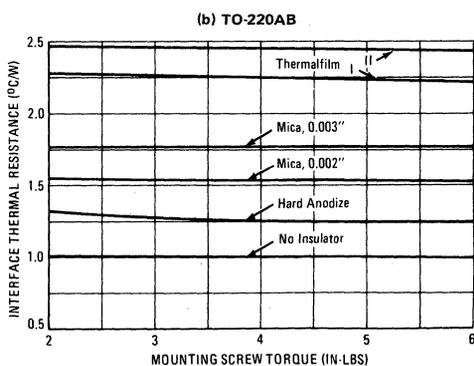
FIGURE 13-3 — INTERFACE THERMAL RESISTANCE WITHOUT THERMAL GREASE AS A FUNCTION OF MOUNTING SCREW TORQUE USING VARIOUS INSULATING MATERIALS
