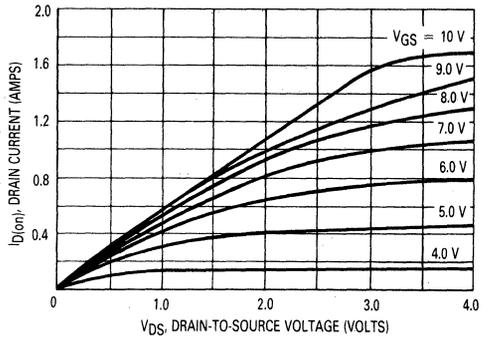
FIGURE 5 — OUTPUT CHARACTERISTICS
