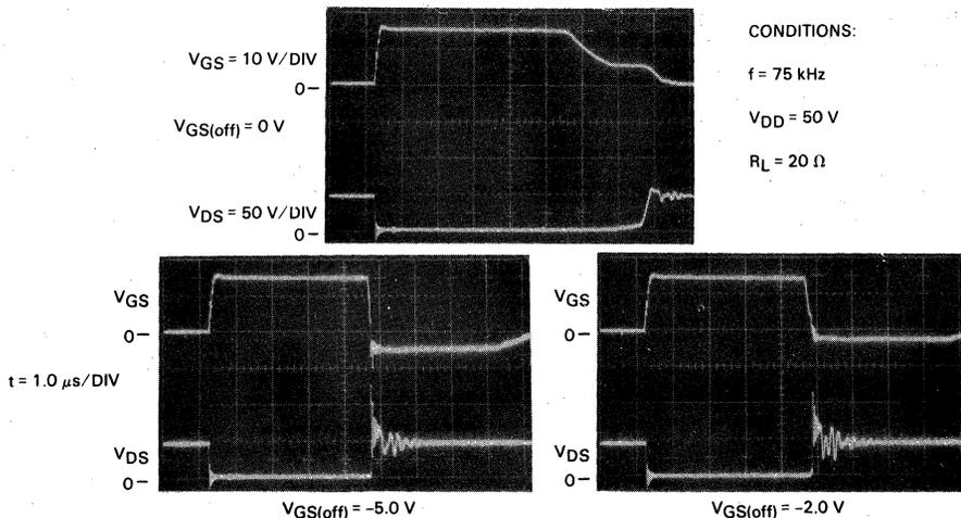
FIGURE 9-8 — THE EFFECT OF OFF-BIAS VOLTAGE  $V_{GS(off)}$  ON TURN-OFF TIMES OF TMOS MTM5N40, RESISTIVE LOAD
