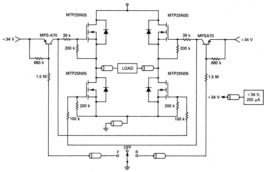
FIGURE 7-28 — "H" SWITCH POWER TMOS CIRCUITS
