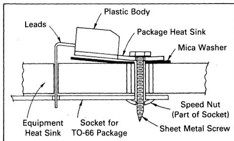
FIGURE 13-1 — EXTREME CASE OF IMPROPERLY MOUNTING A SEMICONDUCTOR (DISTORTION EXAGGERATED)
