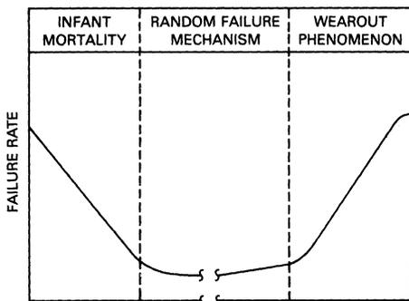
FIGURE 12-1 — FAILURE RATE OF SEMICONDUCTOR
