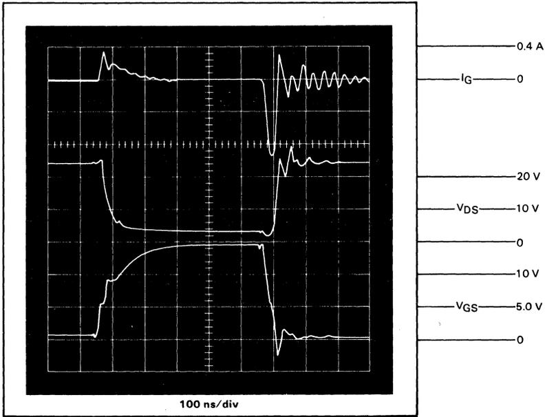
FIGURE 5-13 — POWER MOSFET SWITCHING WAVEFORMS
