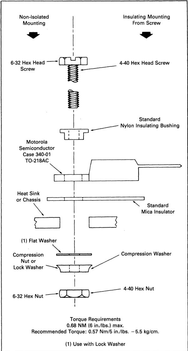
FIGURE 13-8 — MOUNTING ARRANGEMENTS FOR THERMOWATT PACKAGES (TO-220)
