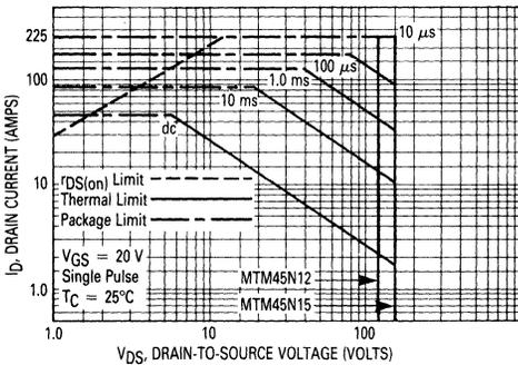
FIGURE 14 — MAXIMUM RATED SWITCHING SAFE OPERATING AREA
