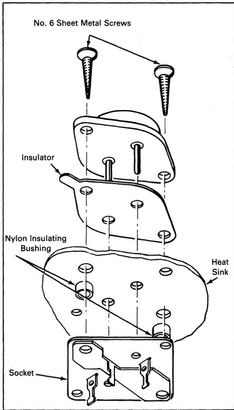
**FIGURE 13-6 — MOUNTING DETAILS FOR FLAT-BASE MOUNTED SEMICONDUCTORS (TO-204AA (TO-3) SHOWN).**
