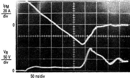
FIGURE 6-45 — REVERSE RECOVERY ( $t_{rr}$ ) OF MR821 FAST RECOVERY RECTIFIER
