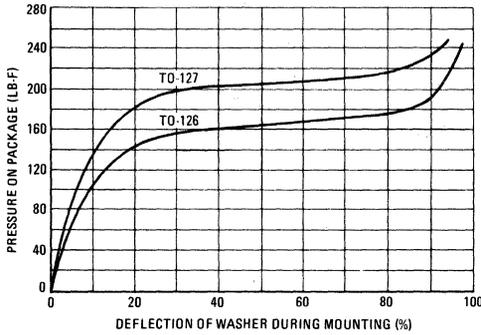
FIGURE 13-5 — CHARACTERISTICS OF THE BELL COMPRESSION WASHERS DESIGNED FOR USE WITH THERMOPAD SEMICONDUCTORS
