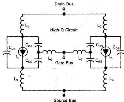
FIGURE 6-20 — PARASITIC HIGH-Q EQUIVALENT CIRCUIT OF PARALLELED MOSFETs WITHOUT GATE DECOUPLING RESISTORS
