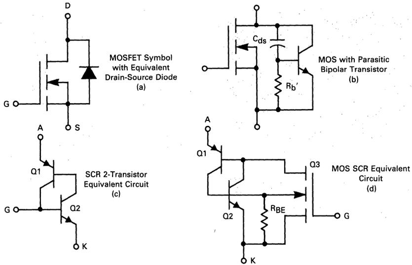
FIGURE 8-19 — EQUIVALENT CIRCUIT EVOLUTION OF THE MOS SCR
