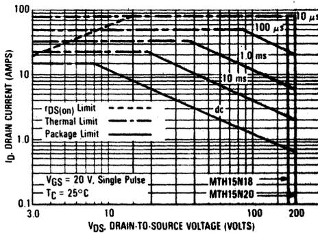
FIGURE 14 — MAXIMUM RATED SWITCHING SAFE OPERATING AREA
