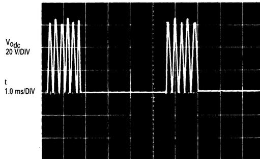
FIGURE 8-30 — GATED FULL-WAVE OUTPUT OF AC POWER SWITCH
