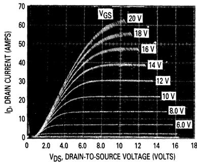
FIGURE 8-4 — OUTPUT CHARACTERISTICS OF GEMFET AT HIGH DRAIN CURRENTS
