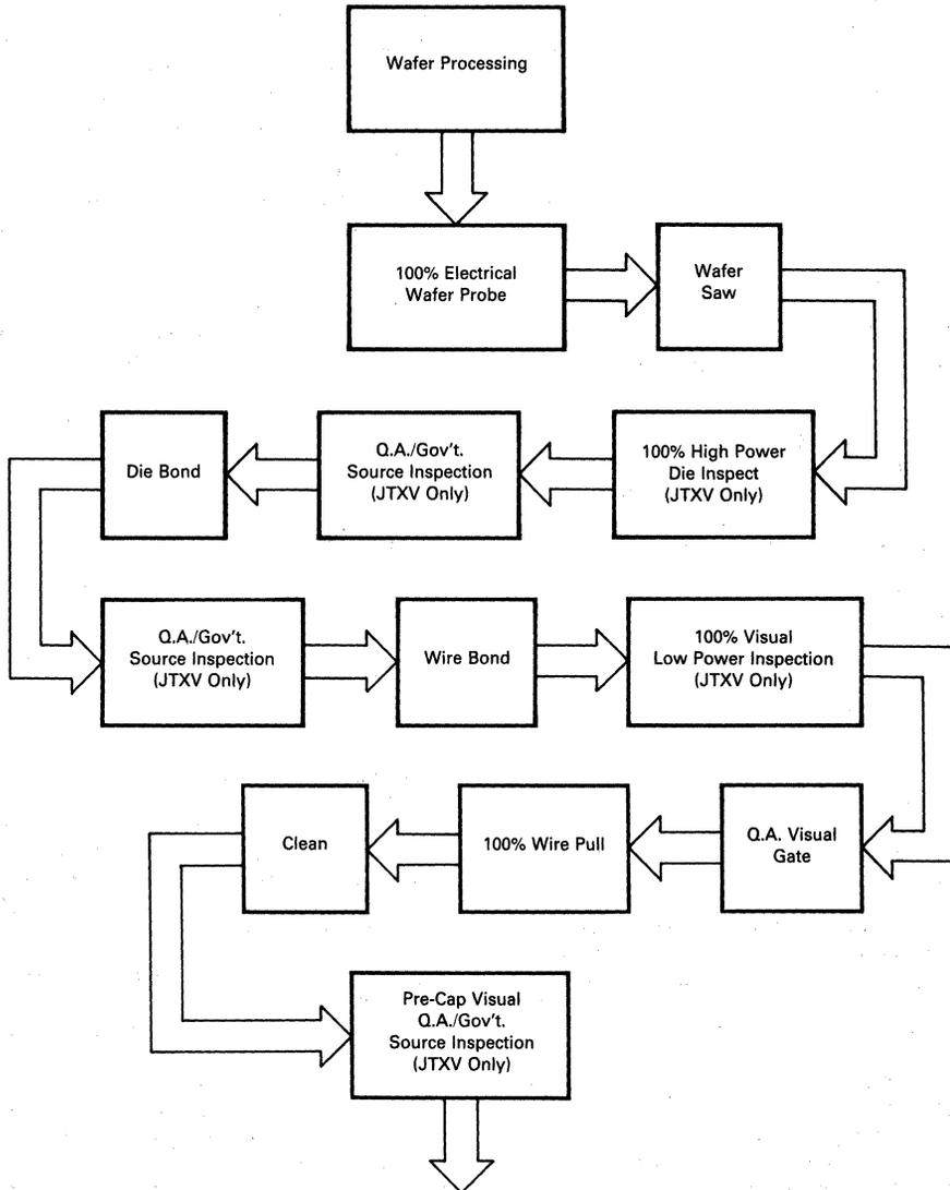
FIGURE 12-3 — JAN, JTX, JTXV AND/OR EQUIVALENT PROCESS FLOW:
