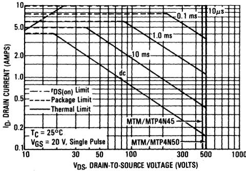
FIGURE 15 — MAXIMUM RATED SWITCHING SAFE OPERATING AREA
