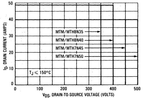
**FIGURE 4-5 — MAXIMUM RATED SWITCHING SAFE OPERATING AREA OF THE MTM8N40**
