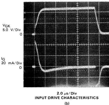
FIGURE 8-25 — SWITCHING CHARACTERISTICS OF THE MCR1000 WITH THE PREFERRED GATE-DRIVE CIRCUIT
