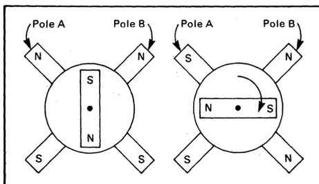
FIGURE 7-16 — SIMPLIFIED STEPPING MOTOR
