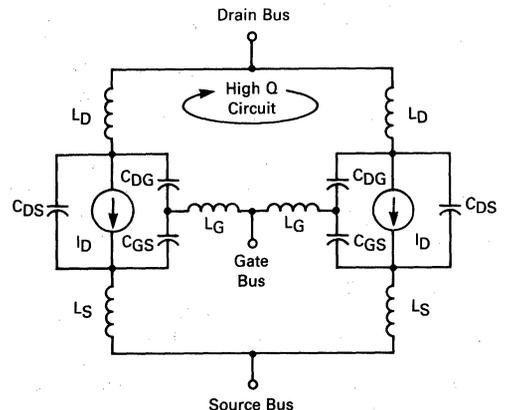
FIGURE 10-2 — PARASITIC HIGH Q CIRCUIT ACCOMPANYING PARALLELED MOSFETs WITH NO GATE DECOUPLING RESISTORS.
