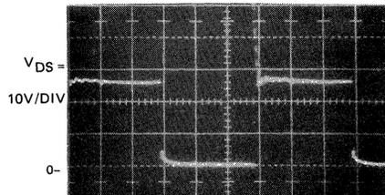
FIGURE 9-12e — TMOS DRAIN-SOURCE VOLTAGE
