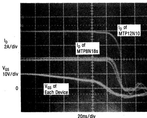
FIGURE 6-14 — INDIVIDUAL  $I_D$  WAVEFORMS OF AN MTP12N10 PARALLELED WITH THREE MTP8N18s — RESISTIVE LOAD — RAPID TURN-OFF
