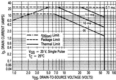
FIGURE 9 — MAXIMUM RATED SWITCHING SAFE OPERATING AREA
