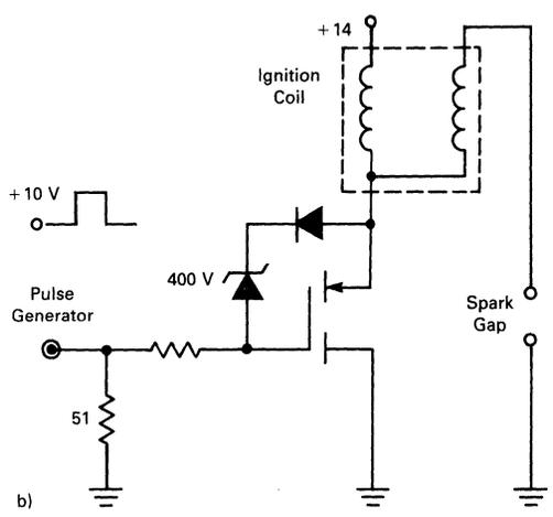
The difference between the  $r_{DS(on)}$  of the MOSFET and the GEMFET becomes evident during the monitoring of the case temperatures. Under the same conditions (using a Thermalloy heat sink #6016B), the GEMFET's  $T_C$  is 37°C, while the MOSFET's is 59°C, representing a 2.5 W difference in power dissipation.
