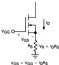
**FIGURE 6-26 — SOURCE RESISTOR SUPPLIES NEGATIVE FEEDBACK TO THE GATE**
