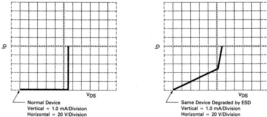
**FIGURE 3-1 — CURVE TRACER DRAWINGS OF A GOOD DEVICE AND A DEVICE WITH A DEGRADED GATE. DEVICE IS A 100 VOLT, 12 AMP POWER MOSFET**
