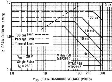
FIGURE 10 — MAXIMUM RATED SWITCHING SAFE OPERATING AREA
