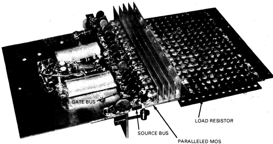
**FIGURE 6-37 — BREADBOARD LAYOUT OF THE SWITCH ILLUSTRATING TIGHT PACKAGING CONCEPTS**
