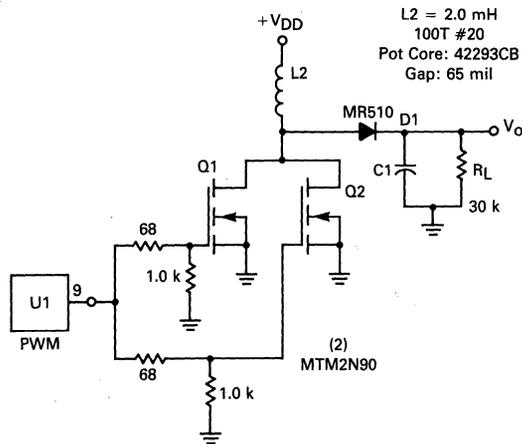
FIGURE 7-10b — TWO PARALLEL MOSFET OUTPUT
