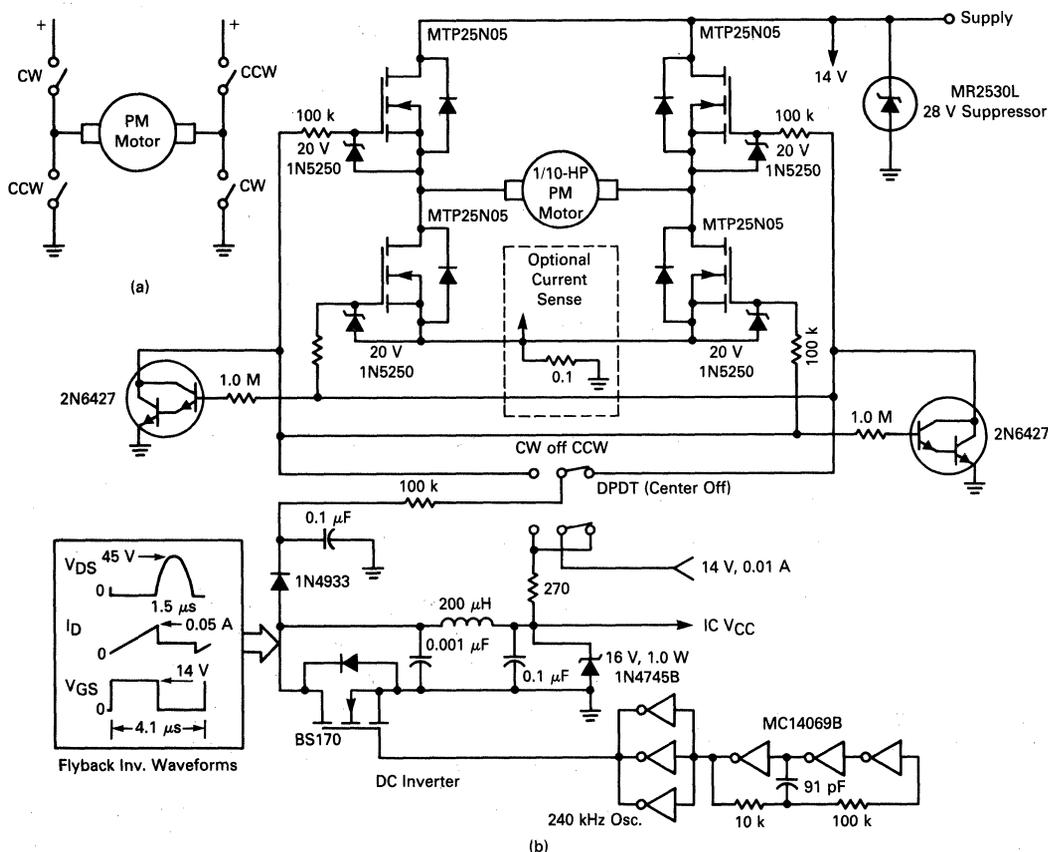
**FIGURE 7-29 — DRIVE FRACTIONAL-HORSEPOWER MOTORS EFFICIENTLY WITH THIS POWER-MOSFET H-BRIDGE CIRCUIT. IT DISSIPATES MUCH LESS POWER THAN A BIPOLAR-TRANSISTOR**
