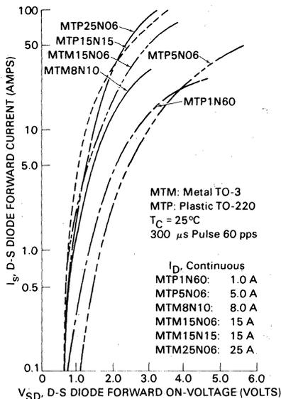
FIGURE 2-19 — FORWARD CHARACTERISTICS OF POWER MOSFETs D-S DIODES
