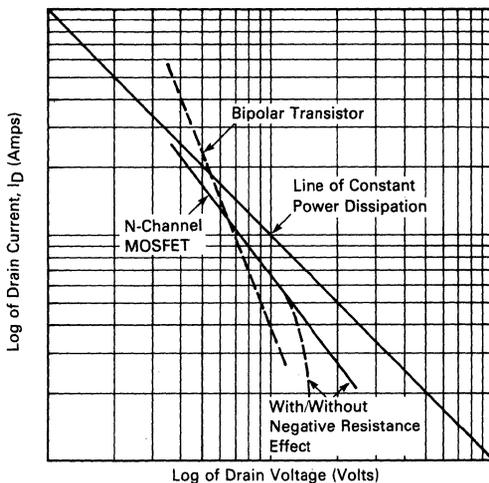
FIGURE 11-5 — COMPARISON OF TYPICAL FBSOA SLOPES
