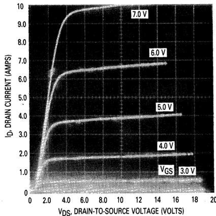
FIGURE 8-3b — OUTPUT CHARACTERISTICS OF GEMFET (MGP20N50)
