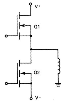
FIGURE 5-18 — TOTEM POLE NETWORK REQUIRES HIGH SIDE SWITCHING
