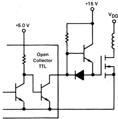
**FIGURE 5-7 — OPEN COLLECTOR TTL-TMOS INTERFACE FOR FASTER TURN-ON AND REDUCED POWER DISSIPATION**
