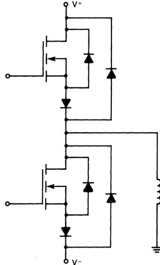
FIGURE 4-13 — CIRCUIT TO ELIMINATE CURRENT CONDUCTION IN THE MOSFET D-S DIODE
