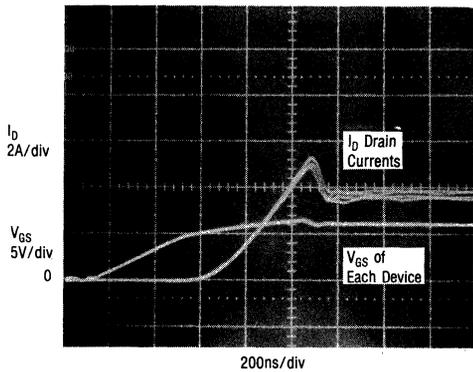
FIGURE 6-15a — PARALLELED TURN-ON
