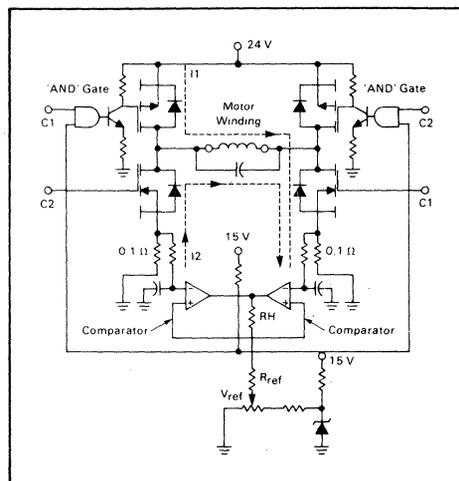
FIGURE 7-21 — HALF- OR FULL-STEP RESISTIVE CURRENT LIMITED DRIVE FOR STEPPING MOTORS WITHOUT CENTER-TAP
