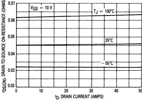
FIGURE 8 — ON-RESISTANCE versus DRAIN CURRENT
