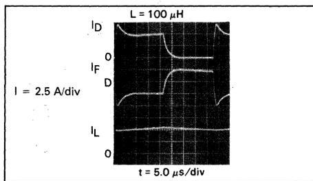
FIGURE 11-16 — SWITCHING CURRENTS OF A CLAMPED INDUCTIVE LOAD
