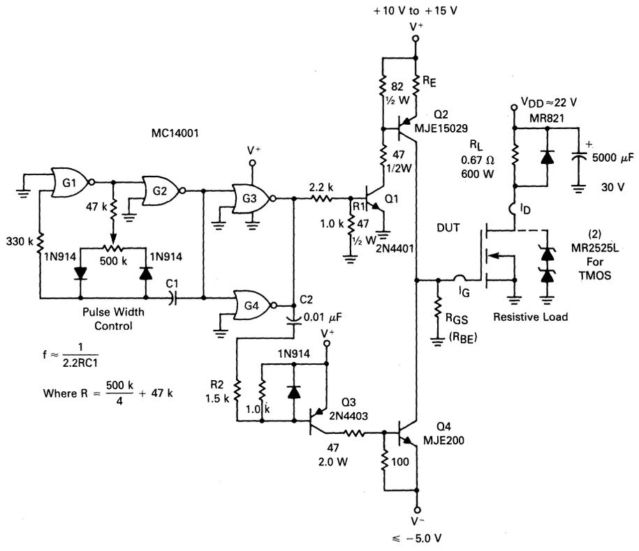
FIGURE 10-17 — TEST CIRCUIT FOR DRIVING DUTs
