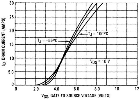
FIGURE 4 — TRANSFER CHARACTERISTICS
