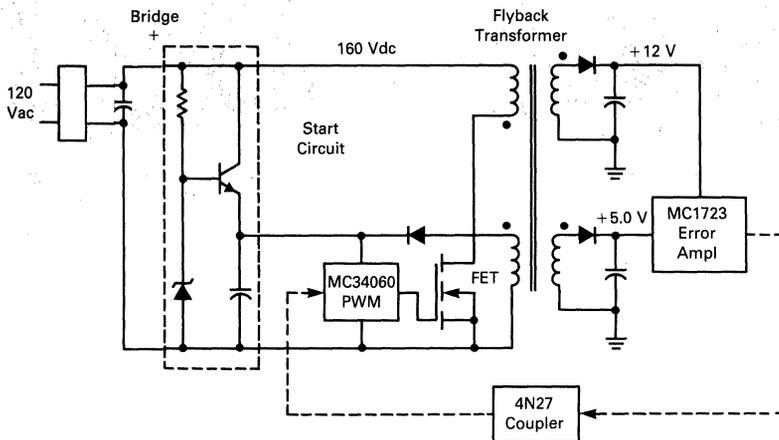
FIGURE 7-1 — REGULATOR BLOCK DIAGRAM
