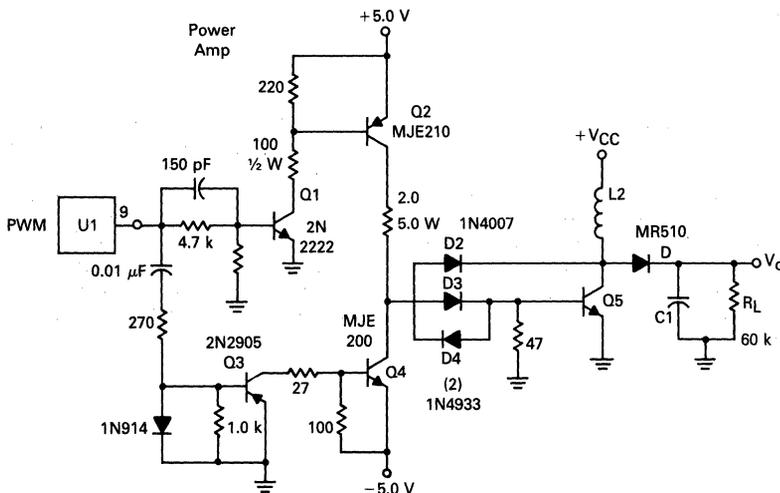
FIGURE 7-10c — DRIVER WITH BIPOLAR OUTPUT
