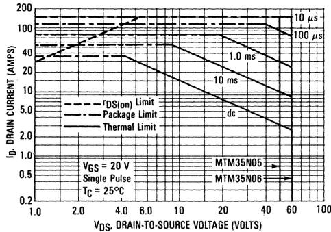
FIGURE 12 — MAXIMUM RATED SWITCHING SAFE OPERATING AREA
