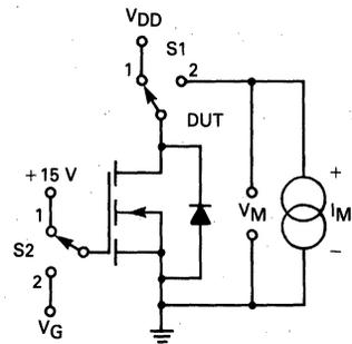
FIGURE 11-26c — DRAIN-SOURCE ON RESISTANCE
