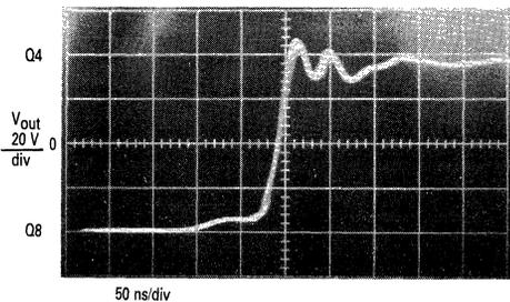
FIGURE 6-44 — NEGATIVE AND POSITIVE TRANSITION, DRAIN Q8, TURN-OFF CLAMP Q10 "ON"
