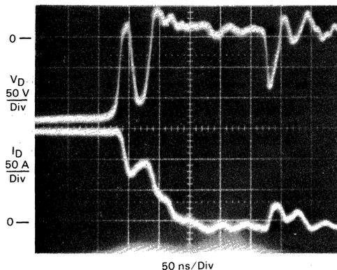
FIGURE 6-40 — TURN-OFF WITH CLAMP,  $R_D = 0$
