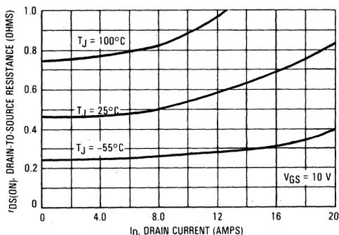
FIGURE 4-3 — ON-RESISTANCE versus DRAIN CURRENT FOR THE MTM8N40
