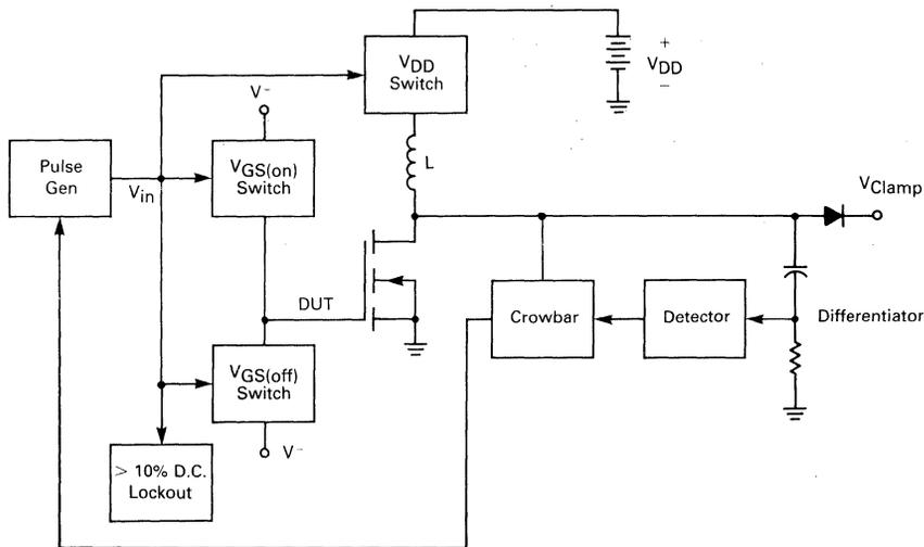
FIGURE 11-10 — BLOCK DIAGRAM OF THE N-CHANNEL NON-DESTRUCT TURN-OFF SWITCHING SOA TEST FIXTURE
