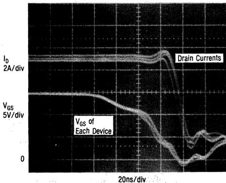
FIGURE 6-15c — PARALLELED TURN-OFF
