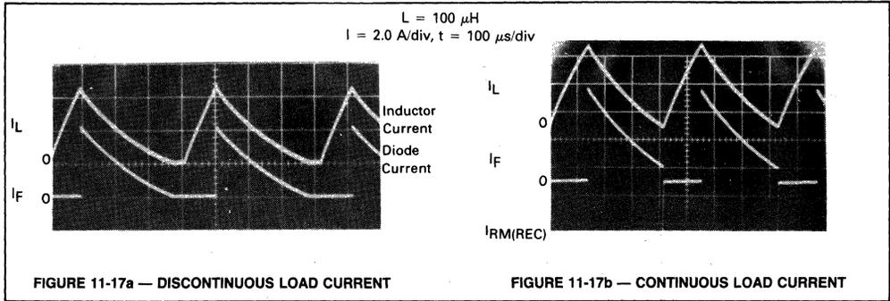
**FIGURE 11-17 — THE EFFECT OF SWITCHING INDUCTIVE LOAD CURRENT ON  $t_{tr}$  AND  $I_{RM(REC)}$  OF D-S DIODE**
