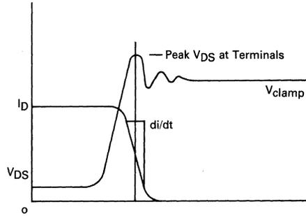
FIGURE 10-8 — CONDITION AT WHICH  $di/dt$ - $V_{DS}$  DERATING IS COMPUTED
