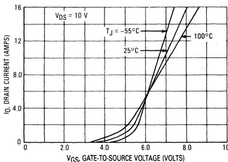
FIGURE 6-25 — TYPICAL TRANSCONDUCTANCE CURVES OF AN MTP8N20
