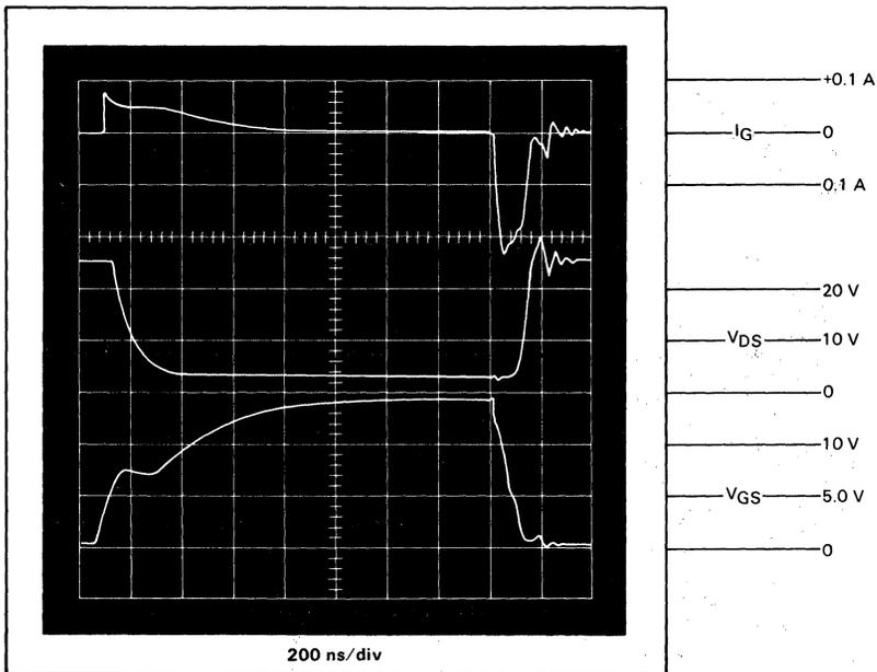
FIGURE 5-14 — POWER MOSFET SWITCHING WAVEFORMS
