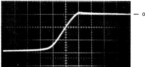
FIGURE 6-41a — TURN-OFF DRAIN VOLTAGE  $R_D = \infty$
