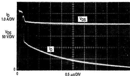
FIGURE 8-5 — CLAMPED INDUCTIVE TURN-OFF OF GEMFET
