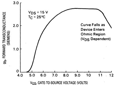
FIGURE 2-6 — SMALL-SIGNAL TRANSCONDUCTANCE versus  $V_{GS}$  OF MTP8N10
