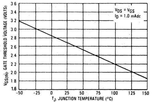
FIGURE 2-8 — GATE-THRESHOLD VOLTAGE VARIATION WITH TEMPERATURE
