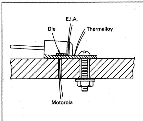
ratings are supposed to be based on this reference point. Unfortunately, the placement of the thermocouple is tedious and leaves the semiconductor in a condition unfit for sale.
