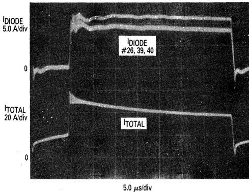
FIGURE 6-35 — DRAIN-SOURCE DIODE ON CHARACTERISTICS OF THREE MTM20N15s WITH MISMATCHED D-S DIODE ON-VOLTAGES
