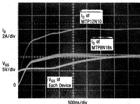
FIGURE 6-13a — PARALLELED TURN-ON
