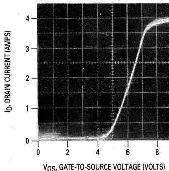
FIGURE 5-5 — TRANSFER CHARACTERISTICS OF AN MTP3N40
