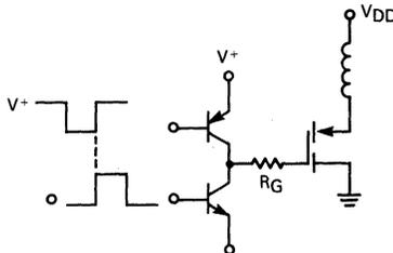
FIGURE 8-6 — CIRCUIT TO TEST VARIATIONS IN CURRENT FALL TIMES WITH CHANGES IN GATE DRIVE IMPEDANCE
