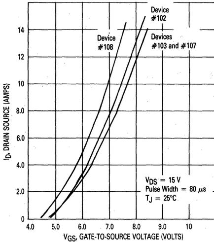
FIGURE 6-16 — WIDEST VARIATION IN TRANSCONDUCTANCE CURVES OF 250 ADDITIONAL MTP8N18s
