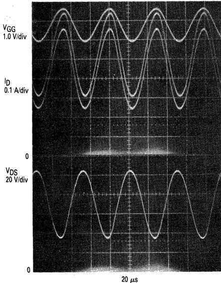
**FIGURE 6-30 —  $V_{GG}$ ,  $I_D$  AND  $V_{DS}$  WAVEFORMS OF MISMATCHED MTP8N20s PARALLELED IN THE LINEAR MODE  $R_S = 3.3 \Omega$**
