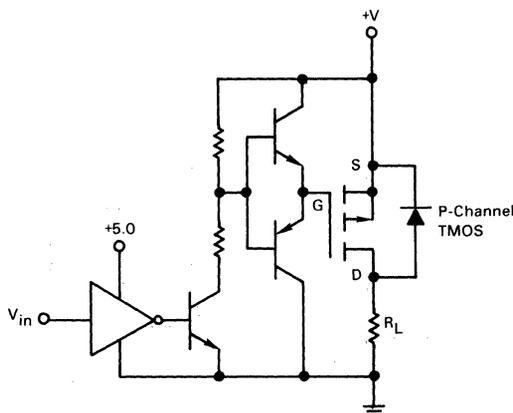
FIGURE 5-19 — LEVEL SHIFTER FOR P-CHANNEL MOSFET DRIVING A GROUNDED LOAD
