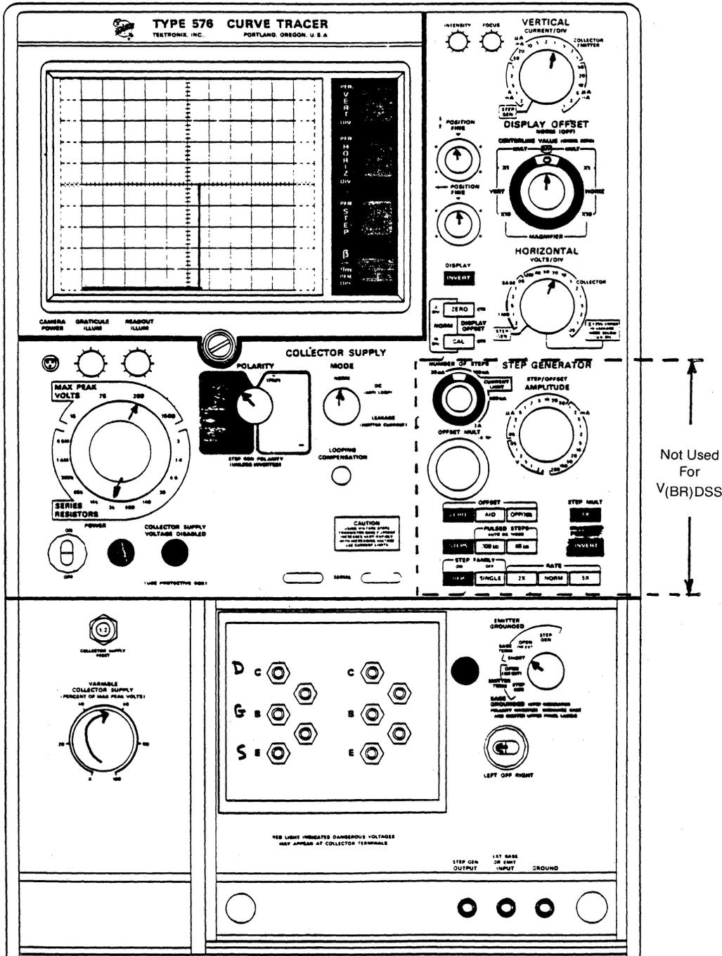
FIGURE 11-29 — TEST SET-UP CHART TYPE 576 FOR MEASURING POWER MOSFET PARAMETERS
