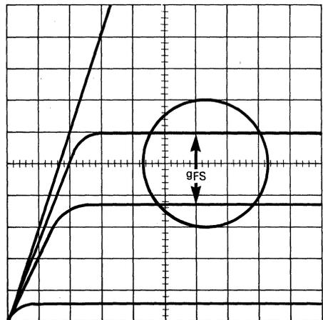
FIGURE 11-32 — CURVE TRACER FOR  $g_{fs}$
