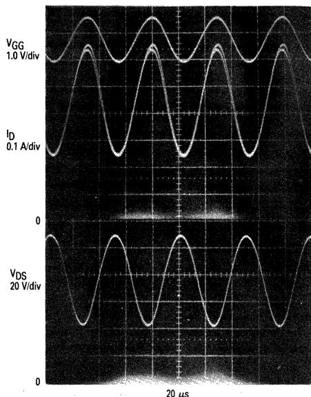
FIGURE 6-32 —  $V_{GG}$ ,  $I_D$  AND  $V_{DS}$  WAVEFORMS OF MATCHED MTP8N20s PARALLELED IN THE LINEAR MODE  $R_S = 3.3 \Omega$
