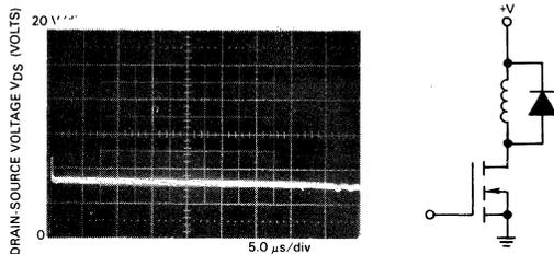
FIGURE 4-7 —  $V_{DS}$  TRANSIENT WITH CLAMPING DIODE
