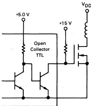
**FIGURE 5-6 — DRIVING TMOS WITH OPEN COLLECTOR TTL**
