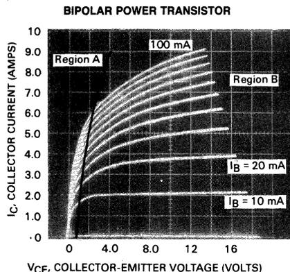
FIGURE 2-2 —  $I_C$ - $V_{CE}$  TRANSFER CHARACTERISTICS OF MJE15030 (NPN,  $I_C$  CONTINUOUS = 8.0 A,  $V_{CE0}$  = 150 V) REGION A IS THE SATURATION REGION. REGION B IS THE LINEAR OR ACTIVE REGION.
