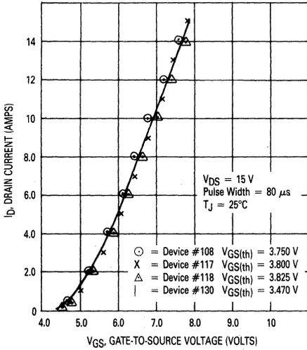
FIGURE 6-10 — TRANSCONDUCTANCE CURVES OF MTP8N18s WITH THRESHOLD VOLTAGE  $V_{GS(th)}$  MISMATCH
