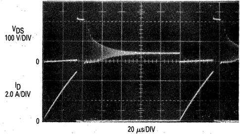
FIGURE 8-10b — CLAMPED INDUCTIVE SWITCHING WAVEFORMS AT 7.0 kHz — MOSFET
