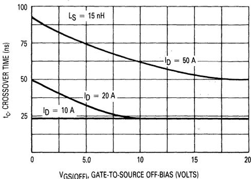
FIGURE 10-14 — Crossover Time versus Gate Off-Bias with Lower  $L_S$
