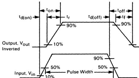
FIGURE 3 — OUTPUT CHARACTERISTICS
