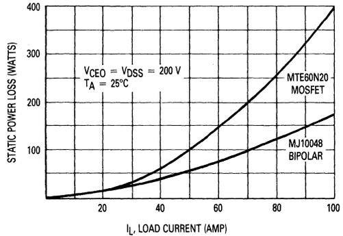
FIGURE 10-10 — STATIC POWER LOSSES OF 200 V MOSFET AND BIPOLARS
