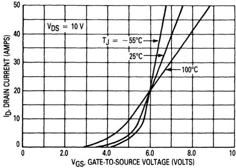
FIGURE 6 — TRANSFER CHARACTERISTICS
