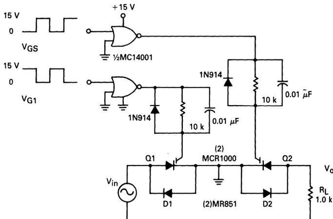
FIGURE 8-31 — BIDIRECTIONAL POWER SWITCH USING TWO MOS SCRs
