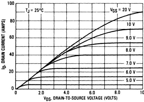
FIGURE 5 — TRANSFER CHARACTERISTICS
