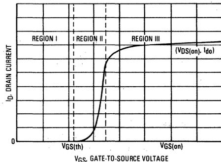
FIGURE 5-2 — TYPICAL POWER MOSFET TRANSFER FUNCTION
