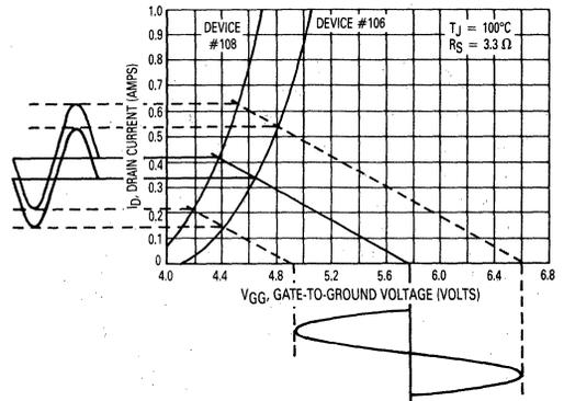
**FIGURE 6-31 — TRANSFER CHARACTERISTICS AND  $R_S$  LOADLINE OF MISMATCHED MTP8N18s**
