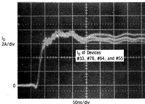
FIGURE 6-6a — PARALLELED TURN-ON
