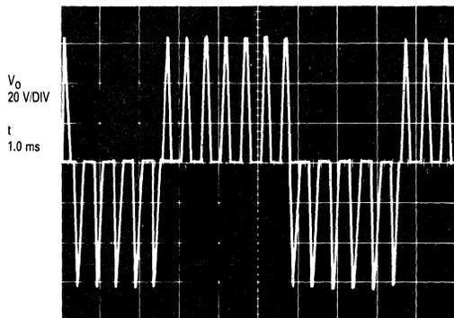
FIGURE 8-32 — 2.0 kHz SIGNAL GATED BY 200 Hz
