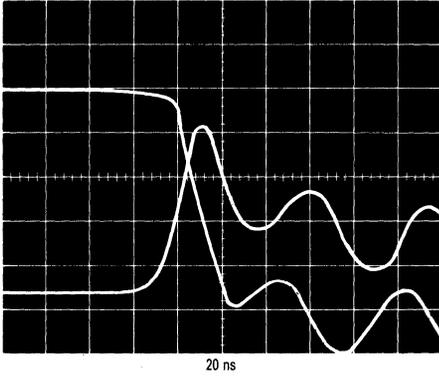
FIGURE 10-6a — DRAIN CURRENT AND DRAIN-SOURCE VOLTAGE APPEARING AT TERMINALS — MTE60N20 — OFF BIAS = -4.0 VOLTS
