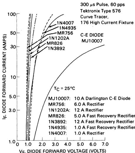
FIGURE 11-23 — FORWARD CHARACTERISTICS OF DISCRETE RECTIFIERS
