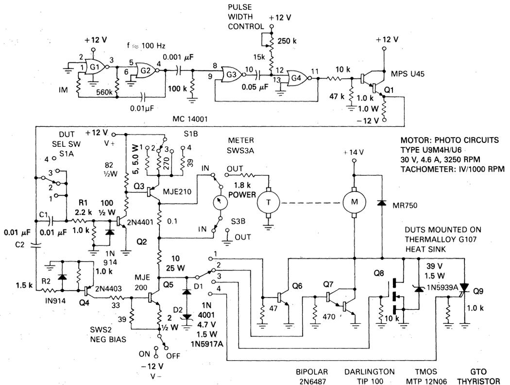
FIGURE 9-9 — TEST CIRCUIT FOR MEASURING RELATIVE EFFICIENCY OF DUT
