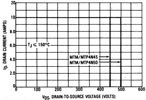
FIGURE 2-14 — MAXIMUM RATED SWITCHING SAFE OPERATING AREA
