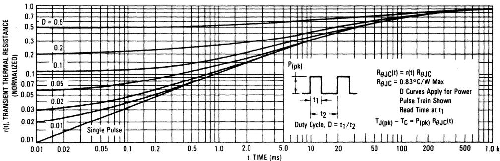
FIGURE 4-2 — THERMAL RESPONSE CURVE OF THE MTM8N40
