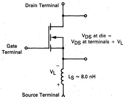
FIGURE 4-11 — VERY RAPID TURN-OFF INCREASES DRAIN-SOURCE VOLTAGE STRESS
