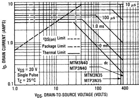
FIGURE 10 — MAXIMUM RATED SWITCHING SAFE OPERATING AREA
