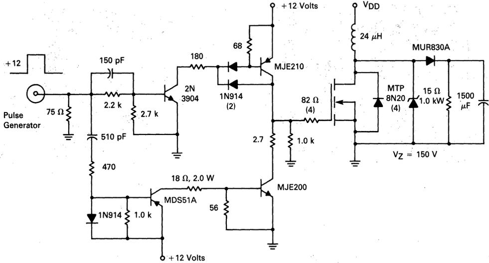
FIGURE 6-21 — CURRENT SHARING TEST CIRCUIT WITH AN INDUCTIVE LOAD
