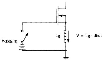
FIGURE 10-13 — PARASITIC SOURCE INDUCTANCE
