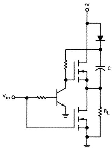
FIGURE 5-23 — BOOTSTRAPPING CIRCUIT TO DRIVE A GROUNDED LOAD WITH N-CHANNEL TMOS
