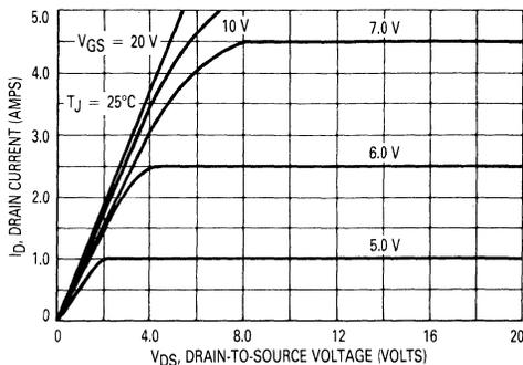
FIGURE 6 — TRANSFER CHARACTERISTICS
