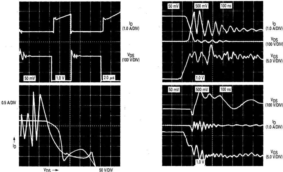
**FIGURE 7-2 — FET WAVEFORMS — 120 Vac, FULL LOAD**
