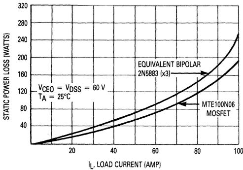
FIGURE 10-9 — STATIC POWER LOSS OF 60 V MOSFET AND EQUIVALENT BIPOLARS
