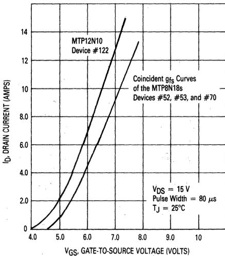
FIGURE 6-11 — TRANSCONDUCTANCE CURVES OF AN MTP12N10 AND THREE MTP8N18s
