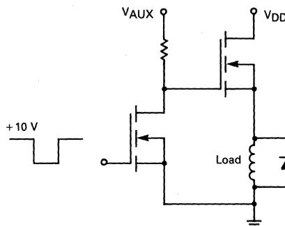
FIGURE 5-20 — HIGH SIDE SWITCHING USING AN AUXILIARY SUPPLY
