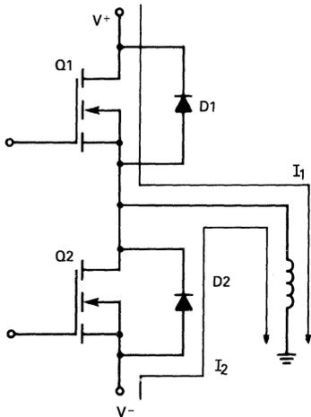
FIGURE 4-12 — TOTEM POLE CIRCUIT IN WHICH  $dv/dt$  MAY BE CONCERN
