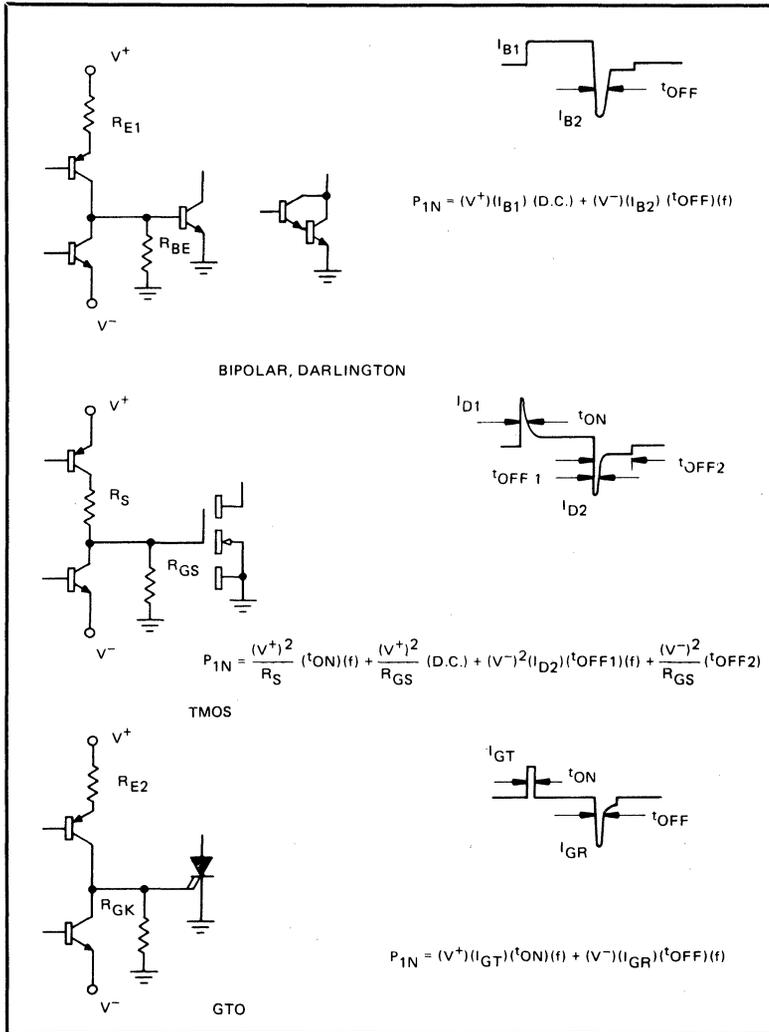
FIGURE 9-10 — DUT DRIVE AND INPUT POWER CALCULATION
