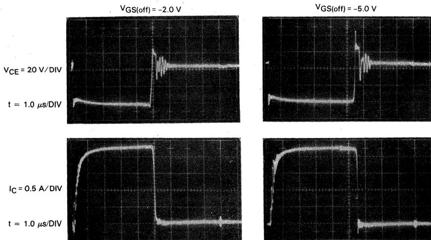
FIGURE 9-4 — RESISTIVE LOAD SWITCHING OF SWITCHMODE III MJ16004 AT TWO OFF-BIAS VOLTAGES
