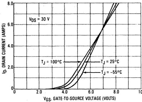
FIGURE 2-7 — TRANSFER CHARACTERISTICS
