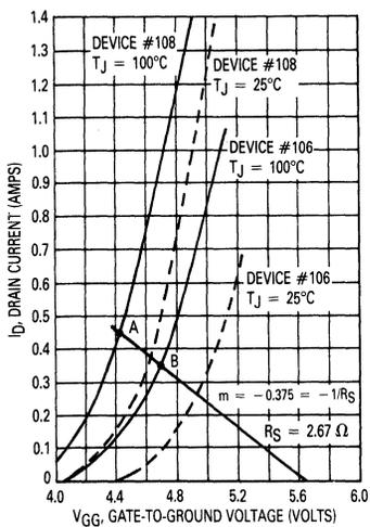
FIGURE 6-28 — USING A SOURCE RESISTOR TO STABILIZE THE QUIESCENT OPERATING POINT
