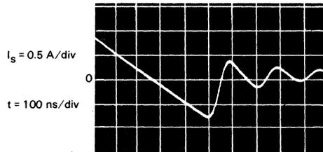
FIGURE 2-20 — REVERSE RECOVERY CHARACTERISTICS OF MTM15N15 DRAIN-SOURCE DIODE
