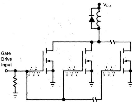
FIGURE 6-19 — METHOD FOR DRIVING PARALLELED MOSFETs USING GATE DECOUPLING RESISTORS
