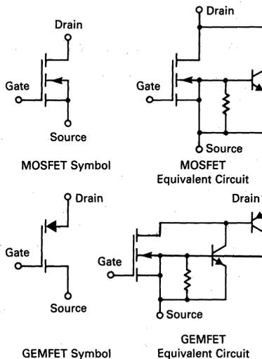
FIGURE 8-2 — MOSFET AND GEMFET SYMBOLS AND EQUIVALENT CIRCUITS
