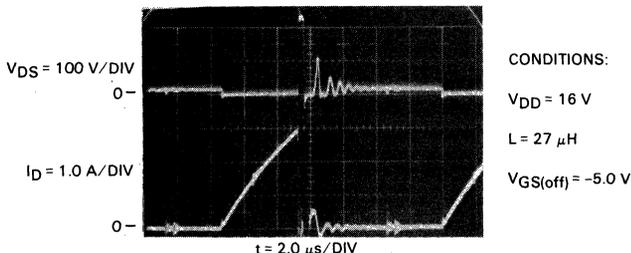
FIGURE 9-6 — CLAMPED INDUCTIVE LOAD SWITCHING WAVEFORMS OF TMOS MTM5N40
