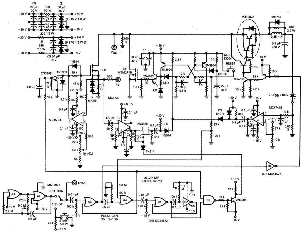
FIGURE 11-2 — P-CHANNEL POWER MOSFET NON-DESTRUCT FBSOA TESTER
