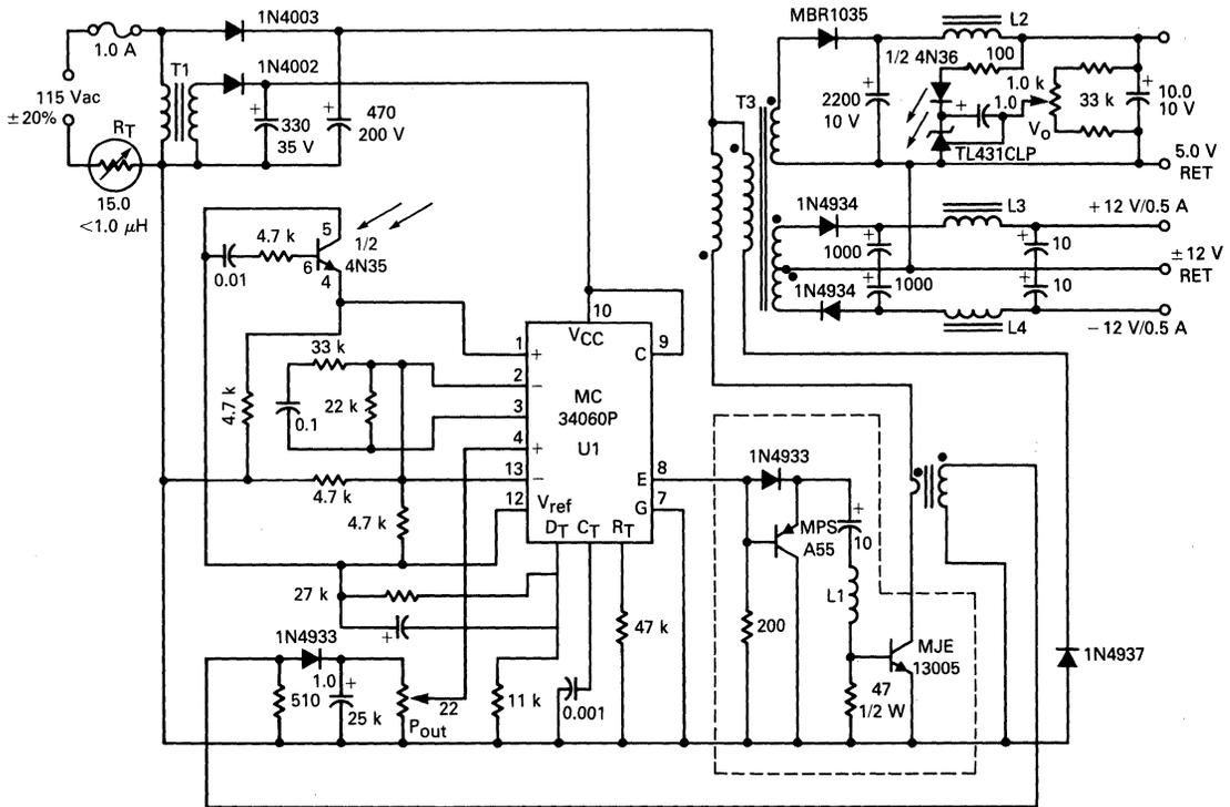
FIGURE 7-5 — 20 kHz SWITCHING POWER SUPPLY USING A BIPOLAR SWITCH
