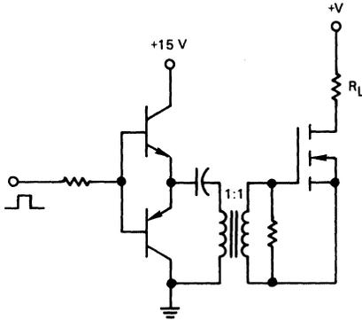
FIGURE 5-10 — CIRCUIT TO ELIMINATE THE VARYING OF  $I_m$  WITH PULSE WIDTH
