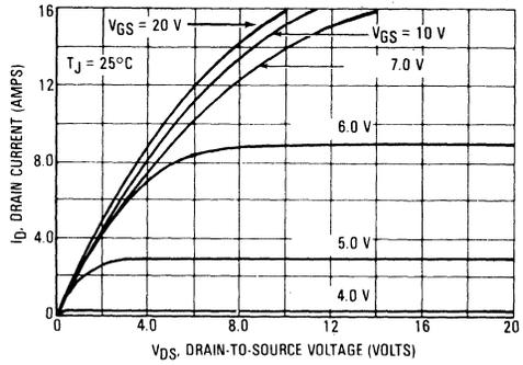
FIGURE 4 — TRANSFER CHARACTERISTICS
