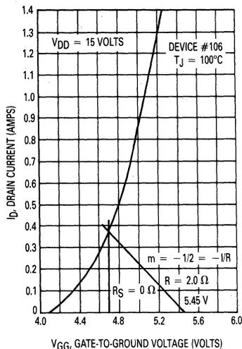
**FIGURE 6-27 — GRAPHICAL METHOD OF PREDICTING THE EFFECT OF A SOURCE RESISTOR ON THE QUIESCENT OPERATING POINT**
