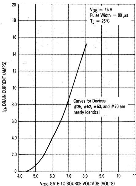
FIGURE 6-3 — TRANSCONDUCTANCE CURVES OF MATCHED MTP8N18s
