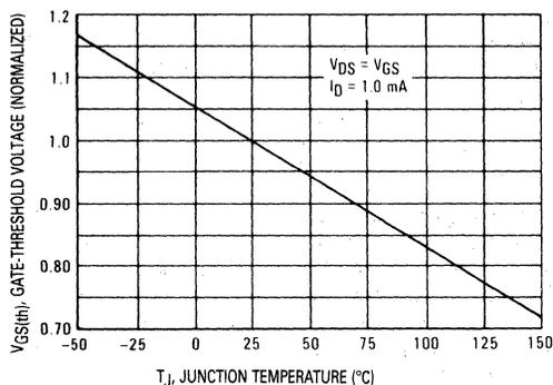
FIGURE 2-16 — GATE-THRESHOLD VOLTAGE VARIATION WITH TEMPERATURE
