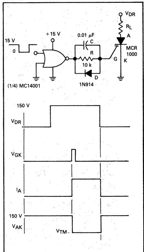
FIGURE 8-24 — PREFERRED CMOS DRIVE CIRCUIT AND WAVEFORMS
