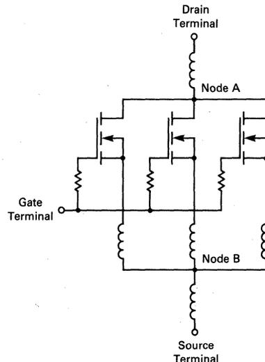
FIGURE 10-5 — INTERNAL CIRCUIT ELEMENTS OF MEDIUM CURRENT POWER MOSFET
