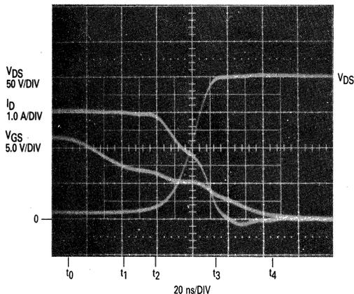
FIGURE 5-4 — CLAMPED INDUCTIVE TURN-OFF WAVEFORMS OF AN MTP3N40
