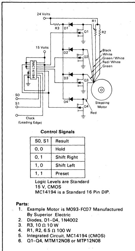
FIGURE 7-19 — CENTER-TAPPED STEPPING MOTOR DRIVE
