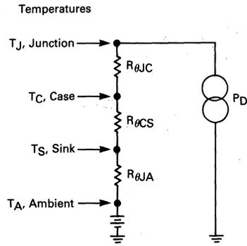
FIGURE 11-25 — BASIC THERMAL RESISTANCE MODEL SHOWING THERMAL TO ELECTRICAL ANALOGY FOR A SEMICONDUCTOR
