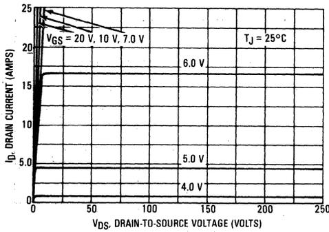
FIGURE 4 — ON CHARACTERISTICS
