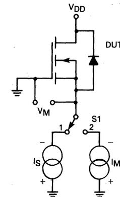
FIGURE 11-26b — GATE-SOURCE THRESHOLD VOLTAGE
