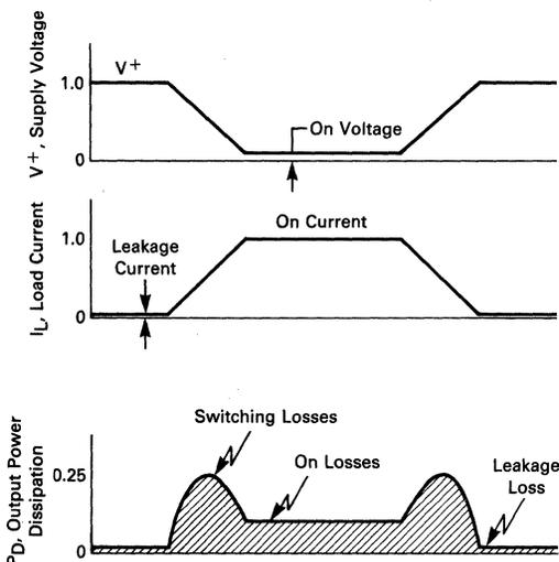
FIGURE 9-1 — NORMALIZED SWITCHING WAVEFORMS FOR A RESISTIVE LOAD
