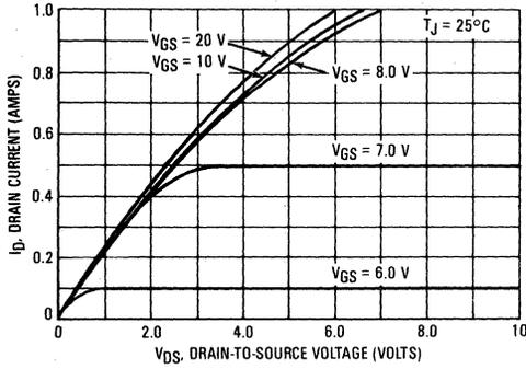
FIGURE 4 — TRANSFER CHARACTERISTICS
