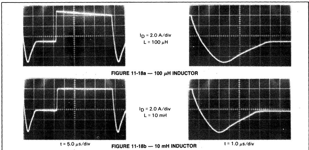
**FIGURE 11-18 — THE EFFECTS OF LOAD INDUCTANCE ON D-S DIODE REVERSE RECOVERY CHARACTERISTICS**
