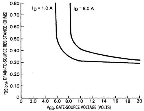
FIGURE 2-4 — VARIATION OF  $r_{DS(on)}$  WITH  $V_{GS}$  AND  $I_D$  FOR MTP8N15 POWER MOSFET
