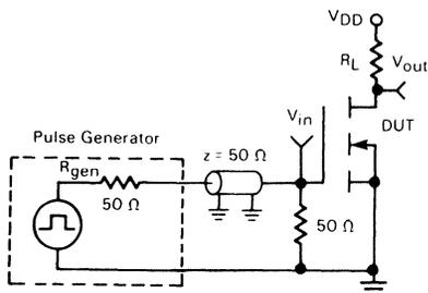
FIGURE 2-10 — SWITCHING TEST CIRCUIT
