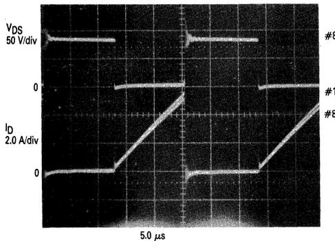
FIGURE 6-22 —  $I_D$  WAVEFORMS OF LOW AND HIGH  $r_{DS(on)}$  DEVICES — INDUCTIVE LOAD
