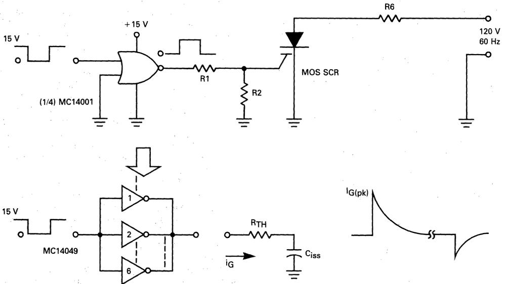
FIGURE 8-20 — EXAMPLES OF INDIVIDUAL OR PARALLEL CONNECTED CMOS DRIVERS FOR MOS SCR
