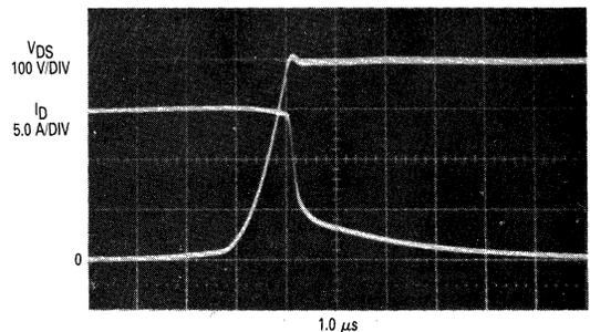
FIGURE 8-16b — CLAMPED INDUCTIVE TURN-OFF WAVEFORMS OF MGM20N50 —  $R_{GS} = 51 \Omega$
