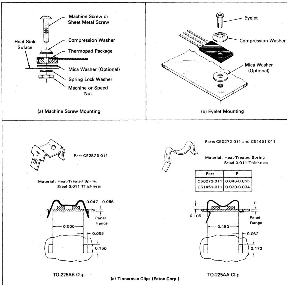
FIGURE 13-7 — RECOMMENDED MOUNTING ARRANGEMENTS FOR TO-225AA (TO-126)
