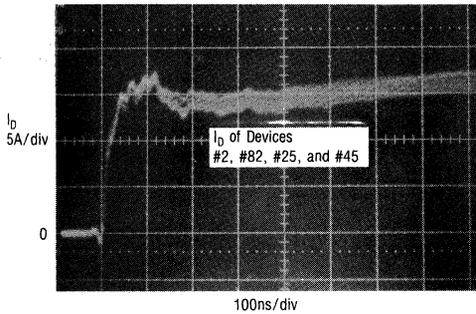
FIGURE 6-7a — PARALLELED TURN-ON
