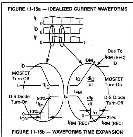
FIGURE 11-15 — CONTINUOUS LOAD CURRENT SWITCHING WAVEFORMS
