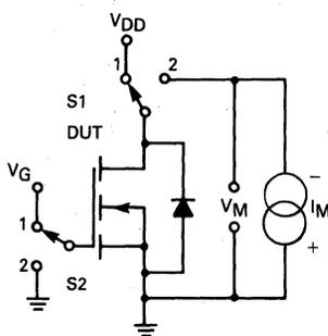
FIGURE 11-26a — DRAIN-SOURCE DIODE VOLTAGE
