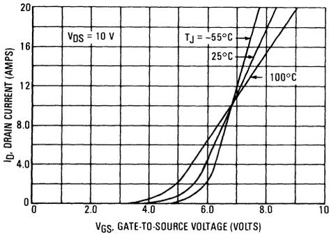
FIGURE 4 — TRANSFER CHARACTERISTICS
