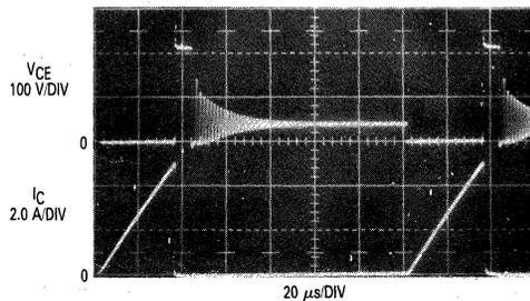
FIGURE 8-10c — CLAMPED INDUCTIVE SWITCHING WAVEFORMS AT 7.0 kHz — BIPOLAR
