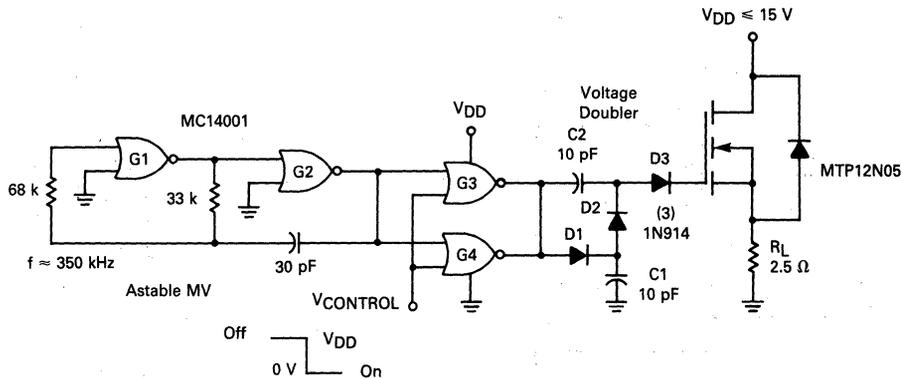
FIGURE 5-24 — N-CHANNEL SOURCE FOLLOWER WITH VOLTAGE DOUBLER DRIVE
