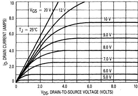
FIGURE 6 — TRANSFER CHARACTERISTICS
