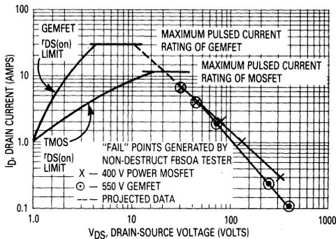
FIGURE 8-12 — COMPARISON OF FBSOA CURVES OF A 400 V MOSFET AND 550 V GEMFET OF EQUAL DIE AREA
