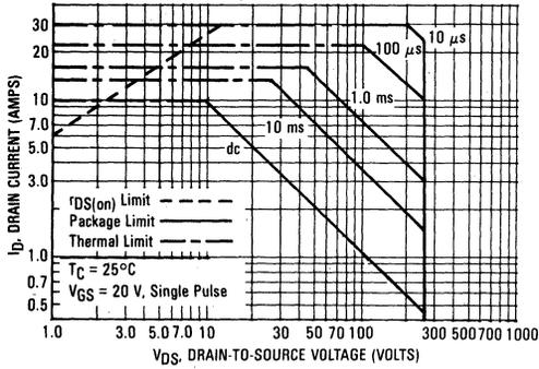
FIGURE 10 — MAXIMUM RATED SWITCHING SAFE OPERATING AREA
