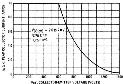
FIGURE 7-11a — RBSOA, REVERSE BIAS SWITCHING SAFE OPERATING AREA
