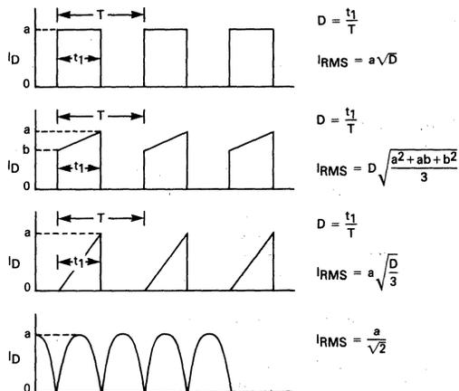
FIGURE 4-4 — RMS VALUES OF SOME COMMON CURRENT WAVEFORMS
