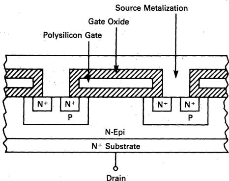
FIGURE 8-1a — CROSS SECTION OF TMOS CELL
