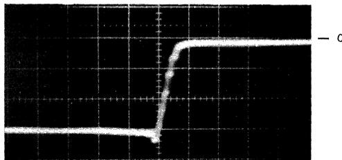
FIGURE 6-41b — TURN-OFF DRAIN VOLTAGE  $R_D = 10 \Omega$
