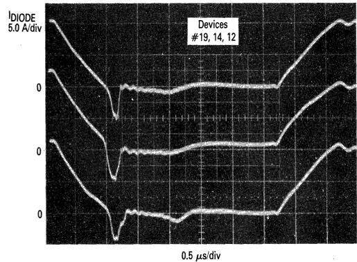
FIGURE 6-36 — PARALLELED DIODE TURN-ON AND TURN-OFF OF MTM15N20s WITH MISMATCHED  $t_{tr}$
