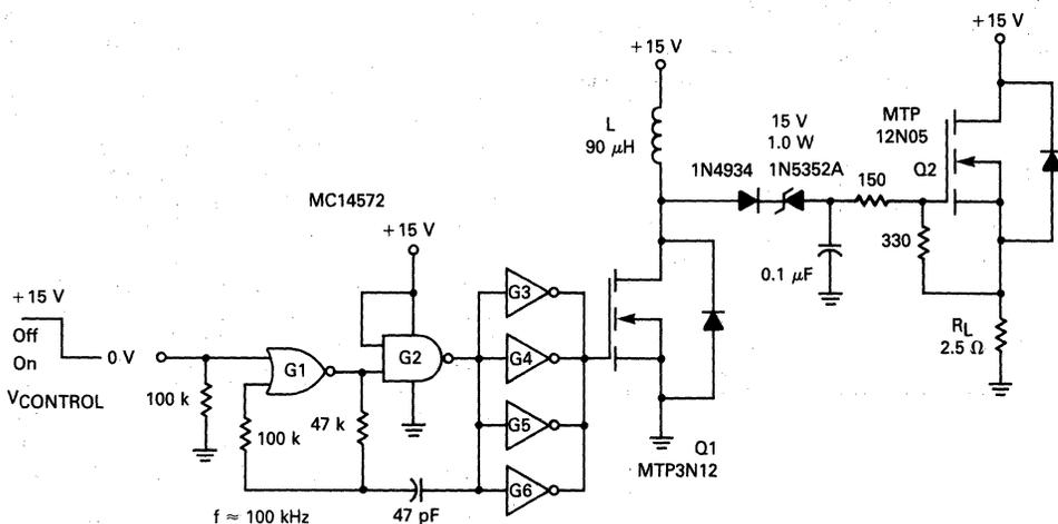
FIGURE 5-25 — N-CHANNEL SOURCE FOLLOWER WITH FLYBACK CONVERTER DRIVE
