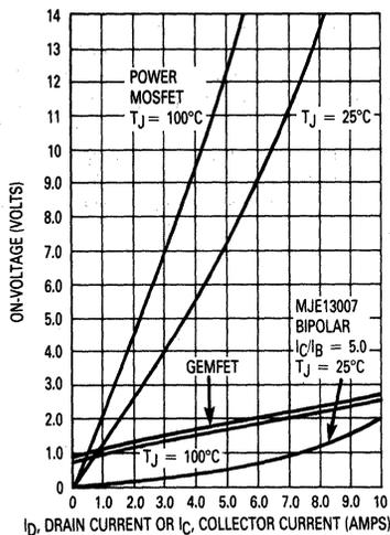
**FIGURE 8-7 — ON-VOLTAGE versus DRAIN OR COLLECTOR CURRENT FOR A GEMFET, MOSFET AND BIPOLAR OF EQUIVALENT DIE SIZE**
