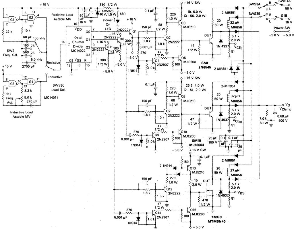
FIGURE 9-2 — TEMPERATURE RISE FIXTURE SWITCHMODE I, SWITCHMODE III, TMOS
