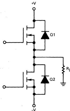
FIGURE 2-21 — TMOS TOTEM POLE NETWORK WITH INTEGRAL DRAIN-SOURCE DIODES
