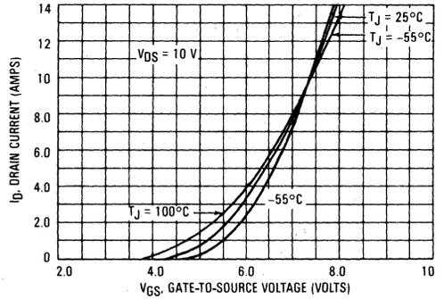
FIGURE 7 — ON-VOLTAGE VARIATION versus TEMPERATURE
