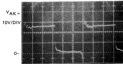
FIGURE 9-12b — GTO ANODE-CATHODE VOLTAGE
