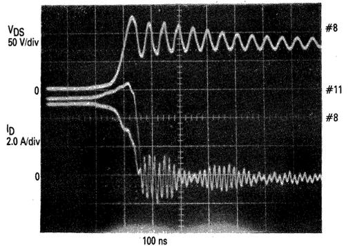
FIGURE 6-23 —  $I_D$  TURN-OFF WAVEFORMS OF LOW AND HIGH  $r_{DS(on)}$  DEVICES — INDUCTIVE LOAD
