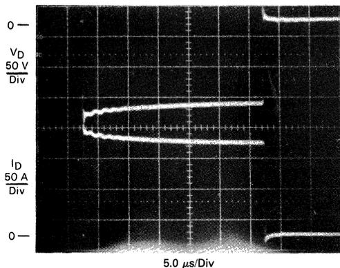
FIGURE 6-38 — SWITCHED VOLTAGE AND CURRENT
