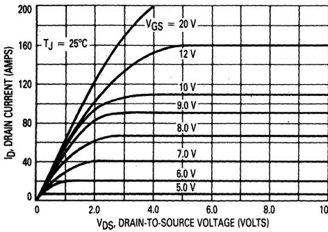
FIGURE 5 — TRANSFER CHARACTERISTICS
