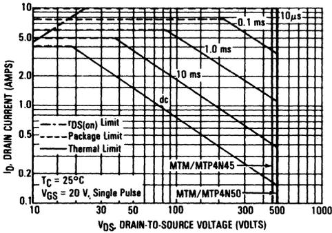
FIGURE 2-13 — MAXIMUM RATED FORWARD BIASED SAFE OPERATING AREA
