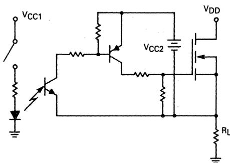
FIGURE 5-22 — DRIVING A SOURCE FOLLOWER WITH AN OPTOCOUPLER
