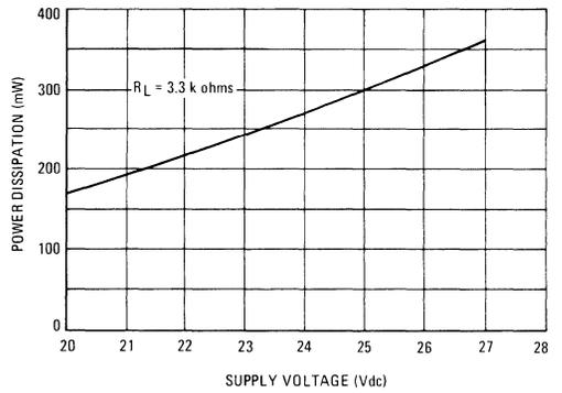
FIGURE 10 – POWER DISSIPATION
