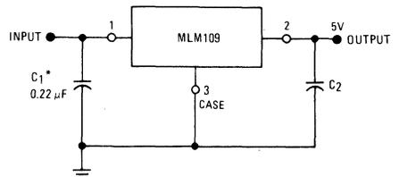
\* Required if regulator is located an appreciable distance from power supply filter. Although no output capacitor is needed for stability, it does improve transient response.
