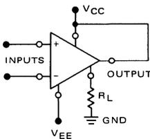
Input polarity is reversed when GND pin is used as an output.
