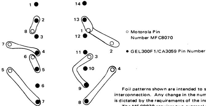
Foil patterns shown are intended to show pin-for-pin interconnection. Any change in the number of components is dictated by the requirements of the individual design. The MFC8070 requires two external reference resistors; one resistor between pin 3 and pin 5 and the other between pin 3 and pin 8.
