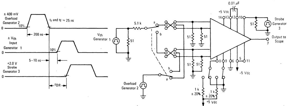
(Pin numbers shown on this page denote the pin numbers for the flat package only; to ascertain the corresponding pin numbers for the dual in-line package, refer to the circuit schematic on the second page.)
