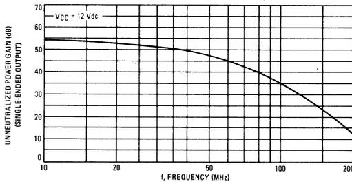
FIGURE 2 – VOLTAGE GAIN versus FREQUENCY
