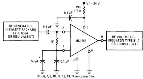
FIGURE 12 – AM REJECTION, DETECTED AUDIO, THD, ATTENUATION TEST CIRCUIT
