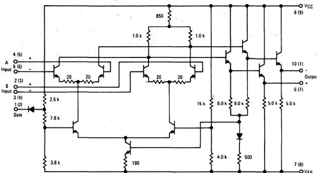
Number in parenthesis denotes pin for F and L packages, number at left in each case denotes corresponding pin for G package.
