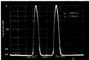
FIGURE 2 - AMPLITUDE-MODULATION OUTPUT WAVEFORM
