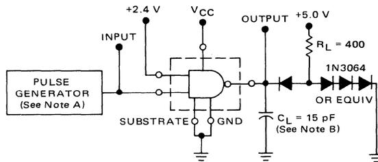
NOTES: A. The pulse generator has the following characteristics:  $t_w = 0.5 \mu s$ ,  $PRR = 1.0 \text{ MHz}$ ,  $z_o \approx 50 \Omega$ .
