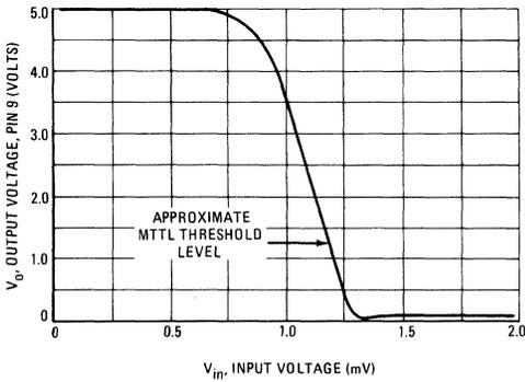
FIGURE 18 – STROBE TO OUTPUT TRANSFER CHARACTERISTICS
