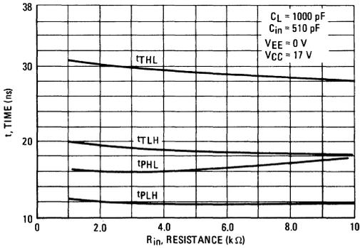
**FIGURE 14 – DC-COUPLED SWITCHING versus  $C_{in}$  (See Figure 4.)**
