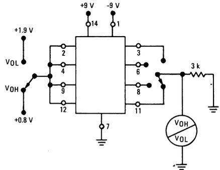
FIGURE 3 – OUTPUT SHORT-CIRCUIT CURRENT
