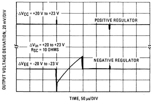
FIGURE 16 – RIPPLE REJECTION
