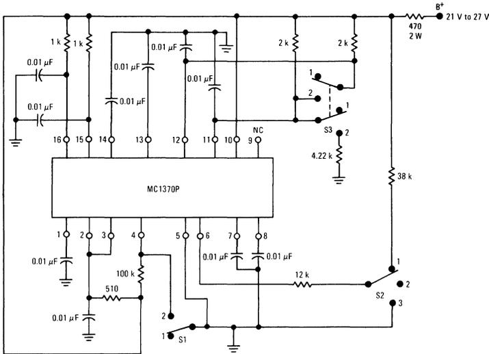
FIGURE 3 – DYNAMIC CHARACTERISTICS TEST CIRCUIT
