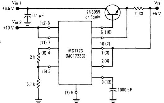
FIGURE 20 – +15 V, 1-AMPERE REGULATOR WITH REMOTE SENSE
