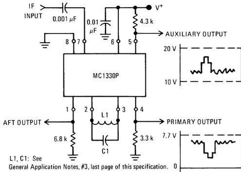
FIGURE 5 – OUTPUT VOLTAGE
