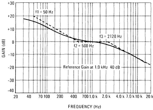
for RIAA equalization. Figure 12 illustrates the RIAA response of the amplifier in Figure 11. The dashed line shows the ideal response with the corner frequencies indicated. The lower corner frequency ( $f_1$ ) is determined by the input capacitance  $C_1$  and the equation
