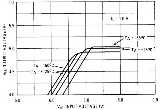
FIGURE 11 – OUTPUT VOLTAGE
