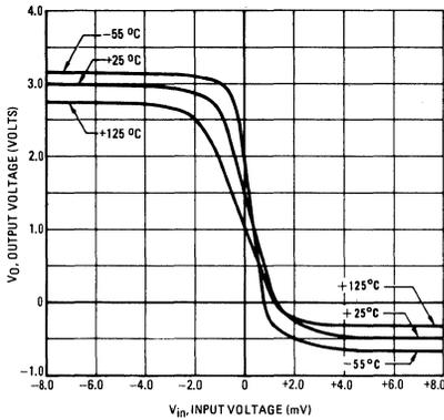
FIGURE 2 - INPUT OFFSET VOLTAGE versus TEMPERATURE
