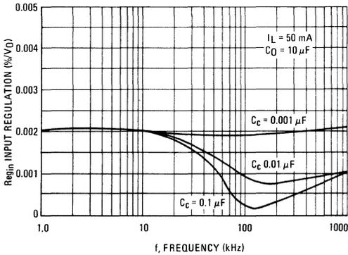
**FIGURE 16 – FREQUENCY DEPENDENCE OF INPUT REGULATION, C<sub>O</sub> = 2.0 μF**
