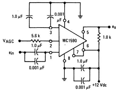
FIGURE 18 – 30-MHz AMPLIFIER (Power Gain = 50 dB, BW ≈ 1.0 MHz)
