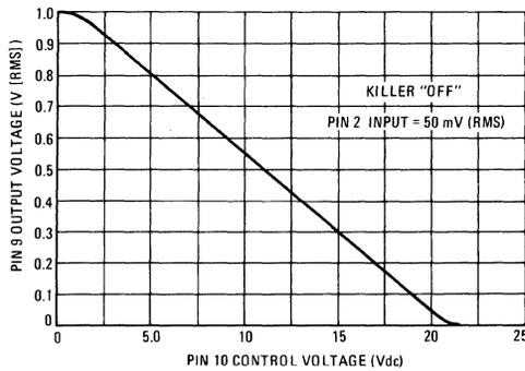
FIGURE 4 – FIRST STAGE GAIN WITH ACC BIAS
