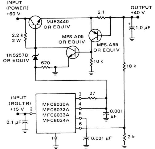
FIGURE 14 – 5.0-VOLT, 5.0-AMPERE REGULATOR with
