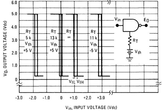
FIGURE 9 – MC1489A INPUT THRESHOLD VOLTAGE ADJUSTMENT
