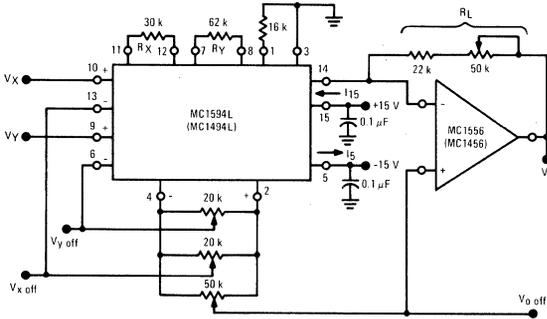
FIGURE 4 - INPUT BIAS CURRENT/INPUT OFFSET CURRENT, OUTPUT RESISTANCE
