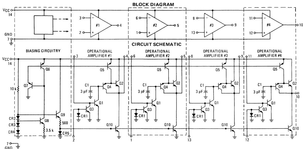
A noninverting input is obtained by adding a current mirror as shown in Figure 17. Essentially all current which enters the non-inverting input,  $I_{in2}$ , flows through the diode CR1. The voltage drop across CR1 corresponds to this input current magnitude and this same voltage is applied to a matched device, Q3. Thus Q3 is biased to conduct an emitter current equal to  $I_{in2}$ . Since the
