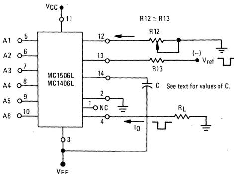
FIGURE 8 – REFERENCE CURRENT SLEW RATE MEASUREMENT TEST CIRCUIT
