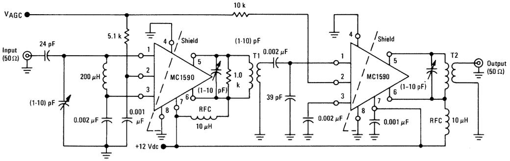
T1: Primary Winding = 15 Turns, #22 AWG Wire, 1/4" ID Air Core
