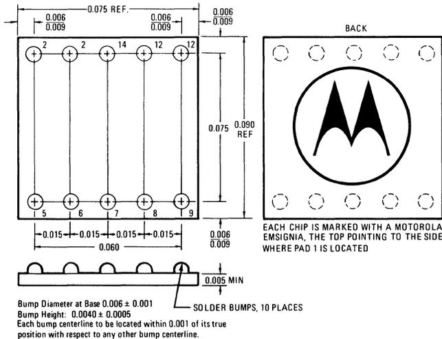
The popular 1558 type dual operational amplifier is now available in three chip forms: 1) conventional chips, 2) beam-lead chips and 3) flip-chips, as well as in a variety of plastic and hermetic packages. The flip-chip consists of a silicon chip with solder bumps on the geometry surface to provide easy mechanical mounting and electrical connection. These devices are protected by a thin layer of phosphorsilicate passivation which covers the interconnect metalization and active areas of the die.
