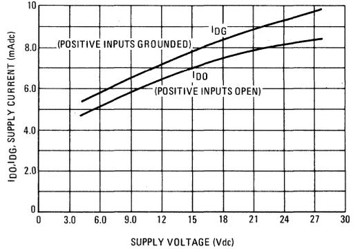
**FIGURE 13 – LINEAR SOURCE CURRENT versus SUPPLY VOLTAGE**
