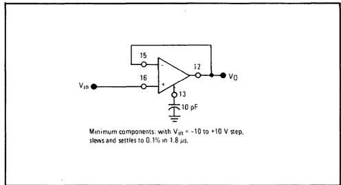
FIGURE 16 – VOLTAGE GAIN = +1
