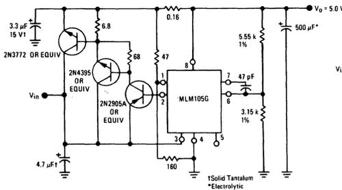
**FIGURE 3 - 1.0 A REGULATOR with PROTECTIVE DIODES**
