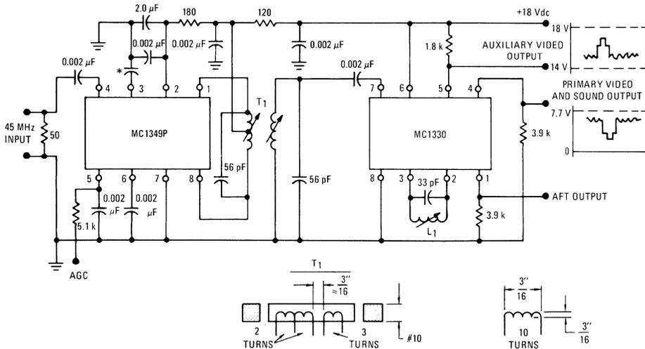
All windings #22 AWG tinned nylon acetate wire tuned with Coilcraft #61 slugs, size 10-32, or equivalent.
