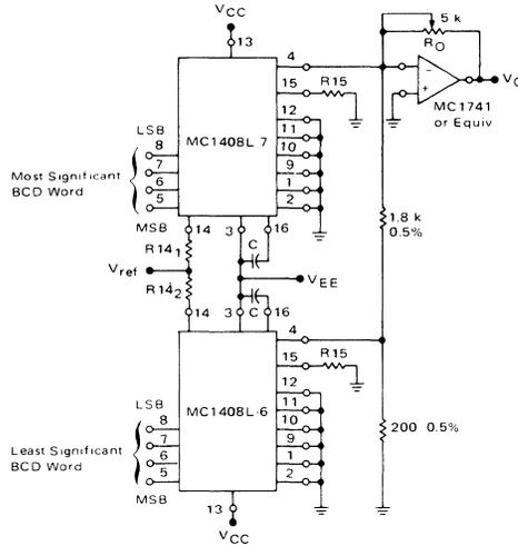
Two 8-bit, D-to-A converters can be used to build a two digit BCD D-to-A or A-to-D converter. If both outputs feed the virtual ground of an operational amplifier, 10:1 current scaling can be achieved with a resistive current divider. If current output is desired, the units may be operated at full scale current levels of
