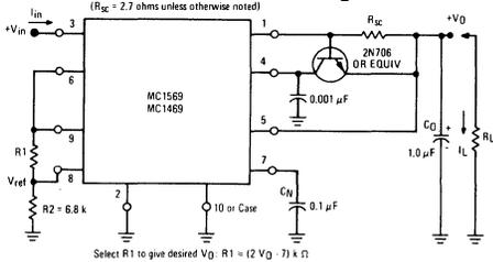
FIGURE 5 - CONNECTION FOR  $2.5 \text{ Vdc} \geq V_O \geq 3.5 \text{ Vdc}$
