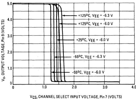
FIGURE 20 – CHANNEL SELECT B to OUTPUT TRANSFER CHARACTERISTICS
