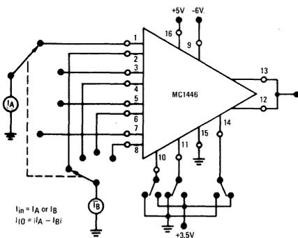
FIGURE 4 – CHANNEL SELECT AND STROBE INPUT CURRENTS
