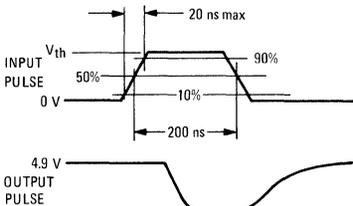
(c) Waveforms for Propagation Delay Test
