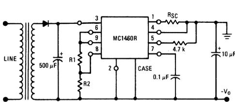
FIGURE 27 – DIGITALLY CONTROLLED 3-TERMINAL NEGATIVE REGULATOR
