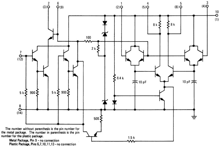
The number without parenthesis is the pin number for the metal package. The number in parenthesis is the pin number for the plastic package.
