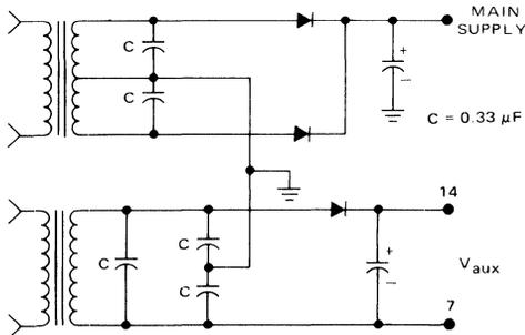
FIGURE 19 - FULL-WAVE RECTIFICATION WITH TRANSIENT SUPPRESSION
