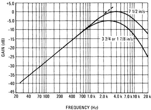
FIGURE 9 – TAPE RECORD AMPLIFIER RESPONSE
