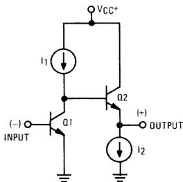
FIGURE 17 – OBTAINING A NONINVERTING INPUT
