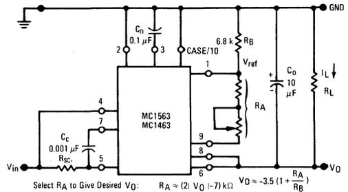
FIGURE 10 –  $R_A$  versus  $V_O$
