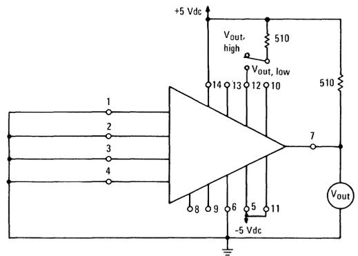
FIGURE 11 – MINIMUM TIME FROM CHANNEL GATE INPUT TO AMPLIFIER INPUT PROPAGATION DELAY FROM CHANNEL GATE INPUT TO AMPLIFIER OUTPUT
