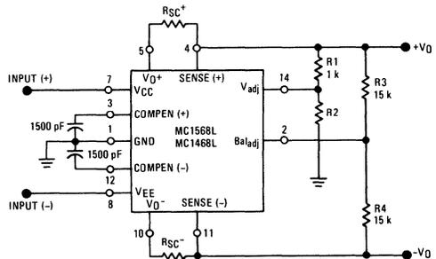
The presence of the Baladj, pin 2, on devices housed in the dual in-line package (L suffix) allows the user to adjust the output voltages down to  $\pm 8.0 \text{ V}$ . The required value of resistor R2 can be calculated from
