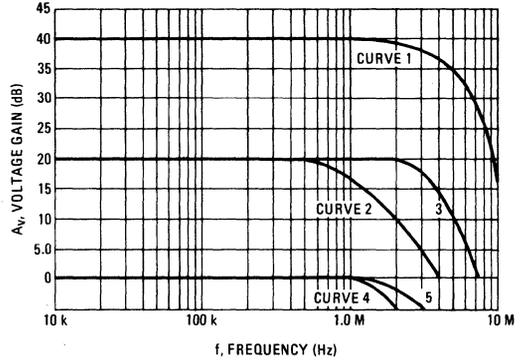
FIGURE 7 – MC1531/MC1431 VOLTAGE GAIN versus FREQUENCY
