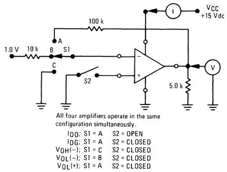
FIGURE 7 – INPUT BIAS CURRENT AND CURRENT MIRROR GAIN
