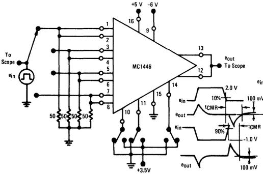
**FIGURE 8 – CIRCUIT PROPAGATION DELAY, OUTPUT RISE AND FALL TIMES, AND DIFFERENTIAL-MODE RECOVERY TIME**
