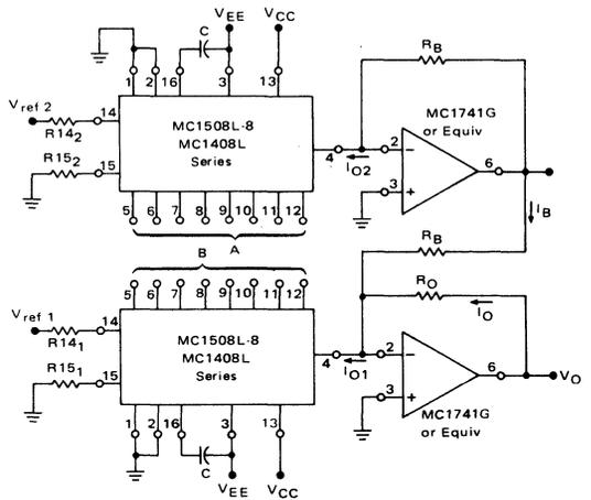
$$I_O = I_{O1} - I_{O2} = \frac{V_{ref1}}{R_{141}} \{A\} - \frac{V_{ref2}}{R_{142}} \{B\}$$
