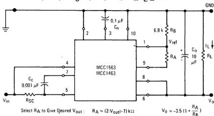
**FIGURE 2 - TYPICAL NPN CURRENT BOOST CONNECTION**
