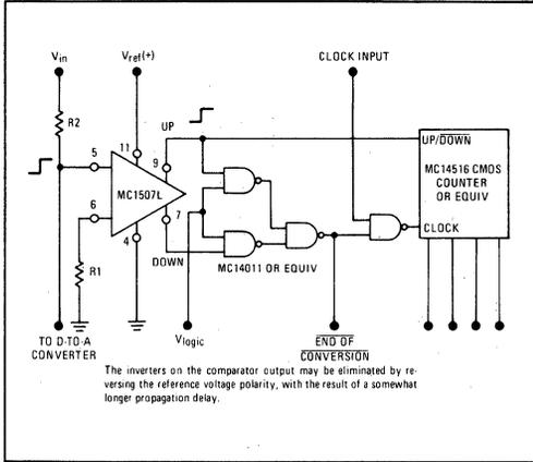
FIGURE 43 – BIPOLAR INPUT
