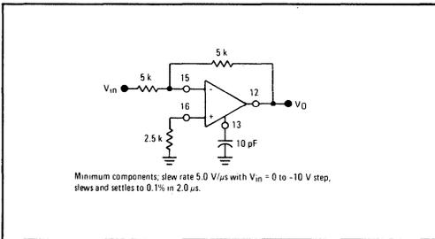
FIGURE 15 – VOLTAGE GAIN = -1
