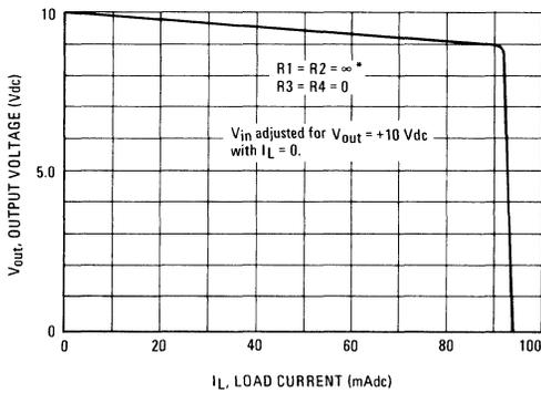
FIGURE 9 – NEGATIVE OUTPUT VOLTAGE SWING versus LOAD CURRENT
