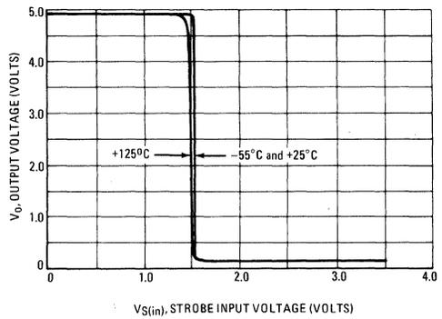
FIGURE 19 – CHANNEL SELECT A to OUTPUT TRANSFER CHARACTERISTICS
