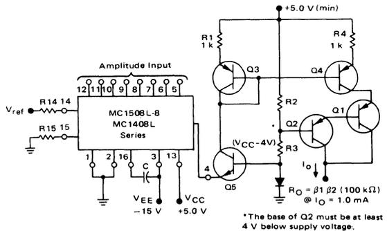
Current pulses, ramps, staircases, and sine waves may be generated by the appropriate digital and reference inputs. This circuit is especially useful in curve tracer applications.
