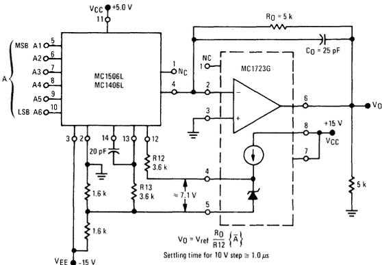
$$V_O = V_{ref} \left( \frac{R_O}{R_{12}} \right) \left( \bar{A}_1 \right)$$
