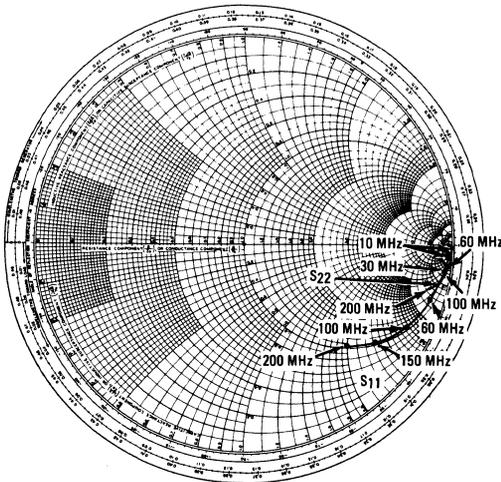
FIGURE 13 –  $S_{11}$ , and  $S_{22}$ , INPUT AND OUTPUT REFLECTION COEFFICIENT
