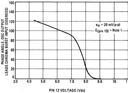
**FIGURE 7 – OSCILLATOR OUTPUT versus PIN 12 VOLTAGE**
