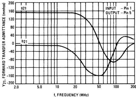
FIGURE 11 –  $Y_{21}$ , FORWARD TRANSFER ADMITTANCE, POLAR FORM
