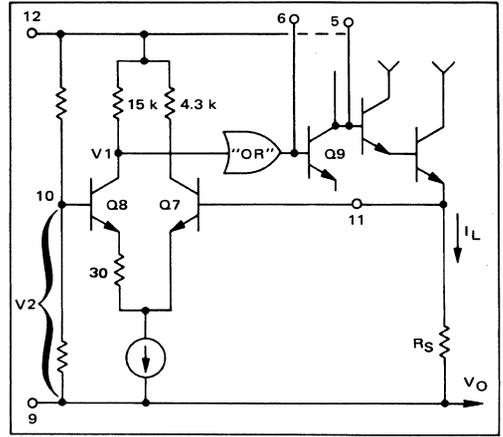
This level is further boosted by the output stage such that in the constant voltage mode overall transconductance is about 300 mA/volt.
