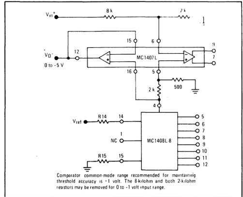
Comparator common-mode range recommended for maintaining threshold accuracy is -1 volt. The 8-kilohm and both 2-kilohm resistors may be removed for 0 to -1 volt input range.
