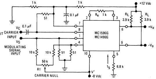
**FIGURE 28 – AM MODULATOR CIRCUIT**
