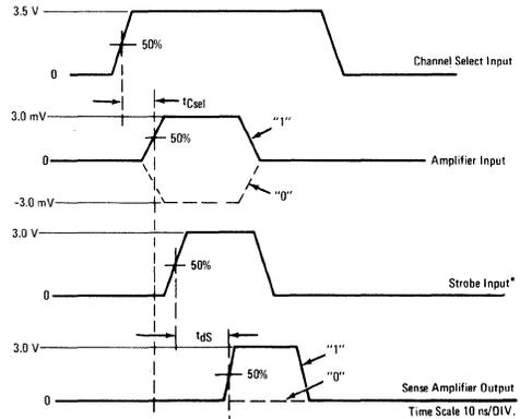
\*The strobe pulse width is smaller than the amplifier input pulse width.
