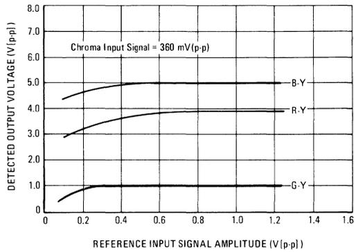
FIGURE 4 – DETECTED OUTPUT VOLTAGE
