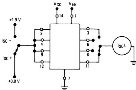
FIGURE 4 – OUTPUT RESISTANCE (POWER-OFF)
