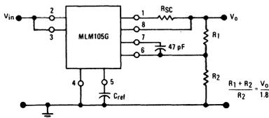
**FIGURE 2 - 10 A REGULATOR with FOLDBACK CURRENT LIMITING**
