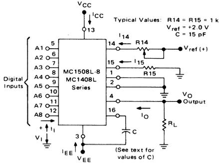
$V_I$  and  $I_I$  apply to inputs A1 thru A8
