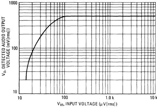
FIGURE 3 – DETECTED AUDIO OUTPUT versus INPUT LEVEL @  $f = 5.5$  MHz,  $\pm 50$  kHz DEVIATION
