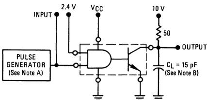
NOTES: A. Pulse generator characteristics:  $t_w = 0.5 \mu s$ , PRR = 1.0 MHz,  $z_0 \approx 50 \Omega$ .
