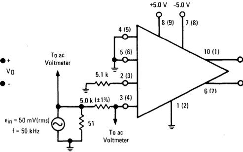
FIGURE 15 – OUTPUT IMPEDANCE TEST CIRCUIT
