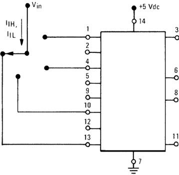
FIGURE 2 – OUTPUT VOLTAGE and INPUT THRESHOLD VOLTAGE
