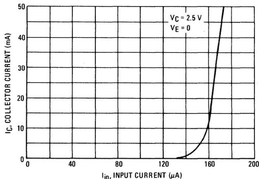
FIGURE 4 – OUTPUT CURRENT versus INPUT CURRENT
