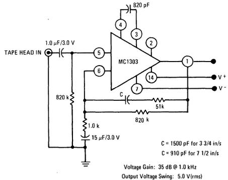
Voltage Gain: 35 dB @ 1.0 kHz
