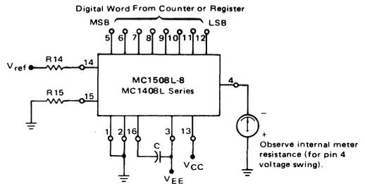
FIGURE 27 - DC COUPLED DIGITAL ATTENUATOR and DIGITAL SUBTRACTION
