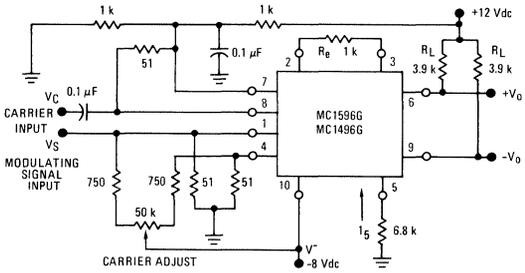
**FIGURE 29 – PRODUCT DETECTOR (+12 Vdc SINGLE SUPPLY)**
