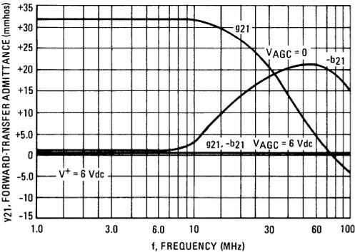
FIGURE 15 –  $y_{21}$ , FORWARD-TRANSFER ADMITTANCE versus AGC VOLTAGE
