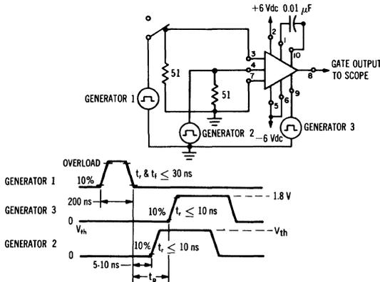
Pin numbers shown for devices in flat package and metal can. See block diagram for dual in-line package pin numbers.
