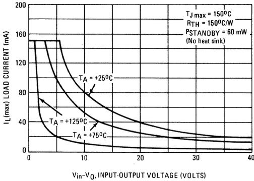
FIGURE 5 – LOAD REGULATION CHARACTERISTICS WITHOUT CURRENT LIMITING
