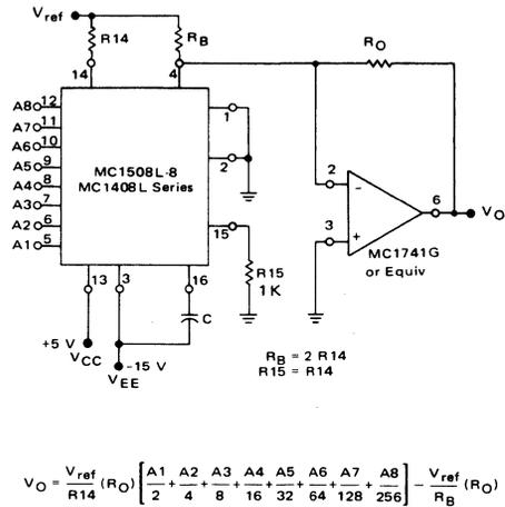
FIGURE 23 — BIPOLAR OR INVERTED NEGATIVE OUTPUT VOLTAGE CIRCUIT
