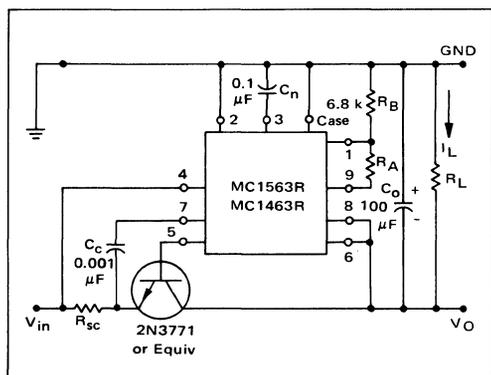
FIGURE 26 – Typical NPN Current Boost Connection
