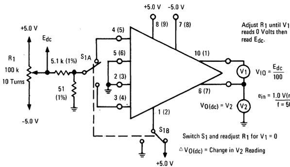
FIGURE 18 – GATE CURRENT (HIGH AND LOW), COMMON-MODE REJECTION AND COMMON-MODE INPUT RANGE TEST CIRCUIT
