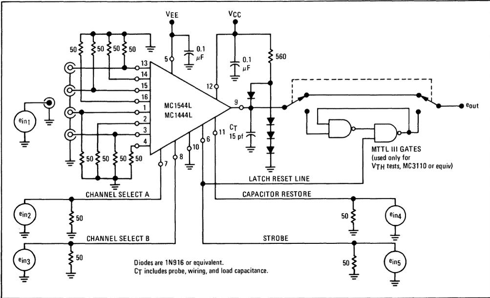
FIGURE 4 – THRESHOLD VOLTAGE TEST
