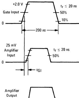
(C) Propagation Delay from Channel Gate Input to Amplifier Output
