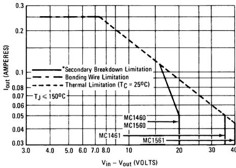
FIGURE 15b - DC SAFE OPERATING AREA ("R" PACKAGE)
