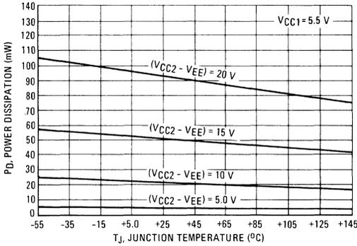
FIGURE 11 – MAXIMUM POWER DISSIPATION OF INTERNAL RESISTOR (R3)
