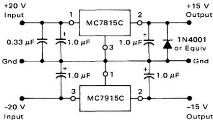
The MC7815 and MC7915 positive and negative regulators may be connected as shown to obtain a dual power supply for operational amplifiers. A clamp diode should be used at the output of the MC7815 to prevent potential latch-up problems.
