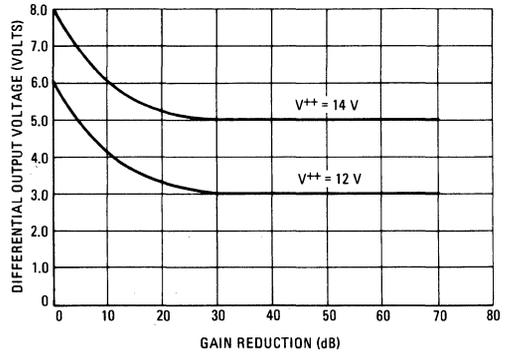
**FIGURE 10 – MC1352 AGC CHARACTERISTICS**
