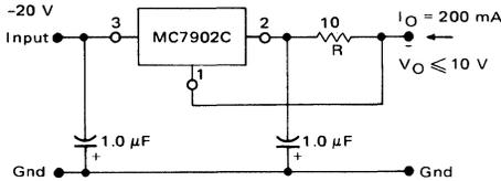
The MC7902, -2.0 V regulator can be used as a constant current source when connected as above. The output current is the sum of resistor R current and quiescent bias current as follows:
