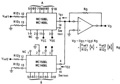
$$V_0 = I_0(1 + I_0/2) R_0$$
