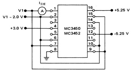
Channel A(-) shown under test, other channels are tested similarly. Devices are tested with V1 from +3.0 V to -3.0 V.
