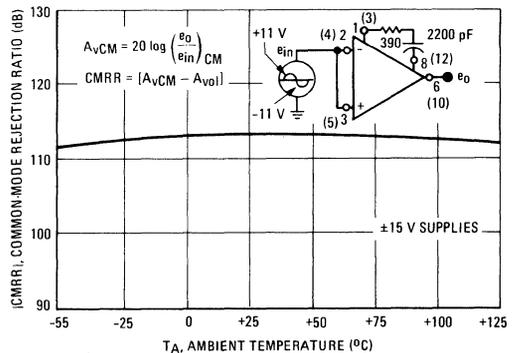
Pin numbers adjacent to terminals apply to 8-pin packages, number in parenthesis apply to 14-pin packages.
