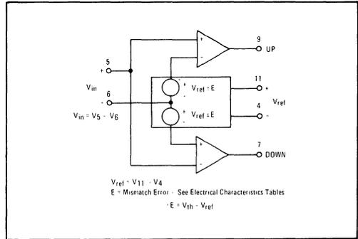
FIGURE 20 — COMPARATOR TRANSFER CHARACTERISTIC, NEGATIVE REFERENCE VOLTAGE
