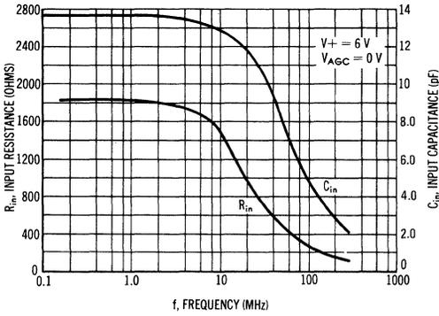
FIGURE 6 – INPUT RESISTANCE AND CAPACITANCE versus AGC VOLTAGE
