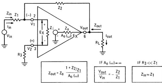
FIGURE 13 – NON-INVERTING FEEDBACK MODEL
