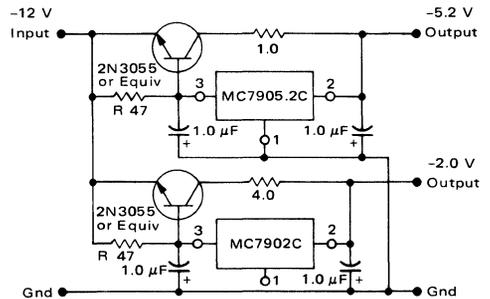
When current-boost power transistors are used, 47-ohm base-to-emitter resistors (R) must be used to bypass the quiescent current at no load. These resistors, in conjunction with the V<sub>BE</sub> of the NPN transistors, determine when the pass transistors begin conducting. The 1-ohm and 4-ohm dropping resistors were chosen to reduce the power dissipated in the boost transistors but still leave at least 2.0 V across these devices for good regulation.
