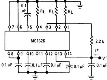
FIGURE 3 — DC OUTPUT VOLTAGE TEST CIRCUIT WITH NORMAL REFERENCE INPUT VOLTAGE (B, R, AND G)
