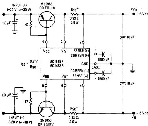
FIGURE 4 - OUTPUT VOLTAGE ADJUSTMENT
