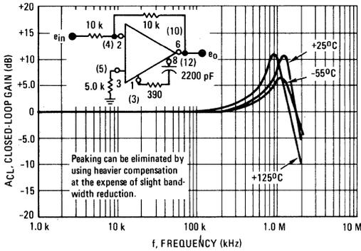
FIGURE 14 –  $A_{CL} = 10$  RESPONSE versus TEMPERATURE
