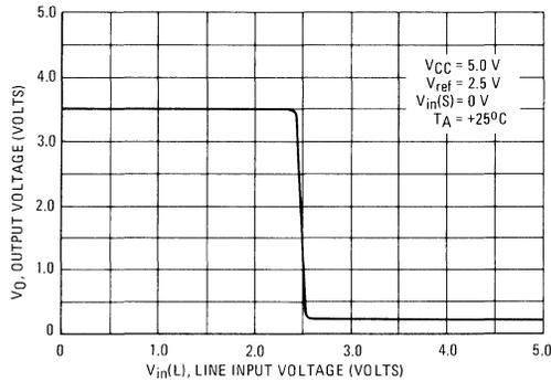
FIGURE 3 – SCHMITT TRIGGER
