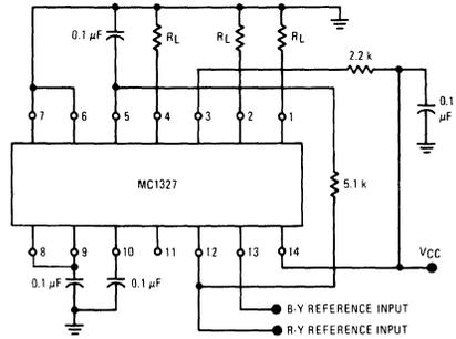
FIGURE 3 – DYNAMIC TEST CIRCUIT
