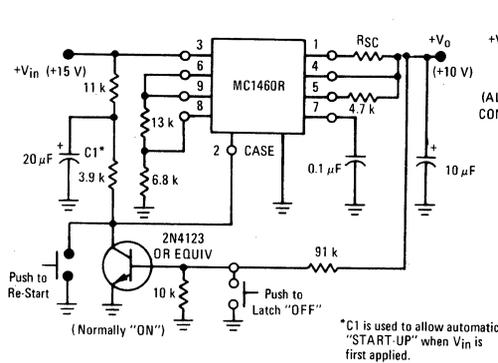
FIGURE 22 – SCR "CROWBAR" OVER VOLTAGE PROTECTION
