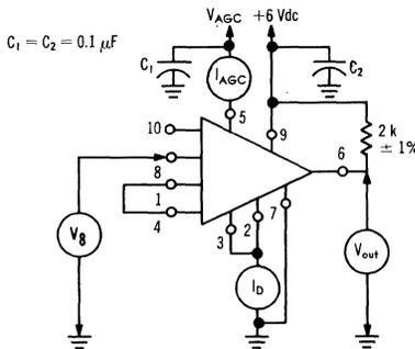
FIGURE 2 – VOLTAGE GAIN AND BANDWIDTH TEST CIRCUIT
