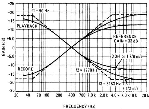
FIGURE 8 – TYPICAL TAPE HEAD OUTPUT CHARACTERISTICS (constant flux)
