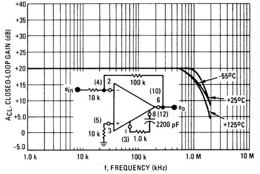
FIGURE 15 –  $A_{CL} = 100$  RESPONSE versus TEMPERATURE
