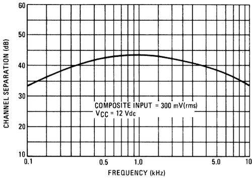
FIGURE 7 – CHANNEL SEPARATION
