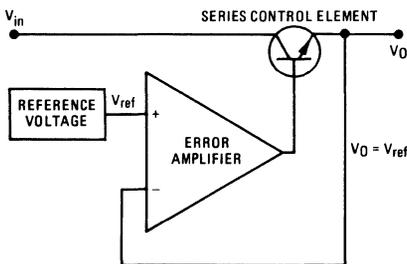
FIGURE 26 – THE "REGULATOR-WITHIN-A-REGULATOR" APPROACH
