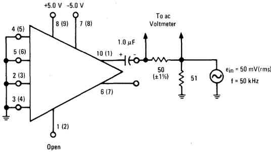
FIGURE 16 – INPUT BIAS CURRENT AND INPUT OFFSET CURRENT TEST CIRCUIT
