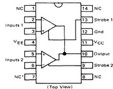
\*Connected to pin 4 via the substrate on some plastic units.
