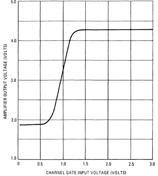
FIGURE 8 – INPUT THRESHOLD FOR OUTPUT VOLTAGE SWING FROM V<sub>OH</sub> TO V<sub>OL</sub> PROPAGATION DELAY FROM INPUT TO OUTPUT
