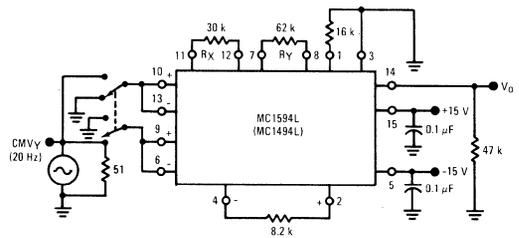
FIGURE 7 - POWER-SUPPLY SENSITIVITY
