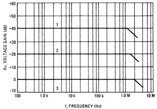
FIGURE 4 – OPEN LOOP VOLTAGE GAIN
