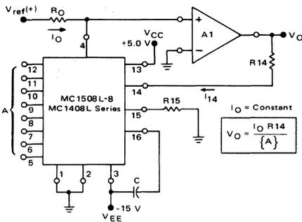
This circuit yields the inverse of a digital word scaled by a constant. For minimum error over the range of operation,  $I_O$  can be set at  $16 \mu\text{A}$  so that  $I_{14}$  will have a maximum value of  $3.984 \text{ mA}$  for a digital bit input configuration of 00000001.
