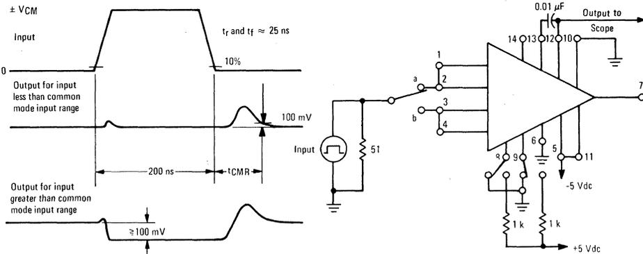
FIGURE 14 – DIFFERENTIAL RECOVERY AND DIFFERENTIAL RANGE
