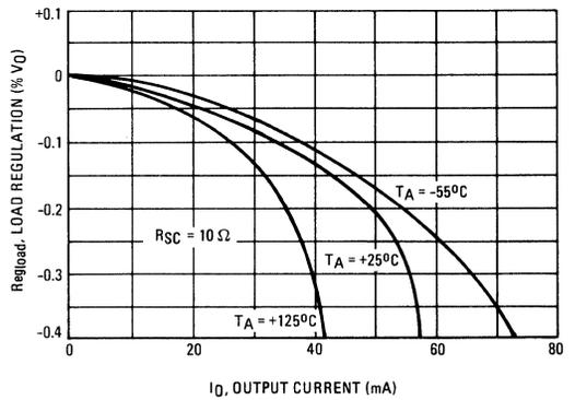
FIGURE 8 – CURRENT LIMITING CHARACTERISTICS
