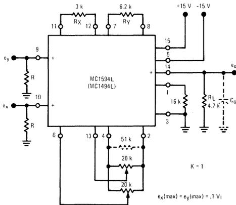
shows a typical ac multiplier circuit with a scale factor  $K \approx 1$ . Again, resistor  $R_X$  and  $R_Y$  are chosen as outlined in the previous section, with  $R_L$  chosen to provide the required scale factor.
