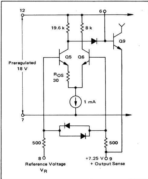
FIGURE 10 – CURRENT CONTROL CIRCUIT
