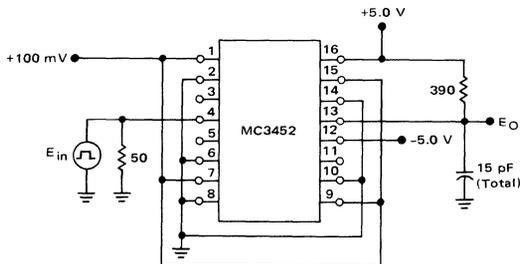
Output of Channel B shown under test, other channels are tested similarly.
