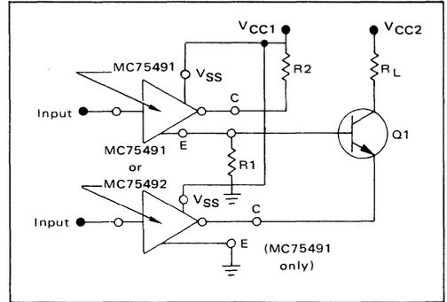
FIGURE 17 – MOS CALCULATOR CHIP-TO-LED INTERFACE CIRCUIT
