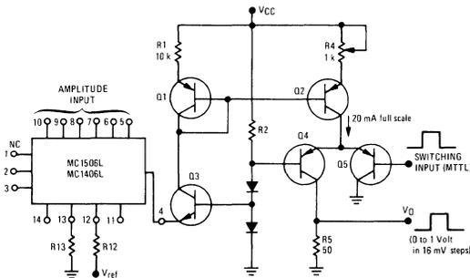
Fast rise and fall times require the use of high speed switching transistors for the differential pair, Q4 and Q5. Linear ramps and sine waves may be generated by the appropriate reference input.
