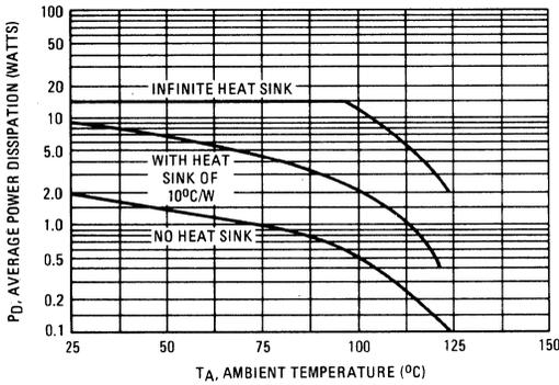
**FIGURE 2 – MAXIMUM AVERAGE POWER DISSIPATION AS A FUNCTION OF AMBIENT TEMPERATURE (TO-3 TYPE PACKAGE)**
