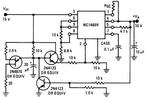
FIGURE 26 – CONNECTION FOR A NEGATIVE OUTPUT VOLTAGE
