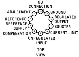
Pin 5 Electrically Connected to Case Through Substrate
