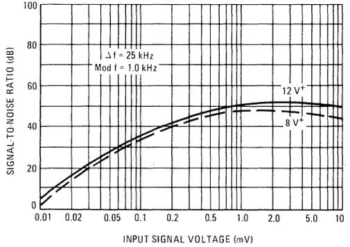
FIGURE 12 – DETECTOR TRANSFER CHARACTERISTIC
