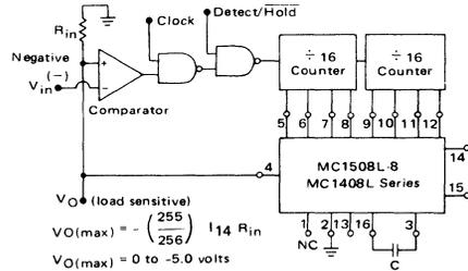
FIGURE 31 – PROGRAMMABLE PULSE GENERATION
