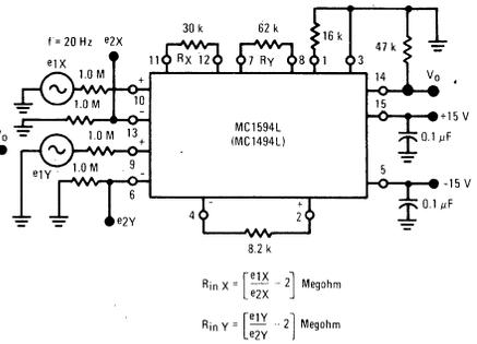
FIGURE 3 - OFFSET VOLTAGES, GAIN
