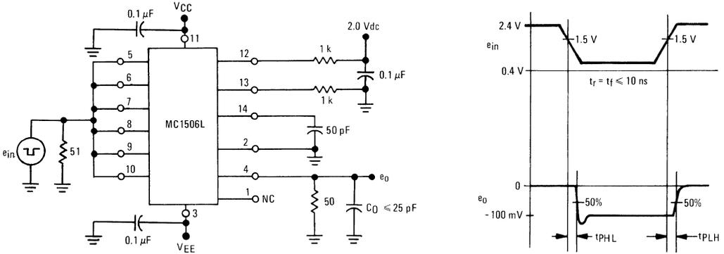
FIGURE 10 – RELATIVE ACCURACY TEST CIRCUIT
