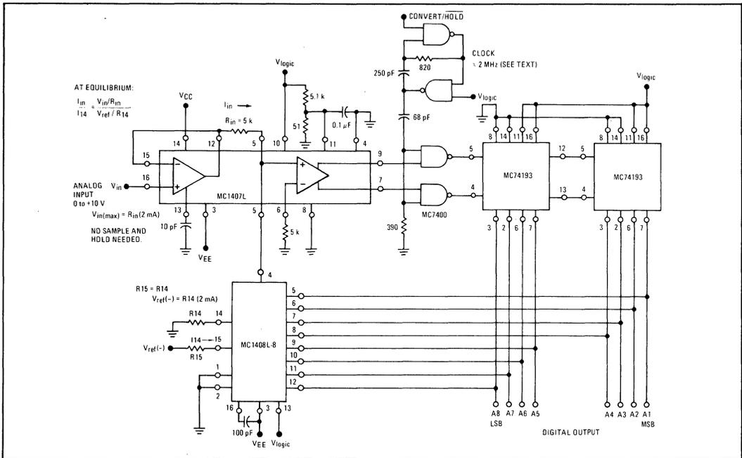
FIGURE 35 - 8-BIT TRACKING A-TO-D CONVERTER
