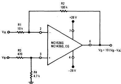
FIGURE 2 – VOLTAGE CONTROLLED CURRENT
