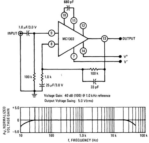
Voltage Gain: 40 dB (100) @ 1.0 kHz reference
