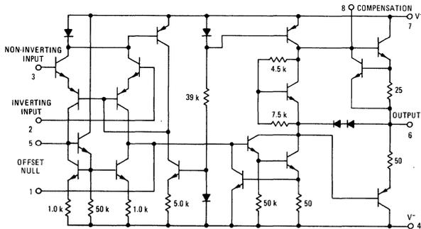
FIGURE 4 – OFFSET ADJUST AND FREQUENCY COMPENSATION
