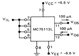
**FIGURE 7 – POWER "OFF" POSITIVE and NEGATIVE OUTPUT COMMON-MODE RANGE**
