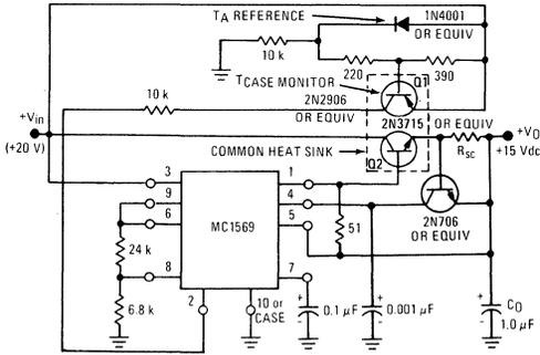
In the case where an external pass transistor is employed, its temperature, rather than that of the IC regulator, requires control. A technique similar to the one just discussed can be used by directly monitoring the case temperature of the pass transistor as is indicated in Figure 40. The case of the normally "OFF" thermal monitoring transistor, Q2, should be in thermal contact with, but electrically isolated from, the case of the boost transistor, Q1.
