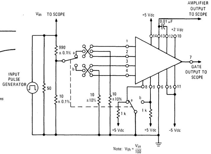
Number at terminal end denotes the pin number for flat package only; to ascertain the corresponding pin number for the dual in line packages refer to the circuit schematic on the second page.
