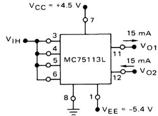
**FIGURE 5 – OUTPUT "OFF" POSITIVE and NEGATIVE OUTPUT COMMON-MODE RANGE**
