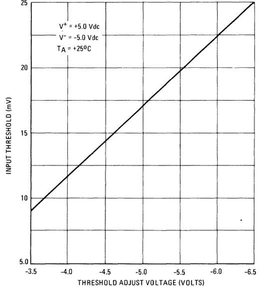
FIGURE 4 – TYPICAL INPUT THRESHOLD versus  $V^-$
