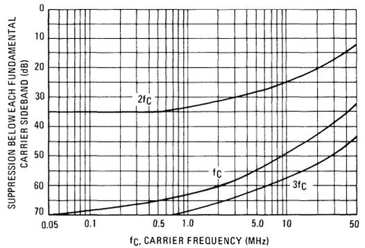
FIGURE 21 – CARRIER FEEDTHROUGH versus FREQUENCY
