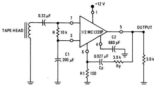
The lower -3.0 dB corner frequency (f1) is determined by the value for capacitor C1 in accordance with equation 1.
