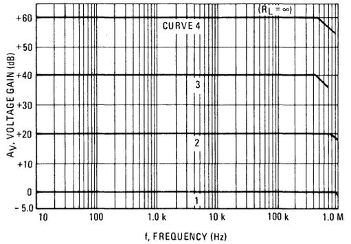
FIGURE 6 – OPEN LOOP VOLTAGE GAIN versus FREQUENCY
