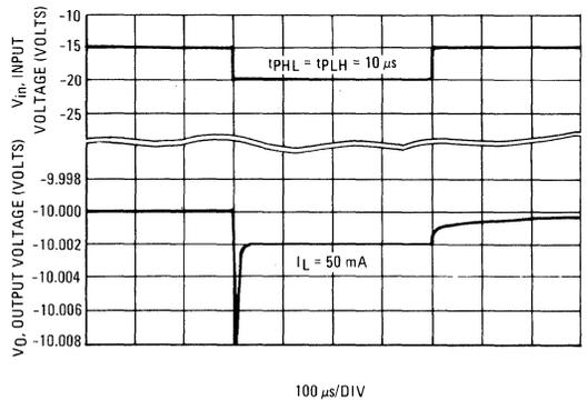
FIGURE 21 – LOAD TRANSIENT RESPONSE
