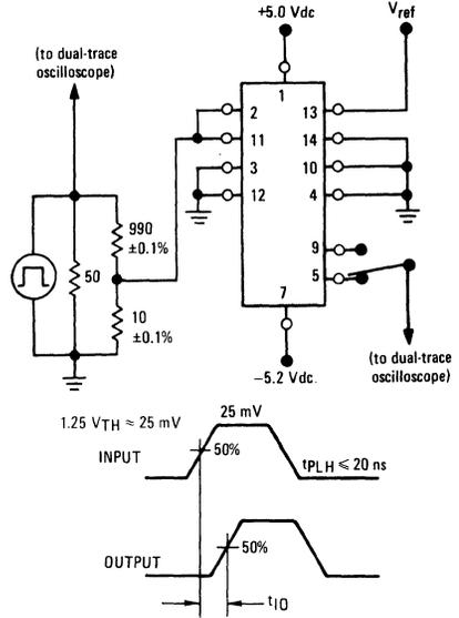
FIGURE 12 – PROPAGATION DELAY – STROBE TO
