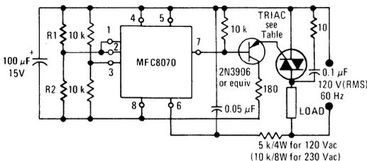
Zero crossing triac control circuit for gate current requirements to 100 mA.
