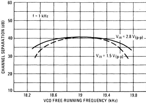
**FIGURE 6 – CHANNEL SEPARATION versus SUPPLY VOLTAGE**
