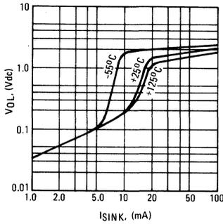
**FIGURE 8 – LOW OUTPUT VOLTAGE @ VCC = 10 Vdc**
