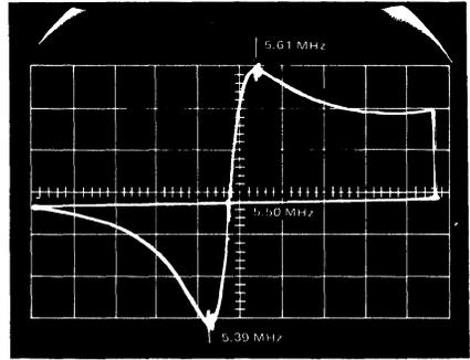
FIGURE 6 – IF VOLTAGE GAIN versus FREQUENCY
