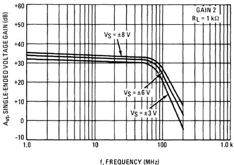
FIGURE 12 – GAIN versus FREQUENCY and TEMPERATURE
