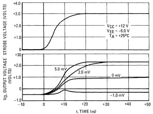
FIGURE 7 – COMMON-MODE PULSE RESPONSE
