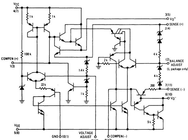
Pin numbers adjacent to terminals are for the G and R suffix packages only. Pin numbers in parentheses are for the L suffix package only.
