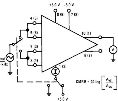
Number in parenthesis denotes pin for F and L packages, number at left in each case denotes corresponding pin for G package.
