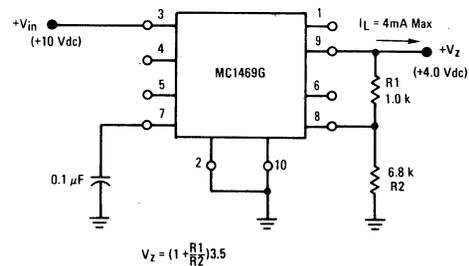
FIGURE 39 — JUNCTION TEMPERATURE LIMITING SHUTDOWN CIRCUIT
