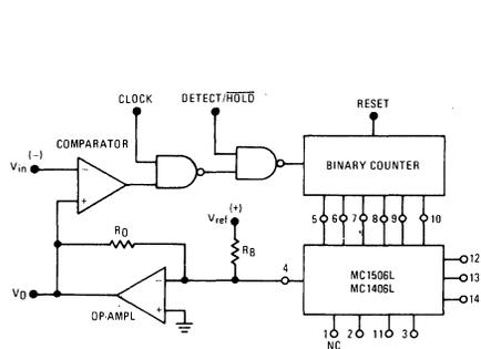
Positive peaks may be detected by inserting a hex inverter between the counter and MC1506L, reversing the comparator inputs, and connecting the output amplifier for unipolar operation.
