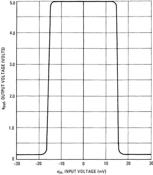
FIGURE 7 – CHANNEL GATE INPUT-AMPLIFIER OUTPUT TRANSFER CHARACTERISTICS
