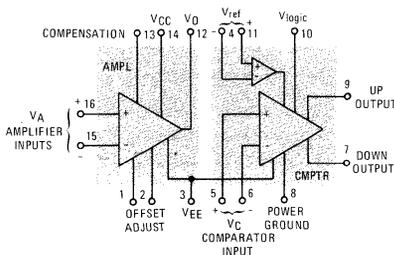
FIGURE 2 – TYPICAL APPLICATION 8-BIT TRACKING
