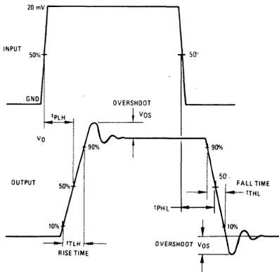
FIGURE 8 – SMALL-SIGNAL TRANSIENT RESPONSE TEST CIRCUIT
