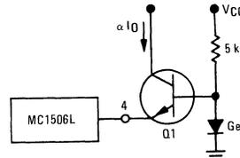
The output voltage range for this circuit is 0 volts to  $BV_{CBO}$  of the transistor. Variations in beta must be considered for wide temperature range applications. An inverted output waveform may be obtained by using a load resistor from a positive reference voltage to the collector of the transistor. Also, high-speed operation is possible with a large output voltage swing.
