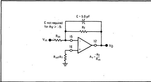
FIGURE 13 – VOLTAGE GAIN = -1
