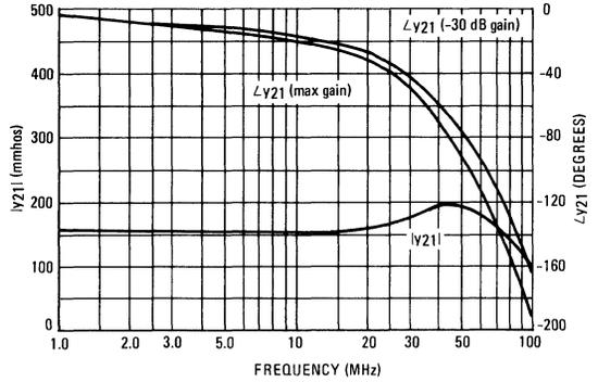
FIGURE 9 – DIFFERENTIAL OUTPUT ADMITTANCE
