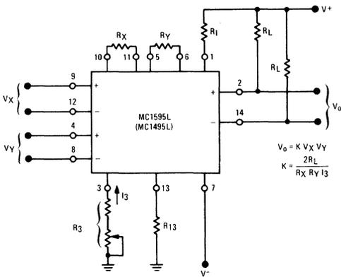
If an operational amplifier is used for level shift, as shown in Figure 21, the output swing (of the multiplier) is greatly reduced. See Section 3 for further details.
