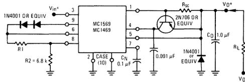
Note: This configuration increases minimum input-output differential voltage by ≈ 0.7 V.
