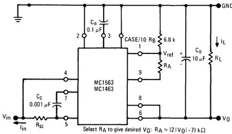
Select  $R_A$  to give desired  $V_O$ :  $V_O \approx (2|V_O| - 7) \text{ k}\Omega$
