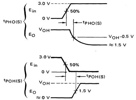
FIGURE 12 – STROBE PROPAGATION DELAY  $t_{PLH(S)}$  AND  $t_{PHL(S)}$
