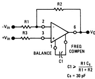
**FIGURE 15 – FEEDFORWARD COMPENSATION**
