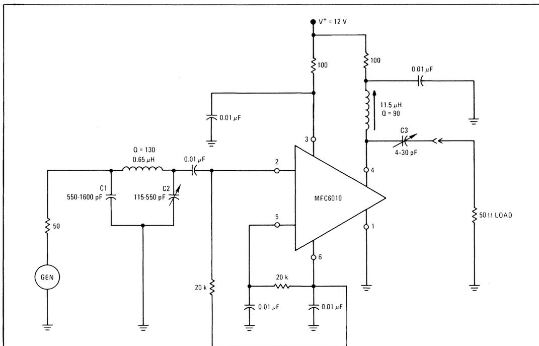
Note: C1 (1000 pF nom), C2 (420 pF nom), C3 (20 pF nom) adjusted for maximum power gain.
