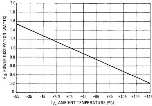
FIGURE 8 – MAXIMUM DIFFERENTIAL LEVEL SHIFT POWER DISSIPATION (WITH BOTH INPUTS HIGH)
