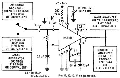
FIGURE 13 – AUDIO VOLTAGE GAIN, AUDIO THD TEST CIRCUIT
