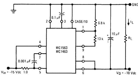
FIGURE 7 – OUTPUT IMPEDANCE
