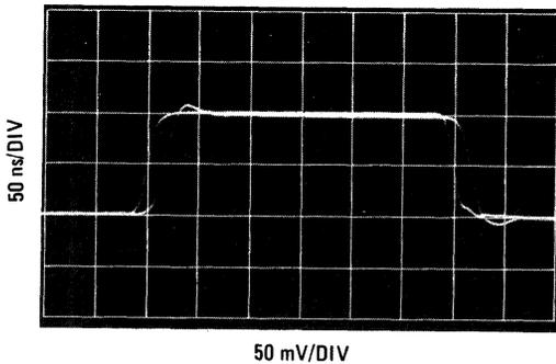
FIGURE 6 – THREE-QUADRANT OPERATIONAL AMPLIFIER PULSE RESPONSE WAVEFORMS
