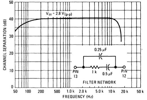
**FIGURE 5 – CHANNEL SEPARATION versus VCO FREE-RUNNING FREQUENCY**
