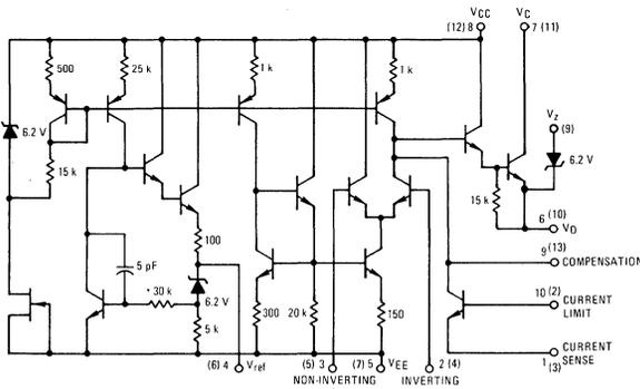
PIN NUMBERS ADJACENT TO TERMINALS ARE FOR THE METAL AND CERAMIC FLAT PACKAGE;
