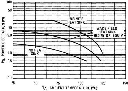
FIGURE 4 – MAXIMUM AVERAGE POWER DISSIPATION (MLM309G)
