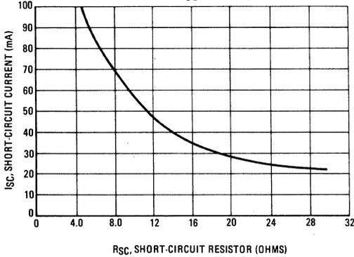
FIGURE 10 - CURRENT-LIMITING CHARACTERISTICS
