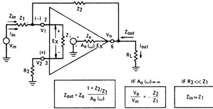
FIGURE 11 – NON-INVERTING FEEDBACK MODEL
