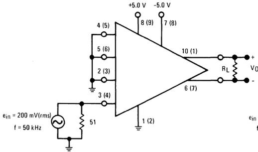
FIGURE 14 – INPUT IMPEDANCE TEST CIRCUIT
