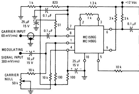
**FIGURE 27 – BALANCED MODULATOR-DEMODULATOR**
