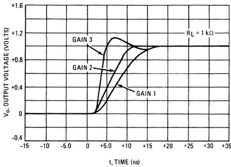
**FIGURE 14 – PULSE RESPONSE versus SUPPLY VOLTAGE**
