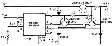
FIGURE 30 - PNP CURRENT BOOST CONNECTION
