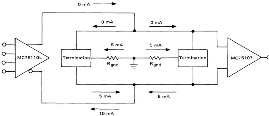
“Push-Pull” Differential Line Driver Typical Mismatch of Output Currents Indicated (2 mA)
