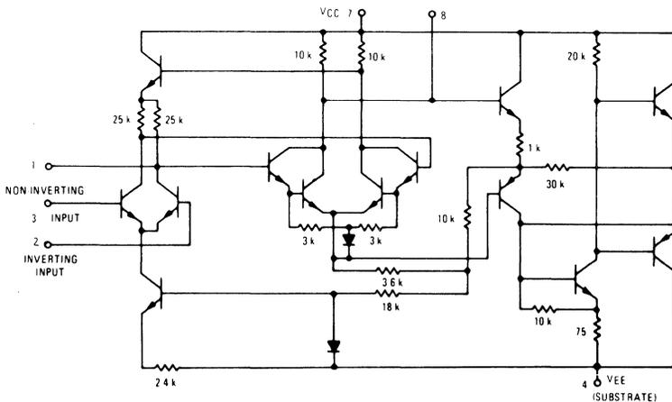
FIGURE 2 - EQUIVALENT CIRCUIT
