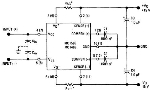
C1 and C2 should be located as close to the device as possible. A 0.1  $\mu\text{F}$  ceramic capacitor ( $C_{in}$ ) may be required on the input lines if the device is located an appreciable distance from the rectifier filter capacitors. C3 and C4 may be increased to improve load transient response and to reduce the output noise voltage. At low temperature operation, it may be necessary to bypass C4 with a 0.1  $\mu\text{F}$  ceramic disc capacitor.
