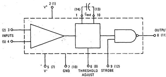
Number at end of terminal represents pin number for devices in flat package and metal can. Number in parenthesis represents pin number for dual in-line package.
