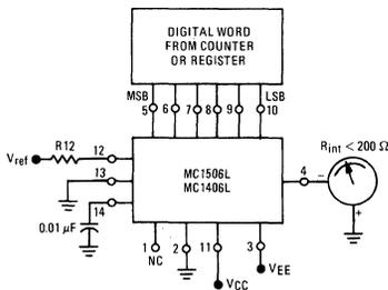
The best frequency response is obtained by not allowing  $I_{12}$  to reach zero.  $R_S$  can be set for a  $\pm 1.0$  mA variation in relation to  $I_{12}$ .  $I_{12}$  can never be negative.
