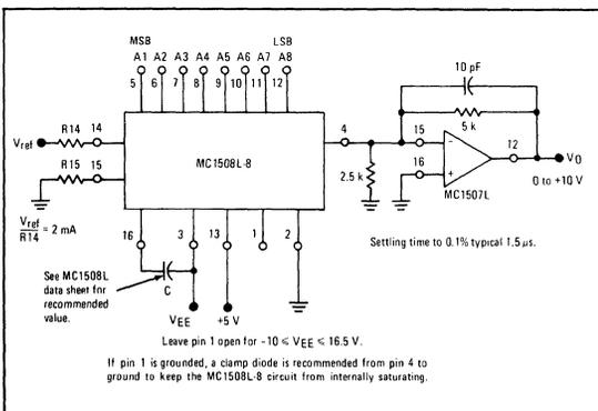
**FIGURE 33 – D-TO-A CURRENT-TO-VOLTAGE CONVERTER (BIPOLAR OUTPUT)**
