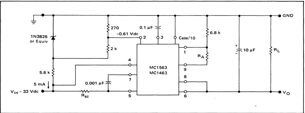
FIGURE 35 – Junction Temperature Limiting Shutdown Circuit
