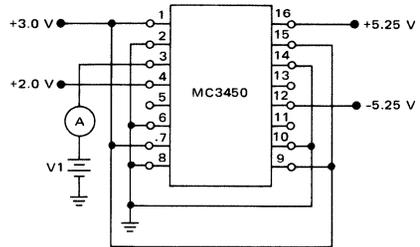
Output of Channel A shown under test, other outputs are tested similarly for V1 = 0.4 V and +2.4 V.
