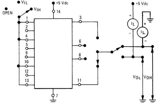
FIGURE 3 – OUTPUT SHORT-CIRCUIT CURRENT
