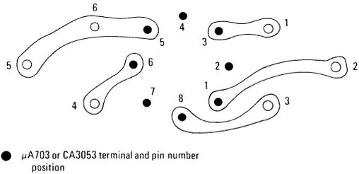
\*Foil patterns shown are intended to show pin-for-pin interconnection. Any change in the number of components is dictated by the requirements of the individual design.
