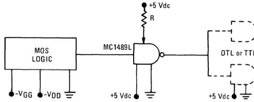
FIGURE 15 – TYPICAL PARALLELING OF TWO MC1489,A RECEIVERS TO MEET RS-232C
