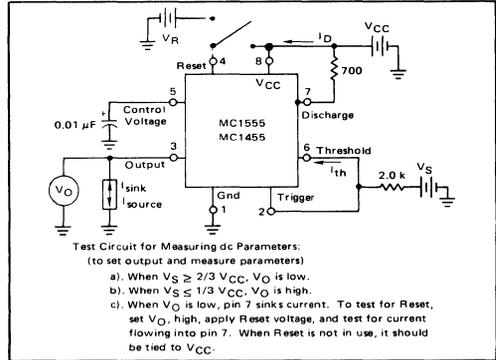
ELECTRICAL CHARACTERISTICS (T<sub>A</sub> = +25°C, V<sub>CC</sub> = +5.0 V to +15 V unless otherwise noted.)
