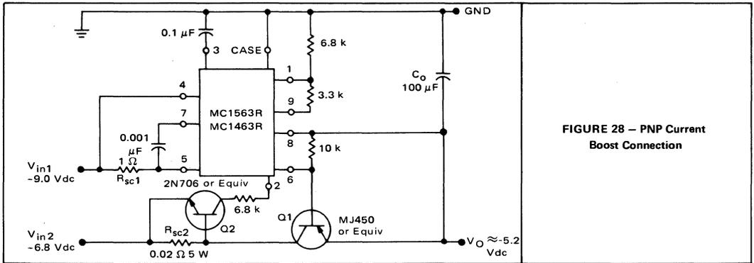
FIGURE 28 – PNP Current Boost Connection
