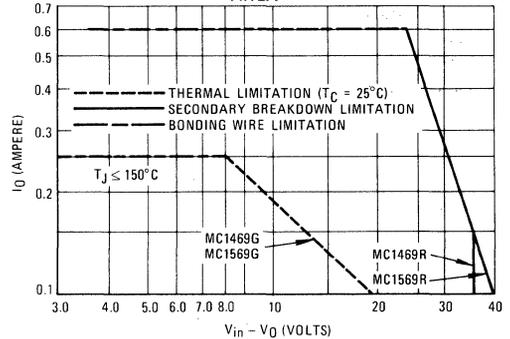
exceed the maximum junction temperature rating during this fault condition and, in addition, the dc safe operating area limit (see Figure 41).
