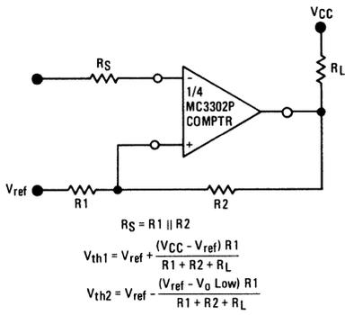
FIGURE 9 – THE COMPARATOR AS AN OPERATIONAL AMPLIFIER
