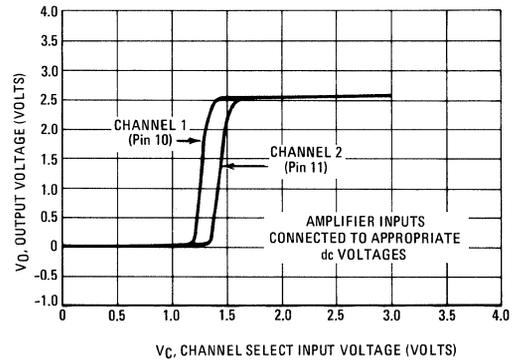
**FIGURE 17 – STROBE INPUT TRANSFER CHARACTERISTICS (Input High)**
