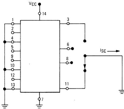
FIGURE 4 – POWER-SUPPLY CURRENT
