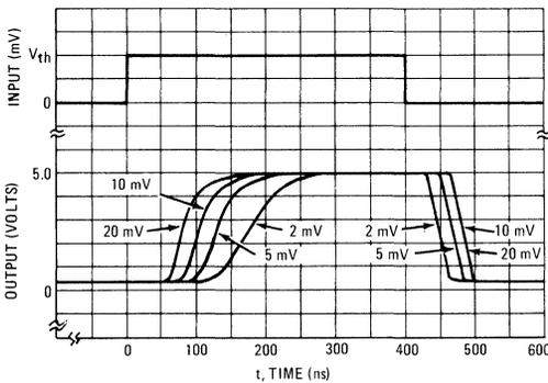
FIGURE 28 – COMPARATOR THRESHOLD versus  $V_{ref}$
