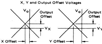
For most dc applications, all three offset adjust potentiometers (P<sub>1</sub>, P<sub>2</sub>, P<sub>4</sub>) will be necessary. One or more offset adjust potentiometers can be eliminated for ac applications (See Figures 28, 29, 30, 31).
