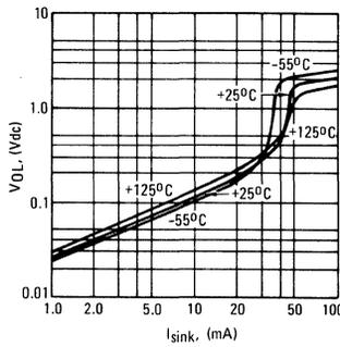
**FIGURE 9 – LOW OUTPUT VOLTAGE @ VCC = 15 Vdc**
