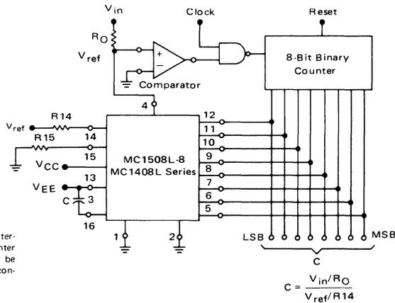
The circuit shown is a simple counter-ramp converter. An UP/DOWN counter and dual threshold comparator can be used to provide faster operation and continuous conversion.
