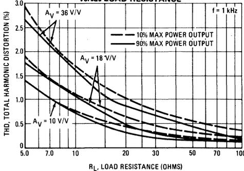
**FIGURE 9 – TOTAL HARMONIC DISTORTION**
