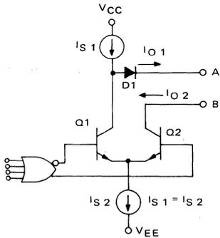
If Q1 is "on", Q2 is "off", Diode D1 is "off" and current  $I_{S1}$  flows through Q1 and  $I_{S2}$  to  $V_{EE}$ . However, if Q1 is "off", and Q2 is "on", the current  $I_{S1}$  flows through diode D1 to output A and current from output B flows through Q2 to current sink  $I_{S2}$ .
