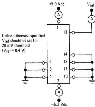
FIGURE 7 – INPUT BIAS CURRENT INPUT OFFSET CURRENT
