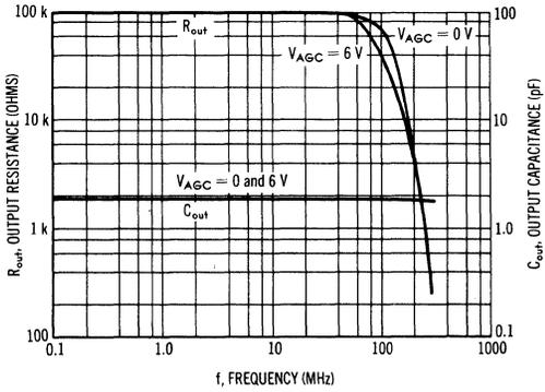
FIGURE 8 – OUTPUT RESISTANCE AND CAPACITANCE versus AGC VOLTAGE
