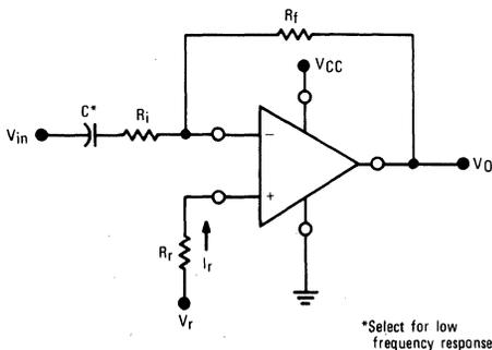
FIGURE 21 – INVERTING AMPLIFIER WITH  $A_v = 100$  AND  $V_r = V_{CC}$
