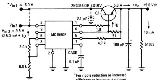
\*For ripple reduction or increased efficiency at low output voltages, the collector of Q1 can tie to a separate low-voltage supply as shown.
