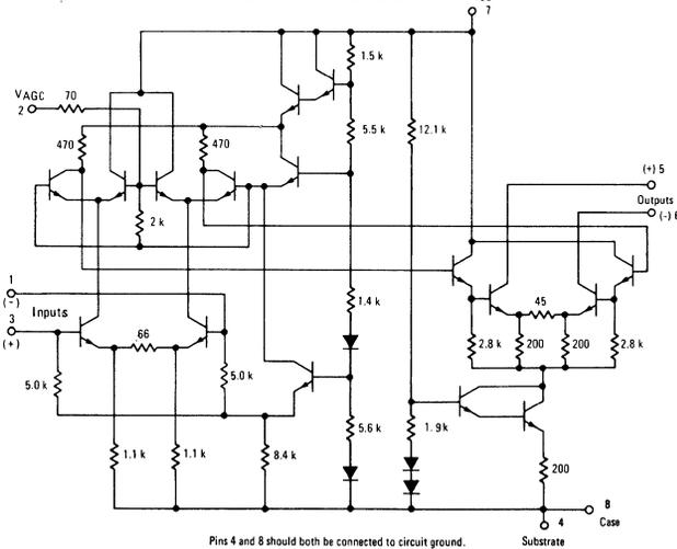
Pins 4 and 8 should both be connected to circuit ground.
