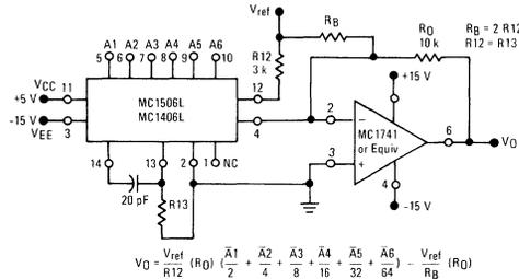
$$V_O = \frac{V_{ref}}{R_{12}} (R_O) \left( \frac{\bar{A}_1}{2} + \frac{\bar{A}_2}{4} + \frac{\bar{A}_3}{8} + \frac{\bar{A}_4}{16} + \frac{\bar{A}_5}{32} + \frac{\bar{A}_6}{64} \right) - \frac{V_{ref}}{R_B} (R_O)$$
