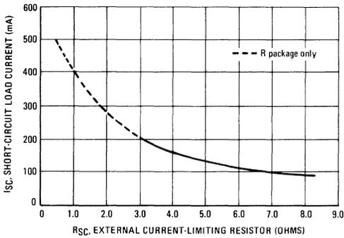
**FIGURE 6 – CURRENT-LIMITING CHARACTERISTICS**
