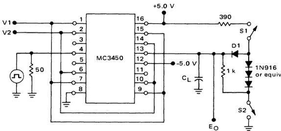
Output of Channel B shown under test, other channels are tested similarly.
