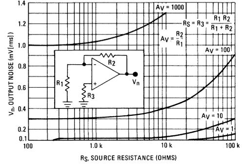
FIGURE 10 – HIGH-IMPEDANCE, HIGH-GAIN INVERTING AMPLIFIER
