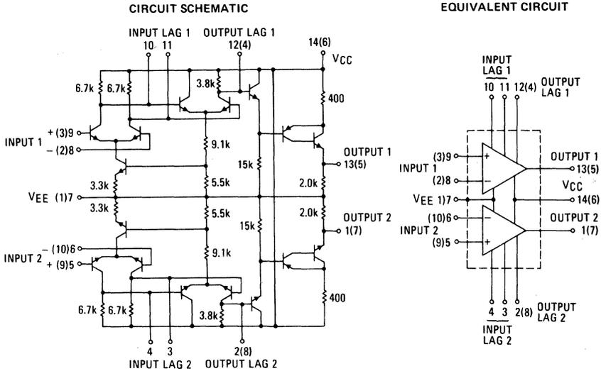
Number at end of terminal is pin number for ceramic packages.
