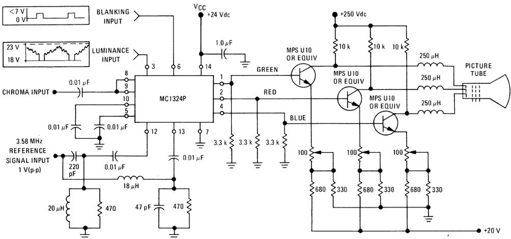
A typical application is given above to indicate the requirements and output functions of this chroma demodulator.
