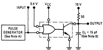
NOTES: A. Pulse generator characteristics:  $t_w = 0.5 \mu s$ ,  $PRR = 1.0 \text{ MHz}$ ,  $z_0 \approx 50 \Omega$ .
