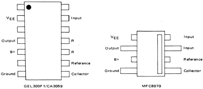
**COMPATIBLE PRINTED CIRCUIT FOIL PATTERN FOR MFC8070, GEL300F1 (PA424) AND CA3059**
