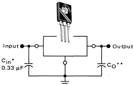
A common ground is required between the input and the output voltages. The input voltage must remain typically 2.0 V above the output voltage even during the low point on the input ripple voltage.
