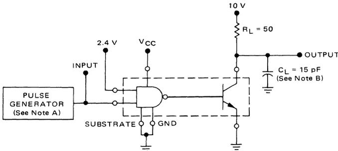
NOTES: A. The pulse generator has the following characteristics:  $t_w = 0.5 \mu s$ , PRR = 1.0 MHz,  $z_o \approx 50 \Omega$ .
