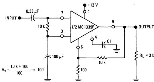
Figure 4 shows the response of the broadband amplifier with two different values of compensation capacitors, C1. Other capacitor values can be used; however, as the phase margin is reduced a greater possibility of oscillation exists.
