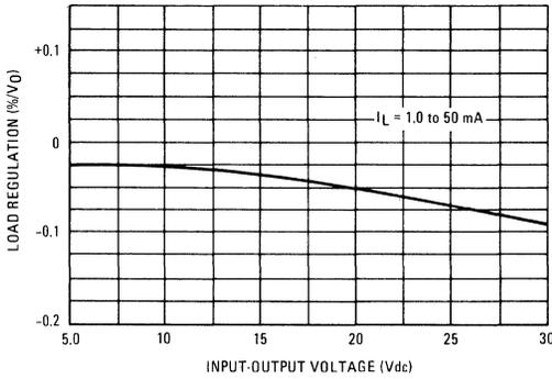
FIGURE 7 – LOAD REGULATION WITH CURRENT LIMITING
