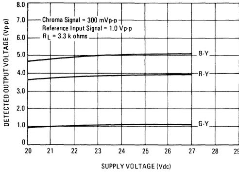
FIGURE 7 – DC OUTPUT VOLTAGE
