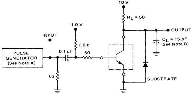
NOTES: A. The pulse generator has the following characteristics:  $t_w = 0.3 \mu s$ , duty cycle  $\leq 1\%$ ,  $z_o \approx 50 \Omega$ .
