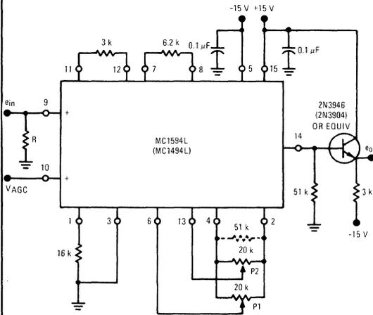
Notice that the resistor values for  $R_X$ ,  $R_Y$ , and  $R_L$  have been modified. This has been done primarily to increase the bandwidth by lowering the output impedance of the MC1594 and then lowering  $R_X$  and  $R_Y$  to achieve a gain of 1. The  $e_c$  can be as large as 1 volt peak and  $e_m$  as high as 2 volts peak. No output offset adjust is employed since we are interested only in the ac output components.
