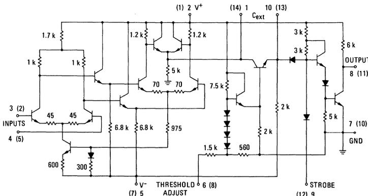
Number at end of terminal represents pin number for devices in flat package and metal can. Number in parenthesis represents pin number for ceramic dual in-line package.
