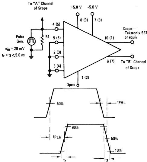
Number in parenthesis denotes pin for F and L packages, number at left in each case denotes corresponding pin for G package.
