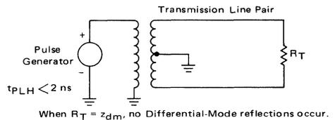
FIGURE 17B – CIRCUIT FOR  $z_{cm}$  MEASUREMENT
