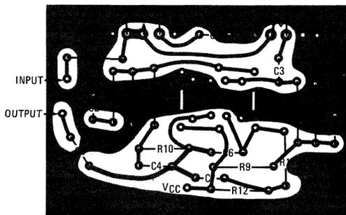
FIGURE 18 – PRINTED CIRCUIT BOARD (Foil Side)
