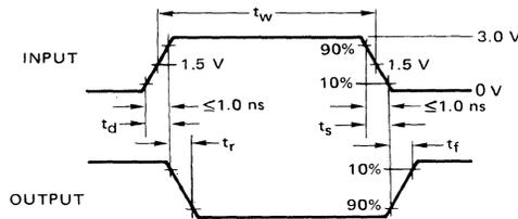
FIGURE 9 – SWITCHING TIMES, GATE AND TRANSISTOR
