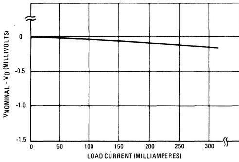
FIGURE 31 – REGULATOR OUTPUT VOLTAGE (under pulsed load condition)
