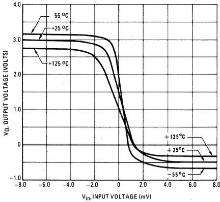
**FIGURE 4 – INPUT OFFSET VOLTAGE versus TEMPERATURE**
