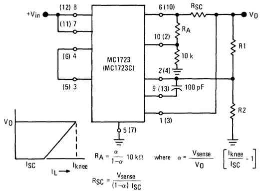
FIGURE 18 – +5 V, 1-AMPERE SWITCHING REGULATOR
