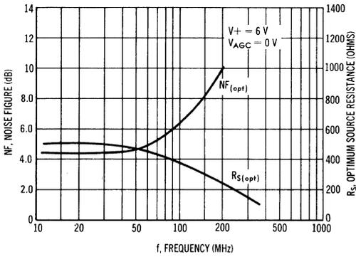
FIGURE 13 – NOISE FIGURE versus SOURCE RESISTANCE
