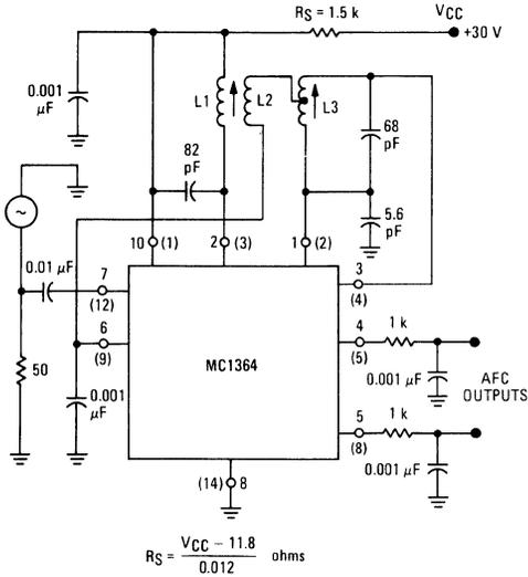
The number without parenthesis is the pin number for the metal package. The number in parenthesis is the pin number for the plastic package.
