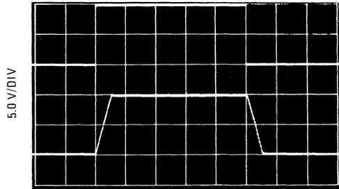
Clock Frequency increases from 5.0 MHz to 20 MHz with voltage controlled MC4024 in Panic Mode operation.
