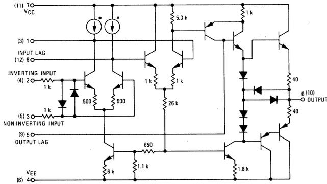
Pin numbers adjacent to terminals apply to 8-pin packages, numbers in parenthesis apply to 14-pin packages.
