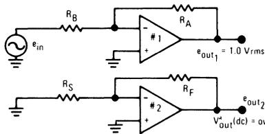
Induced output signal (μV of induced output signal in amplifier #2 per volt of output signal at amplifier #1).
