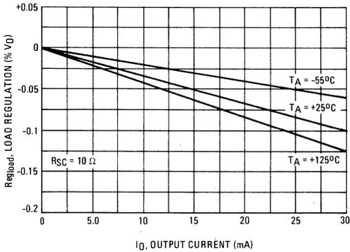
FIGURE 7 – LOAD REGULATION CHARACTERISTICS WITH CURRENT LIMITING
