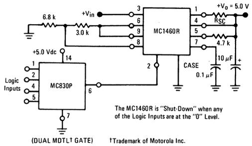
FIGURE 21 – AUTOMATIC LATCH INTO SHUT-DOWN WHEN OUTPUT IS SHORT-CIRCUITED WITH MANUAL RE-START
