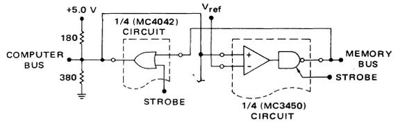
The three-state capability of the MC3450 permits bidirectional data transmission as illustrated.
