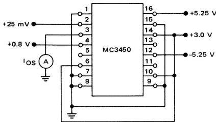
Channel A shown under test, other channels are tested similarly. Only one output shorted at a time.
