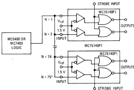
\*Most MC5400/MC7400 devices are capable of maintaining a 2.4-volt level under loads up to 7.5 mA.
