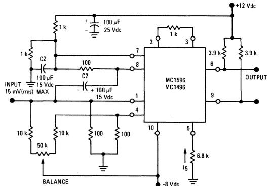
Pin number references pertain to this device when packaged in a metal can. To ascertain the corresponding pin numbers for a ceramic packaged device refer to the PIN CONNECTION CHART on the first page of this specification.
