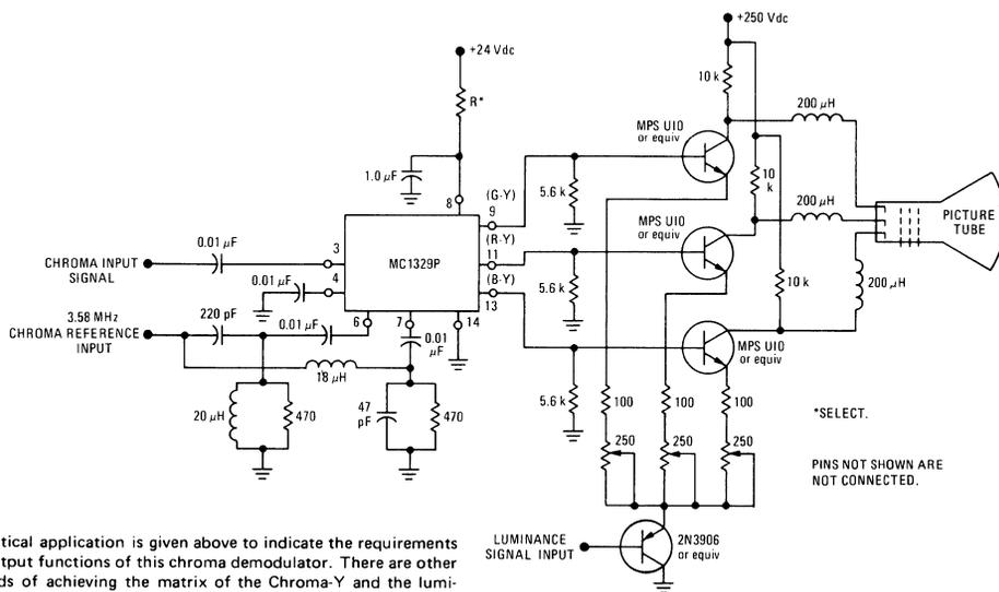
A practical application is given above to indicate the requirements and output functions of this chroma demodulator. There are other methods of achieving the matrix of the Chroma-Y and the luminance components without degradation of performance other than the one indicated. E.g., it is a common practice for color TV manufacturers to matrix in the picture tube.
