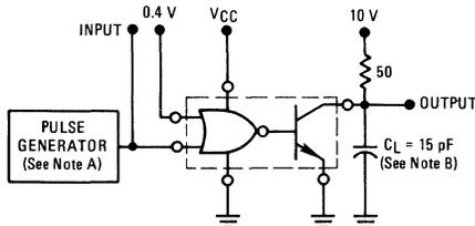
NOTES: A. Pulse generator characteristics:  $t_w = 0.5 \mu s$ ,  $PRR = 1.0 \text{ MHz}$ ,  $z_0 \approx 50 \Omega$
