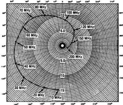
FIGURE 15 –  $S_{12}$ , REVERSE TRANSMISSION COEFFICIENT (FEEDBACK)
