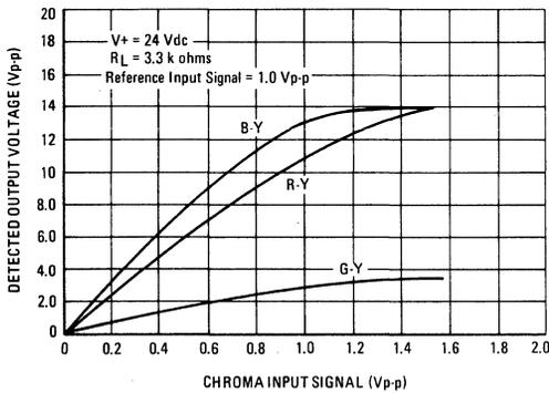
FIGURE 5 – DETECTED OUTPUT
