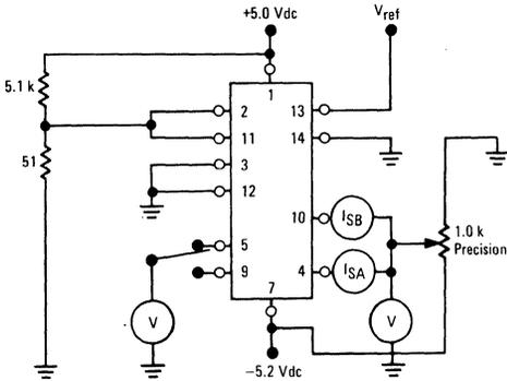
FIGURE 11 – PROPAGATION DELAY –
