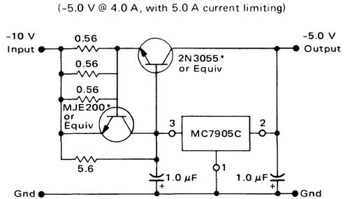
\*Mounted on common heat sink, Motorola MS-10 or equivalent.
