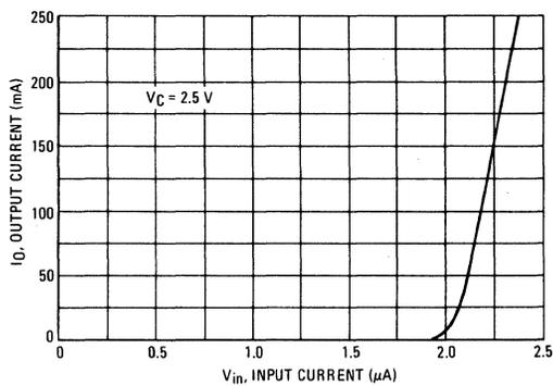
FIGURE 3 – COLLECTOR CURRENT versus INPUT CURRENT
