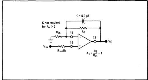
FIGURE 14 – VOLTAGE GAIN = +1
