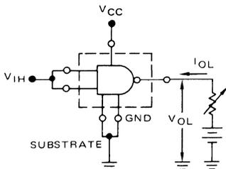
Both inputs are tested simultaneously.
