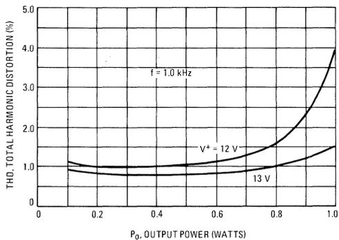
FIGURE 9 - TOTAL HARMONIC DISTORTION
