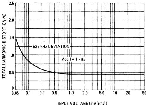
**FIGURE 7 – IF AMPLIFIER AND DETECTOR THD**
