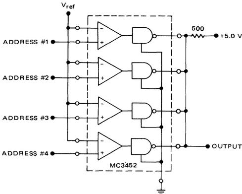
The MC3452 can be used for address decoding as illustrated above. All outputs of the MC3452 are tied together through a common resistor to +5.0 volts. In this configuration the MC3452 provides the "AND" function. All addresses have to be true before the output will go high. This scheme eliminates the need for an "AND" gate and enhances speed throughput for address decoding.
