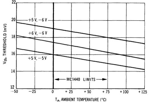
FIGURE 11 – TYPICAL THRESHOLD versus POWER SUPPLIES
