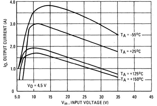
FIGURE 7 – PEAK OUTPUT CURRENT (G PACKAGE)
