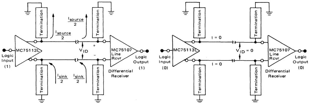
**FIGURE 15 – COMPARISON OF GROUND CURRENTS IN “PUSH-PULL” AND “PULL-ONLY” DATA TRANSMISSION SYSTEMS**
