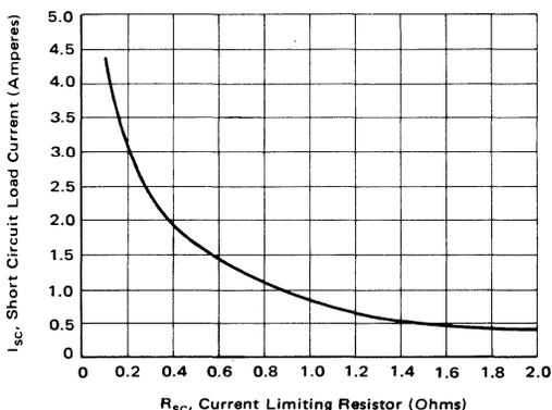
FIGURE 27 –  $I_{SC}$  versus  $R_{SC}$  (reference Figure 26)
