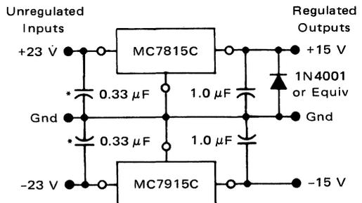
\*Required only if the regulators are located an appreciable distance from the power supply filters.
