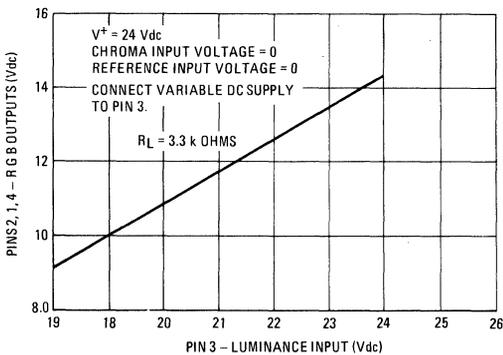
**FIGURE 11 – DETECTED OUTPUT VOLTAGE**
