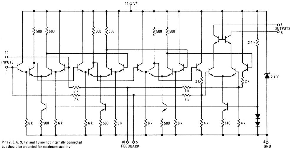
Pins 2, 3, 6, 9, 12, and 13 are not internally connected but should be grounded for maximum stability.
