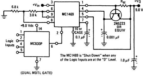
**FIGURE 35 – AUTOMATIC LATCH INTO SHUT-DOWN WHEN OUTPUT IS SHORT-CIRCUITED WITH MANUAL RE-START**
