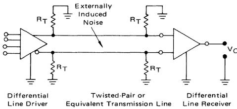
Another advantage of differential line driver systems over single-ended line driver systems is that a noise spike coupled into adjacent lines from the positive-going signal line is cancelled by an equal and opposite noise spike coupled from the negative-going signal line. In single-ended systems, a shield would be required for each transmission line to prevent coupling to adjacent lines in the cable.
