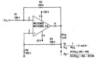
FIGURE 3 – TYPICAL NON-INVERTING X10
