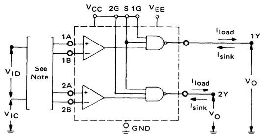
NOTE: When testing one channel, the inputs of the other channel are grounded.
