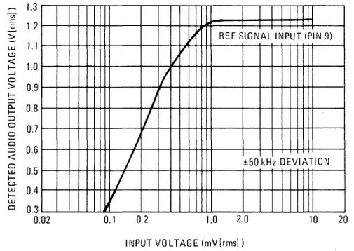
FIGURE 6 – DETECTOR TRANSFER CHARACTERISTIC
