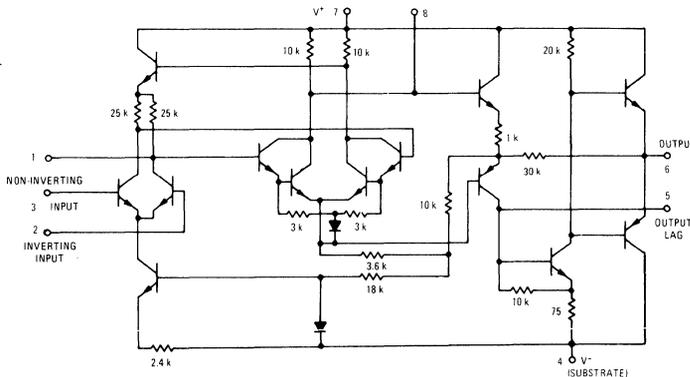
FIGURE 2 - EQUIVALENT CIRCUIT
