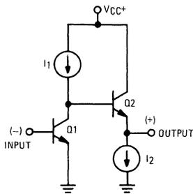
FIGURE 17 – OBTAINING A NONINVERTING INPUT
