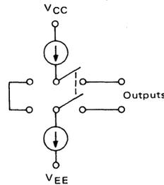
FIGURE 14 – "PUSH-PULL" SYSTEM SHOWING BOTH LOGIC CONDITIONS
