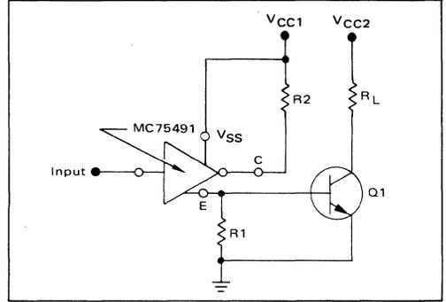
FIGURE 15 – QUAD-OR-HEX HIGH-CURRENT PNP TRANSISTOR DRIVER
