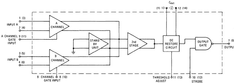
Number at terminal end denotes pin number for flat package. Number in parenthesis denotes pin number for dual in-line package.
