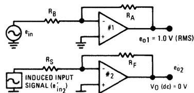
Induced input signal (μV of induced input signal in amplifier #2 per volt of output signal at amplifier #1)
