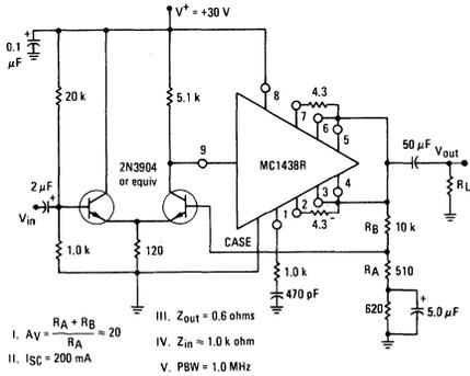
FIGURE 15 – NON-INVERTING POWER AMPLIFIER
