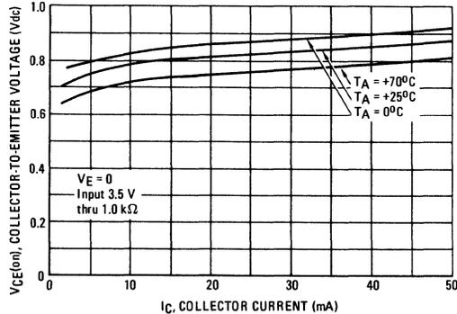
FIGURE 6 – OUTPUT VOLTAGE LOW versus OUTPUT CURRENT
