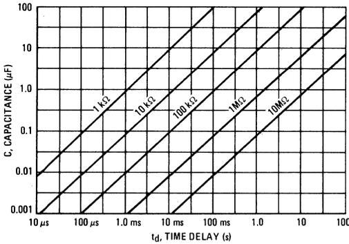
FIGURE 17 – ASTABLE CIRCUIT
