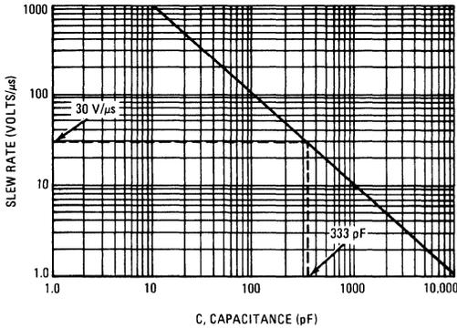
fast for this requirement. The current limited output of the device can be used to control this slew rate by connecting a capacitor to each driver output. The required capacitor can be easily determined by using the relationship  $C = I_{SC} \times \Delta T / \Delta V$  from which Figure 12 is derived. Accordingly, a 330-pF capacitor on each output will guarantee a worst case slew rate of 30 volts per microsecond.
