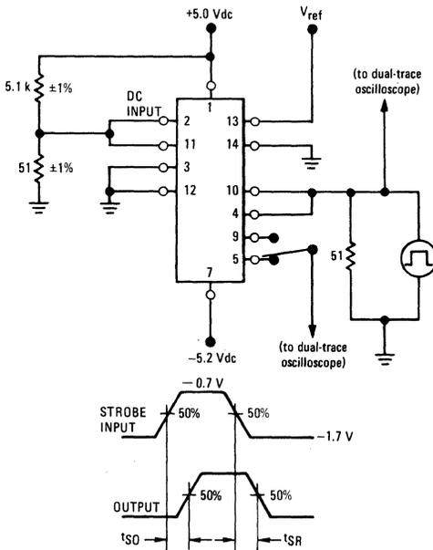
FIGURE 13 – DIFFERENTIAL MODE RECOVERY TIME
