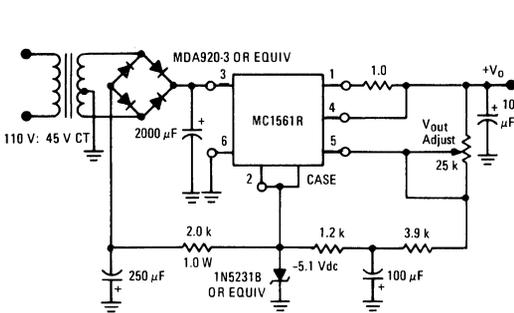
FIGURE 17 - PROVIDING TWO REGULATED OUTPUT VOLTAGES
