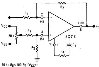
FIGURE 3 – OUTPUT LIMITING CIRCUIT
