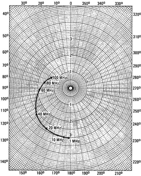
**FIGURE 23 –  $s_{12}$ , REVERSE TRANSMISSION COEFFICIENT (FEEDBACK)**
