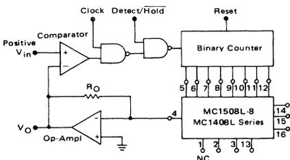
FIGURE 32 – PROGRAMMABLE CONSTANT CURRENT SOURCE
