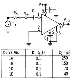
FIGURE 5c – CAPACITIVE COUPLED INPUT ( $R_S < 500\ \Omega$ )
