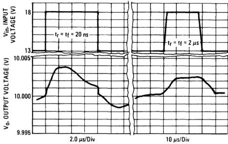
**FIGURE 4 – LOAD TRANSIENT RESPONSE**
