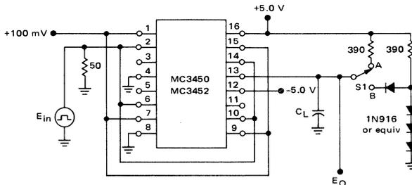
Output of Channel B shown under test, other channels are tested similarly.
