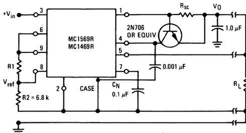
FIGURE 38 — AN ADJUSTABLE "ZERO-TC" VOLTAGE SOURCE
