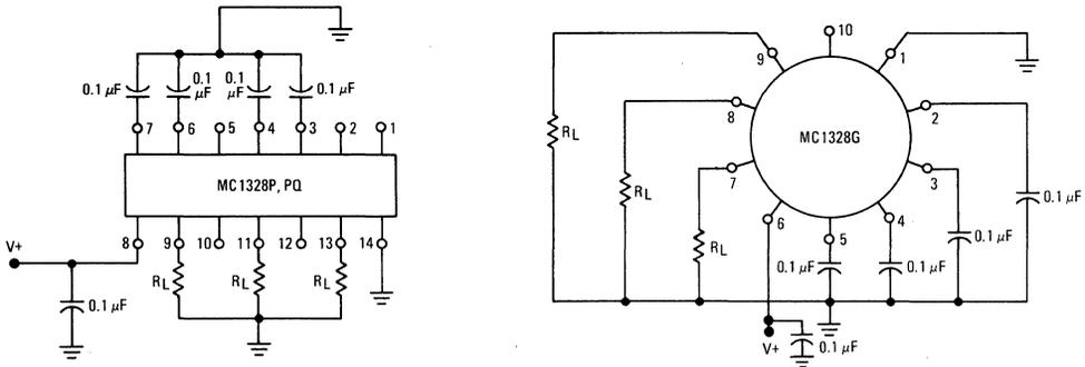
FIGURE 3 – TEST CIRCUIT WITH REFERENCE INPUT SIGNAL
