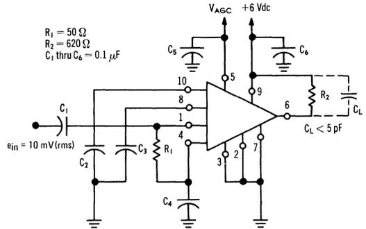
FIGURE 3 – POWER GAIN TEST CIRCUIT @ 60 MHz
