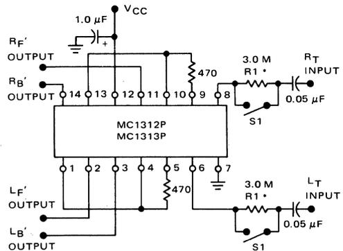
\* R1 is used for input impedance measurement.
