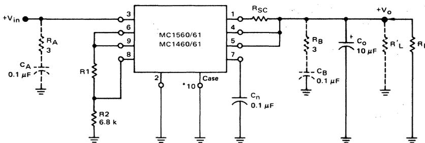
\* G-Package Pin 10 is ground, R package Case is ground.
