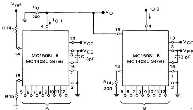
$$V_O = -I_{O1} R_O = \frac{V_{ref}}{R_{141}} \{A\} R_O$$
