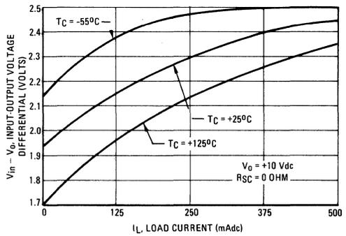
**FIGURE 13 – EFFECT OF INPUT-OUTPUT VOLTAGE DIFFERENTIAL ON INPUT REGULATION**
