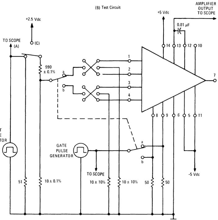
(Pin numbers shown on this page denote the pin numbers for the flat package only; to ascertain the corresponding pin numbers for the dual in-line package, refer to the circuit schematic on the second page.)
