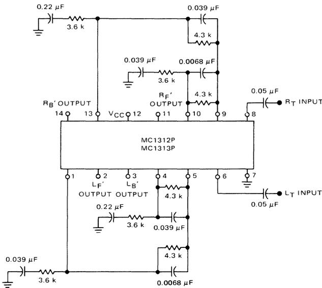
Note: For optimum performance  $\pm 5\%$  tolerance components are recommended with the exception of the input capacitors.
