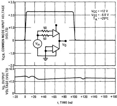
FIGURE 8 – OUTPUT PULSE STRETCHING WITH CAPACITIVE LOADING
