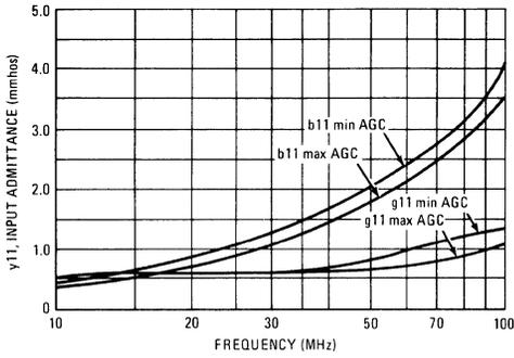
FIGURE 6 – SINGLE-ENDED INPUT ADMITTANCE (PIN 3 BYPASSED TO GROUND)
