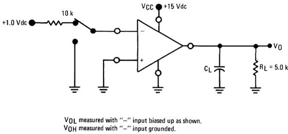
**FIGURE 8 – PEAK-TO-PEAK OUTPUT VOLTAGE**
