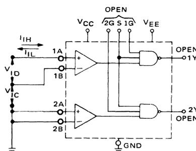
NOTE: Each pair of differential inputs is tested separately. The inputs of the other pair are grounded.
