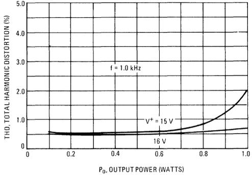
FIGURE 13 – TOTAL HARMONIC DISTORTION
