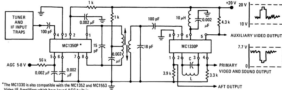
\*The MC1330 is also compatible with the MC1352 and MC1553 Video IF Amplifiers which have keyed AGC built-in.
