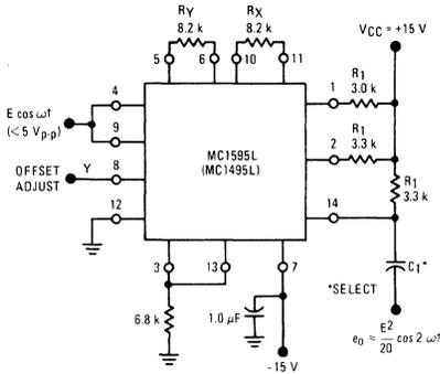
When two equal cosine waves are applied to X and Y, the result is a wave shape of twice the input frequency. For this example the input was a 10 kHz signal, output was 20 kHz.
