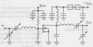
FIGURE 2 — A Typical Common Source MOSFET
