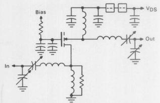
FIGURE 3 — A Typical Common Gate MOSFET
