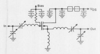
FIGURE 4 — A Typical Common Drain, Narrow Band MOSFET Power Amplifier Circuit
