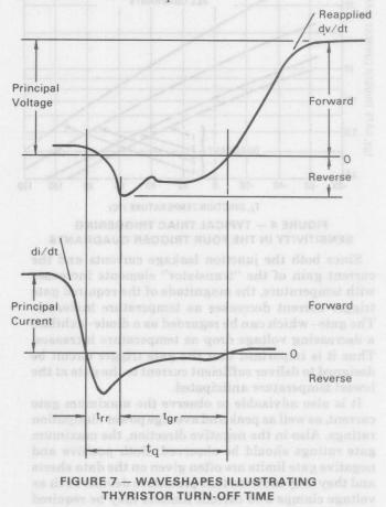
Turn-off time depends upon a number of circuit conditions including on-state current prior to turn-off, rate of change of current during the forward-to-reverse transition, reverse-blocking voltage, rate of change of reapplied forward voltage, the gate bias, and junction temperature, Increasing junction temperature and on-state current both increase turn-off time and have a more significant effect than any of the other factors. Negative gate bias will decrease the turn-off time.
