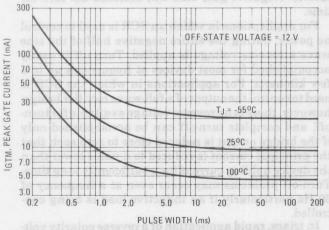
FIGURE 5 — TYPICAL BEHAVIOR OF GATE TRIGGER CURRENT AS PULSE WIDTH AND TEMPERATURE ARE VARIED
