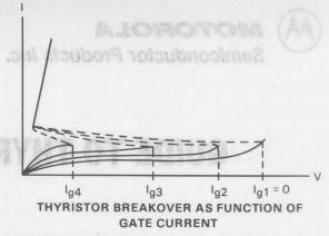
FIGURE 2 — Thyristor Characteristics Illustrating Breakover as a Function of Gate Current.
