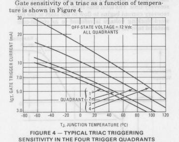
Since both the junction leakage currents and the current gain of the "transistor" elements increases with temperature, the magnitude of the required gate trigger current decreases as temperature increases. The gate - which can be regarded as a diode - exhibits a decreasing voltage drop as temperature increases. Thus it is important that the gate trigger circuit be designed to deliver sufficient current to the gate at the lowest temperature anticipated.
