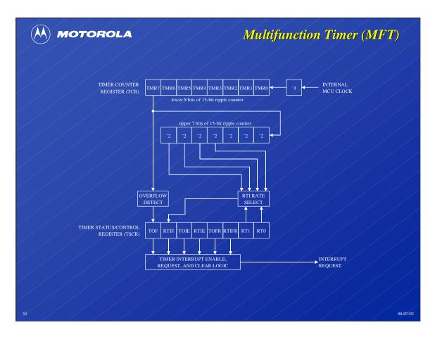
Simple 68HC05 devices have a simple timer, the multifunction timer (MFT). Consisting of a 15-bit ripple counter, the lower eight bits of which can be read from the timer counter register (TCR), the MFT is clocked at one fourth the internal MCU clock frequency.
