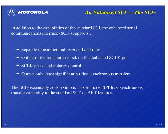
As noted above, the SCI+ can perform simple, output-only, synchronous transmissions in addition to its standard UART functions.
