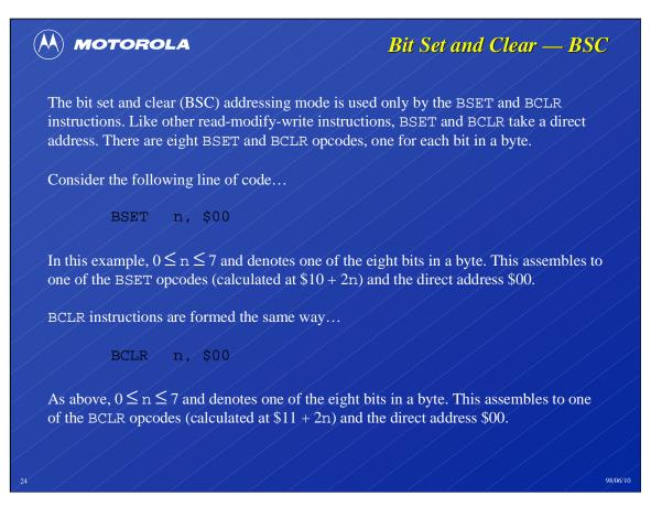
Bit set and bit clear instructions have a unique addressing mode that is similar to direct mode. The source code format for these instructions is:
