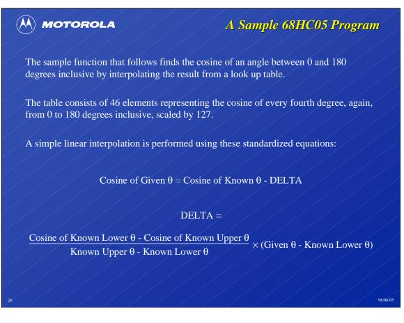
To simplify the interpolation math, the look up table includes the cosine of every fourth degree  $(0^{\circ}, 4^{\circ}, 8^{\circ}, \text{ and so on})$  rather than, say, every fifth degree  $(0^{\circ}, 5^{\circ}, 10^{\circ}, \text{ and so on})$ .
