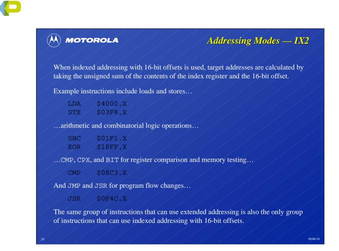
Instructions that use indexed addressing with 16-bit offsets can read from or write to any location in the 68HC05 memory map. These instructions always require three bytes of storage.
