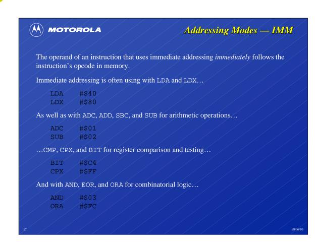
Immediate addressing is used to specify values that remain constant during program execution. On the 68HC05, the address from which an immediate value is read is always one more than the address of the instruction reading that value.
