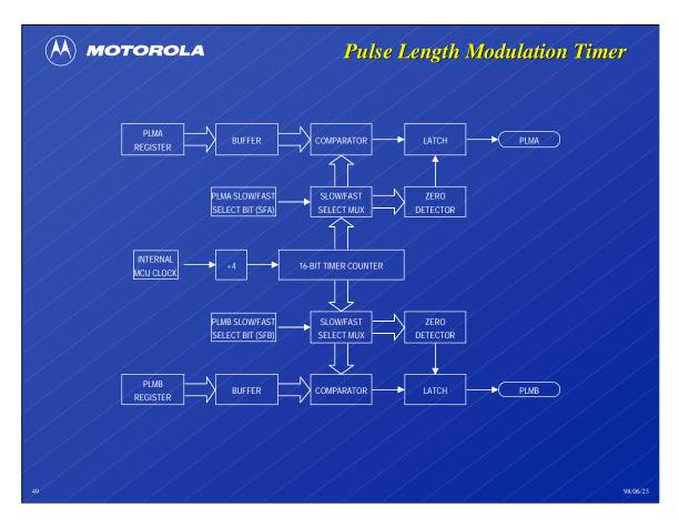
The pulse length modulation (PLM) timer has two channels, each with an 8-bit, buffered duty cycle register, an 8-bit comparator, zero detection circuitry, a slow/fast rate multiplexer, and a latch that drives an associated output pin.
