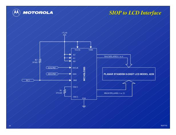
The cycling computer can display the following statistics on its Planar Standish 8-digit LCD: temperature, relative humidity, speed, distance traveled, pulse rate, and stopwatch time.
