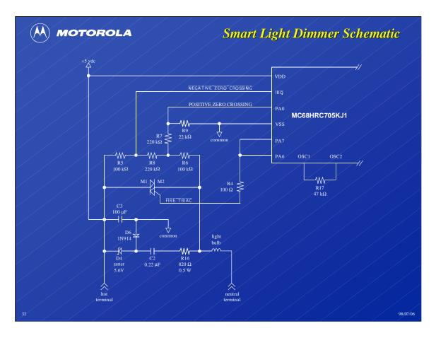
All 68HC05 devices have some number of pins, either dedicated or shared with other peripherals, that can be used as digital inputs and outputs. The partial circuit for the smart light dimmer, shown above, illustrates two useful features available on the I/O pins of the MC68HRC705KJ1.
