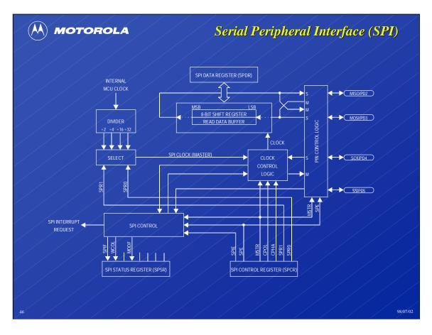
The serial peripheral interface (SPI) is the full-duplex, synchronous data transfer mechanism upon which the simpler serial input/output port (SIOP) is based. Differences between the SIOP and the SPI are discussed below.
