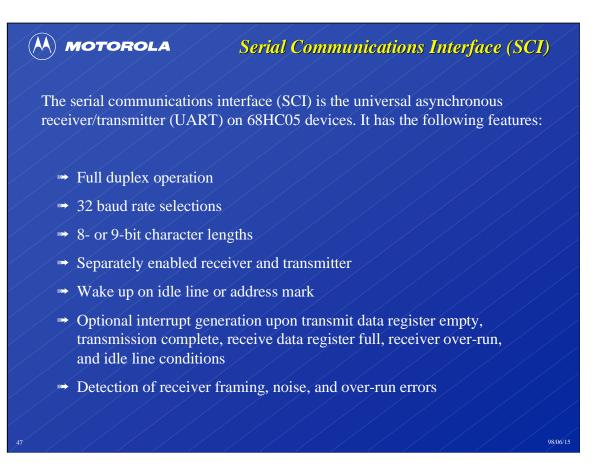
The serial communications interface (SCI) is the universal asynchronous receiver/transmitter (UART) peripheral on 68HC05 devices.
