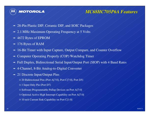
Based on a Motorola University Design Contest entry, this next example makes extensive use of the features found on the MC68HC705P6A. The peripherals used in this application (analog-to-digital converter, timer, serial input/output port, and I/O pins) are found on many different 68HC05 devices.
