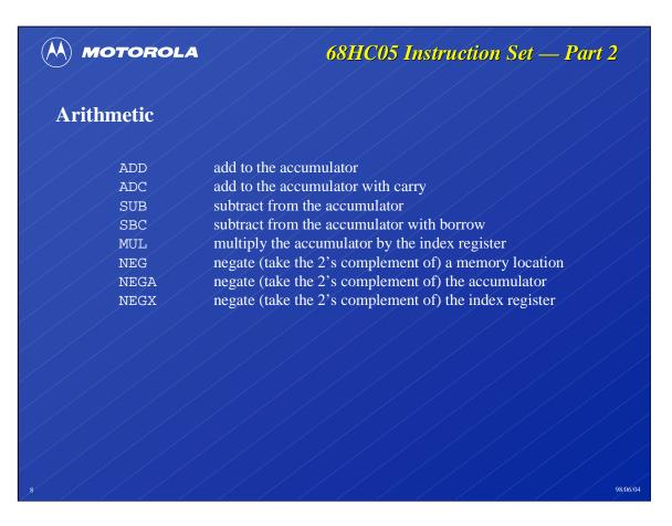
The ADD and SUB instructions, respectively, add or subtract a byte to or from the accumulator. ADC and SBC do the same but with a carry or borrow if the condition code register carry bit (C) is set.
