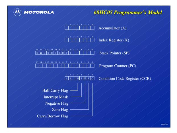
The 68HC05 central processor unit (CPU) consists of an accumulator (A), an index register (X), a stack pointer (SP), a program counter (PC), and a condition code register (CCR).
