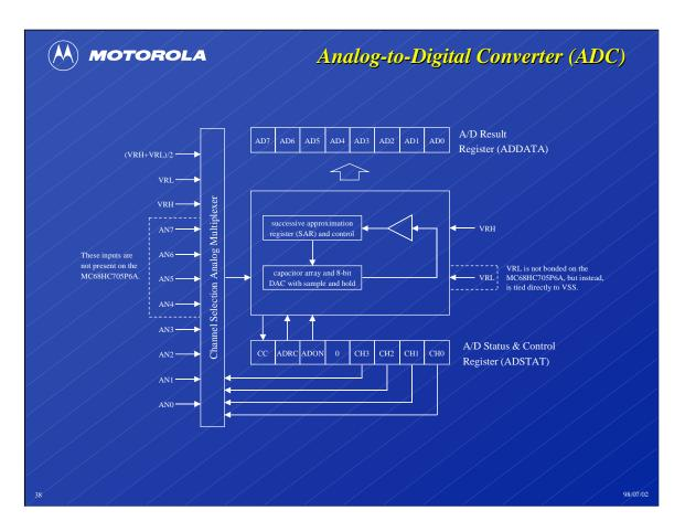
The MC68HC705P6A incorporates a 4-channel version of the 8-bit analog-todigital converter (ADC) used on several 68HC05 devices.
