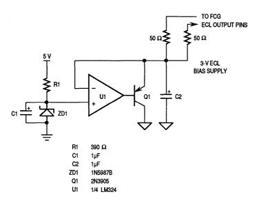
Figure 5-5. ECL Test Load
