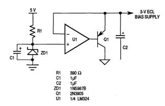
Figure 4-5. Discrete Bias Supply Generator
