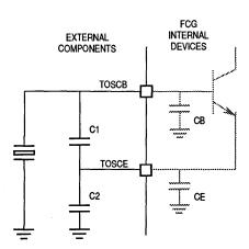
Figure 3-5. Transmitter Crystal Oscillator
