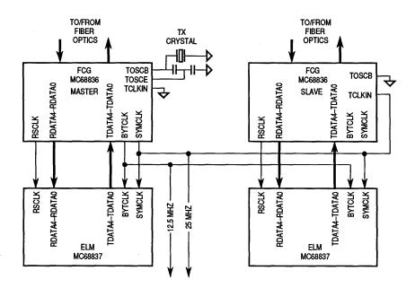
Figure 4-1. Dual Attached Station
