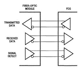
Figure 4-2. Differential Raised ECL Interface
