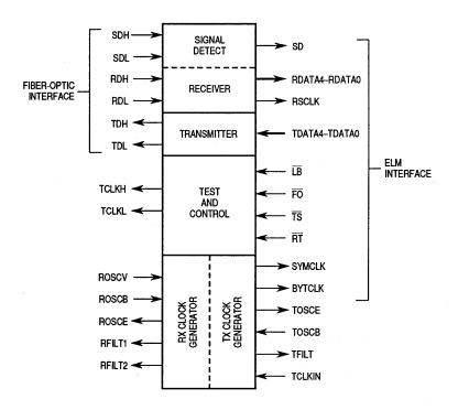
Figure 3-1. FCG Functional Pinout
