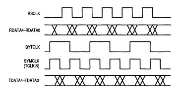
Figure 2-2. FCG-ELM Functional Timing
