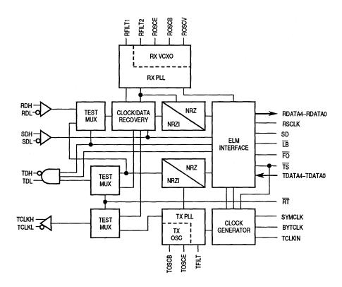
Figure 2-1. FCG Block Diagram
