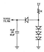
Figure 5-1. TTL Test Load
