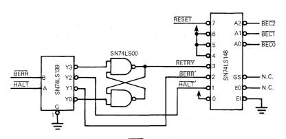
Figure 4-11. Example BEC Signal Generation Circuit
