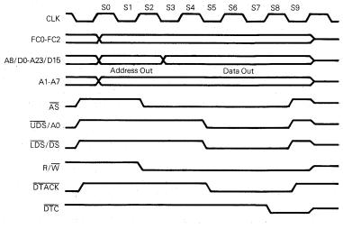
Figure 4-7. Dual Address Write Cycle Timing Diagram
