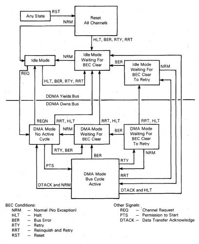
Figure 4-19. Bus Exception Control Flow Diagram
