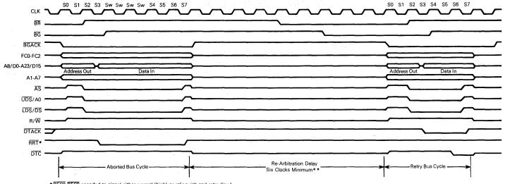
\*BEC2-BEC0 encoded to signal either normal (high) or relinquish and retry (low).
