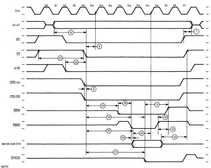
Timing measurements are referenced to and from a low voltage of 0.8 volts and a high voltage of 2.0 volts, unless otherwise noted. The voltage swing through this range should start outside and pass through the range such that the rise or fall will be linear between 0.8 volts and 2.0 volts.
