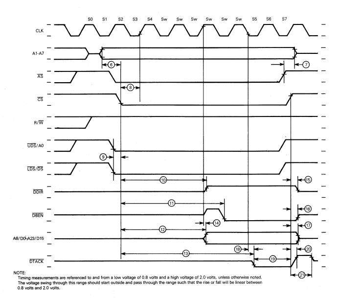
Figure 6-4. MPU Read Cycle Timing Diagram
