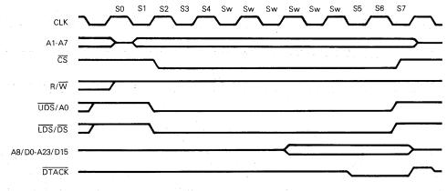
Figure 4-3. MPU Read Cycle Timing Diagram
