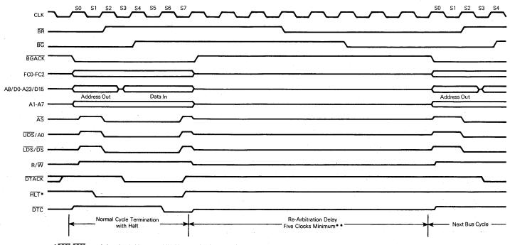
\* BEC2-BEC0 encoded to signal either normal (high) or halt (low). \*\* This minimum delay will occur if BG is asserted prior to the clock edge on which BR is asserted.
