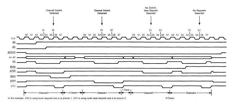
Figure 4-21. Inter-Cycle Overhead Timing Diagram
