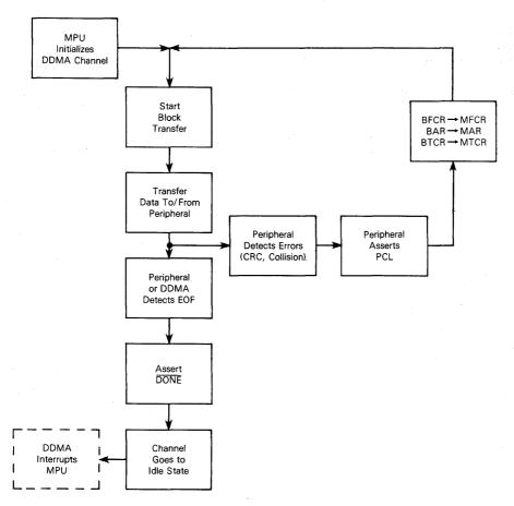
Figure 5-4. Reload Operation Flowchart
