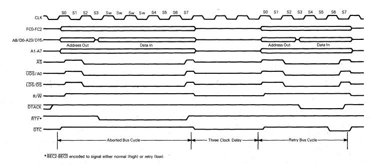
Figure 4-16. Retry Operation Timing Diagram
