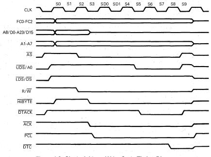
Figure 4-9. Single Address Write Cycle Timing Diagram
