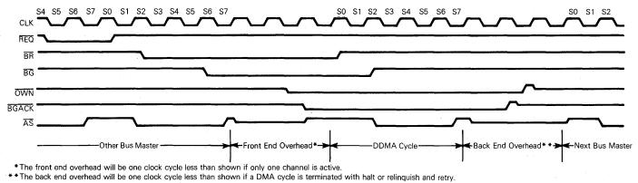
Figure 4-20. Bus Arbitration Timing Diagram
