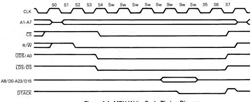
Figure 4-4. MPU Write Cycle Timing Diagram
