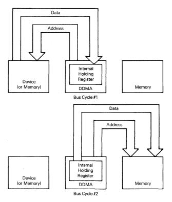
Figure 1-4. Dual-Address Transfer Sequence
