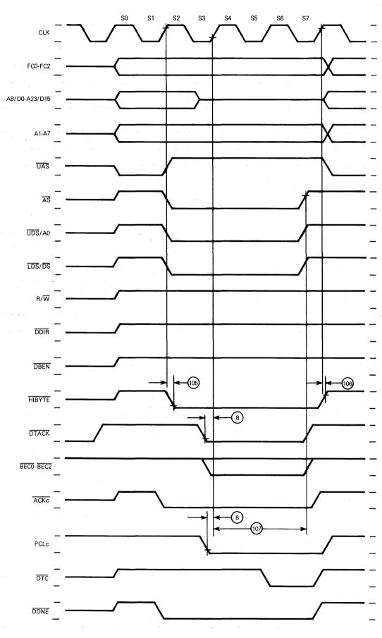
NOTE: Timing measurements are referenced to and from a low voltage of 0.8 volts and a high voltage of 2.0 volts, unless otherwise noted. The voltage swing through this range should start outside and pass through the range such that the rise or fall will be linear between 0.8 volts and 2.0 volts.
