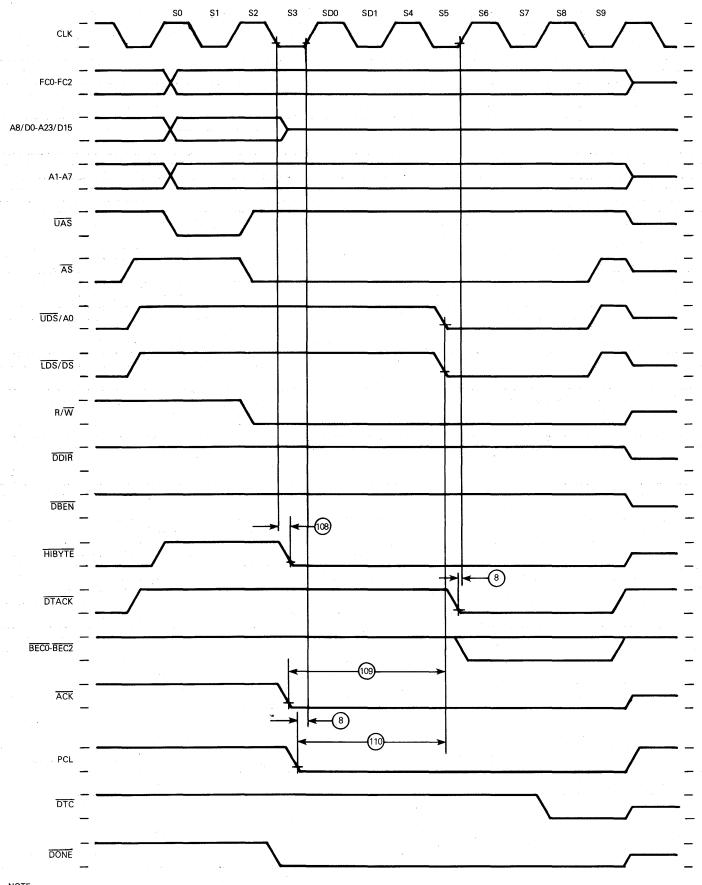
NOTE: Timing measurements are referenced to and from a low voltage of 0.8 volts and a high voltage of 2.0 volts, unless otherwise noted. The voltage swing through this range should start outside and pass through the range such that the rise or fall will be linear between 0.8 volts and 2.0 volts.
