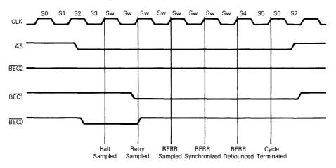
Figure 4-13. BEC Debouncer Timing Diagram
