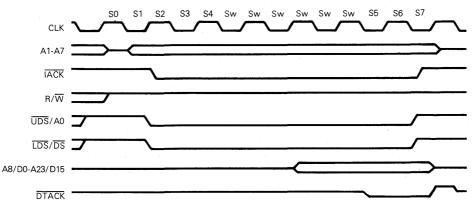
Figure 4-5. Interrupt Acknowledge Cycle Timing Diagram
