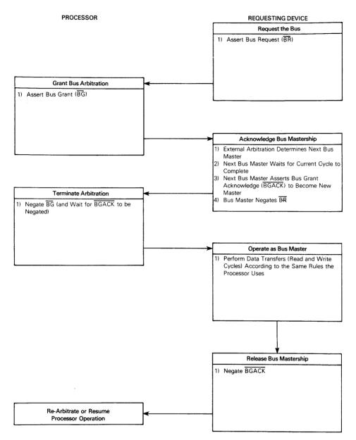
Figure 4-11. Bus Arbitration Cycle Flowchart
