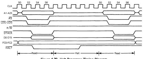
Figure 4-20. Halt Processor Timing Diagram
