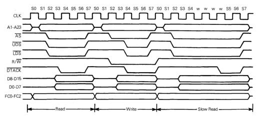
Figure 4-4. Read and Write Cycle Timing Diagram
