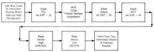
NOTE: SSP refers to the value of the supervisor stack pointer before the interrupt occurs.
