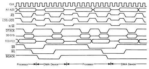
Figure 4-12. Bus Arbitration Cycle Timing Diagram
