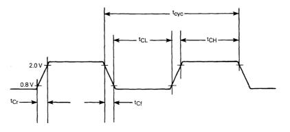
Figure 8-5. Clock Input Timing Diagram
