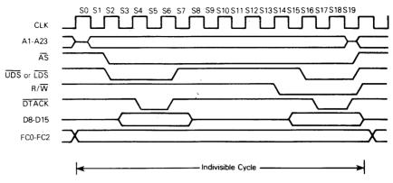
Figure 4-10. Read-Modify-Write Cycle Timing Diagram
