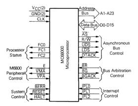
Figure 4-1. Input and Output Signals
