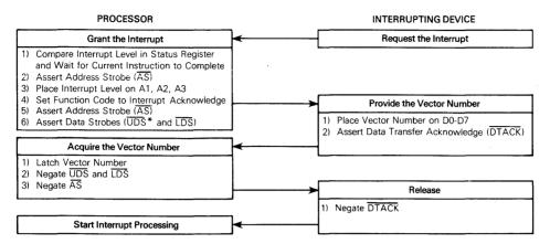
\*Although a vector number is one byte, both data strobes are asserted due to the microcode used for exception processing. The processor does not recognize anything on data lines D8 through D15 at this time.
