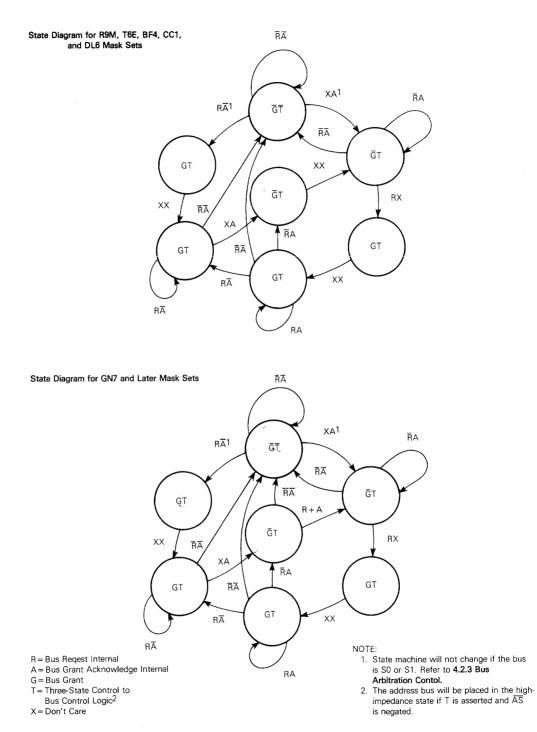
Figure 4-13. MC68000 Bus Arbitration Unit State Diagram
