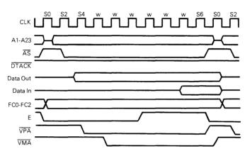
Figure 6-2. MC68000 to M6800 Peripheral Timing - Best Case
