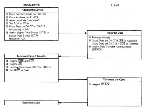
Figure 4-7. Byte Write Cycle Flowchart
