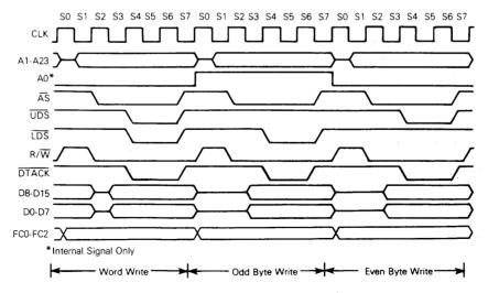
Figure 4-8. Word and Byte Write Cycle Timing Diagram
