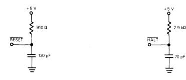
Figure 8-1. RESET Test Load
