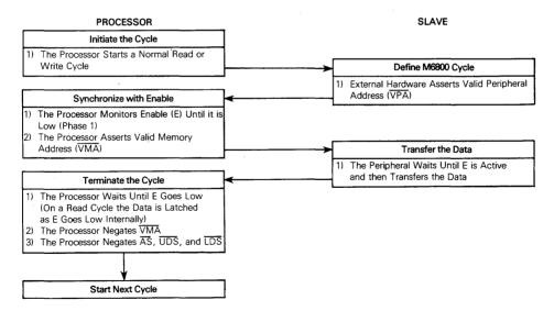
Figure 6-1. M6800 Interfacing Flowchart
