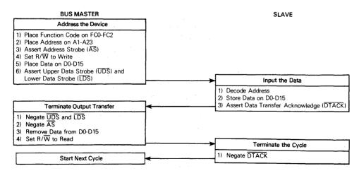
Figure 4-6. Word Write Cycle Flowchart
