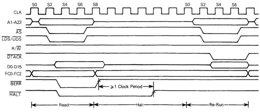
Figure 4-19. Re-Run Bus Cycle Timing Diagram
