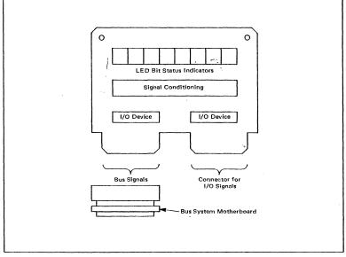
Figure 13.5 Possible Mechanical I/O Card Arrangement
