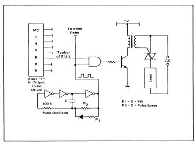
Figure 6.16 Picket Fence Triac Firing
