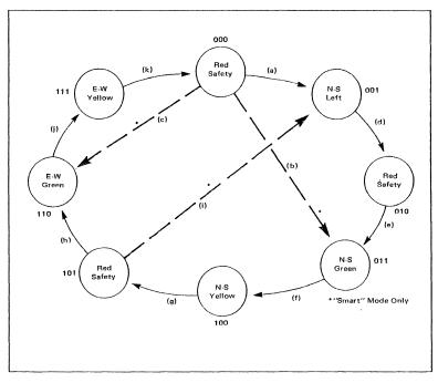
Figure 11.1 Traffic Controller - Simplified State Diagram
