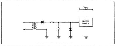
Figure 6.11 Phase Detection of AC Signals
