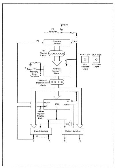
Figure 5.1 Demonstration System Block Diagram
