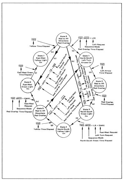
Figure 11.2 Complete State Diagram with Conditional Linkages
