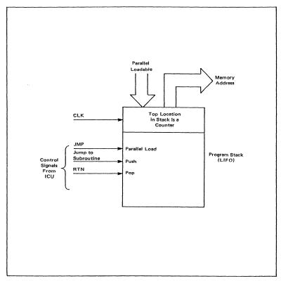
Figure 12.2 Block Diagram of Subroutine Structure
