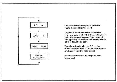
Figure 2.5 Example LOAD = A • B Program
