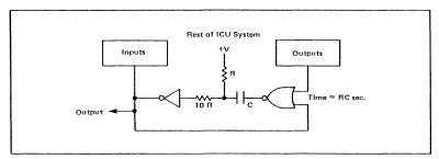
Figure 6.2 CMOS Monostable Timer
