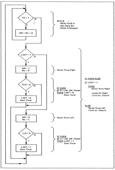
Figure 10.4 Structured Flow Chart for Shuttle Motor Control
