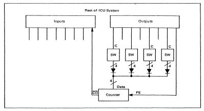
Figure 6.5 Multiple Interval Timer
