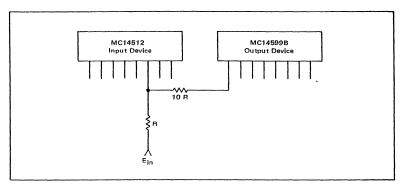
Figure 6.17 Adding Input Signal Hysteresis
