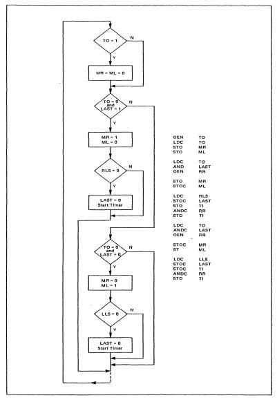
Figure 10.5 Final Structured Flow Chart and Motor Control Code
