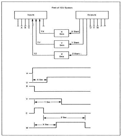
Figure 6.3 Complex Timing Waveforms
