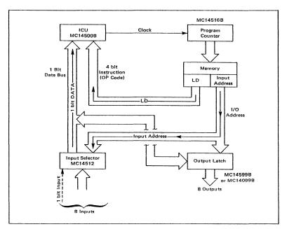
Figure 2.1 Typical Small System Organization & Data Flow
