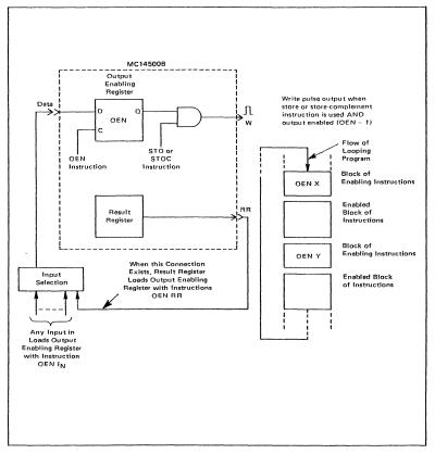
Figure 7.1 Output Enable Concepts
