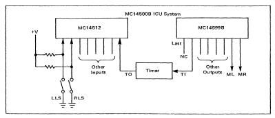
Figure 10.3 Shuttle Motor Signal Connections
