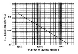
Figure 1.4 Typical Clock Frequency Versus Resistor (R<sub>C</sub>)
