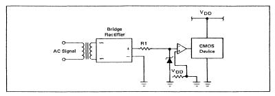
Figure 6.10 Amplitude Detection of AC Signal
