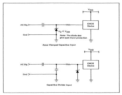
Figure 6.12 Capacitive Input Schemes
