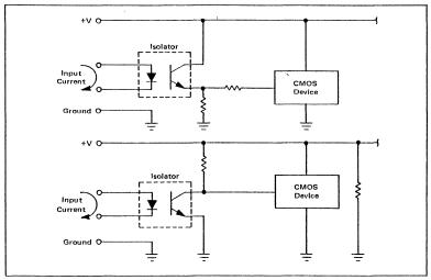
Figure 6.9 Optically Isolated Inputs
