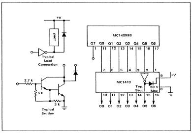
Figure 6.13 High Current Output Buffers
