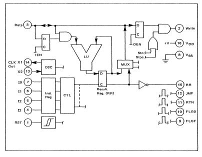
Figure 1.2 MC14500B Block Diagram
