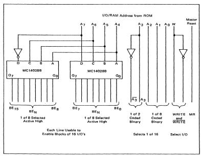
Figure 13.2 I/O Card Enables for 8 Bit Address
