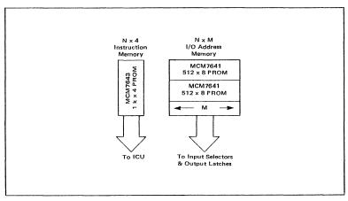
Figure 4.3 An Approach to I/O Address Expansion
