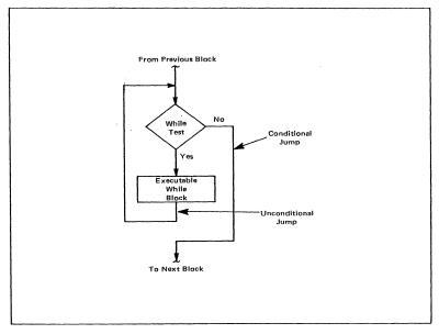
Figure 9.2 Jump - Back - While Structure
