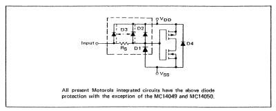
Figure 6.8 - Schematic Diagram, Diode-Resistor Input Protection
