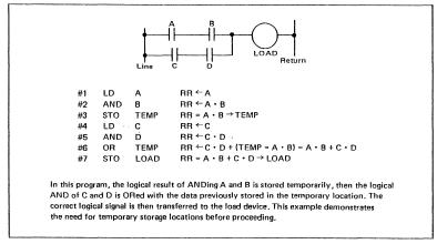
Figure 3.8 Correct Method of Solving the Problem
