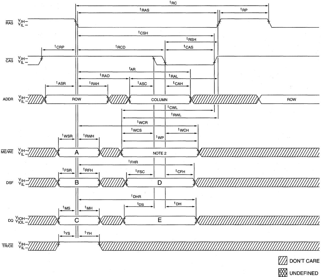
**NOTE:** 1. The logic states of "A", "B", "C", "D" and "E" determine the type of WRITE operation performed. See the Write Cycle Function Table for a detailed description.
