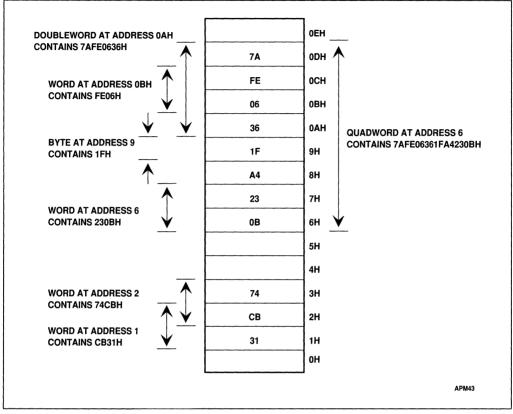
Figure 3-3. Bytes, Words, Doublewords and Quadwords in Memory
