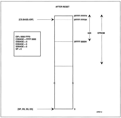
Figure 16-3. Processor State After Reset
