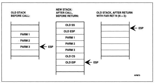
Figure 12-9. Stack Frame During Interlevel Call
