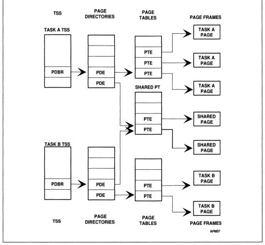
Figure 13-7. Overlapping Linear-to-Physical Mappings
