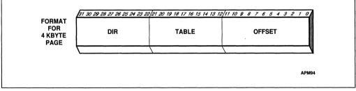
Figure 11-12. Format of a Linear Address
