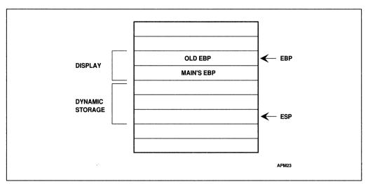
Figure 4-16. Stack Frame After Entering MAIN
