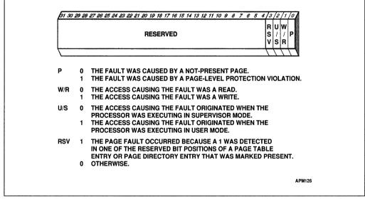
Figure 14-7. Page Fault Error Code
