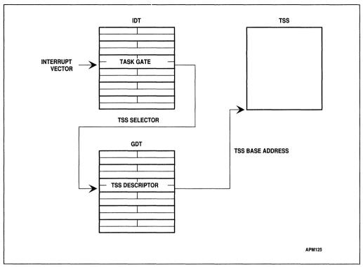
Figure 14-5. Interrupt Task Switch
