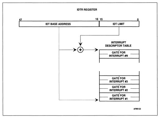
Figure 14-1. IDTR Locates IDT in Memory
