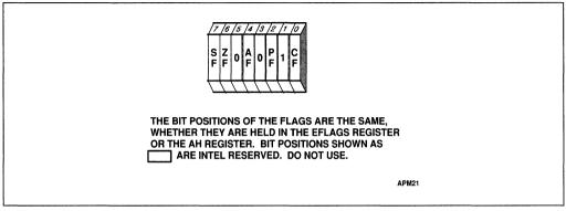
Figure 4-20. Low Byte of EFLAGS Register
