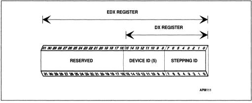
Figure 16-1. Contents of the EDX Register After Reset
