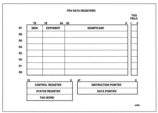
Figure 6-1. Floating-point Unit Register Set
