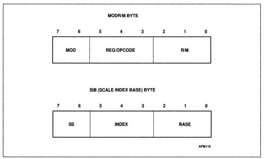
Figure 25-2 shows the formats of the ModR/M and SIB bytes.
