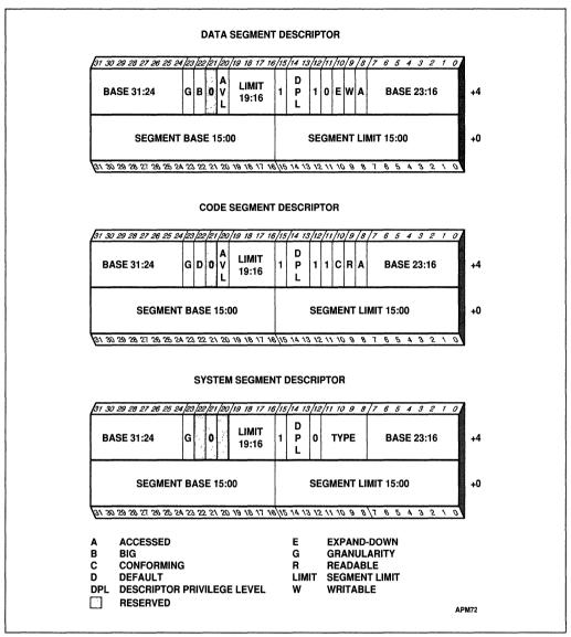
Figure 12-1. Descriptor Fields Used for Protection
