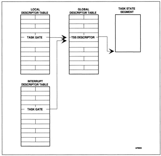
Figure 13-5. Task Gates Reference Tasks
