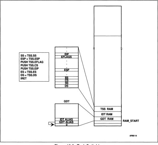
Figure 16-6. Task Switching (Lines 282-296 of List File)
