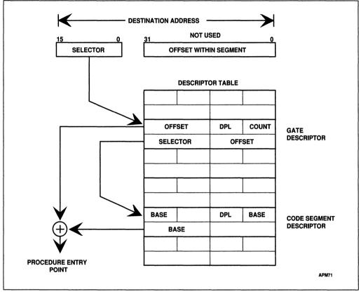
Figure 12-6. Call Gate Mechanism
