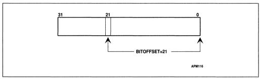
Figure 25-3. Bit Offset for BIT[EAX,21]
