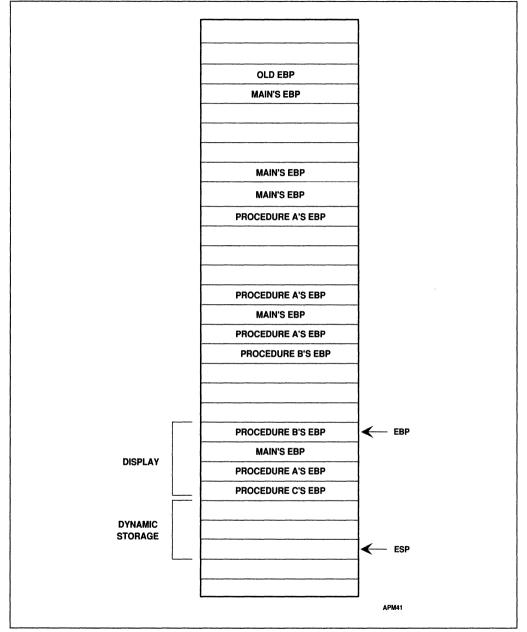
Figure 4-19. Stack Frame After Entering PROCEDURE C
