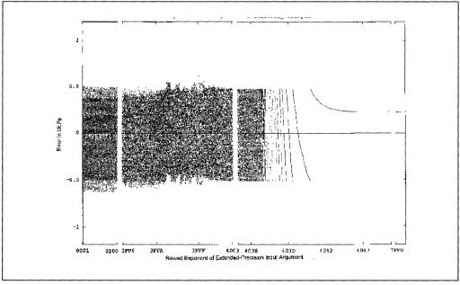
Figure G-22. Scatterplot for FPATAN (0001-7FFD)
