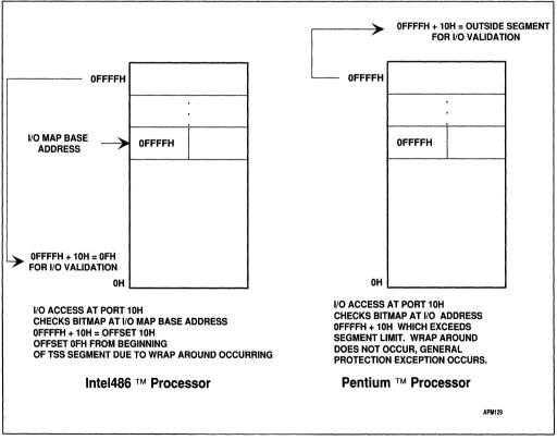
Figure 23-3. I/O Map Base Address Differences
