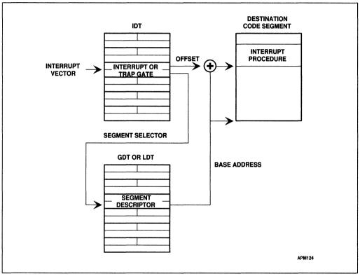
Figure 14-3. Interrupt Procedure Call
