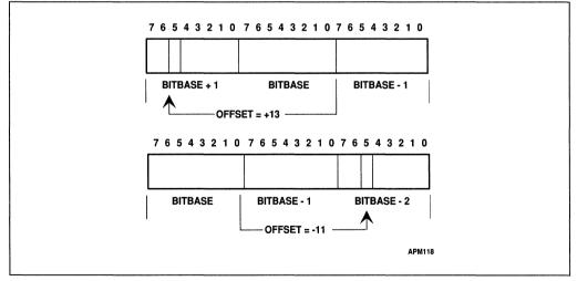
Figure 25-4. Memory Bit Indexing
