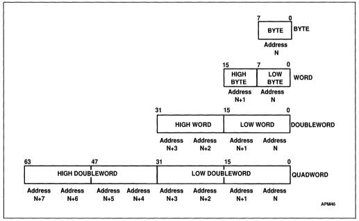
Figure 3-2. Fundamental Data Types
