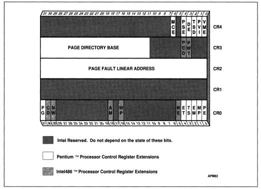
Figure 23-2. Control Register Extensions
