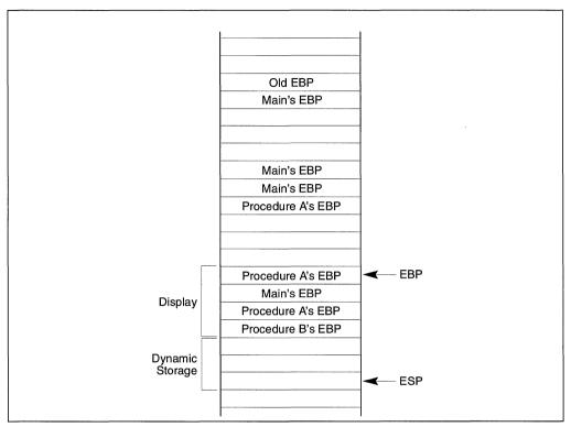
Figure 4-8. Stack Frame after Entering Procedure B
