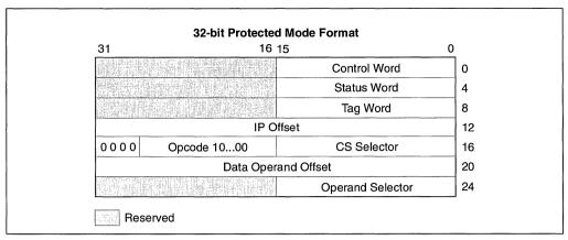
Figure 7-13. Protected-Mode FPU State Image in Memory, 32-Bit Format
