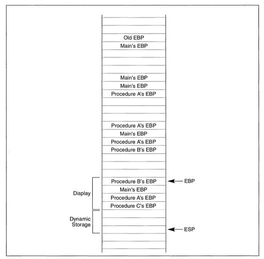
Figure 4-9. Stack Frame after Entering Procedure C
