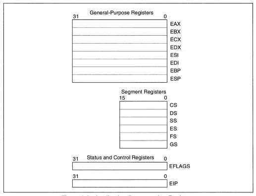
Figure 3-3. Application Programming Registers
