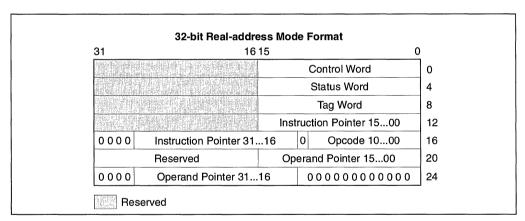
Figure 7-14. Real Mode FPU State Image in Memory, 32-Bit Format
