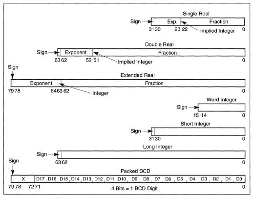
Figure 7-17. Floating-Point Unit Data Type Formats
