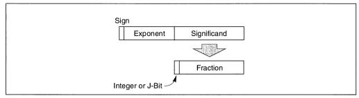
Figure 7-2. Binary Floating-Point Format
