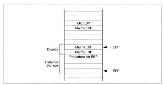
Figure 4-7. Stack Frame after Entering Procedure A
