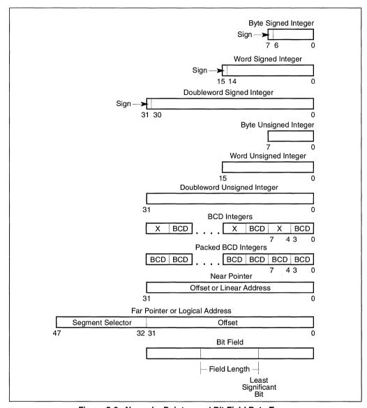
Figure 5-3. Numeric, Pointer, and Bit Field Data Types
