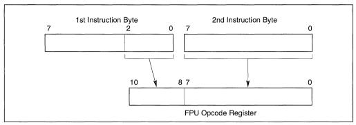
Figure 7-12. Contents of FPU Opcode Registers
