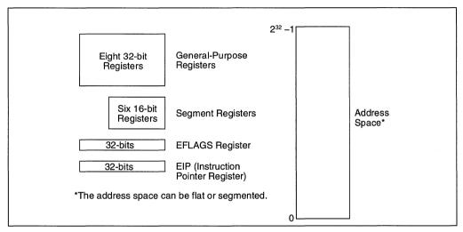
Figure 3-1. Pentium® Pro Processor Basic Execution Environment
