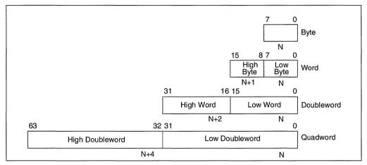
Figure 5-1. Fundamental Data Types
