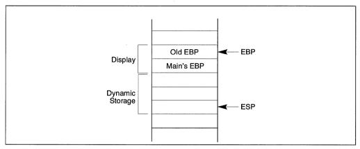
Figure 4-6. Stack Frame after Entering the MAIN Procedure
