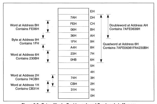
Figure 5-2. Bytes, Words, Doublewords and Quadwords in Memory
