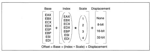
Figure 5-5. Offset (or Effective Address) Computation
