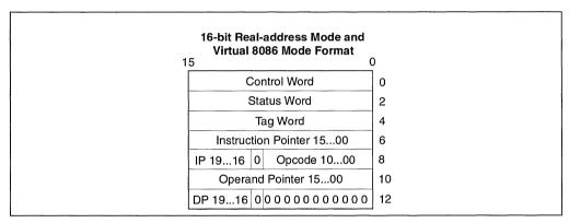
Figure 7-16. Real Mode FPU State Image in Memory, 16-Bit Format
