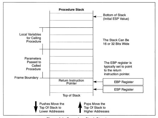
Figure 4-1. Procedure Stack Structure
