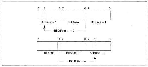
Figure 11-3. Memory Bit Indexing
