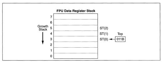
Figure 7-6. FPU Data Register Stack
