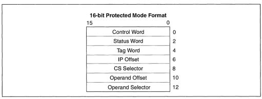
Figure 7-15. Protected-Mode FPU State Image in Memory, 16-Bit Format
