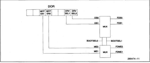
Figure 10-2. Virtual Drive Configuration
