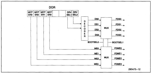
Figure 10-2. Virtual Drive Configuration
