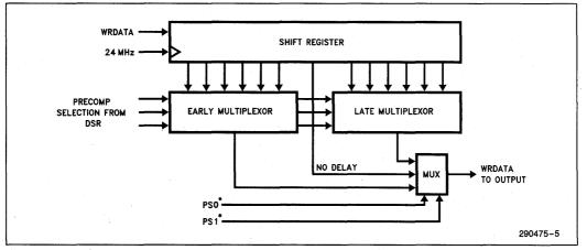
Figure 3-3. Precompensation Block Diagram
