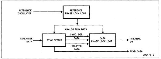
Figure 3-1. Data Separator Block Diagram
