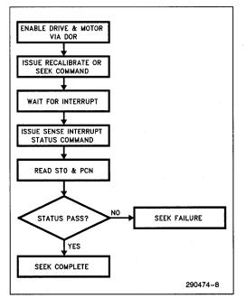
Figure 9-4. Recalibrate and Seek Operations
