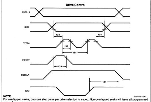
For overlapped seeks, only one step pulse per drive selection is issued. Non-overlapped seeks will issue all programmed step pulses.
