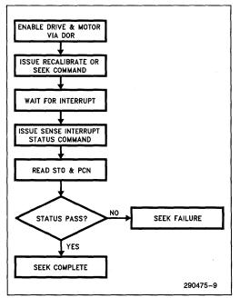
Figure 9-4. Recalibrate and Seek Operations
