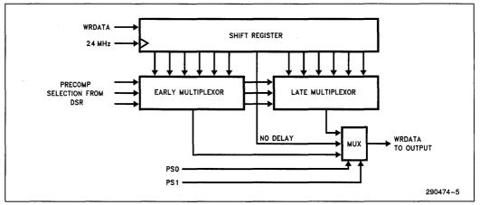
Figure 3-3. Precompensation Block Diagram
