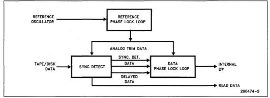
Figure 3-1. Data Separator Block Diagram
