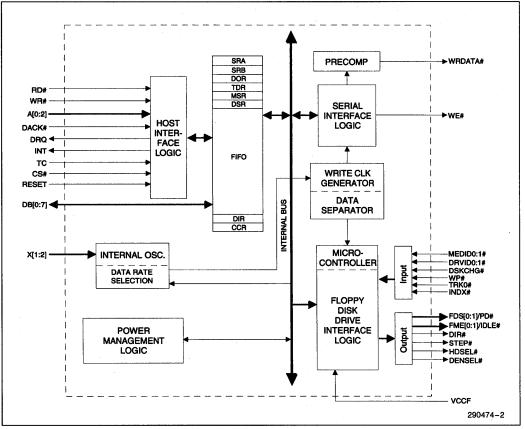
Figure 1-1. 82078 Block Diagram
