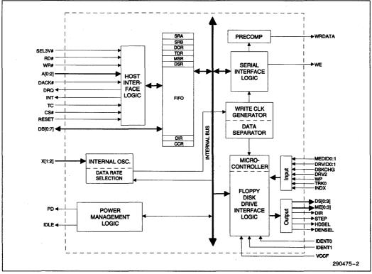
Figure 1-1. 82078 Block Diagram
