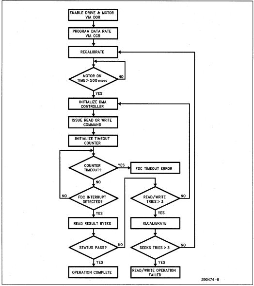
Figure 9-5. Read/Write Operation
