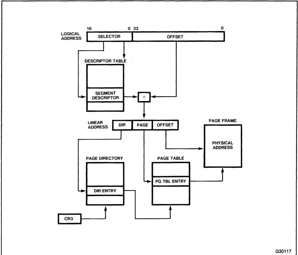
Figure 5-12. 80386 Addressing Mechanism
