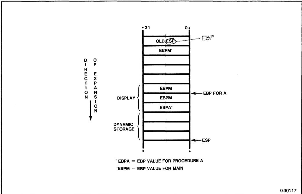
Figure 3-19. Stack Frame for Procedure A
