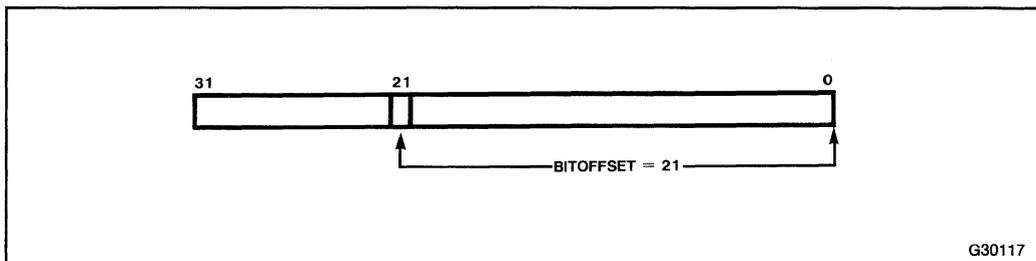
Figure 17-3. Bit Offset for BIT[EAX, 21]
