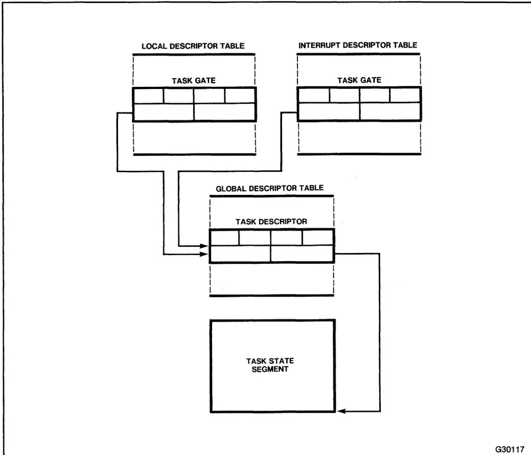
Figure 7-5. Task Gate Indirectly Identifies Task
