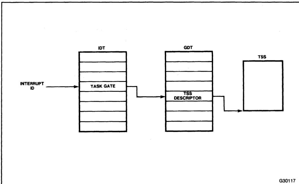
Figure 9-6. Interrupt Vectoring for Tasks
