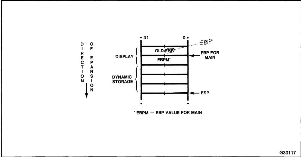
Figure 3-18. Stack Frame for MAIN at Level 1
