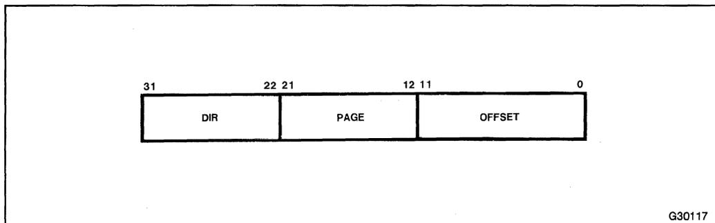
Figure 5-8. Format of a Linear Address
