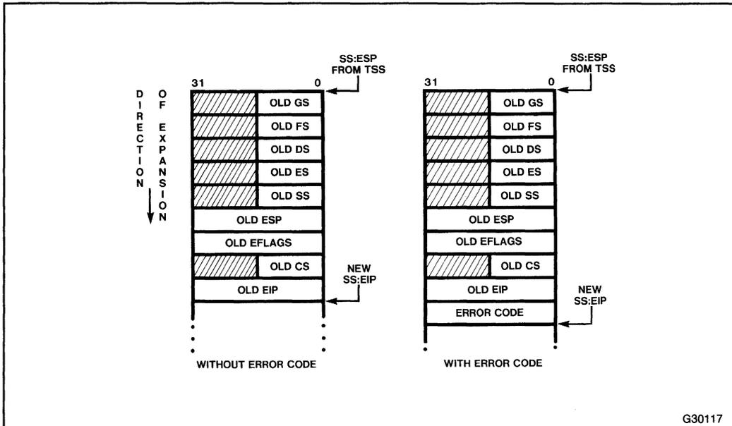
Figure 15-3. PL 0 Stack after Interrupt in V86 Task
