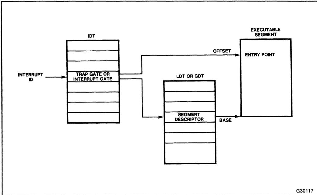
Figure 9-4. Interrupt Vectoring for Procedures
