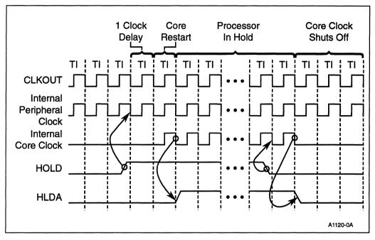
Figure 5-11. HOLD/HLDA During Idle Mode
