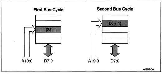
Figure 3-5. 8-Bit Data Bus Word Transfers
