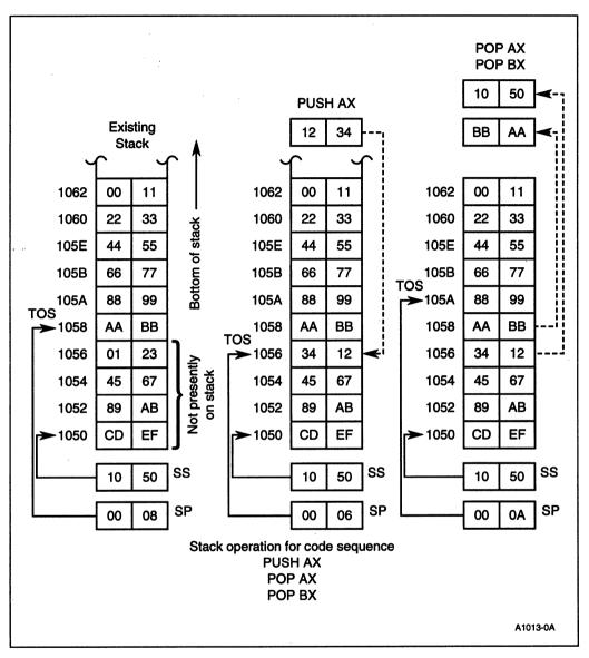
Figure 2-10. Stack Operation
