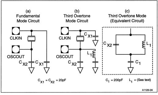
Figure 5-3. Crystal Connections to Microprocessor
