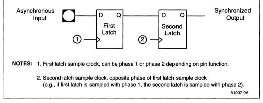
Figure B-1. Input Synchronization Circuit
