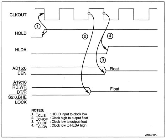
Figure 3-33. Timing Sequence Entering HOLD
