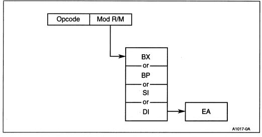
Figure 2-14. Register Indirect Addressing
