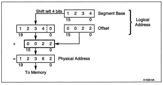
Figure 2-2. Physical Address Generation
