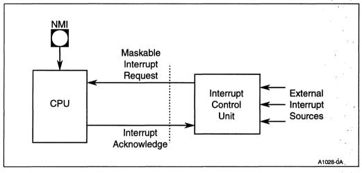
Figure 2-24. Interrupt Control Unit
