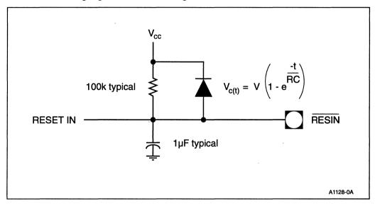
Figure 5-5. Simple RC Circuit for Powerup Reset
