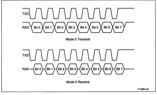
Figure 10-7. Mode 0 Waveforms
