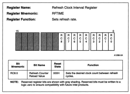
Figure 7-7. Refresh Clock Interval Register
