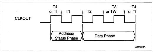
Figure 3-9. T-State and Bus Phases
