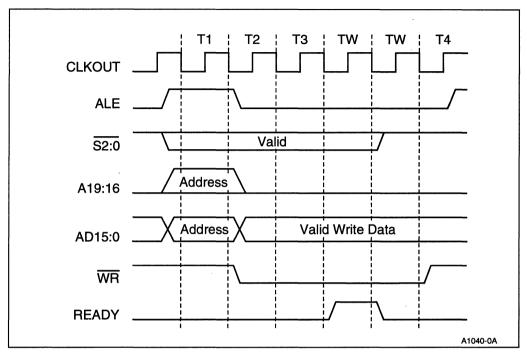
Figure 3-13. Typical Bus Cycle with Wait States
