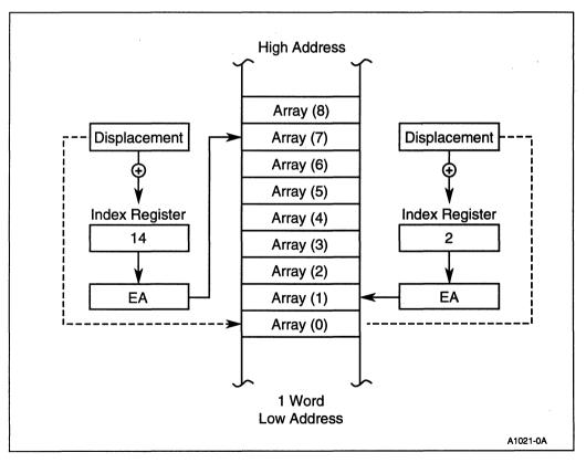
Figure 2-18. Accessing an Array with Indexed Addressing
