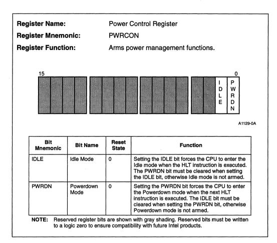
Figure 5-9. Power Control Register
