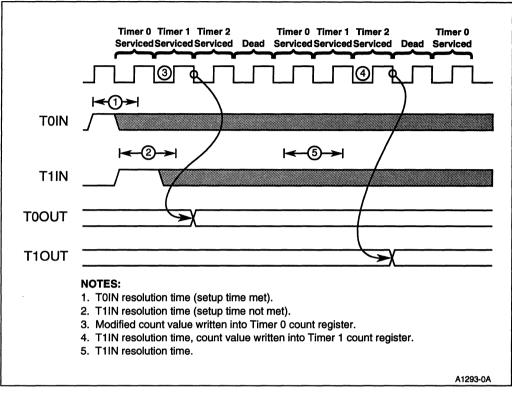
Figure 9-2. Counter Element Multiplexing and Timer Input Synchronization
