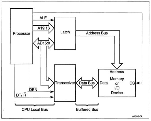
Figure 3-31. Buffered AD Bus System
