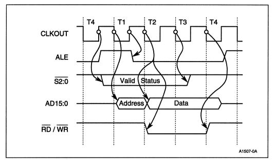
Figure 3-6. Typical Bus Cycle
