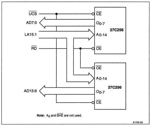
Figure 3-20. Read-Only Device Interface
