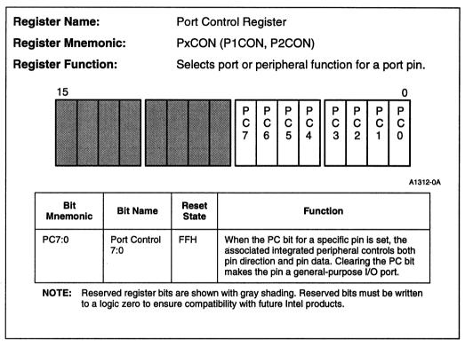
Figure 11-5. Port Control Register (PxCON)
