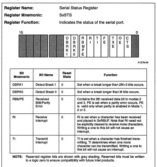
Figure 10-14. Serial Port Status Register (SxSTS)
