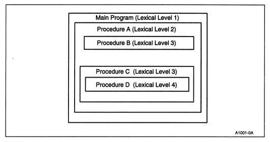
Figure A-2. Variable Access in Nested Procedures
