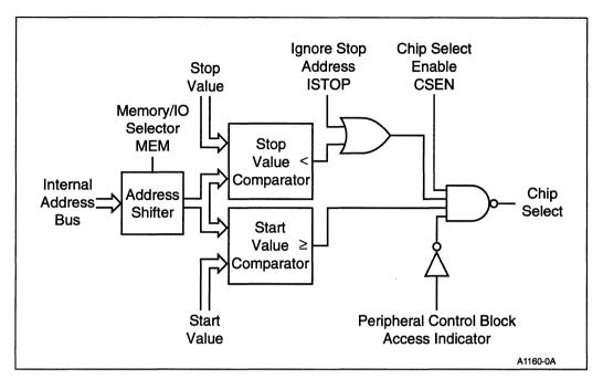
Figure 6-2. Chip-Select Block Diagram
