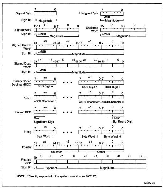
Figure 2-23. 80C186 Modular Core Family Supported Data Types
