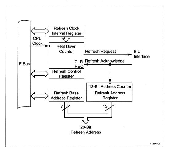
Figure 7-1. Refresh Control Unit Block Diagram
