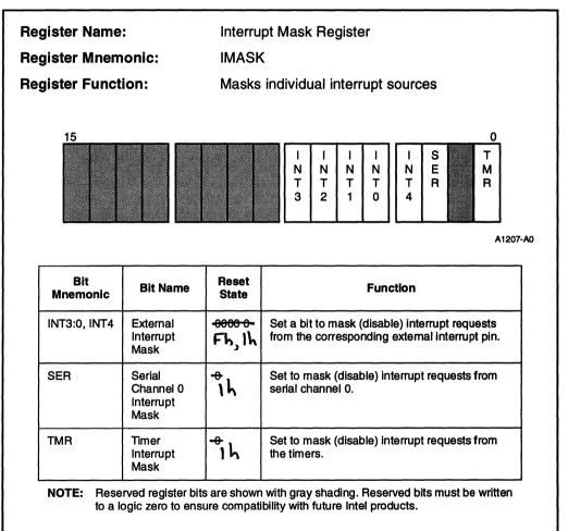
Figure 8-8. Interrupt Mask Register
