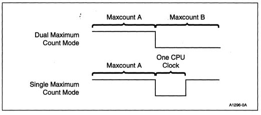
Figure 9-4. Timer/Counter Unit Output Modes
