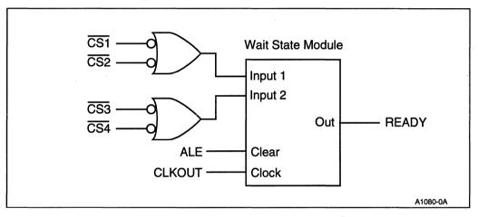
Figure 3-15. Generating a Normally Not-Ready Bus Signal
