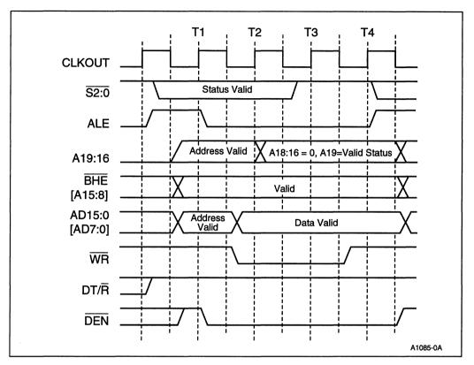
Figure 3-21. Typical Write Bus Cycle
