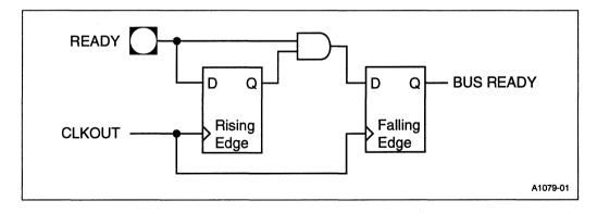
Figure 3-14. READY Pin Block Diagram
