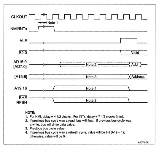
Figure 3-29. Exiting HALT (Active/Idle Mode)
