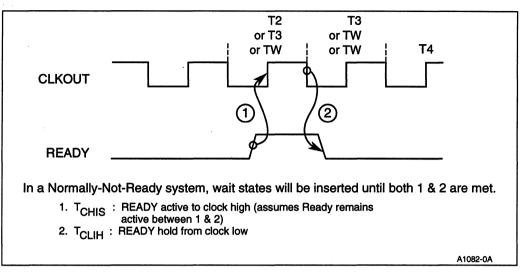
Figure 3-17. Normally Not-Ready System Timing
