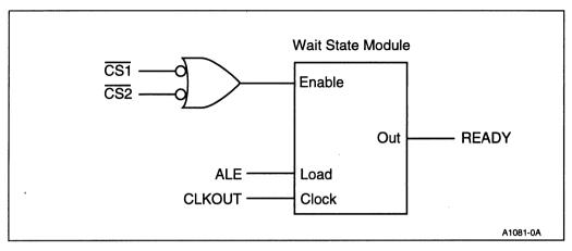
Figure 3-16. Generating a Normally Ready Bus Signal
