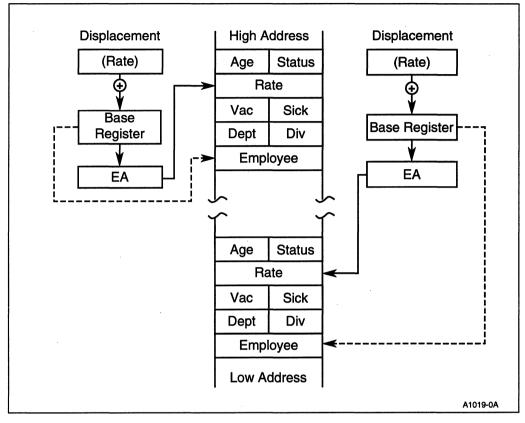
Figure 2-16. Accessing a Structure with Based Addressing
