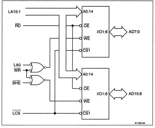
Figure 3-22. 16-Bit Bus Read/Write Device Interface
