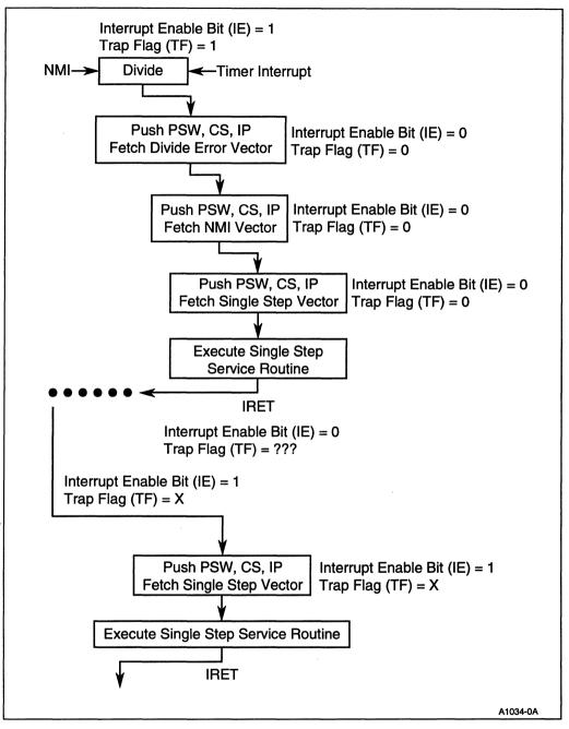
Figure 2-30. Simultaneous NMI, Single Step and Maskable Interrupt
