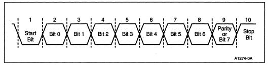
Figure 10-1. Typical 10-Bit Asynchronous Data Frame
