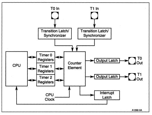
Figure 9-1. Timer/Counter Unit Block Diagram
