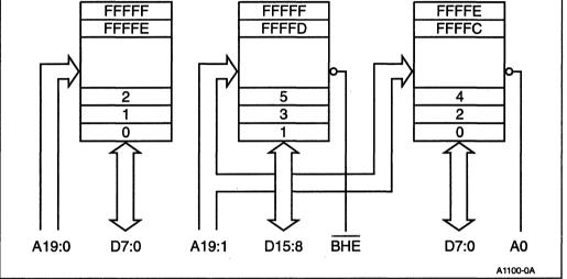
Figure 3-1. Physical Data Bus Models
