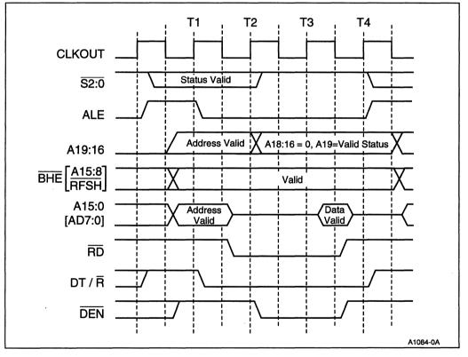
Figure 3-19. Typical Read Bus Cycle
