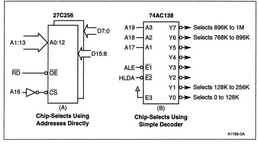
Figure 6-1. Common Chip-Select Generation Methods
