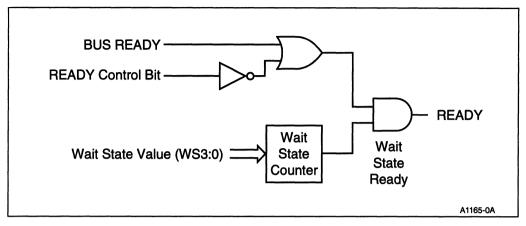
Figure 6-7. Wait State and Ready Control Functions
