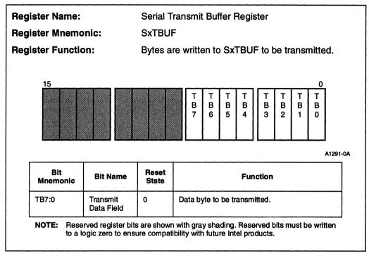
Figure 10-9. Serial Transmit Buffer Register (SxTBUF)
