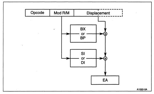
Figure 2-19. Based Index Addressing
