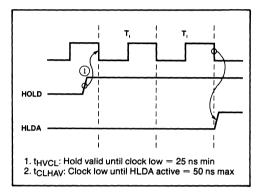
Figure 26. 80186 Idle Bus Hold/HLDA Timing
