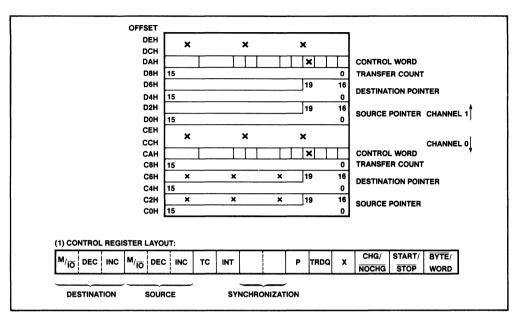
Figure 32. 80186 DMA Register Layout
