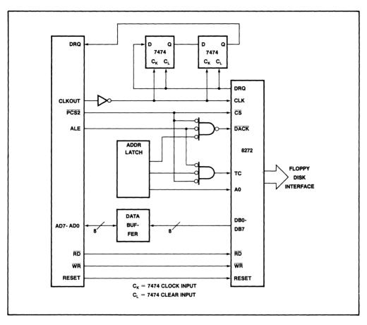
Figure 39. Example 8272/80186 DMA Interface
