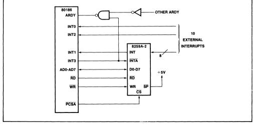
Figure 64. 80186/8259A Interrupt Cascading
