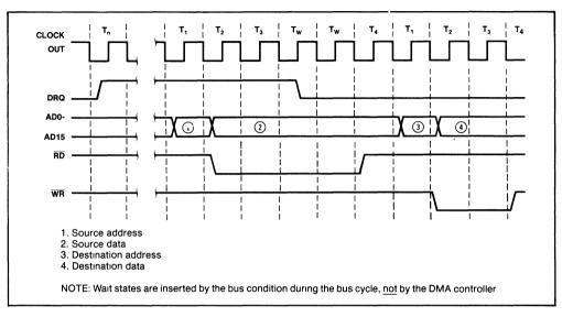
Figure 34. Example DMA Transfer Cycle on the 80186
