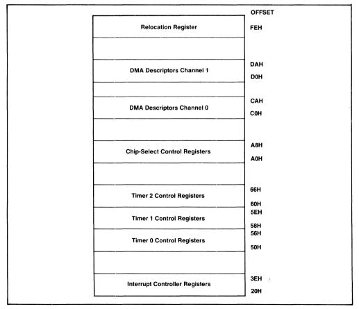
Figure A-1. 80186 Integrated Peripheral Control Block
