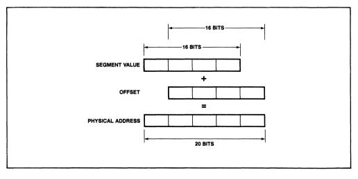
Figure 2. Physical Address Generation in the 80186
