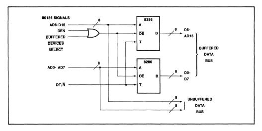
Figure 9. Example 80186 Buffered/Unbuffered Data Bus
