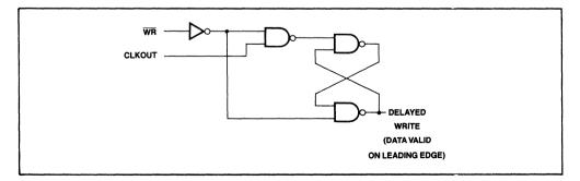
Figure 13. Synthesizing Delayed Write from the 80186
