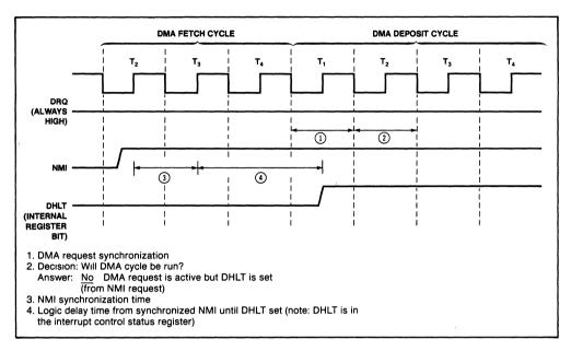
Figure 38. NMI and DMA Interaction
