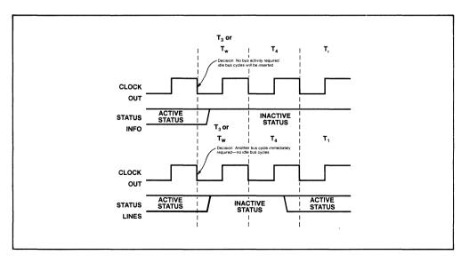
Figure 5. Active-Inactive Status Transitions in the 80186
