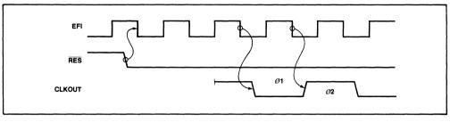
Figure 68. 80186 Clock Generator Reset
