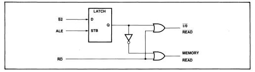
Figure 11. Generating I/O and Memory Read Signals from the 80186 9
