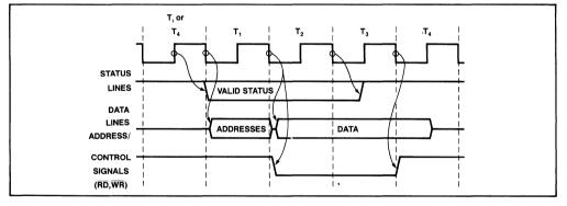
Figure 4. Example Bus Cycle of the 80186
