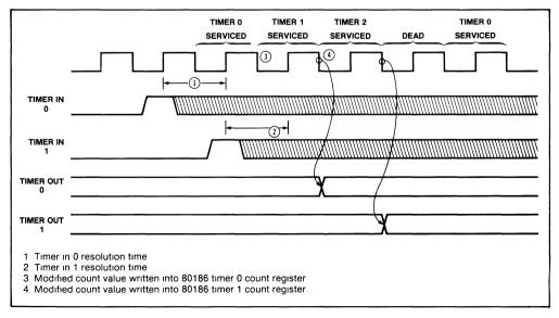
Figure 42. 80186 Counter Element Multiplexing and Timer Input Synchronization
