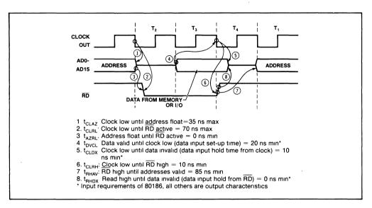
Figure 10. Read Cycle Timing of the 80186
