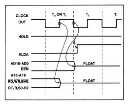
Figure 25. Signal Float/HLDA Timing of the 80186
