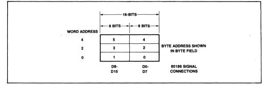
Figure 8. Physical Memory Byte/Word Addressing in the 80186
