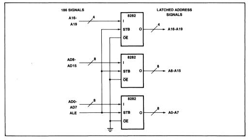
Figure 7. Demultiplexing the Address Bus of the 80186
