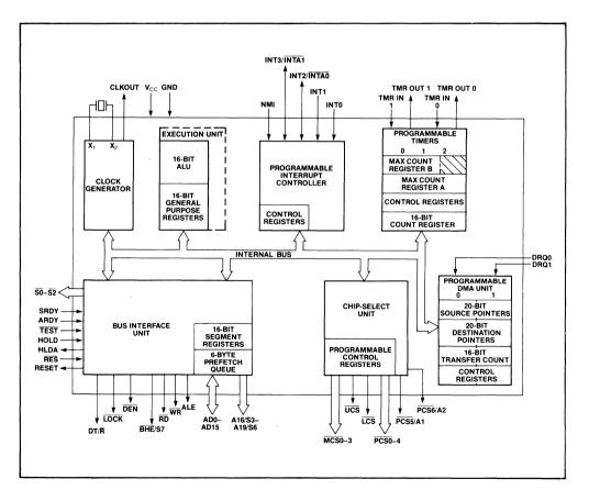
Figure 1. 80186 Block Diagram
