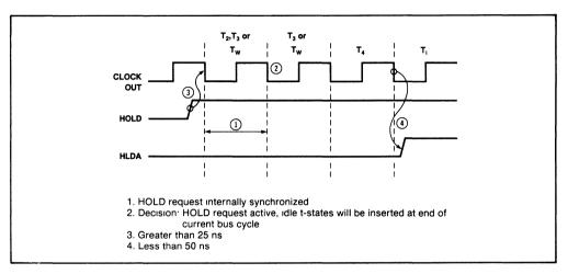
Figure 27A. HOLD/HLDA Timing in the 80186
