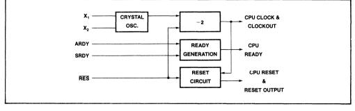
Figure 66. 80186 Clock Generator Block Diagram
