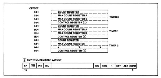
Figure 43. 80186 Timer Register Layout
