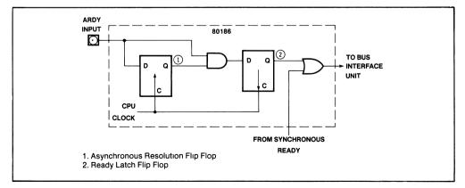
Figure 17. Asynchronous Ready Circuitry of the 80186
