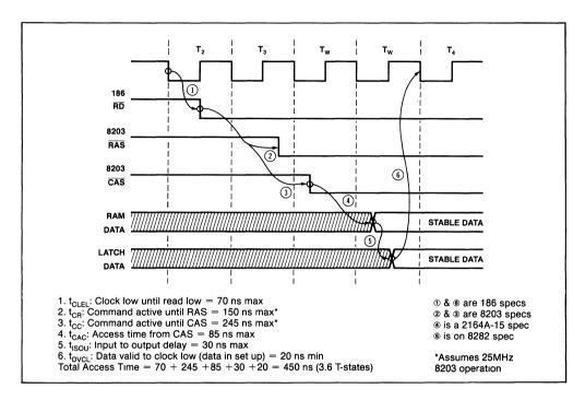
Figure 23. 8203/2164A-15 Access Time Calculation
