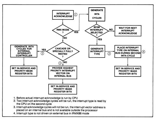
Figure 58. 80186 Interrupt Acknowledge Sequencing
