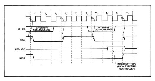
Figure 60. 80186 Cascaded Interrupt Acknowledge Timing
