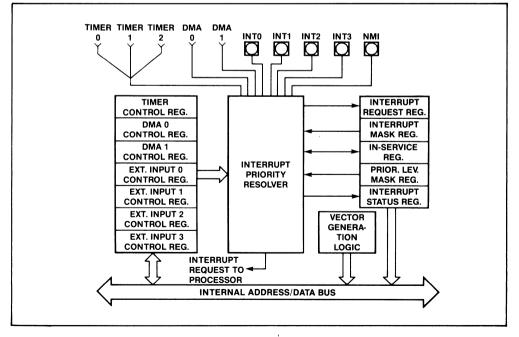
Figure 48. 80186 Interrupt Controller Block Diagram
