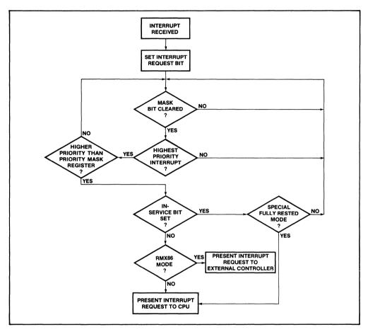
Figure 57. 80186 Interrupt Request Sequencing
