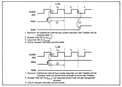
Figure 27. HOLD/HLDA Timing in the 80186
