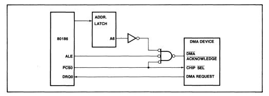
Figure 36. DMA Acknowledge Synthesis from the 80186
