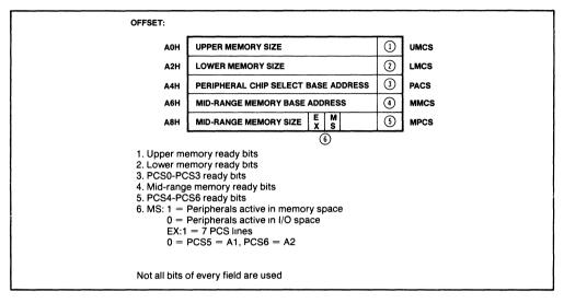
Figure 72. 80186 Chip Select Control Registers
