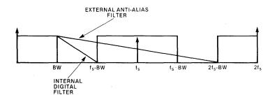
b. Spectrum using double rate sampling. External filter passes BW, stops beyond 2f<sub>s</sub>-BW, internal digital filter performs rest of anti-alias function.
