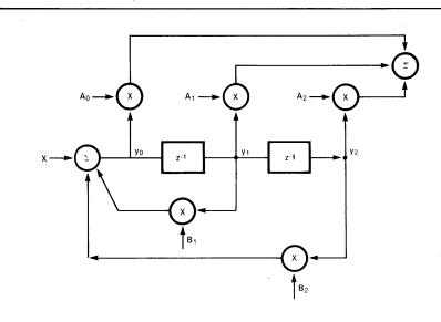
Figure H-1. Digital Filter Module (Second Order Section) 121533-34
