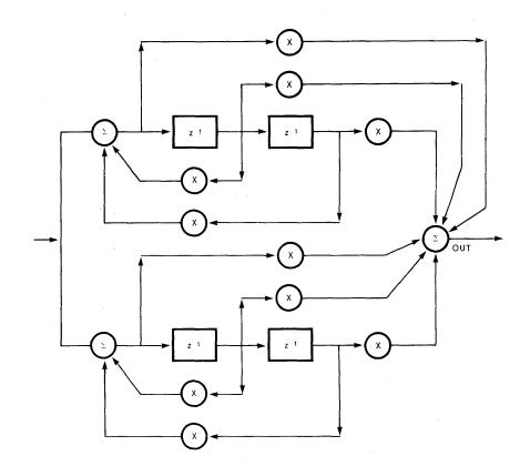
Figure H-8b. Parallel Structure for Complex Filters (May Result From Impulse Invariant Transform)
