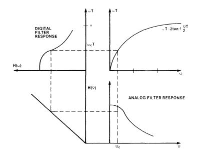
Figure H-4. Transfer Function From  $\Omega$  to w
