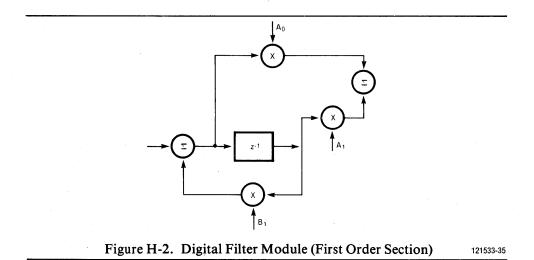
The diagram of Figure 2 corresponds to a stage realizing a single real pole. Its impulse response takes the form:
