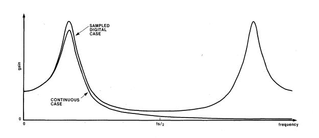
Figure H-3. Comparison of Digital and Continuous Frequency Response
