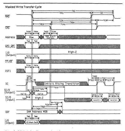
Note: 1. I/O Mask Data(In new mask mode) Low: Mask High: Non Mask I/O: don't care in persistent mask mode
