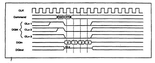
(2) Operation for the column in other ROW of the same bank: To execute write or block write for other row of the same bank, it is necessary to execute a precharge command and bank active command before executing these commands. (3) Operation for another bank: For another bank in active state, burst write command can be executed from the next cycle after the preceding write command is issued. If another bank is in the idle state, bank active command should be executed.
