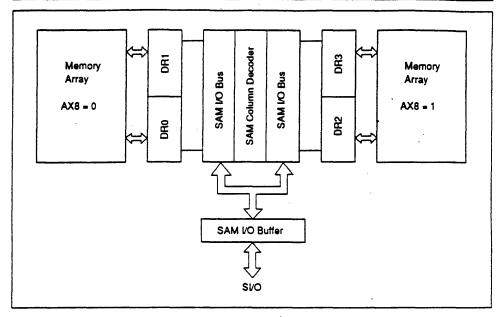
Figure 4 Block Diagram for Split Transfer
