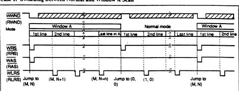
Case 1: Switching Between Normal and Window A Scan
