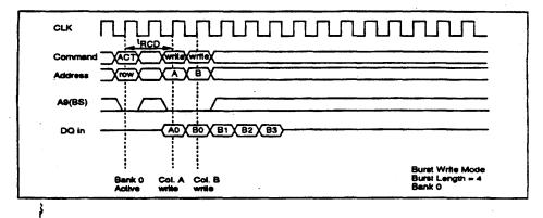
(2) Operation for the column in other ROW of the same bank: To write data on other row of the same bank, it is necessary to execute a precharge command and bank active command before executing next write command.
