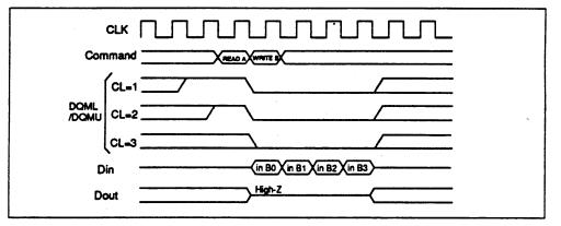
(2) Same bank, different ROW address: When the ROW address changes, consecutive write commands cannot be executed; it is necessary to separate the two write commands with a precharge command or a bank-active command. (3) Different bank: When the bank changes, the write command can be performed after an interval of no less than 1 cycle, provided that the other bank is in the bank-active state. However, DQML/DQMU must be set High so that the output buffer becomes High-Z before data input.
