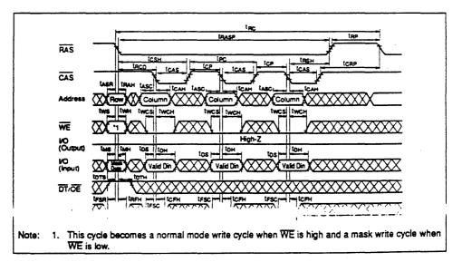
Page Mode Write Cycle (Delayed Write)
