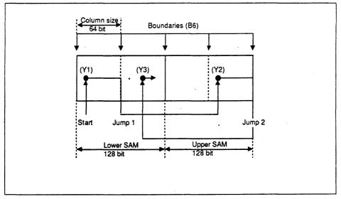
Figure 6 Example of Boundary Split Register
