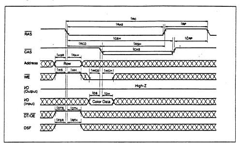
Color Register Set Cycle (Delayed Write)
