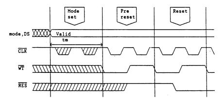
Note: When mode pins are fixed with  $V_{\rm CC}, \, V_{\rm SS}$  in mode set while the power supply is on,  $t_m$  spec is not needed.
