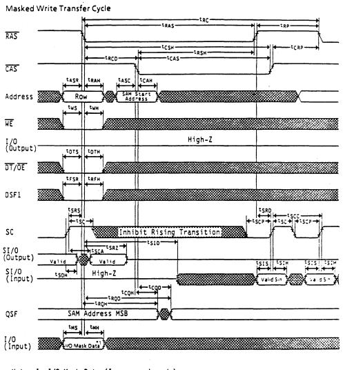
Note: 1. I/O Mask Data (In new mask mode) Low : Mask High : Non Mask I/O : Don't care in persistent mask mode.
