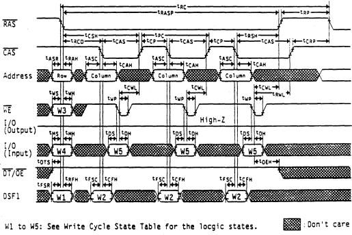
Fast Page Mode Write Cycle (Delayed Write)
