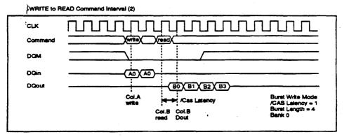
(2) Operation for the column in other ROW of the same bank: To execute read command for other row of the same bank, it is necessary to execute a precharge command and bank active command. (3) Operation for another bank: For another bank in active state, burst read command can be executed from the next cycle after the preceding write command is issued. If another bank is in the idle state, bank active command should be executed prior to execute these command.
