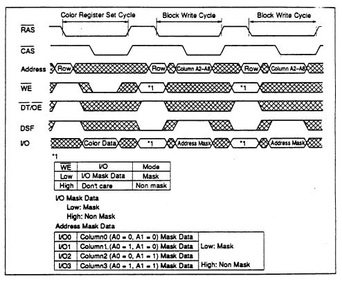
Figure 2 Use of Block Write
