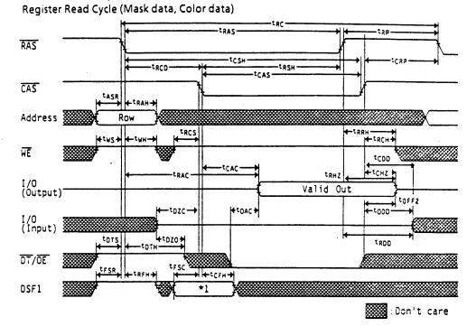
Note: 1. State of DSF1 at falling edge of  $\overline{CAS}$
