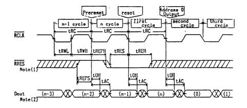
Notes: 1. The <u>read</u> address counter is reset at the first falling edge of <u>RCLK</u> after <u>RRES</u> falls, meeting the specifications of t<sub>REPS</sub> <u>and tREPH</u>, and it is not reset at the next falling edge of <u>RCLK</u> even if <u>RRES</u> is kept low.
