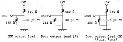
DEC output load Dout output load (A)
