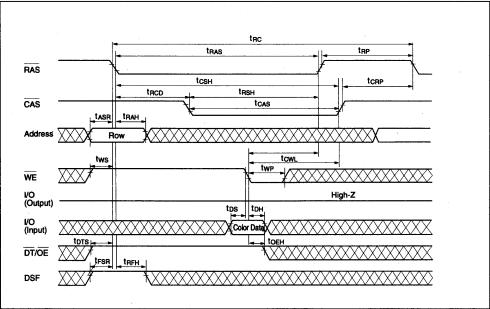
Color Register Set Cycle (Delayed Write)
