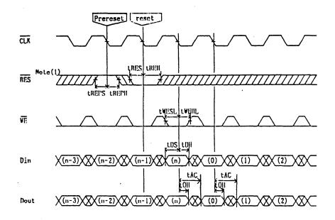
Note: The read address counter is reset at the first falling edge of  $\overline{\text{CLK}}$  after  $\overline{\text{RES}}$  falls, meeting the specifications of t<sub>REPS</sub> and t<sub>REPH</sub>, and it is not reset at the next falling edge of  $\overline{\text{CLK}}$  even if  $\overline{\text{RES}}$  is kept low.
