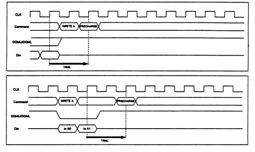
Burst Length = 4 (To stop write operation)
