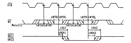
Note: When  $t_{WTSL}$ ,  $t_{WTHL}$ ,  $t_{WTSH}$ , and  $t_{WTHH}$  cannot meet the specifications, the decode output operation is not guaranteed.
