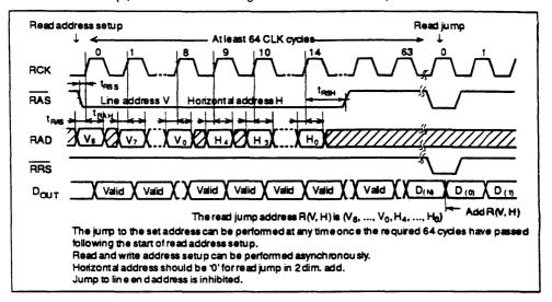
Read address setup (2 dimensional addressing: 324 line × 1024 dot mode)
