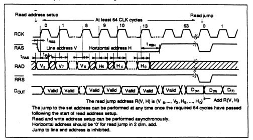
Read address setup (2 dimensional addressing: 288 line × 1152 dot mode)
