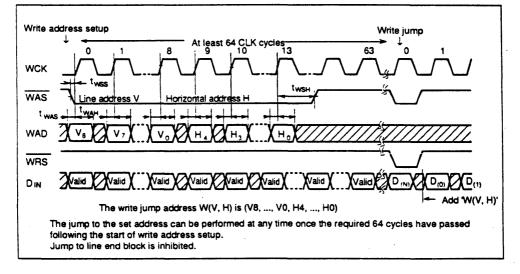
Write address setup (2 dimensional addressing: 324 line × 1024 dot mode)
