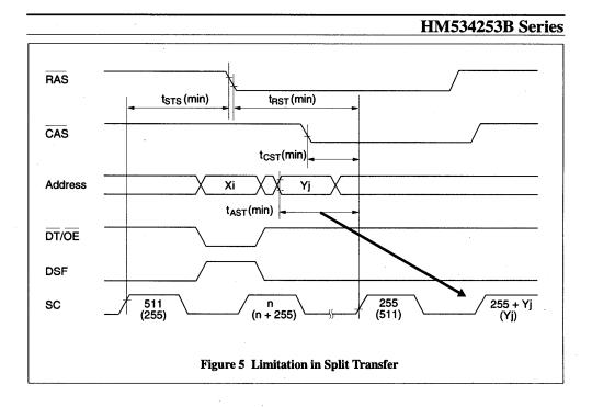
Split Write Transfer Cycle ( $\overline{CAS}$  high,  $\overline{DT}/\overline{OE}$  low,  $\overline{WE}$  low and DSF high at the falling edge of  $\overline{RAS}$ )
