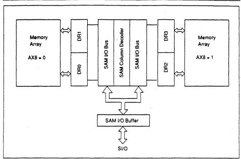
Figure 4 Block Diagram for Split Transfer
