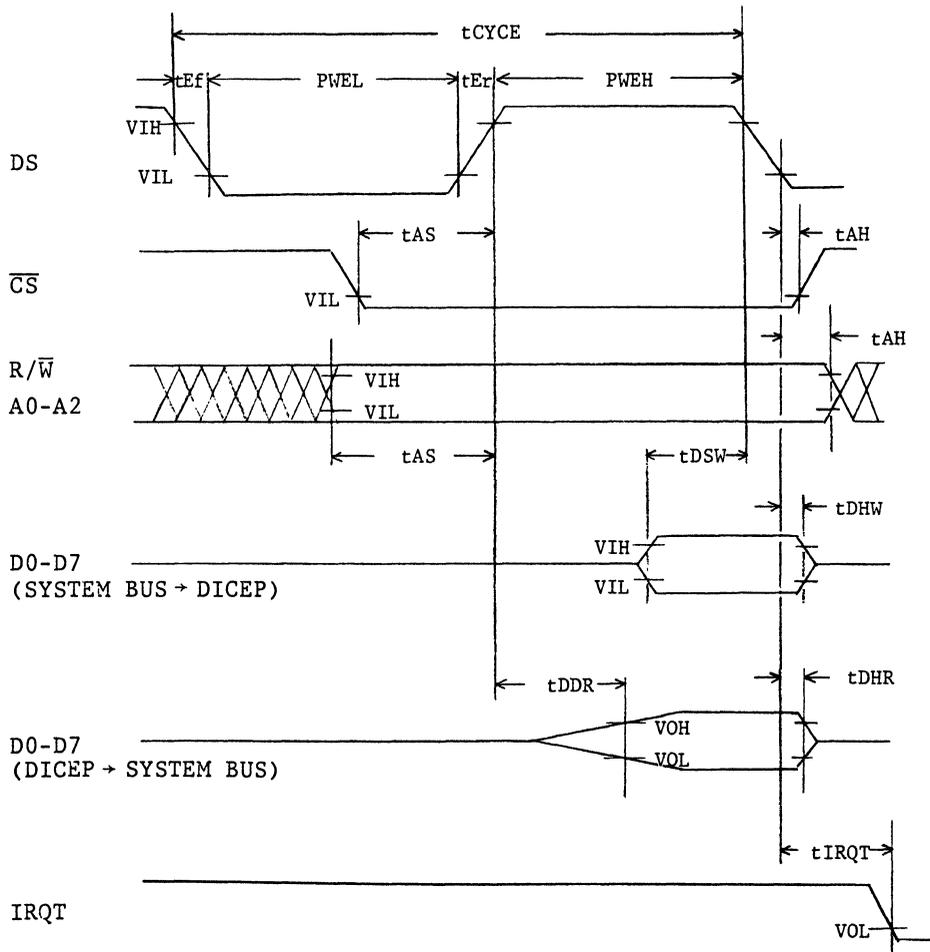
Fig. 1-2 System Bus Read/Write Timing
