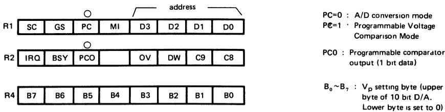
Figure 19 Registers of the PC Mode
