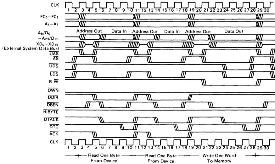
Figure 23 Dual Addressing Mode, Read/Write Cycle
