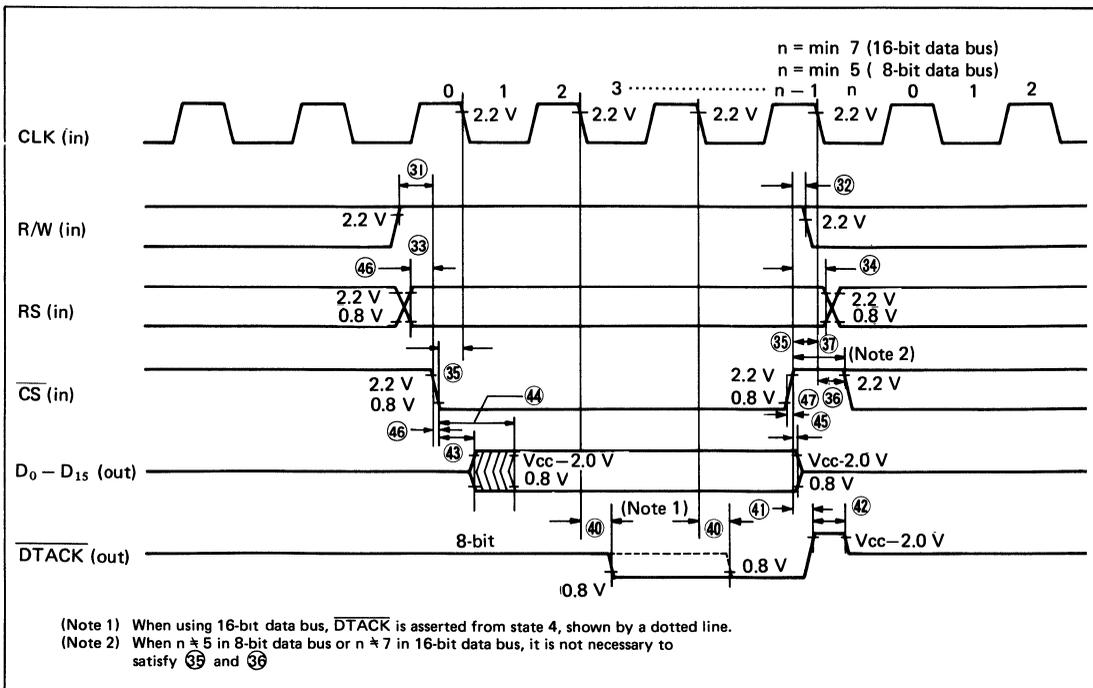
Figure 18 MPU Read Cycle
