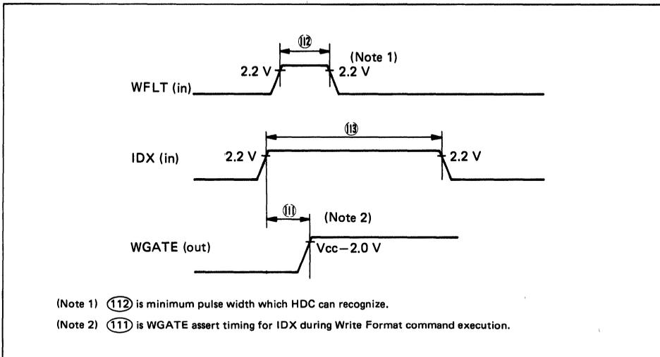
Figure 23 WFLT, IDX, WGATE Timing (ST506)
