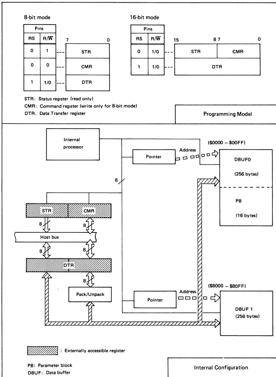
Figure 5 Internal Configuration and Programming Model
