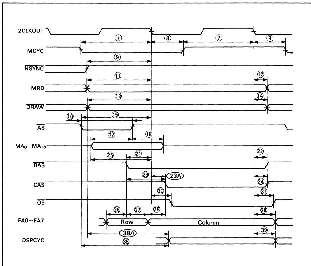
Figure 20. Memory Read Cycle (Drawing Read and Display)
