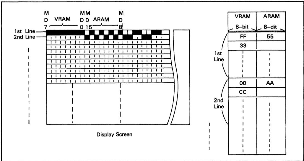
Figure 9. Relation between Graphic Screen and Memory Contents
