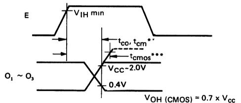
Figure 6 Output Delay
