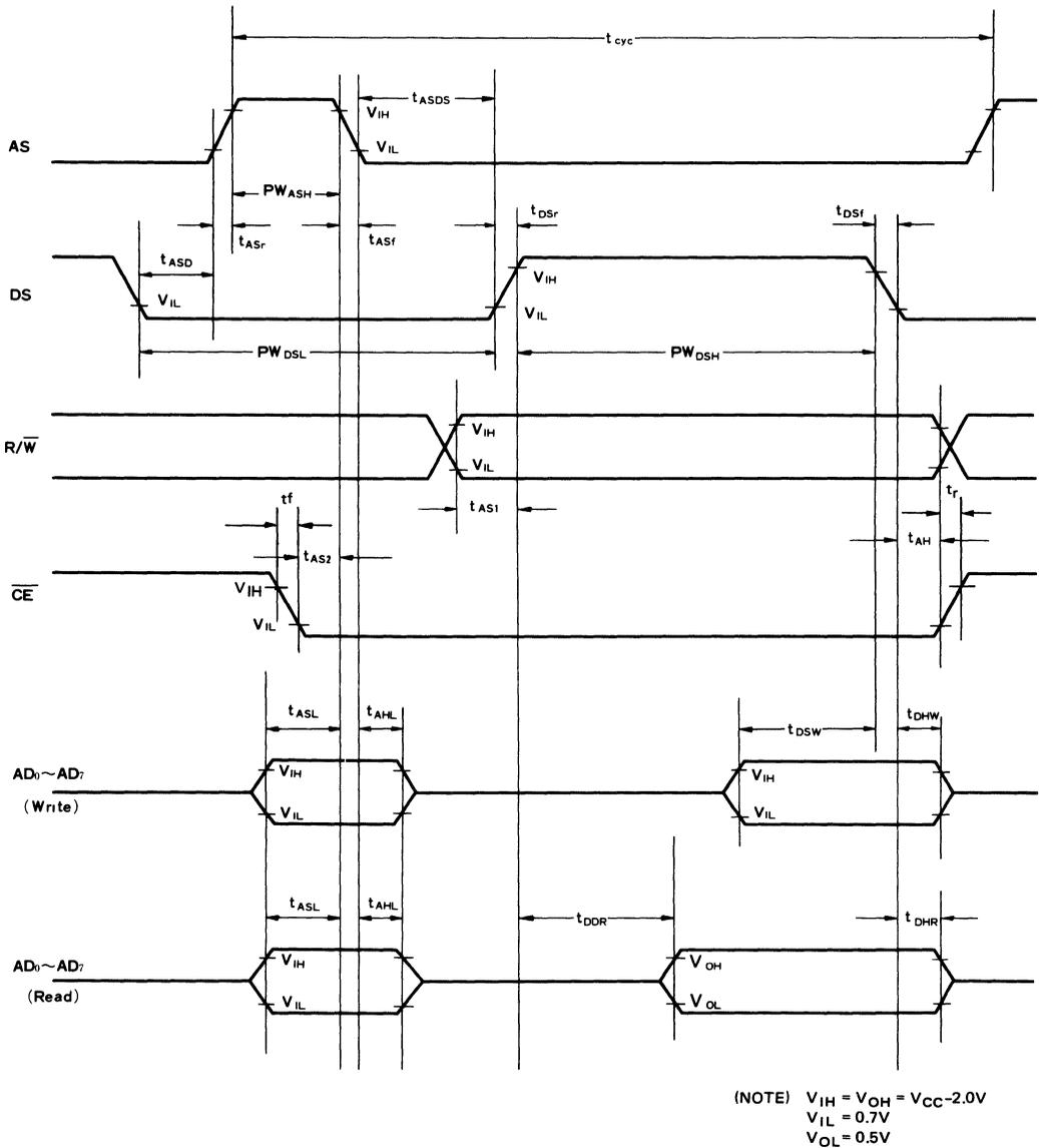
Figure 1 Bus Read, Write Timing (6801 Family)
