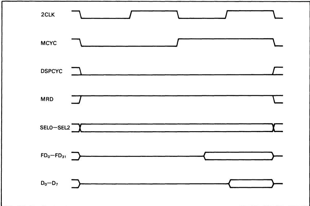
**Figure 5. Drawing Read Cycle**
