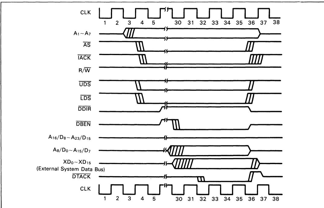
Figure 37 MPU  $\overline{IACK}$  Cycle to DMAC
