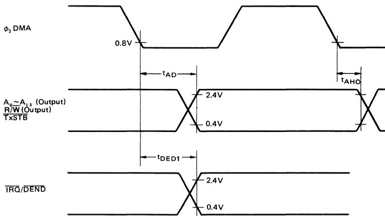
Figure 6 Timing of Address and  $\overline{IRQ}/\overline{DEND}$  Outputs
