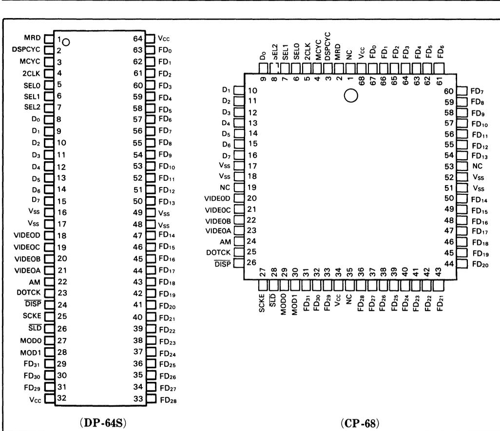
Figure 1. Pin Arrangement
