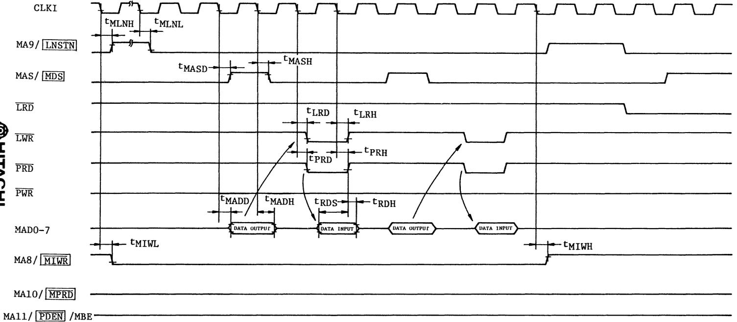
Fig. 1-16 Memory Bus Interface Timing in B Mode (1)
