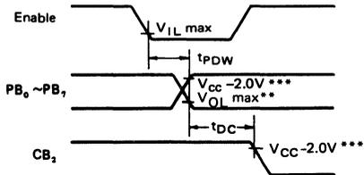
(Note) CB<sub>2</sub> goes "Low" as a result of the positive transition of Enable.
