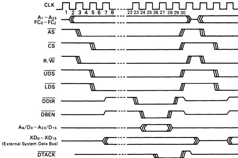
Figure 12 MPU Write to DMAC – Word
