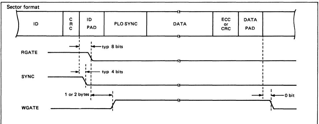
Figure 28 Write Data Timing (ST506)
