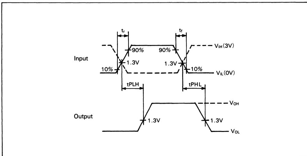
Figure 25. Input/Output waveforms
