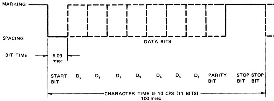
Figure 10 110 Baud Serial ASCII Data Timing
