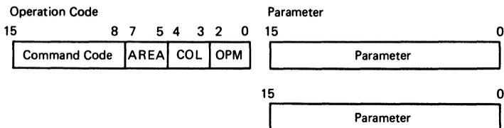
Figure 36 Graphic Drawing Command Format
