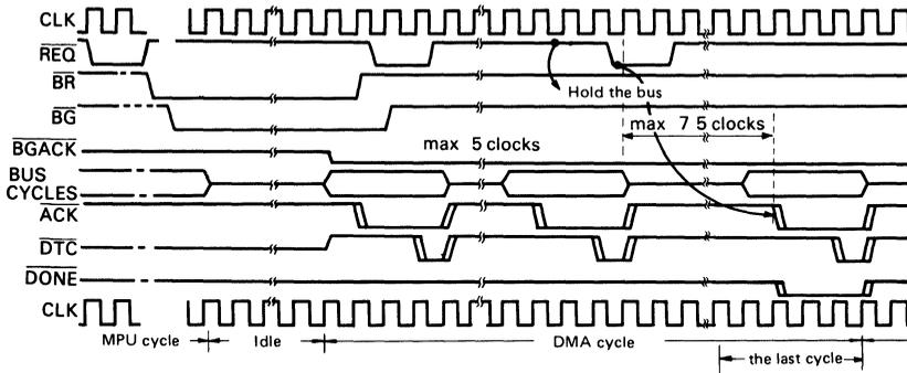
Figure 18 Cycle Steal Bus Hold Mode Request Timing
