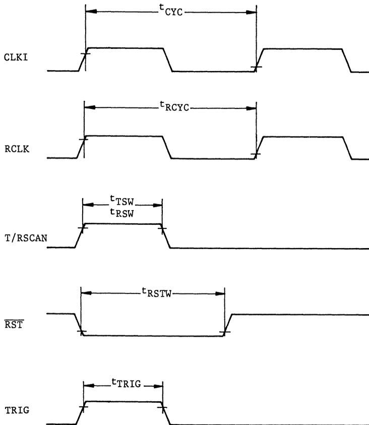
Fig. 1-7 CLKI, RCLK, T/RSCAN,  $\overline{RST}$  and TRIG Input Timing
