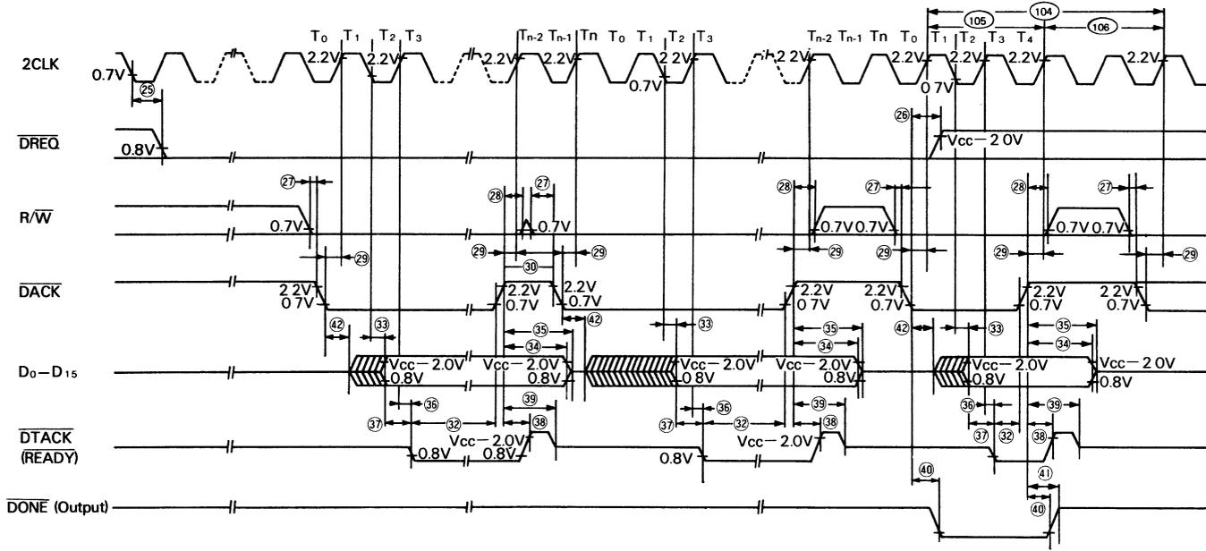
(Note)  $\overline{DACK}$  "high" level width must satisfy spec (30). Unless satisfying spec (106),  $\overline{DTACK}$  and the read data delay to the succeeding cycle. When the ACRTC is used with the synchronous bus timing, specifications (104), (105) and (106) must be satisfied.
