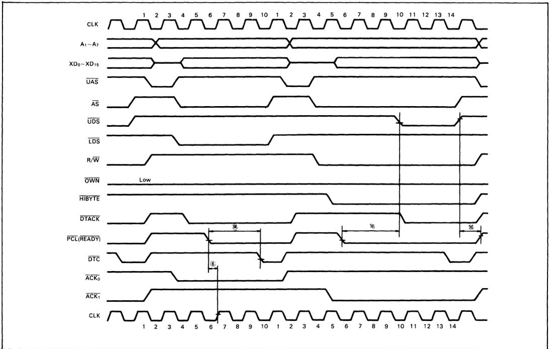
Figure 7 AC Electrical Waveforms-DMA Read/Write (Single Cycle with  $\overline{ACK}$  and  $\overline{READY}$ )
