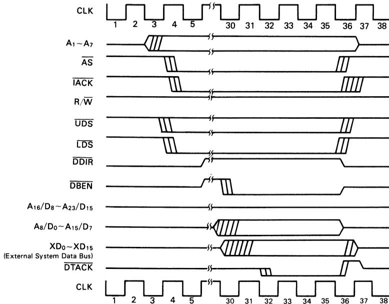
Figure 36 MPU  $\overline{TACK}$  Cycle to DMAC
