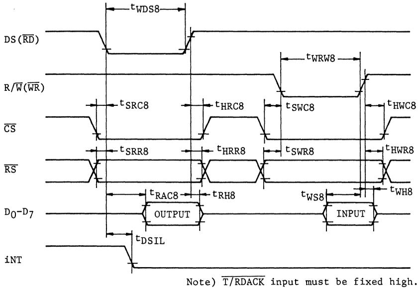
Fig. 1-3 Intel MPU Access Timing
