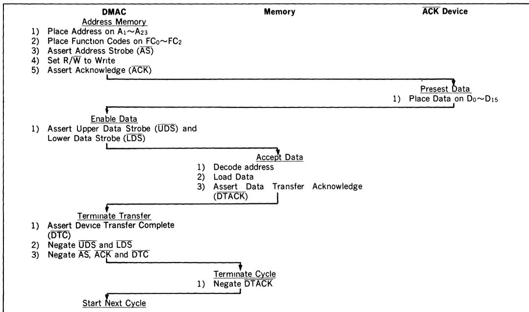
Figure 29 Word from Device with  $\overline{ACK}$  to Memory
