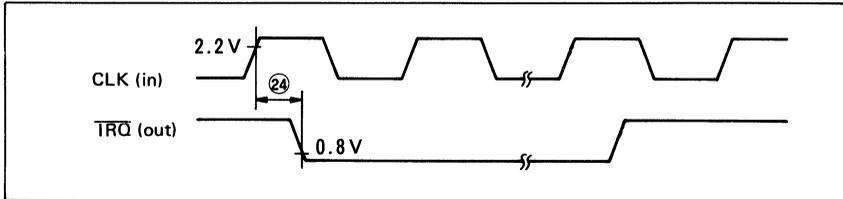
Figure 17 TRQ Output Timing
