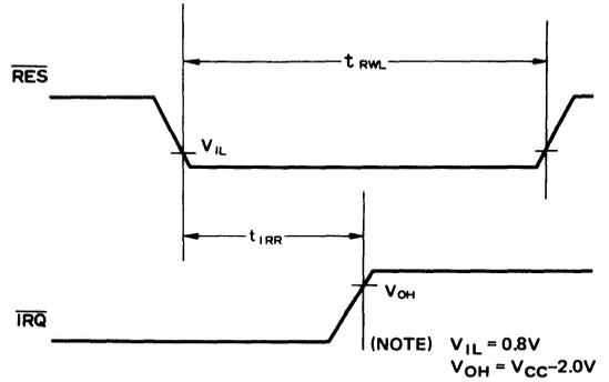
Figure 5  $\overline{IRQ}$  Release Delay (from  $\overline{RES}$ )
