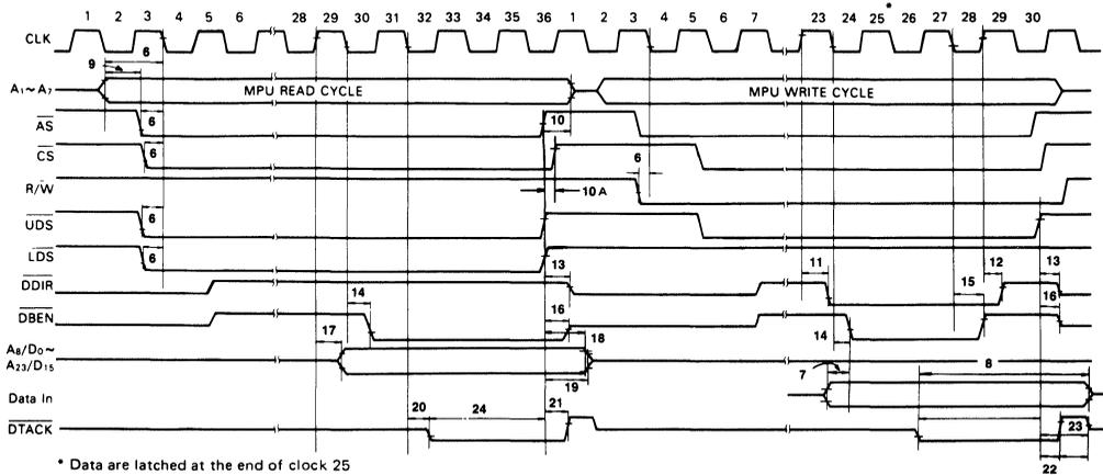
Figure 3 AC Electrical Waveforms – MPU Read/Write
