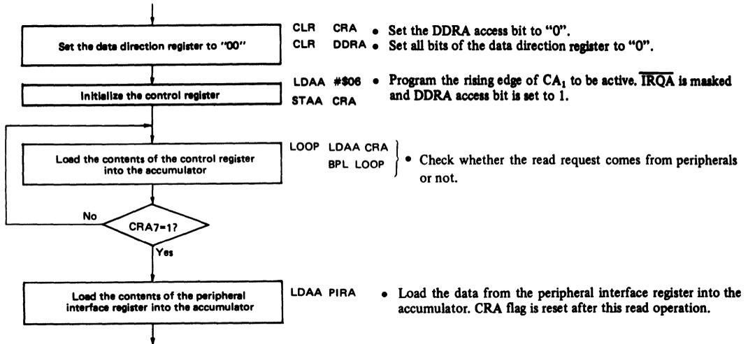
To read the peripheral data, the data is directly transferred to the data buses D<sub>0</sub>~D<sub>7</sub> through PA<sub>0</sub>~PA<sub>7</sub> or PB<sub>0</sub>~PB<sub>7</sub>, and they are not latched in the PIA. If necessary, the data should be held in the external latch until MPU completes reading it.
