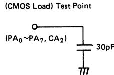
Figure 14 Bus Timing Test Loads
