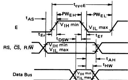
Figure 2 Bus Write Timing (Write Information into PTM)
