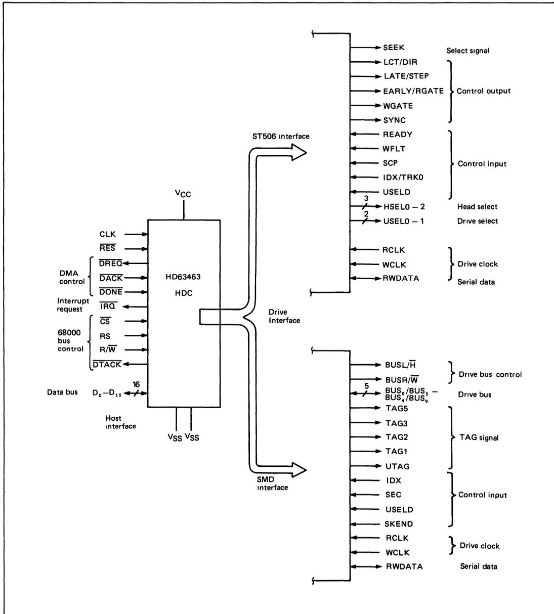
Figure 1 Input/Output Signals
