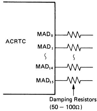
**Figure 24 Damping Resistor**
