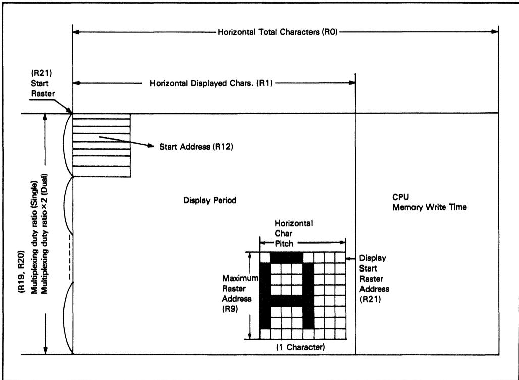
Figure 5. Relation between Display Screen and Registers
