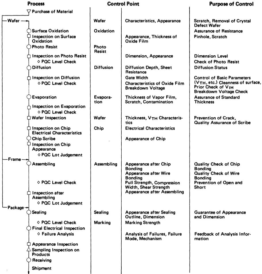
Figure 3 Example of Inner Process Quality Control
