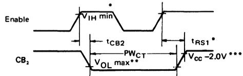
Figure 6 CB<sub>2</sub> Delay Time (Write Mode; CRB5=CRB3=1, CRB4=0)
