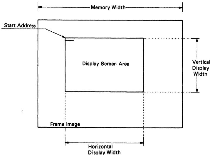
Figure 46 Frame Memory and Display Screen Area
