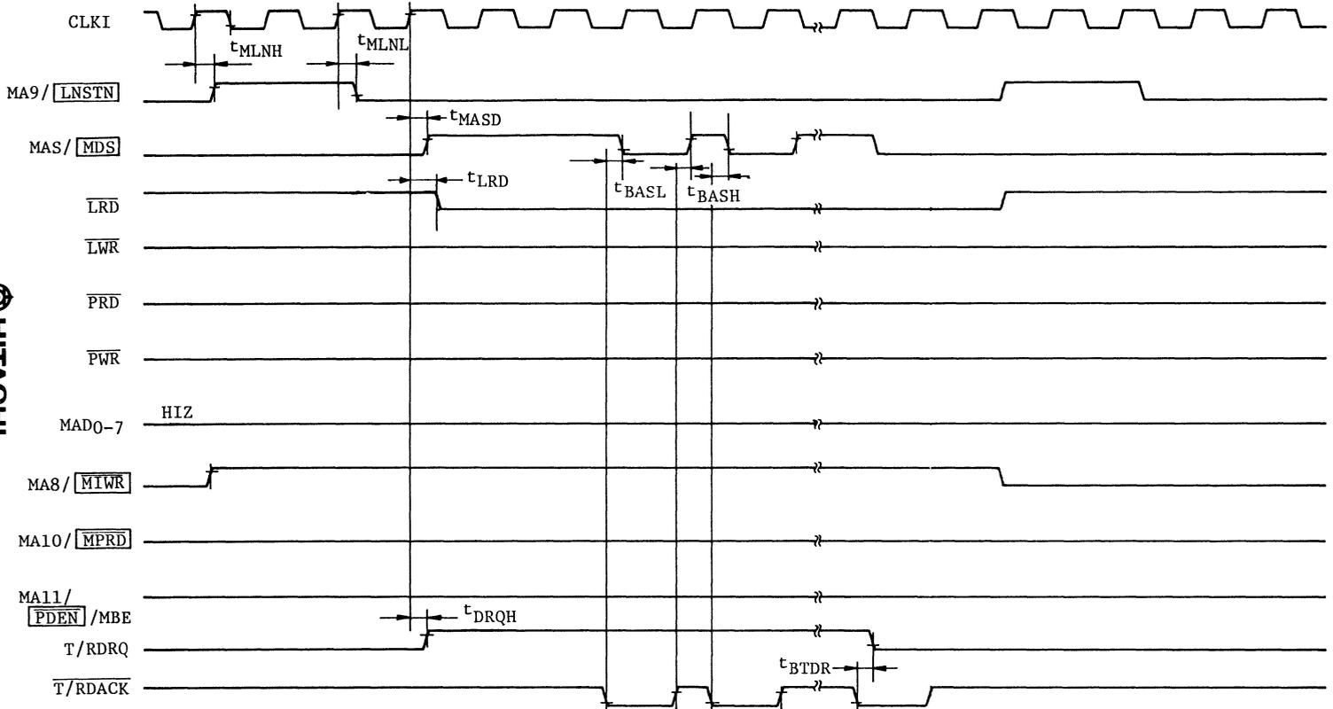
Fig. 1-17 Memory Bus Interface Timing in B Mode (2)
