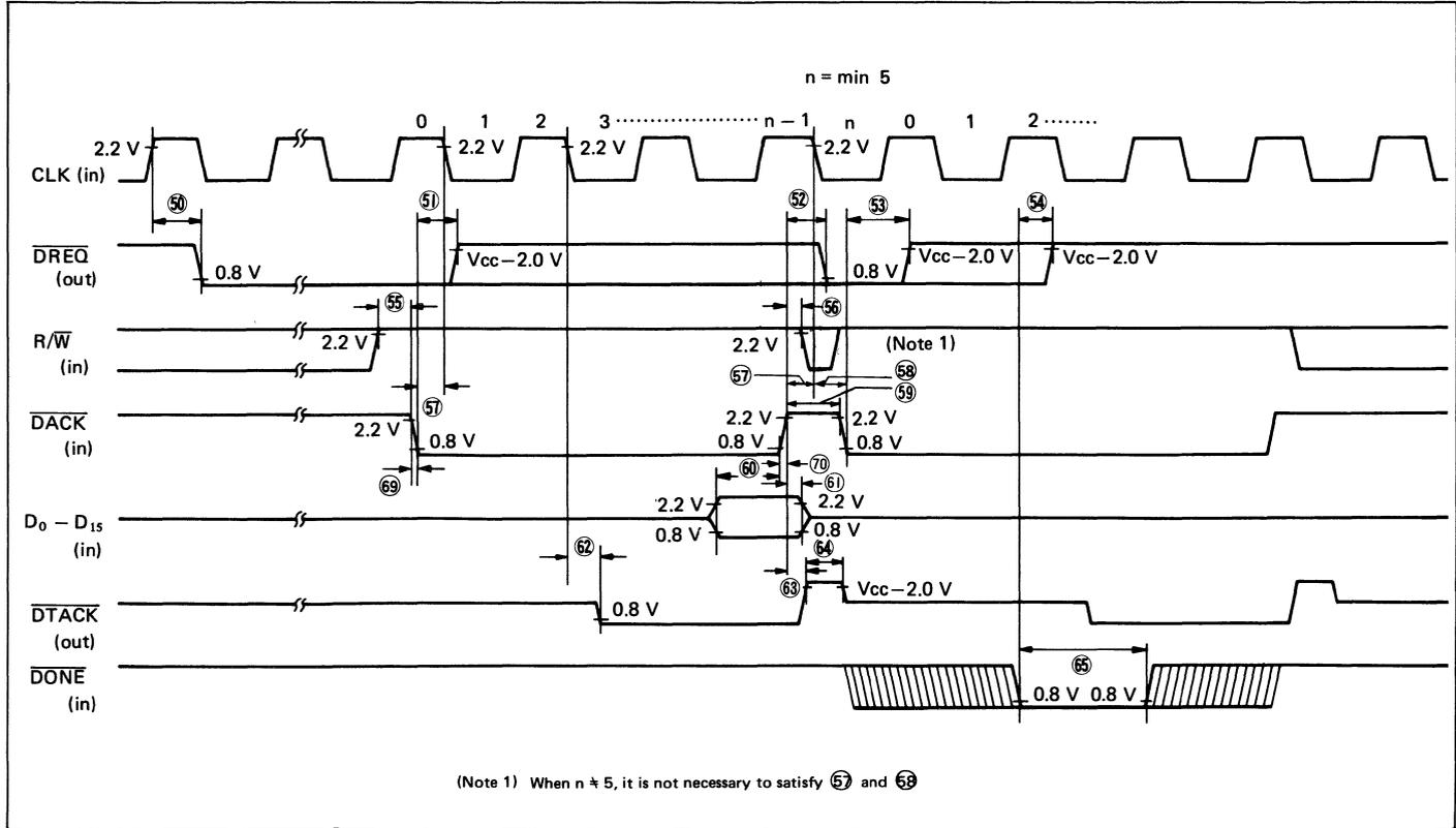
Figure 21 DMA Write Cycle
