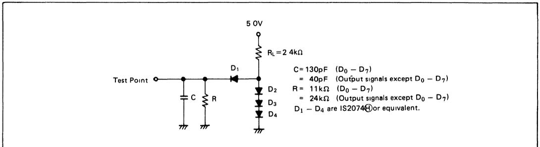
Figure 39 Test Load
