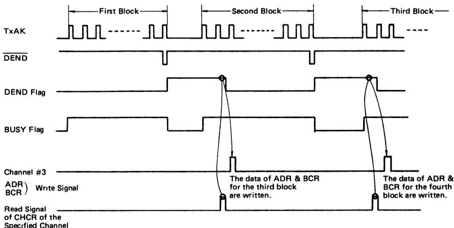
Figure 34 Sequence of More than 3-block Data Chain
