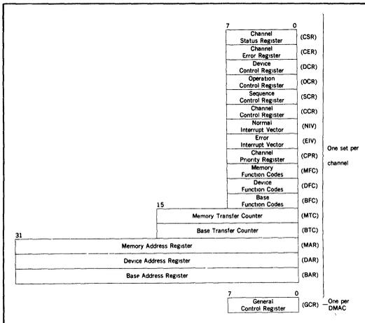
Figure 11 Internal Registers
