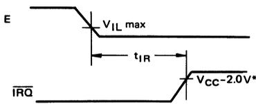
Figure 7  $\overline{IRQ}$  Release Time
