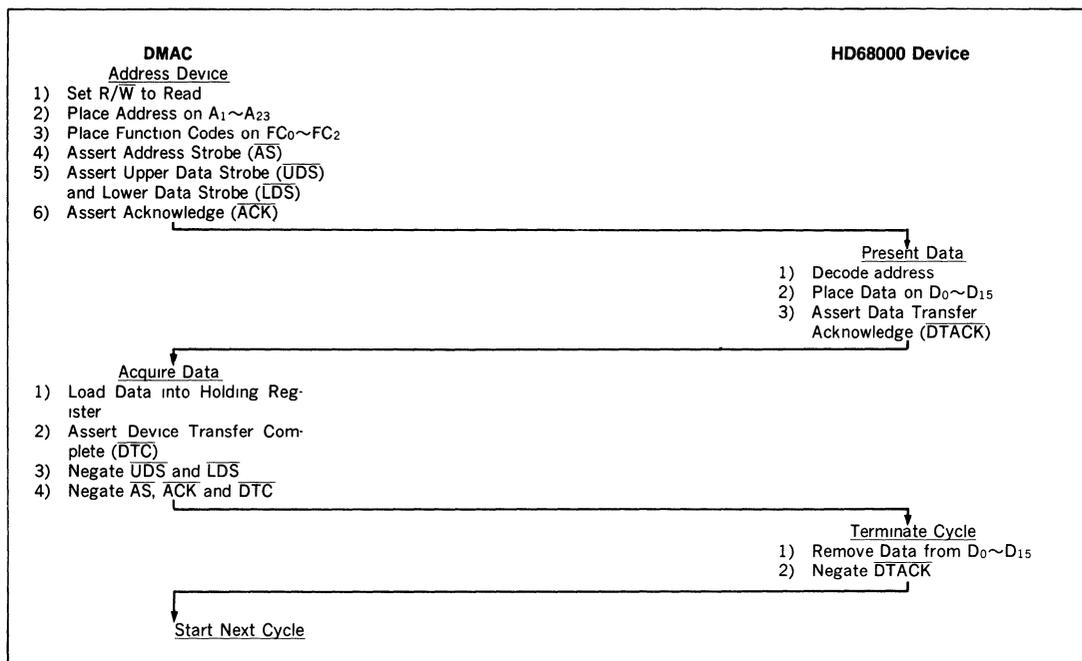
Figure 19 Word Read Cycle Flowchart HD68000 Type Device
