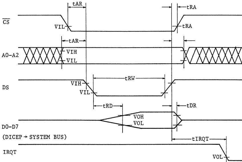
Fig. 1-3 System Bus Read Timing
