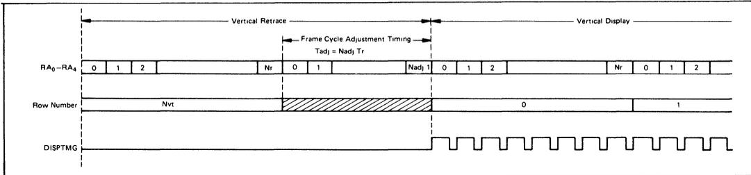
Figure 5 Frame Cycle Adjustment Timing
