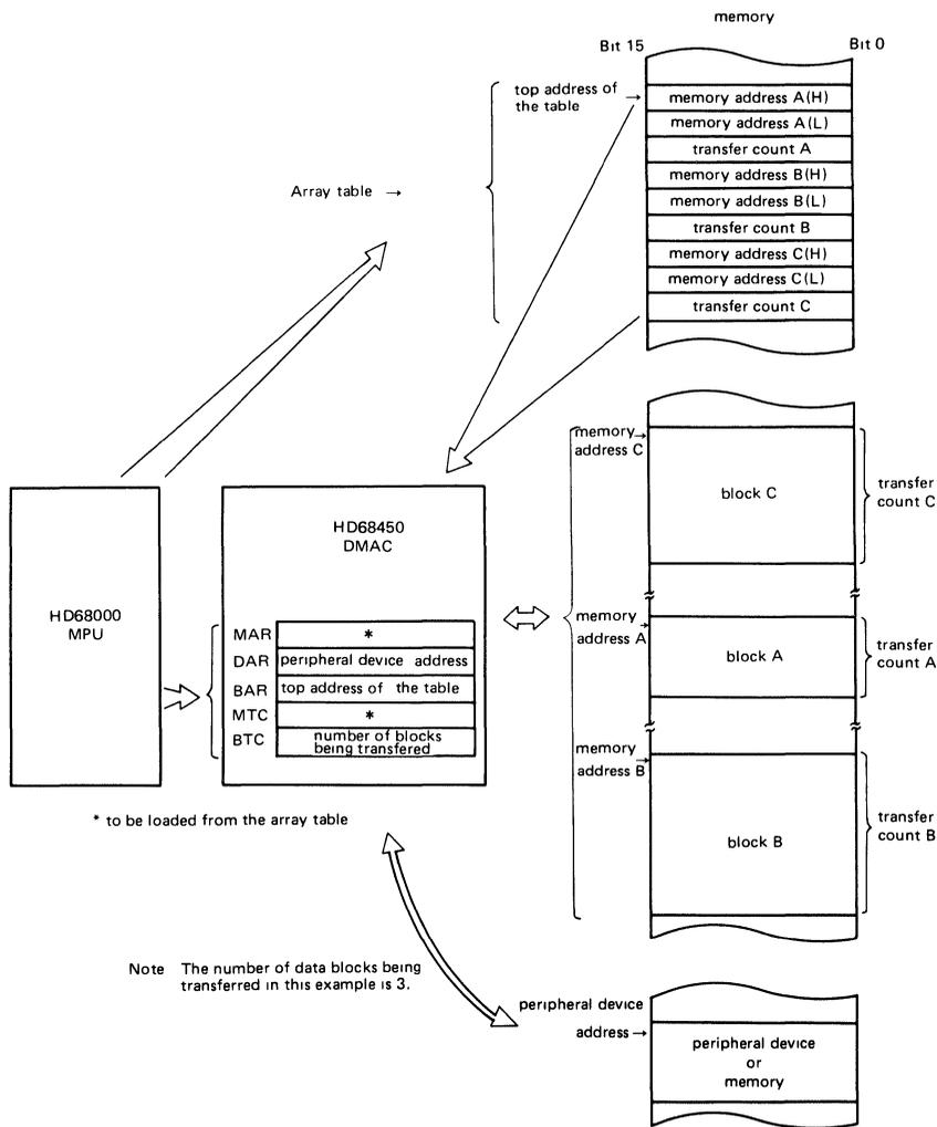
Figure 37 Transfer Example of the Array Chaining Mode
