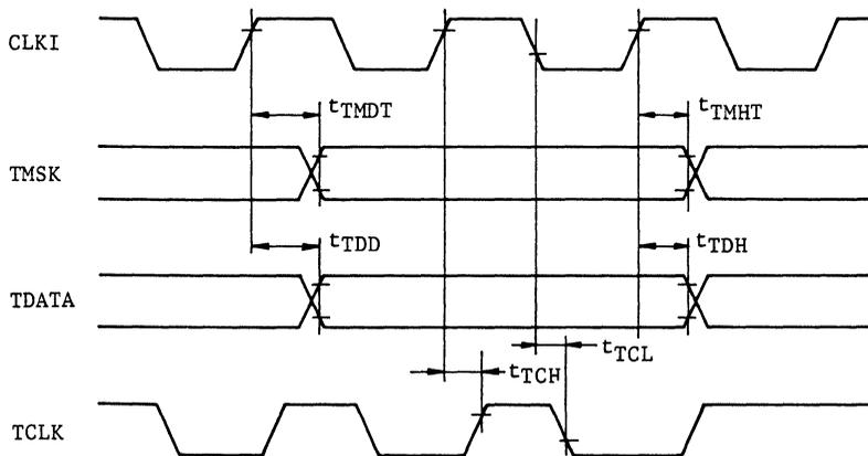
Fig. 1-8 Serial Output Timing (in Read (T) Mode)
