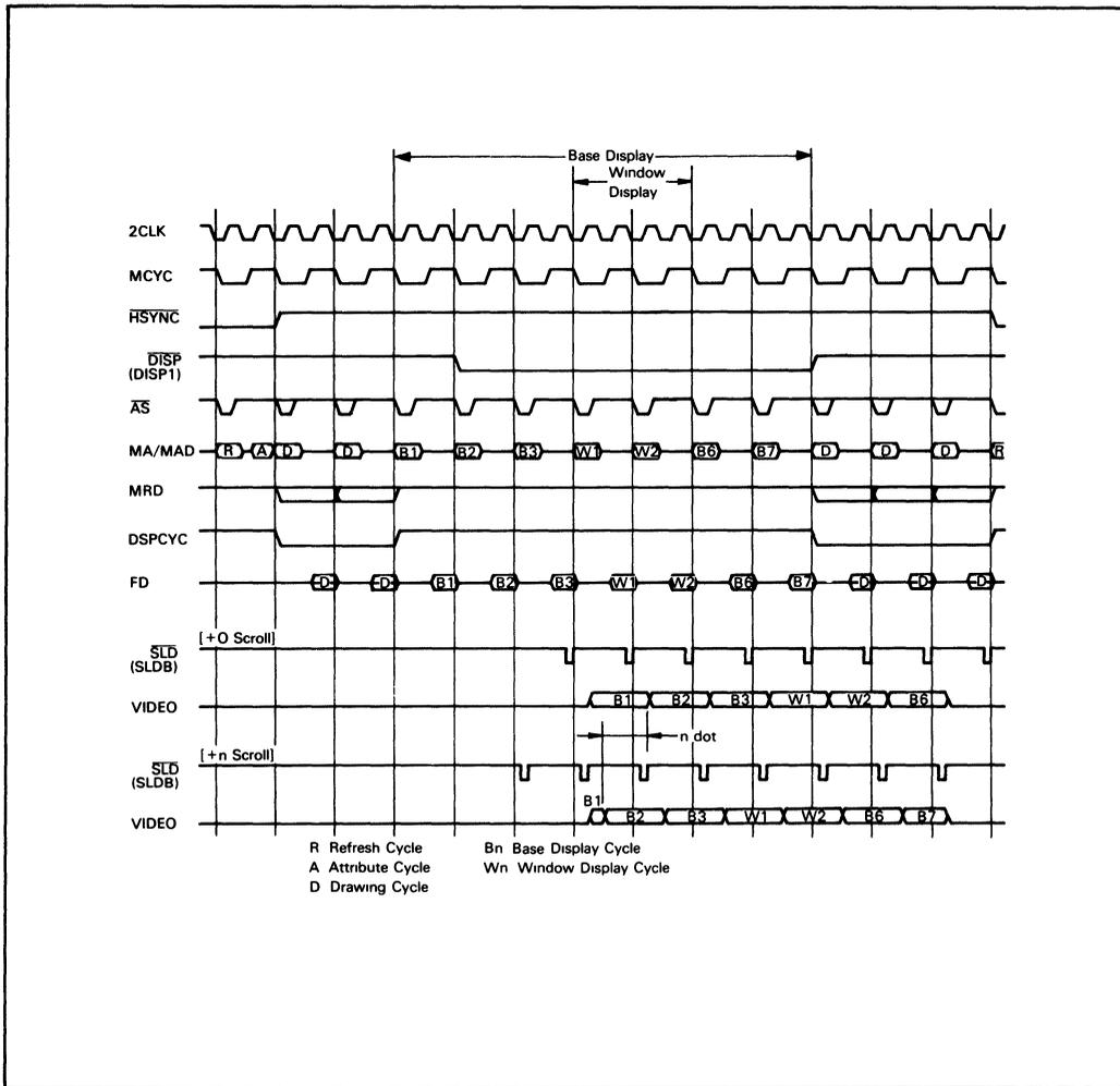
Figure 9. Video Output Timing (Single Access Mode)
