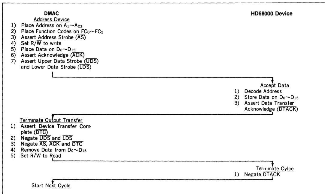
Figure 20 Word Write Cycle Flowchart HD68000 Type Device
