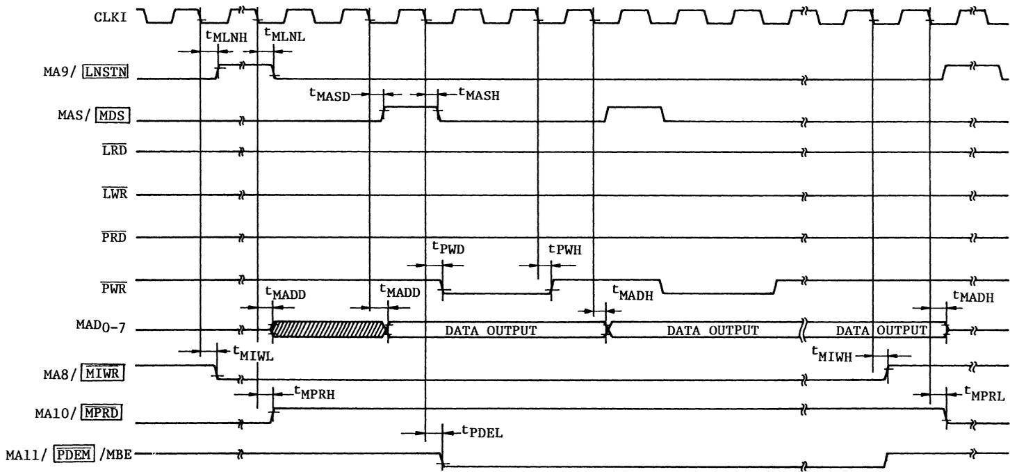
Fig. 1-18 Memory Bus Interface Timing in B Mode (3)
