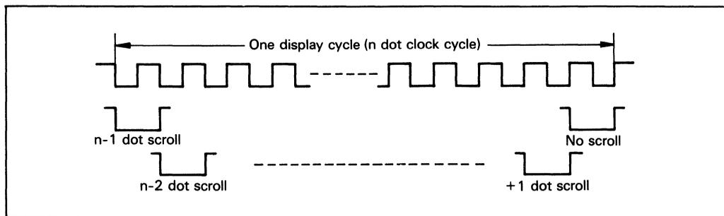
**Figure 8. Shift Load ( $\overline{SLDB}$ ,  $\overline{SLDW}$ ) Output Timing**
