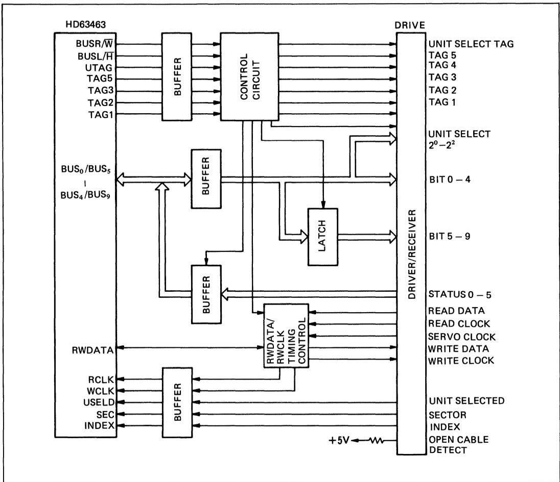
Figure 4 SMD Interface Circuit
