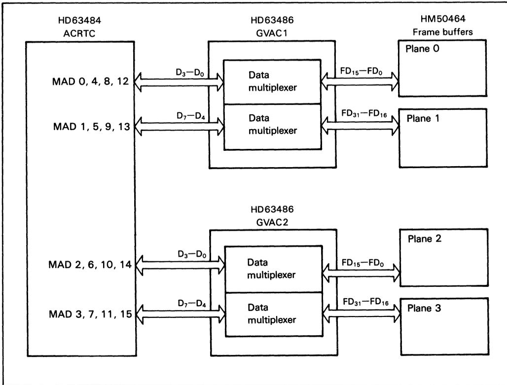
**Figure 6. FD Pin Connection (MOD1, MOD0 = 00)**
