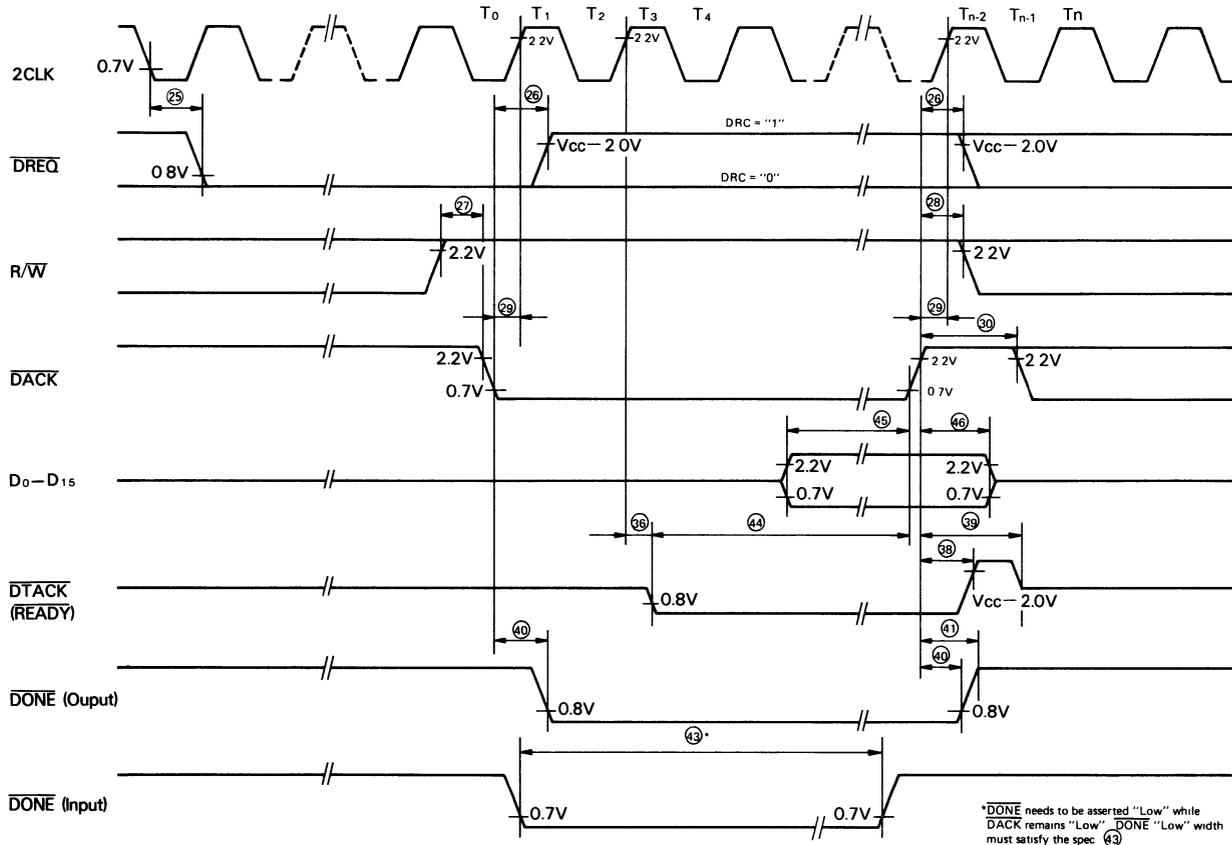
Figure 7 DMA Write Cycle Timing (System Memory → ACRTC)
