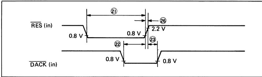
Figure 16 RES – DACK Input Timing (Data Bus Width Selection)
