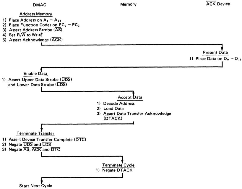
Figure 29 Word from Device with  $\overline{ACK}$  to Memory
