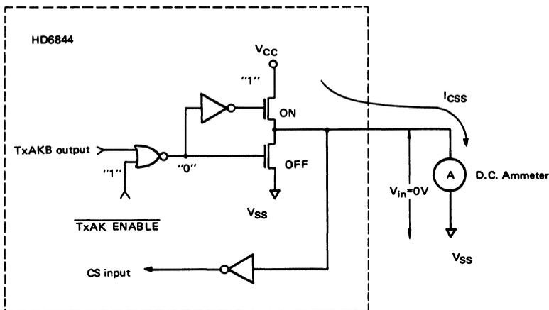
Figure 10 Source Current Measurement Circuit for CS/TxAKB Terminal
