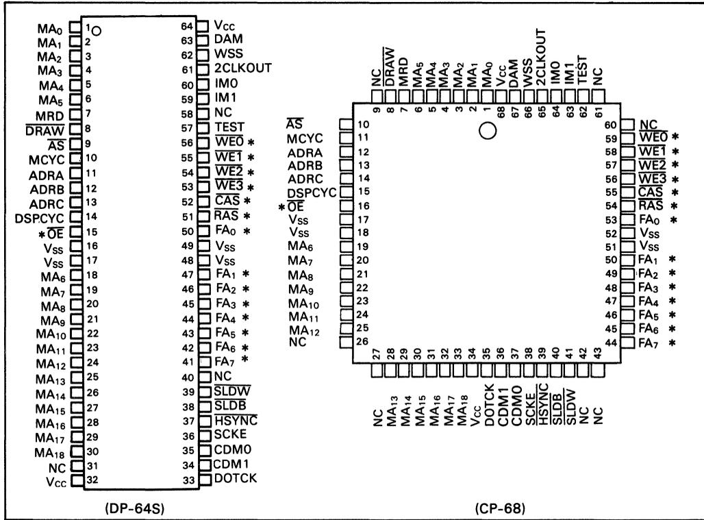
Figure 1. Pin arrangement
