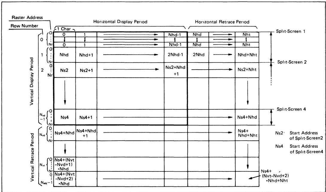
Figure 7 Memory Address and Raster Address in Split-Screens
