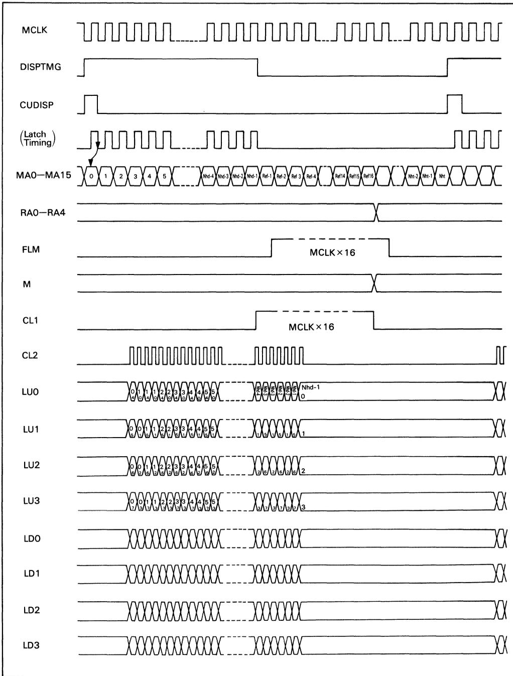
Figure 6. LCTC Timing Chart (In Mode 5: Single Screen, 4-Bit Transfer, Normal Character Display)
