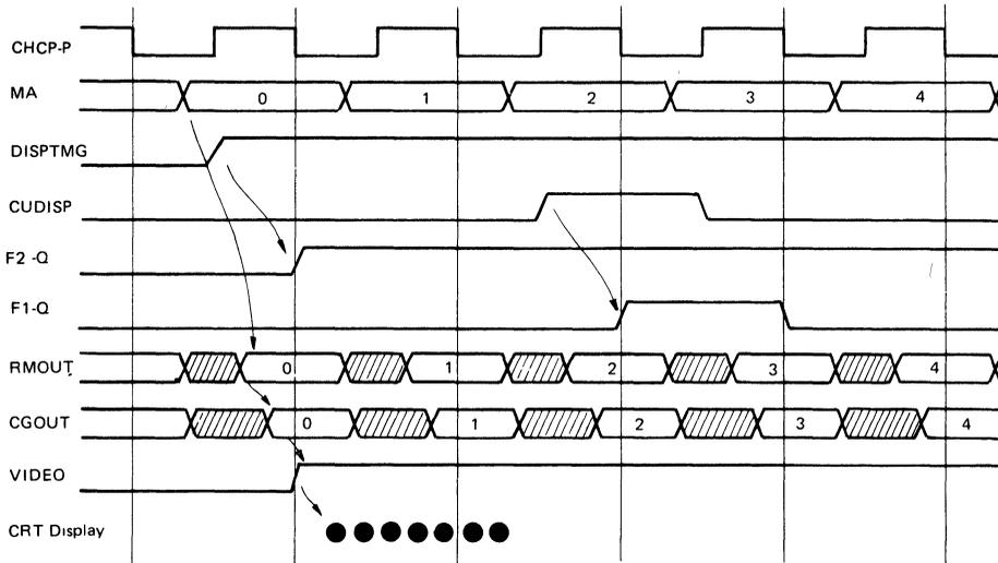
Figure 24 Time Chart of Display Control Unit (1)
