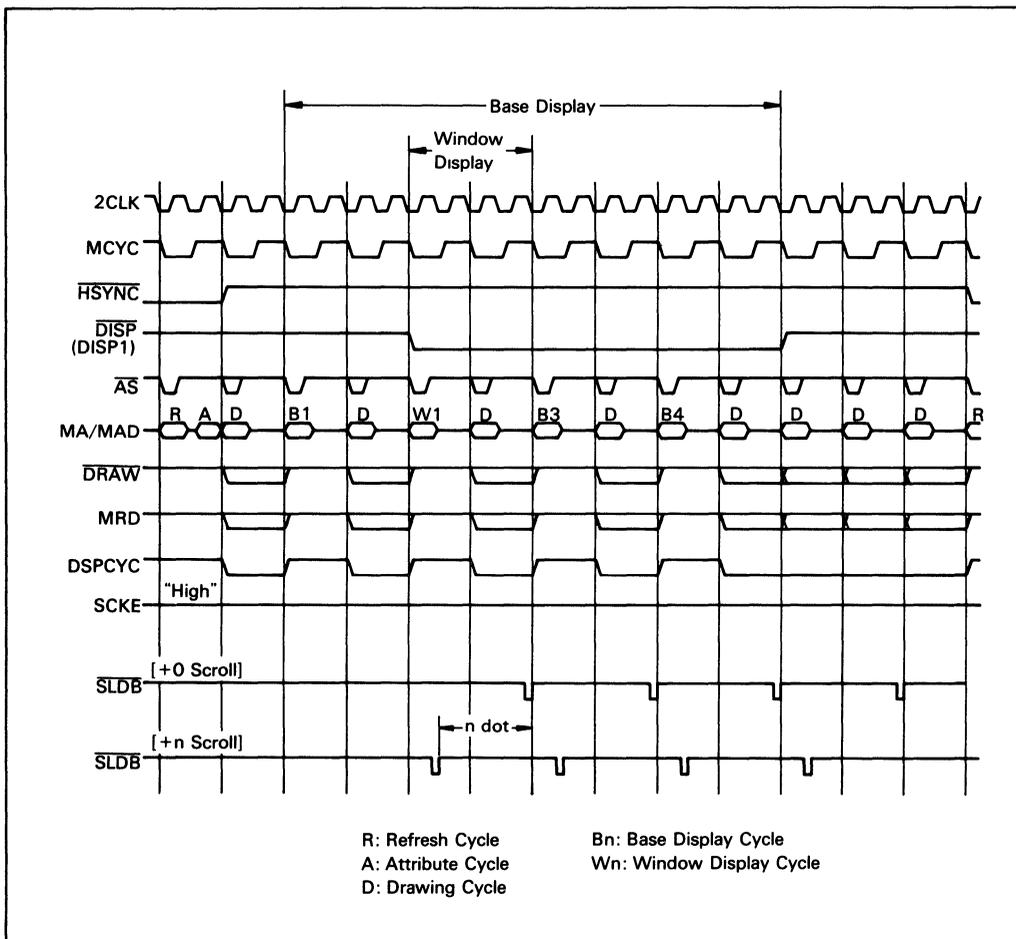
Figure 10. SLDB Timing (Dual Access Mode 0)
