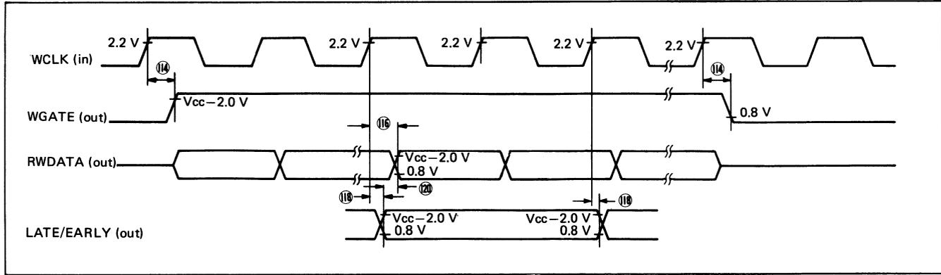
Figure 24 Write Operation (ST506)
