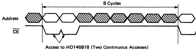
As shown in the above [example 2], when HD146818 is accessed continuously, continuous access must not be executed over fifty times.
