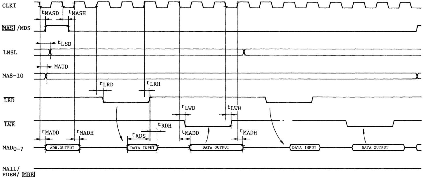
Fig. 1-14 Memory Bus Interface Timing in A Mode (1) During Image Data Processing
