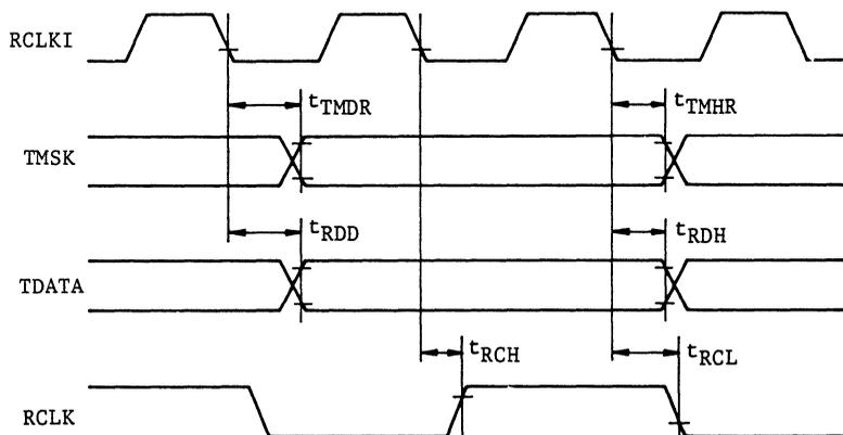
Fig. 1-9 Serial Output Timing (in Receive (R) Mode)
