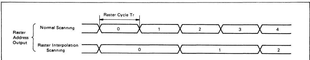
Figure 20 Raster Address Output and Raster Interpolation
