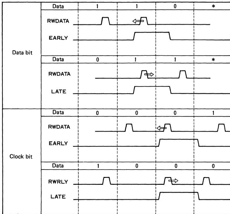
Figure 8 Write Precompensation
