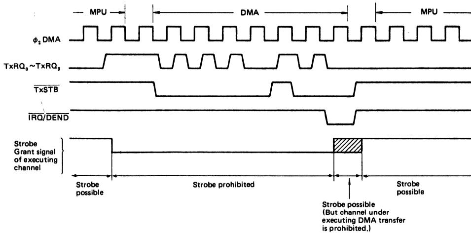
Figure 20 Strobe Timing of Executing-Channel-Number-Latch-Circuit (the burst mode)
