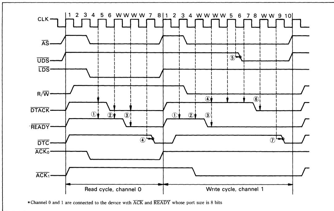
Figure 33 Device with  $\overline{\text{ACK}}$  and  $\overline{\text{READY}}$  Mode Timing
