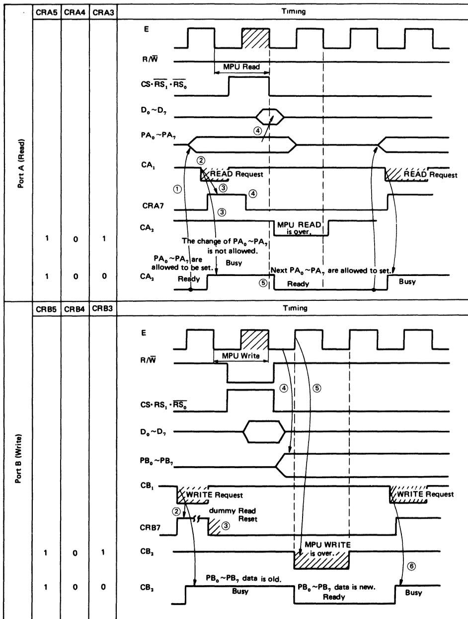
Figure 17 Timing of Hand-shake Mode and Pulse Mode
