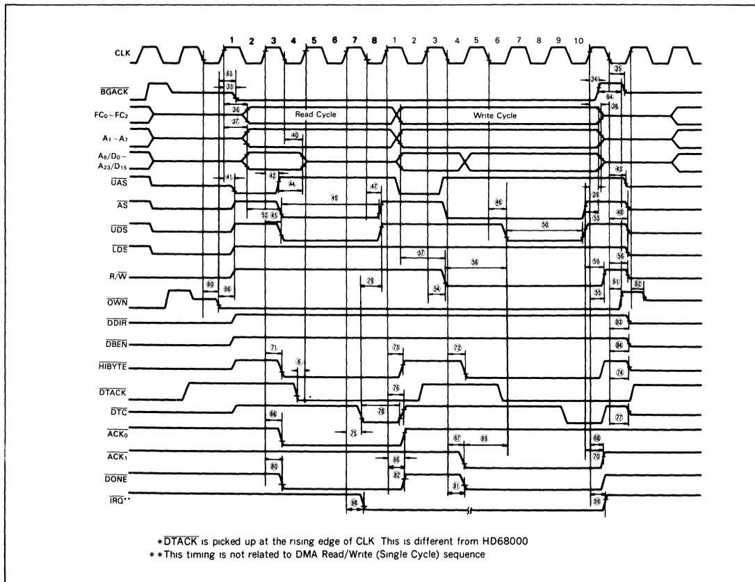
Figure 5 AC Electrical Waveforms-DMA Read/Write (Single Cycle)
