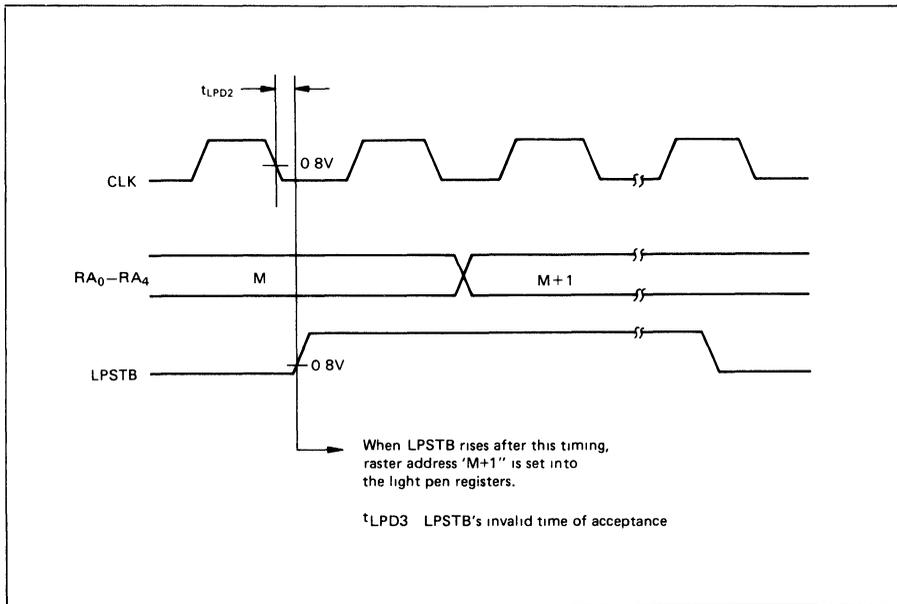
Figure 33 CRTC-CLK, RA<sub>0</sub> – RA<sub>4</sub> and LPSTB Timing
