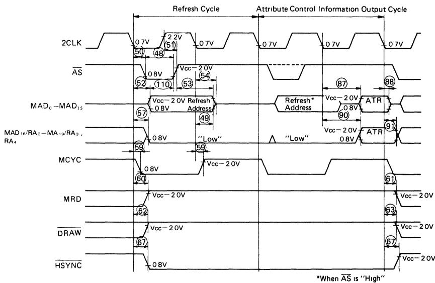
**Figure 12 Frame Memory Refresh/Video Attribute Output Cycle Timing**
