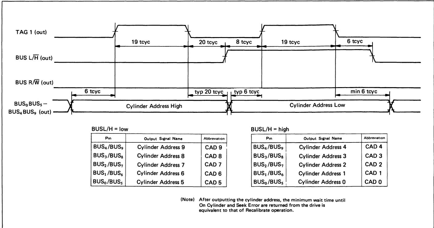
Figure 39 Seek Command Execution Timing (SMD)
