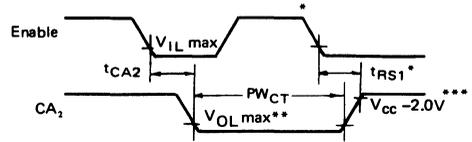
Figure 2 CA<sub>2</sub> Delay Time (Read Mode; CRA5=CRA3=1, CRA4=0)
