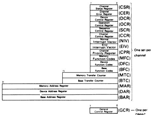
Figure 10 Internal Registers
