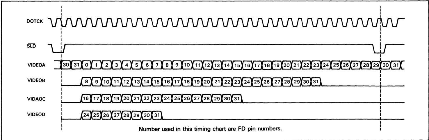
Figure 12. Video Signal Output (32-Dot Shift)
