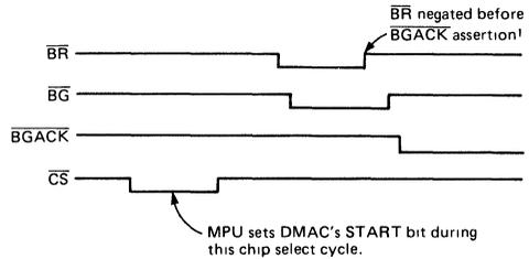
In this timing, the BR is negated too early, e.g. before the BGACK is asserted. This will cause bus contention between the DMAC and the MPU. For the description of these problems, please contact the sales office.
