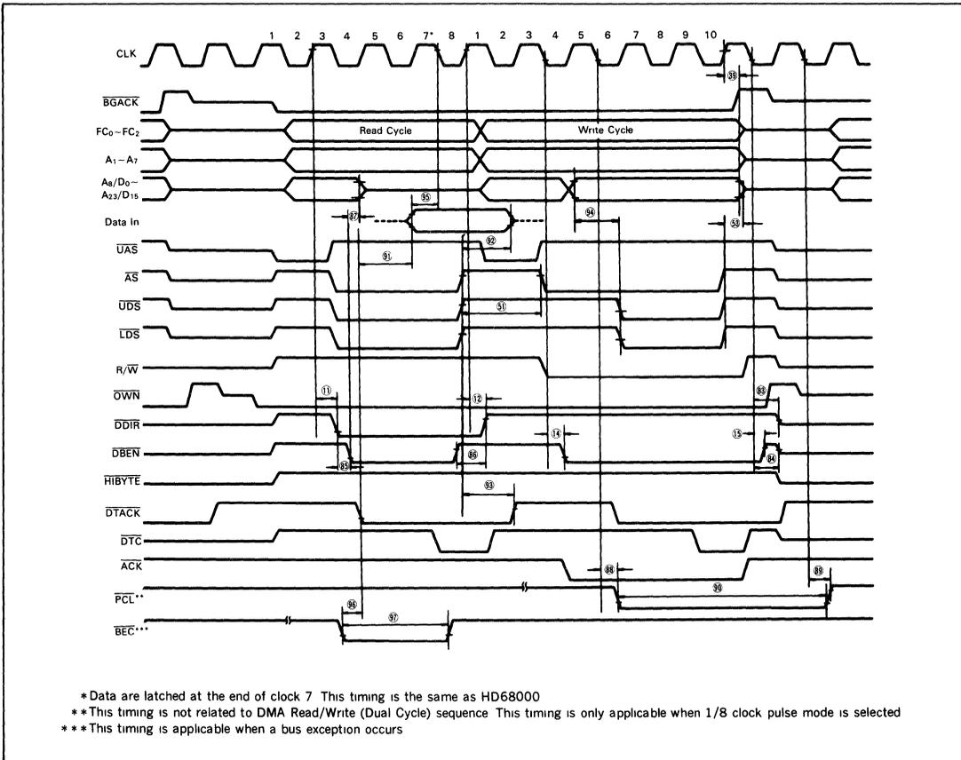
Figure 6 AC Electrical Waveforms-DMA Read/Write (Dual Cycle)
