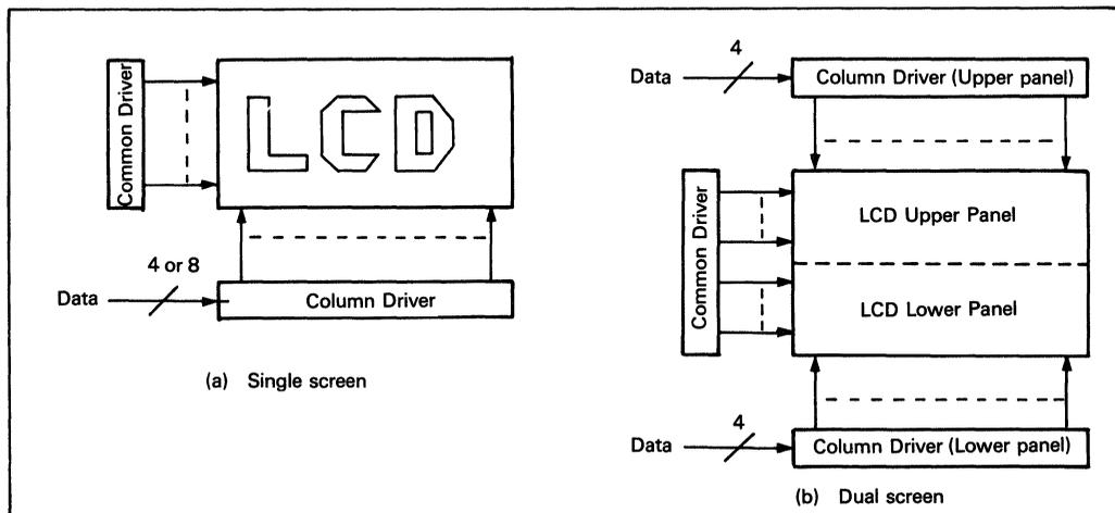
Figure 18. Hardware Configuration According to Screen Format
