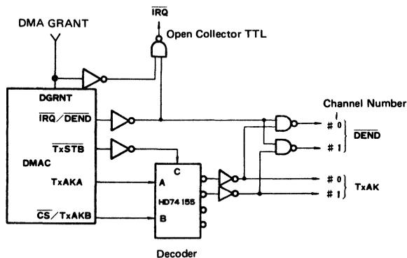
Figure 30 How to Use  $\overline{\text{IRQ}}/\overline{\text{DEND}}$  Output Signal
