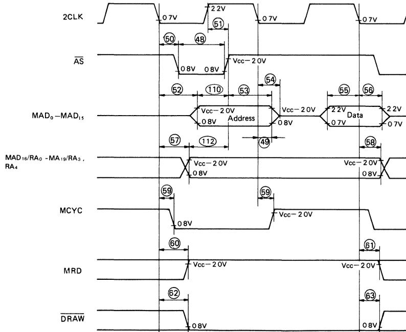
Figure 10 Frame Memory Read Cycle Timing
