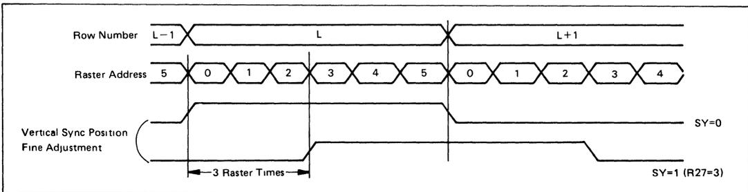
Figure 27 Vertical Sync Position (Vertical Sync Pulse Width = 6)
