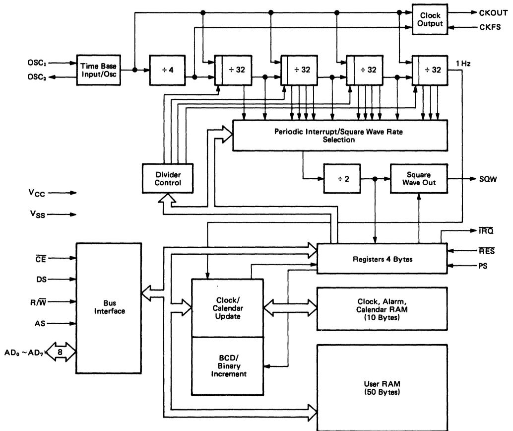
Figure 10 Block Diagram
