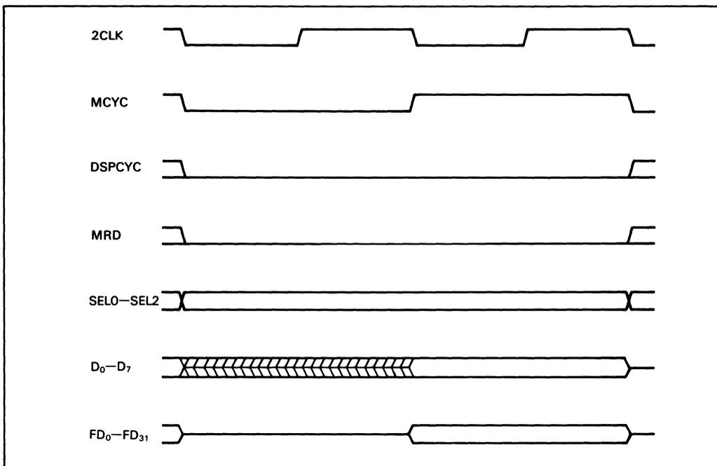
**Figure 4. Drawing Write Cycle**
