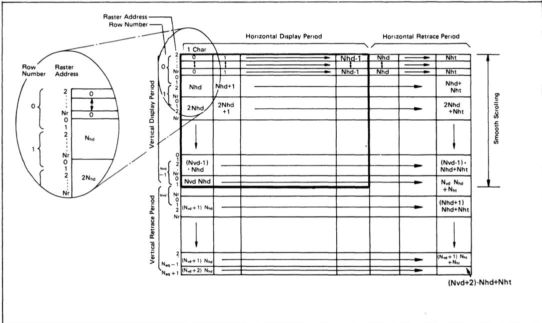
Figure 17 Memory Address and Raster Address in Smooth Scrolling (R29=2)
