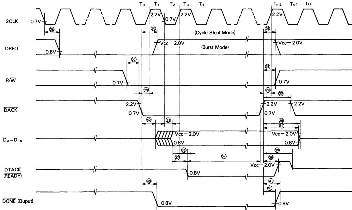
Figure 5 DMA Read Cycle Timing (System Memory ← ACRTC)
