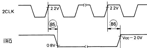
**Figure 18 IRQ Output Timing**
