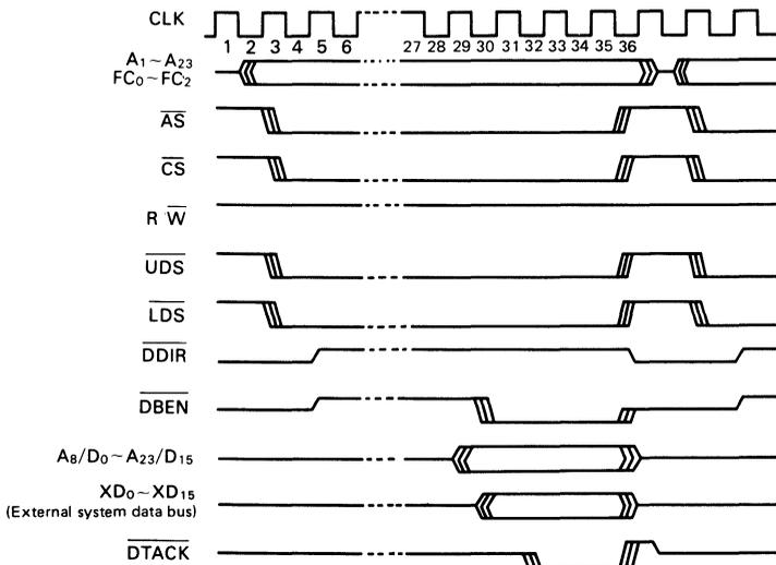
Figure 11 MPU Read from DMAC - Word
