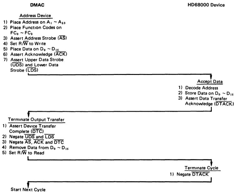
Figure 20 Word Write Cycle Flowchart HD68000 Type Device
