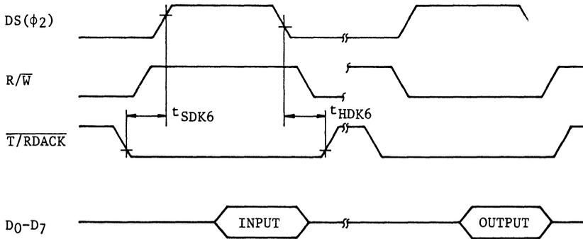
Note)  $\overline{CS}$  input must be fixed high.
