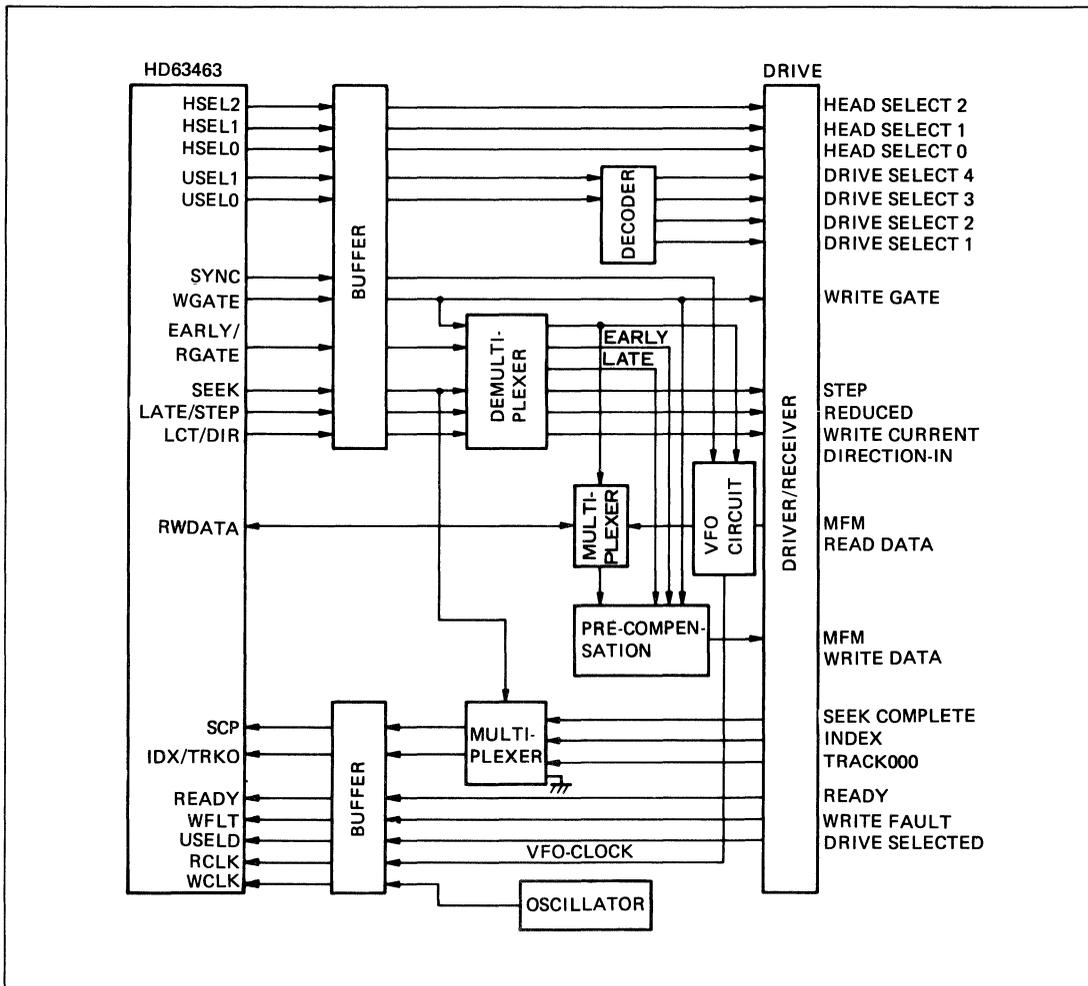
Figure 3 ST506 Interface Circuit
