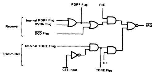
Figure 14 IRQ Internal Circuit
