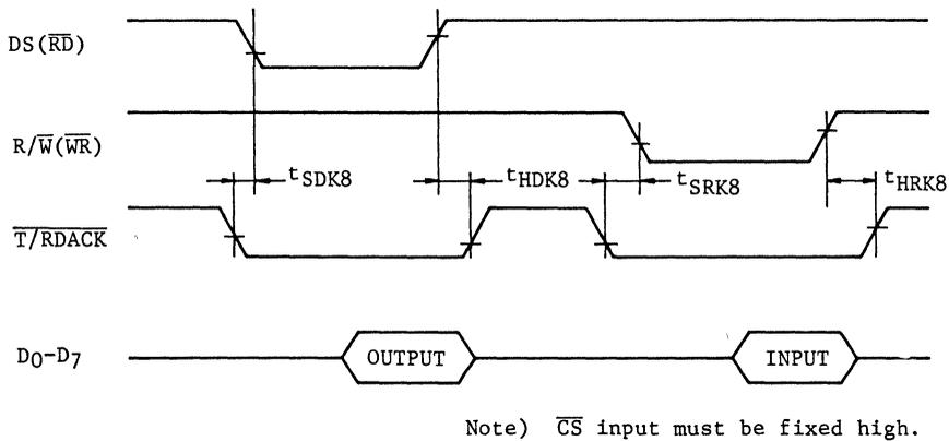
Fig. 1-4 DMA Operation Timing (Using Intel MPU)
