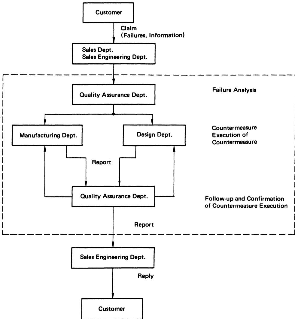
Figure 4 Process Flow Chart of Field Failure
