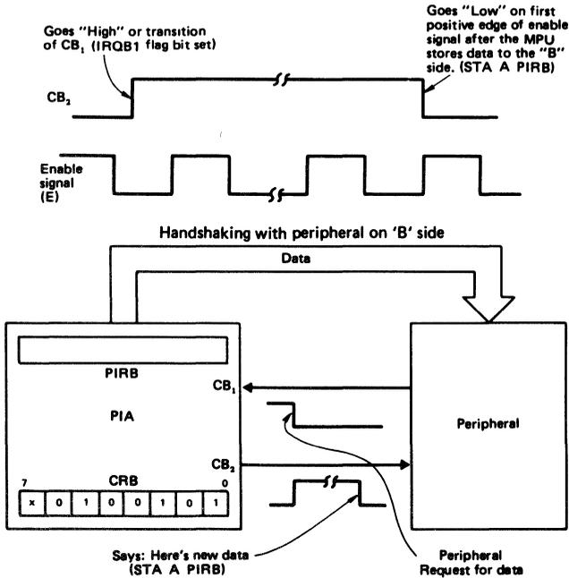
Figure 19 Bits 5, 4, 3 of CRB = 100 (Hand-shake Mode)
