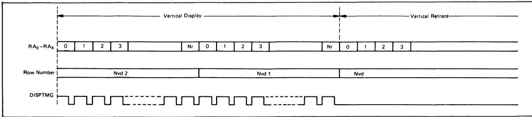
Figure 4 Vertical Display / Retrace Timing
