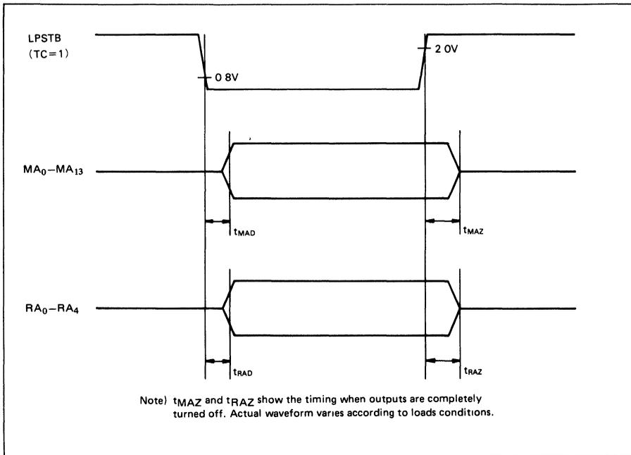
Figure 31 Three-State Delay Timing (Three-state mode: TC = 1)
