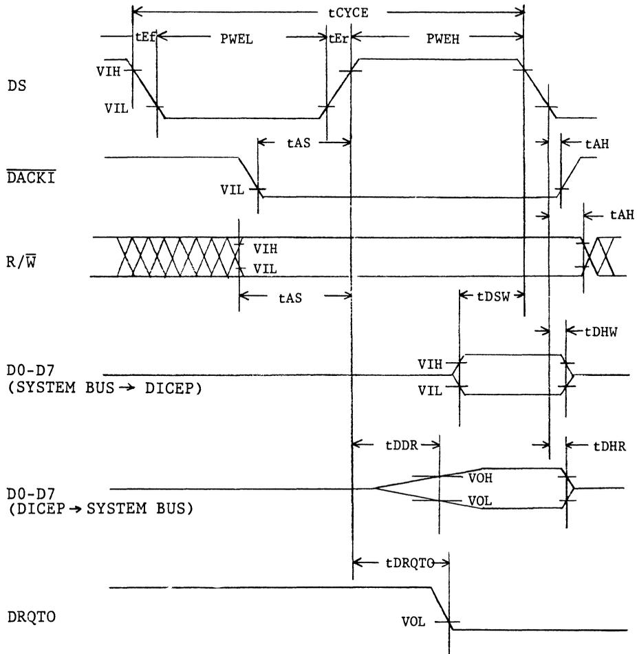
Fig. 1-5 System Bus DMA Timing
