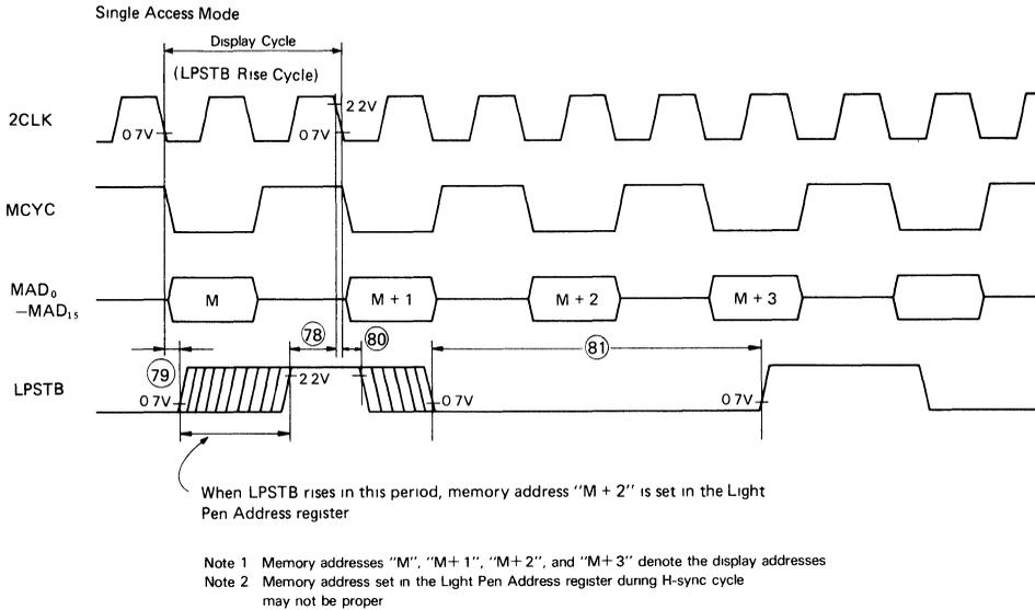
**Figure 15 LPSTB Input Timing (Single Access Mode)**
