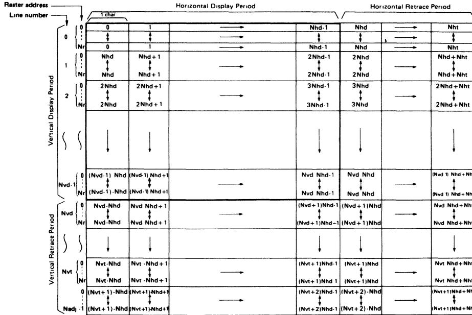
Valid refresh memory address (0~Nvd-Nhd-1) are shown within the thick-line square. Refresh memory address are provided even during horizontal and vertical retrace period. This is an example in the case where the programmed value of start address register is 0.
