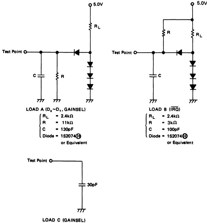
Figure 7 Test Load
