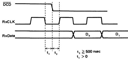
Figure 14  $\overline{DCD}$  Input Timing in External Sync Mode
