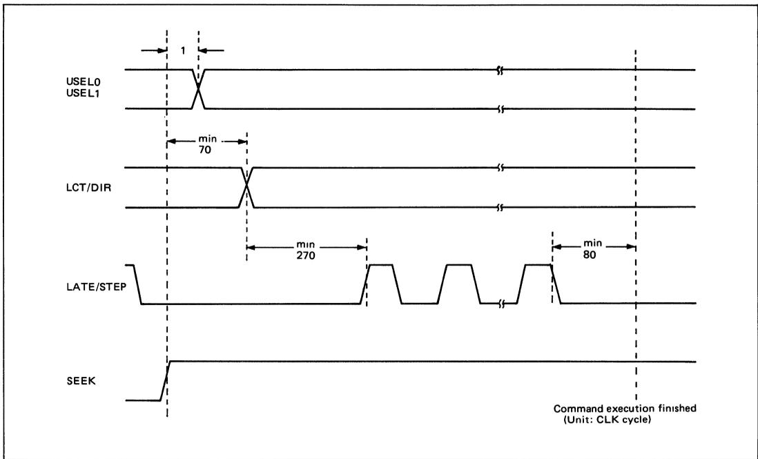
Figure 30 Seek, Recalibrate Command Execution Timing (ST506)
