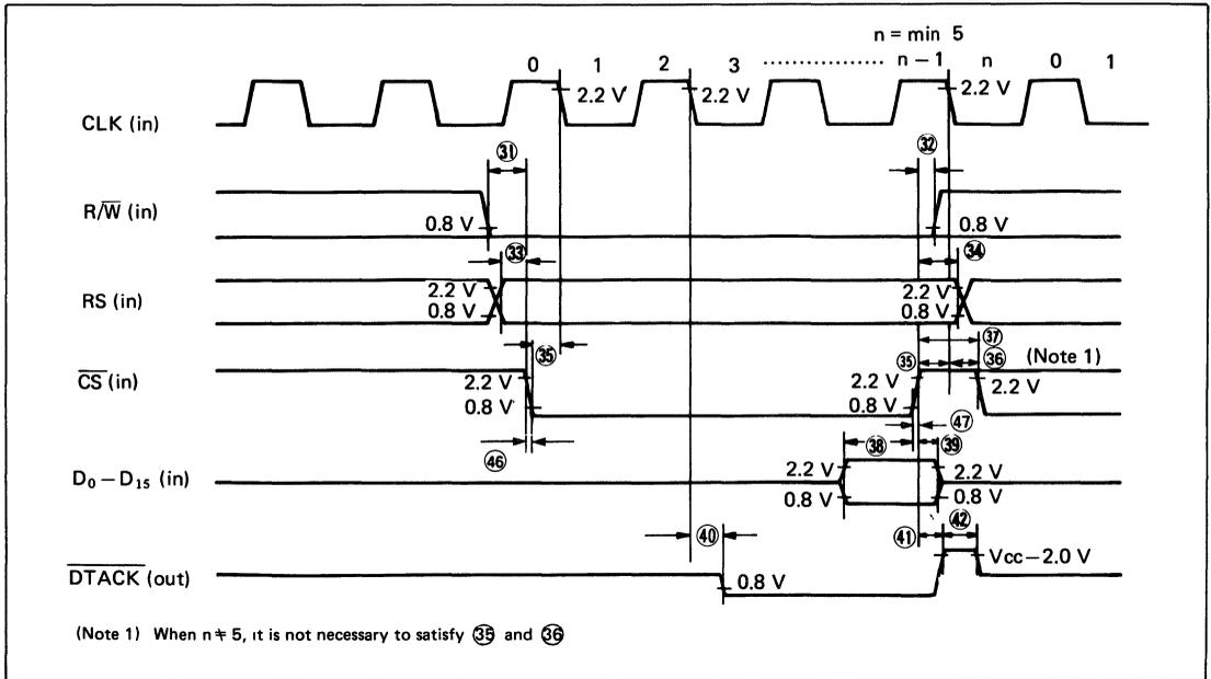
Figure 19 MPU Write Cycle
