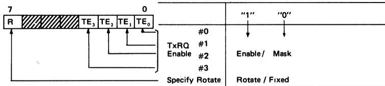
(5) ICR (Interrupt Control Register) (5 bit x 1)
