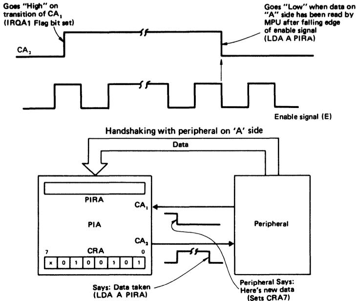
Figure 18 Bits 5, 4, 3 of CRA = 100 (Hand-shake Mode)
