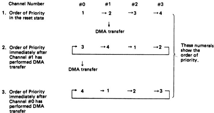
Figure 21 Example of Operation in the Rotate Mode
