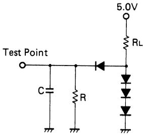
Figure 20 Test Load Circuit A
