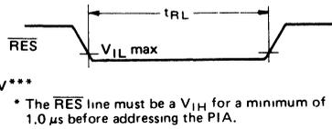
Figure 10  $\overline{\text{RES}}$  Low Time
