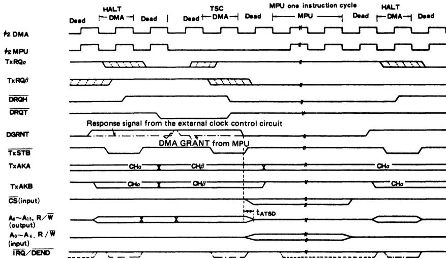
Figure 25 Channel Change (HALT Mode → TSC Mode → HALT Mode)
