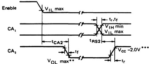
Figure 3 CA<sub>2</sub> Delay Time (Read Mode; CRA5=1, CRA3=CRA4=0)
