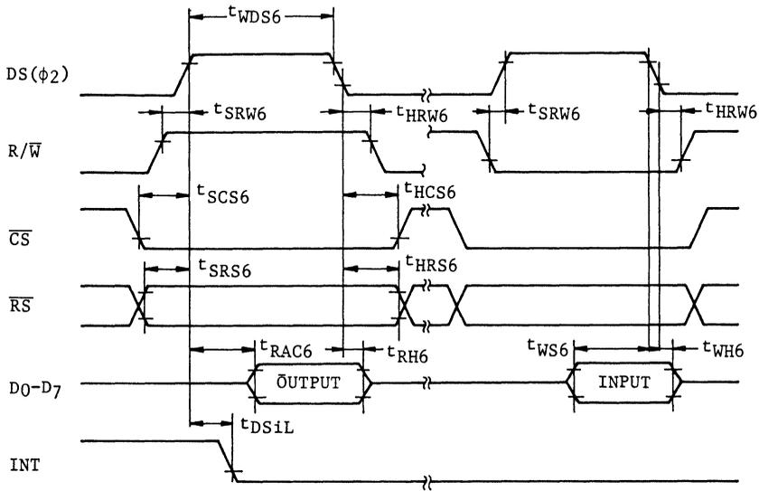
Note)  $\overline{T/RDACK}$  input must be fixed high.
