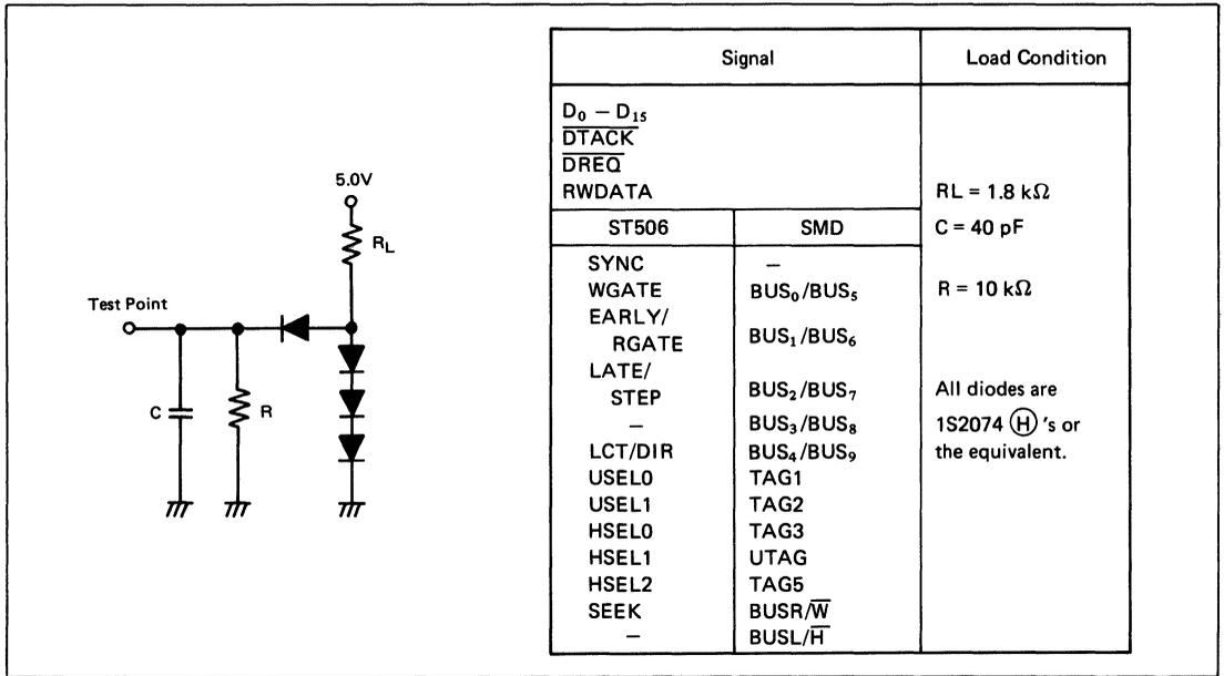
Figure 13 Test Load Circuit A
