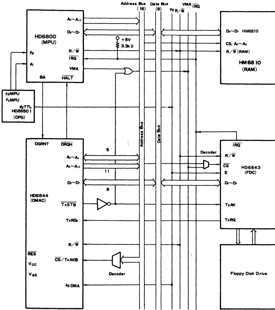
Figure 38 Example of DMA System Structure (1) (minimum)
