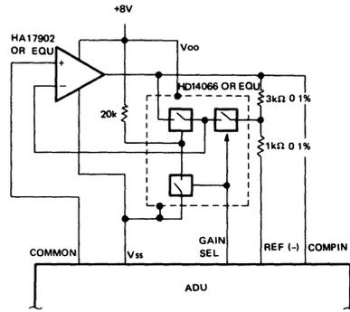
Figure 15 Pre-amplifier Circuit
