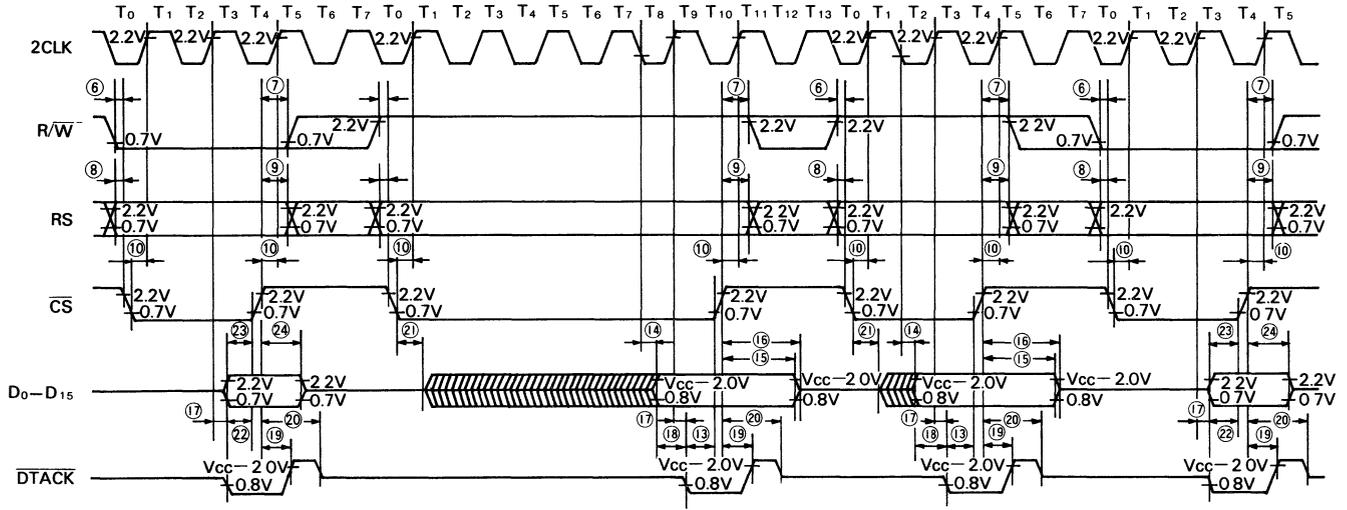
(Note) When the MPU read cycle immediately follows the MPU write cycle execution,  $\overline{DTACK}$  and the read data responses delay (by 3 tcy) even though spec (102) is satisfied.
