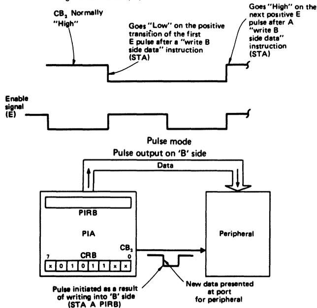
Figure 21 Bits 5, 4, 3 of CRB = 101 (Pulse Mode)
