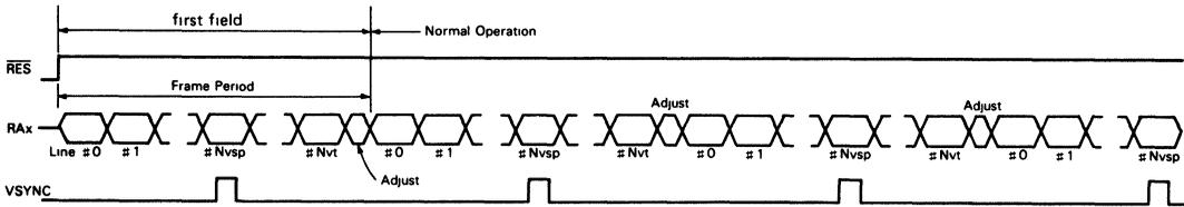
Figure 43 RES Release Sequence in The Non-interlace Mode
