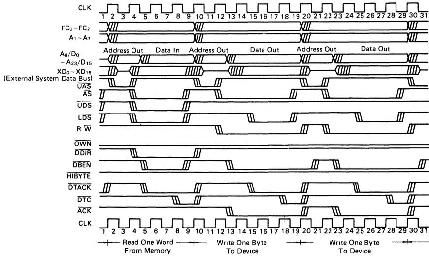
Figure 24 Dual Addressing Mode, Read/Write Cycle,
