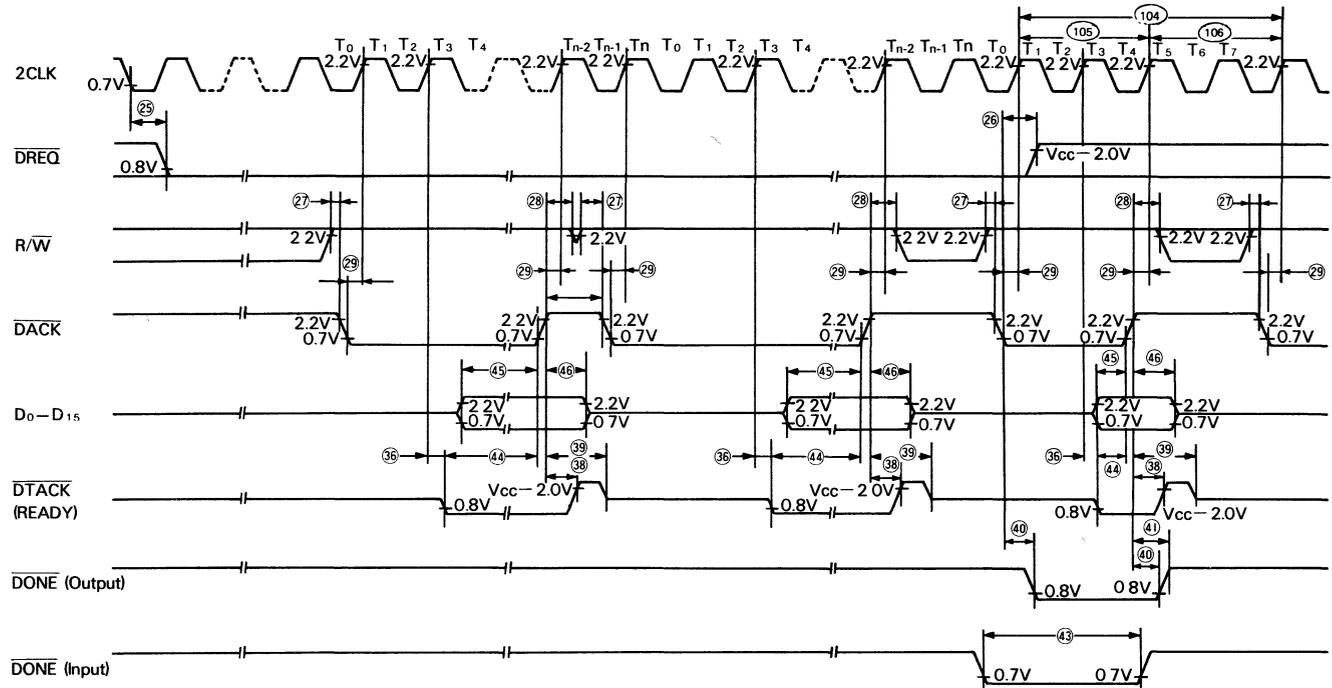
(Note)  $\overline{DACK}$  "high" level width must satisfy spec (30). Unless satisfying spec (106), DTACK response delays to the succeeding cycle. When the ACRTC is used with the synchronous bus timing, specifications (104), (105) and (106) must be satisfied.
