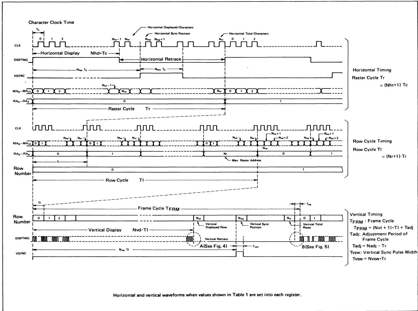
Figure 3 CRTC-II Timing Chart (Non-Interlace mode)
