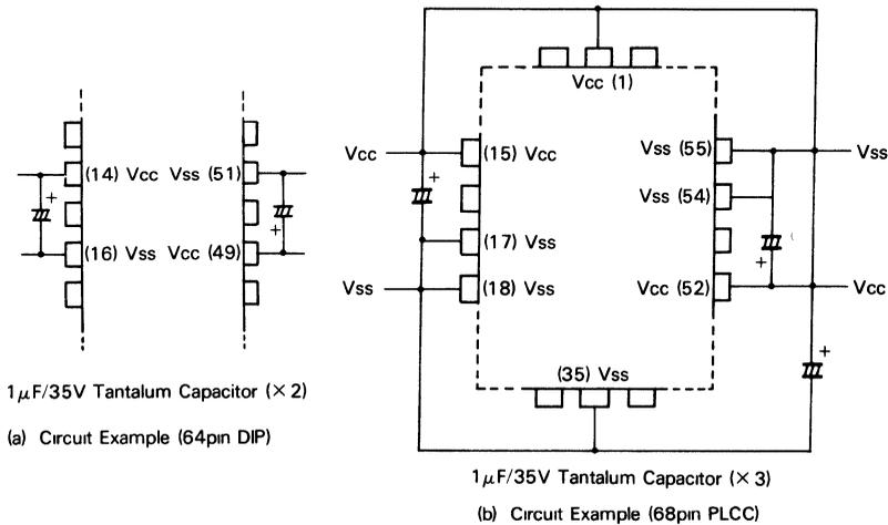
**Figure 25 Note for Designing Power Supply Circuit**
