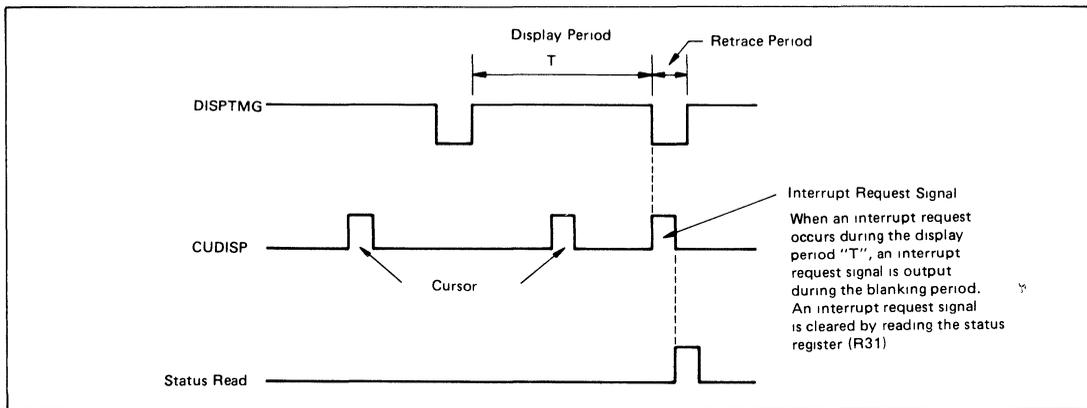
Figure 23 Interrupt Timing
