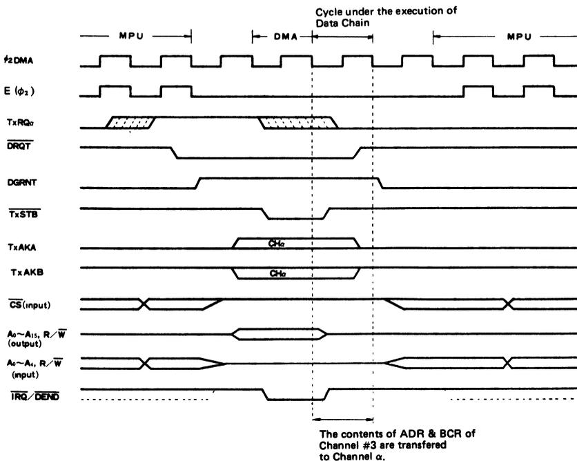
Figure 33 Data Chain Operation (TSC Mode)
