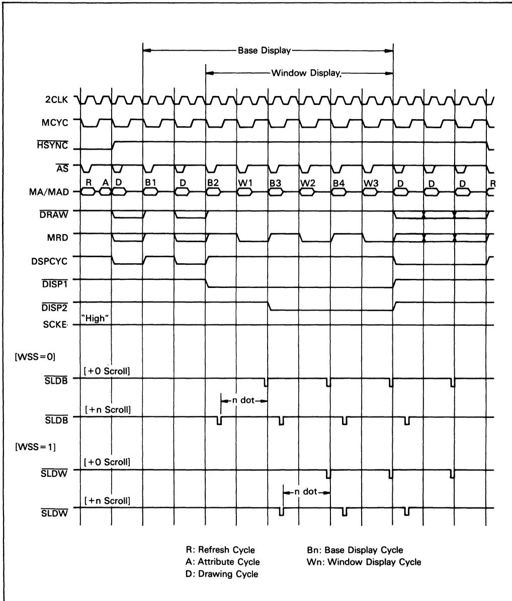
Figure 11. SLDB and SLDW Timing (Dual Access Mode 1)
