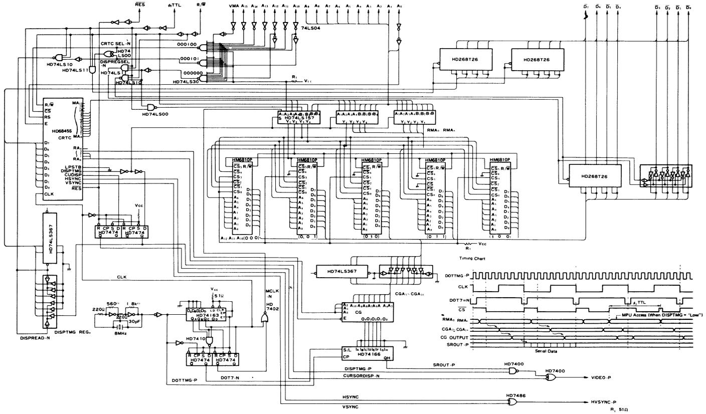
Figure 41 Example of Applied Circuit of the CRTC (Monochrome Character Display)
