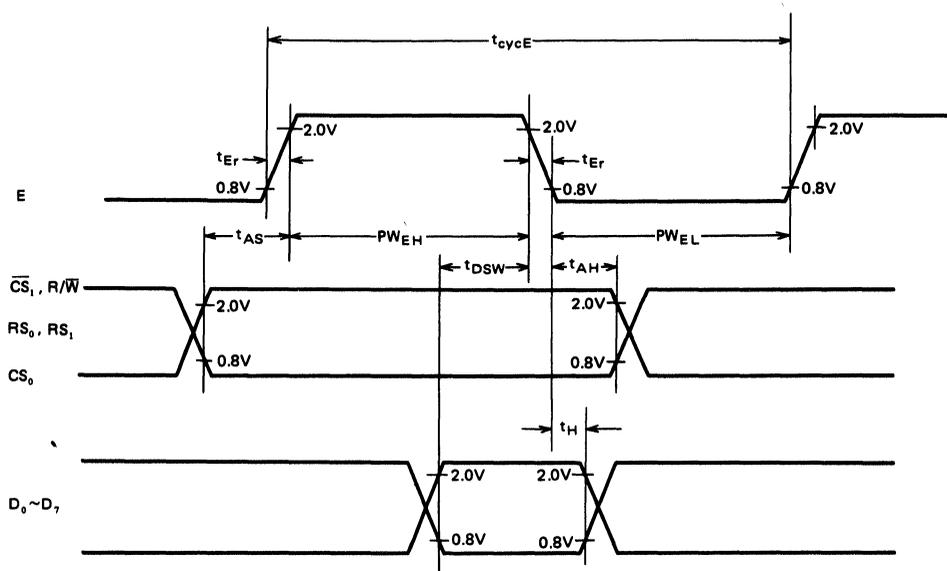
Figure 6 Write Timing
