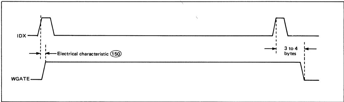
Figure 29 Write Format Timing (ST506)
