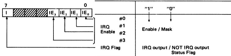
(6) DCR (Data Chain Control Register) (4 bit x 1)
