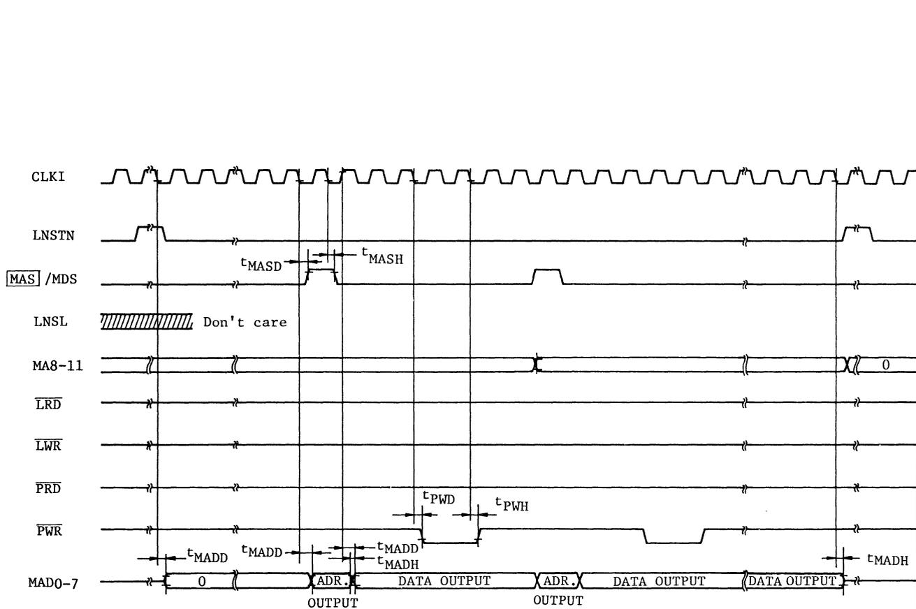
Fig. 1-20 Memory Bus Interface Timing in C or D Mode (2)
