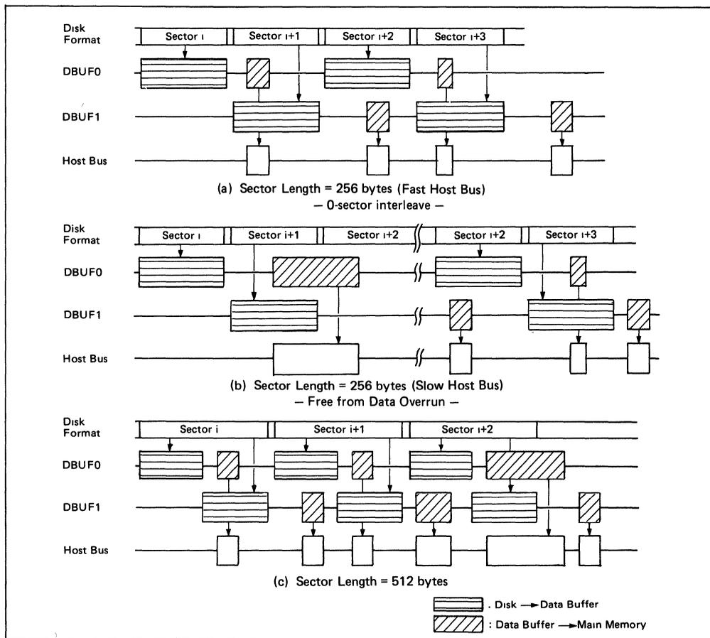
Figure 9 DMA Data Transfer in Read Data and Read Erroneous Data Command Execution
