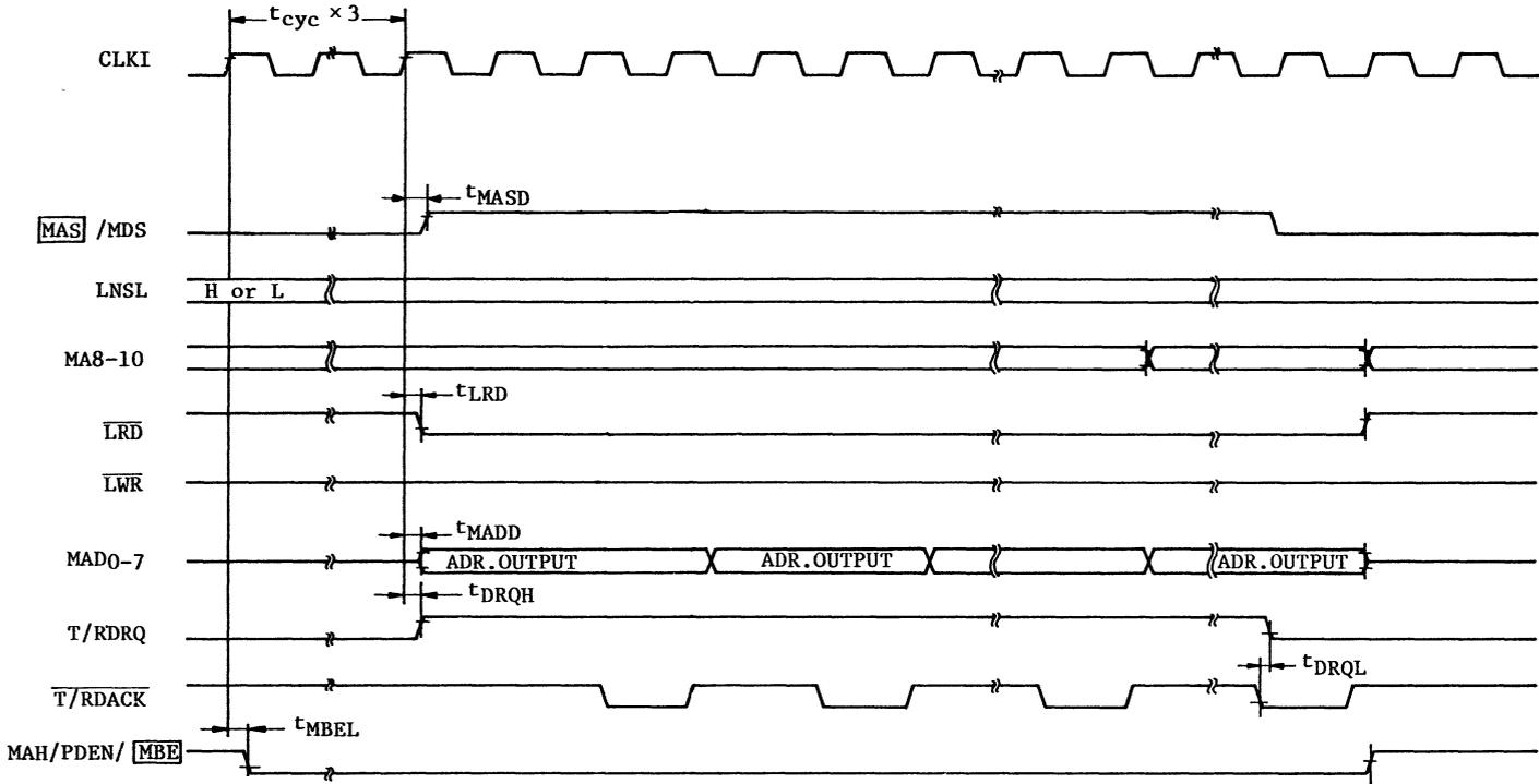
Fig. 1-15 Memory Bus Interface Timing in A Mode (2)
