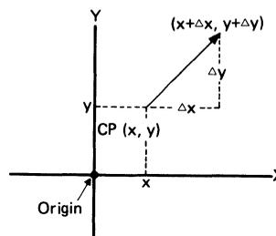
Figure 35 Relative Coordinate Specification
