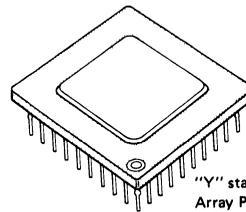
"Y" stands for Pin Grid Array Package.
