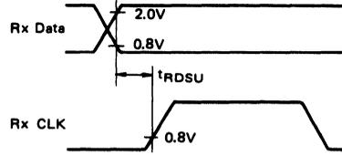
Figure 4 Receive Data Setup Time (±1 Mode)
