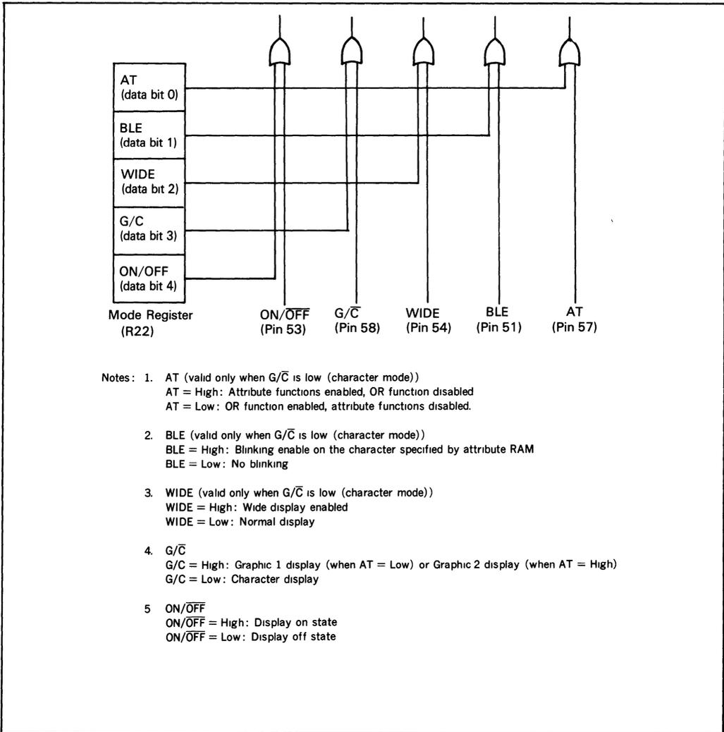
**Figure 31. Correspondence between Mode Register and External Pins**
