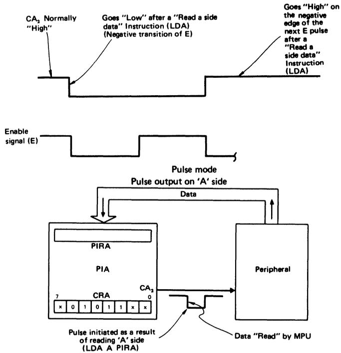
Figure 20 Bits 5, 4, 3 of CRA = 101 (Pulse Mode)
