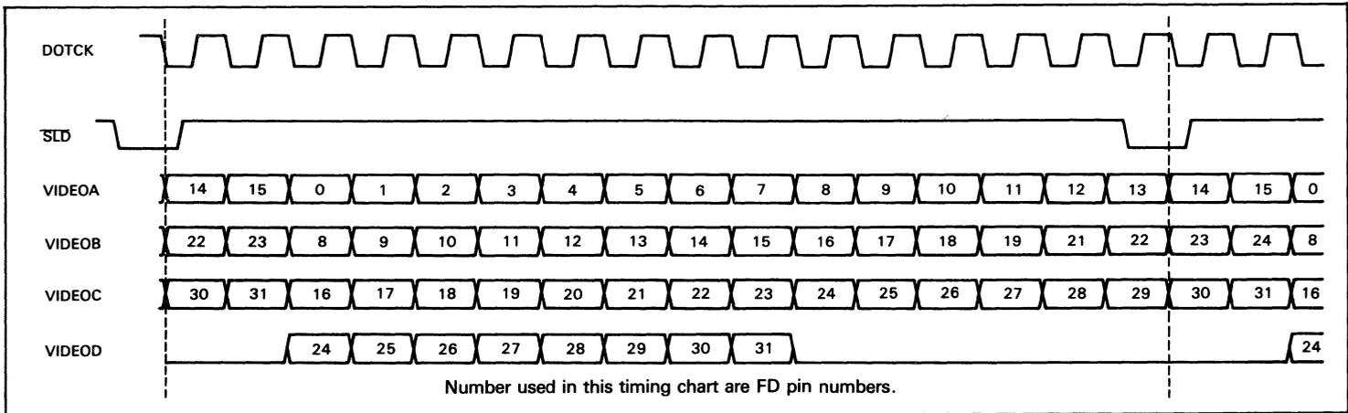
Figure 13. Video Signal Output (16-Dot Shift)
