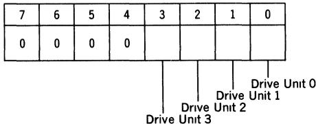
In SMD interface, bits 0–7 correspond to drives 0–7 respectively. To connect a drive, write “1” into the corresponding bit (up to 8 drives can be connected).
