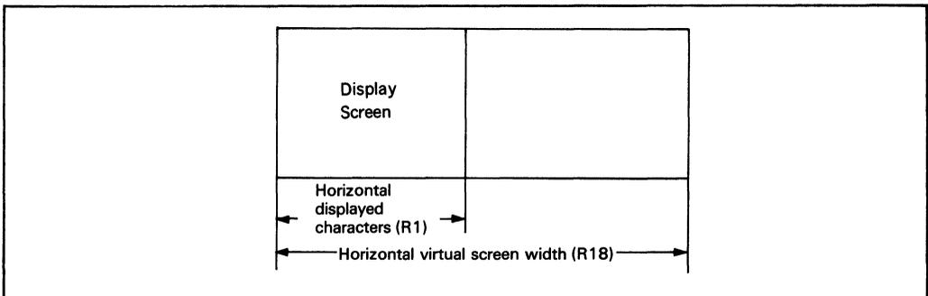
Figure 10. Horizontal Virtual Screen Width
