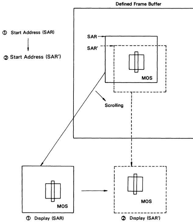
Figure 55 Scrolling by SAR (Start Address Register) Rewrite
