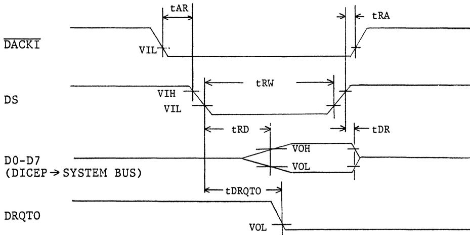
Fig. 1-6 System Bus DMA Timing
