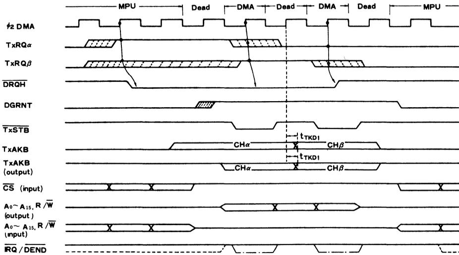
Figure 23 Channel Change (HALT Mode → HALT Mode)
