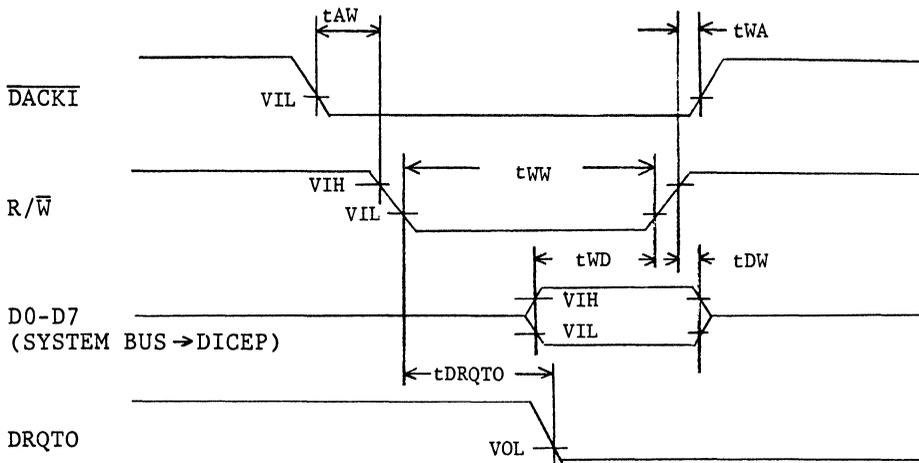
Fig. 1-7 System Bus DMA Timing
