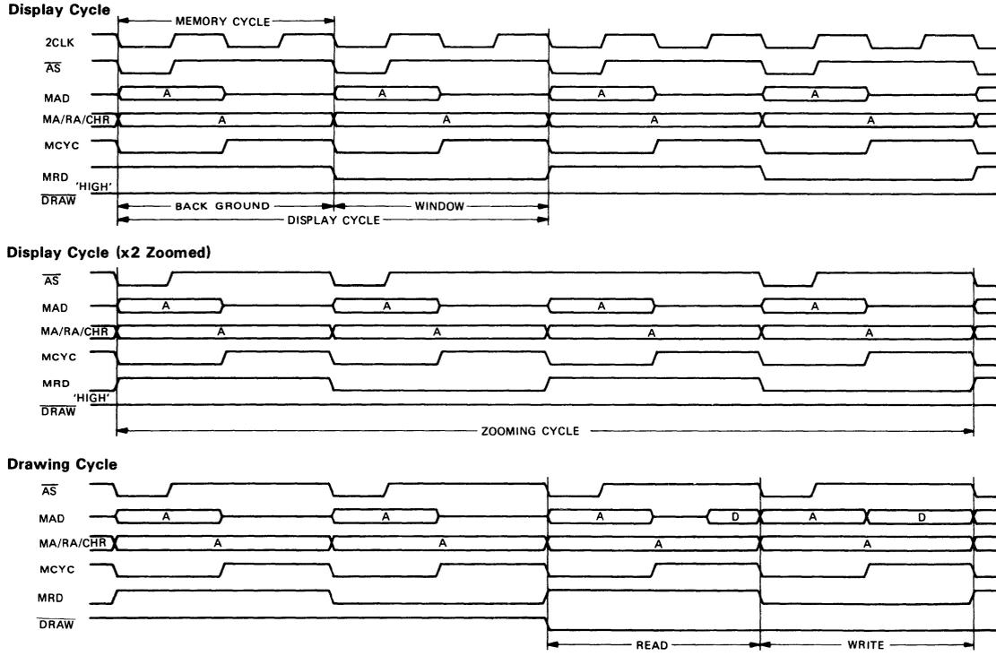
Figure 41 Superimposed Access Mode Timing
