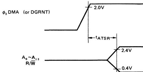
Delay Time of Address Three-state
