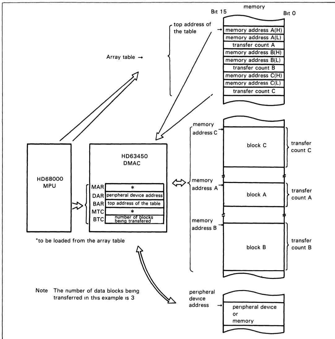
Figure 38 Transfer Example of the Array Chaining Mode
