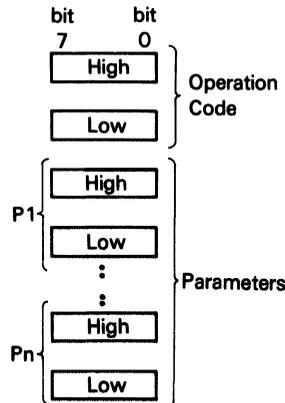
Figure 31(b) 8-bit Interface Command Format
