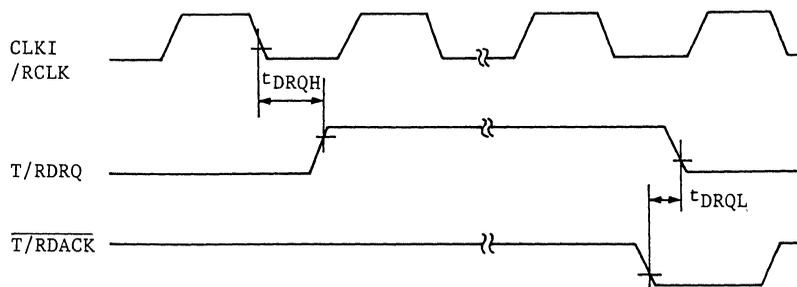
Fig. 1-5 T/RDRQ Output Timing
