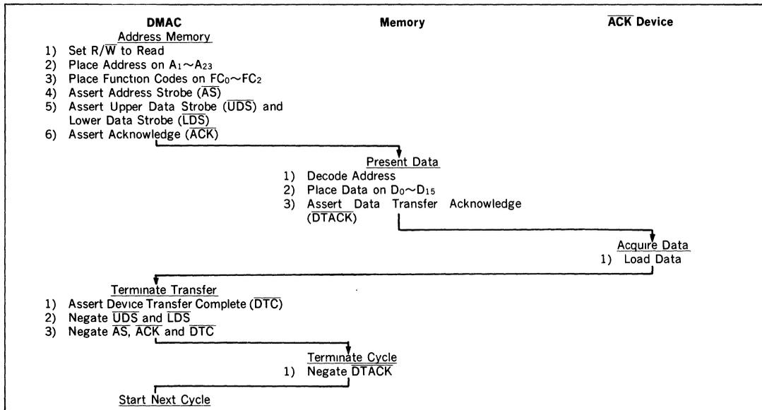
Figure 28 Word from Memory to Device with  $\overline{ACK}$
