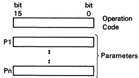
Figure 31(a) 16-bit Interface Command Format
