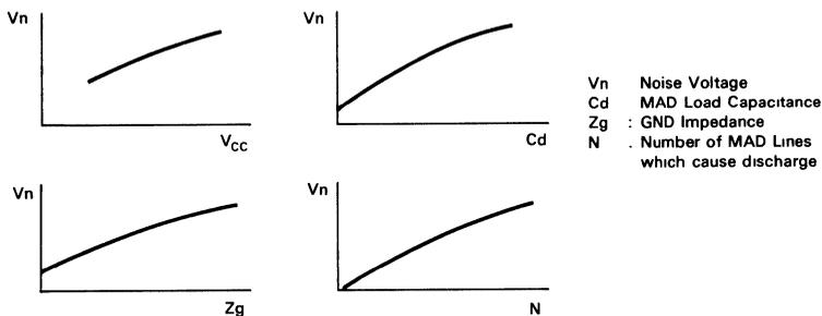
Figure 63 Relations Between the Noise Voltage and Parameter
