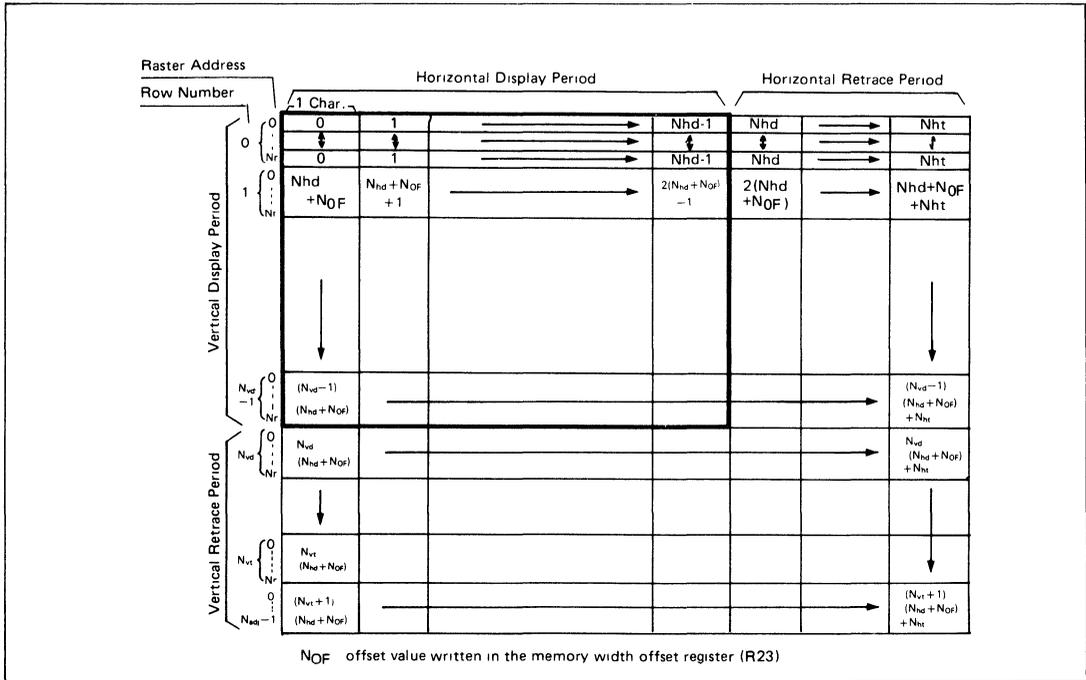
Figure 15 Memory Address and Raster Address in Memory Width Setting
