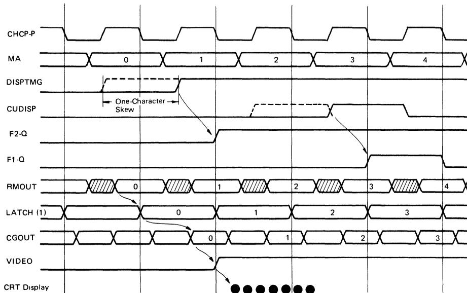
Figure 25 Time Chart of Display Control Unit (2)
