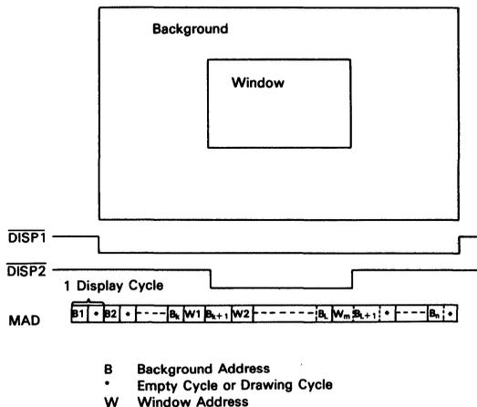
Figure 57 Horizontal Smooth Scroll – Window Screen (WSS=1)
