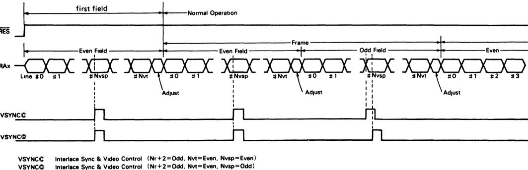
Figure 45 RES Release Sequence in The Interlace Mode (2)
