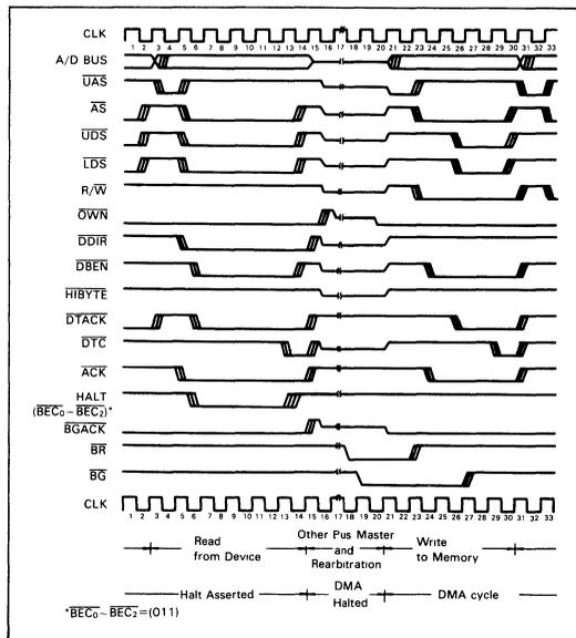
Figure 40 Halt Operation
