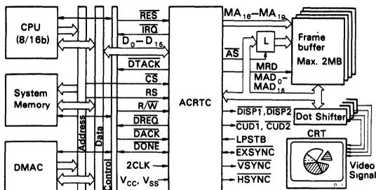
Figure 26 System Configuration
