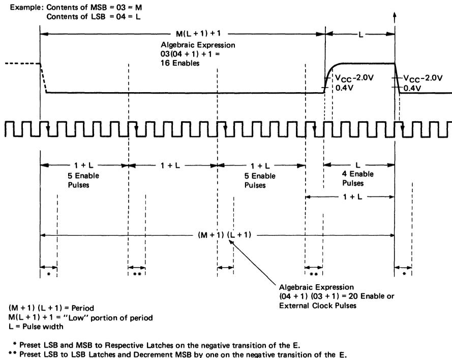
Figure 9 Timer Output Waveform Example
