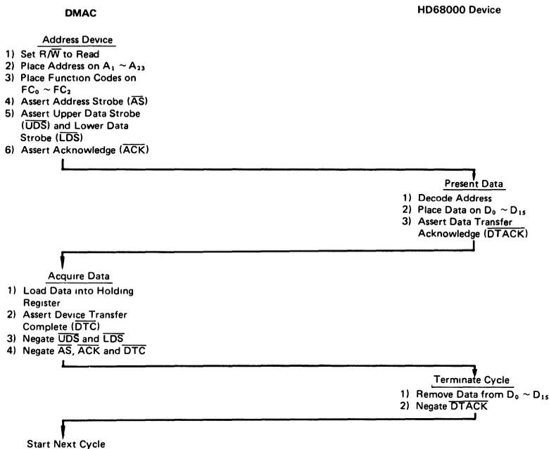
Figure 19 Word Read Cycle Flowchart HD68000 Type Device
