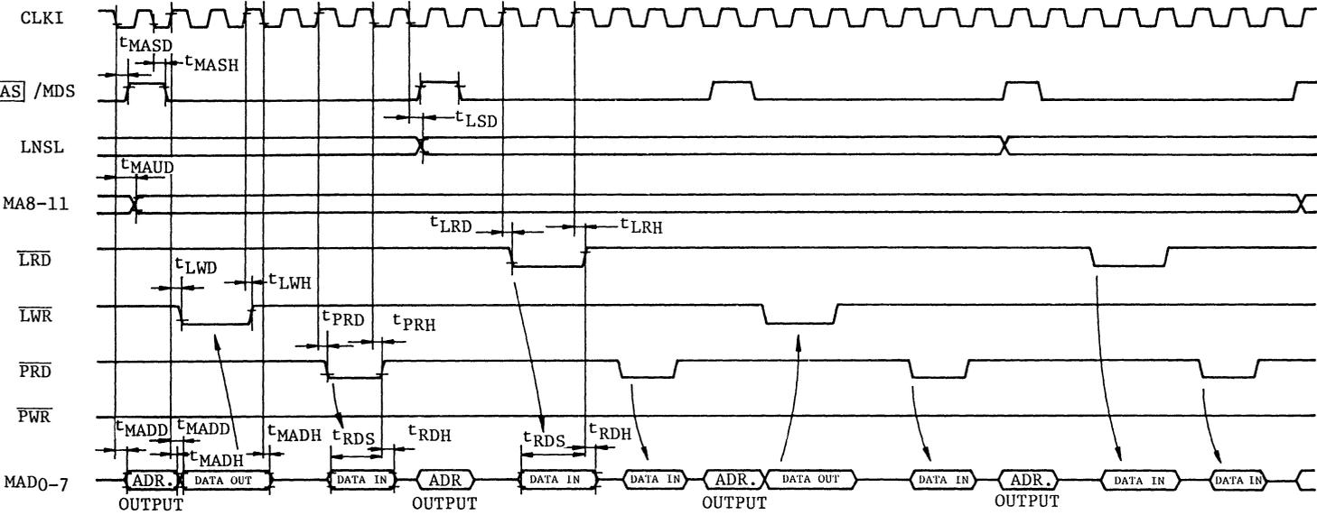
Fig. 1-19 Memory Bus Interface Timing in C or D Mode (1) During Image Data Processing
