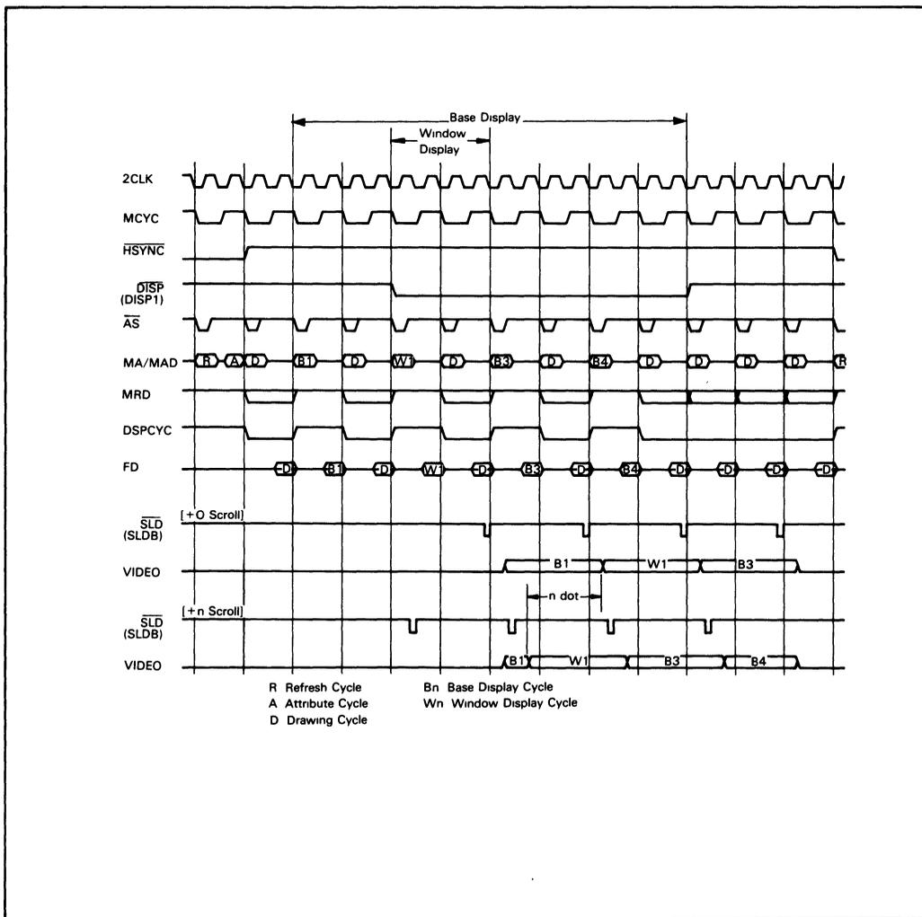
Figure 10. Video Output Timing (Dual Access Mode 0)
