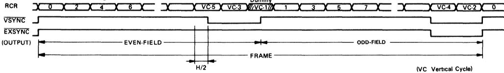
Figure 59 Raster Scan Timing
