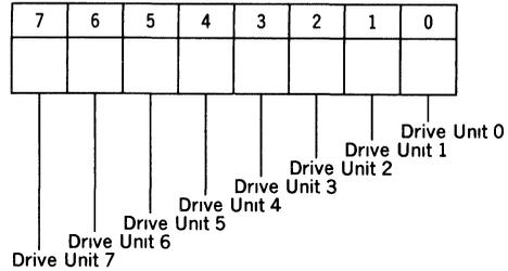
In SMD interface, OM2 specifies drive control output signal from the HDC during data read command execution. In data write command (all the commands that assert WGATE signal) and SEK, RCLB command execution, outputs of drive control signals are low regardless of the contents of OM2. Bits 4–7 in OM2 are to be set to “0”.
