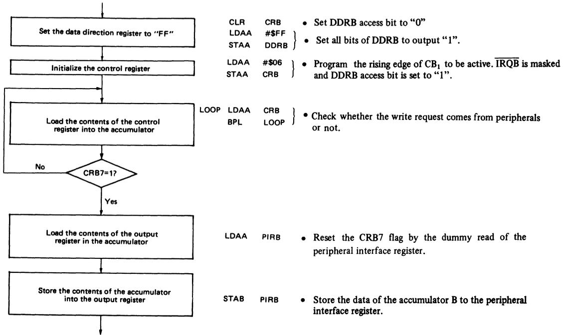
Interrupt request flag bits (CRA7, CRA6, CRB7 and CRB6) cannot be written and they cannot be also reset by write operation to the peripheral interface register. So dummy read of peripheral interface register is needed to reset the flags.
