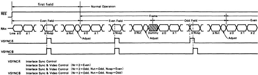
Figure 44 RES Release Sequence in The Interlace Mode (1)
