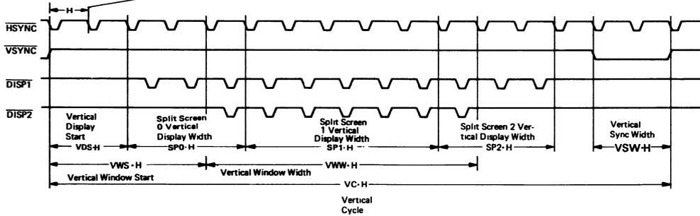
Figure 49 Display Scan Sequence (Horizontal and Vertical)
