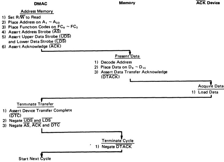
Figure 28 Word from Memory to Device with  $\overline{ACK}$
