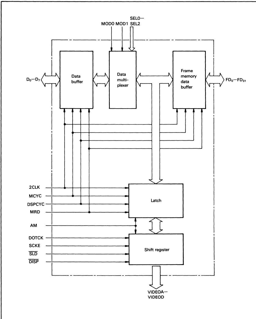
Figure 2. GVAC Block Diagram
