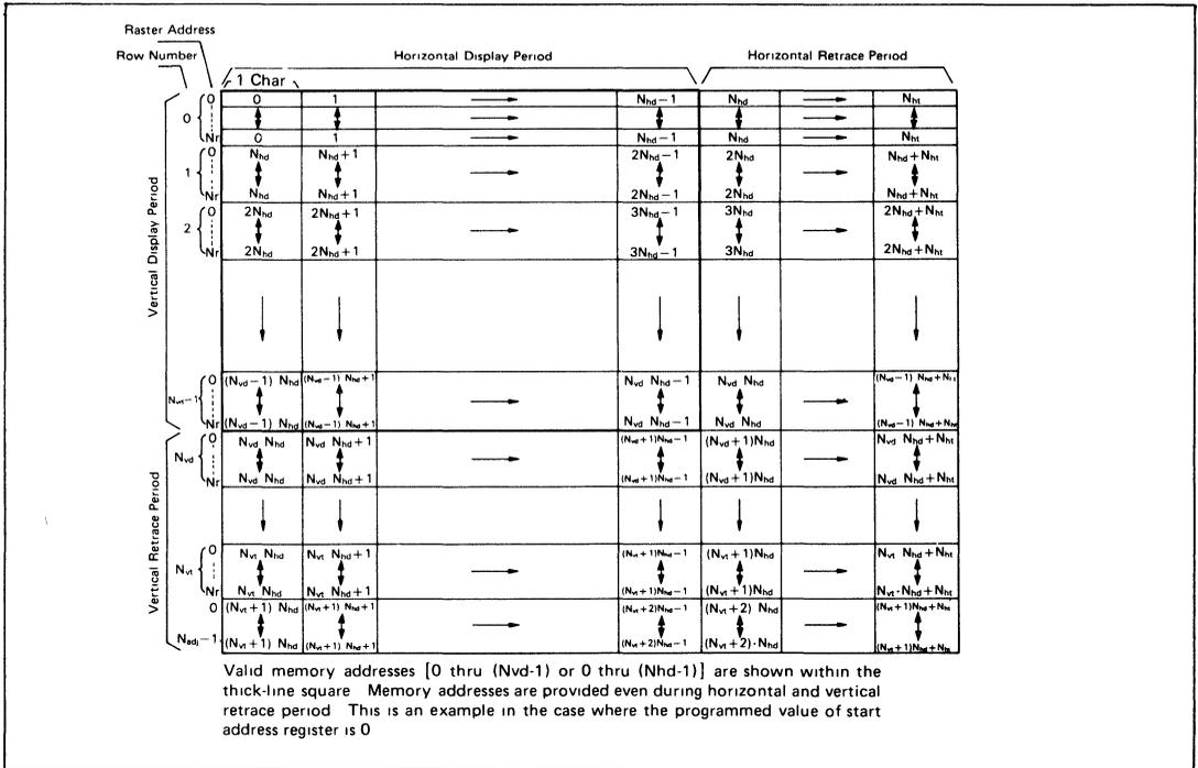
Valid memory addresses [0 thru (Nvd-1) or 0 thru (Nhd-1)] are shown within the thick-line square. Memory addresses are provided even during horizontal and vertical retrace period. This is an example in the case where the programmed value of start address register is 0.
