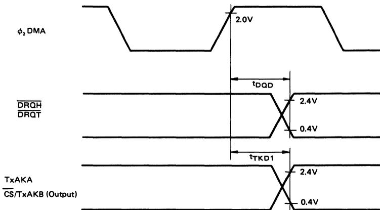
Figure 5 Timing of  $\overline{\text{DRQH}}$ ,  $\overline{\text{DRQT}}$ , TxAK Outputs
