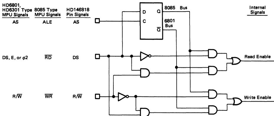
Figure 13 Functional Diagram of the Bus Control Circuit
