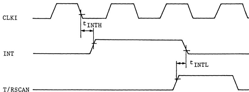
Fig. 1-6 INT Output Timing
