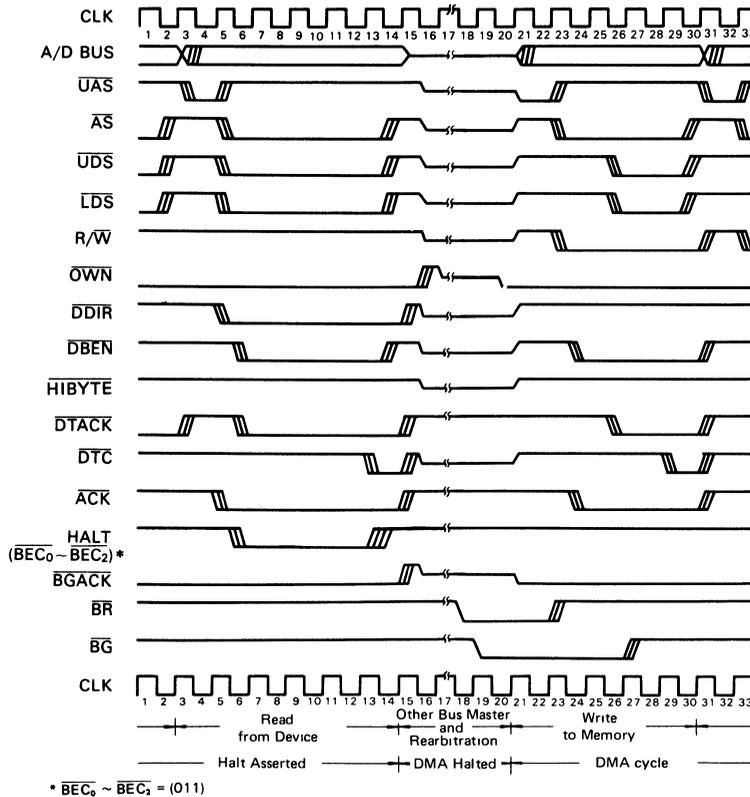
Figure 39 Halt Operation
