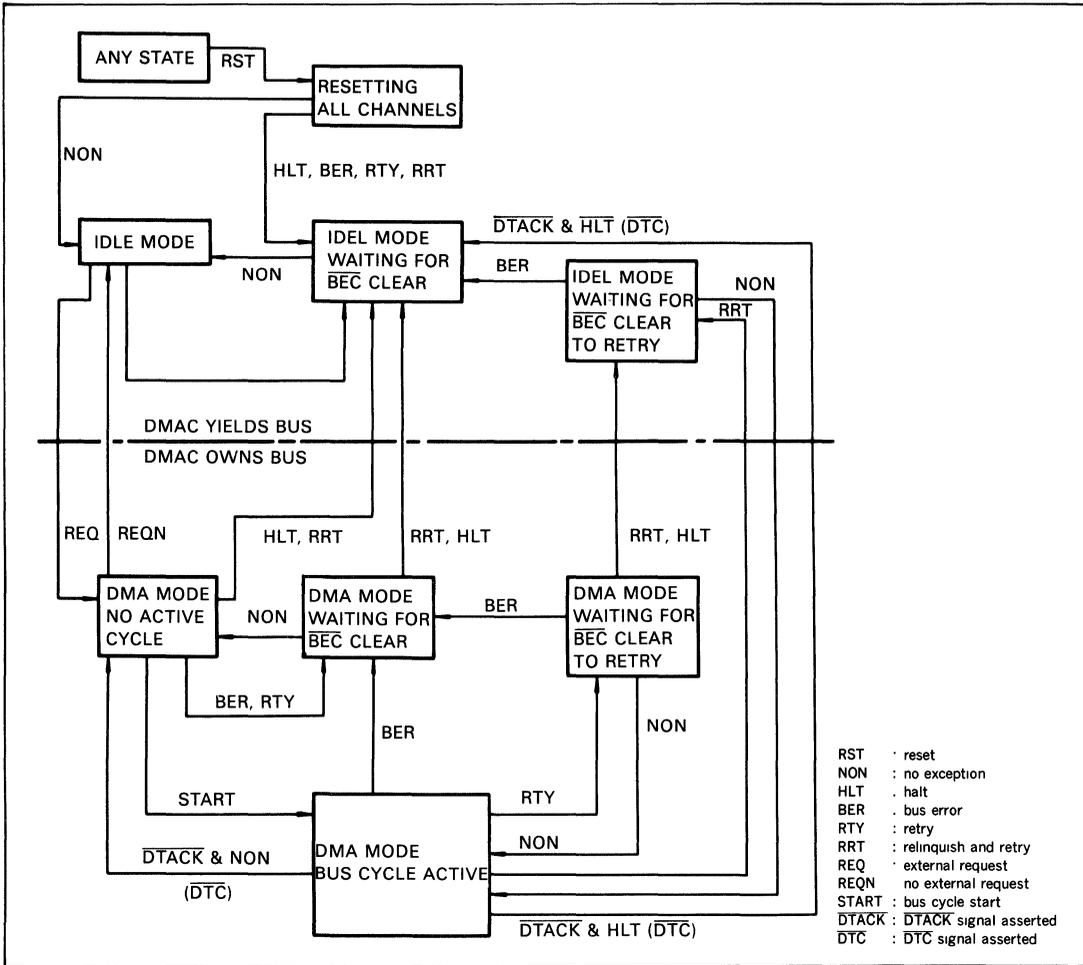
Figure 44 Bus Exception Flow Diagram
