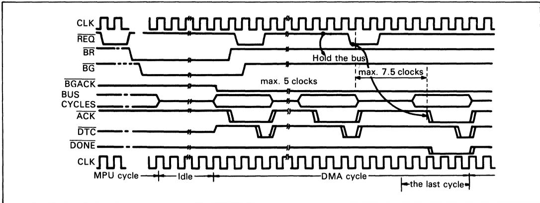
Figure 18 Cycle Steal Bus Hold Mode Request Timing
