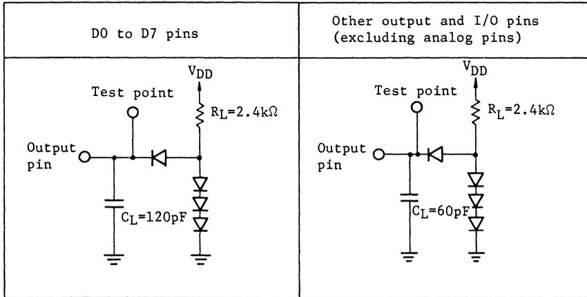
[Notes] 1.  $C_L$  includes stray capacitance caused by the probe and load capacitance.
