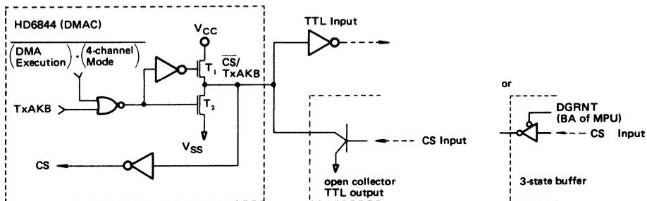
In  $\overline{\text{CS}}$  input mode T1 turns ON and T2 turns OFF. T1 functions as pull-up resistance.
