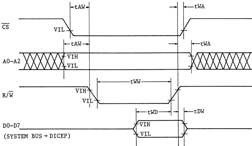
Fig. 1-4 System Bus Write Timing
