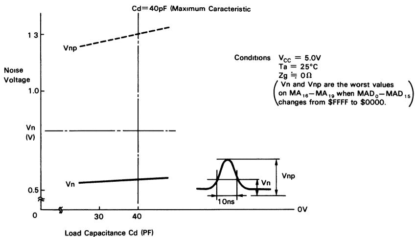
Figure 65 Relation Between the Noise and MAD Load Capacitance
