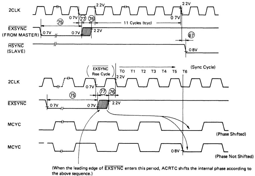
Figure 14 EXSYNC Input Timing
