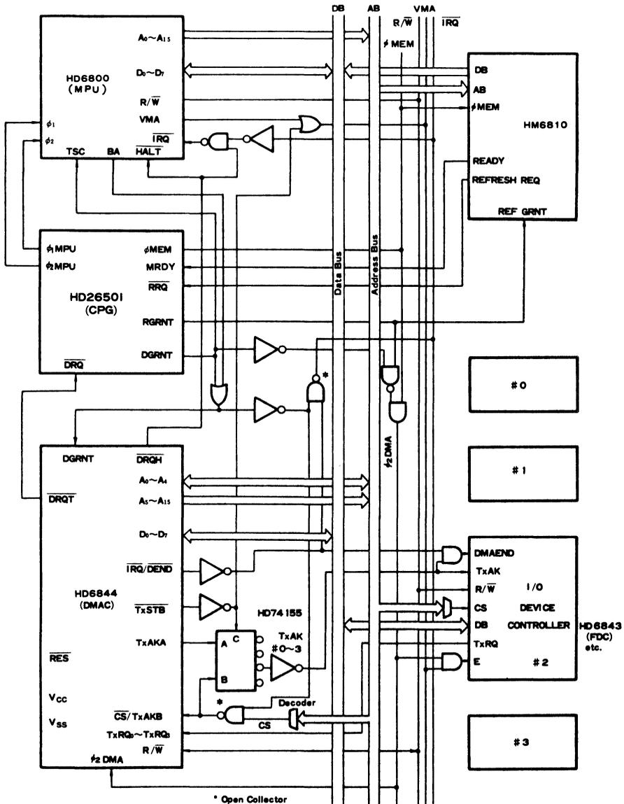
Figure 39 Example of DMA System Structure (2) (maximum)
