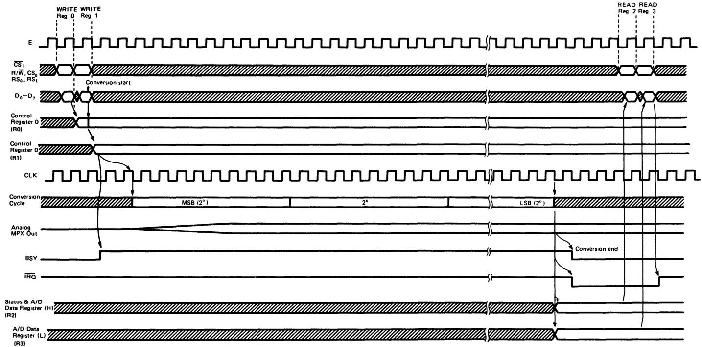
Figure 13 A/D Conversion Timing Chart (Basic Sequence)
