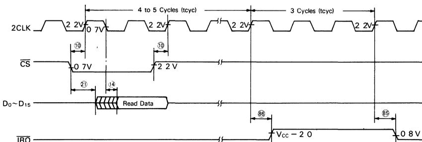
This is an  $\overline{IRQ}$  output timing example. In this case,  $\overline{IRQ}$  is generated by status flag RFF (Read FIFO Full).
