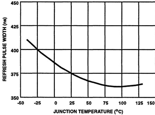
FIGURE 16.  $T_{REF-PW}$  REFRESH PULSE WIDTH vs TEMPERATURE
