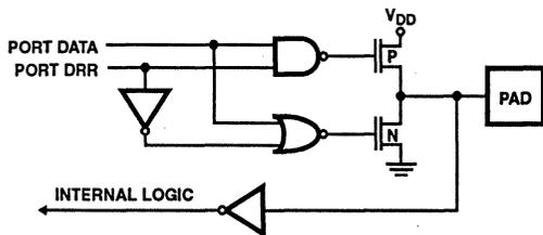
FIGURE 5A. PORT A I/O PAD CIRCUITRY
