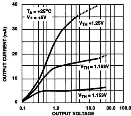
FIGURE 19. OUTPUT CURRENT AS A FUNCTION OF OUTPUT VOLTAGE
