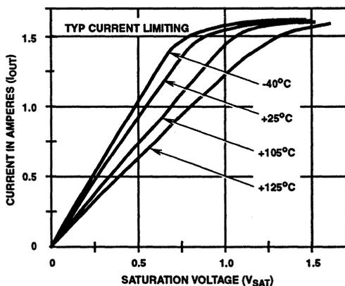
FIGURE 4B. CA3282 TYPICAL OUTPUT DRIVER  $R_{DS(ON)}$  CHARACTERISTICS OF CURRENT OUT vs SATURATION VOLTAGE,  $V_{SAT}$  FOR A  $-40^{\circ}\text{C}$  TO  $+125^{\circ}\text{C}$  JUNCTION TEMPERATURE
