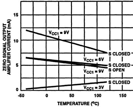
FIGURE 6C. OUTPUT AMPLIFIER CHARACTERISTICS OF I<sub>CC2</sub> CURRENT vs AMBIENT TEMPERATURE
