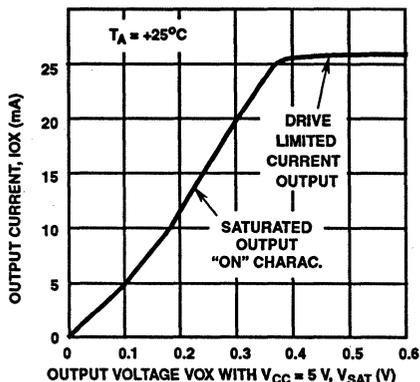
FIGURE 2. TYPICAL OUTPUT DRIVER SATURATED "ON" CHARACTERISTIC
