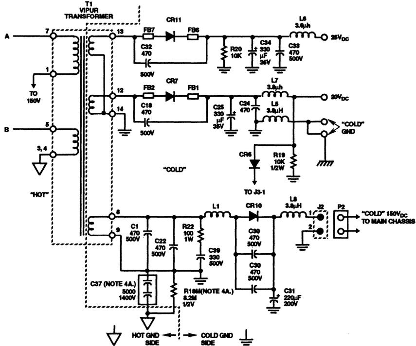
FIGURE 14. APPLICATION OF THE CA1523 VIPUR IN RCA CTC-130 TELEVISION CHASSIS POWER SUPPLY MODULE
