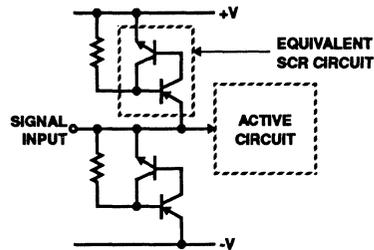
FIGURE 4. PROTECTION CELLS OF THE SP720 SCR ARRAY
