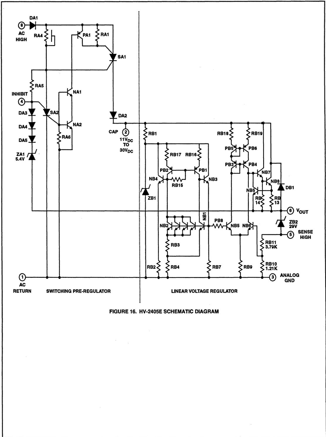
FIGURE 16. HV-2405E SCHEMATIC DIAGRAM
