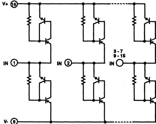
**FIGURE 6. EQUIVALENT CIRCUIT DIAGRAM OF THE SP720**
