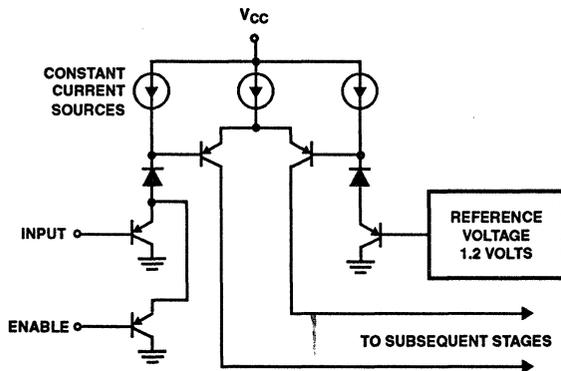
FIGURE 2. CA3262A EQUIVALENT SCHEMATIC OF ONE INPUT STAGE
