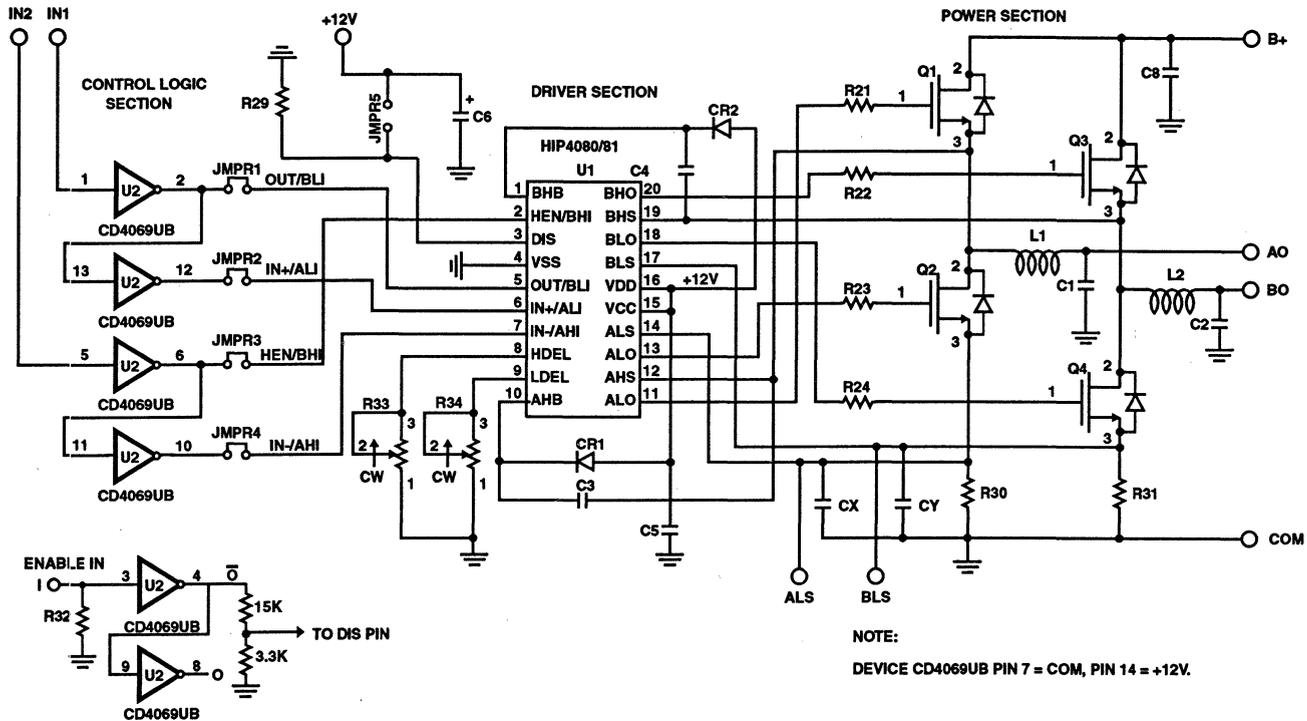
FIGURE 31. HIP4081 EVALUATION BOARD SCHEMATIC
