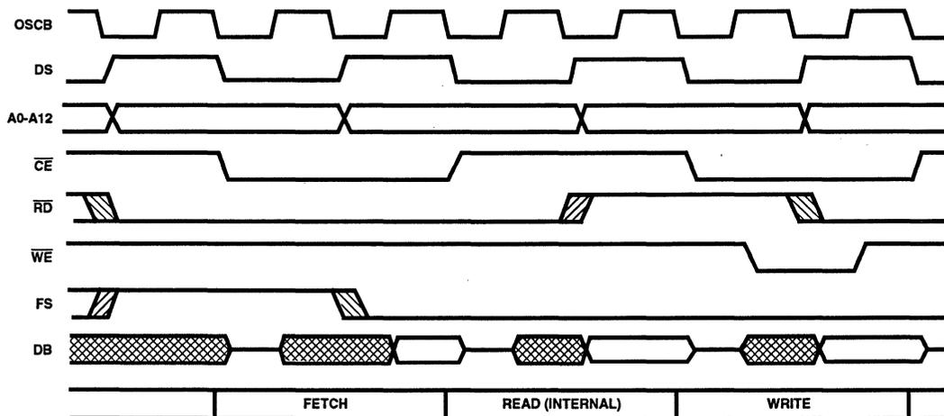
FIGURE 5. SIGNAL TIMING DIAGRAM (ALC = 1)
