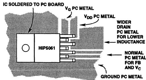
FIGURE 37. SHOWING WIDER PC BOARD METAL FOR CRITICAL
