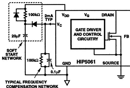
FIGURE 4. SOFT START CIRCUIT FOR THE HIP5061
