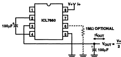
FIGURE 20. EFFICIENT SUPPLY SPLITTING
