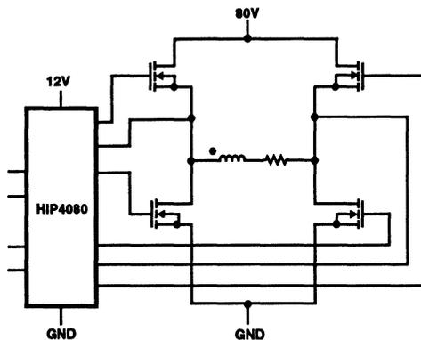
FIGURE 1. HIP4080 SIMPLIFIED APPLICATION DIAGRAM
