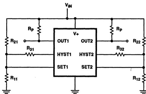
FIGURE 11. AN ALTERNATIVE HYSTERESIS CIRCUIT
