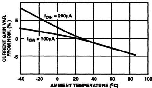
FIGURE 5B. CURRENT MULTIPLIER CURRENT GAIN vs TEMPERATURE CHARACTERISTIC
