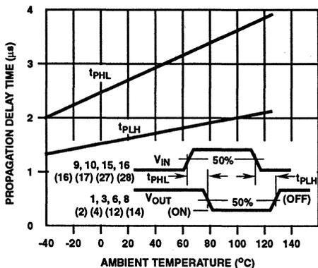
FIGURE 5C. TYPICAL PROPAGATION DELAY TIME CHARACTERISTICS
