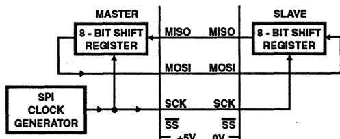
**FIGURE 23. SERIAL PERIPHERAL INTERFACE (SPI) MASTER-SLAVE INTERCONNECTION**
