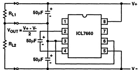
FIGURE 21. SPLITTING A SUPPLY IN HALF
