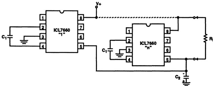
FIGURE 13. PARALLELING DEVICES
