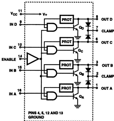
**FIGURE 1. CA3242 FUNCTIONAL BLOCK DIAGRAM**
