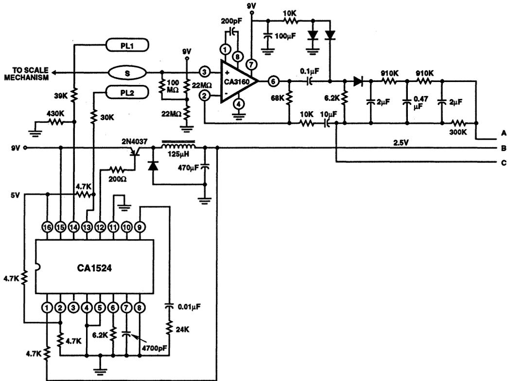
FIGURE 26. SCHEMATIC DIAGRAM OF DIGITAL READOUT SCALE
