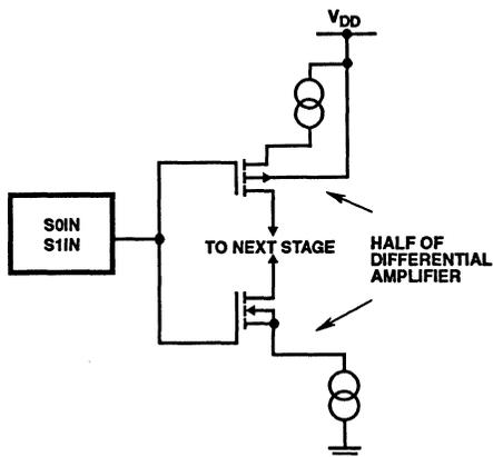
FIGURE 4A. S0IN AND S1IN INPUT CIRCUIT
