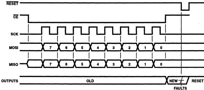
FIGURE 2. BYTE TIMING DIAGRAM WITH ASYNCHRONOUS RESET
