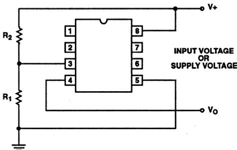
FIGURE 26. COMBINED INPUT AND SUPPLY VOLTAGES
