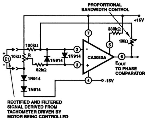
FIGURE 27A. VOLTAGE COMPARATOR
