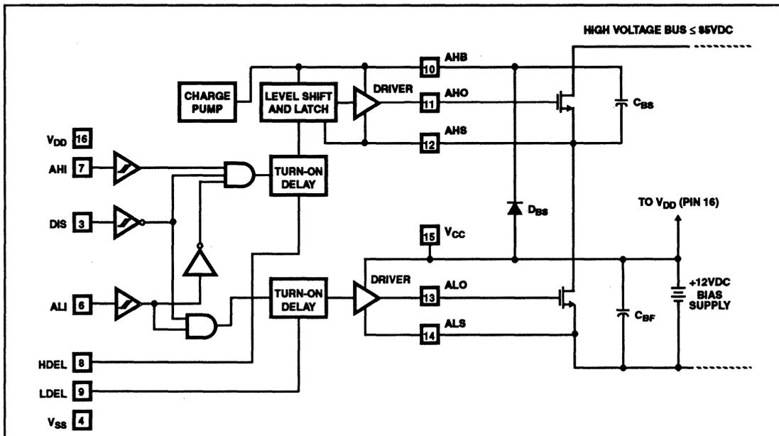
FIGURE 3. HIP4081 FUNCTIONAL BLOCK DIAGRAM
