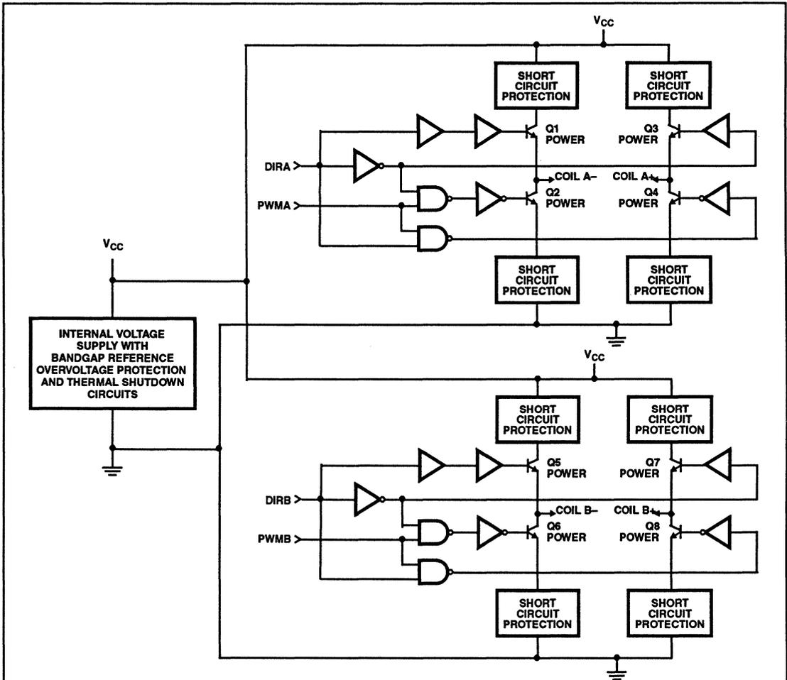
FIGURE 1. CA3275 DUAL FULL BRIDGE DRIVER SCHEMATIC
