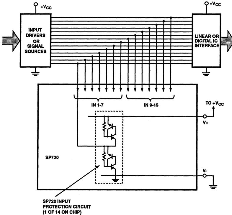
FIGURE 4. TYPICAL APPLICATION OF THE SP720 AS AN INPUT CLAMP FOR OVER-VOLTAGE, GREATER THAN  $1V_{BE}$  ABOVE  $V+$  OR LESS THAN  $-1V_{BE}$  BELOW  $V-$
