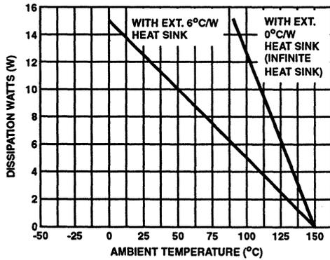
FIGURE 1. DISSIPATION DERATING CURVES
