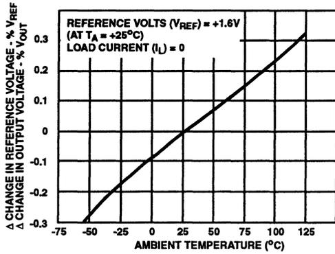
FIGURE 14. TEMPERATURE COEFFICIENT OF  $V_{REF}$  AND  $V_{OUT}$
