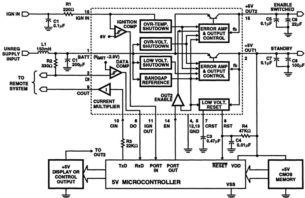
FIGURE 1. TYPICAL APPLICATION OF THE CA3277 USING THE SERIAL DATA BUFFERS
