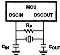
FIGURE 4A. CRYSTAL/RESONATOR CIRCUIT CONNECTIONS
