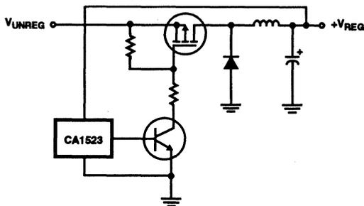
FIGURE 2C. BUCK CONVERTER REGULATOR
