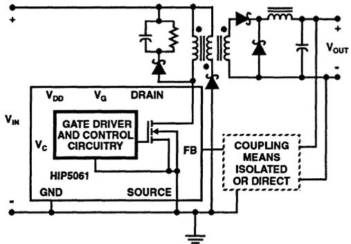
FIGURE 41. FORWARD CONVERTER
