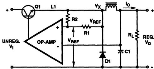
FIGURE 17A. SELF-OSCILLATING SWITCHING REGULATOR
