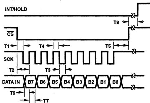
FIGURE 6. SPI TIMING
