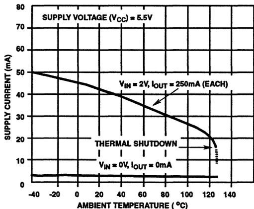
FIGURE 4A. TYPICAL SUPPLY CURRENT (PIN 11) CHARACTERISTICS
