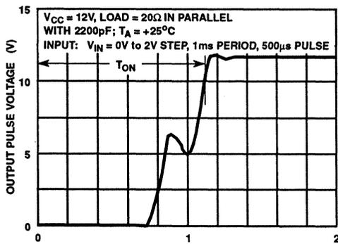
FIGURE 3A. OUTPUT TURN-ON TIME ( $\mu s$ )
