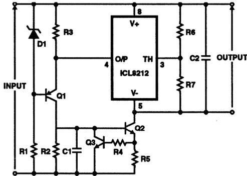
FIGURE 10. CURRENT LIMITED NEGATIVE REGULATOR - NPN + PNP BOOST
