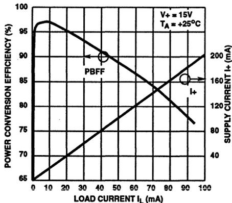
FIGURE 11. SUPPLY CURRENT AND POWER CONVERSION EFFICIENCY AS A FUNCTION OF LOAD CURRENT
