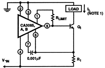
$Q_1$ : Any N-P-N Silicon Transistor that can handle a 2A Load Current such as 2N3772 or Equivalent
