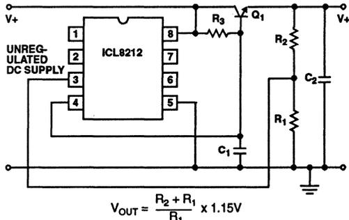
FIGURE 34. PRECISION VOLTAGE REGULATOR
