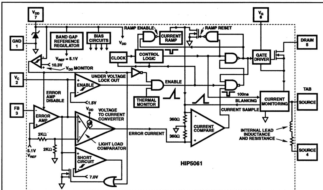
FIGURE 2. FUNCTIONAL BLOCK DIAGRAM OF THE HIP5061
