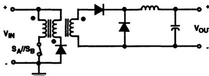
**FORWARD CONVERTER WITH DIODE CLAMP**
