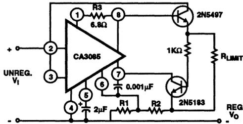
FIGURE 6B. WITH AUXILIARY SHORT-CIRCUIT PROTECTION
