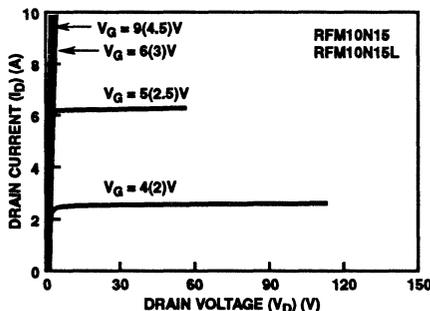
FIGURE 1. DRAIN CURRENT vs. DRAIN VOLTAGE CURVES FOR REPRESENTATIVE STANDARD AND L<sup>2</sup>FET DEVICES
