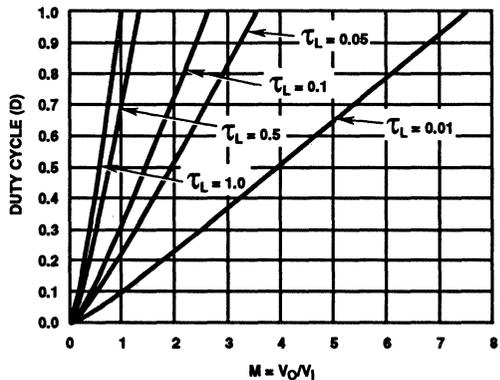
FIGURE 12. SEPIC CONVERTER IN THE DCM MODE FOR A FAMILY OF LOAD PARAMETERS,  $\tau$ , WITH THE VOLTAGE TRANSFER RATIO,  $M < 8$
