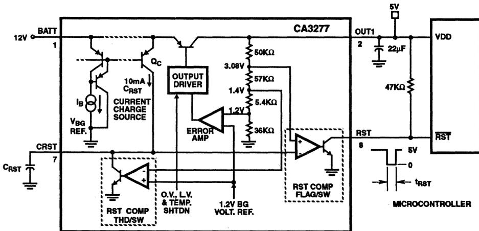
FIGURE 3. LOW VOLTAGE RESET CIRCUITRY
