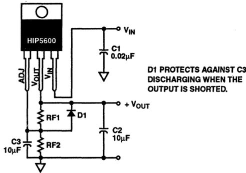
FIGURE 5. REGULATOR WITH PROTECTION DIODE
