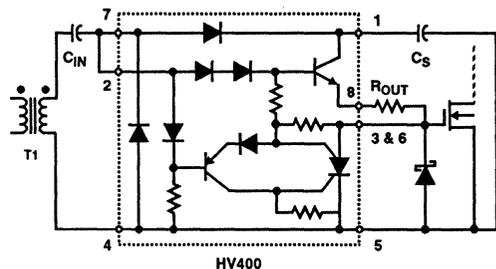
FIGURE 2. BIPOLAR DRIVE WITH DC BLOCKING CAPACITOR
