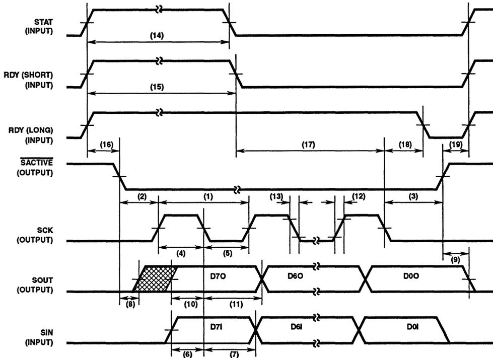
FIGURE 1. SERIAL INTERFACE TIMING DIAGRAM
