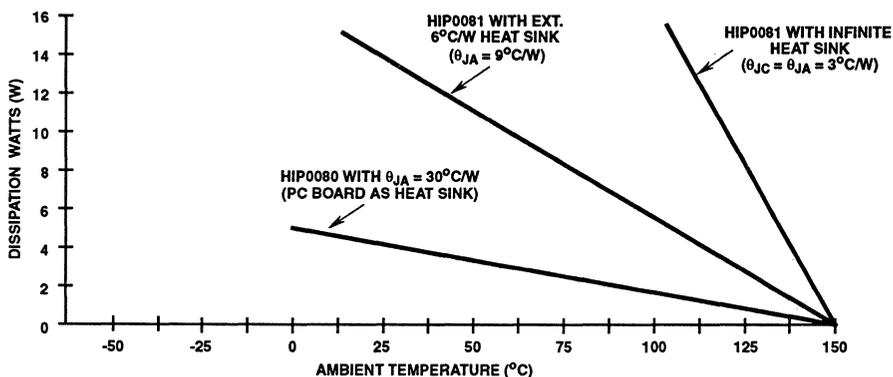
FIGURE 6. DISSIPATION DERATING CURVES
