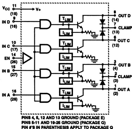
FIGURE 3. CA3262 AND CA3262A FUNCTIONAL BLOCK DIAGRAM
