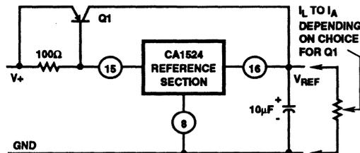
FIGURE 3. CIRCUIT FOR EXPANDING THE REFERENCE CURRENT CAPABILITY
