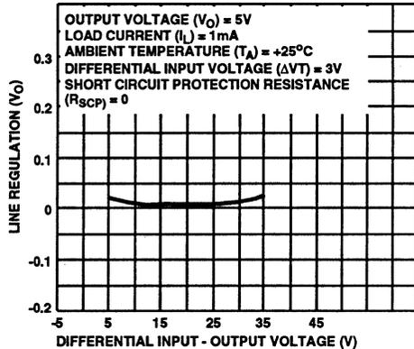
FIGURE 15. LINE REGULATION vs DIFFERENTIAL INPUT-OUTPUT VOLTAGE
