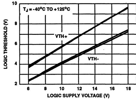
FIGURE 8. INPUT LOGIC THRESHOLD vs SUPPLY VOLTS
