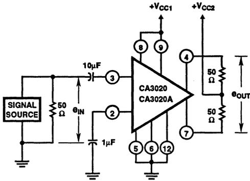
FIGURE 8. MEASUREMENT OF BANDWIDTH AT -3dB POINTS
