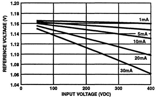
FIGURE 34. REFERENCE VOLTAGE vs  $V_{IN}$ ; CASE TEMPERATURE OF +25°C
