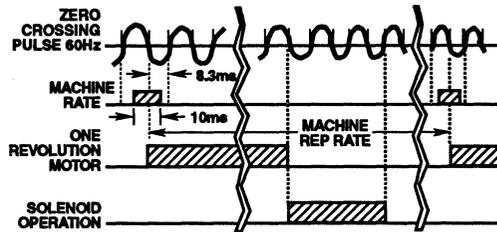
FIGURE 44. TIMING DIAGRAM FOR SOLID-STATE MACHINE CONTROL
