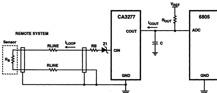
FIGURE 8. ANALOG SIGNAL TRANSMISSION USING THE CA3277 CURRENT MULTIPLIER
