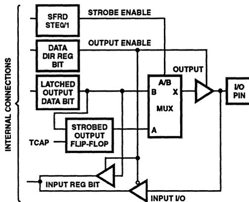
**FIGURE 6. STROBED OUTPUT BLOCK DIAGRAM (PD0, PD1)**
