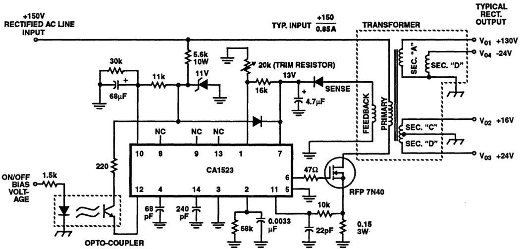
FIGURE 2. TYPICAL APPLICATION CIRCUIT FOR THE CA1523
