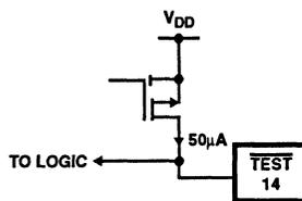
FIGURE 4C.  $\overline{\text{TEST}}$  PMOS TRANSISTOR HAS EQUIVALENT CURRENT PULLUP CAPABILITY OF A 50k TO 200k RESISTOR
