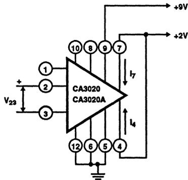
FIGURE 3A. TEST SETUP
