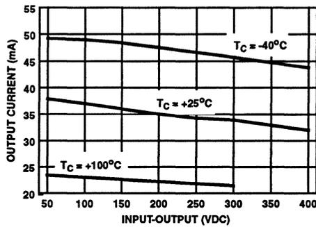
FIGURE 39. CURRENT LIMIT vs TEMPERATURE
