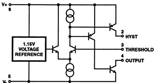
FIGURE 2. ICL8212 FUNCTIONAL DIAGRAM
