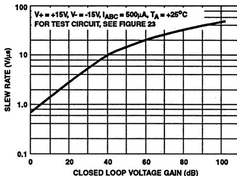
FIGURE 14. SLEW RATE vs CLOSED LOOP VOLTAGE GAIN
