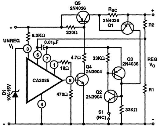
FIGURE 16. HIGH-VOLTAGE REGULATOR INCORPORATING CURRENT "SNAP-BACK" PROTECTION
