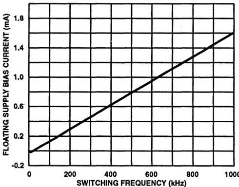
FIGURE 8.  $I_{AHB}$ ,  $I_{BHB}$  NO-LOAD FLOATING SUPPLY CURRENT vs FREQUENCY
