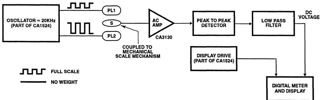
FIGURE 39. BLOCK DIAGRAM - DIGITAL READOUT SCALE CIRCUIT
