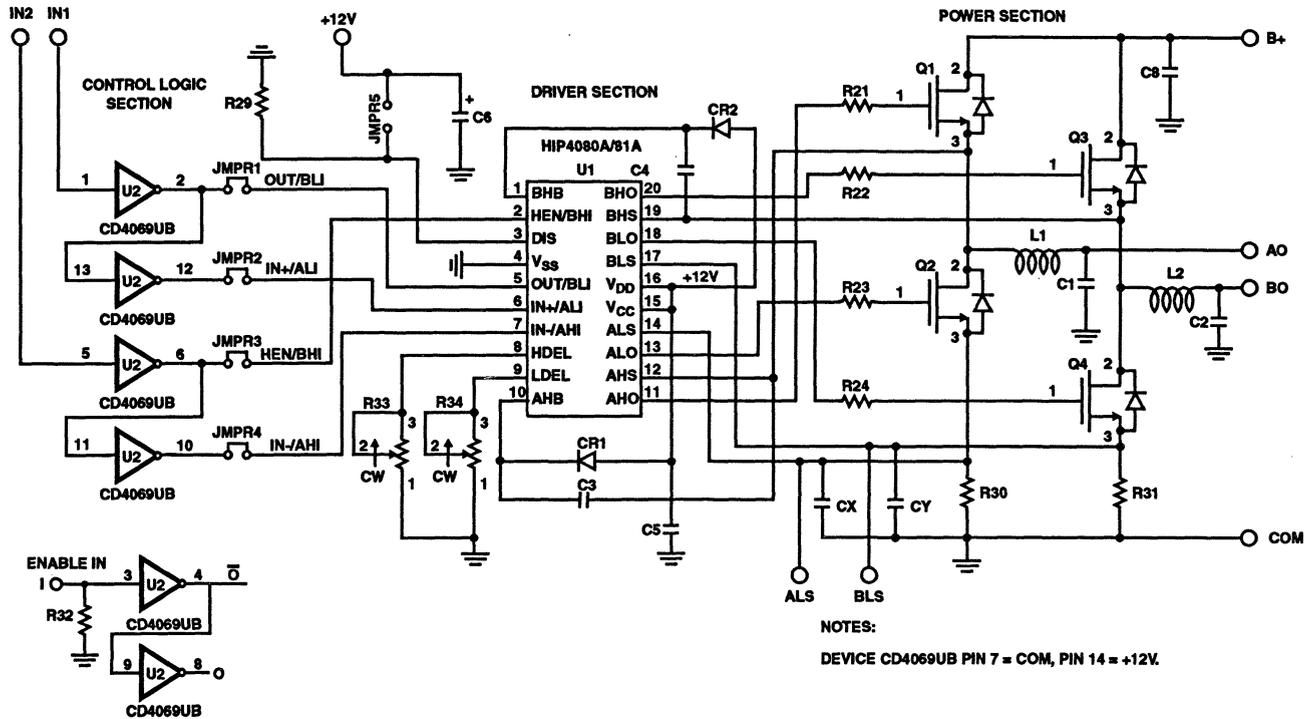
FIGURE 13. HIP4081A EVALUATION PC BOARD SCHEMATIC
