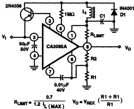
FIGURE 18. TYPICAL SWITCHING REGULATOR CIRCUIT
