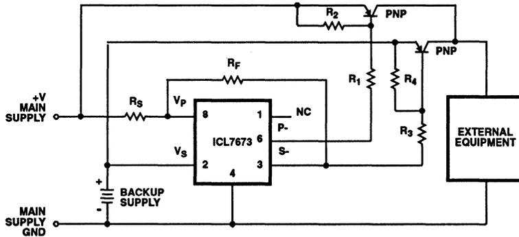
FIGURE 13. HIGH CURRENT BACKUP SYSTEM WITH HYSTERESIS
