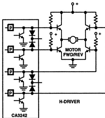
FIGURE 3. TYPICAL APPLICATIONS FOR THE CA3242 QUAD
