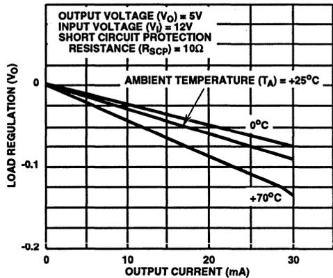
FIGURE 11. LOAD REGULATION WITH CURRENT LIMITING
