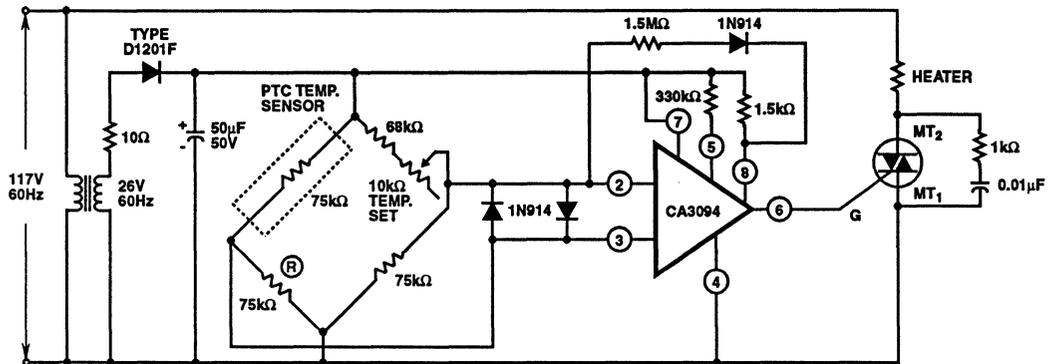
FOR NTC SENSOR, INTERCHANGE POSITION OF SENSOR AND (R).
