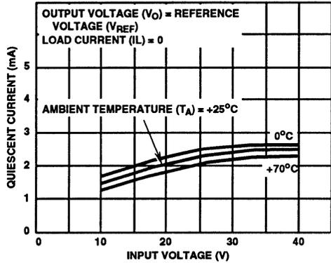
FIGURE 13. QUIESCENT CURRENT vs INPUT VOLTAGE
