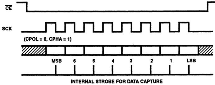
FIGURE 1A. DATA AND CLOCK TIMING DIAGRAM
