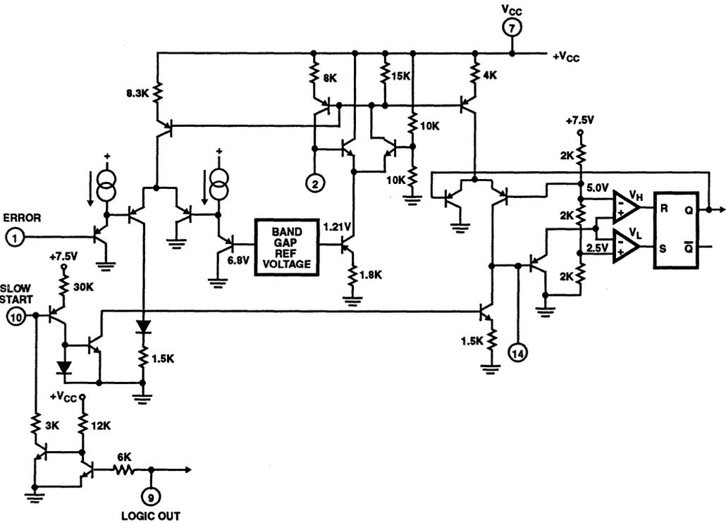
FIGURE 3. TIMING CIRCUIT FOR THE CA1523
