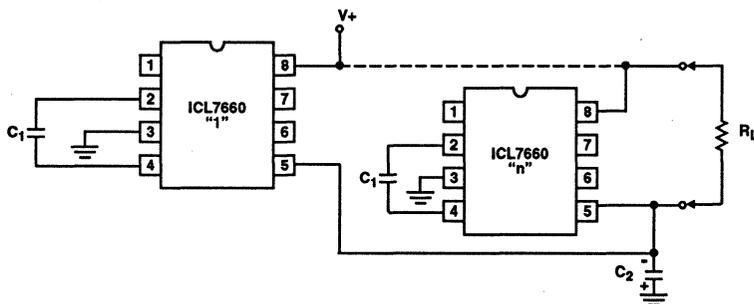
FIGURE 15. PARALLELING DEVICES
