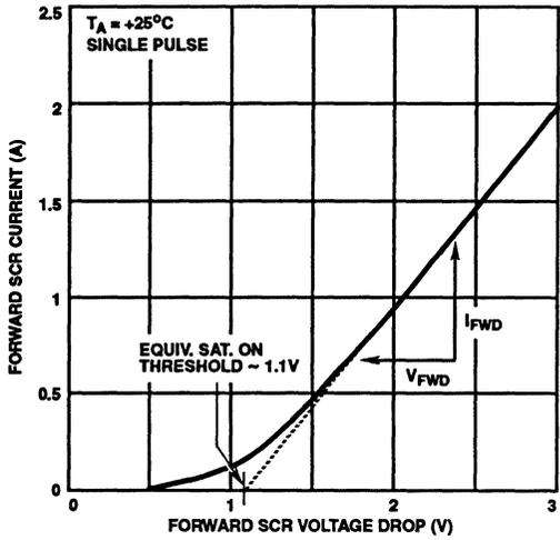
FIGURE 3. HIGH CURRENT SCR FORWARD VOLTAGE DROP CURVE
