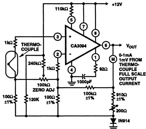
**FIGURE 4. SINGLE SUPPLY AMPLIFIER FOR THERMOCOUPLE SIGNALS**
