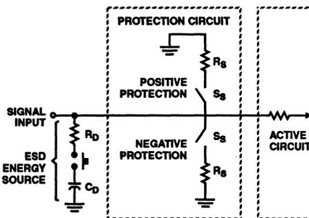
FIGURE 3. ESD AND TRANSIENT PROTECTION CIRCUIT
