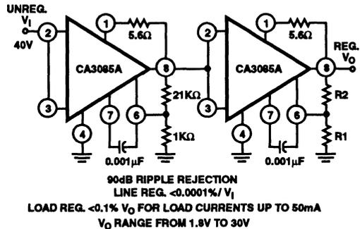
FIGURE 21A. VOLTAGE REGULATOR WITH HIGH RIPPLE REJECTION
