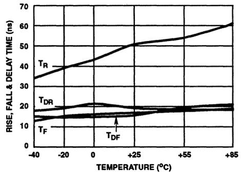
FIGURE 12. RISE, FALL AND DELAY TIMES vs TEMPERATURE
