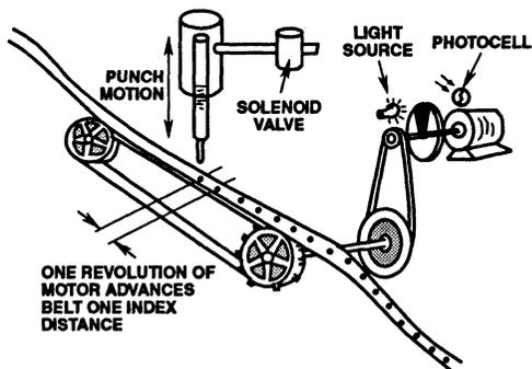
**FIGURE 42. STEP-AND-PUNCH MACHINE**
