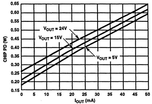
FIGURE 22. CHIP POWER DISSIPATION vs OUTPUT CURRENT
