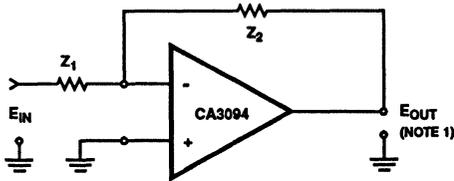
Where  $\frac{E_{OUT}}{E_{IN}} = f\left(\frac{Z_2}{Z_1}\right)$  depends on the characteristics of Z1 and Z2
