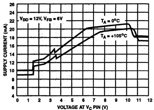
FIGURE 6. TYPICAL SUPPLY CURRENT vs VOLTAGE AT PIN  $V_C$  FOR  $0^\circ C$  AND  $+105^\circ C$
