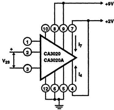
FIGURE 2A. TEST SETUP
