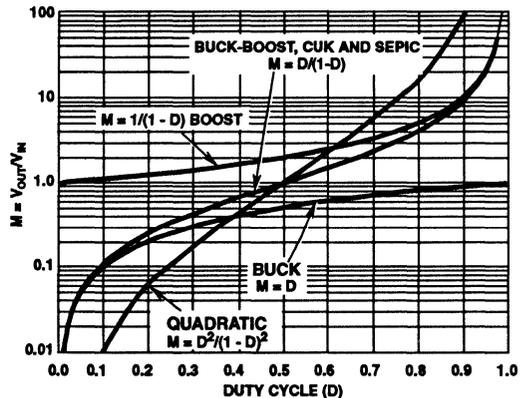
FIGURE 12. VOLTAGE TRANSFER AS A FUNCTION OF DUTY CYCLE FOR VARIOUS TOPOLOGIES
