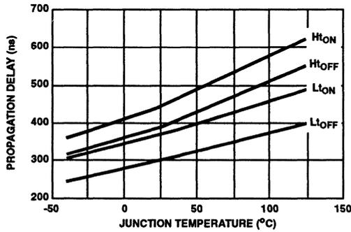
FIGURE 15. PROPAGATION DELAYS AT  $V_{CC} = 15V$
