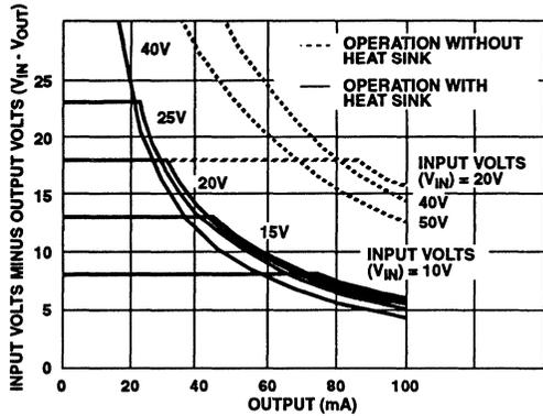
FIGURE 15. DISSIPATION LIMITATION ( $V_{IN} - V_{OUT}$  vs  $I_{OUT}$ )
