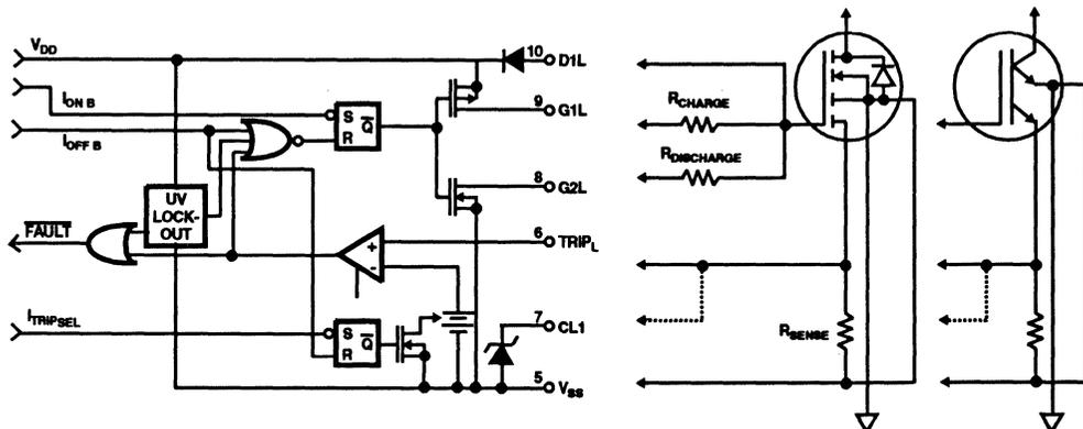
FIGURE 3. POWER-OUTPUT SECTION INTERFACING WITH CURRENT SENSING MOSFET OF IGT.
