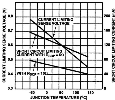
FIGURE 17. CURRENT LIMITING CHARACTERISTIC vs JUNCTION TEMPERATURE
