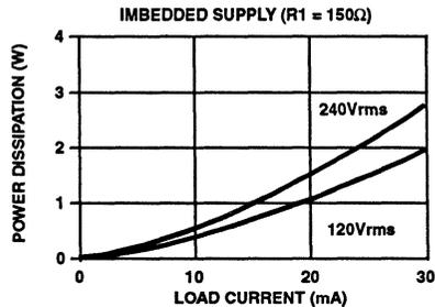
**FIGURE 11. POWER DISSIPATION IN R1 vs LOAD CURRENT**
