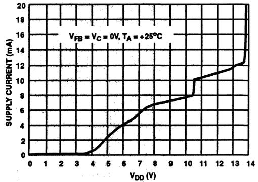
FIGURE 4. TYPICAL SUPPLY CURRENT vs SUPPLY VOLTAGE
