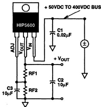
FIGURE 12. DC/DC CONVERTER
