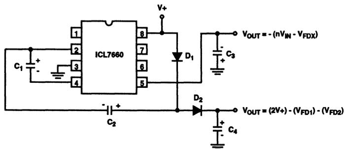
FIGURE 19. COMBINED NEGATIVE CONVERTER AND POSITIVE MULTIPLIER
