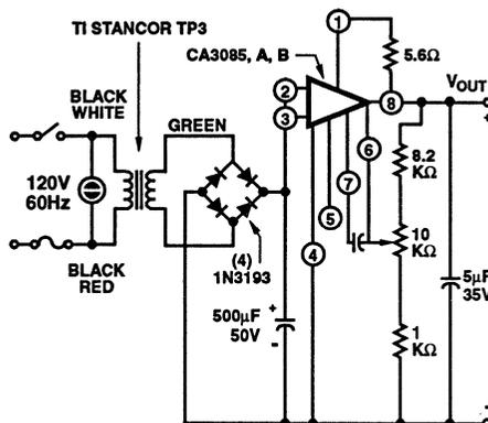
$V_{OUT} = 3.5\text{V to } 20\text{V}$  (0 to 90mA)
