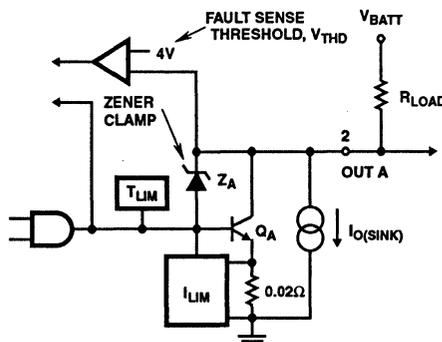
FIGURE 3. OUTPUT OPEN LOAD DETECTION WHERE  $I_{O(SINK)}$  IS AN ACTIVE CURRENT SINK PULLDOWN FOR OPEN-LOAD FAULT DETECTION. THE CURRENT  $I_{CEX}$  IS  $I_{O(SINK)}$  PLUS LEAKAGE CURRENTS OF THE OUTPUT DRIVER
