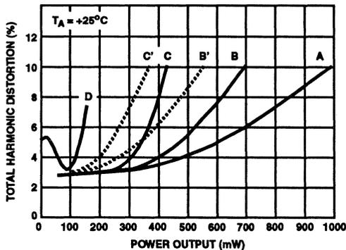
**FIGURE 6. TOTAL HARMONIC DISTORTION OF THE CA3020 OR CA3020A AS A FUNCTION OF POWER OUTPUT**
