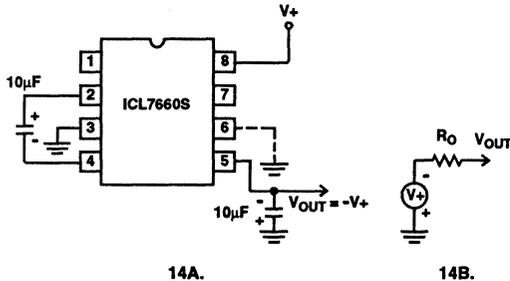
**FIGURE 14. SIMPLE NEGATIVE CONVERTER AND ITS OUTPUT EQUIVALENT**
