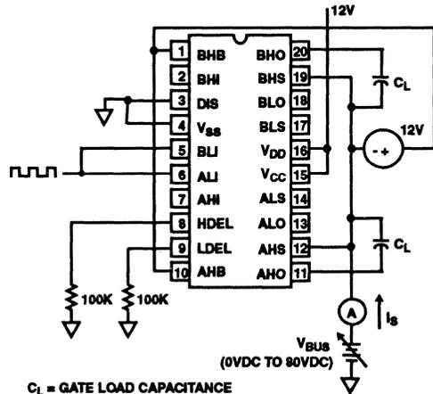
FIGURE 10. HIGH VOLTAGE LEVEL-SHIFT CURRENT TEST CIRCUIT
