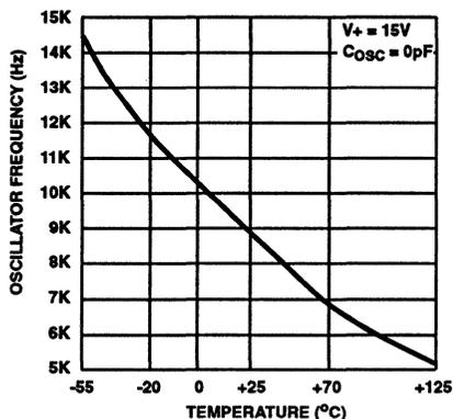
FIGURE 7. UNLOADED OSCILLATOR FREQUENCY AS A FUNCTION OF TEMPERATURE
