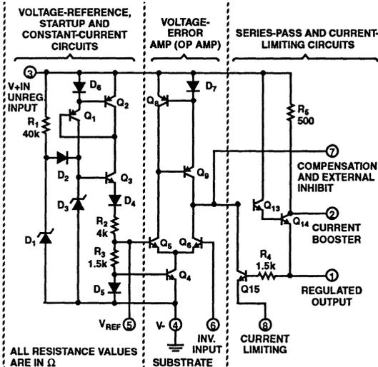
FIGURE 2. SCHEMATIC DIAGRAM OF CA3085 SERIES
