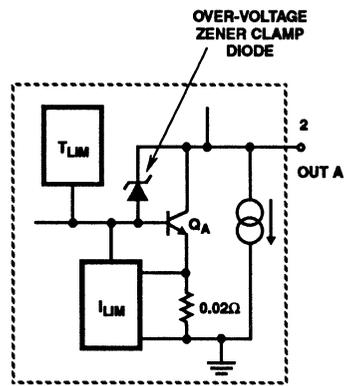
**FIGURE 6B. CA3292A OUTPUT STAGE WITH CLAMP DIODE**
