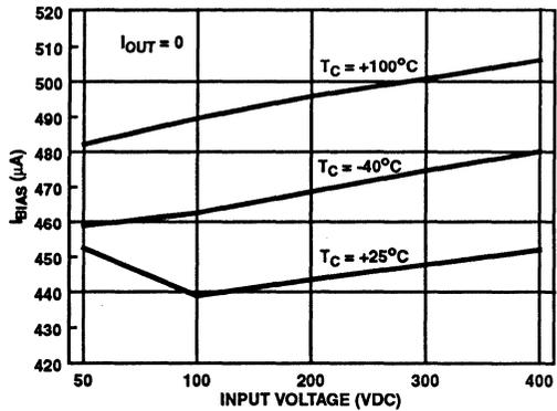
FIGURE 28.  $I_{BIAS}$  vs INPUT VOLTAGE
