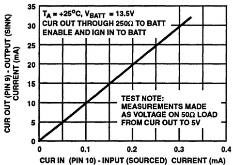
FIGURE 4D. TYPICAL CURRENT MULTIPLIER CURRENT GAIN CHARACTERISTIC
