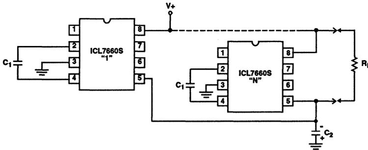
FIGURE 16. PARALLELING DEVICES
