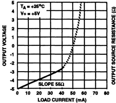
FIGURE 7. OUTPUT CHARACTERISTICS
