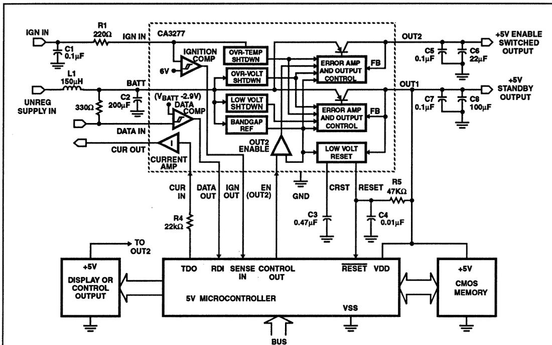
NOTE: DATA IN and CUR OUT are remote/host Serial Data Communication Buffers. Typical Remote Source Impedance for DATA IN is 1k $\Omega$ . Typical Remote Load for CUR OUT is 250 $\Omega$ .
