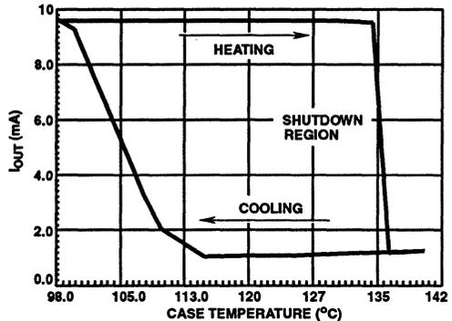
FIGURE 9. THERMAL HYSTERESIS CURVE
