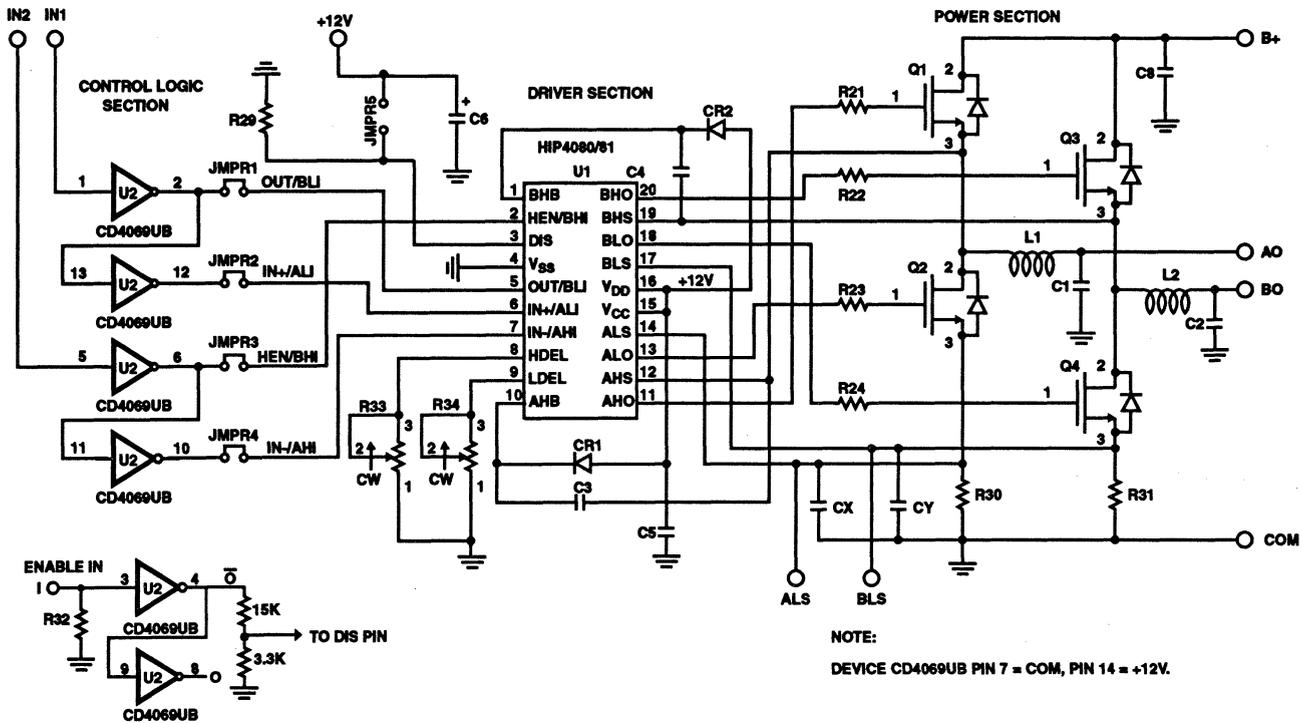
FIGURE 12. HIP4081 EVALUATION PC BOARD SCHEMATIC
