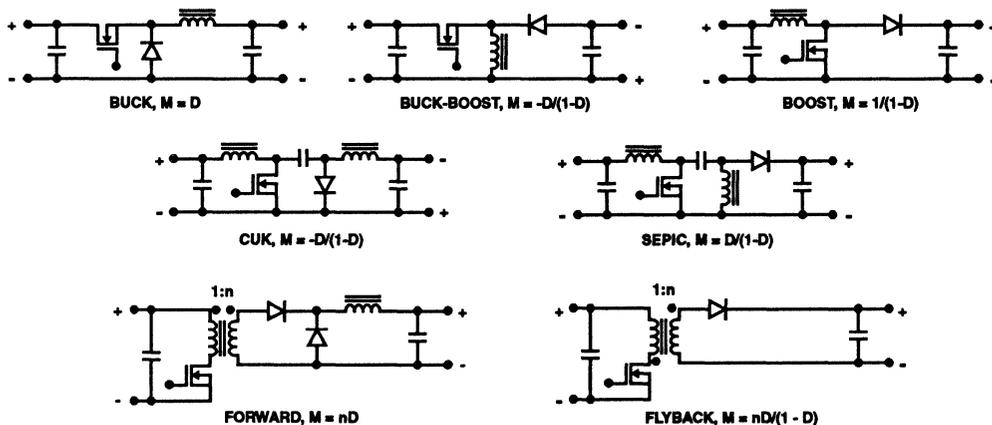
FIGURE 1. CONVERTER CIRCUITS,  $M = V_O/V_I$
