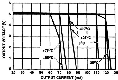
FIGURE 23. OUTPUT CURRENT LIMIT (5V<sub>OUT</sub>) 50Hz
