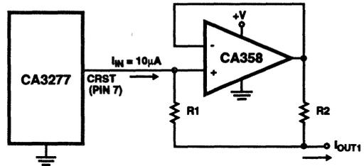
FIGURE 4. CURRENT-TO-CURRENT MULTIPLIER
