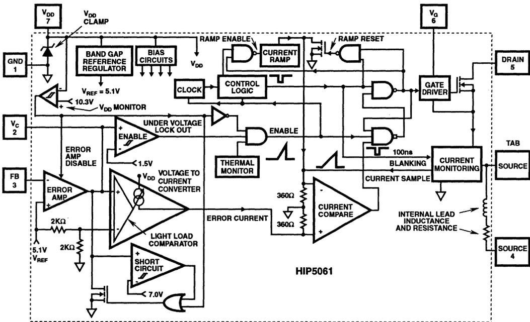
FIGURE 2. FUNCTIONAL BLOCK DIAGRAM OF THE HIP5061
