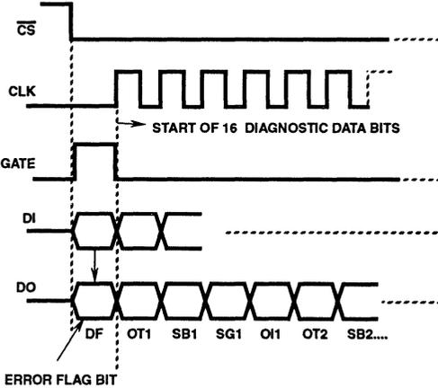
FIGURE 2. DATA AND CLOCK TIMING
