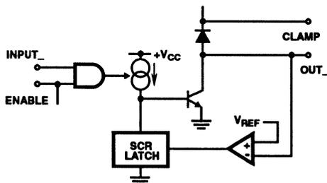
FIGURE 2. CA3242 FUNCTIONAL DIAGRAM FOR EACH OUTPUT CHANNEL SHOWN WITH PROTECTION CIRCUIT
