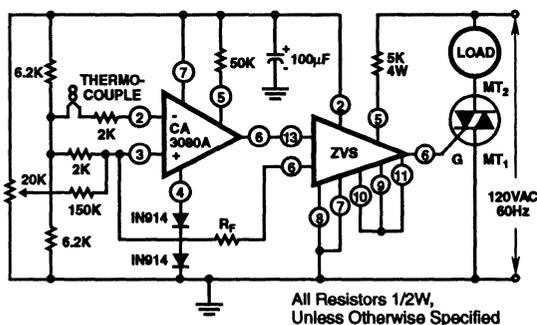
**FIGURE 40. THERMOCOUPLE TEMPERATURE CONTROL WITH ZERO-VOLTAGE SWITCHING**
