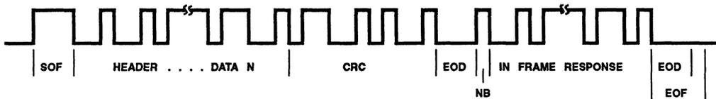
FIGURE 26. J1850 MESSAGE WITH IN-FRAME-RESPONSE
