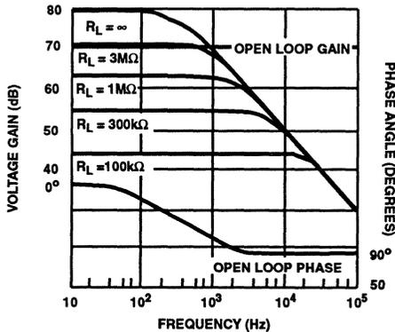
FIGURE 6. OPEN-LOOP ERROR AMPLIFIER RESPONSE CHARACTERISTICS.
