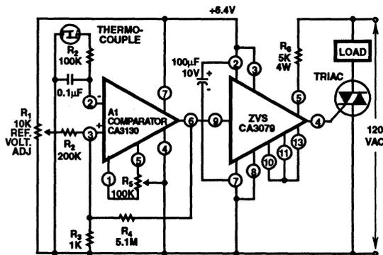
$$\text{Hysteresis} = R_3/R_4 \times 6.4V = 1K/5.1M \times 6.4V = 1.25mV$$
