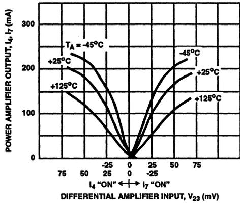
FIGURE 2B. CHARACTERISTICS WITH  $R_{10}$  SHORTED OUT
