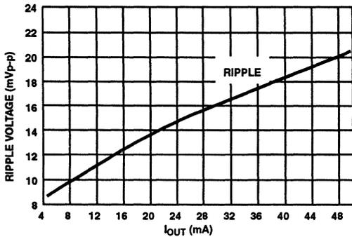
FIGURE 21. OUTPUT RIPPLE VOLTAGE vs LOAD CURRENT
