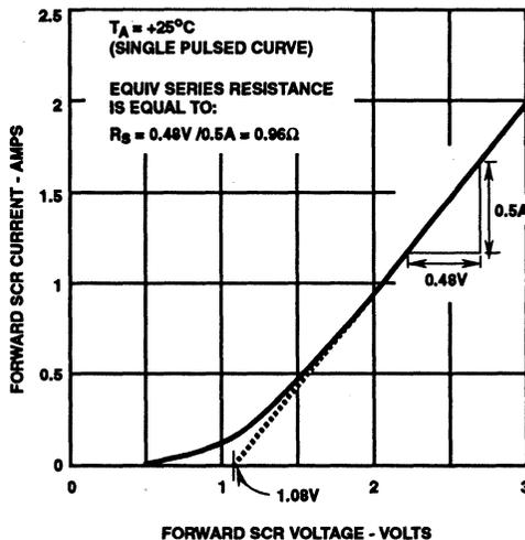
**FIGURE 7. SCR FORWARD CURRENT vs VOLTAGE CHARACTERISTICS**
