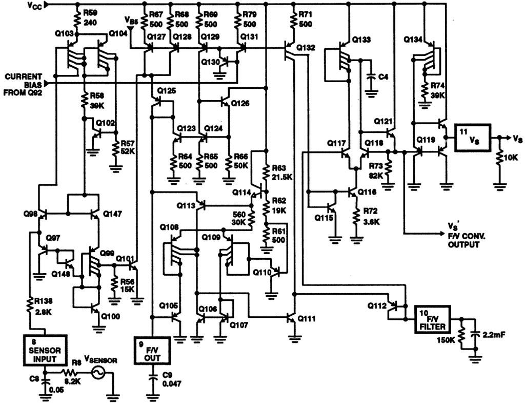
FIGURE 5. FREQUENCY TO VOLTAGE (F/V) CONVERTER CIRCUIT
