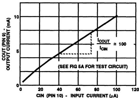
FIGURE 5C. CURRENT GAIN CHARACTERISTIC OF THE CA3277 CURRENT MULTIPLIER
