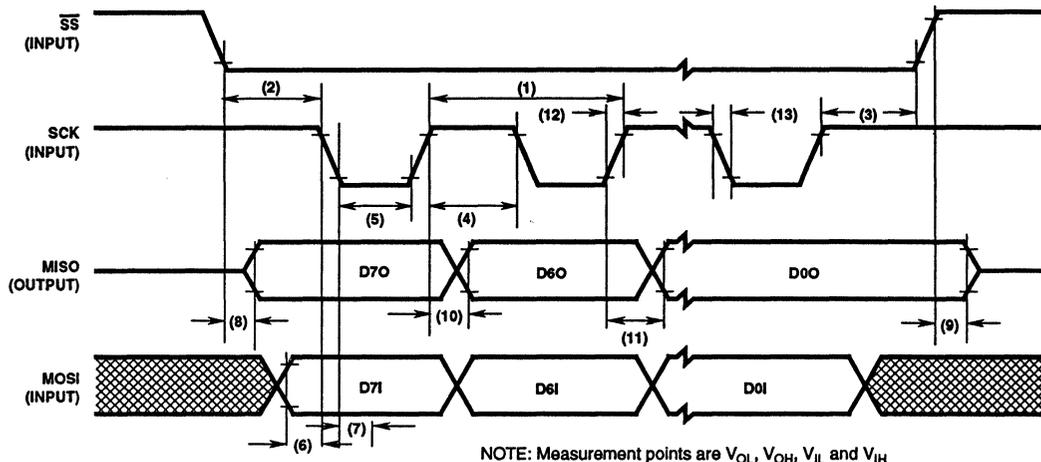
FIGURE 3H. SPI SLAVE TIMING CPOL = 1, CPHA = 0
