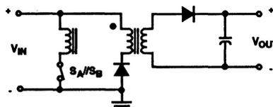
**FLYBACK CONVERTER WITH CLAMP WINDING**
