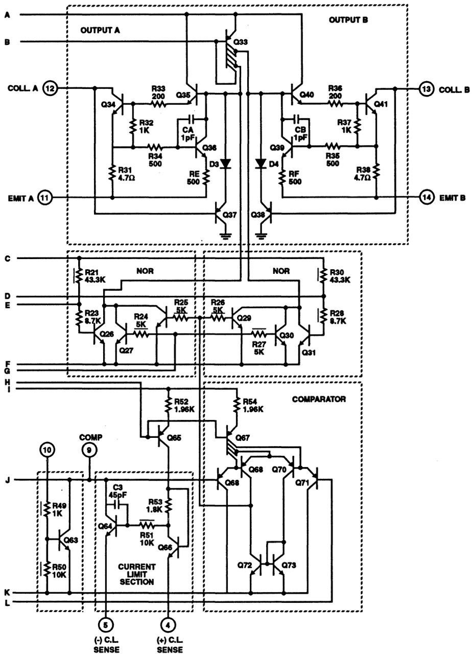
FIGURE 4. SCHEMATIC DIAGRAM OF CA1524 SERIES IC (Continued)
