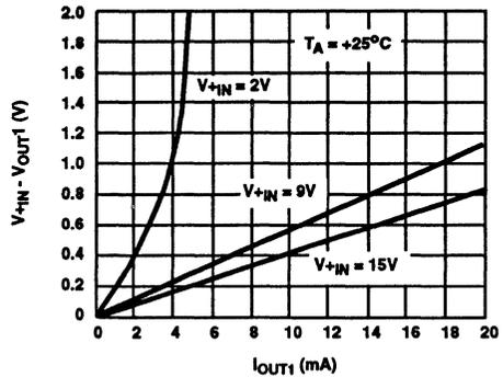
FIGURE 2.  $V_{OUT1}$  INPUT-OUTPUT DIFFERENTIAL vs OUTPUT CURRENT
