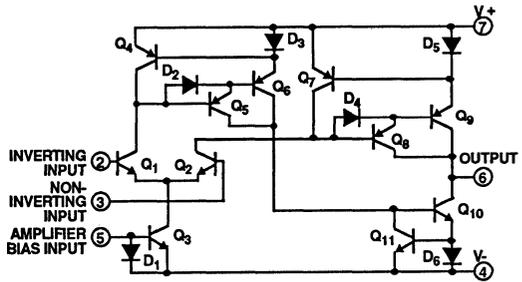
FIGURE 23. SCHEMATIC DIAGRAM OF THE CA3080
