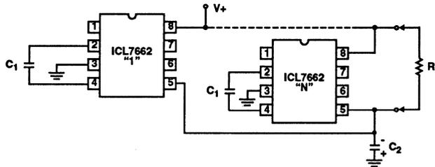
FIGURE 18. PARALLELING DEVICES
