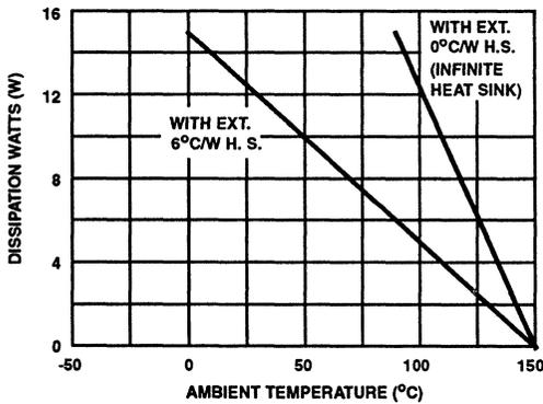
FIGURE 1. DISSIPATION DERATING CURVES
