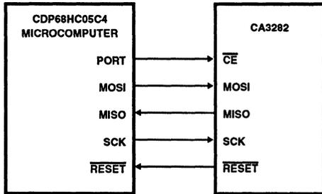
**FIGURE 3. TYPICAL MICROCOMPUTER INTERFACE WITH THE CA3282**
