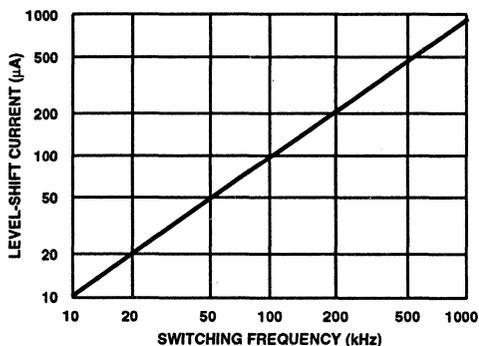
FIGURE 30. HIGH VOLTAGE LEVEL-SHIFT CURRENT vs FREQUENCY AND BUS VOLTAGE
