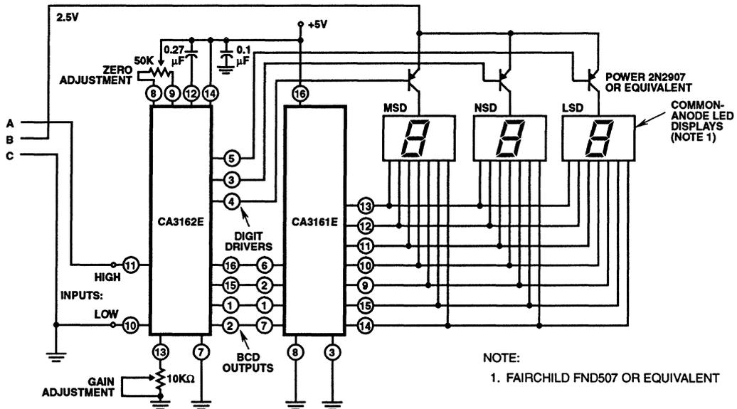
FIGURE 25. SCHEMATIC DIAGRAM OF DIGITAL READOUT SCALE (CONT'D)
