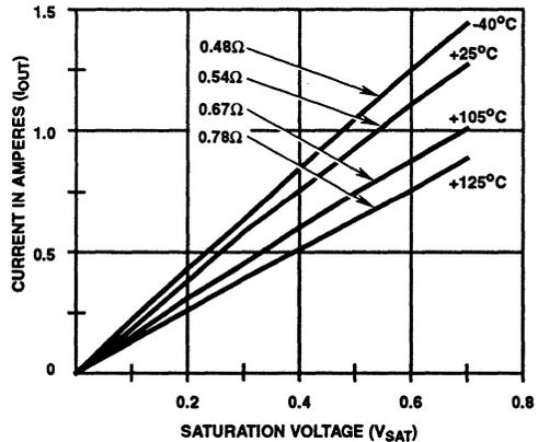
**FIGURE 4A. CA3282 TYPICAL OUTPUT DRIVER  $R_{DS(ON)}$  CHARACTERISTICS OF CURRENT OUT vs SATURATION VOLTAGE,  $V_{SAT}$  FOR A  $-40^{\circ}\text{C}$  TO  $+125^{\circ}\text{C}$  JUNCTION TEMPERATURE**
