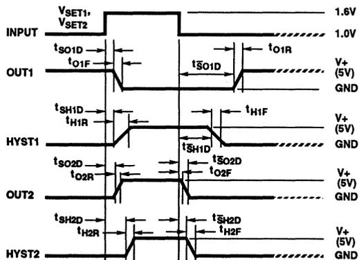
FIGURE 8. SWITCHING WAVEFORMS
