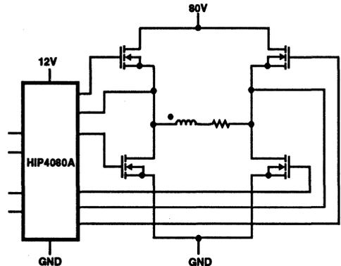
FIGURE 1. HIP4080A SIMPLIFIED APPLICATION DIAGRAM
