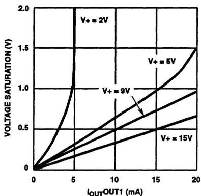
FIGURE 1. OUT1 SATURATION VOLTAGE AS A FUNCTION OF OUTPUT CURRENT
