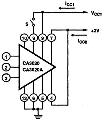
FIGURE 5A. TEST SETUP
