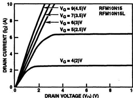
FIGURE 2. DRAIN CURRENT vs. LOW DRAIN VOLTAGE CURVES FOR REPRESENTATIVE STANDARD AND L<sup>2</sup>FET DEVICES DEMONSTRATING THAT R<sub>ON</sub> HAS NOT BEEN SACRIFICED IN THE L<sup>2</sup>FET
