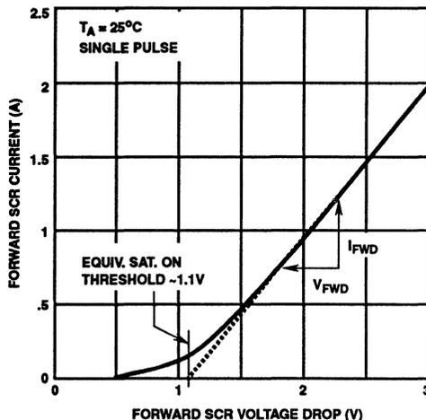
FIGURE 3. HIGH CURRENT SCR FORWARD VOLTAGE DROP CURVE
