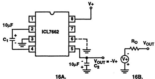
FIGURE 16. SIMPLE NEGATIVE CONVERTER AND ITS OUTPUT EQUIVALENT
