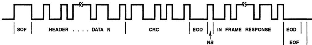
FIGURE 5. J1850 MESSAGE WITH IN-FRAME-RESPONSE
