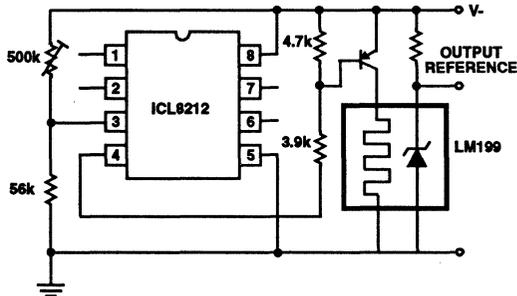
FIGURE 38. LOW VOLTAGE POWER SUPPLY DISCONNECT
