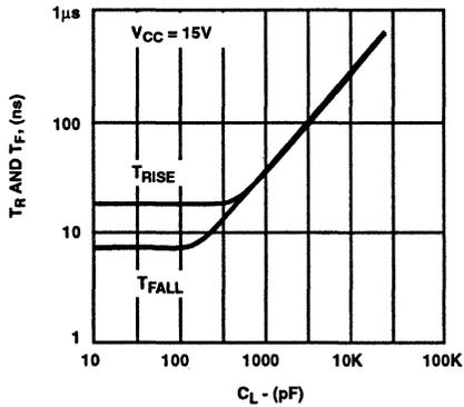
FIGURE 1. RISE AND FALL TIMES vs  $C_L$
