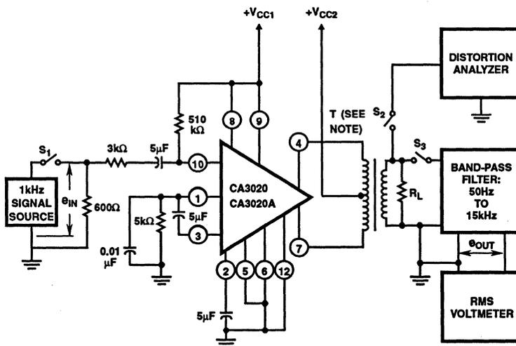
NOTE: Push-pull output transformer; load resistance ( $R_L$ ) should be selected to provide indicated collector-to-collector load impedance ( $R_{CC}$ ).
