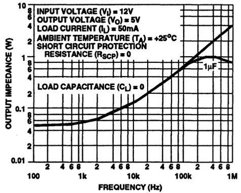
FIGURE 19. OUTPUT IMPEDANCE vs FREQUENCY
