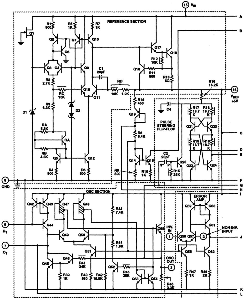
FIGURE 4. SCHEMATIC DIAGRAM OF CA1524 SERIES IC
