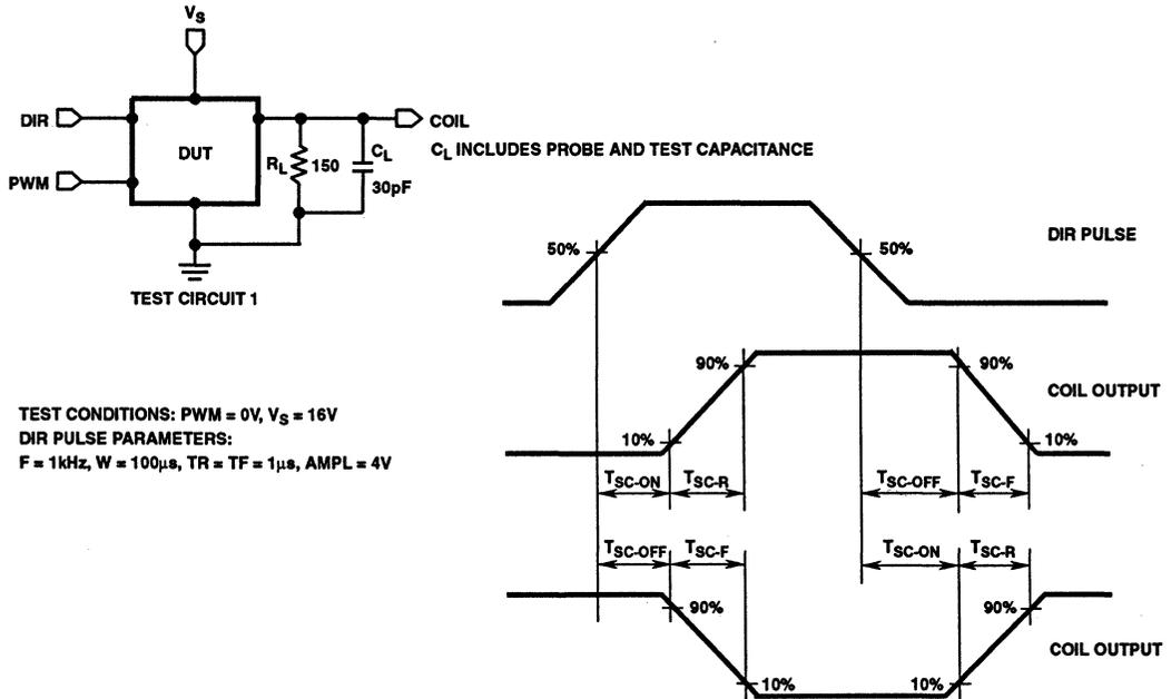
FIGURE 3. SOURCE SWITCHING TEST CIRCUIT AND VOLTAGE WAVEFORMS
