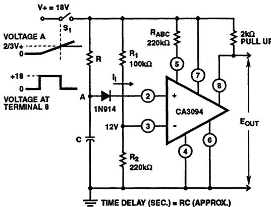
Problem: To calculate the maximum value of R required to switch a 100mA output current comparator
