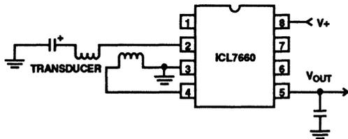
FIGURE 24. TRANSDUCER DRIVER AND DETECTOR
