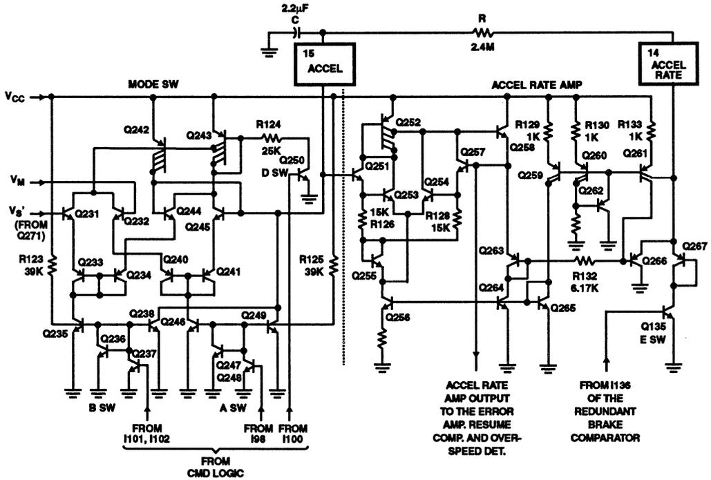
FIGURE 13. MODE SWITCH AND ACCELERATION-RATE AMPLIFIER CIRCUIT
