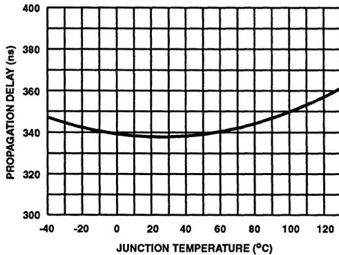
FIGURE 14. DISABLE TO UPPER ENABLE  $T_{UEN}$  PROPAGATION DELAY vs TEMPERATURE
