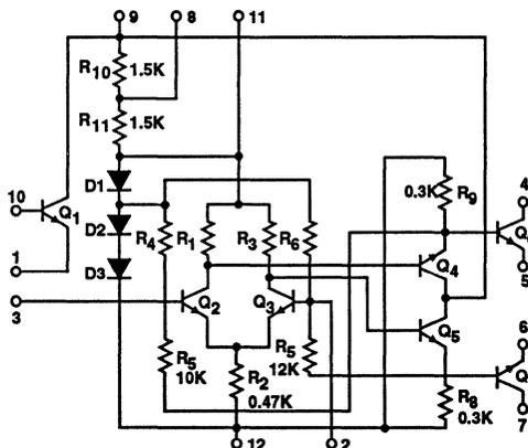
The resistance values included on the schematic diagram have been supplied as a convenience to assist Equipment Manufacturers in optimizing the selection of "outboard" components of equipment designs. The values shown may vary as much as 30%.
