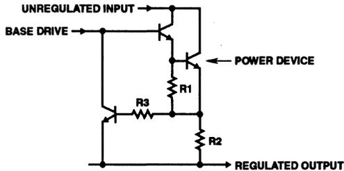
FIGURE 14. STANDARD CURRENT LIMIT
