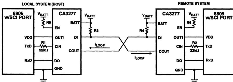
FIGURE 7. USING THE CA3277 FOR FULL DUPLEX SIGNAL TRANSMISSION
