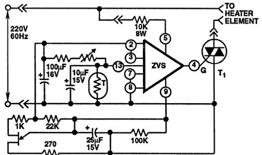
FIGURE 17. SCHEMATIC DIAGRAM OF PROPORTIONAL ZERO-VOLTAGE SWITCHING CONTROL
