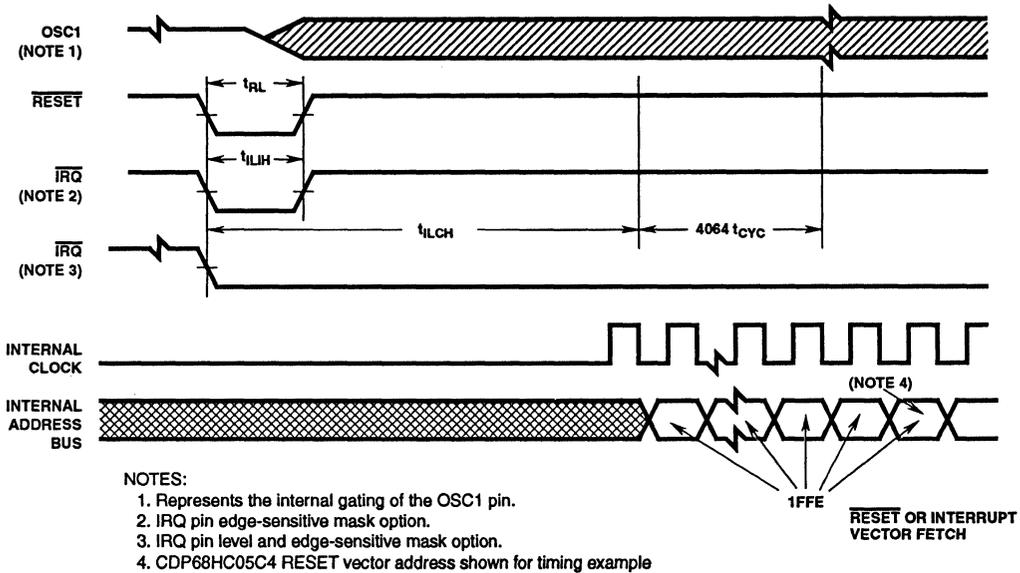
FIGURE 1. STOP RECOVERY TIMING DIAGRAM
