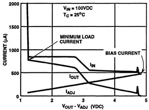
FIGURE 38. TERMINAL CURRENTS vs FORCED  $V_{REF}$
