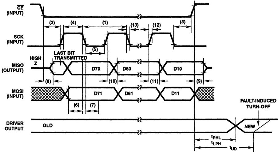
FIGURE 1B. SPI TIMING DIAGRAM
