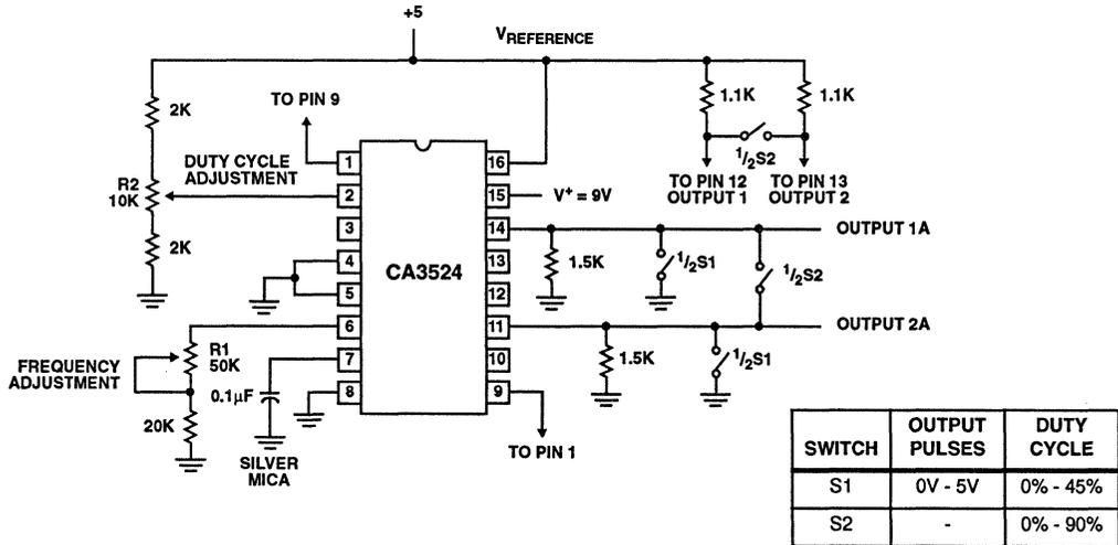
FIGURE 38. LOW FREQUENCY PULSE GENERATOR
