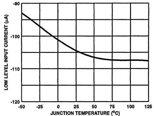
FIGURE 9. ALI, BLI, AHI, BHI LOW LEVEL INPUT CURRENT  $I_L$  vs TEMPERATURE
