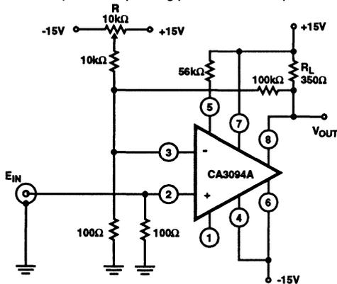
FIGURE 5. CLASS A AMPLIFIER -280mW CAPABILITY INTO A RESISTIVE LOAD
