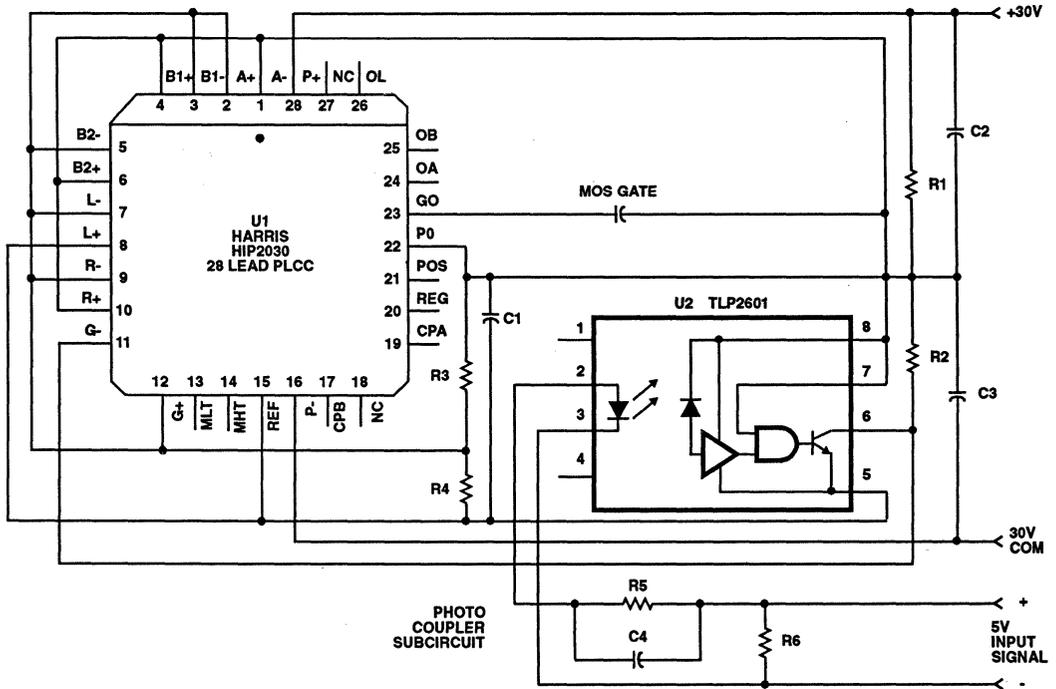
FIGURE 1. HARRIS PHOTO-COUPLED ISOLATED GATE DRIVE
