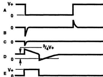
On a negative going transient at input (A), a negative pulse at C will turn "on" the CA3094, and the output (E) will go from a low to a high level.
