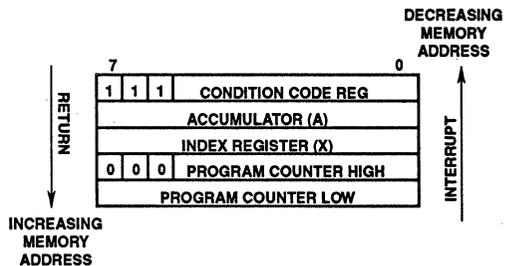
FIGURE 10. STACKING ORDER DURING INTERRUPTS
