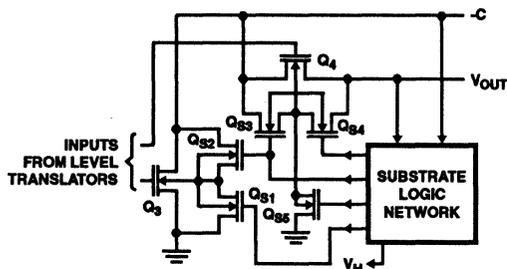
FIGURE 5. THE SUBSTRATE LOGIC NETWORK
