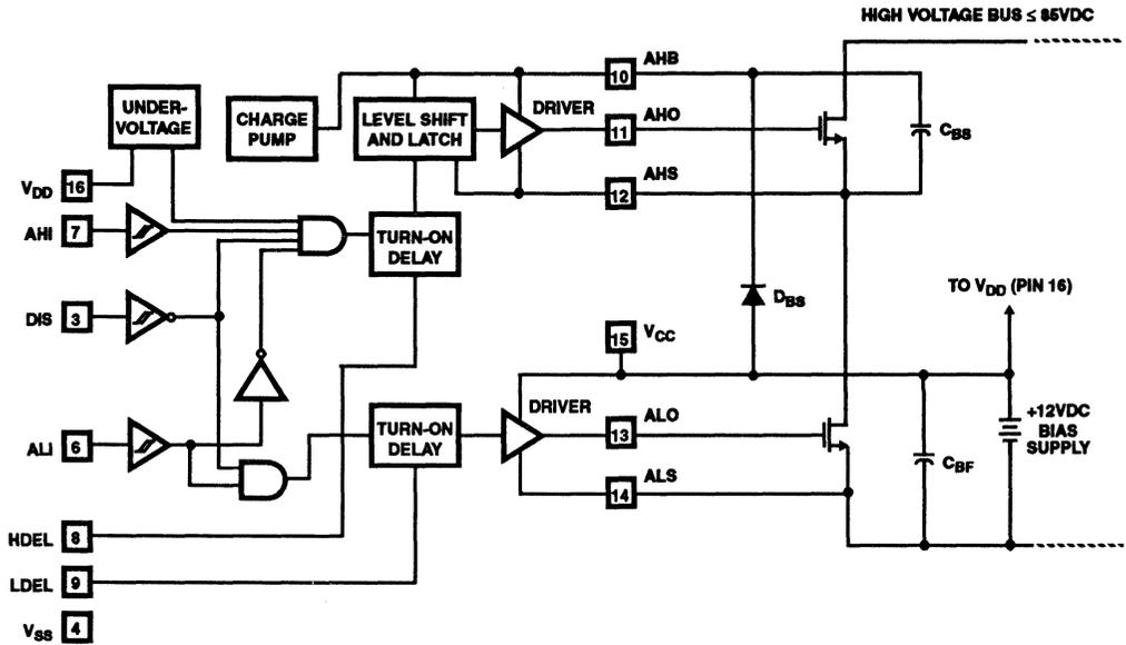
FIGURE 4. HIP4081A BLOCK DIAGRAM
