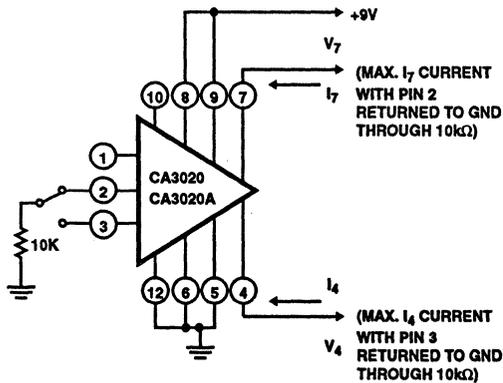
FIGURE 4A. TEST SETUP
