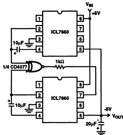
FIGURE 14. SYNCHRONIZING TWO ICL7660s
