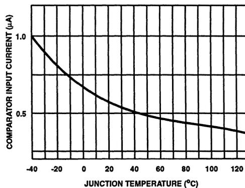
FIGURE 9. COMPARATOR INPUT CURRENT  $I_I$  vs TEMPERATURE AT  $V_{CM} = 5V$
