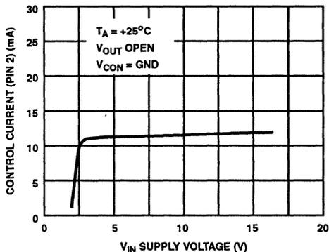
FIGURE 6. CONTROL (QUIESCENT) CURRENT CHARACTERISTIC WITH NO LOAD
