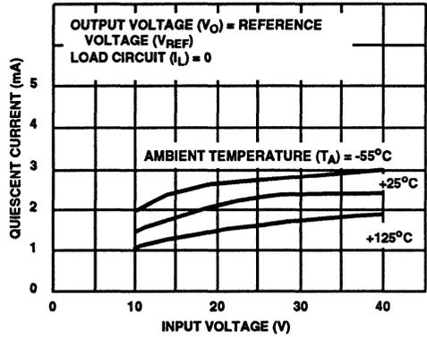
FIGURE 7. QUIESCENT CURRENT vs INPUT VOLTAGE
