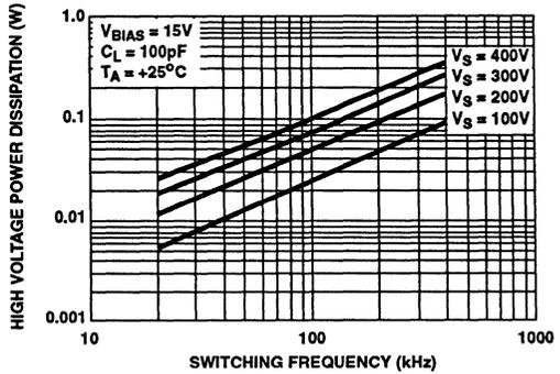
FIGURE 2. HIGH VOLTAGE POWER DISSIPATION vs SWITCHING FREQUENCY
