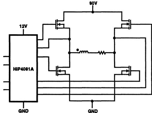
FIGURE 1. HIP4081A SIMPLIFIED APPLICATION DIAGRAM
