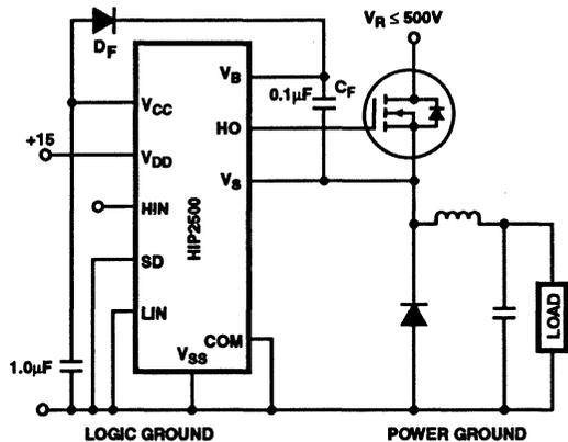
FIGURE 2. HIGH SIDE SWITCH OR "BUCK CONVERTERS"
