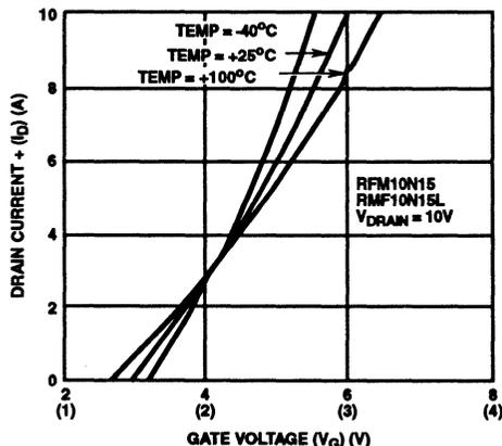
FIGURE 3. TRANSFER CHARACTERISTIC
