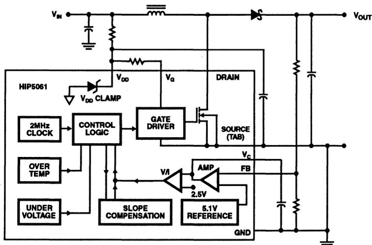
FIGURE 1. SIMPLIFIED BLOCK DIAGRAM OF THE HIP5061 IN A TYPICAL "BOOST" CONFIGURATION
