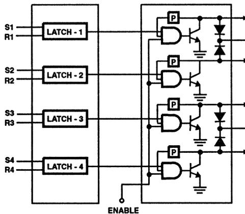
FIGURE 5. TYPICAL APPLICATIONS FOR THE CA3242 QUAD DRIVER
