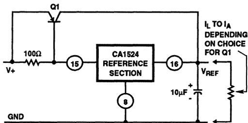
FIGURE 10. CIRCUIT FOR EXPANDING THE REFERENCE CURRENT CAPABILITY
