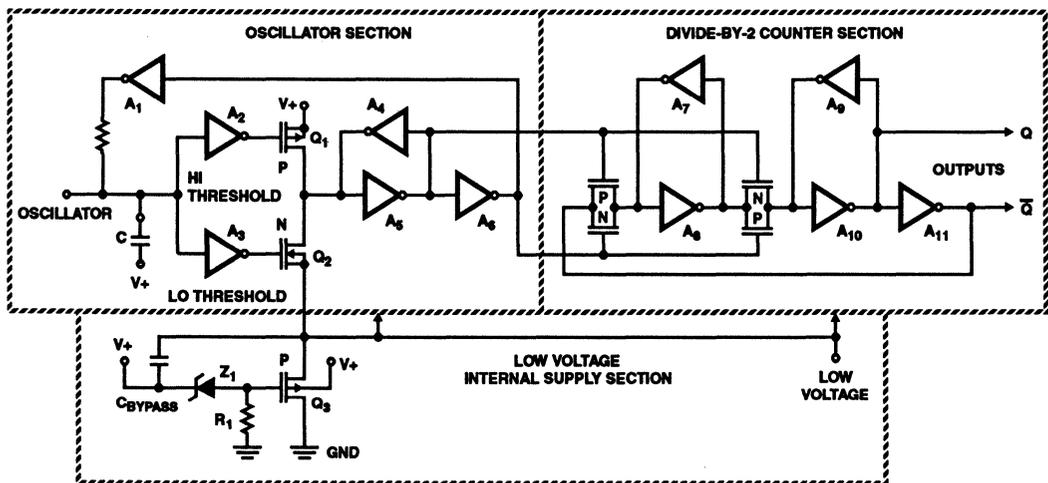
FIGURE 3. THE ICL7660s OSCILLATOR, DIVIDER AND INTERNAL REGULATOR
