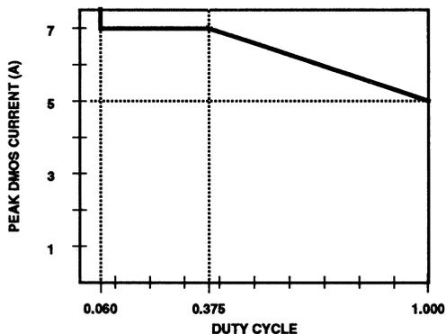
FIGURE 3. PEAK DMOS TRANSISTOR DRAIN CURRENT vs DUTY CYCLE
