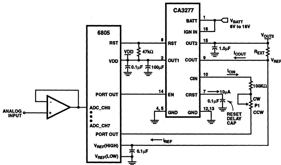
FIGURE 9. PROGRAMMABLE VOLTAGE REFERENCE FOR MICROPROCESSOR APPLICATIONS
