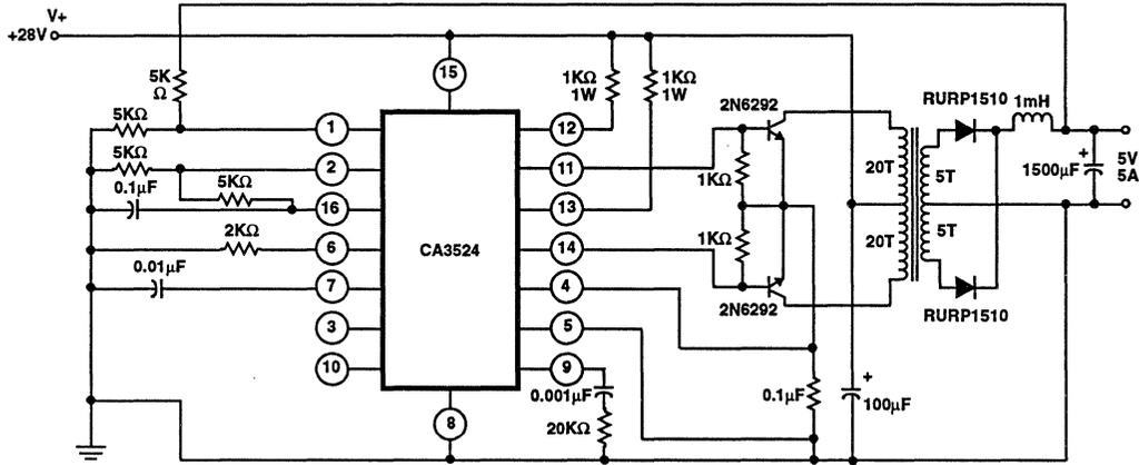
FIGURE 37. PUSH-PULL TRANSFORMER COUPLED CONVERTER
