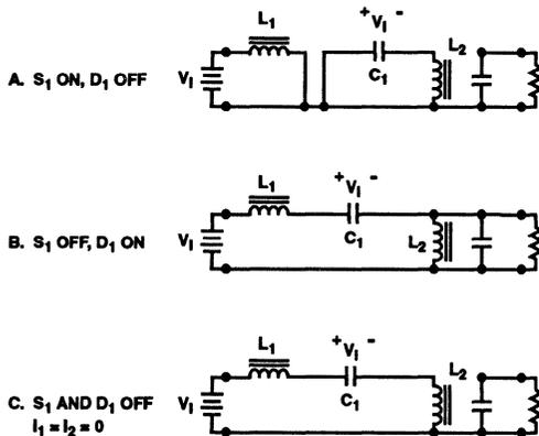
FIGURE 10. SEPIC DCM CIRCUIT STATES  $L_2/L_1 = M$
