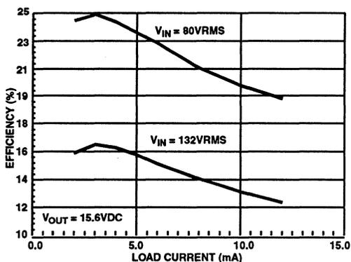
FIGURE 11. EFFICIENCY AS A FUNCTION OF LOAD CURRENT
