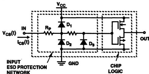
FIGURE 9. TYPICAL CMOS IC INPUT PROTECTION CIRCUIT
