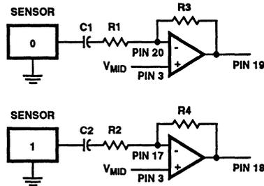
FIGURE 3. INPUT AMPLIFIER CONNECTIONS
