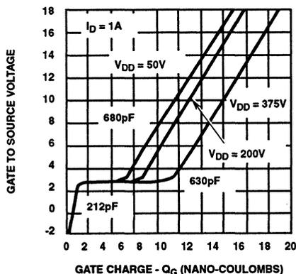
FIGURE 9. MOSFET GATE DYNAMIC CHARACTERISTICS
