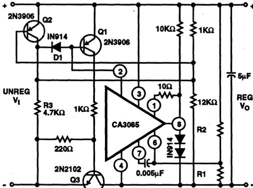
FIGURE 10. NEGATIVE VOLTAGE REGULATOR
