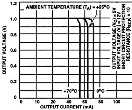
FIGURE 12. CURRENT LIMITING CHARACTERISTICS
