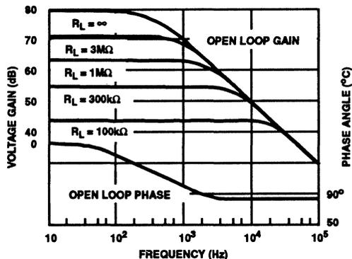
FIGURE 12. OPEN-LOOP ERROR AMPLIFIER RESPONSE CHARACTERISTICS
