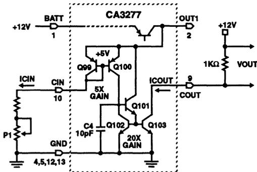
FIGURE 5A. CURRENT GAIN LINEARITY TEST CIRCUIT SHOWN WITH THE CA3277 CURRENT MULTIPLIER
