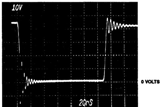
FIGURE 5. DMOS TRANSISTOR DRAIN VOLTAGE DURING CONDUCTION.
