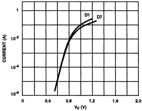
FIGURE 15. DIODE D1 AND D7 CURRENT vs  $V_F$
