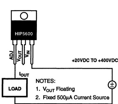
FIGURE 15. CONSTANT 450 $\mu$ A CURRENT SOURCE
