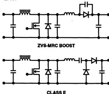
FIGURE 4. MULTI-RESONANT CONVERTERS
