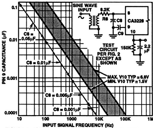
FIGURE 6. F/V CONVERTER RANGE EXTENSION WITH ADJUSTMENT OF C8 AND C9
