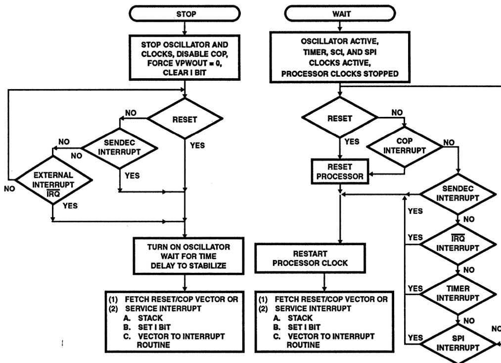
FIGURE 14. STOP AND WAIT FLOW DIAGRAM
