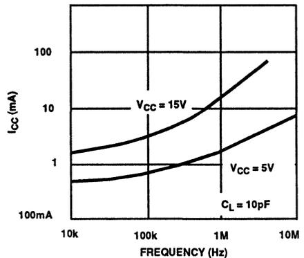
FIGURE 6. NO LOAD  $I_{CC}$  vs FREQUENCY
