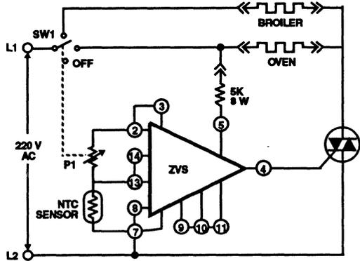
FIGURE 37. SCHEMATIC DIAGRAM OF BASIC OVEN CONTROL
