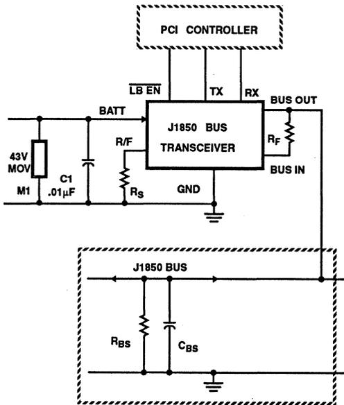
FIGURE 3. TEST/APPLICATION CIRCUIT DIAGRAM
