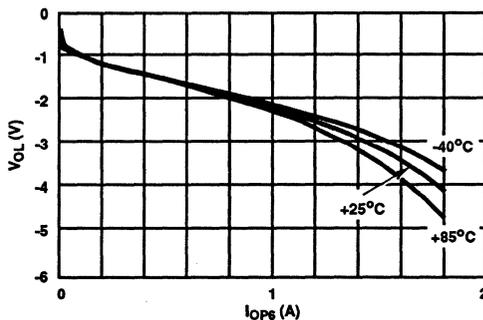
FIGURE 8. PIN 3/6 VOLTAGE vs REVERSE CURRENT 300 $\mu\text{s}$  PULSES
