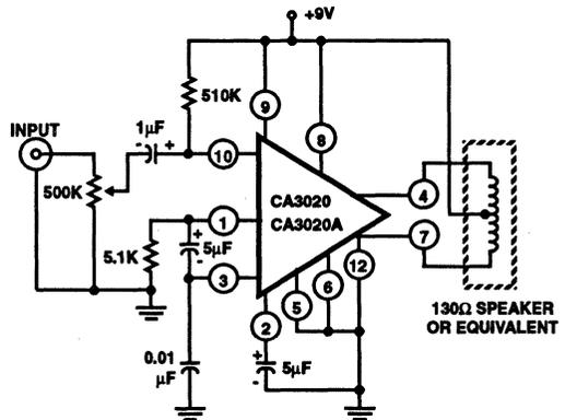
**FIGURE 8. 310mW AUDIO AMPLIFIER WITHOUT TRANSFORMERS**
