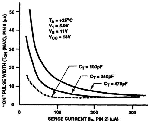
FIGURE 8. PULSE/FREQUENCY MODULATOR CHARACTERISTIC  $T_{ON(MAX)}$  OUTPUT PULSE WIDTH (PIN 6) vs. CURRENT SENSE (PIN 2). ( $T_A = 25^\circ\text{C}$ ,  $V_1 = 5.9\text{V}$ ,  $V_S = 11\text{V}$ ,  $V_{CC} = 13\text{V}$ )
