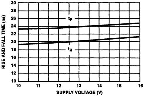
FIGURE 13. RISE AND FALL TIME vs SUPPLY VOLTAGE
