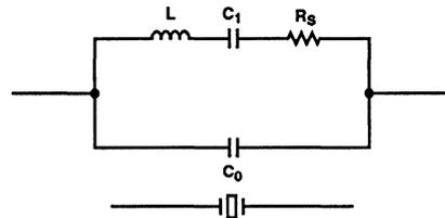
FIGURE 4D. CRYSTAL/RESONATOR EQUIVALENT CIRCUIT
