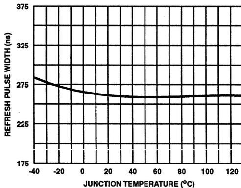
FIGURE 14.  $T_{REF-PW}$  REFRESH PULSE WIDTH vs TEMPERATURE
