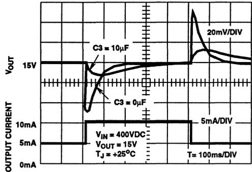
FIGURE 30. LOAD TRANSIENT RESPONSE
