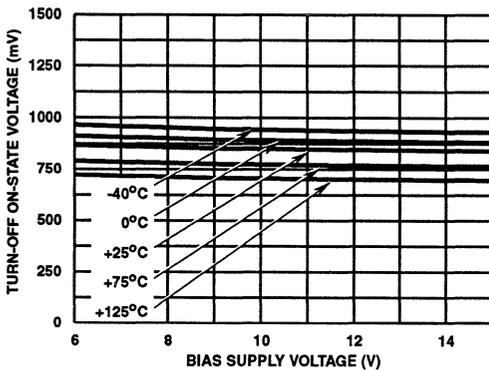
FIGURE 26. LOW LEVEL OUTPUT VOLTAGE  $V_{OL}$  vs BIAS SUPPLY AND TEMPERATURE AT 100mA
