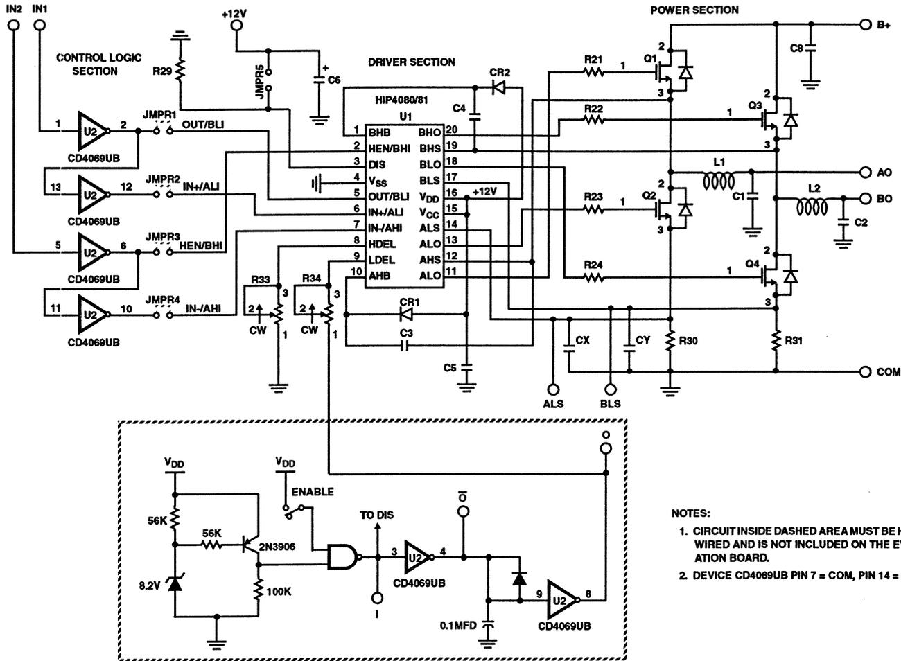
FIGURE 33. HIP4080 EVALUATION PC BOARD SCHEMATIC
