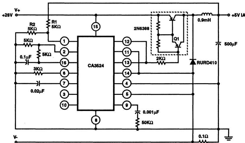
FIGURE 34. SINGLE-ENDED LC SWITCHING REGULATOR CIRCUIT
