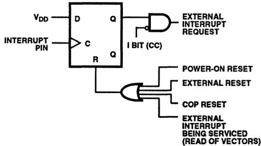
FIGURE 12A. INTERRUPT FUNCTION DIAGRAM
