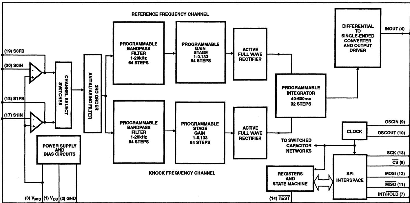
FIGURE 1. SIMPLIFIED BLOCK DIAGRAM OF THE HIP9010
