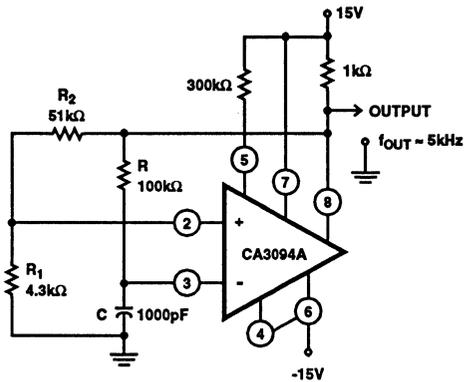
$$\text{NOTE: } f_{\text{OUT}} = \frac{1}{2RC \ln\left(\frac{2R_1}{R_2} + 1\right)}$$
