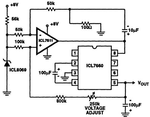
FIGURE 22. REGULATING THE OUTPUT VOLTAGE
