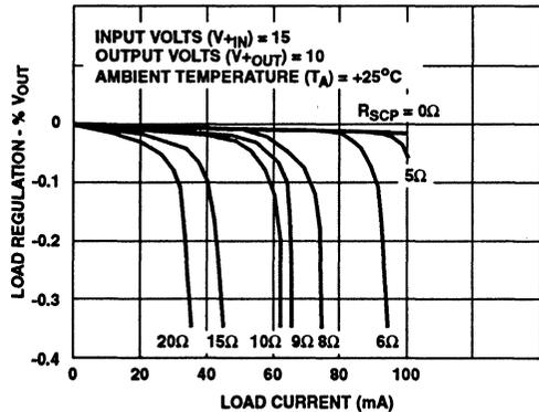
FIGURE 8. LOAD REGULATION CHARACTERISTICS
