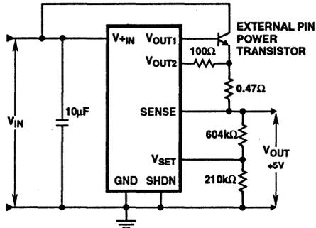
FIGURE 10. BOOSTING OUTPUT CURRENT WITH EXTERNAL TRANSISTOR
