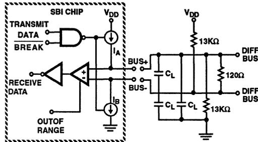
FIGURE 4. DIFFERENTIAL DRIVER/RECEIVER
