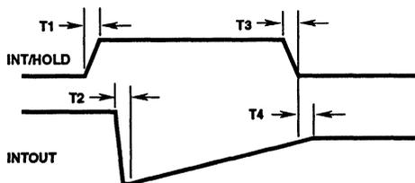
FIGURE 8. INTEGRATOR TIMING
