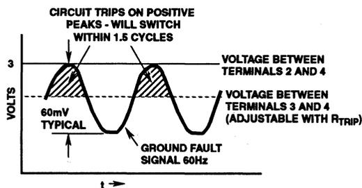
FIGURE 32. GROUND FAULT INTERRUPTER (GFI) AND WAVEFORM PERTINENT TO GROUND FAULT DETECTOR
