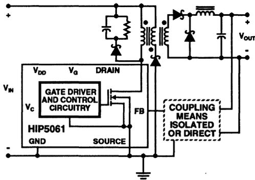
FIGURE 9. FORWARD CONVERTER
