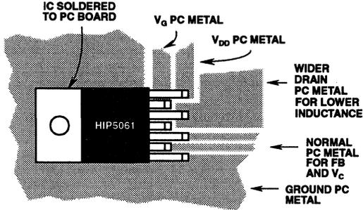
**FIGURE 6. SHOWING WIDER PC BOARD METAL FOR CRITICAL LEADS**
