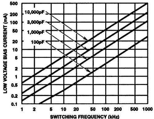
FIGURE 8. LOW VOLTAGE BIAS CURRENT  $I_{BD}$  (LESS QUIESCENT COMPONENT) vs FREQUENCY AND GATE LOAD CAPACITANCE
