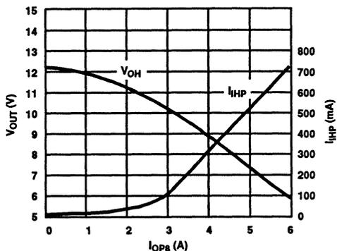
FIGURE 4. PIN 2  $I_{IHP}$  &  $V_{OH}$  vs OUTPUT SOURCE CURRENT
