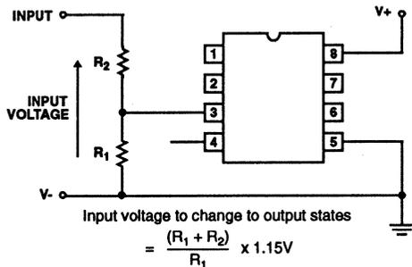
FIGURE 24. RANGE OF INPUT VOLTAGE GREATER THAN +1.15 VOLTS
