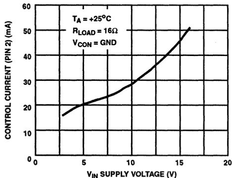
FIGURE 5. CONTROL (QUIESCENT) CURRENT CHARACTERISTIC WITH LOAD
