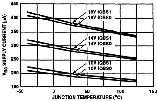
FIGURE 9. QUIESCENT  $V_{BS}$  SUPPLY CURRENT vs TEMPERATURE
