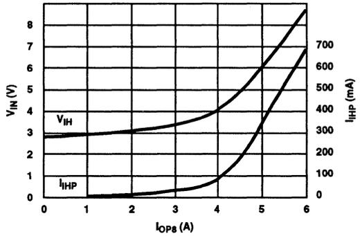
FIGURE 18.  $V_{IH}$  AND  $I_{IHP}$  vs  $I_{OP8}$  [ $V_{OUT}$  (PIN 8) = 0,  $V_+ = 15\text{V}$ , 1 $\mu\text{s}$  PULSE]
