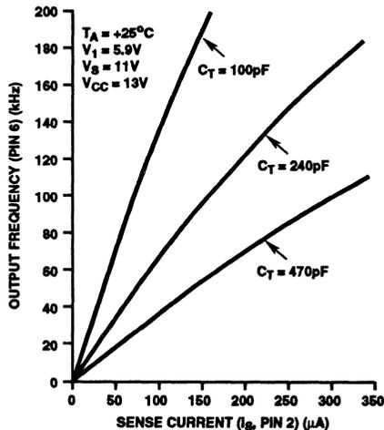
FIGURE 7. PULSE/FREQUENCY MODULATOR CHARACTERISTIC OF FREQUENCY vs. TIMING CAPACITOR  $C_T$  AND SENSE CURRENT  $I_S$  ( $T_A = +25^\circ\text{C}$ ,  $V_1 = 5.9\text{V}$ ,  $V_S = 11\text{V}$ ,  $V_{CC} = 13\text{V}$ )
