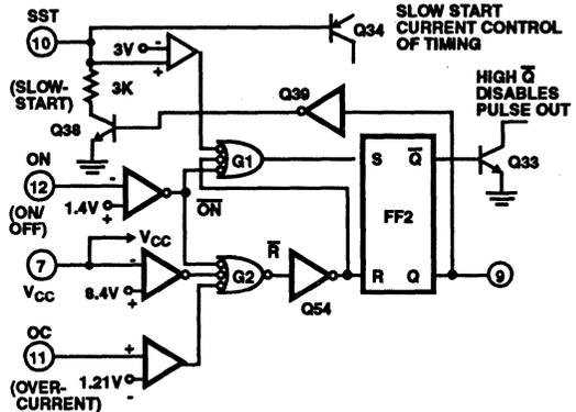
FIGURE 5. CA1523 LOGIC CONTROL DIAGRAM
