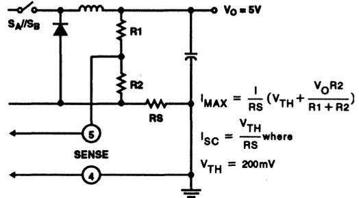
FIGURE 14. FOLDBACK CURRENT-LIMITING CIRCUIT USED TO REDUCE POWER DISSIPATION UNDER SHORTED OUTPUT CONDITIONS
