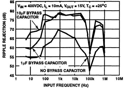
FIGURE 24. RIPPLE REJECTION RATIO (INPUT FREQUENCY)
