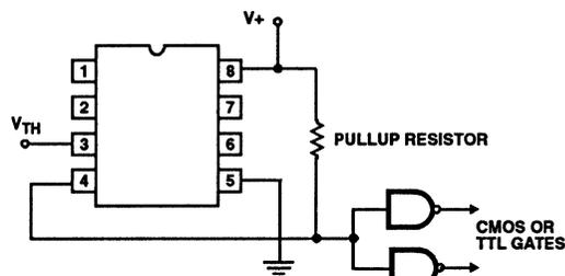
FIGURE 22. OUTPUT LOGIC INTERFACE
