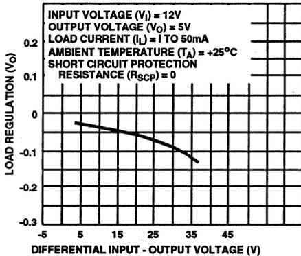
FIGURE 14. LOAD REGULATION vs DIFFERENTIAL INPUT-OUTPUT VOLTAGE
