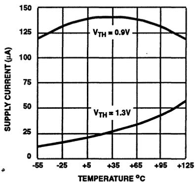
FIGURE 5. SUPPLY CURRENT AS A FUNCTION OF TEMPERATURE
