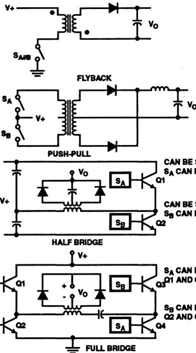
**FIGURE 19. TRANSFORMER-COUPLED OUTPUTS**
