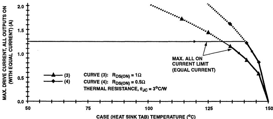
FIGURE 5. HIP0081 CURRENT vs CASE (TAB) TEMPERATURE, ALL OUTPUTS ON WITH EQUAL CURRENT
