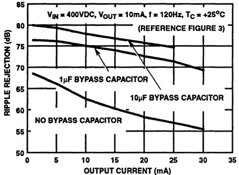
FIGURE 26. RIPPLE REJECTION RATIO (OUTPUT CURRENT)
