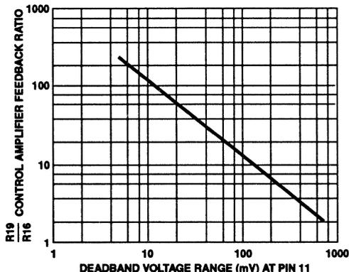
FIGURE 17. DEADBAND VOLTAGE RANGE IN OUTPUT CIRCUIT AS A FUNCTION OF CONTROL AMPLIFIER FEEDBACK RATIO (GAIN ADJUSTMENT) REFERENCED TO V<sub>S</sub> AT PIN 11
