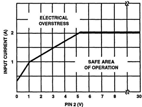
FIGURE 18. HV-2405E SAFE INTERRUPT CURRENT vs PIN 2 VOLTAGE
