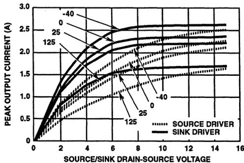
FIGURE 11. DRIVER SINK/SOURCE V-I CHARACTERISTIC
