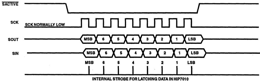
FIGURE 7. SERIAL BUS TIMING
