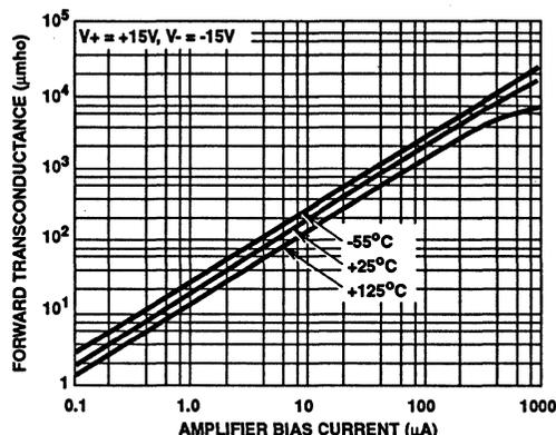
FIGURE 12. FORWARD TRANSCONDUCTANCE vs AMPLIFIER BIAS CURRENT
