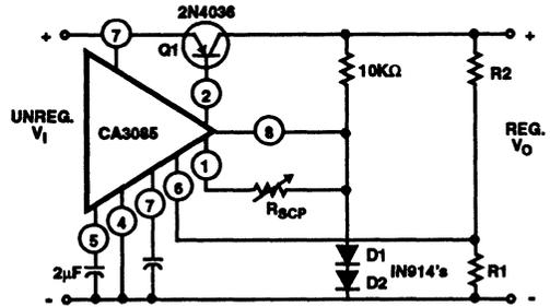
FIGURE 7. VOLTAGE REGULATOR FOR LOW  $V_1 - V_0$
