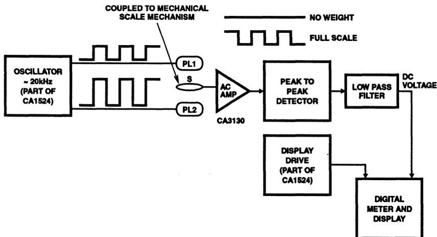
FIGURE 1. BLOCK DIAGRAM - DIGITAL READOUT SCALE CIRCUIT
