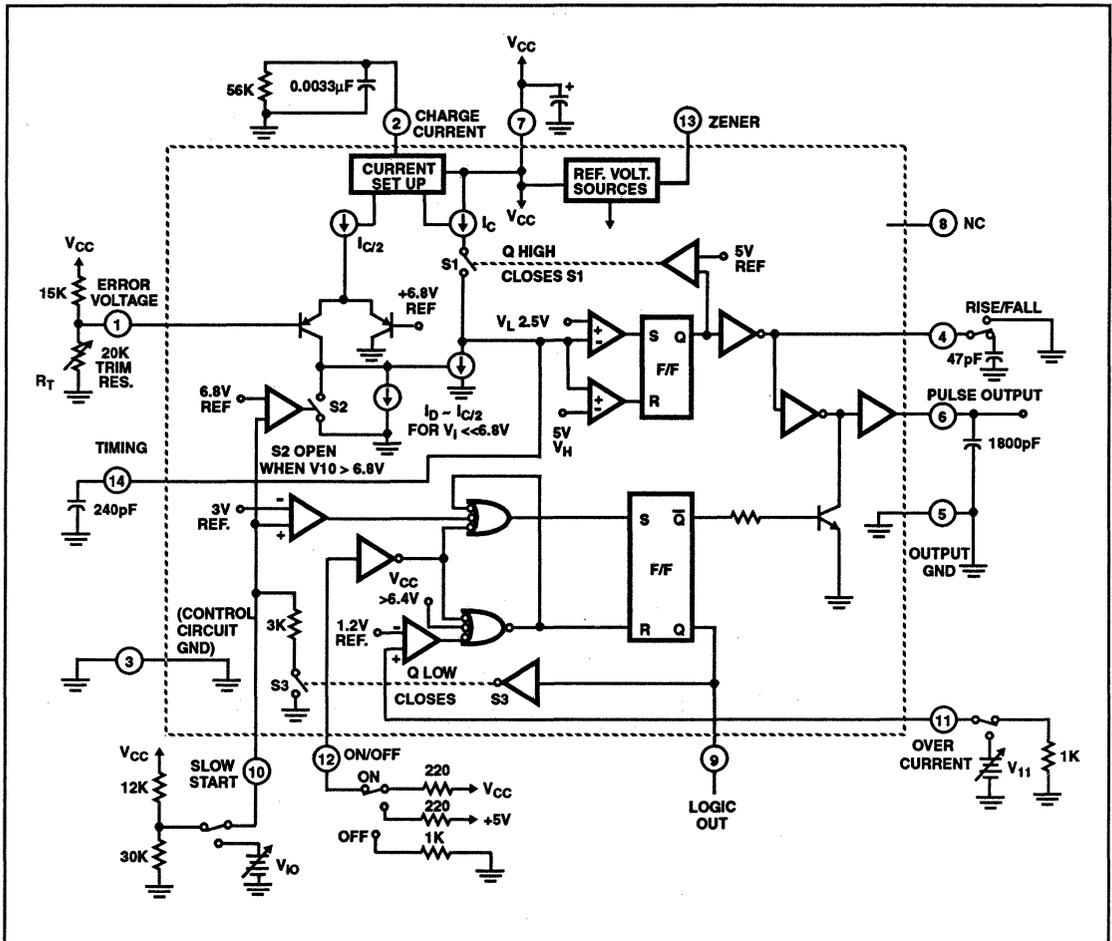
FIGURE 1. TEST CIRCUIT FOR THE CA1523
