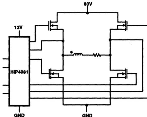
FIGURE 1. HIP4081 SIMPLIFIED APPLICATION DIAGRAM
