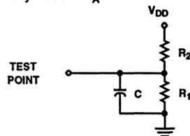
EQUIVALENT TEST LOAD (SEE TABLE FOR VALUES OF  $R_1$  AND  $R_2$ )
