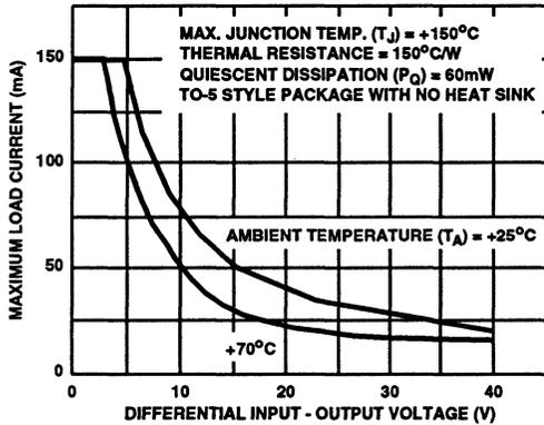
FIGURE 8. MAX LOAD CURRENT vs DIFFERENTIAL INPUT-OUTPUT VOLTAGE
