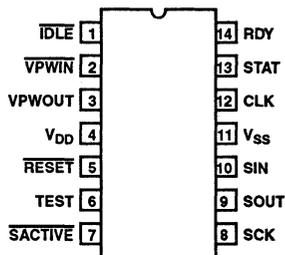
FIGURE 2. 14 PIN DIP AND SO TERMINAL ASSIGNMENTS
