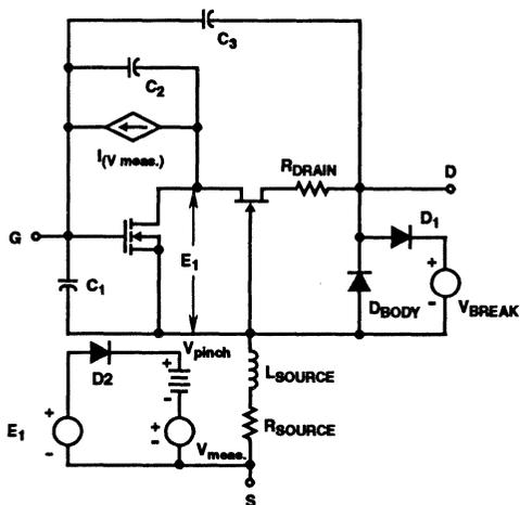
FIGURE 1. SPICE-2 SUBCIRCUIT FOR POWER MOSFET SIMULATION.
