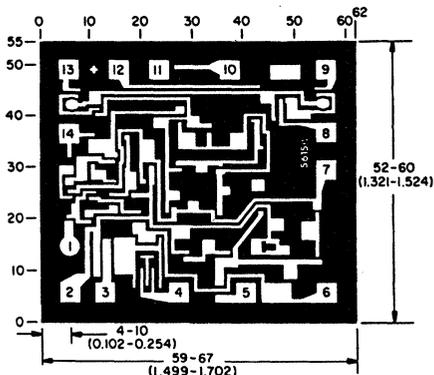
Dimensions in parentheses are in millimeters and are derived from the basic inch dimensions as indicated. Grid gradations are in mils (10<sup>-3</sup> inch).
