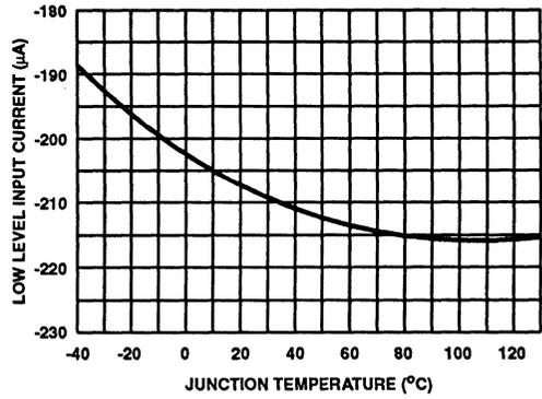
FIGURE 11. HEN LOW LEVEL INPUT CURRENT  $I_{IL}$  vs TEMPERATURE
