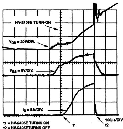
FIGURE 4. TYPICAL WAVEFORMS OF THE MOSFET ( $I_{OUT} = 250mA$ )
