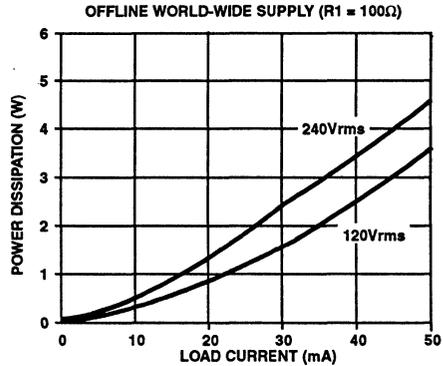
FIGURE 5. POWER DISSIPATION IN R1 vs LOAD CURRENT
