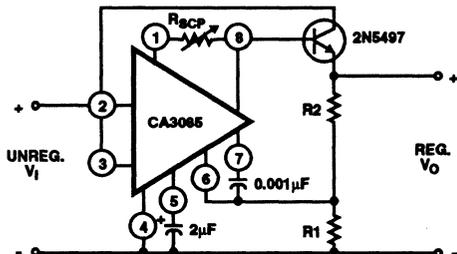
FIGURE 6A. WITH SIMPLIFIED SHORT-CIRCUIT PROTECTION
