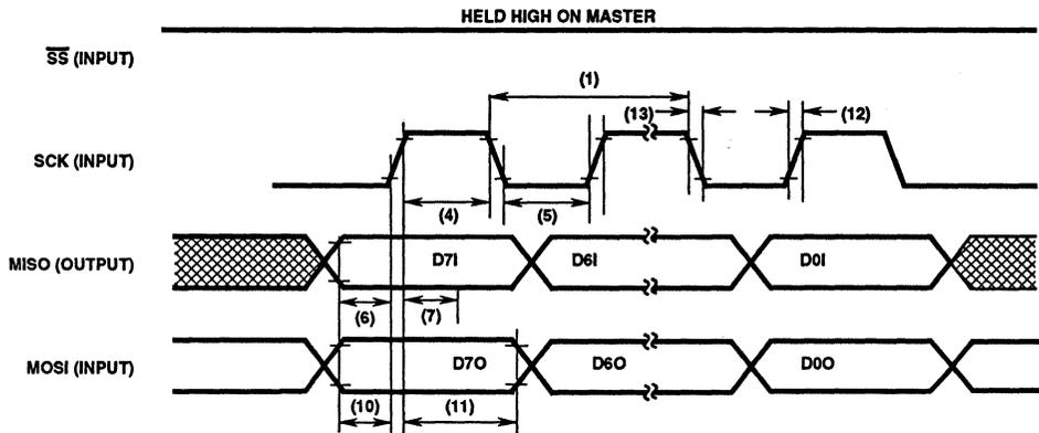
**FIGURE 3C. SPI MASTER TIMING CPOL = 0, CPHA = 0**
