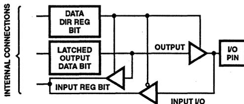
FIGURE 5B. PORT A FUNCTIONAL BLOCK DIAGRAM
