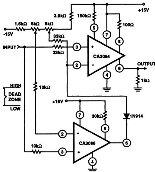
FIGURE 19. DUAL LIMIT THRESHOLD DETECTOR
