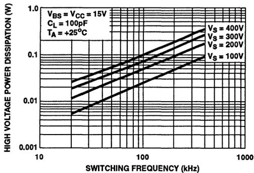
FIGURE 22. HIGH VOLTAGE POWER DISSIPATION vs SWITCHING FREQUENCY
