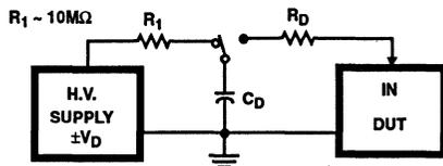
**FIGURE 1. ELECTROSTATIC DISCHARGE TEST
