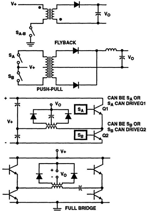
FIGURE 17. TRANSFORMER-COUPLED OUTPUTS
