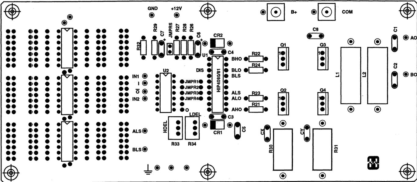
FIGURE 32. HIP4081A EVALUATION BOARD SILKSCREEN
