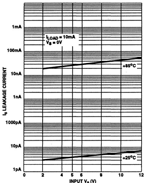
FIGURE 5.  $I_B$  LEAKAGE CURRENT  $V_P$  TO  $V_S$  AS A FUNCTION OF INPUT VOLTAGE
