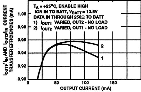
FIGURE 4F. TYPICAL CHARACTERISTIC CURVES FOR CURRENT TRANSFER EFFICIENCY OF  $I_{\text{OUT}_1}/I_{\text{IN}}$  AND  $I_{\text{OUT}_2}/I_{\text{IN}}$  WHERE  $I_{\text{IN}}$  INCLUDES ( $I_{\text{IGN IN}} + I_{\text{DATA IN}}$ ) BIAS CURRENTS
