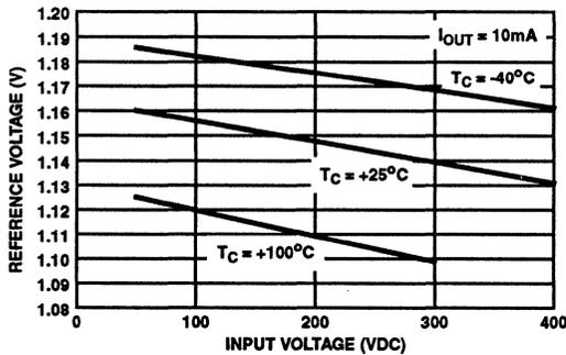
FIGURE 33. REFERENCE VOLTAGE vs INPUT VOLTAGE
