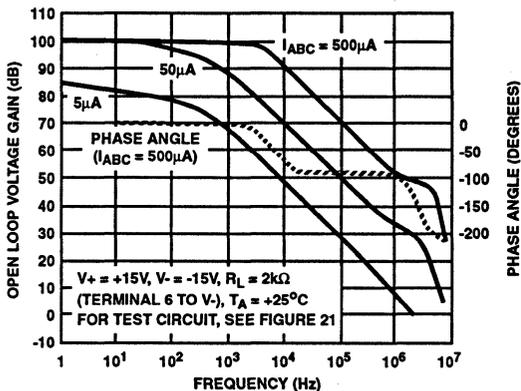
FIGURE 11. OPEN LOOP VOLTAGE GAIN vs FREQUENCY
