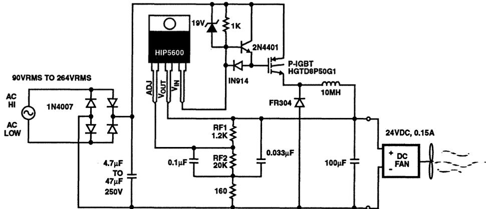
FIGURE 17. HIGH CURRENT "BUCK" REGULATOR
