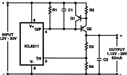
FIGURE 7. POSITIVE REGULATOR - PNP BOOST CURRENT LIMITED
