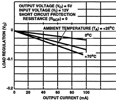
FIGURE 10. LOAD REGULATION WITHOUT CURRENT LIMITING
