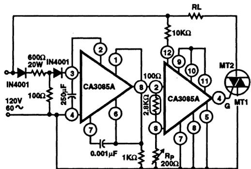
FIGURE 22. VOLTAGE REGULATOR FOR SENSOR AND ZERO-VOLTAGE SWITCH
