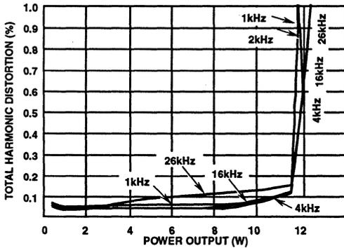
FIGURE 17. TOTAL HARMONIC DISTORTION OF THE AMPLIFIER WITH AN UNREGULATED POWER SUPPLY
