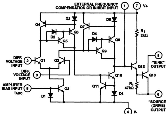
FIGURE 1. CA3094 CIRCUIT SCHEMATIC DIAGRAM
