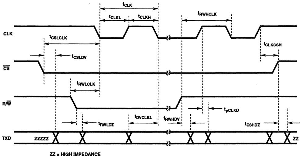
FIGURE 1. SERIAL INTERFACE TIMING DIAGRAM
