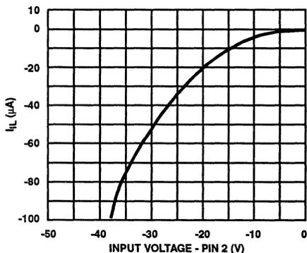
FIGURE 5. PIN 2  $I_{IL}$  vs INPUT VOLTAGE
