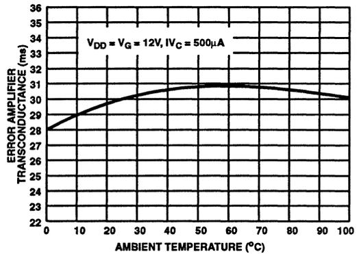
FIGURE 12. TYPICAL ERROR AMPLIFIER TRANSCONDUCTANCE vs TEMPERATURE
