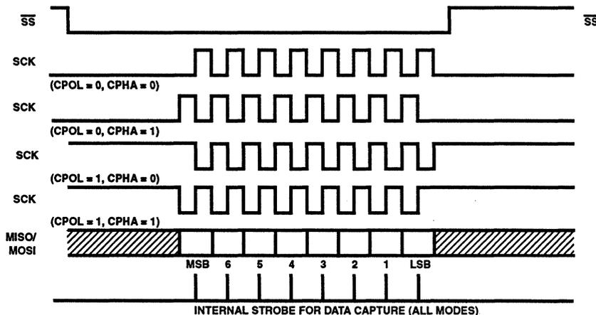
FIGURE 21. DATA CLOCK TIMING DIAGRAM
