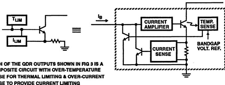
EACH OF THE QDR OUTPUTS SHOWN IN FIG 3 IS A COMPOSITE CIRCUIT WITH OVER-TEMPERATURE SENSE FOR THERMAL LIMITING & OVER-CURRENT SENSE TO PROVIDE CURRENT LIMITING
