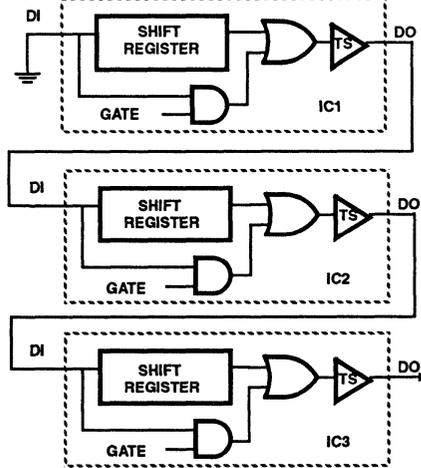
FIGURE 3. CASCADED CHIP OPERATION TO READ DIAGNOSTIC DATA
