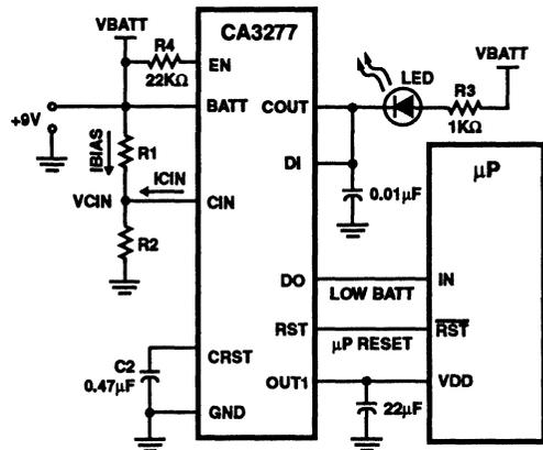
FIGURE 6. EXAMPLE OF A LOW BATTERY FAULT INDICATOR CIRCUIT
