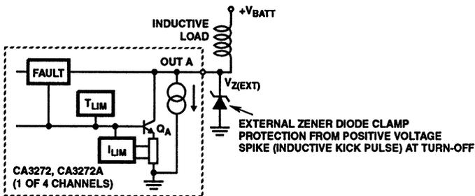
FIGURE 4B. CA3272 AND CA3272A OVER-VOLTAGE PROTECTION IS AN EXTERNAL ZENER DIODE CLAMP WHERE  $V_{Z(EXT)} \leq V_{CE(SUS)}$ . THE  $V_{CE(SUS)}$  VOLTAGE RATING IS THE MAXIMUM VOLTAGE FOR FULL LOAD SWITCHING.
