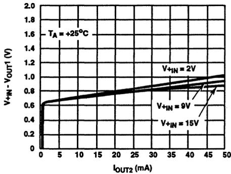
FIGURE 3.  $V_{OUT2}$  INPUT-OUTPUT DIFFERENTIAL vs OUTPUT CURRENT
