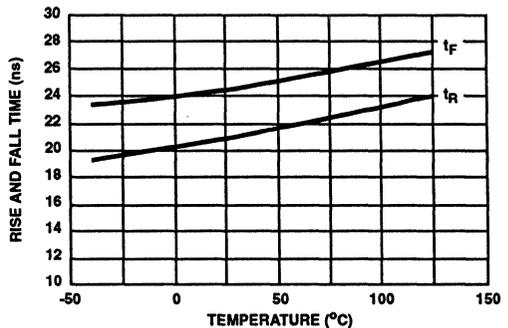
FIGURE 12. RISE AND FALL TIME vs TEMPERATURE
