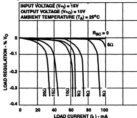
FIGURE 4. LOAD REGULATION CHARACTERISTICS FOR CIRCUIT OF FIGURE 3
