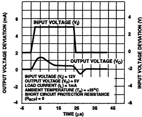
FIGURE 18. LOAD TRANSIENT RESPONSE
