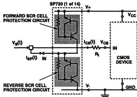
FIGURE 10. SP720 SCR INTERFACE TO A CMOS INPUT WITH  $R_1$  ADDED TO ILLUSTRATE MORE EFFECTIVE ESD PROTECTION FOR CMOS DEVICES
