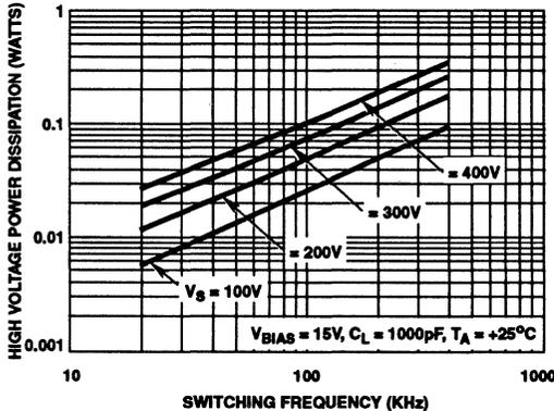
FIGURE 11. HIGH VOLTAGE POWER DISSIPATION vs SWITCHING FREQUENCY
