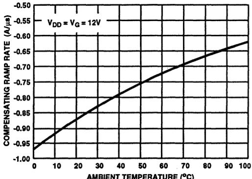
FIGURE 30. TYPICAL COMPENSATING RAMP RATE vs TEMPERATURE
