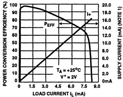
FIGURE 10. SUPPLY CURRENT AND POWER CONVERSION EFFICIENCY AS A FUNCTION OF LOAD CURRENT
