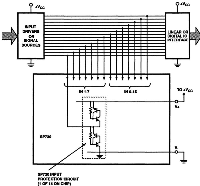
**FIGURE 8. PRACTICAL APPLICATION AND TEST EVALUATION CIRCUIT**
