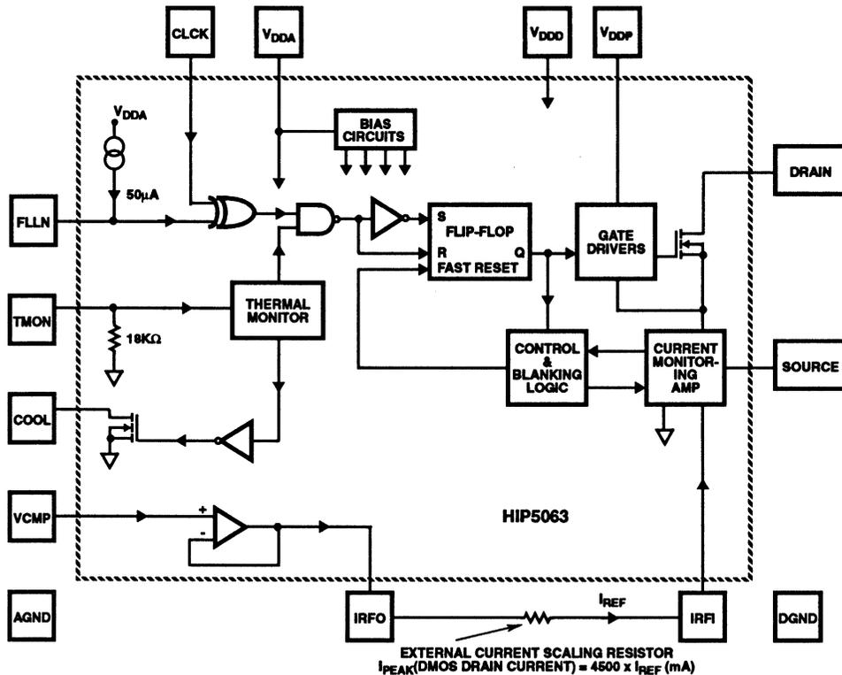
FIGURE 9. FUNCTIONAL BLOCK DIAGRAM OF THE HIP5063
