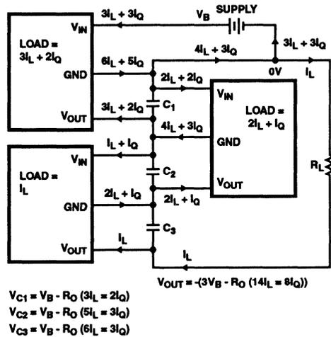
FIGURE 17. CURRENT FLOW FOR CASCADED DEVICES
