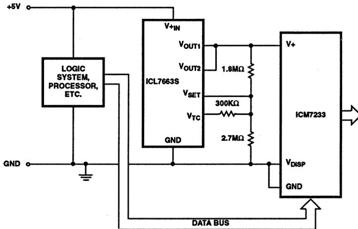
FIGURE 11. GENERATING A MULTIPLEXED LCD DISPLAY DRIVE VOLTAGE
