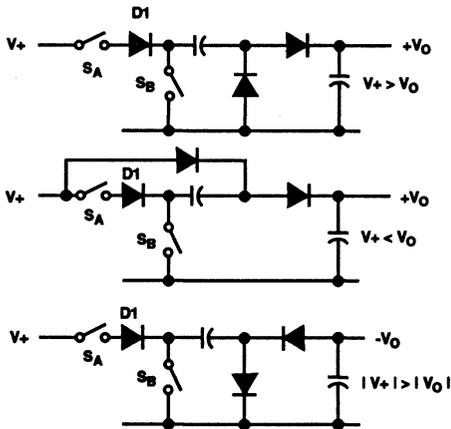
NOTE: Diode D1 is Necessary To Prevent Reverse Emitter-Base Breakdown of Transistor Switch  $S_A$
