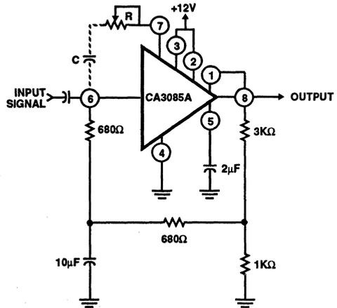
FIGURE 23. GENERAL-PURPOSE AMPLIFIER USING CA3085A
