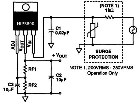
FIGURE 13. AC/DC CONVERTER
