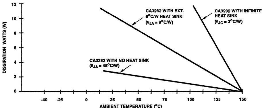
FIGURE 5. DISSIPATION DERATING CURVE
