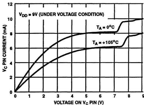
FIGURE 16. TYPICAL  $V_C$  PIN CURRENT vs VOLTAGE ON  $V_C$  PIN FOR  $0^\circ\text{C}$  AND  $+105^\circ\text{C}$
