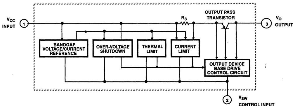
FIGURE 1. FUNCTIONAL BLOCK DIAGRAM OF CA3273
