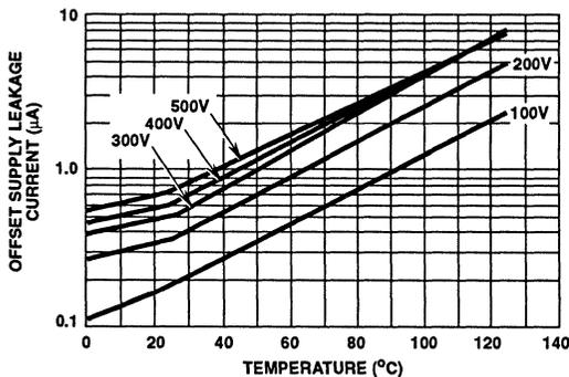
FIGURE 5. OFFSET SUPPLY LEAKAGE vs TEMPERATURE
