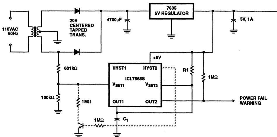
FIGURE 17. AC POWER FAIL AND BROWNOUT DETECTOR
