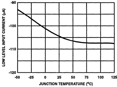
FIGURE 10. DIS LOW LEVEL INPUT CURRENT  $I_{IL}$  vs TEMPERATURE
