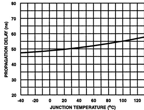
FIGURE 15. DISABLE TO LOWER ENABLE  $T_{DLPH}$  PROPAGATION DELAY vs TEMPERATURE
