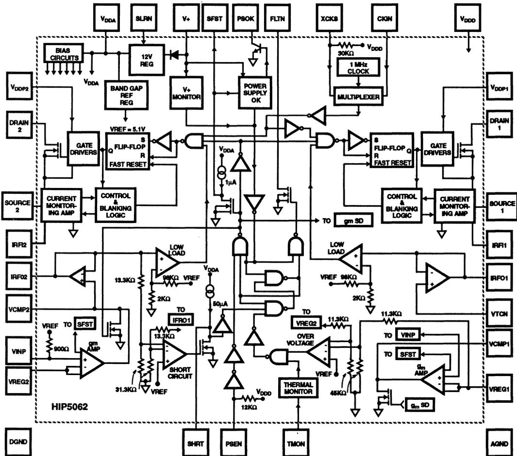
FIGURE 7. FUNCTIONAL BLOCK DIAGRAM OF THE HIP5062
