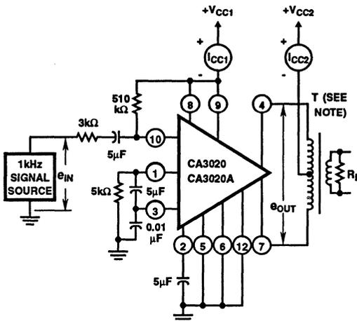
NOTE: Push-pull output transformer; load resistance ( $R_L$ ) should be selected to provide indicated collector-to-collector load impedance ( $R_{CC}$ ).
