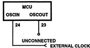
FIGURE 4E. EXTERNAL CLOCK SOURCE CONNECTIONS
