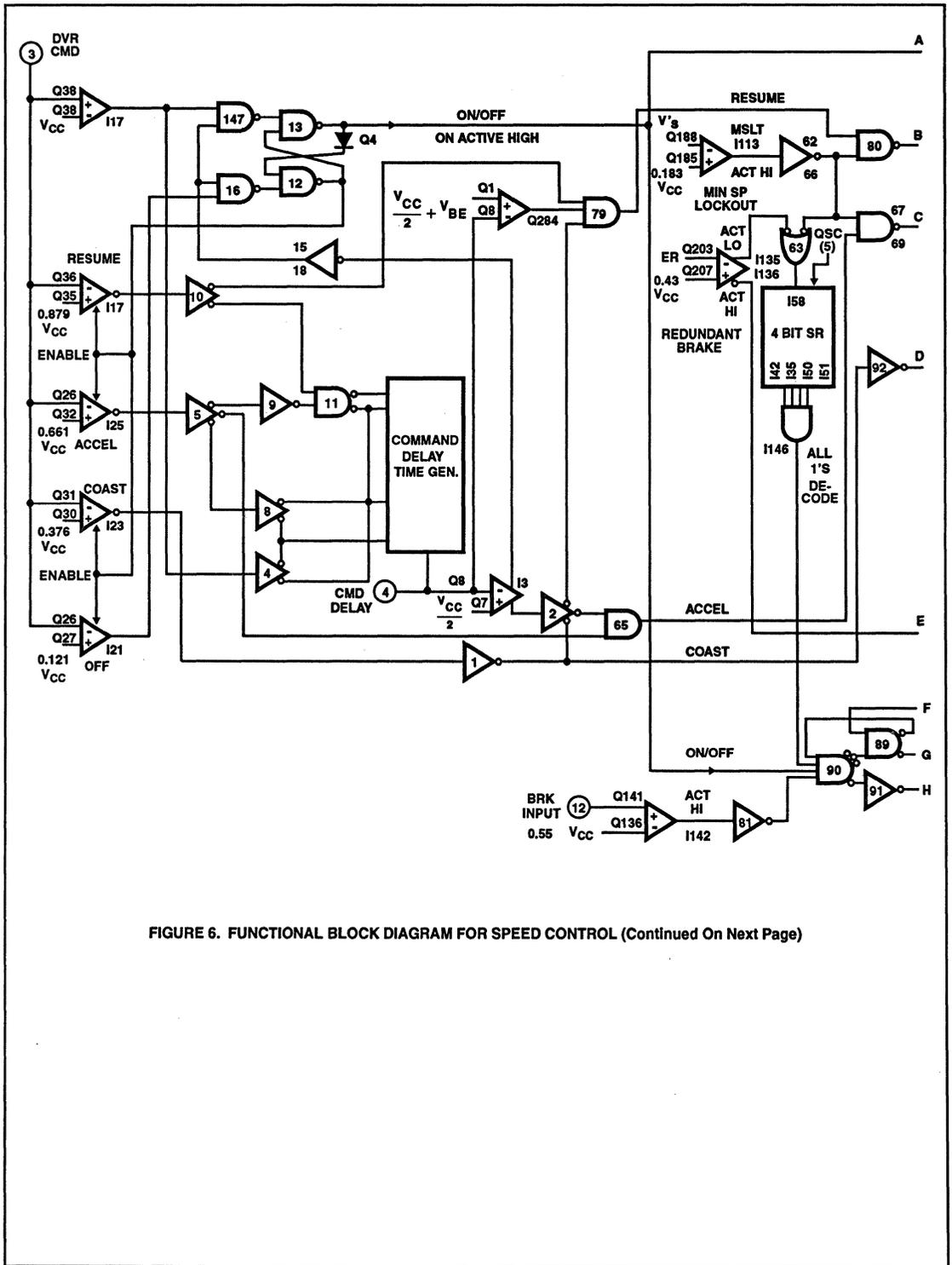
FIGURE 6. FUNCTIONAL BLOCK DIAGRAM FOR SPEED CONTROL (Continued On Next Page)
