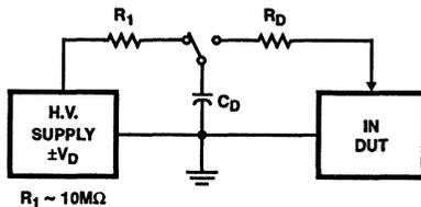
**FIGURE 1. ELECTROSTATIC DISCHARGE TEST
