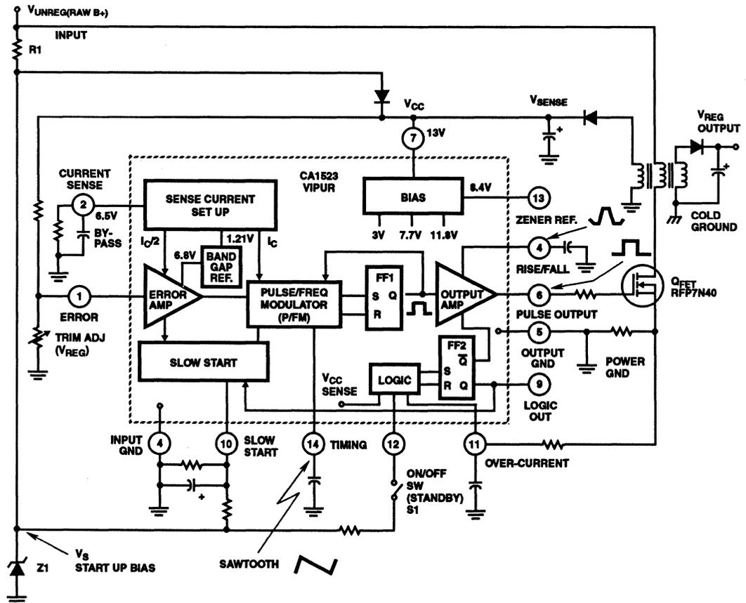
FIGURE 1. BLOCK DIAGRAM OF THE CA1523
