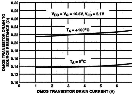
FIGURE 23. TYPICAL DMOS TRANSISTOR DRAIN TO SOURCE RESISTANCE vs DRAIN CURRENT I<sub>DRAIN</sub> AT 0°C AND +100°C
