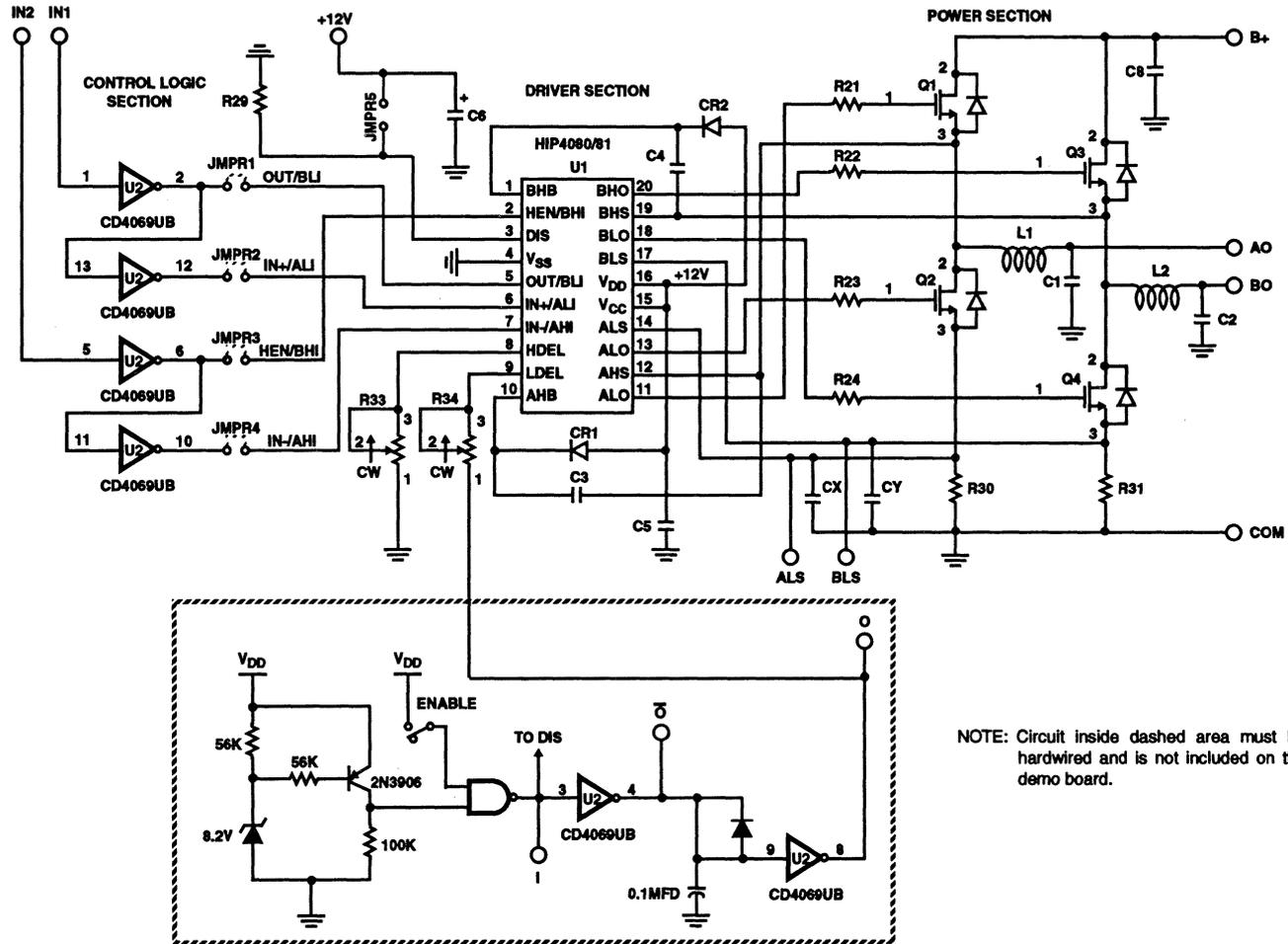
FIGURE 12. HIP4080 EVALUATION PC BOARD SCHEMATIC
