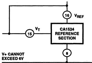
NOTE: V+ Should Be in the 5V Range And Must Not Exceed 6V
