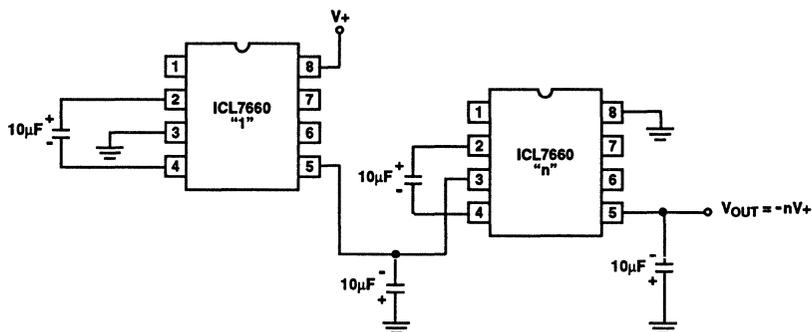
FIGURE 16. CASCADING DEVICES FOR INCREASED OUTPUT VOLTAGE
