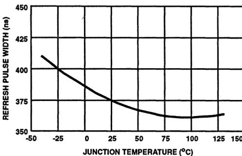
FIGURE 14.  $T_{REF-PW}$  REFRESH PULSE WIDTH vs TEMPERATURE
