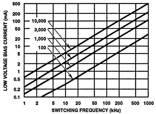
FIGURE 29. LOW VOLTAGE BIAS CURRENT  $I_{DP}$  AND  $I_{CC}$  (LESS QUIESCENT COMPONENT) vs FREQUENCY AND GATE LOAD CAPACITANCE
