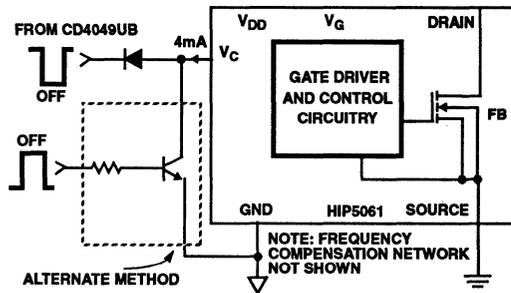
FIGURE 36. TWO METHODS OF SHUTTING DOWN THE HIP5061
