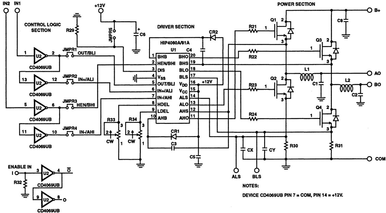
FIGURE 31. HIP4081A EVALUATION PC BOARD SCHEMATIC
