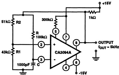
FIGURE 10. ASTABLE MULTIVIBRATOR USING DUAL SUPPLY
