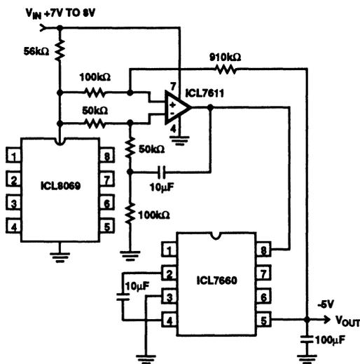
FIGURE 22. REGULATED OUTPUT INVERTER
