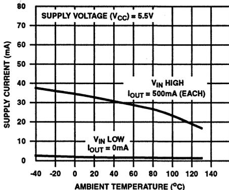
FIGURE 5A. TYPICAL SUPPLY CURRENT (PIN 11) CHARACTERISTICS
