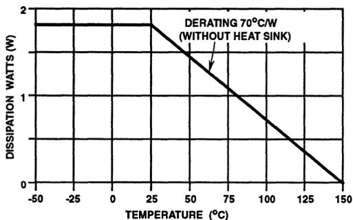
FIGURE 4. DISSIPATION DERATING CURVES
