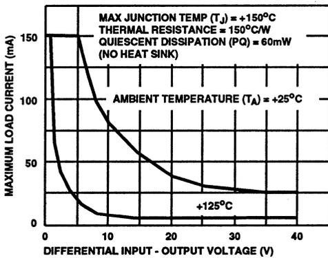
FIGURE 2. MAX LOAD CURRENT vs DIFFERENTIAL INPUT-OUTPUT VOLTAGE
