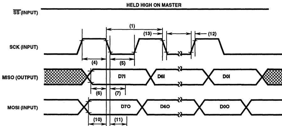
FIGURE 3A. SPI MASTER TIMING CPOL = 0, CPHA = 1
