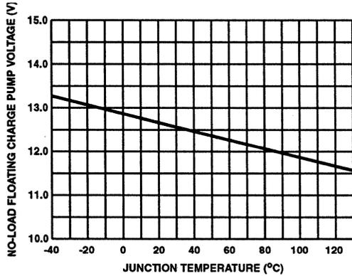
FIGURE 10. AHB - AHS, BHB - BHS NO-LOAD CHARGE PUMP VOLTAGE vs TEMPERATURE
