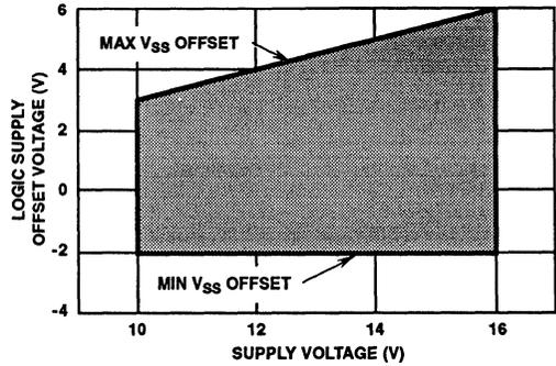
FIGURE 4.  $V_{SS}$  OFFSET vs  $V_{CC}$  SUPPLY VOLTAGE
