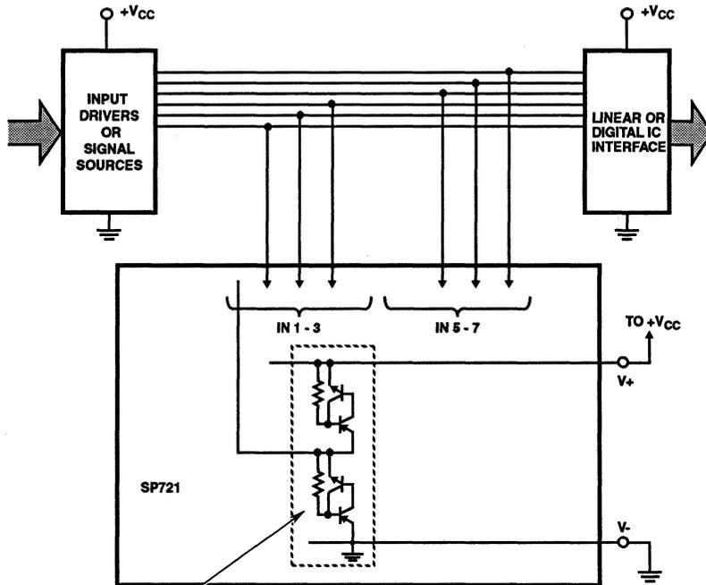
SP721 INPUT PROTECTION CIRCUIT (1 OF 14 ON CHIP)
