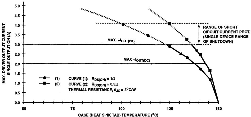
FIGURE 4. HIP0081 MAXIMUM SINGLE OUTPUT CURRENT vs CASE (TAB) TEMPERATURE
