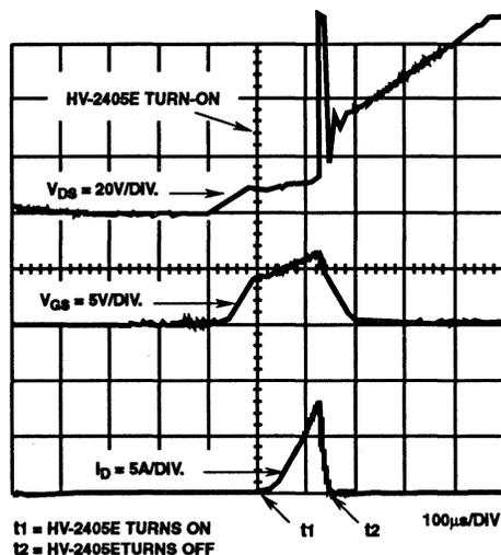
FIGURE 3. TYPICAL WAVEFORMS OF THE MOSFET ( $I_{OUT} = 50mA$ )
