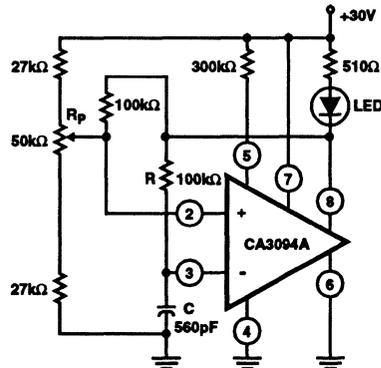
FIGURE 12. ASTABLE POWER MULTIVIBRATOR WITH PROVISIONS FOR VARYING DUTY CYCLE
