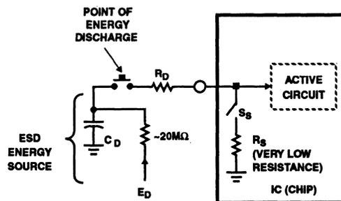
FIGURE 1. ESD TEST FOR AN ON-CHIP PROTECTION CIRCUIT USING THE MIL-STD-883, METHOD 3015.7 (HUMAN BODY MODEL)
