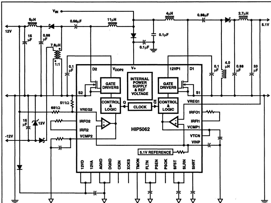
**FIGURE 8. SCHEMATIC DIAGRAM OF THE HIP5062 IN A TRIPLE OUTPUT POWER SUPPLY**
