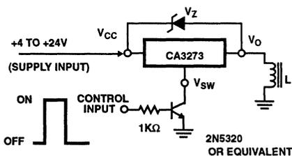
FIGURE 2. TYPICAL APPLICATION WITH ZENER DIODE FOR OVER-VOLTAGE PROTECTION WITH INDUCTIVE LOAD SWITCHING.  $V_z$  SHOULD BE LESS THAN 35V. WHEN CURRENT IS SWITCHED OFF IN THE OUTPUT LOAD (L), THE INDUCTIVE KICK PULSE GOES NEGATIVE. THE CLAMPED CLAMP LEVEL OF THE NEGATIVE GOING PULSE IS  $V_{CC} - V_z$ .
