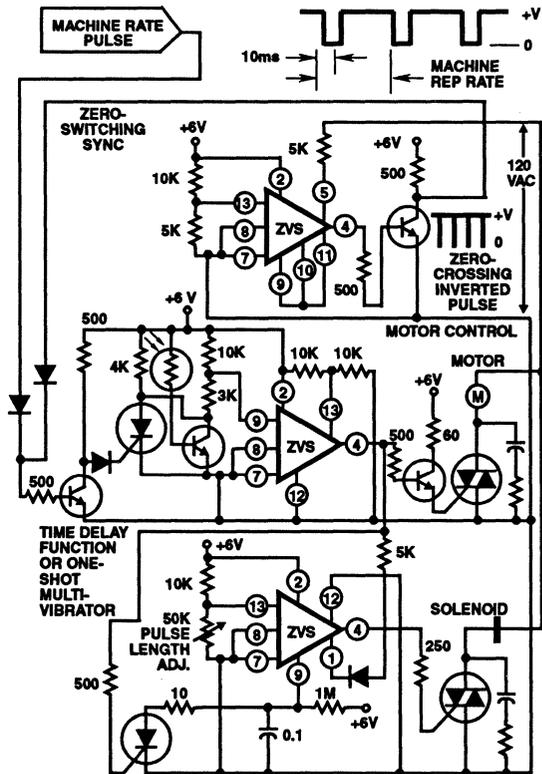
FIGURE 45. SCHEMATIC OF PROPOSED SOLID-STATE MACHINE CONTROL
