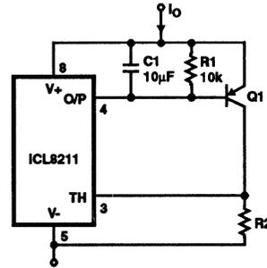
FIGURE 13. PROGRAMMABLE CURRENT SOURCE
