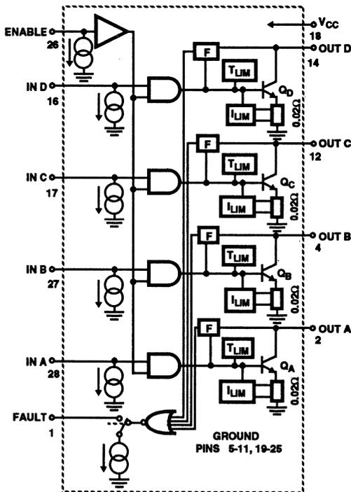
**FIGURE 5. CA3272 AND CA3272A FUNCTIONAL BLOCK DIAGRAM**
