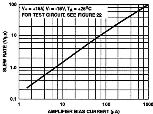
FIGURE 13. SLEW RATE vs AMPLIFIER BIAS CURRENT
