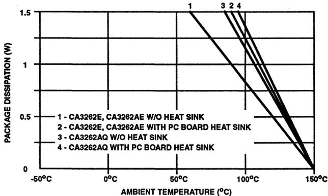
FIGURE 6. PACKAGE DISSIPATION RATING CHART
