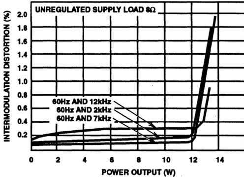
FIGURE 8. INTERMODULATION DISTORTION vs POWER OUTPUT
