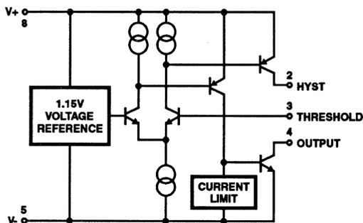
FIGURE 1. ICL8211 FUNCTIONAL DIAGRAM
