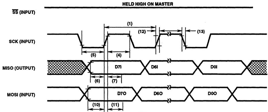
NOTE: Measurement points are  $V_{OL}$ ,  $V_{OH}$ ,  $V_{IL}$  and  $V_{IH}$
