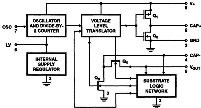
FIGURE 2. FUNCTIONAL DIAGRAM OF COMPLETE CHIP
