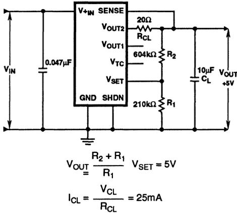
FIGURE 8. POSITIVE REGULATOR WITH CURRENT LIMIT
