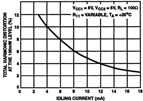
**FIGURE 7. TOTAL HARMONIC DISTORTION AS A FUNCTION OF I<sub>CC2</sub> IDLING CURRENT FOR A SUPPLY VOLTAGE OF 6V AND AN OUTPUT OF 100mW**
