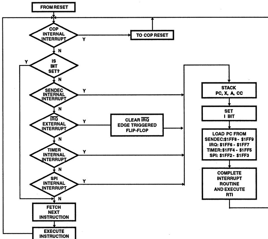
FIGURE 13. HARDWARE INTERRUPT FLOW DIAGRAM
