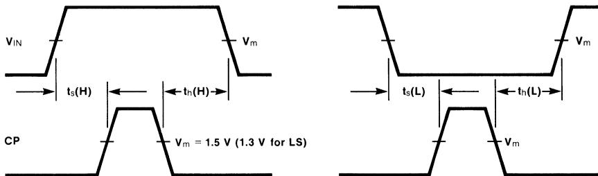
**Fig. 3-18 Setup and Hold Times, Active HIGH Clock**
