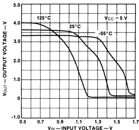
**Fig. 2-20 Voltage Transfer Function of an S-TTL Gate**
