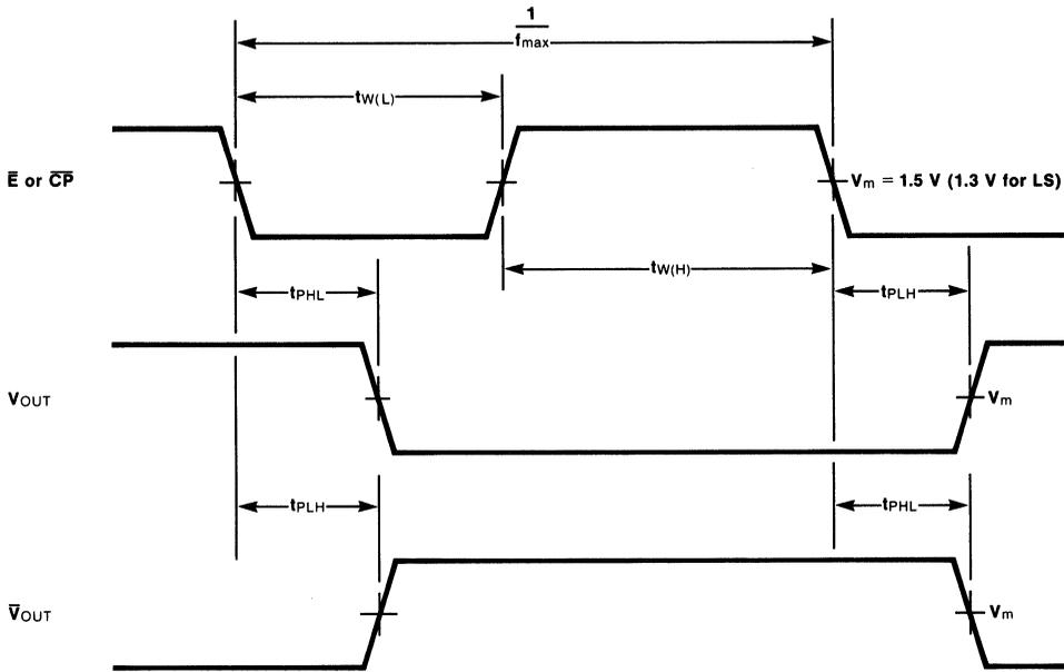
**Fig. 3-9 Propagation Delays from Falling-Edge Clock or Enable**
