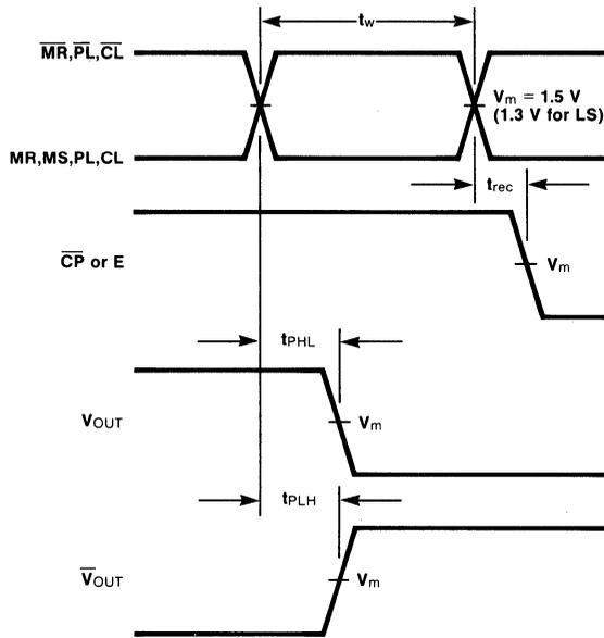
**Fig. 3-17 Asynchronous Set, Reset, Parallel Load or Clear, Active Falling Edge Clock or Active HIGH Enable**
