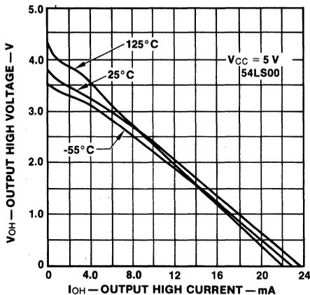
Fig. 2-16 LS-TTL Gate Output HIGH Characteristics
