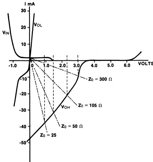
Fig. 2-23 Initial Output Voltage of TTL Driving Transmission Line
