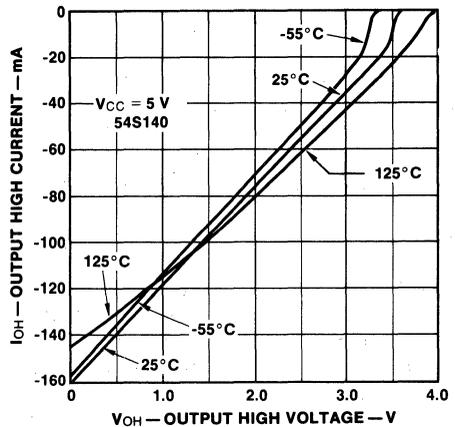
Fig. 2-15 S-TTL Line Driver Output HIGH Characteristics
