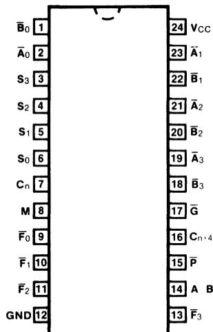
**DESCRIPTION**—The '41 4-bit arithmetic logic units can perform all the possible 16 logic operations on two variables and a variety of arithmetic operations; the Add and Subtract modes are the most important. The '41 is a pin replacement for the 54/74181.
