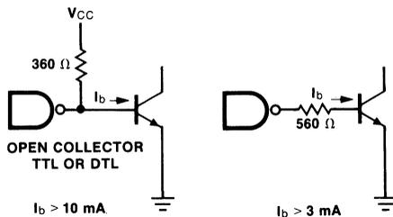
Fig. 2-31 TTL Driving NPN Transistors
