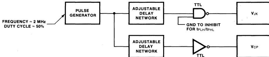
DTL9932 gates with adjustable capacitors connected from extender inputs to ground make suitable delay elements.
