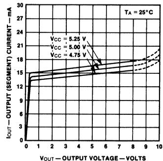
**Fig. b Typical Constant Segment Current Versus Output Voltage**
