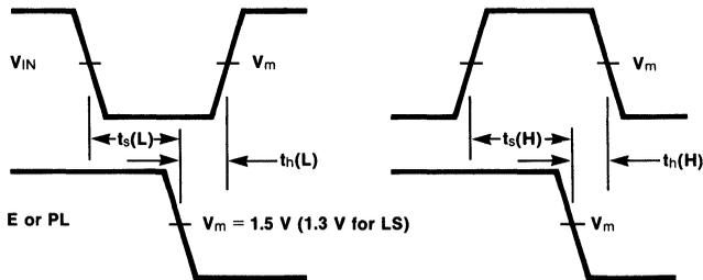
**Fig. 3-14 Setup and Hold Times to Active HIGH Enable or Parallel Load**
