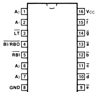
**DESCRIPTION** — The '447 is the same as the '247 except that the Output OFF Voltage,  $V_{OH}$ , is specified as 7.0 V rather than 15 V, with the same  $I_{OH}$  limit of 250  $\mu$ A. For all other information please refer to the '247 data sheet.
