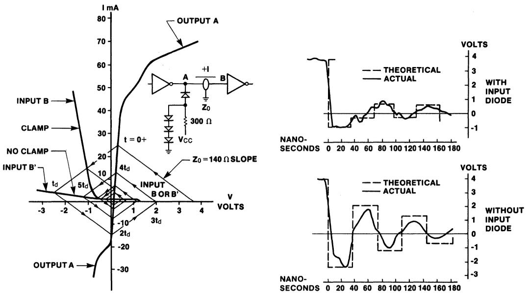
Fig. 2-25 Ringing Caused by Reflections
