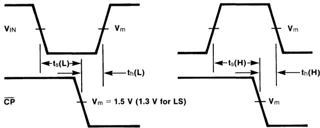
**Fig. 3-7 Set-up and Hold Times, Falling-Edge Clock**
