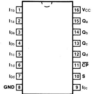
**DESCRIPTION** — The '298 is a quad 2-port register. It is the logical equivalent of a quad 2-input multiplexer followed by a quad 4-bit edge-triggered register. A Common Select input selects between two 4-bit input ports (data sources). The selected data is transferred to the output register synchronous with the HIGH-to-LOW transition of the Clock input.
