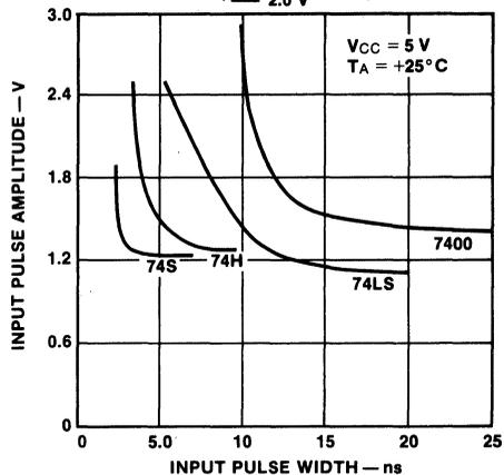
**Fig. 2-22 Pulse Noise Immunity of TTL Gates**
