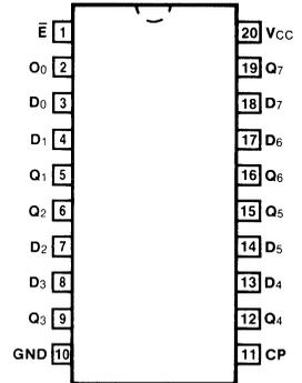
**DESCRIPTION** — The '377 is an 8-bit register built using advanced low power Schottky technology. This register consists of eight D-type flip-flops with a buffered common clock and a buffered common input enable. The device is packaged in the space-saving (0.3 inch row spacing) 20-pin package.
