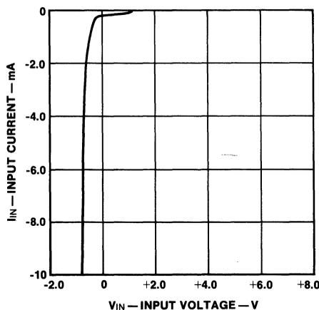
Fig. 2-11 LS-TTL Input Characteristics
