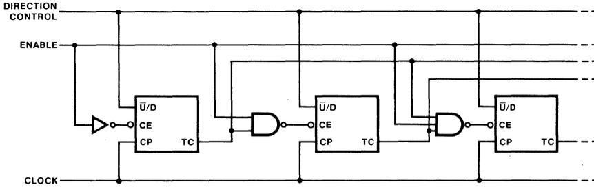
**Fig. c Synchronous N-Stage Counter with Parallel Gated Carry/Borrow**
