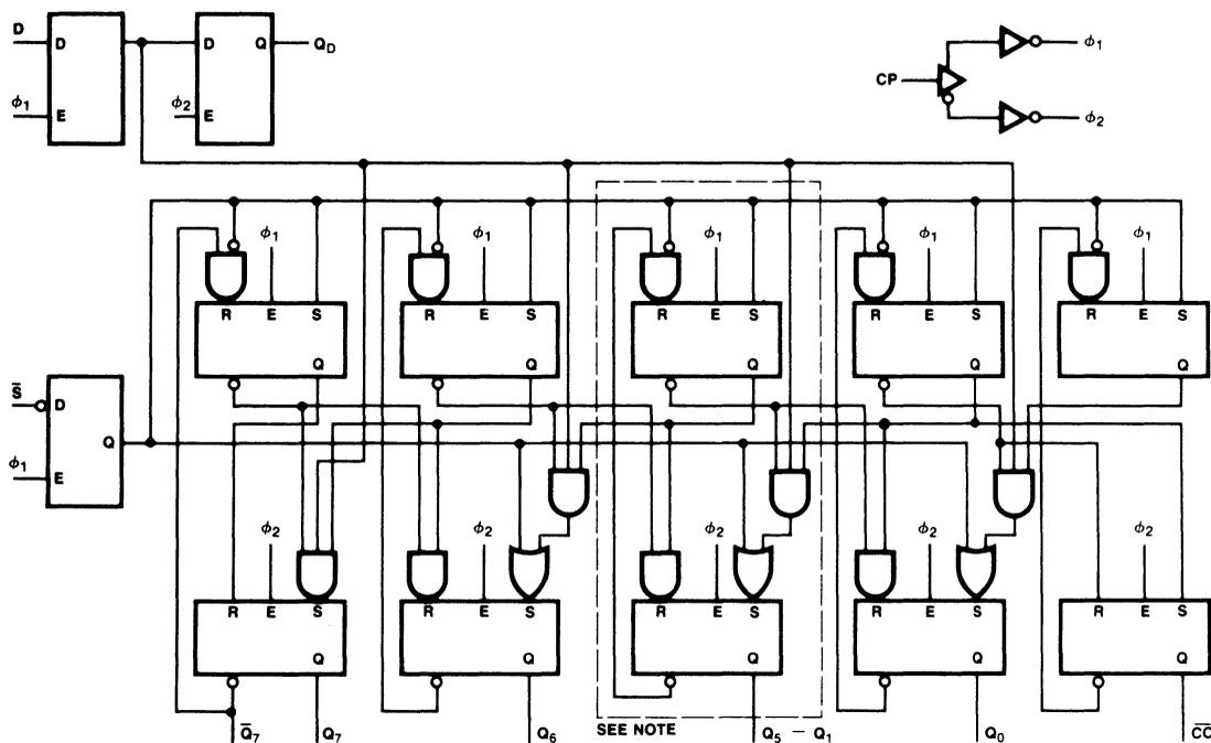
Note: Cell logic is repeated for register stages Q<sub>5</sub> to Q<sub>1</sub>.
