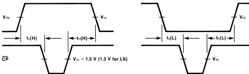
**Fig. 3-19 Setup and Hold Times, Active LOW Clock**
