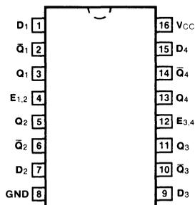
**DESCRIPTION** — The '375 is a 4-bit D-type latch for use as temporary storage for binary information between processing units and input/output or indicator units. When its Enable (E) input is HIGH, a latch is transparent, i.e., the Q output will follow the D input each time it changes. When E is LOW a latch stores the last valid data present on the D input preceding the HIGH-to-LOW transition of E. The '375 is functionally identical to the '75 except for the corner power pins.
