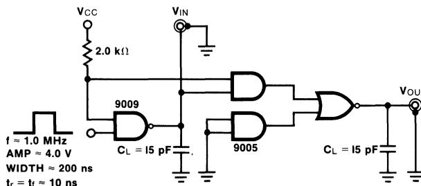
Note: Capacitance includes probe and jig capacitance
