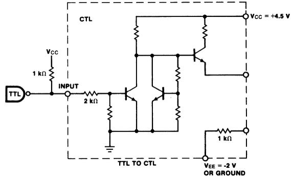
Fig. 2-29 TTL to CTL Conversion
