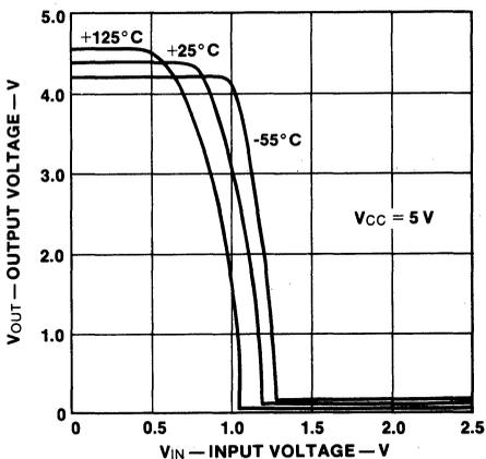
**Fig. 2-21 Voltage Transfer Function of an LS-TTL Gate**
