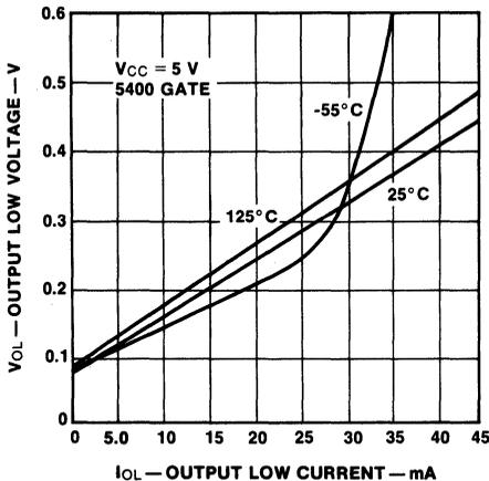
Fig. 2-12 TTL Gate Output LOW Characteristics
