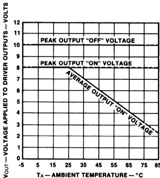
**Fig. a Output Voltage Safe Operating Area**
