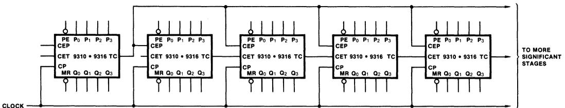
**Fig. b Synchronous Multistage Counting Scheme (Fast)**
