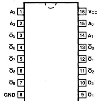
**DESCRIPTION** — The '02 is a multipurpose decoder designed to accept four inputs and provide ten mutually exclusive outputs. The open-collector outputs provide wired-OR capability which can be used for numerous summing, decoding and demultiplexing operations.
