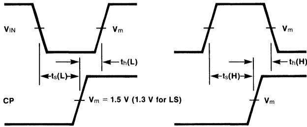
**Fig. 3-6 Set-up and Hold Times, Rising-Edge Clock**
