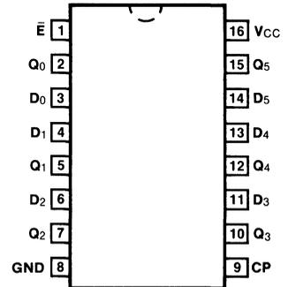
**DESCRIPTION** — The '378 is a 6-bit register with a buffered common enable. This device is similar to the '174, but with common Enable rather than common Master Reset.
