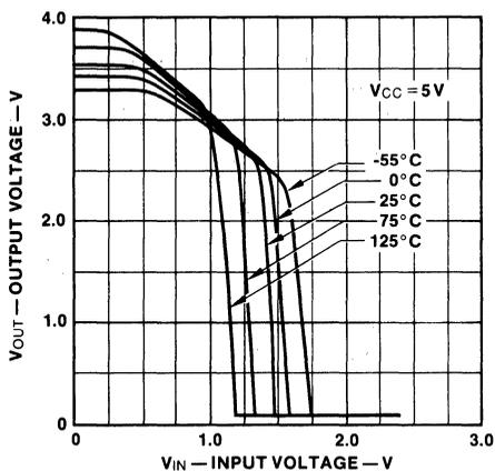
**Fig. 2-19 Voltage Transfer Function of a 9000 Series Gate**
