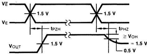
**Fig. 3-12 3-State Output HIGH Enable and Disable Times**
