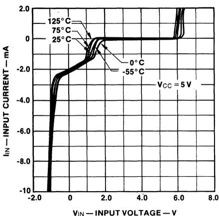
Fig. 2-10 TTL Buffer Input Characteristics
