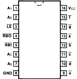
**DESCRIPTION** — The '74 is a 7-segment decoder driver incorporating input latches and output circuits to directly drive common anode LED displays.
