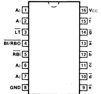
**DESCRIPTION** — The '347 is the same as the '47 except that the Output OFF Voltage,  $V_{OH}$ , is specified as 7.0 V rather than 15 V, with the same  $I_{OH}$  limit of 250  $\mu$ A. For all other information please refer to the '47 data sheet.
