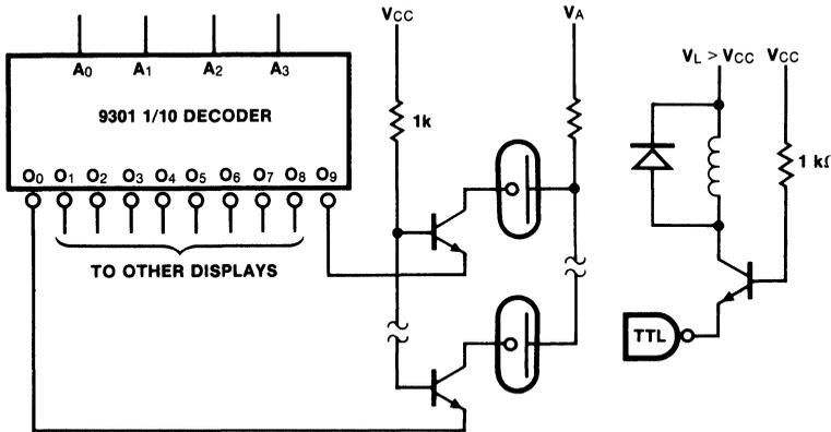
**Fig. 2-33 Non-Inverting High Voltage Drivers**
