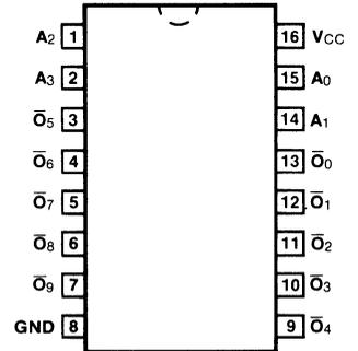
**DESCRIPTION** — The '01 multipurpose decoders are designed to accept four inputs and provide ten mutually exclusive outputs.
