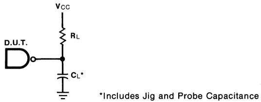
**Fig. 3-2 Test Load for Open-Collector Outputs**
