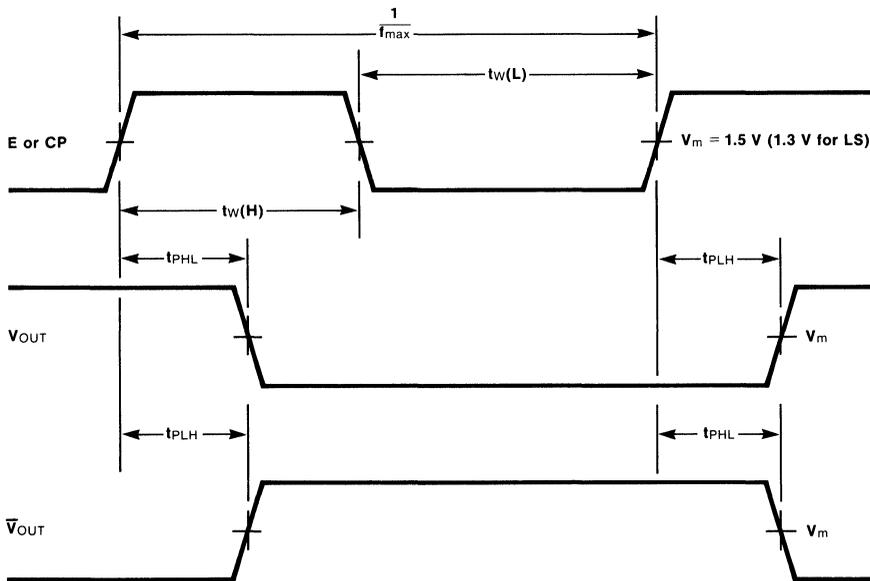
**Fig. 3-8 Propagation Delays from Rising-Edge Clock or Enable**
