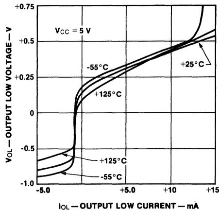
Fig. 2-13 LS-TTL Gate Output LOW Characteristics
