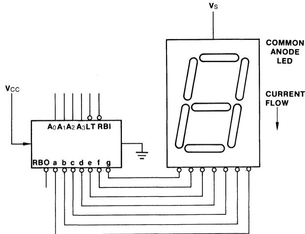
**Fig. c Separate Supply for LED Displays**
