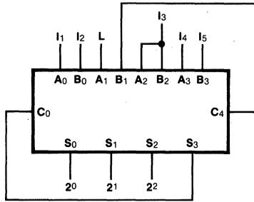
Fig. c 5-Input Encoder
