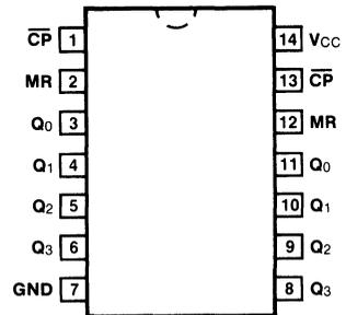
**DESCRIPTION** — The '393 contains a pair of high speed 4-stage ripple counters. Each half of the '393 operates as a modulo-16 binary divider, with the last three stages triggered in a ripple fashion. The flip-flops are triggered by a HIGH-to-LOW transition of their  $\overline{CP}$  inputs. Each half of each circuit type has a Master Reset input which responds to a HIGH signal by forcing all four outputs to the LOW state. For detail specifications, please refer to the '390 data sheet.
