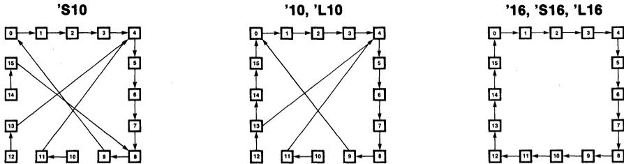
NOTE: The '20 can be preset to any state, but will not count beyond 9. If preset to state 10,11,12,13,14 or 15, it will return to its normal sequence within two clock pulses.
