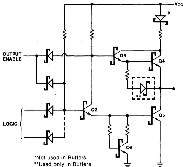
Fig. 2-18 Typical 3-State Output Control
