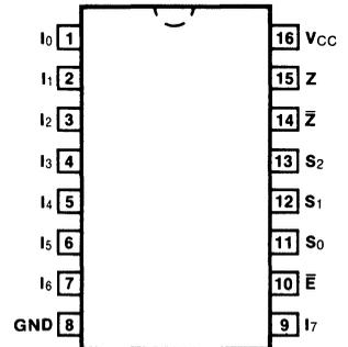
**DESCRIPTION** — The '12 is a monolithic, high speed, 8-input digital multiplexer circuit. It provides, in one package, the ability to select one bit of data from up to eight sources. The '12 can be used as a universal function generator to generate any logic function of four variables. Both assertion and negation outputs are provided.
