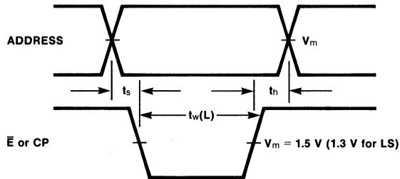
**Fig. 3-21** Storage Address Setup and Hold Times
