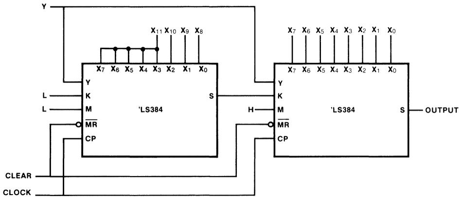
Fig. c A 12-Bit by N-Bit Two's Complement Multiplier
