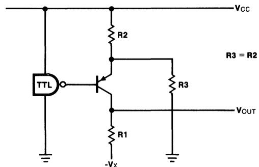
Fig. 2-32 PNP Transistor Shifting TTL Output
