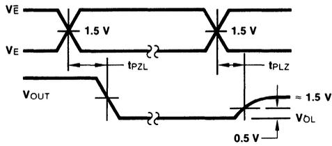
**Fig. 3-11 3-State Output LOW Enable and Disable Times**
