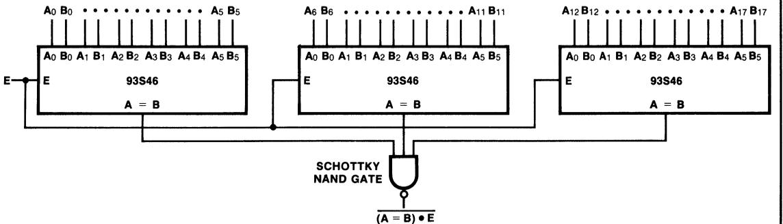
NOTE: This method of expansion adds one gate delay (≈3 ns) to the '46, independent of the word length that is compared.
