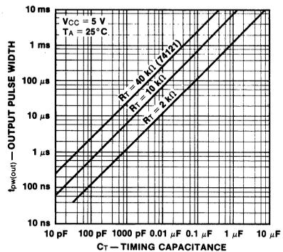
Fig. i Output Pulse Width Versus External Capacitance
