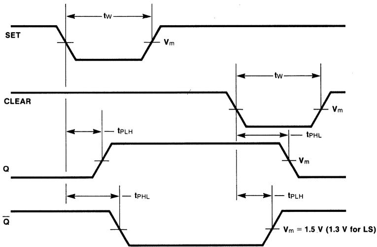
**Fig. 3-10 Propagation Delays from Set and Clear (or Reset)**
