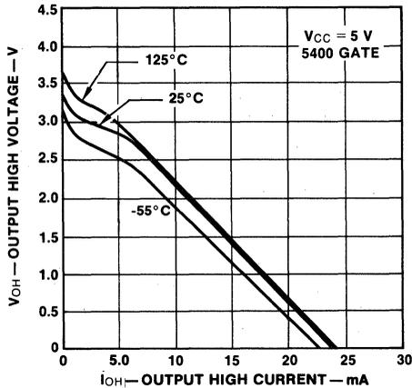
Fig. 2-14 TTL Output HIGH Characteristics
