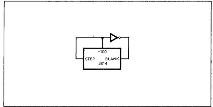
Fig. 11. Self-driven multiplexer with blanking between digits.
