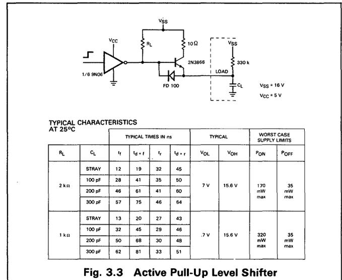
**Fig. 3.3 Active Pull-Up Level Shifter**
