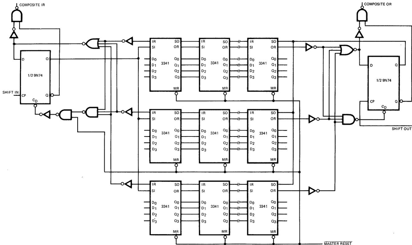
NOTE: Composite Shift In should be LOW when Master Reset goes HIGH. Input data may be changed after Composite IR goes LOW. Composite IR will not go HIGH until Composite Shift In goes LOW. When Composite IR goes HIGH FIFO's will accept new data. 3341's will operate at their highest natural speeds if these rules are followed.
