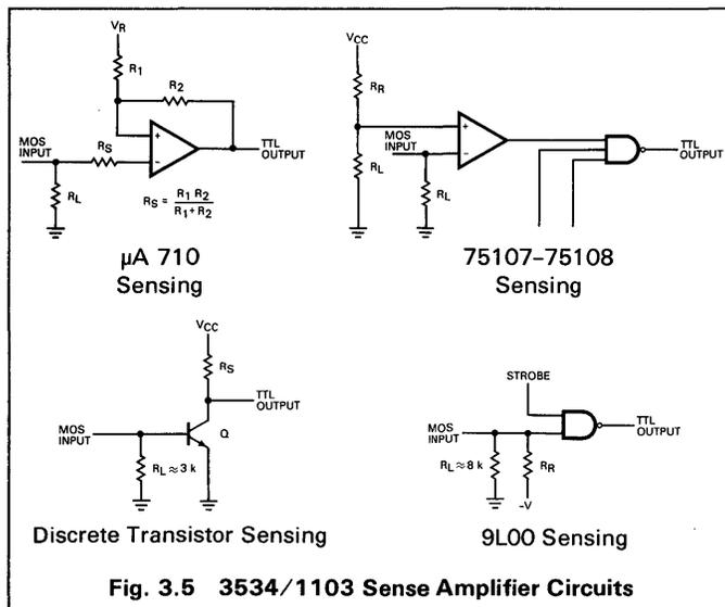
Fig. 3.5 3534/1103 Sense Amplifier Circuits
