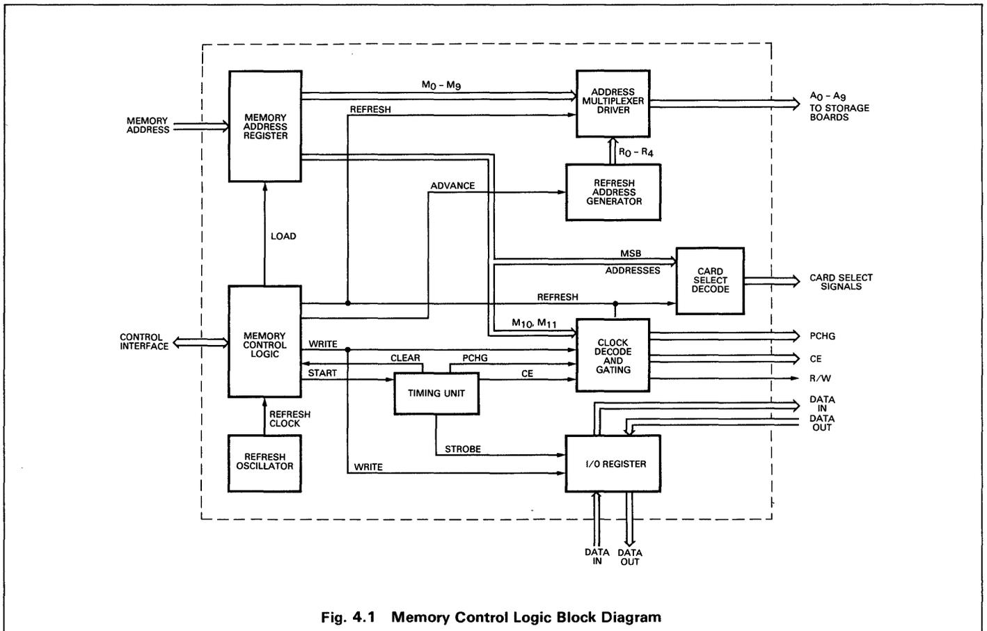
Fig. 4.1 Memory Control Logic Block Diagram
