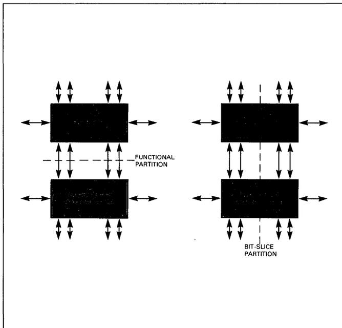
Figure 4. Bit Slice and Functional Partitioning
