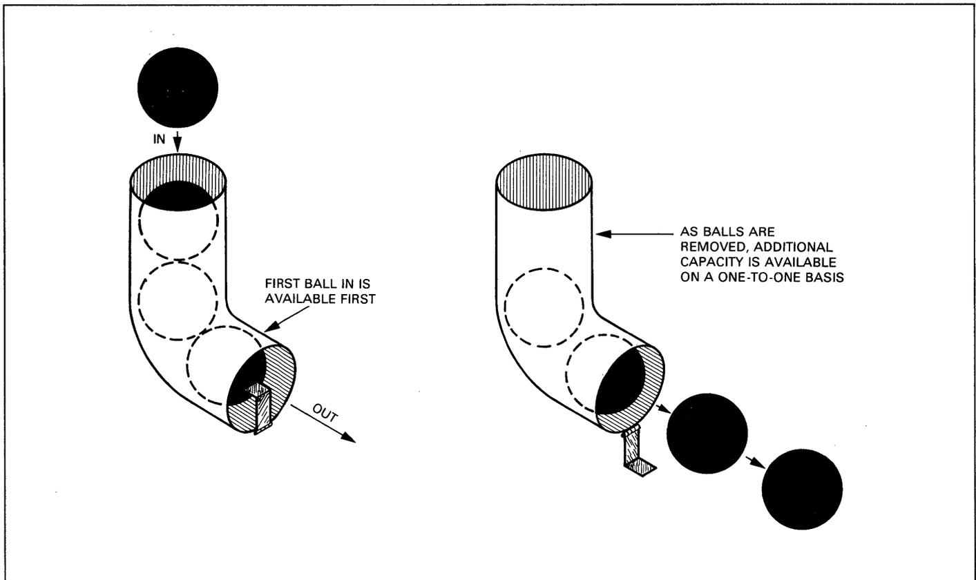
Figure 1. The FIFO Principle, First Input In is Available First
