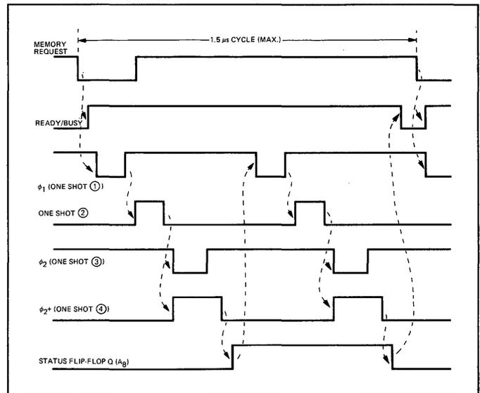
Fig. 6 Memory Internal Timing 256x8
