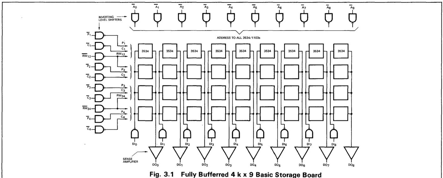
Fig. 3.1 Fully Buffered 4 k x 9 Basic Storage Board
