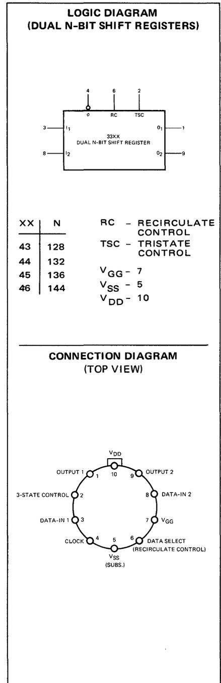
**DC CHARACTERISTICS:**  $V_{SS} = +5.0\text{ V} \pm 5\%$ ,  $V_{DD} = 0\text{ V}$ ,  $V_{GG} = -12.0\text{ V} \pm 5\%$ ,  $T_A = 0^\circ\text{C}$  to  $+70^\circ\text{C}$
