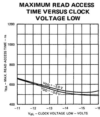
(35322) AC CHARACTERISTICS:  $V_{SS} = +5.0 \text{ V} \pm 5\%$ ,  $V_{DD} = -3 \text{ V} \pm 10\%$ ,  $T_A = 0^\circ\text{C to } 75^\circ\text{C}$  (Cont'd)
