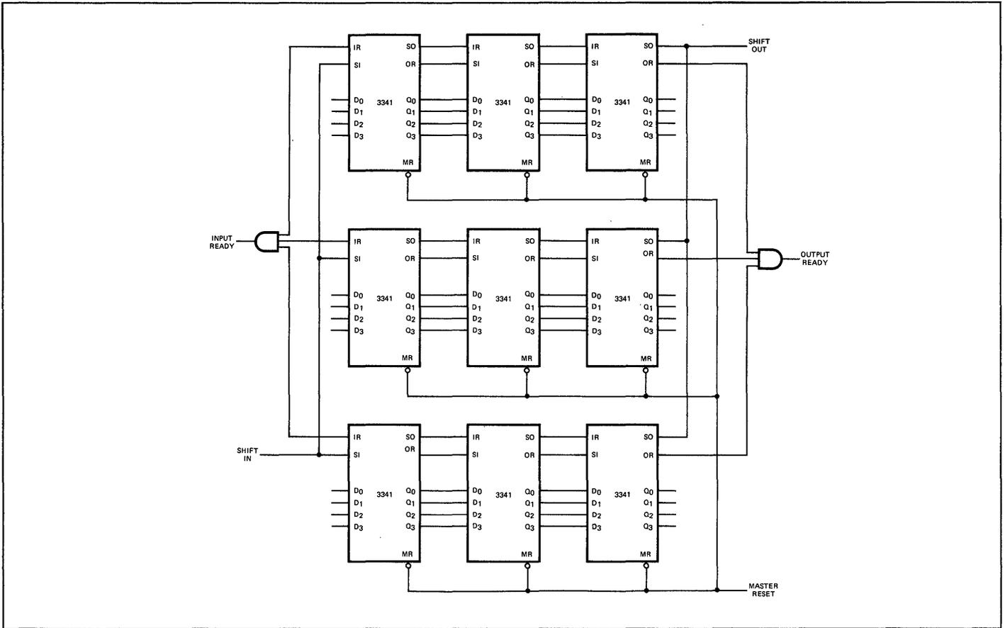
Figure 8. Serial and Parallel Expansion of the 3341 FIFO
