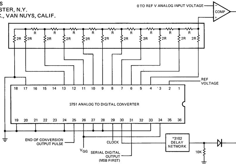
When the serial digital output is used, a delay network is required between the comparator output and the converter as shown. This is to inhibit any change of the comparator return signal at the input of the converter during a clock pulse.
