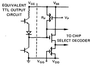
R<sub>p</sub> is enabled if V<sub>p</sub> = V<sub>GG</sub>, disabled if V<sub>p</sub> = V<sub>SS</sub>.
