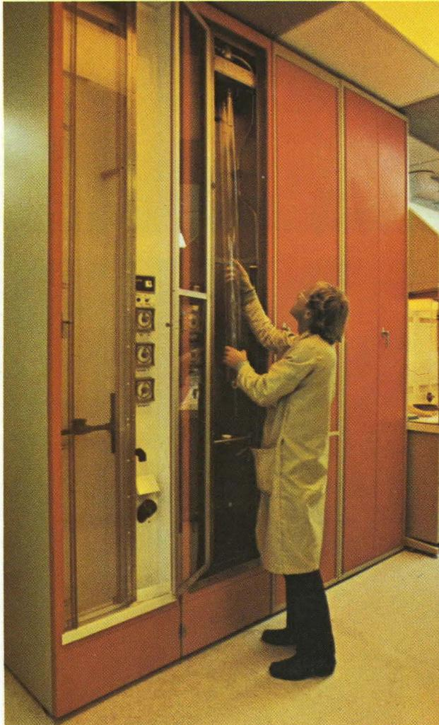
The diffusion furnace tubes are regularly cleaned by flushing with HF (hydrofluoric acid), rinsed with DI water and dried with N<sub>2</sub>.
