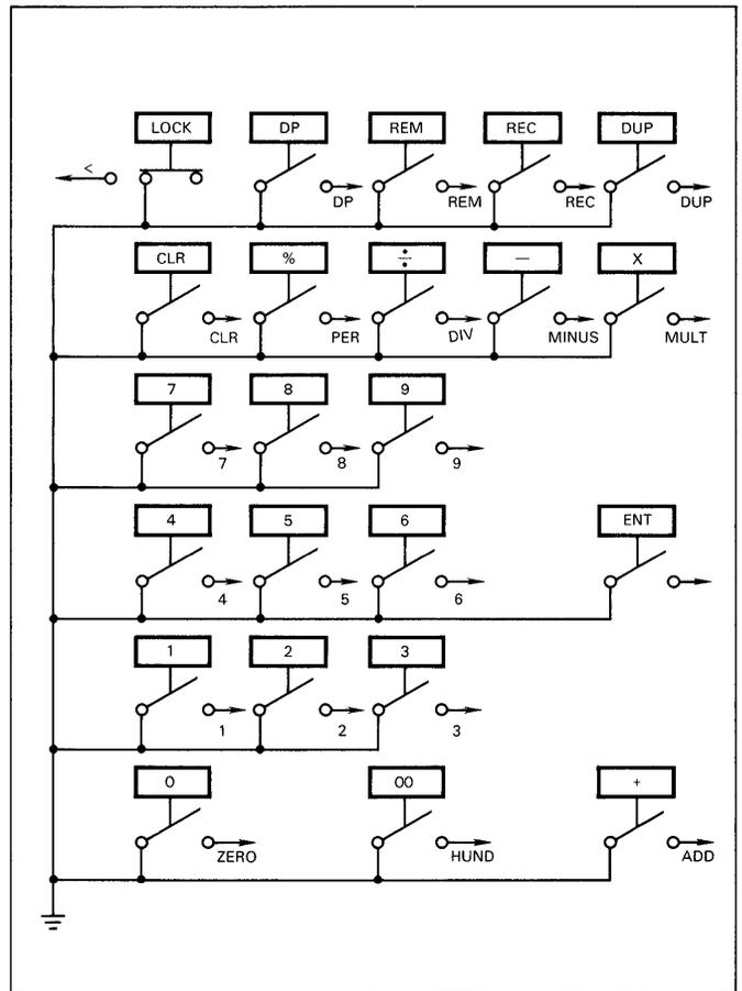
Fig. C-3. Keyboard Switch Schematic Single Pole Single Throw Switches
