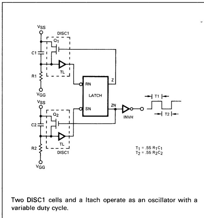
Fig. D-28. DISC2 as Oscillator
