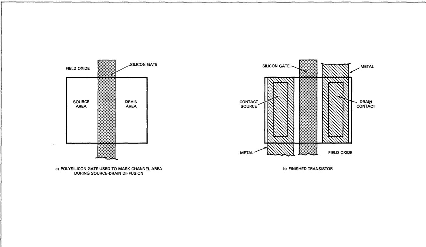
Fig. G-1. Top Views of a Silicon Gate MOS Transistor before and after Diffusion and Metallization
