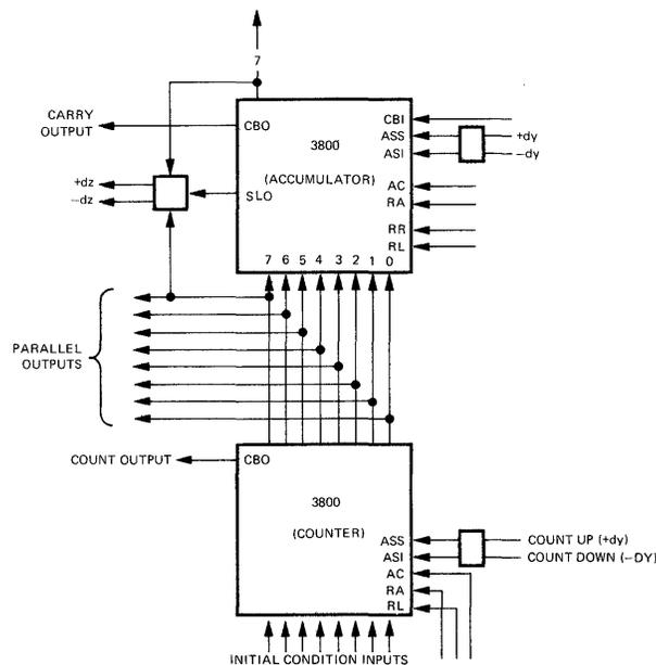
The DDA shown above utilizes one 3800 for a remainder register and a second 3800 for a y accumulator counter.
