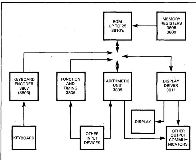
Fig. B-1. PPS-25 Micro-Programmed Processor System
