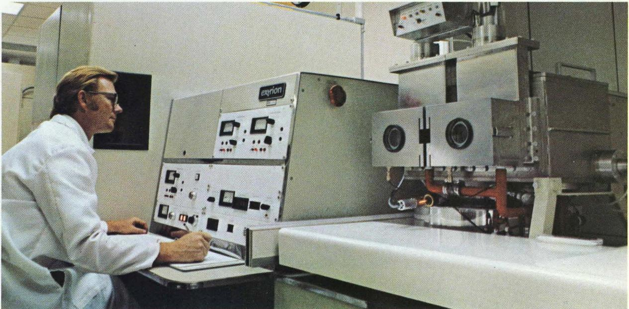
Ion implantation equipment installed in production diffusion room for use with Isoplanar to provide superior density and performance.
