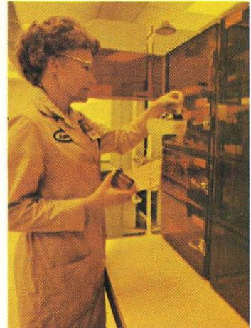
The exposed wafers are developed in the right-hand station. A rinse removes the unexposed etch resist exposing the surface for future chemical action. The center station is an in-process inspection station. The light-filtered box in the foreground stores exposed wafers until they are developed.
