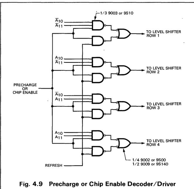
Fig. 4.9 Precharge or Chip Enable Decoder/Driver
