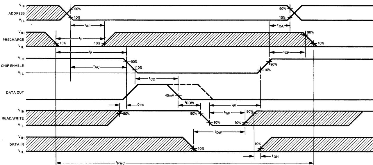
Fig. 1.8 3534 Read/Write Cycle
