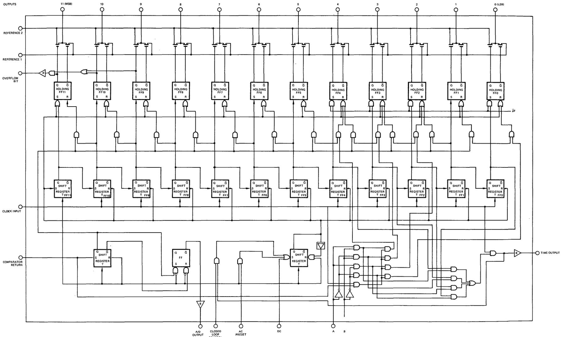
NOTE: Polarity indicators (0) external to the solid box conform to MIL-STD-806B where 0 indicates the less positive state is active. Internal to the box and in the remainder of this data sheet conventional MOS polarities are used, where HI = "1"  $\approx$  -10 V and 1.0 = "0"  $\approx$  Gnd.
