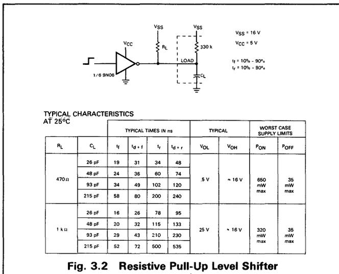
**Fig. 3.2 Resistive Pull-Up Level Shifter**
