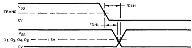
Fig. 4. Propagation delay-BCD outputs
