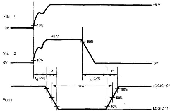
V<sub>IN1</sub>: RC INPUT NETWORK DETERMINES t<sub>pw</sub>. ALL PARAMETERS APPLICABLE EXCEPT t<sub>d</sub> off.
