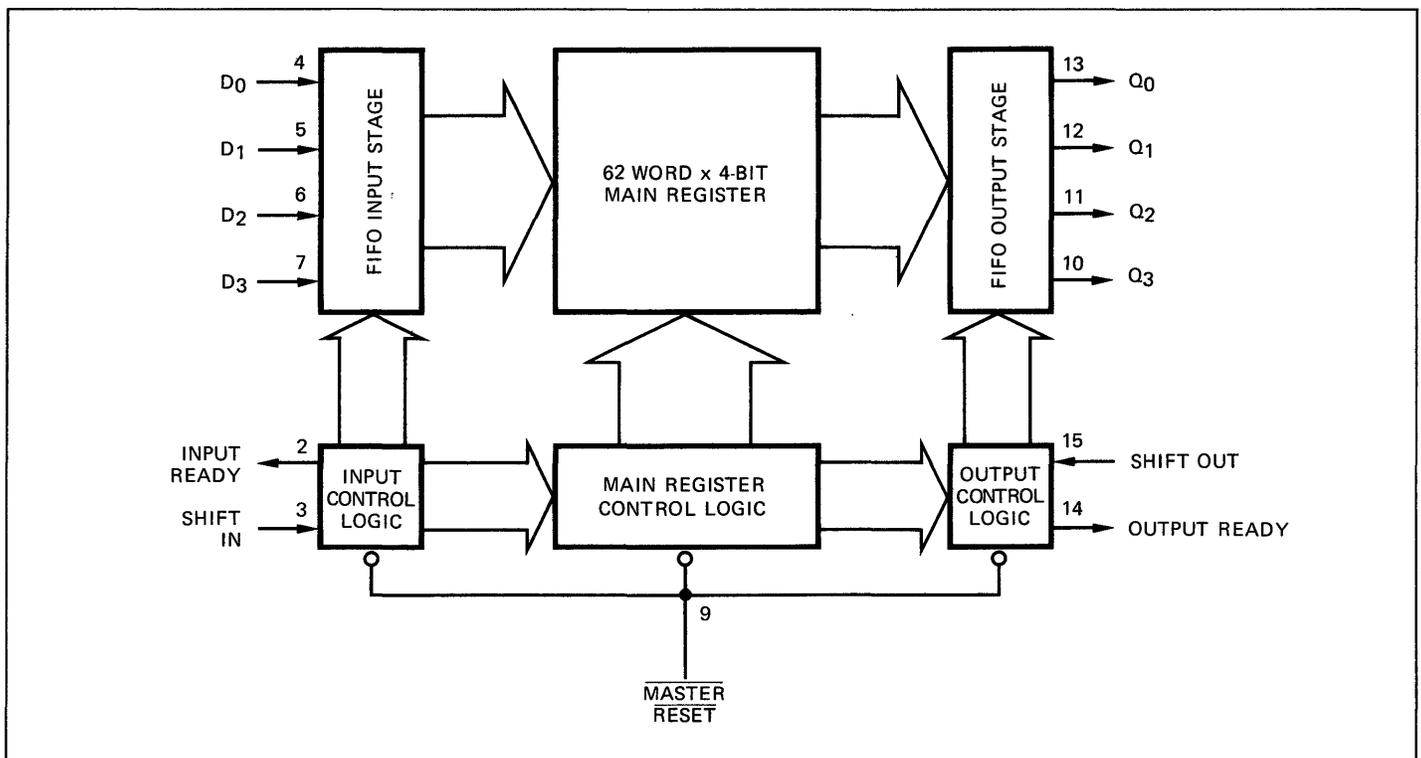
Figure 3. The 3341 Logic Block Diagram
