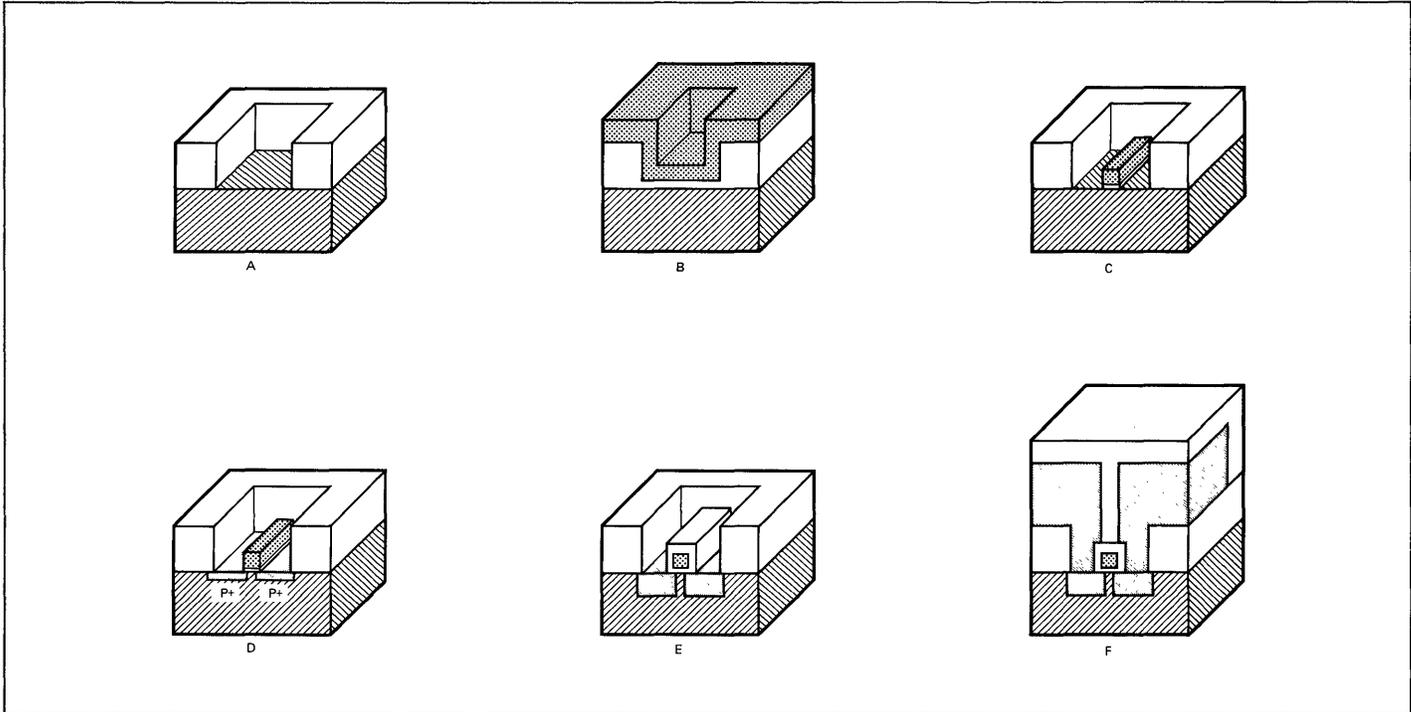
Fig. G-2. Silicon Gate Process Steps
