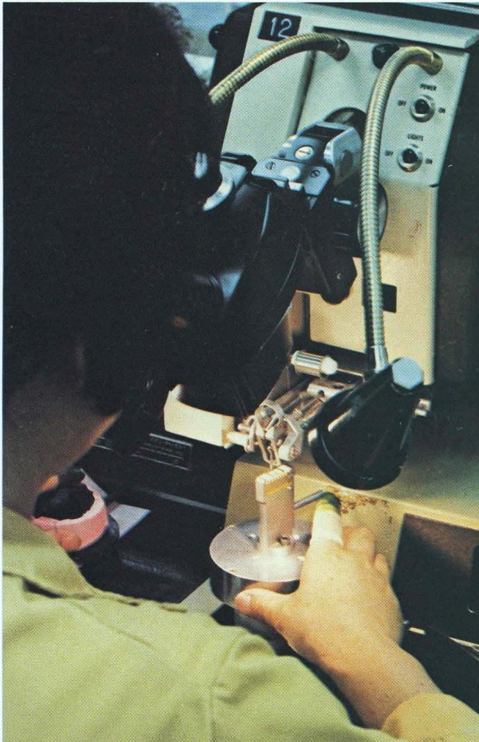
Wire bonding connects the pads on the die to the leads of the package.
