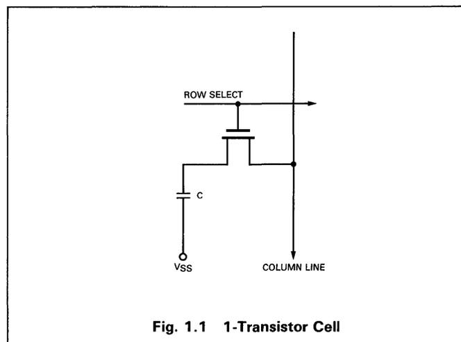
Fig. 1.1 1-Transistor Cell
