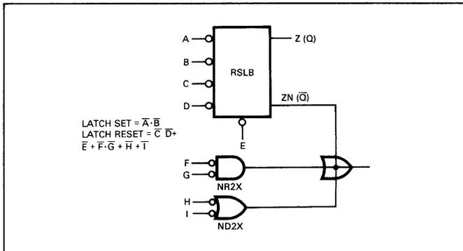
Fig. D-23. Latch Control With Expanders
