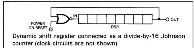
Fig. D-30. Shift Register Counter
