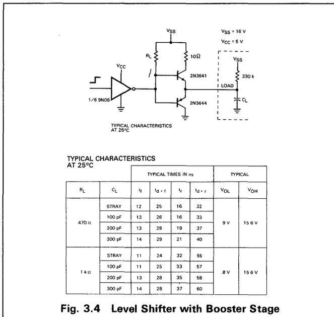
Fig. 3.4 Level Shifter with Booster Stage
