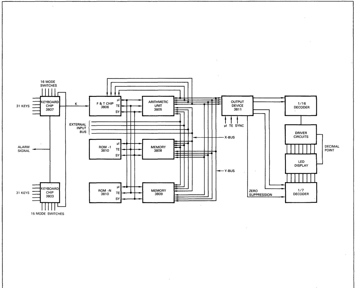
Fig. B-2. Typical Processor System
