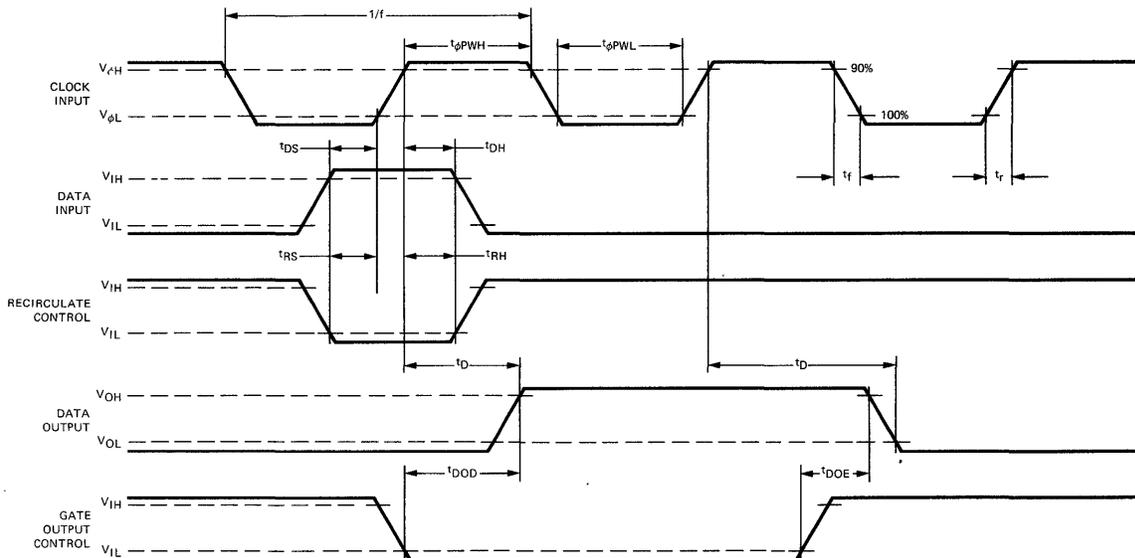
Fig. 1. 3348/3349 I/O TIMING DIAGRAM AND VOLTAGE WAVEFORMS
