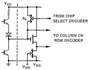
R<sub>p</sub> is enabled if the input pull up option is chosen and if chip is selected.
