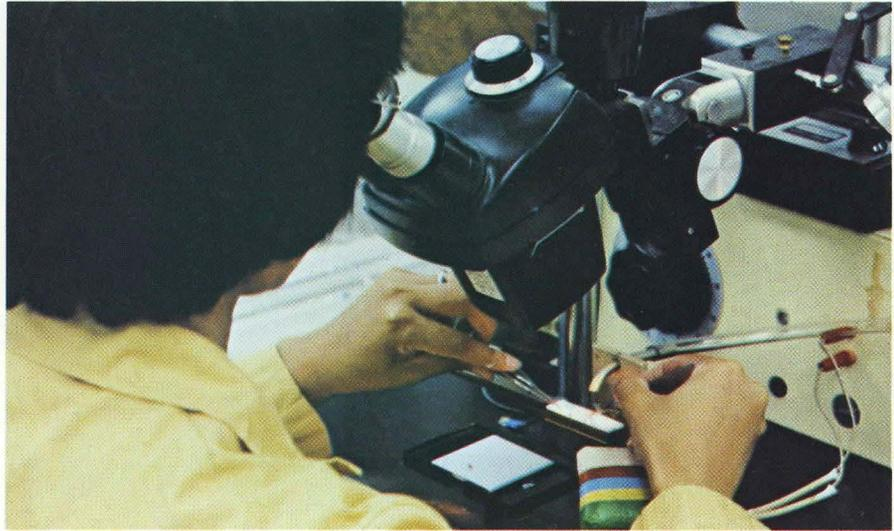
Die bonding welds acceptable dice into a package for interconnection purposes.
