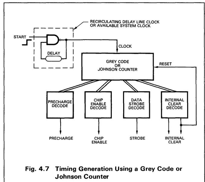
Fig. 4.7 Timing Generation Using a Grey Code or Johnson Counter
