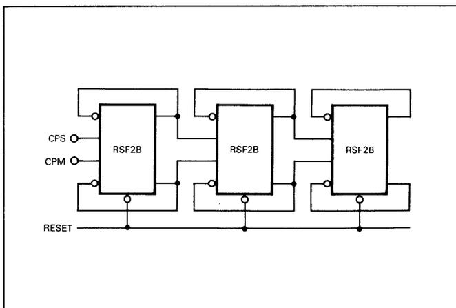
Fig. D-24. HIGH-Level Reset With Inverters
