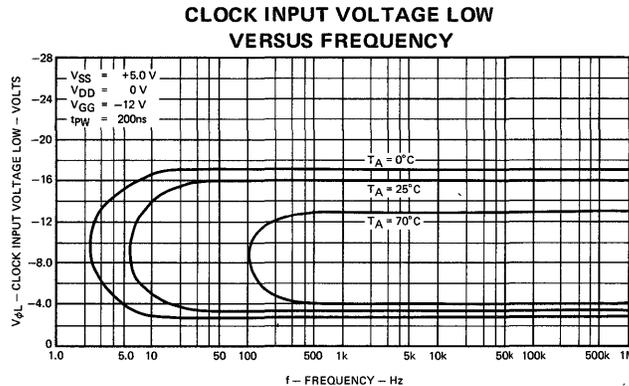
AC CHARACTERISTICS:  $V_{SS} = +5.0 \text{ V} \pm 10\%$ ,  $V_{DD} = 0 \text{ V}$ ,  $V_{GG} = -12.0 \text{ V} \pm 10\%$ ,  $T_A = 0^\circ\text{C to } +70^\circ\text{C}$
