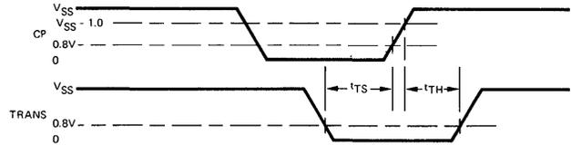
Fig. 2. Transfer setup and hold times
