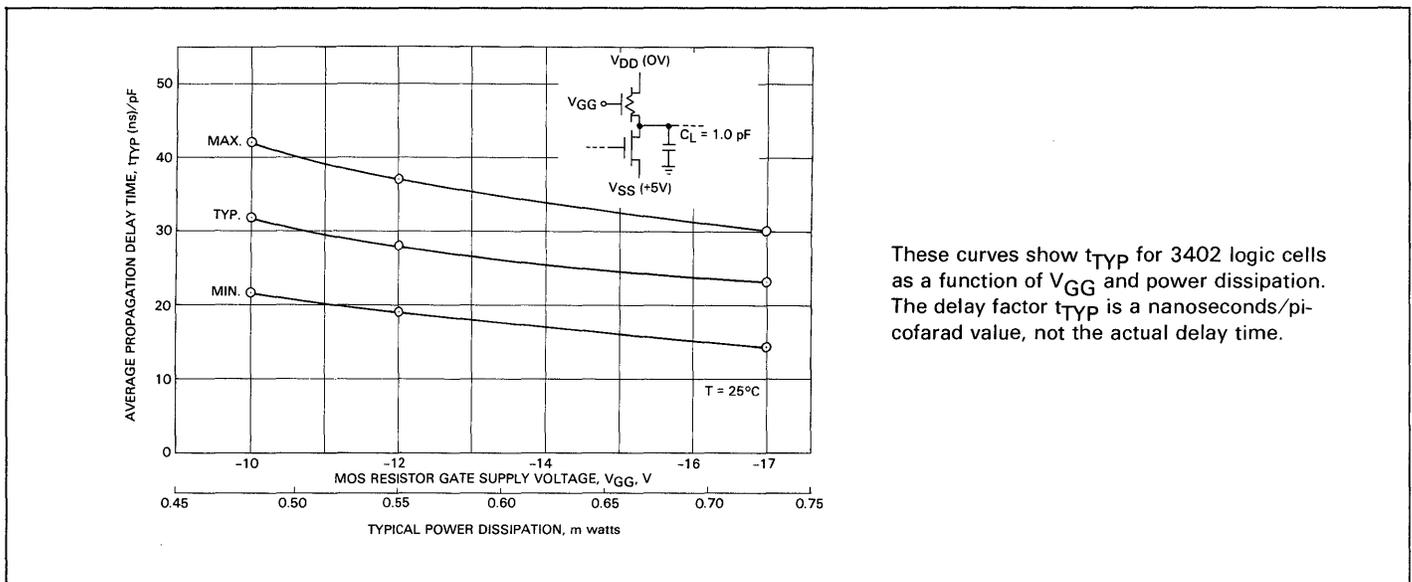
These curves show  $t_{TYP}$  for 3402 logic cells as a function of  $V_{GG}$  and power dissipation. The delay factor  $t_{TYP}$  is a nanoseconds/picofarad value, not the actual delay time.
