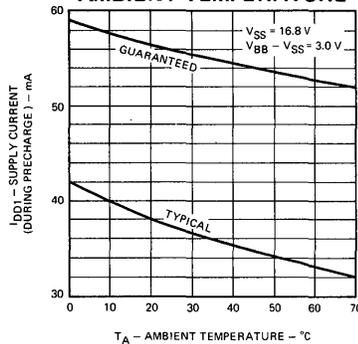
Fig. 2 SUPPLY CURRENT DURING OVERLAP VERSUS AMBIENT TEMPERATURE
