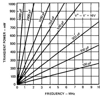
**Fig. 13 TRANSIENT POWER VERSUS FREQUENCY FOR 20 VOLT SUPPLY DIFFERENCE**
