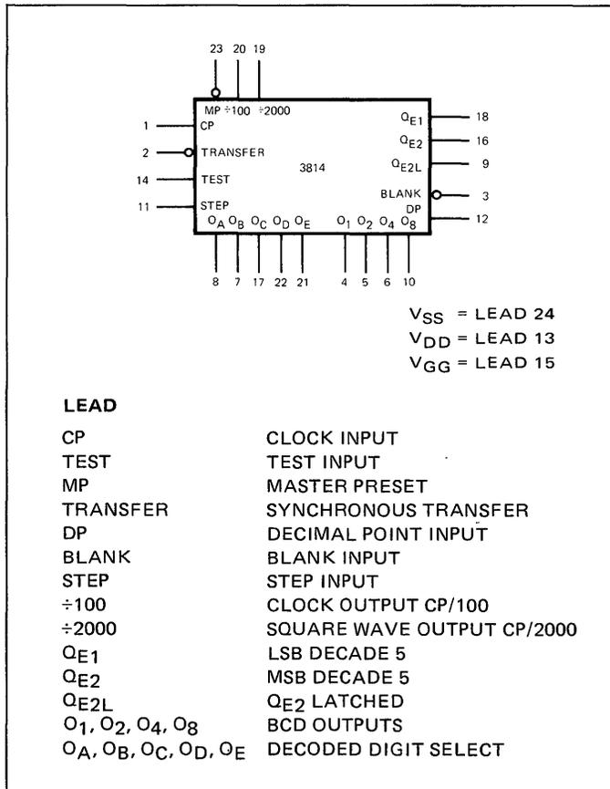
Fig. 1. Logic symbol and lead designation.
