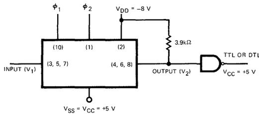
Clock amplitude  $V_{\phi} = +5 \text{ V to } -19 \text{ V}$ .
