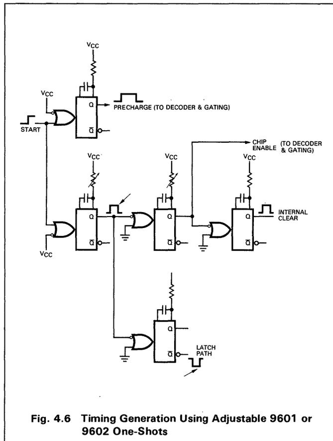
Fig. 4.6 Timing Generation Using Adjustable 9601 or 9602 One-Shots
