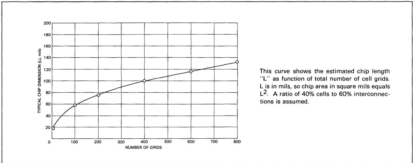
This curve shows the estimated chip length "L" as function of total number of cell grids. L is in mils, so chip area in square mils equals  $L^2$ . A ratio of 40% cells to 60% interconnections is assumed.
