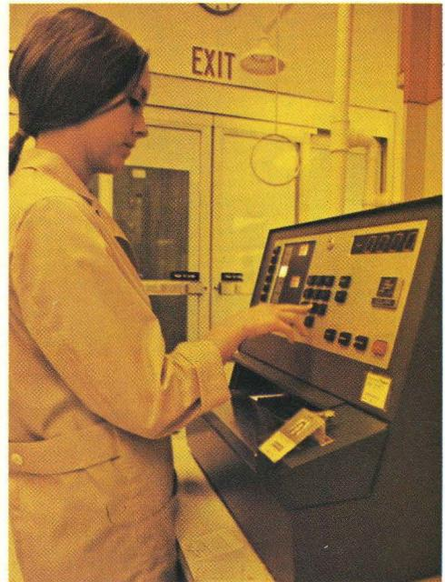
In these mask aligners, new mask patterns (from working plate) are aligned to the existing pattern on the wafer. A box of working plates is shown in foreground.
