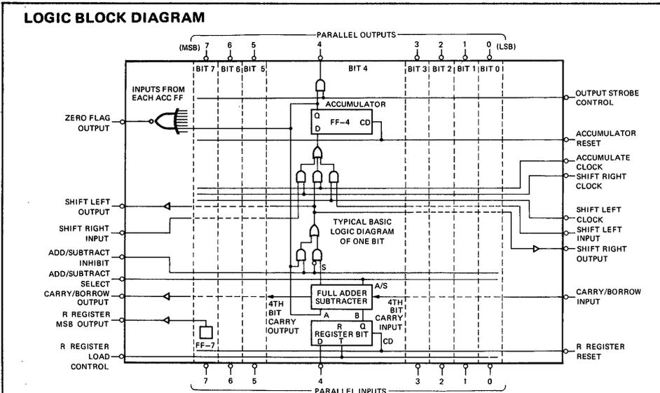
**NOTE:** Polarity indicators (○) external to the solid box conform to MIL-STD-806B where 0 indicates the less positive state is active. Internal to the box conventional MOS polarities are used, where "1"  $\approx$  -10 V and "0"  $\approx$  GND.
