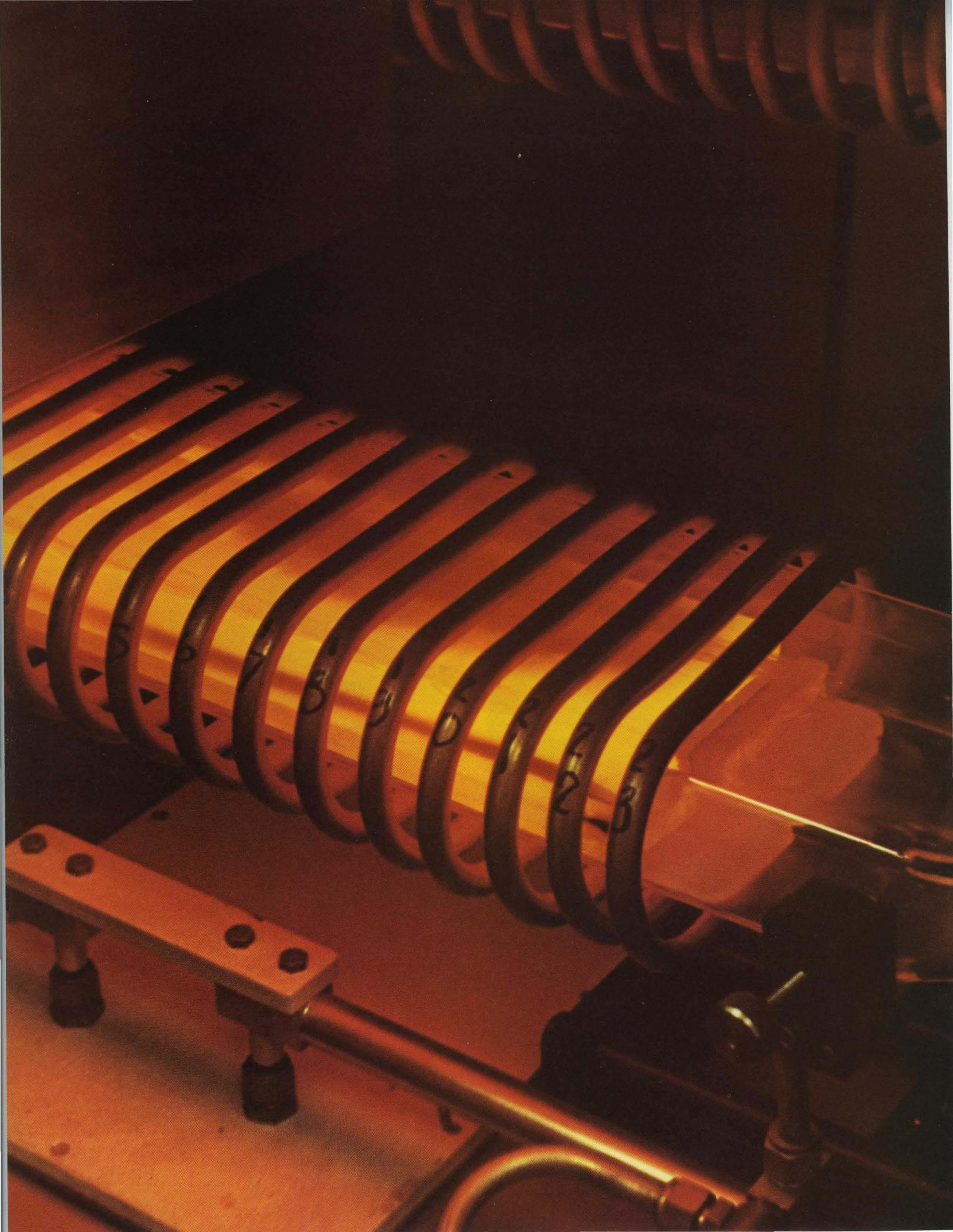
Wafers are loaded into a silicon reactor which deposits polysilicon metal in the gate and interconnection areas.
