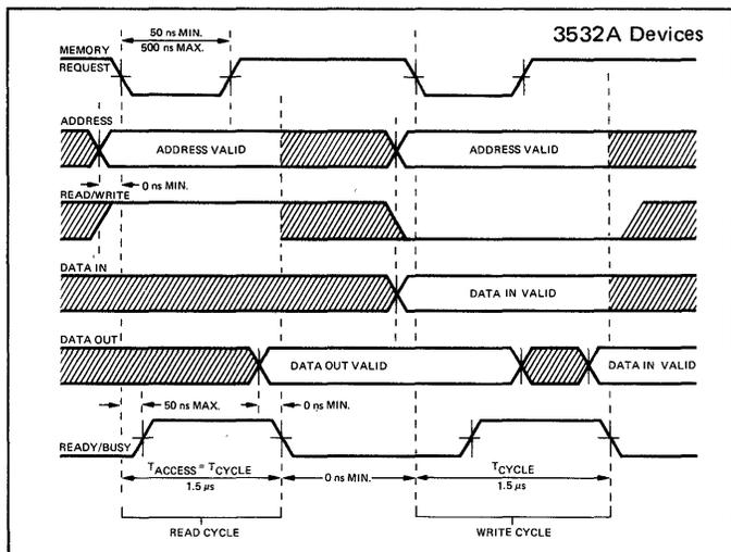
Fig. 5 Memory Interface Timing 256x8
