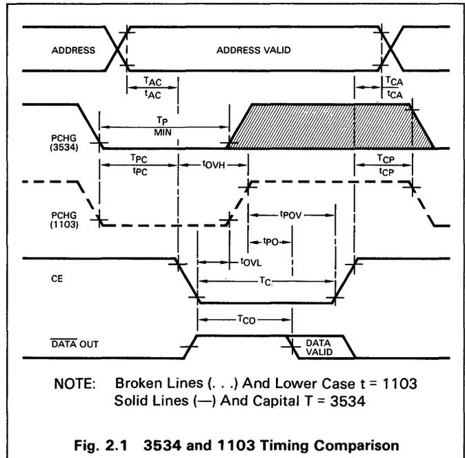
The elimination of overlap constraints provides another important system benefit, illustrated by the relationship between the leading edge of CE and valid DATA OUT. Data is available T<sub>CO</sub> (165 ns max) after CE on the 3534 and is not referenced to the trailing (positive-going) edge of PCHG as in the 1103. At the system level, this eliminates the clock skew associated with the rising edge of PCHG, providing faster access and cycle times in a worst case design.
