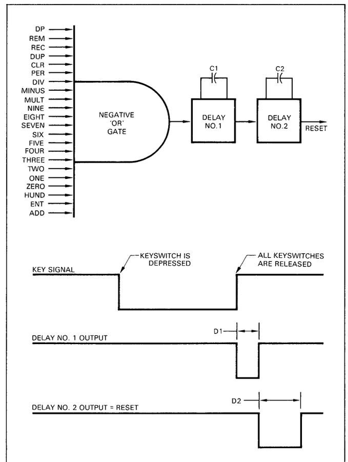
Fig. C-4. Logic Required for Single Pole Single Throw Switches
