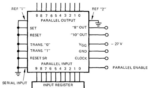
SERIAL TO SERIAL BUFFER REGISTER
