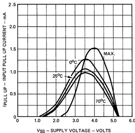
Figure 4. Input Characteristics of the 3341
