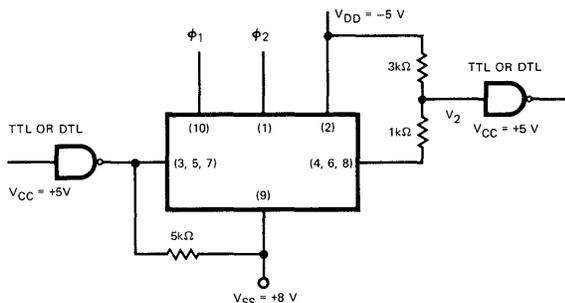
Clock amplitude  $V_{\phi} = +8 \text{ V to } -16 \text{ V}$ .
