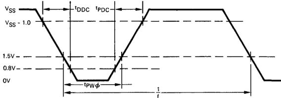
Fig. 1. Input clock waveform
