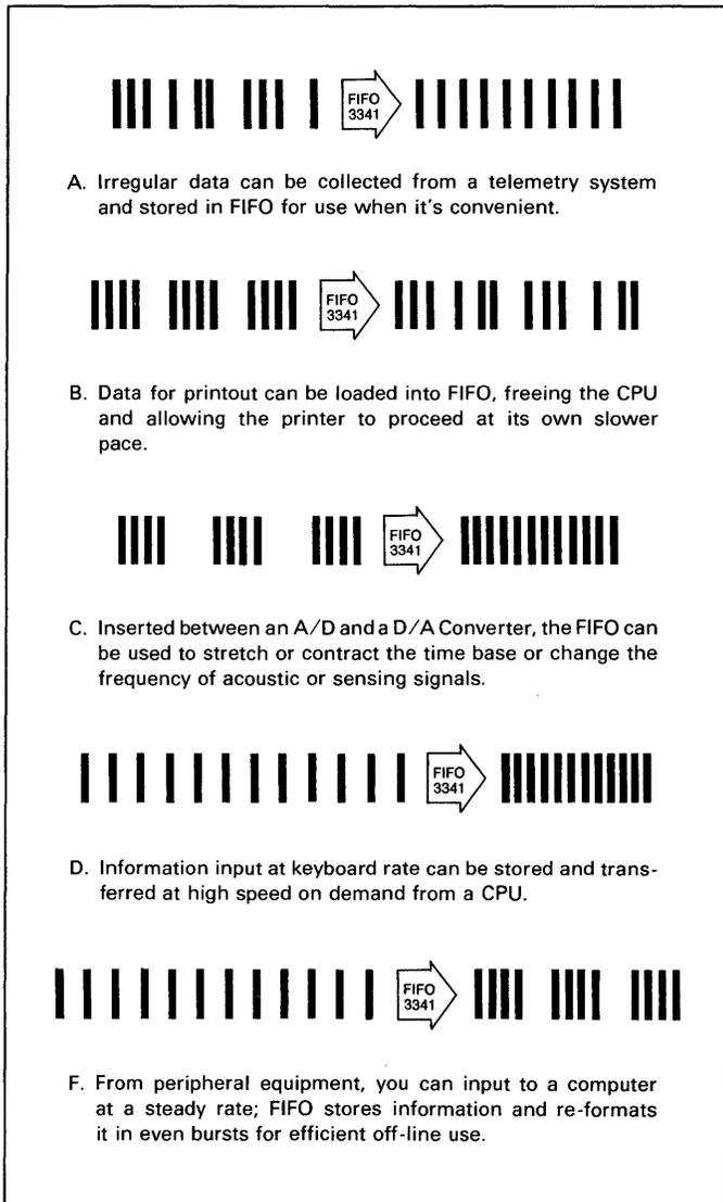
Figure 6. Examples of FIFO Handling of Differing Data Rates
