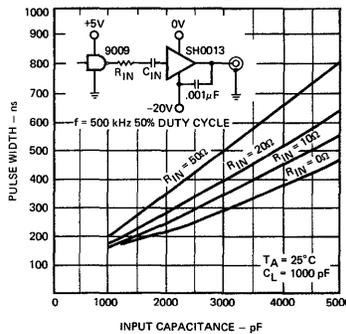
Fig. 3 PULSE WIDTH AS A FUNCTION OF  $R_{IN}$  AND  $C_{IN}$  FOR SH0013 AND 9002 NAND GATE
