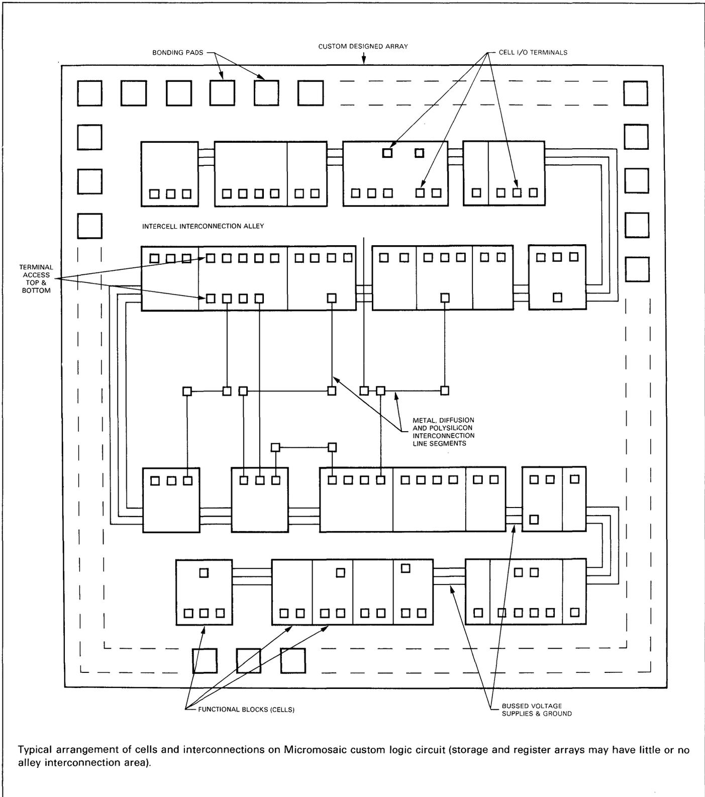
Typical arrangement of cells and interconnections on Micromosaic custom logic circuit (storage and register arrays may have little or no alley interconnection area).
