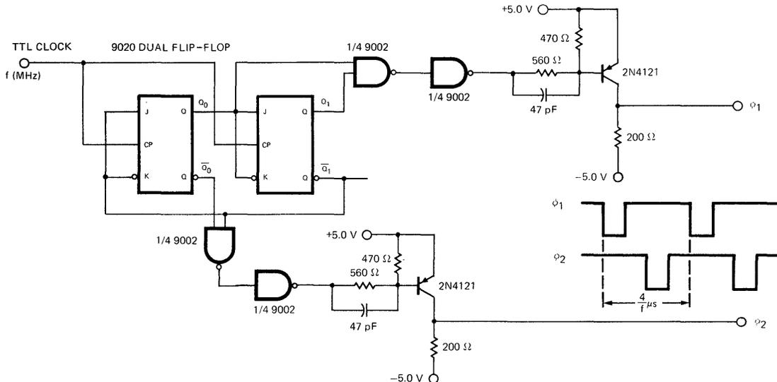
Fig. 2 2-PHASE NON-OVERLAPPING CLOCK GENERATOR
