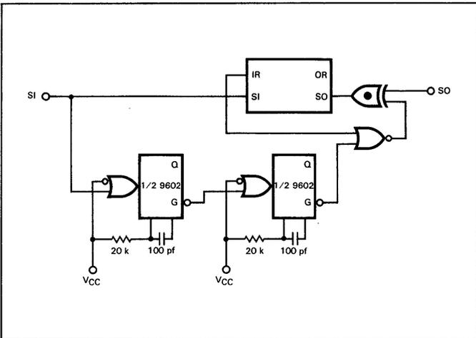
Figure 11. Automatic Dump of One Word from a Full FIFO
