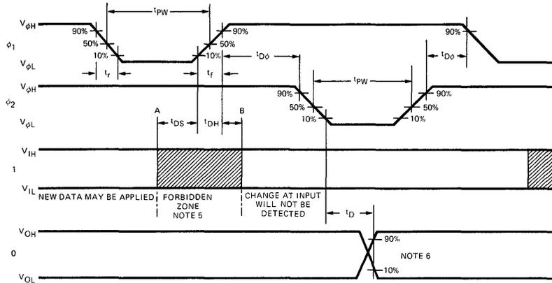
Fig. 1 TIMING DIAGRAM
