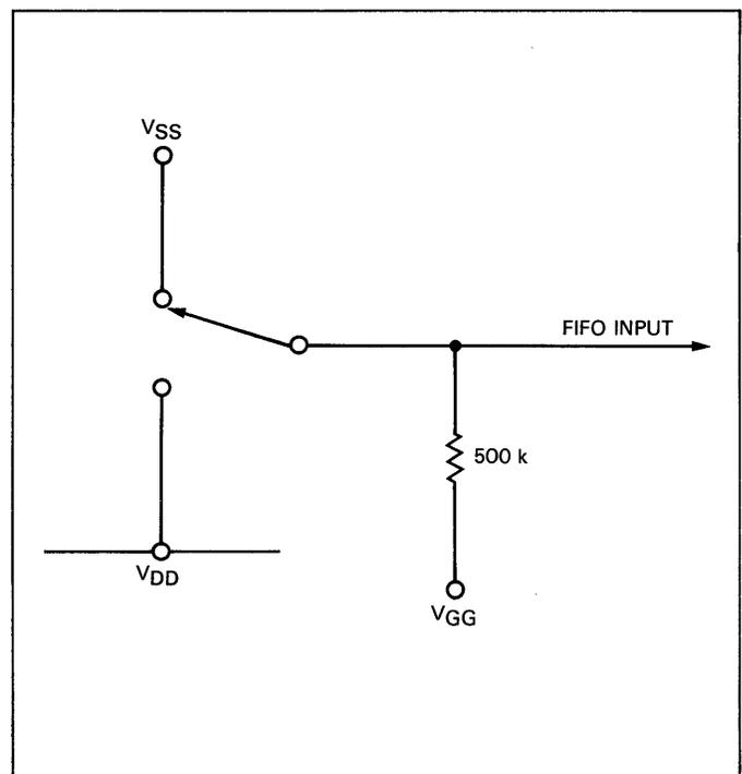
Figure 5. Switch Bounce Eliminator Using 3341 Unique Input Pullup Circuit
