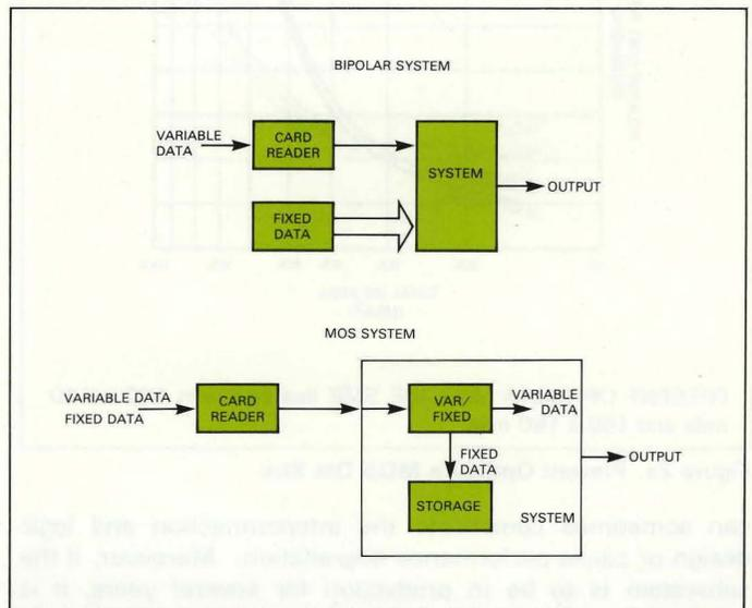
Figure 3. Structural Change from Bipolar to MOS
