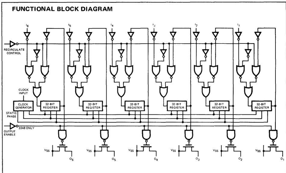
**FUNCTIONAL DESCRIPTION** — The 3348/3349 is a 2-phase static shift register. The single external clock phase generates two shift phases as well as a static operation phase via the on chip clock generator. Data is accepted at the inputs after the negative going transition of the external clock. Output information is available after the positive clock transition as illustrated in Figure 1. For long term storage, the external clock should be held HIGH.
