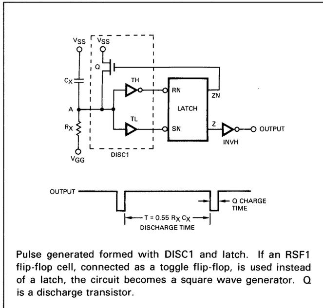
Fig. D-27. DISC1 as Pulse Generator
