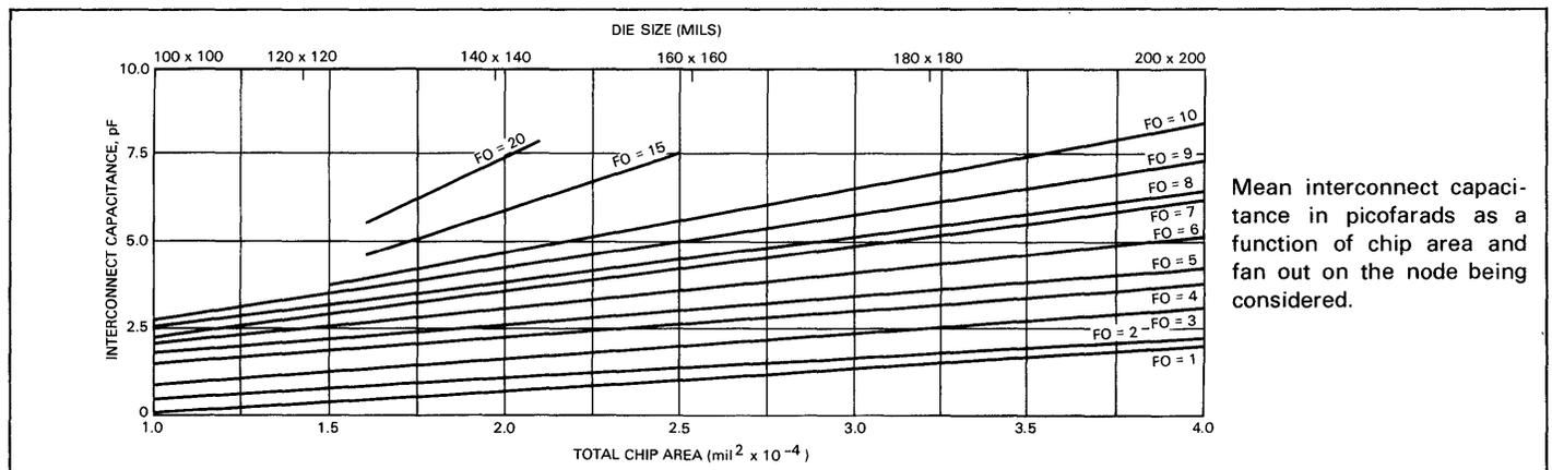
Mean interconnect capacitance in picofarads as a function of chip area and fan out on the node being considered.
