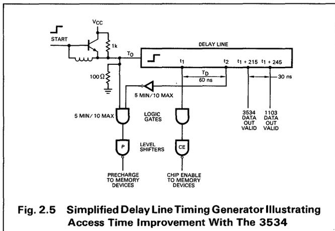
Fig. 2.5 Simplified Delay Line Timing Generator Illustrating Access Time Improvement With The 3534
