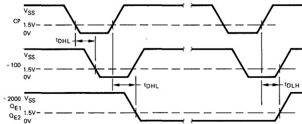
Fig. 3. Propagation delay-outputs
