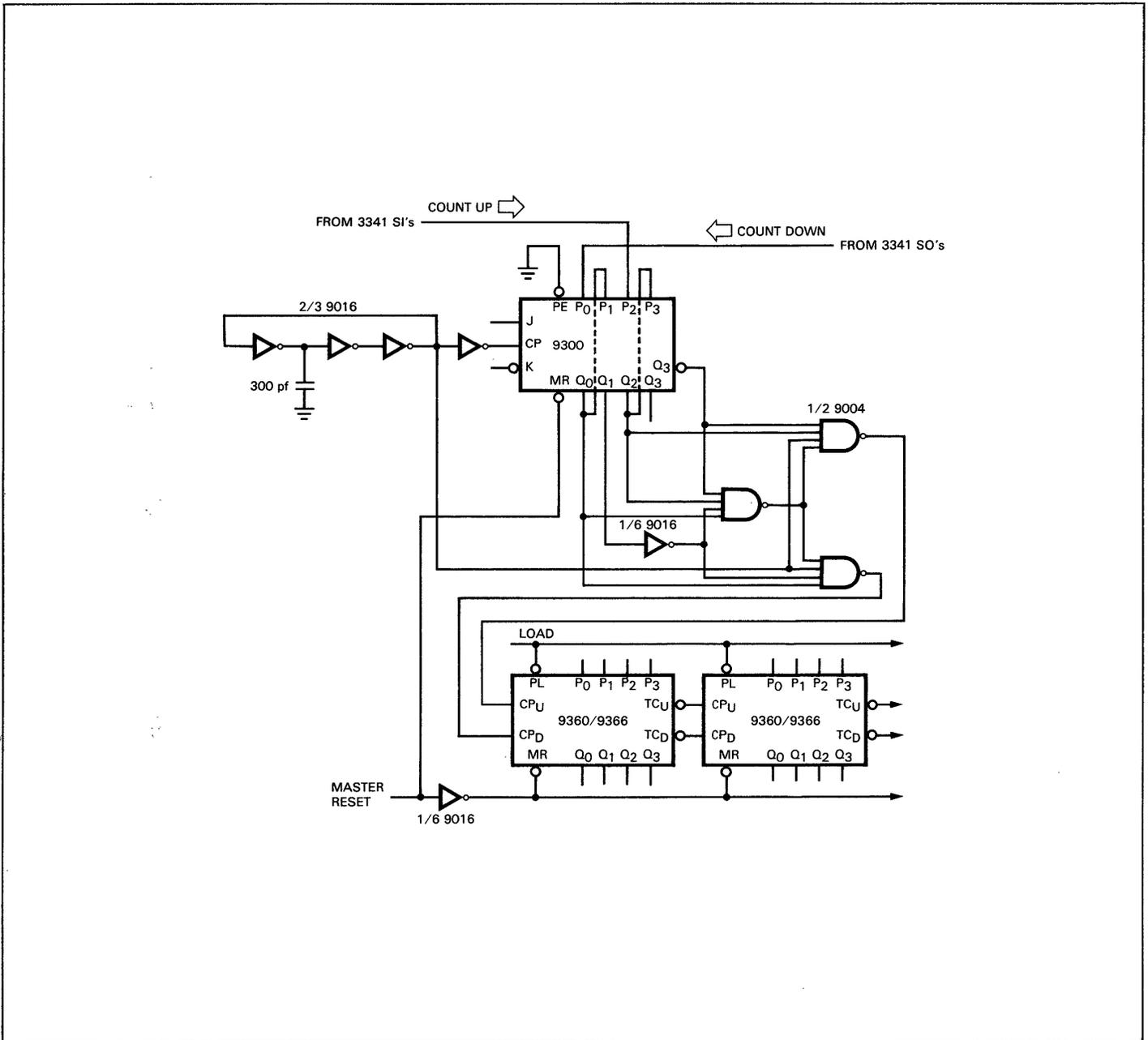
Figure 10. Content Indicator for 3341 FIFO Memories
