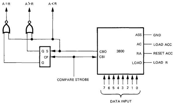
COMPARE OPERATION: To compare two numbers, simply insert the first into a previously cleared accumulator by pulsing ac. Enabling the subtract control will immediately indicate whether  $R > A$ , as a borrow output will appear. If the borrow output follows a pulse on the borrow input, the numbers are equal. If neither, then  $R < A$ . The logic is shown to the left.
