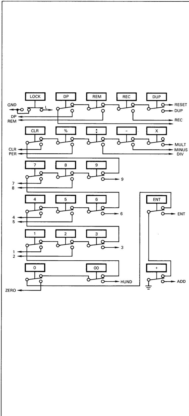
Fig. C-2. Keyboard Switch Schematic Single Pole Double Throw Switches
