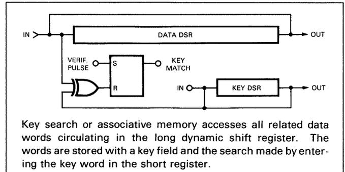
Fig. D-31. Shift Register CAM
