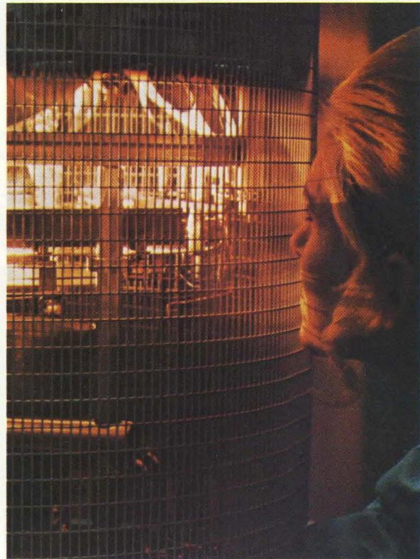
Aluminum metal is deposited in vacuum chambers. A planetary gear arrangement insures that the metal forms evenly over the steps in the oxide surface.
