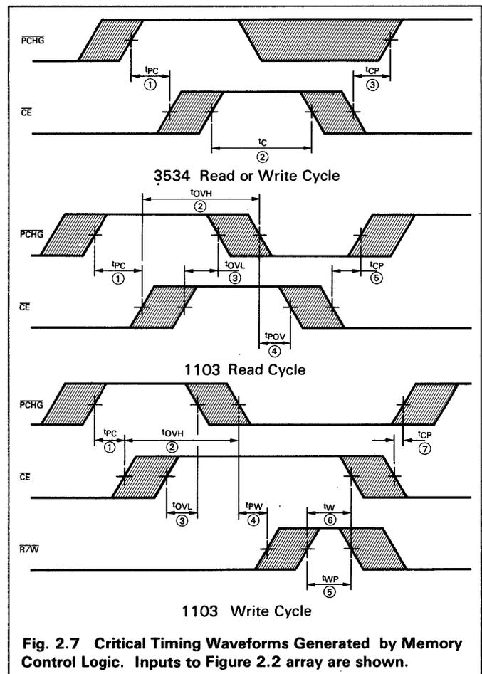
Fig. 2.7 Critical Timing Waveforms Generated by Memory Control Logic. Inputs to Figure 2.2 array are shown.
