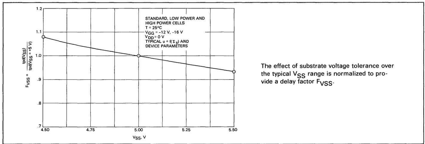
The effect of substrate voltage tolerance over the typical  $V_{SS}$  range is normalized to provide a delay factor  $F_{VSS}$ .
