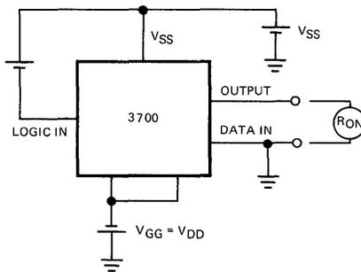
Voltage levels between semiconductor electrodes are normally referenced to one of the electrodes. In MOS, this electrode is the substrate (body). The voltages can be translated to an equivalent level and referenced to another electrode. In order to measure the ON resistance of the data channel accurately, the data input is at ground potential and all other terminals are changed correspondingly to test worst case conditions.
