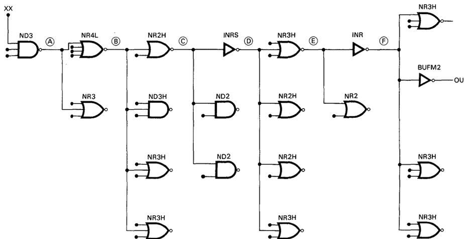
Propagation delay example showing method of tabulating and adding nodal capacitances.
