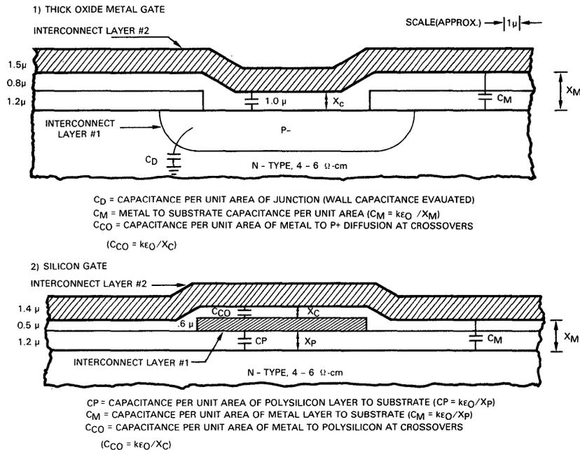
Fig. G-3. Thick Oxide Metal Gate (Top) and Silicon Gate Interconnection Segments and Capacitance Components
