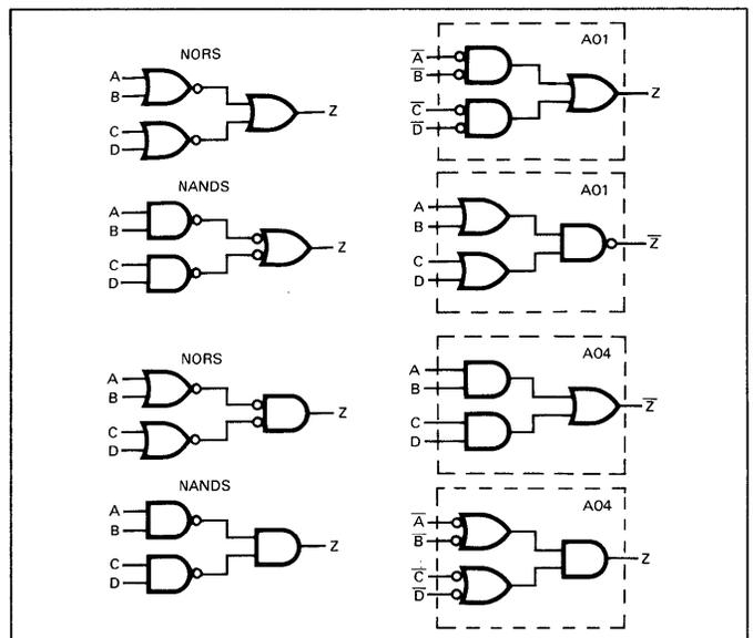
Substituting a complex gate for several simple gates saves chip area. The A04, for example is five grids long while three NAND gates take nine grids.
