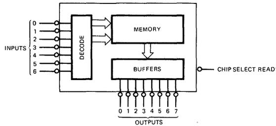
\*When chip select read is at ground the outputs are floating.
