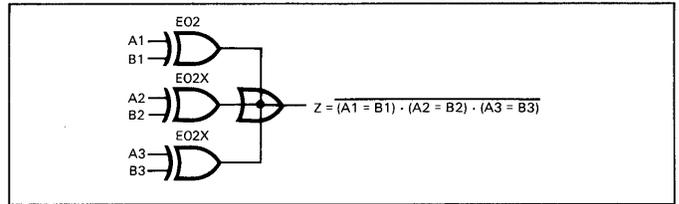
Fig. D-18. Expanded EXCLUSIVE-OR Cells as Multi-bit Comparators
