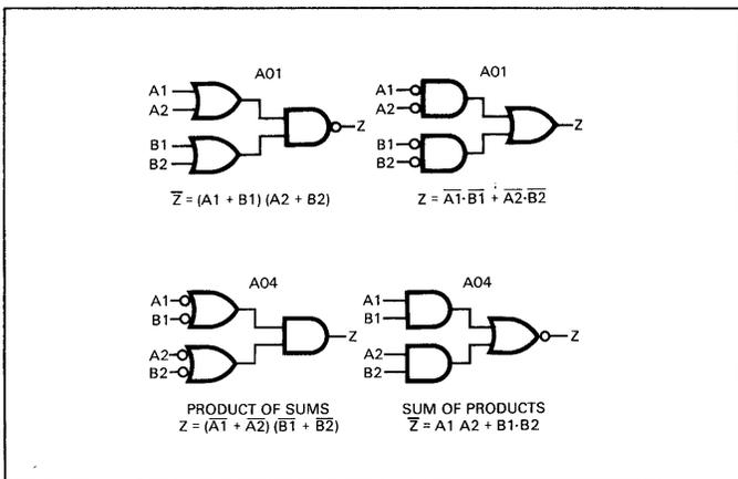
Fig. D-16. Boolean Function of AND-OR Invert Cells
