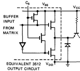
If chip is selected voltage C<sub>s</sub> = V<sub>SS</sub>, output = the programmed bit.
