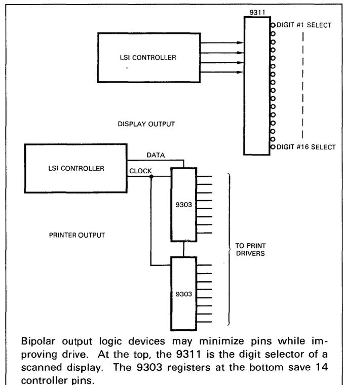
Fig. D-4. MOS with Bipolar Augmentation
