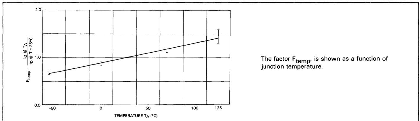
The factor  $F_{\text{temp}}$  is shown as a function of junction temperature.
