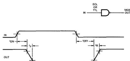
Table 2.2 Level Shifter Switching Characteristics
