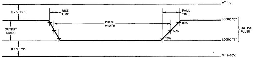
Logic "0" = Most positive output voltage
