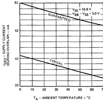
Fig. 3 SUPPLY CURRENT DURING CHIP ENABLE VERSUS AMBIENT TEMPERATURE
