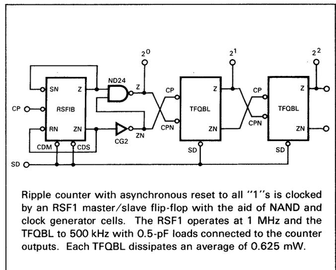
Fig. D-26. Ripple Counter Clocking
