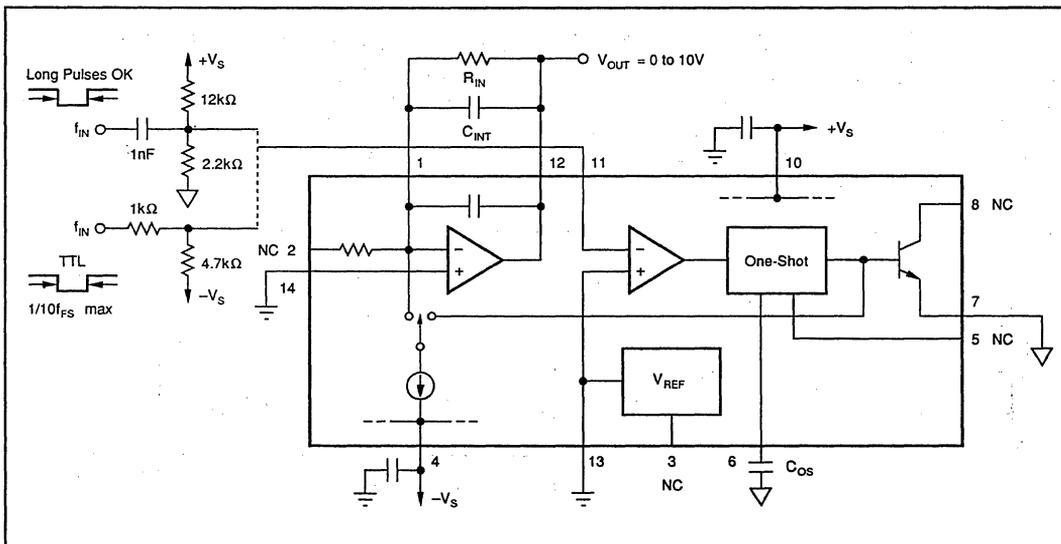
FIGURE 4. Frequency-to-Voltage Conversion.
