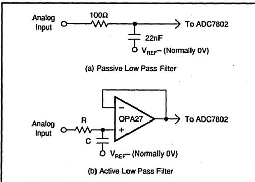
FIGURE 9. Input Signal Conditioning.
