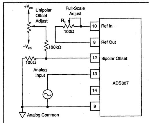
FIGURE 4. Unipolar Connection.
