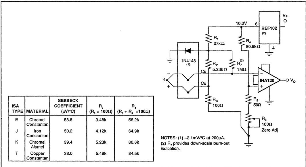
FIGURE 7. Thermocouple Amplifier With Cold Junction Compensation.
