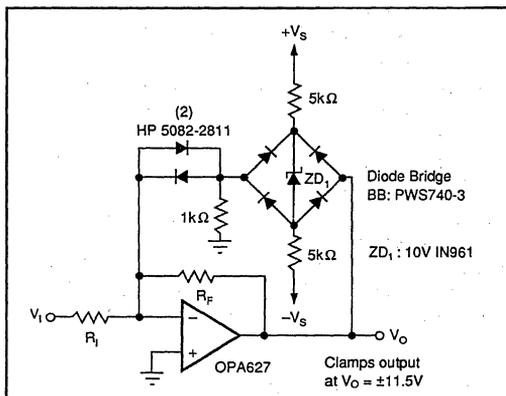
FIGURE 5. Clamp Circuit for Improved Overload Recovery.
