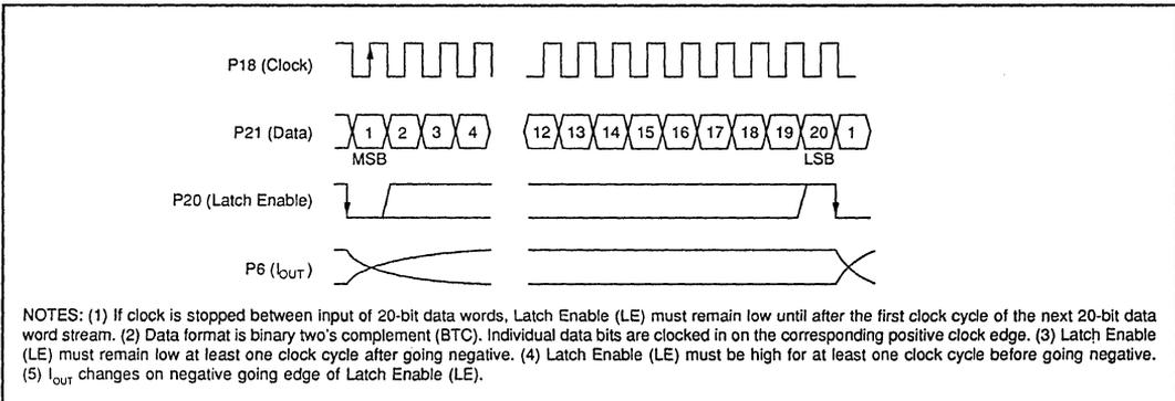
FIGURE 2. Timing Diagram.
