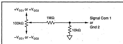
FIGURE 3.  $V_{OS}$  Adjust.
