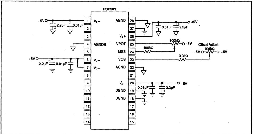
FIGURE 14. DSP201 Power Supply Connections and Adjust Circuits.
