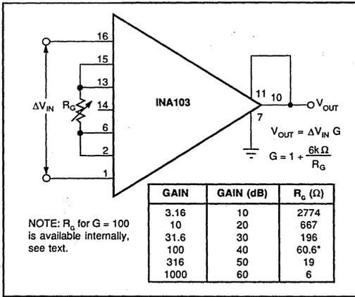
FIGURE 8. Gain Setting Using External Resistor.
