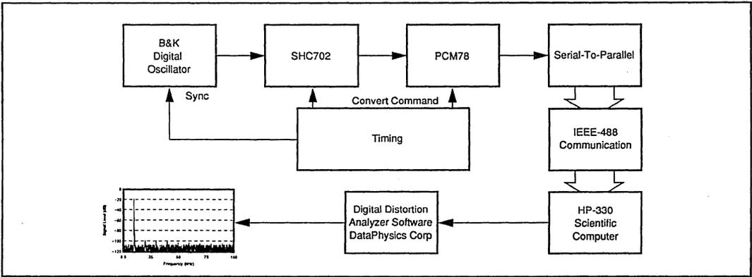
FIGURE 2. Block Diagram of Distortion Test Circuit.
