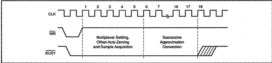
FIGURE 2. Converter Timing.
