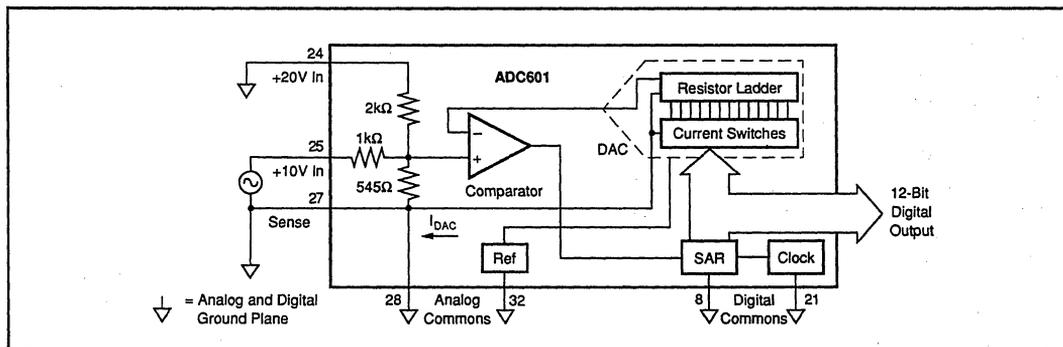
FIGURE 3. Analog and Digital Grounds, and Analog Input Sense.
