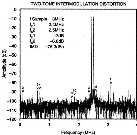
NOTE: Sample rate = 8MHz; highest IMD product is cursor number 1:  $f_1 + f_2$ . The second-order  $-76.3\text{dBc}$  product determines the wideband spurious-free dynamic range of this example. For RF applications third-order IMD products such as those at cursors 3 and 6 are the limiting spurs. Under these conditions spurious-free dynamic range is limited by  $2f_2 + f_1$  to  $84.3\text{dBc}$ .
