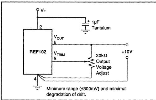
FIGURE 3. REF102 Optional Output Voltage Adjust.
