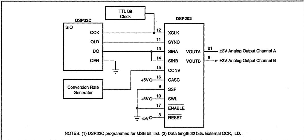
FIGURE 11. Using DSP202 with DSP32C in Cascade Mode.
