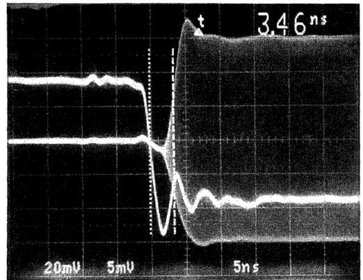
FIGURE 9. OPA675 Input Selection Time. Input B to A.
