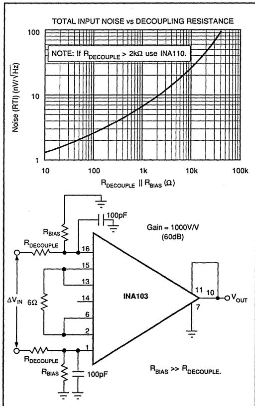
FIGURE 13. Input Decoupling and Protection.
