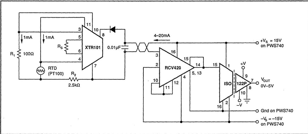
FIGURE 11. Isolated 4–20mA Instrument Loop (RTD shown).
