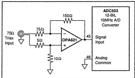
FIGURE 17. Differential Input Buffer Amplifier ( $G = -2V/V$ ).
