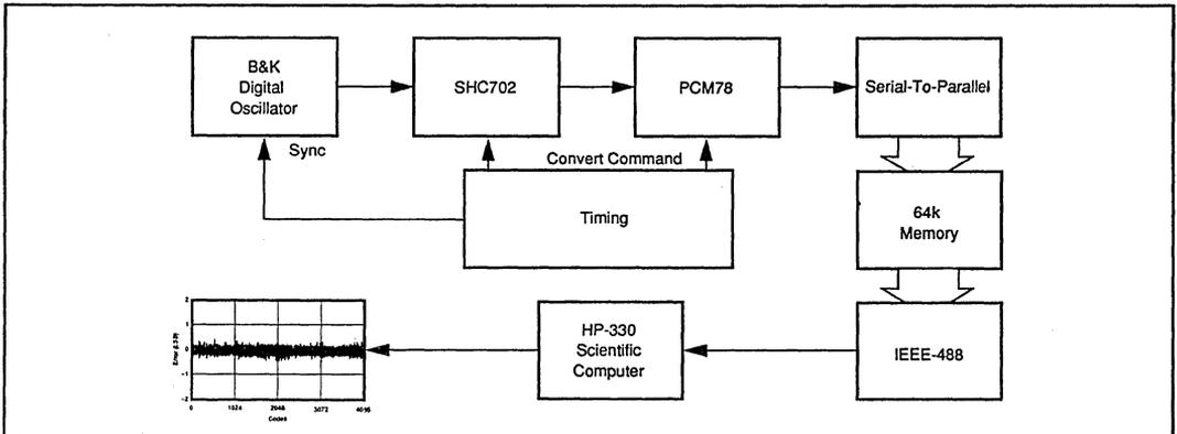
FIGURE 3. Block Diagram of Histogram Test .
