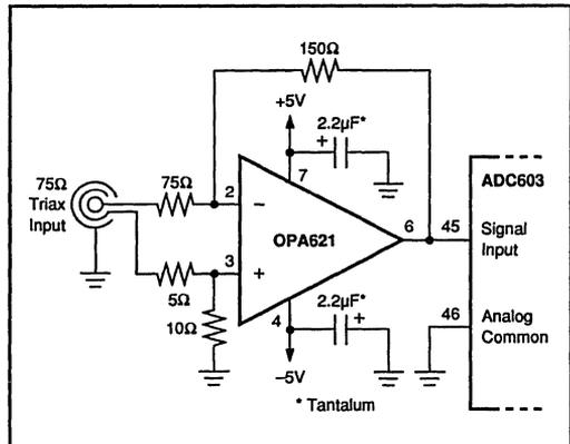
FIGURE 10. Differential Input Buffer Amplifier (Gain = -2V/V).
