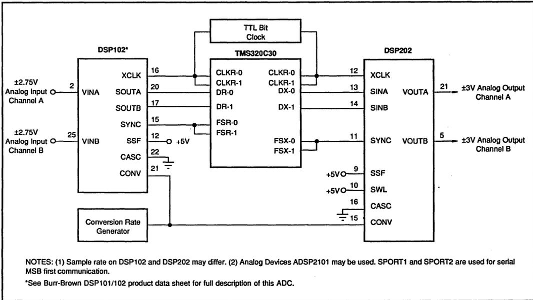
FIGURE 6. Two-Channel Analog Input and Output System with TMS320C30.
