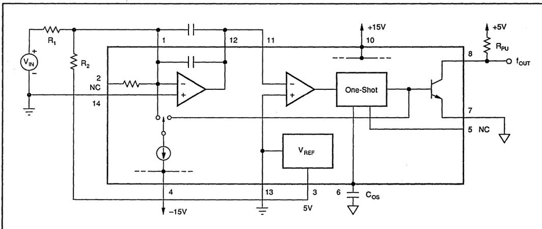
FIGURE 3. Offsetting the Frequency Output.
