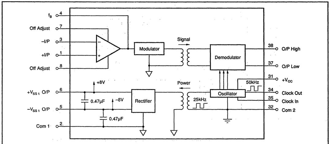
FIGURE 2. Simplified Diagram of Isolation Amplifier.
