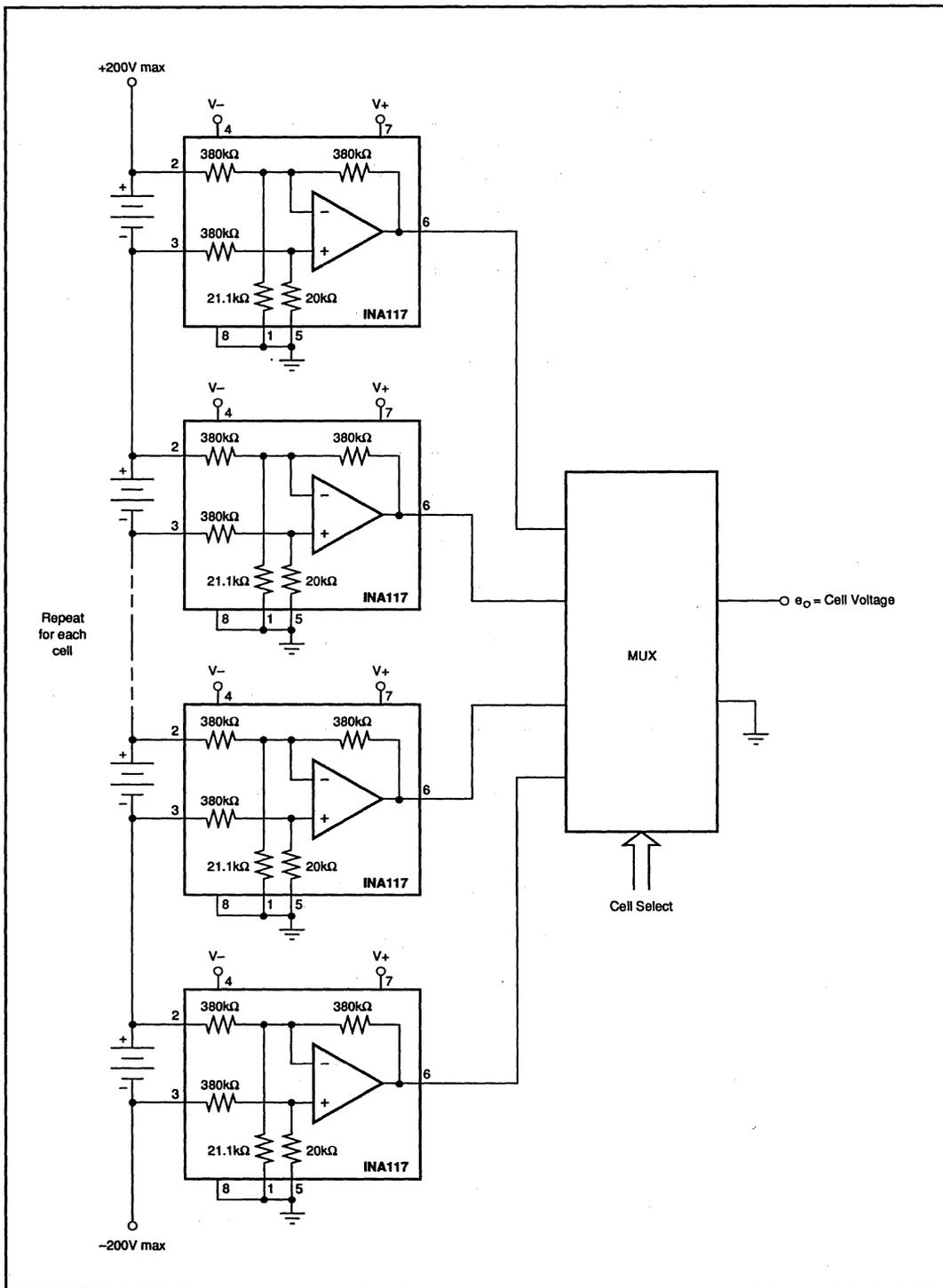
FIGURE 14. Battery Cell Voltage Monitor.
