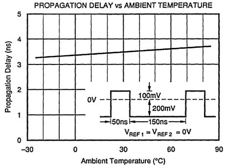
NOTE: Propagation Delay vs Overdrive is shown for two amplitudes of input pulse: from  $-200\text{mV} \rightarrow +V_{OD}$  (0.2nV/ns slew rate) and  $-1\text{V} \rightarrow +V_{OD}$  (1V/ns slew rate). For an inverse input waveform: from  $+1\text{V} \rightarrow -V_{OD}$  and from  $+200\text{mV} \rightarrow -V_{OD}$ , propagation delays identical to those above are produced.
