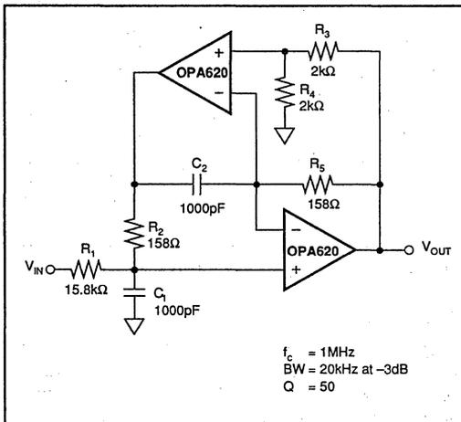
FIGURE 12. High-Q 1MHz Bandpass Filter.
