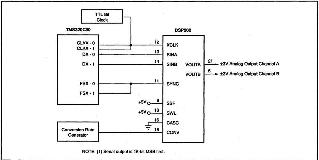
FIGURE 4. Using DSP202 with TMS320C30's Dual SIO.
