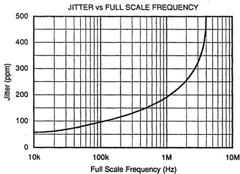
Jitter is the ratio of the  $1\sigma$  value of the distribution of the period ( $1/f_{OUT, max}$ ) to the mean of the period.
