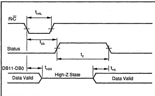
FIGURE 6.  $\overline{R/C}$  Pulse Low — Output Enables After Conversion.
