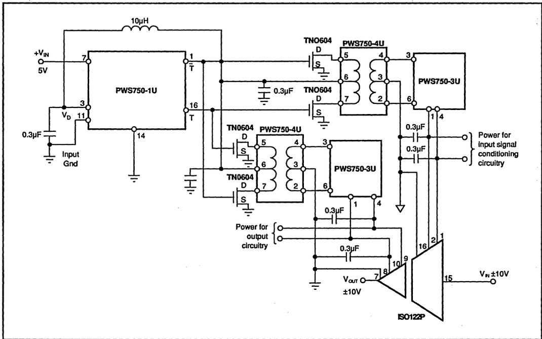
FIGURE 5. A Complete  $\pm 10V$  Signal Acquisition System Operating From a Single 5V Supply.
