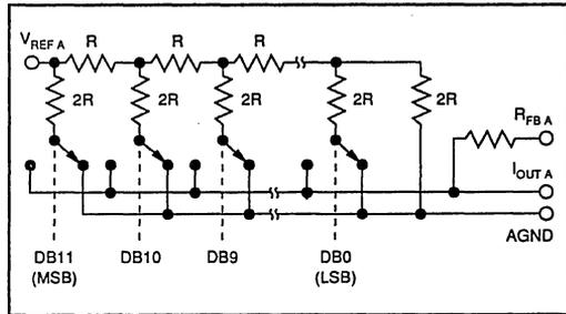
FIGURE 1. Simplified DAC Circuit.
