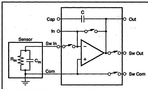
FIGURE 6. Capacitance of Circuit at Input of Integrator.
