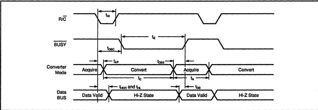
FIGURE 6. Convert Mode: R/C Pulse LOW — Outputs Enabled After Conversion.
