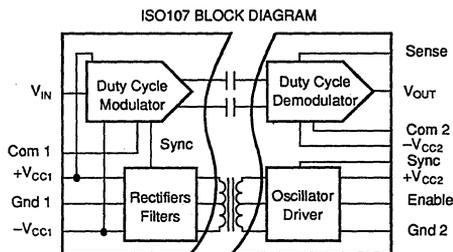
rol is used to turn off transformer drive while keeping the signal channel demodulator active. This feature provides a convenient way to reduce quiescent current for low power applications.
