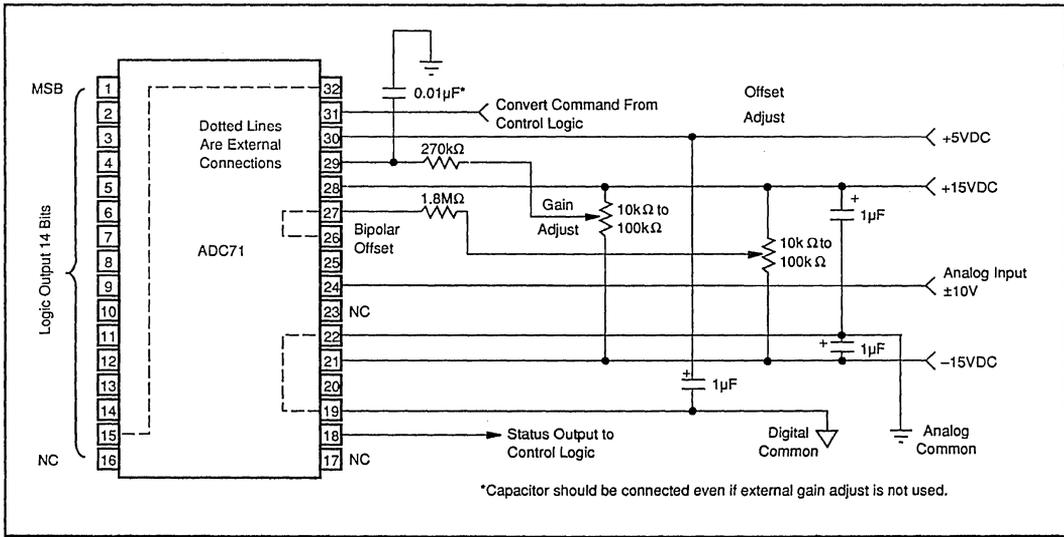
FIGURE 5. ADC71 Connections for:  $\pm 10V$  Analog Input, 14-Bit Resolution (Short-Cycled), Parallel Data Output.
