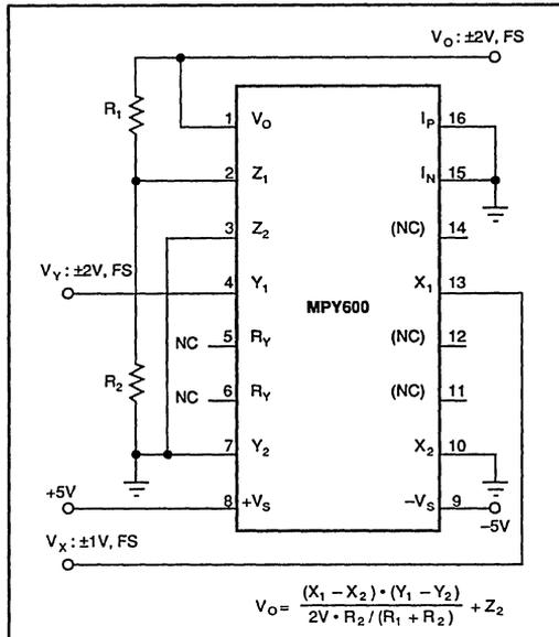
FIGURE 2. Adjusting the Scale Factor with Feedback.
