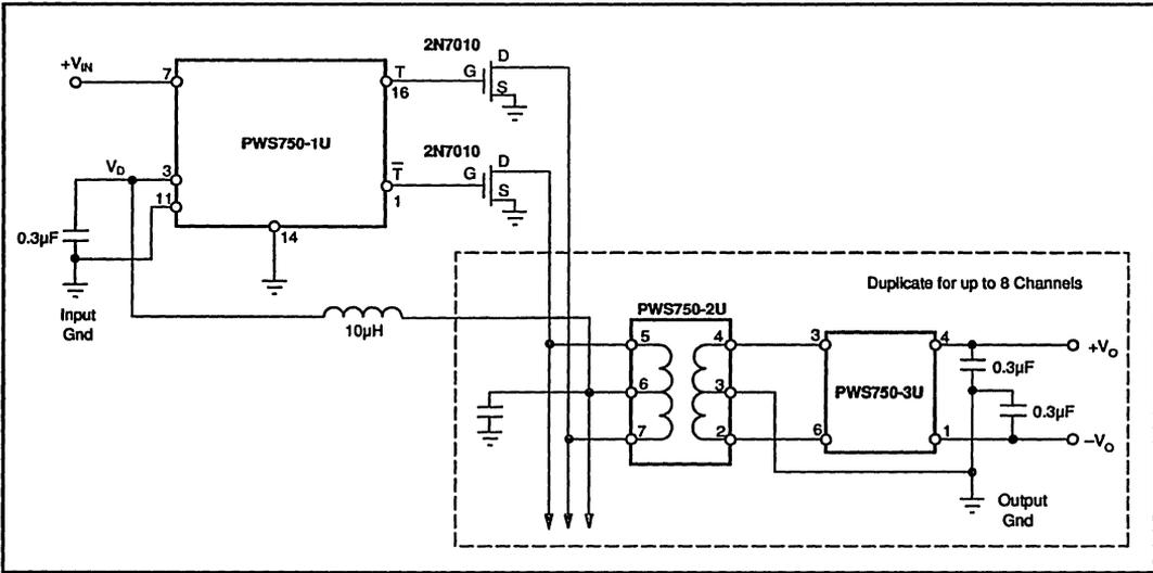
FIGURE 9. FET Pair Driving Up to Eight-Channels.
