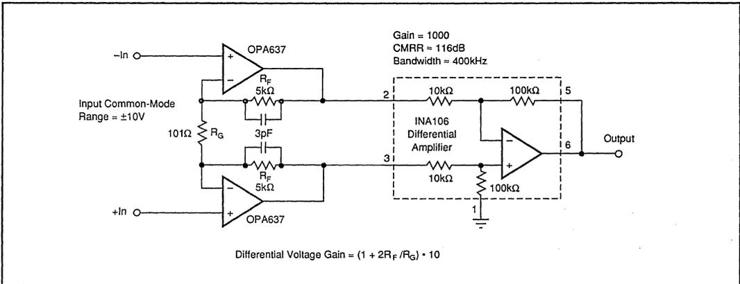
FIGURE 13. High Speed Instrumentation Amplifier, Gain = 1000.
