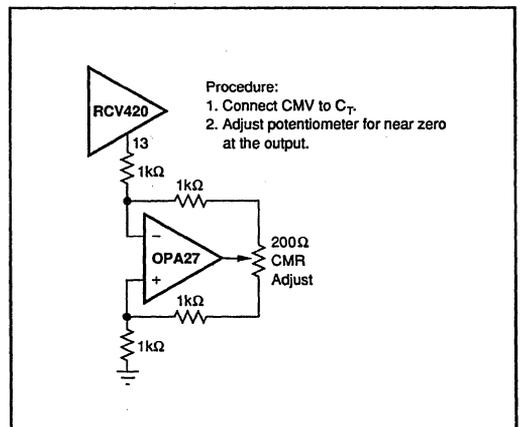
FIGURE 5. Optional Circuit for Externally Trimming CMR.
