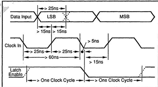
FIGURE 1. PCM1700P Setup and Hold Timing Diagram.
