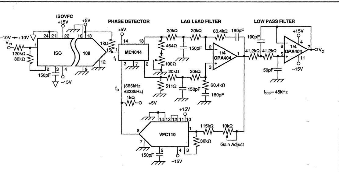
FIGURE 6. PLL Analog Isolator with High (10kV/ $\mu$ s) Transient Immunity.
