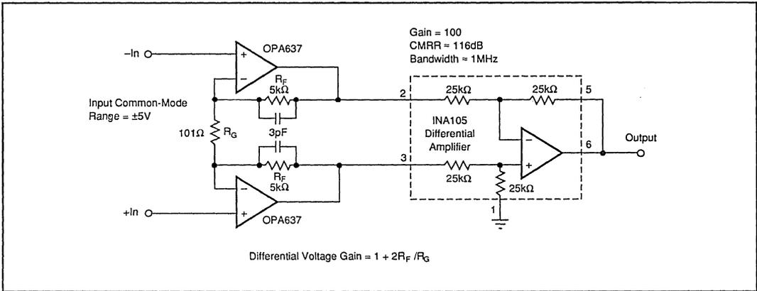
FIGURE 12. High Speed Instrumentation Amplifier, Gain = 100.
