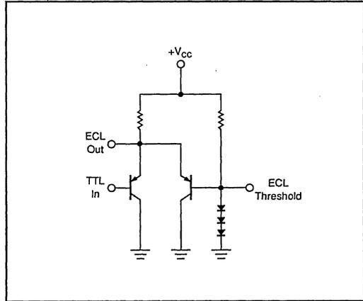
FIGURE 2. Internal OPA676 TTL Logic Level Shifter.
