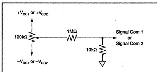
FIGURE 3.  $V_{OS}$  Adjust.
