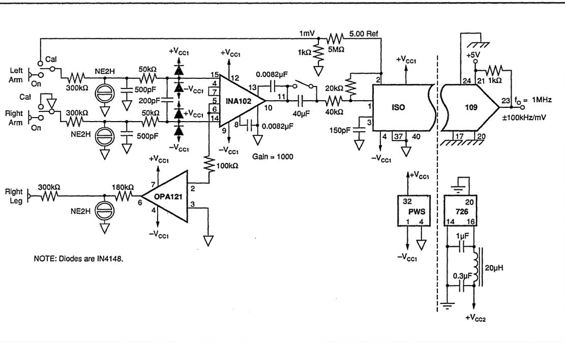
FIGURE 5. Serial TTL Output ECG Amplifier.
