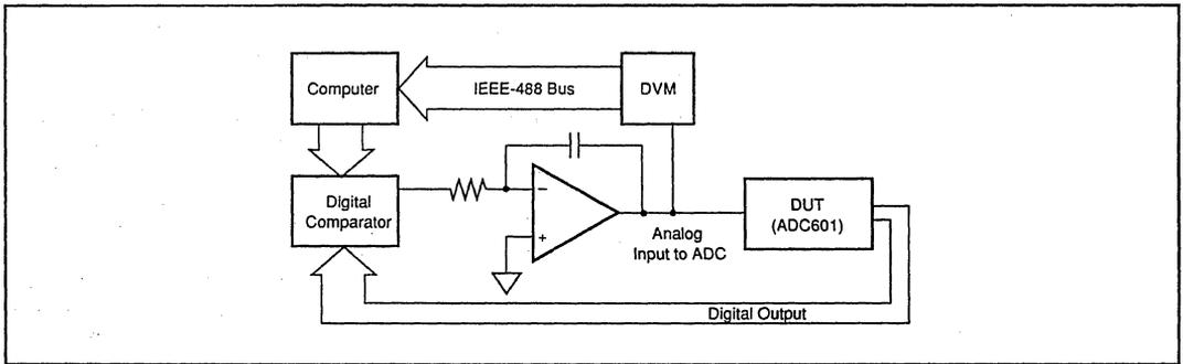
FIGURE 13. Servo Loop Analog-to-Digital Tester.
