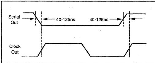
FIGURE 3. Timing Relationship of Serial Data to Clock.
