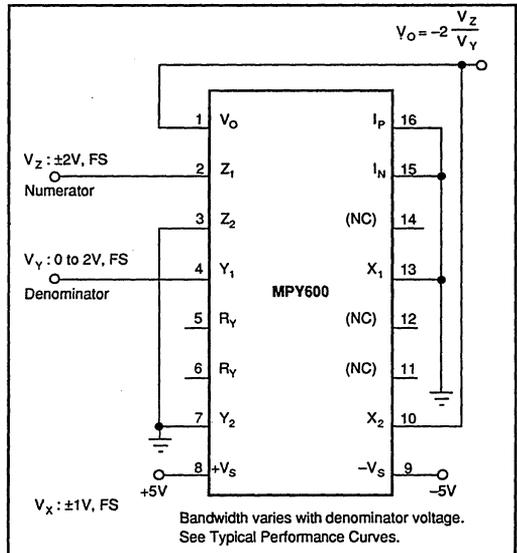
FIGURE 7. Divider Circuit.
