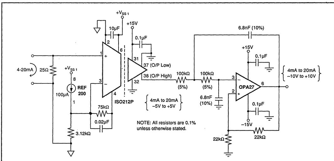
FIGURE 8. Isolated 4-20mA Current Receiver with Output Filter.
