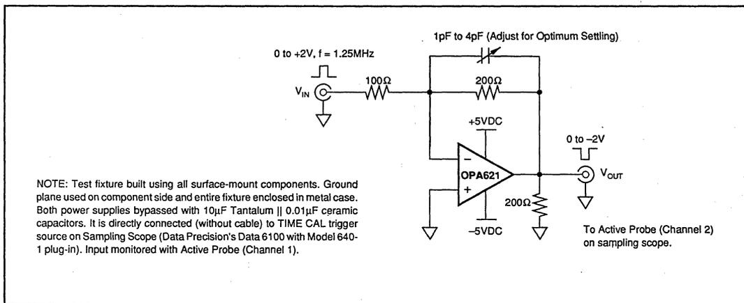
FIGURE 7. Settling Time Test Circuit.
