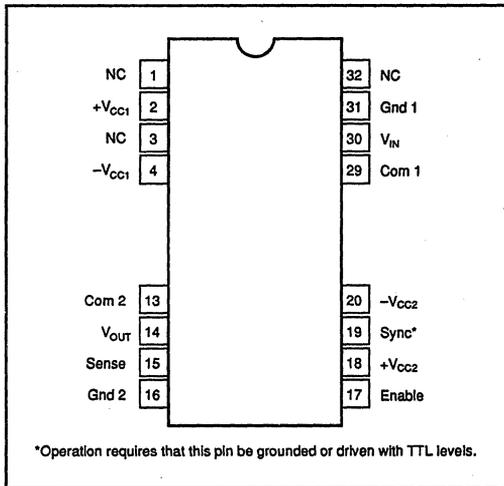
\*Operation requires that this pin be grounded or driven with TTL levels.
