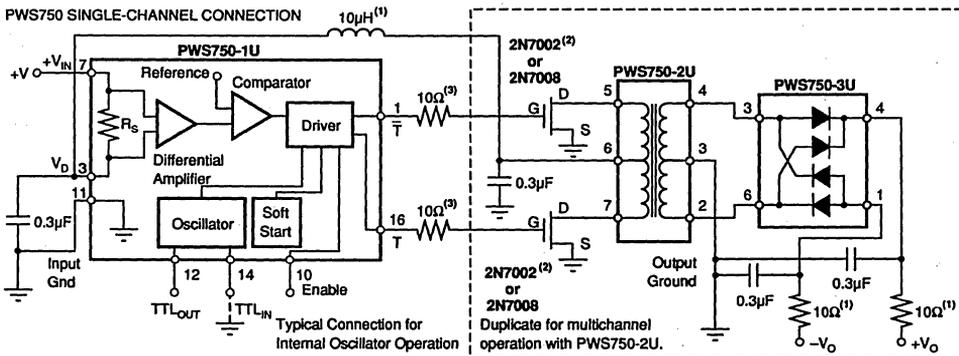
NOTES:(1) User option. (2) Use TN0604 for 5V to ±15V operation. (3) Multichannel Operation.
