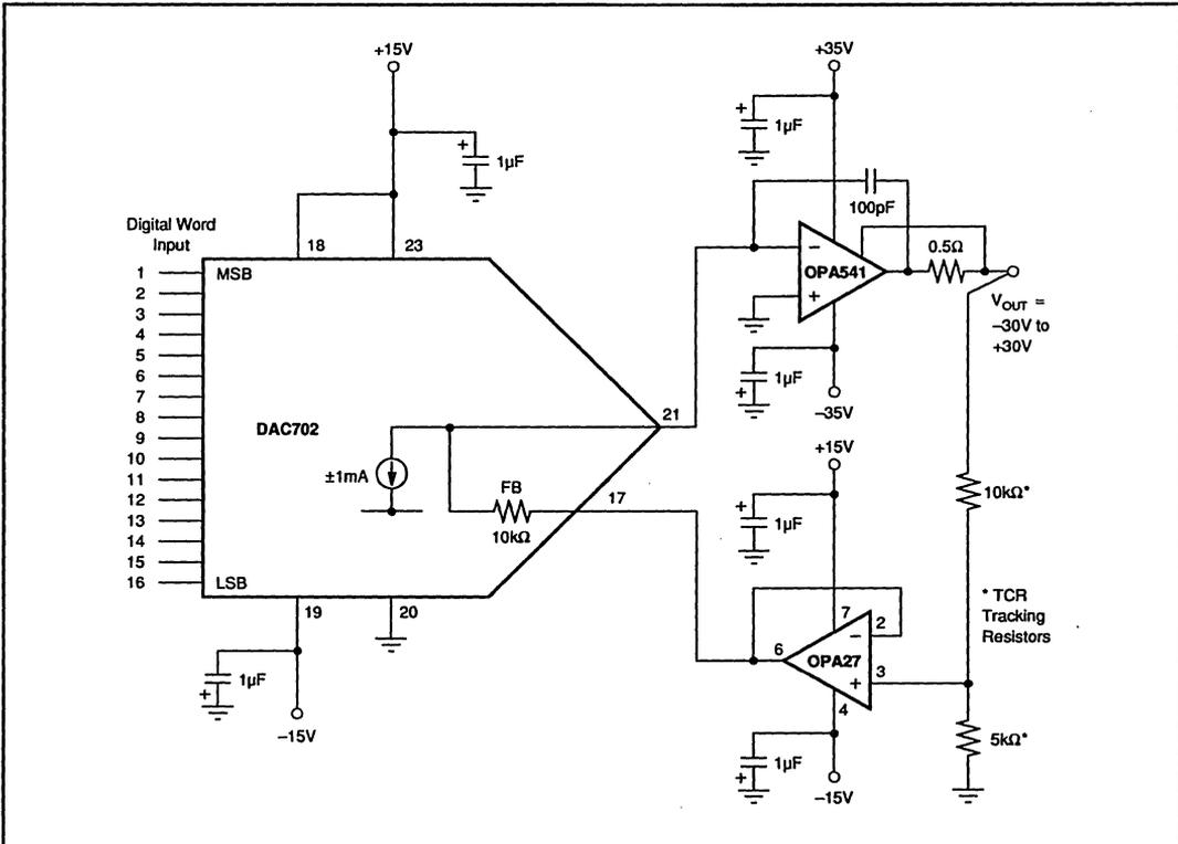
FIGURE 7. 16-Bit Programmable Voltage Source.
