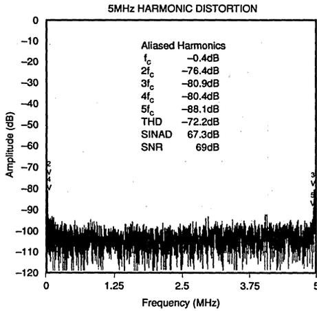
NOTE: Sample rate = 9.99 MHz; even harmonics folded to left edge and odd harmonics folded to right edge. Any non-harmonically related spurious products show clearly in the center.
