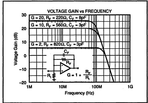
FIGURE 5. Bandwidth Results with Added Capacitor  $C_F$ .
