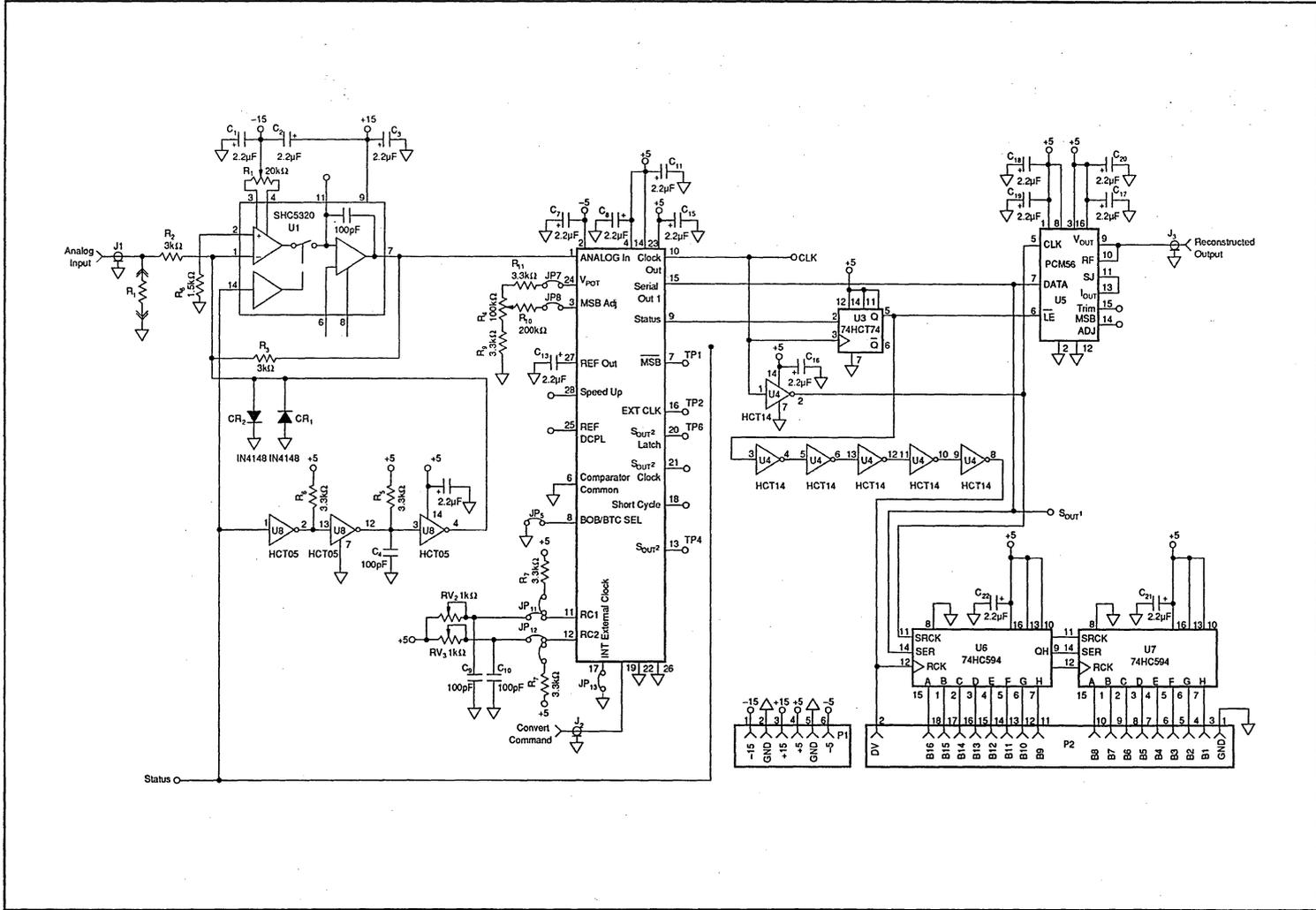
FIGURE 21. Schematic for Demonstration Board (DEM1122).
