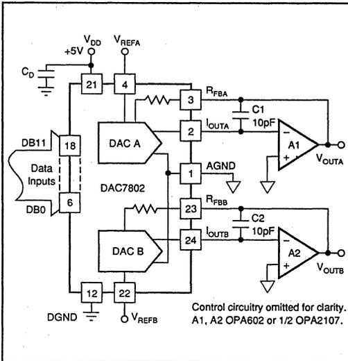
FIGURE 2. Unipolar Configuration.
