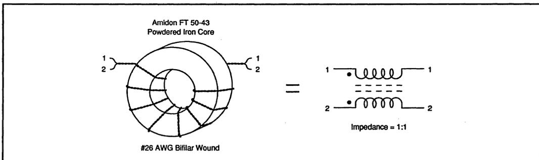
FIGURE 7. Balun Transformer Windings.
