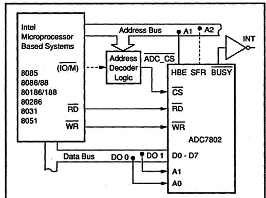
FIGURE 16. Interface to Intel Microprocessors.
