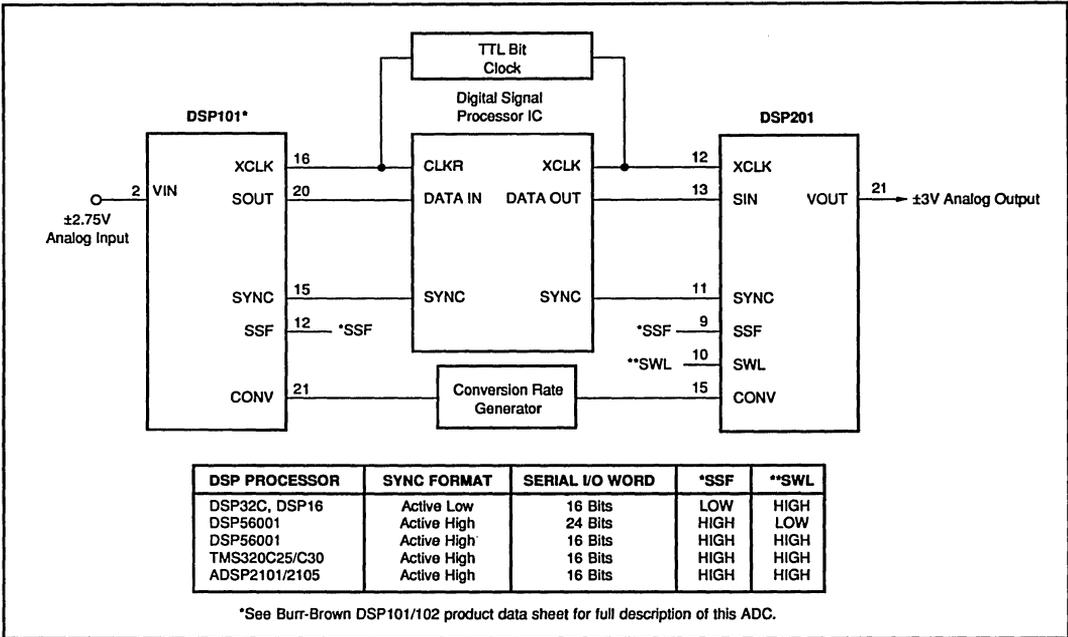
FIGURE 2. Analog Input and Analog Output System.
