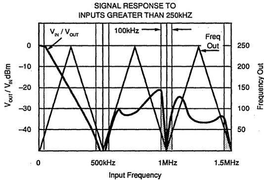
(NOTE: Shaded area shows aliasing frequencies that cannot be removed by a low-pass filter at the output.)
