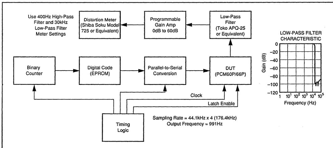
FIGURE 4. THD + N Test Setup Diagram.
