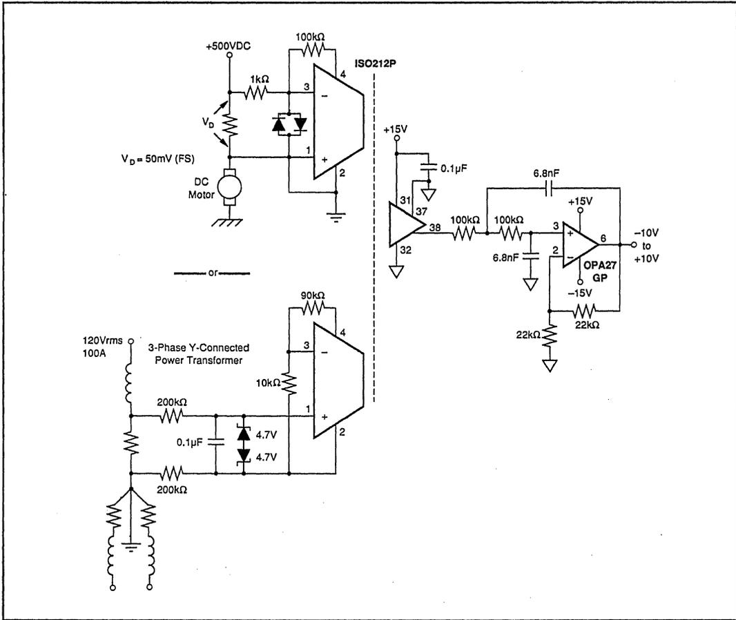
FIGURE 12. Isolated Current Monitoring Applications.
