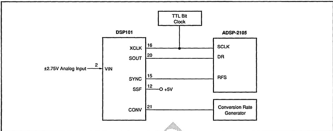
FIGURE 13. Using DSP101 with ADSP-2105.
