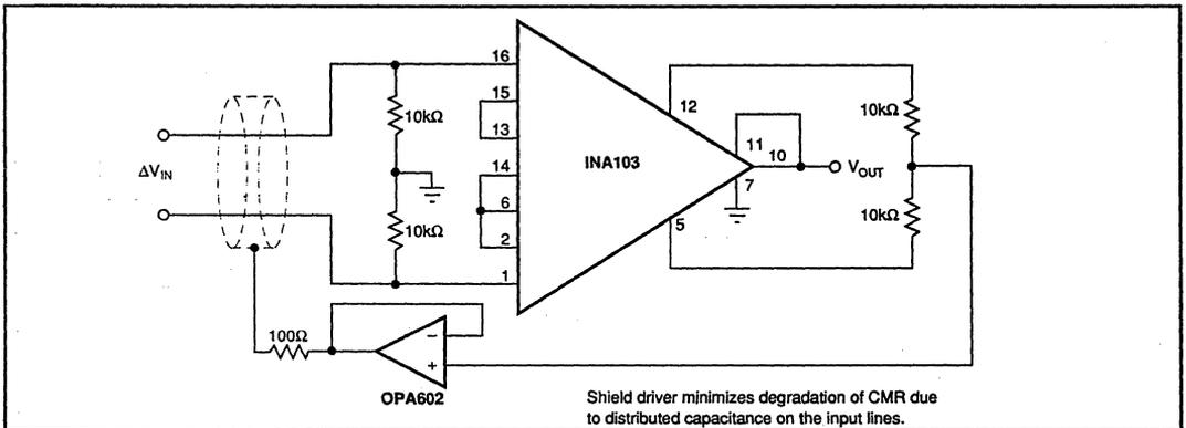
FIGURE 16. Instrumentation Amplifier with Shield Driver.
