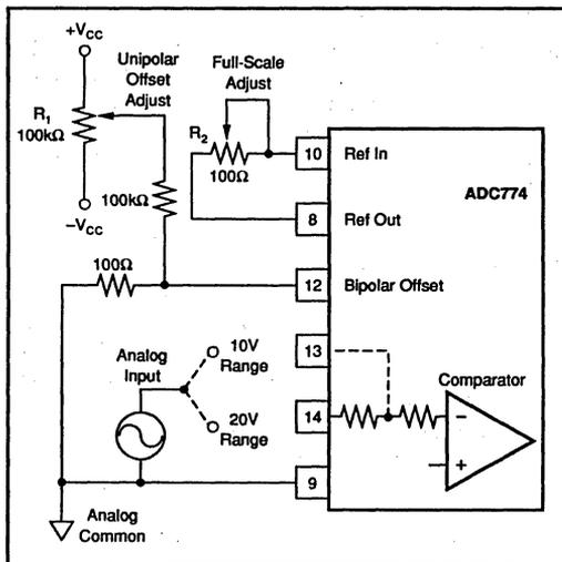
FIGURE 2. Unipolar Configuration.
