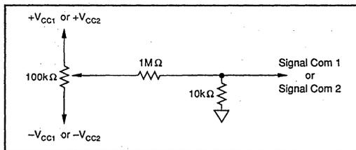
FIGURE 3.  $V_{OS}$  Adjust.
