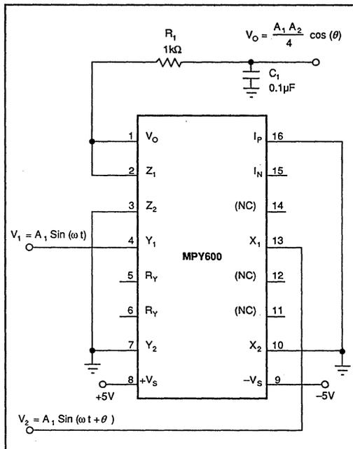
FIGURE 10. Phase Detector.
