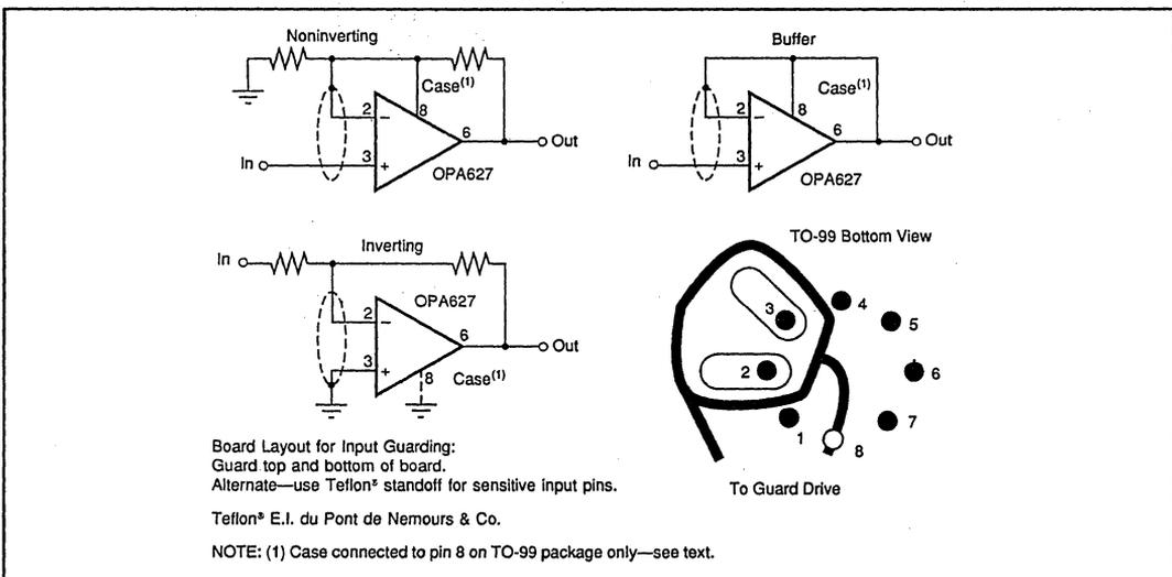
FIGURE 4. Connection of Input Guard for Lowest  $I_B$ .
