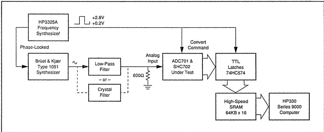
FIGURE 6. FFT Test Configuration for Single-Tone Testing.
