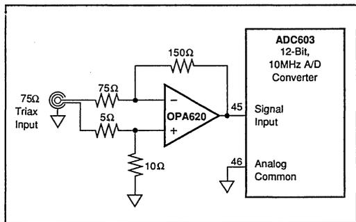
FIGURE 17. Differential Input Buffer Amplifier ( $G = -2V/V$ ).
