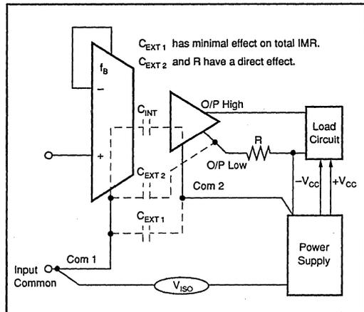
FIGURE 3. Technique for Connecting Com 1 and Com 2.
