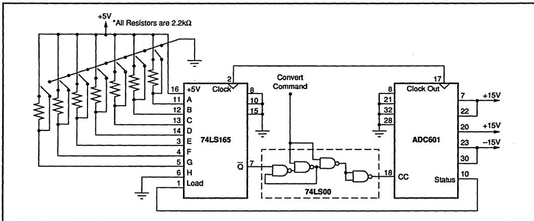
FIGURE 8. External Short Cycle Circuit.
