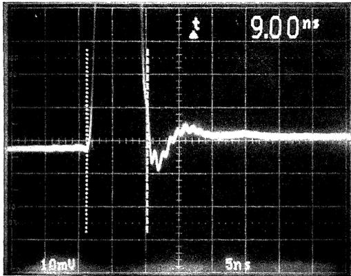
FIGURE 3. 1% Settling Time.
