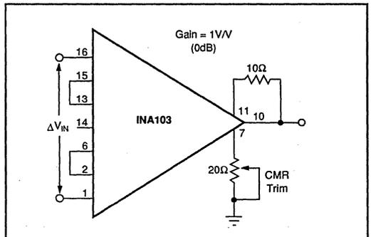
FIGURE 11. Optional Circuit for Externally Trimming CMR.
