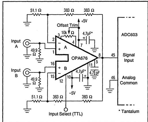
FIGURE 21. Multiplexed Input  $+16V/V$  Gain (24dB) Buffer Amplifier.
