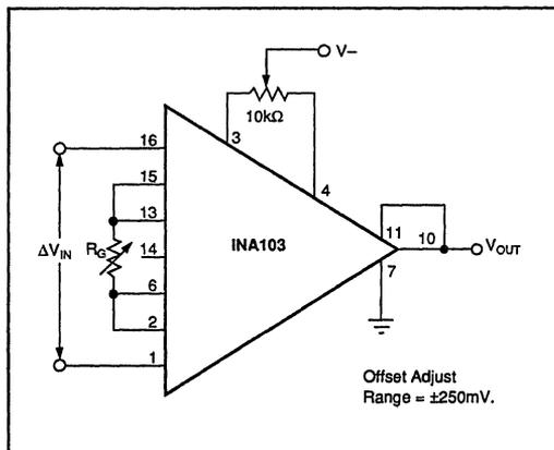
FIGURE 3. Offset Adjustment Circuit.
