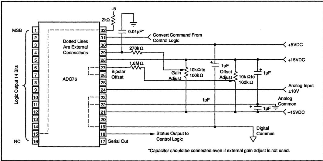
FIGURE 5. ADC76 Connections for:  $\pm 10\text{V}$  Analog Input, 14-Bit Resolution (Short-Cycled), Parallel Data Output.
