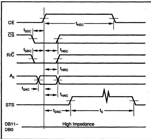
FIGURE 6. Conversion Cycle Timing.
