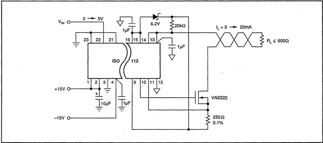
FIGURE 6. Isolated Current Loop Driver.
