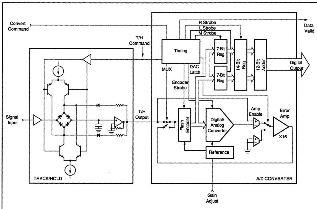
FIGURE 1. ADC603 Block Diagram—A Two-Step Subranging Architecture.
