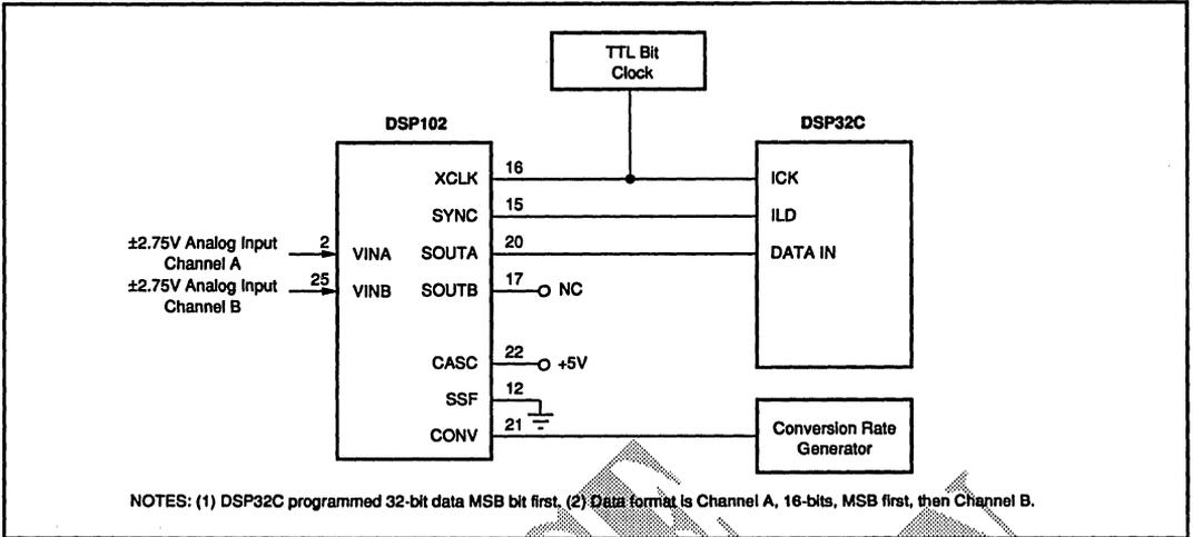
FIGURE 10. Using DSP102 with DSP32C in Cascade Mode.
