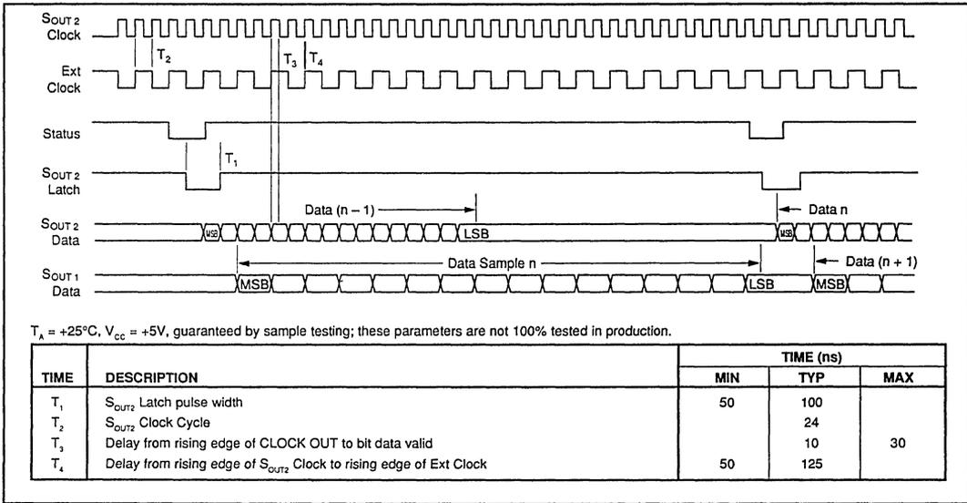
FIGURE 9. Timing when using  $S_{OUT2}$  Latch.
