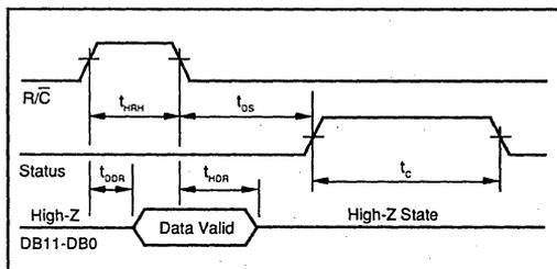
FIGURE 7. R/C Pulse High—Output Enables Only While R/C Is High.
