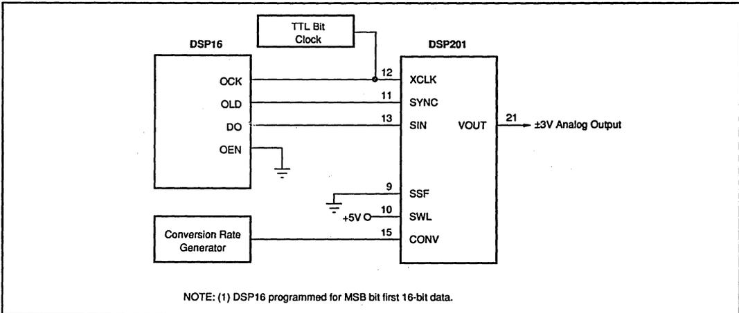
FIGURE 12. Using DSP201 with DSP16.
