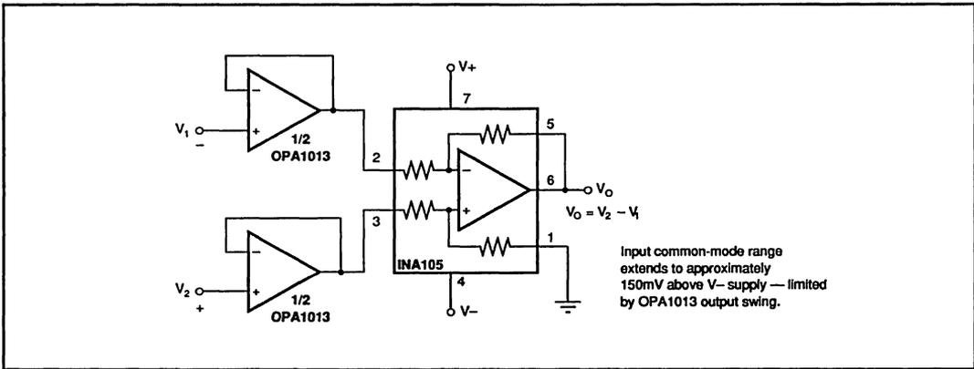
FIGURE 2. Instrumentation Amplifier.
