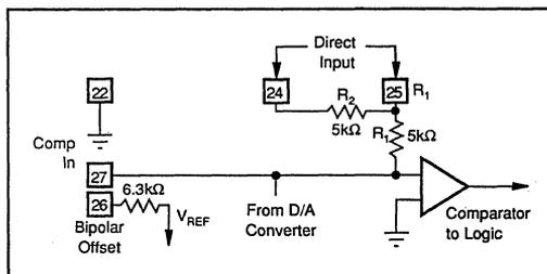
FIGURE 8. ADC76 Input Scaling Circuit.
