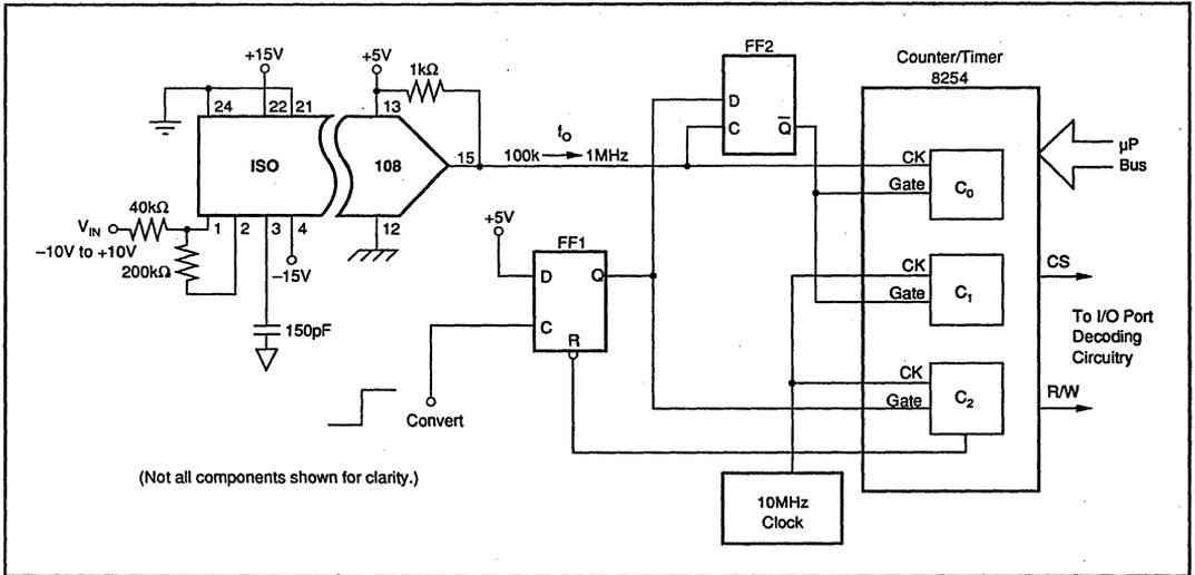
FIGURE 4. Isolated A/D Conversion System Using Ratiometric Counting and Microprocessor Interface.
