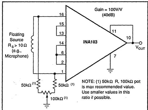
FIGURE 7. Input Offset Adjustment for Floating Source.
