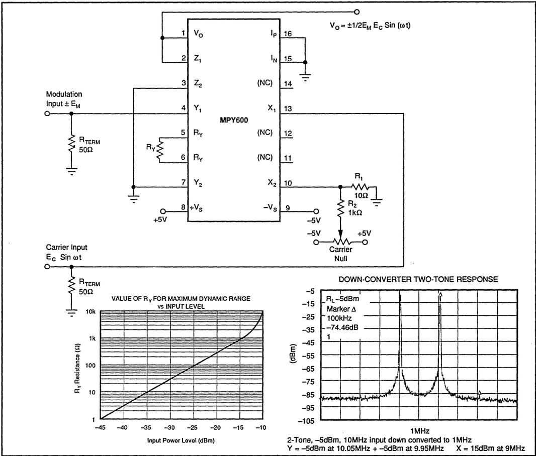
FIGURE 5. Balanced Modulator.
