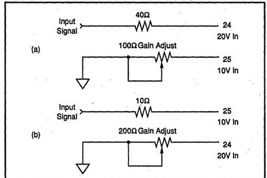
FIGURE 6. Optional Gain Adjust: (a) ±10VBipolar Operation, (b) ±15V Bipolar or 0 to -10V Unipolar Operation
