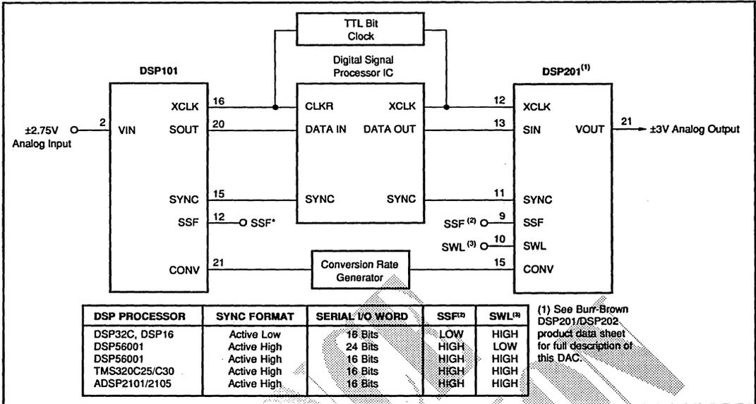
FIGURE 2. Analog Input and Analog Output System.
