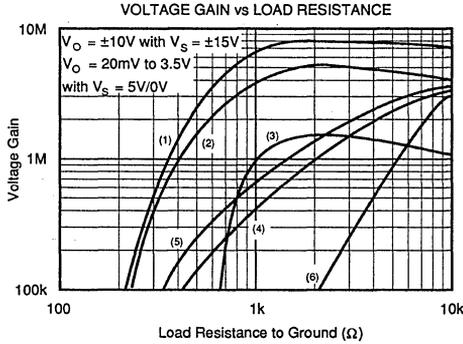
NOTES: (1)  $T_A = -55^\circ\text{C}$ ,  $V_S = \pm 15V$ . (2)  $T_A = +25^\circ\text{C}$ ,  $V_S = \pm 15V$ . (3)  $T_A = 125^\circ\text{C}$ ,  $V_S = \pm 15V$ . (4)  $T_A = +25^\circ\text{C}$ ,  $V_S = 5V/0V$ . (5)  $T_A = -55^\circ\text{C}$ ,  $V_S = 5V/0V$ . (6)  $T_A = 125^\circ\text{C}$ ,  $V_S = 5V/0V$ .
