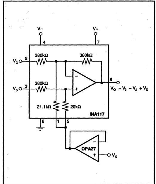
FIGURE 11. Summing V<sub>X</sub> in Output.
