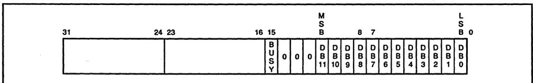
FIGURE 15. Conversion Results in Motorola Register D0.
