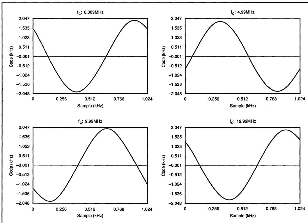
FIGURE 15. Digitized Sine Waves ( $f_s = 10\text{MHz}$ ).
