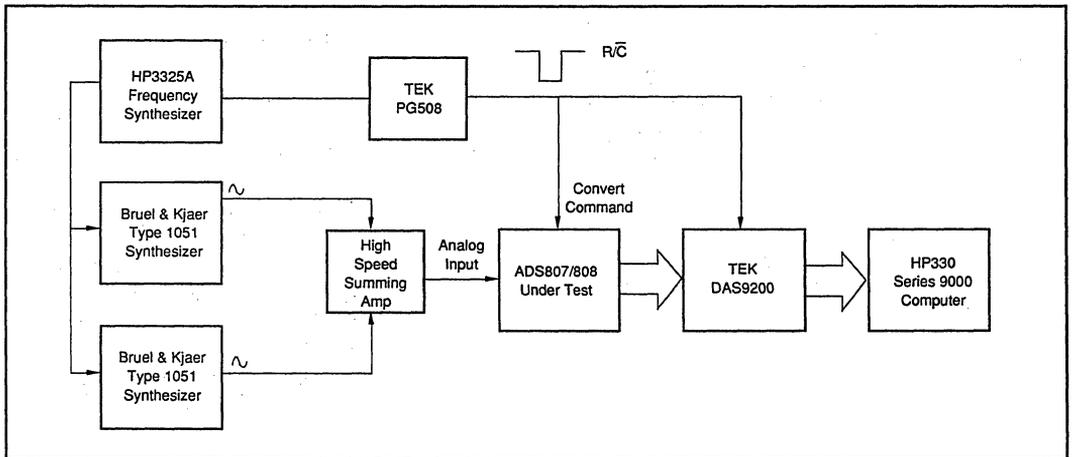
FIGURE 3. Equipment Configuration for Two-Tone Spectral Characterization.
