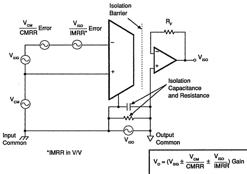
Figure 2. Typical Isolation Amplifier, Voltage (Input) Mode.
