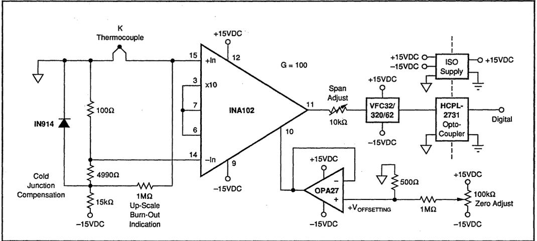
FIGURE 7. Isolated Thermocouple Amplifier with Cold Junction Compensation.
