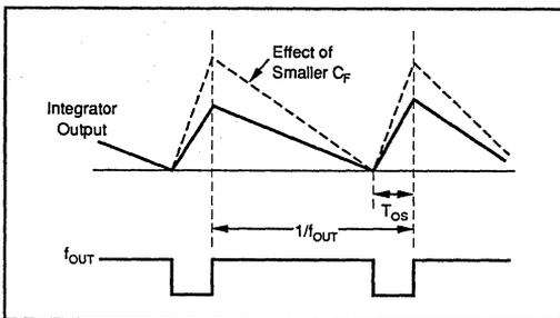
FIGURE 1. Basic Charge-Balance Waveforms.
