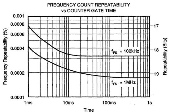
This graph describes the low frequency stability of the VFC110: the ratio of the  $1\sigma$  point of the distribution of 100 runs (where each mean frequency came from 1000 readings for each gate time) to the overall mean frequency.
