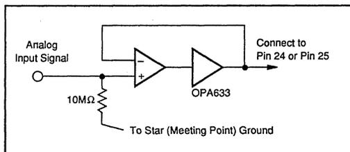
FIGURE 9. Source Impedance Buffering.
