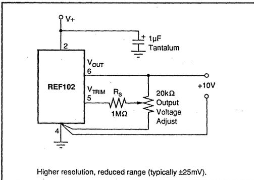
FIGURE 4. REF102 Optional Output Voltage Fine Adjust.
