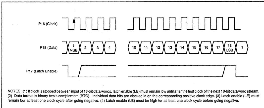
FIGURE 2. PCM61P Timing Diagram.
