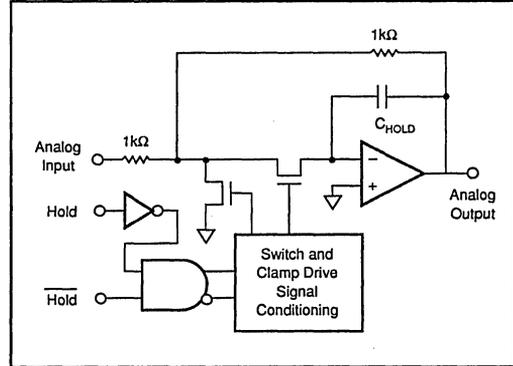
FIGURE 1. Simplified Block Diagram of the SHC702.
