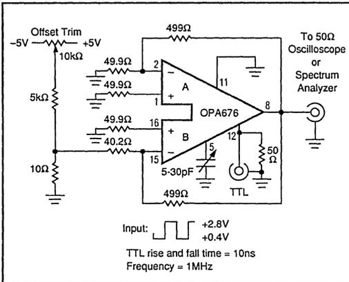
FIGURE 11. OPA676 Carrier Feedthrough and Switching Transient Test Circuit.
