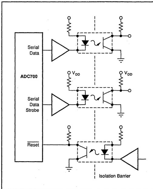
FIGURE 10. Serial Data Output Providing Convenient Isolation.
