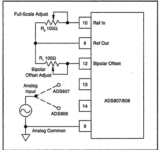
FIGURE 5. Bipolar Connection.
