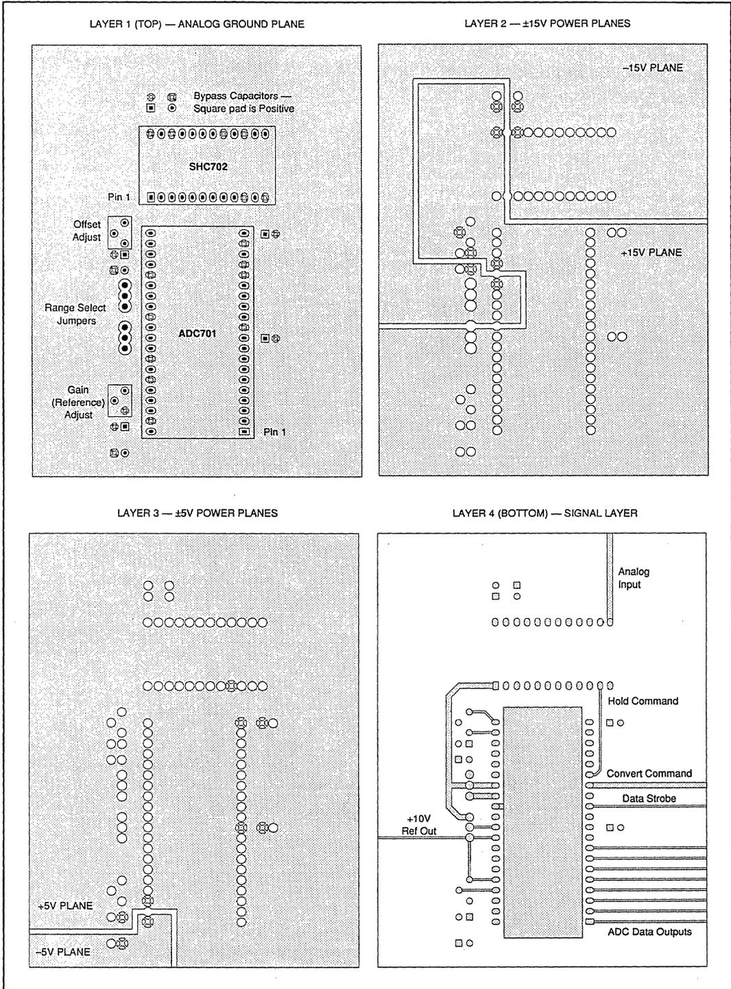
FIGURE 4. Example of Four-Layer PC Board Layout.
