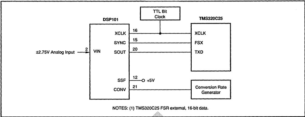
FIGURE 7. Using DSP101 with TMS320C25.
