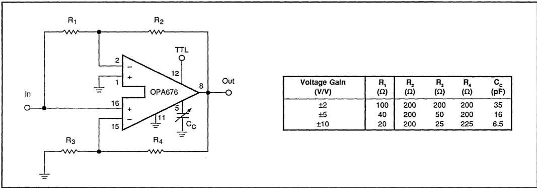
FIGURE 25. Synchronous Modulator/Demodulator (with gain).
