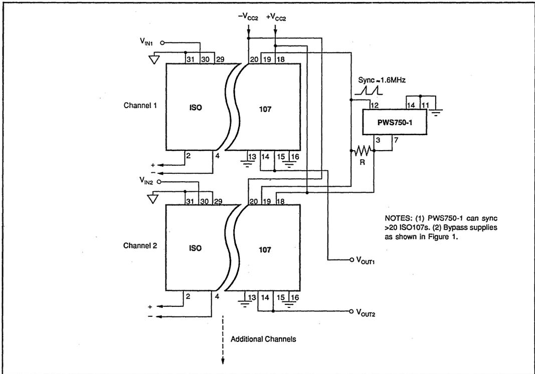
FIGURE 6. Synchronized-Multichannel Isolation.
