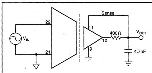
FIGURE 4. Ripple Reduction.
