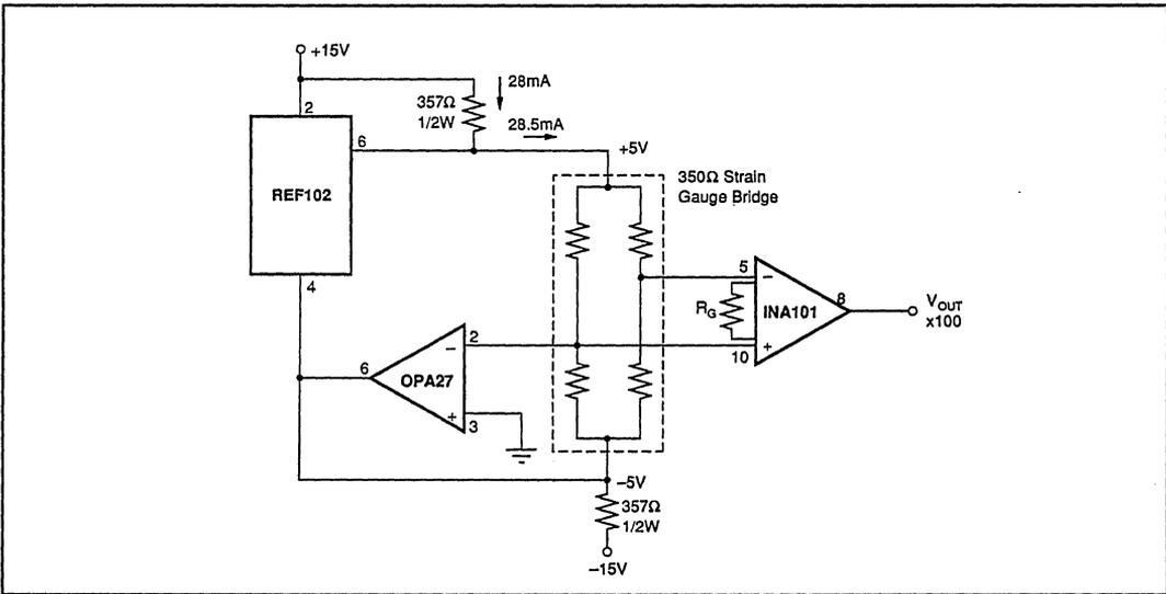
FIGURE 8. Strain Gauge Conditioner for 350Ω Bridge.
