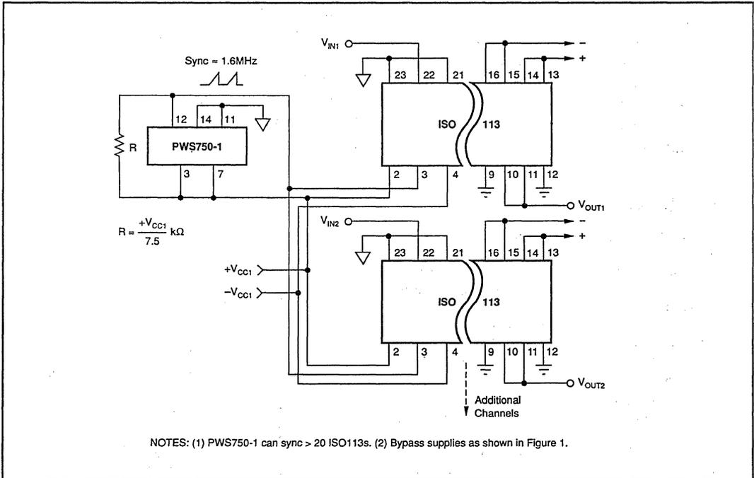
FIGURE 7. Synchronized-Multichannel Isolation.
