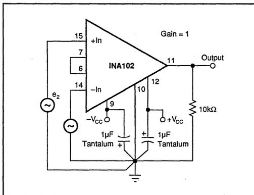
FIGURE 2. Basic Circuit Connection for the INA102.
