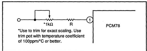
FIGURE 15. PCM78 Input Scaling Circuit.
