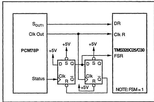
FIGURE 18. PCM78 Interface to TMS320C25/C30 DSP Processors.
