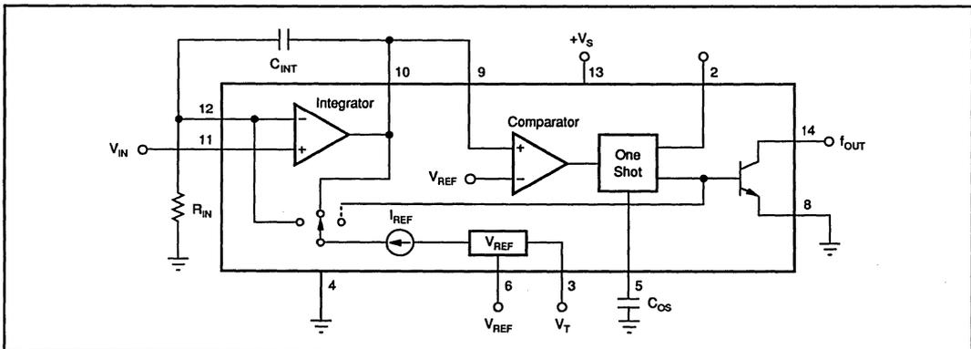
FIGURE 1. VFC121 Architecture.
