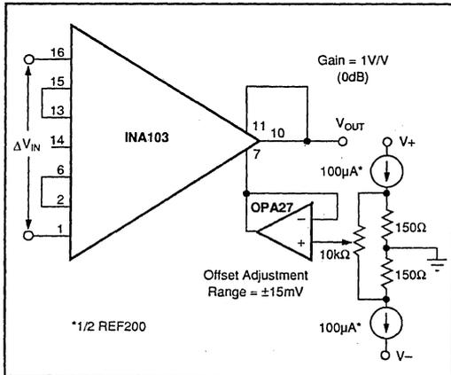
FIGURE 4. Output Offsetting.
