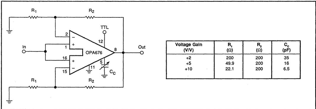
FIGURE 23. Programmable-Gain Amplifier.
