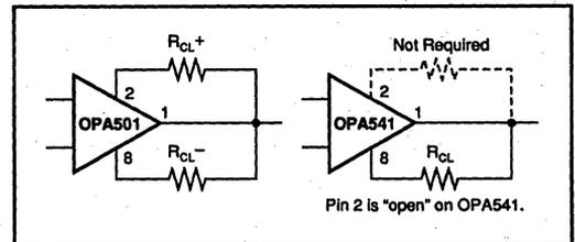
FIGURE 4. Replacing OPA501 with OPA541.
