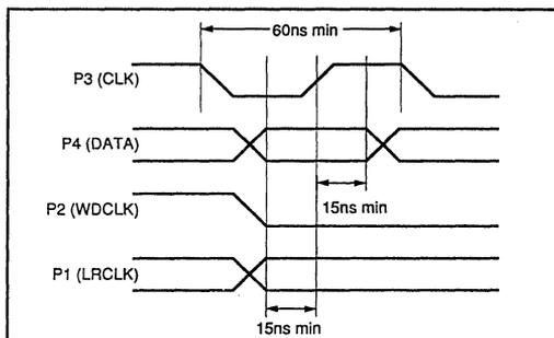
FIGURE 5. PCM60P/66P Setup and Hold Timing Diagram.
