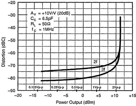
5MHz HARMONIC DISTORTION vs POWER OUTPUT
