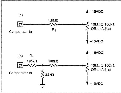
FIGURE 10. Two Methods of Connecting Optional Offset Adjust.
