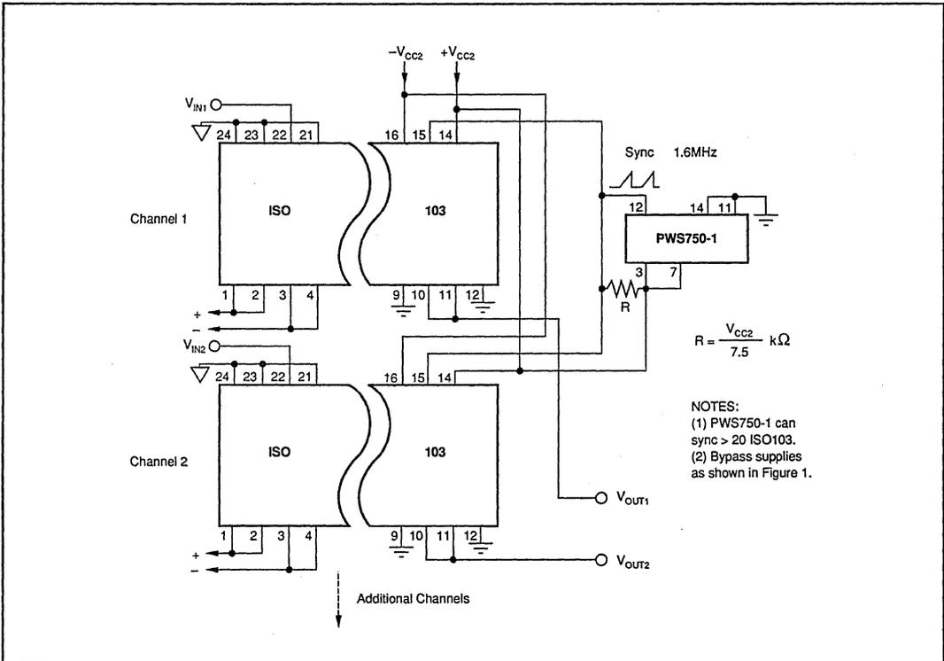
FIGURE 7. Synchronized-Multichannel Isolation.
