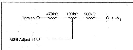
FIGURE 4. MSB Adjust Circuit.
