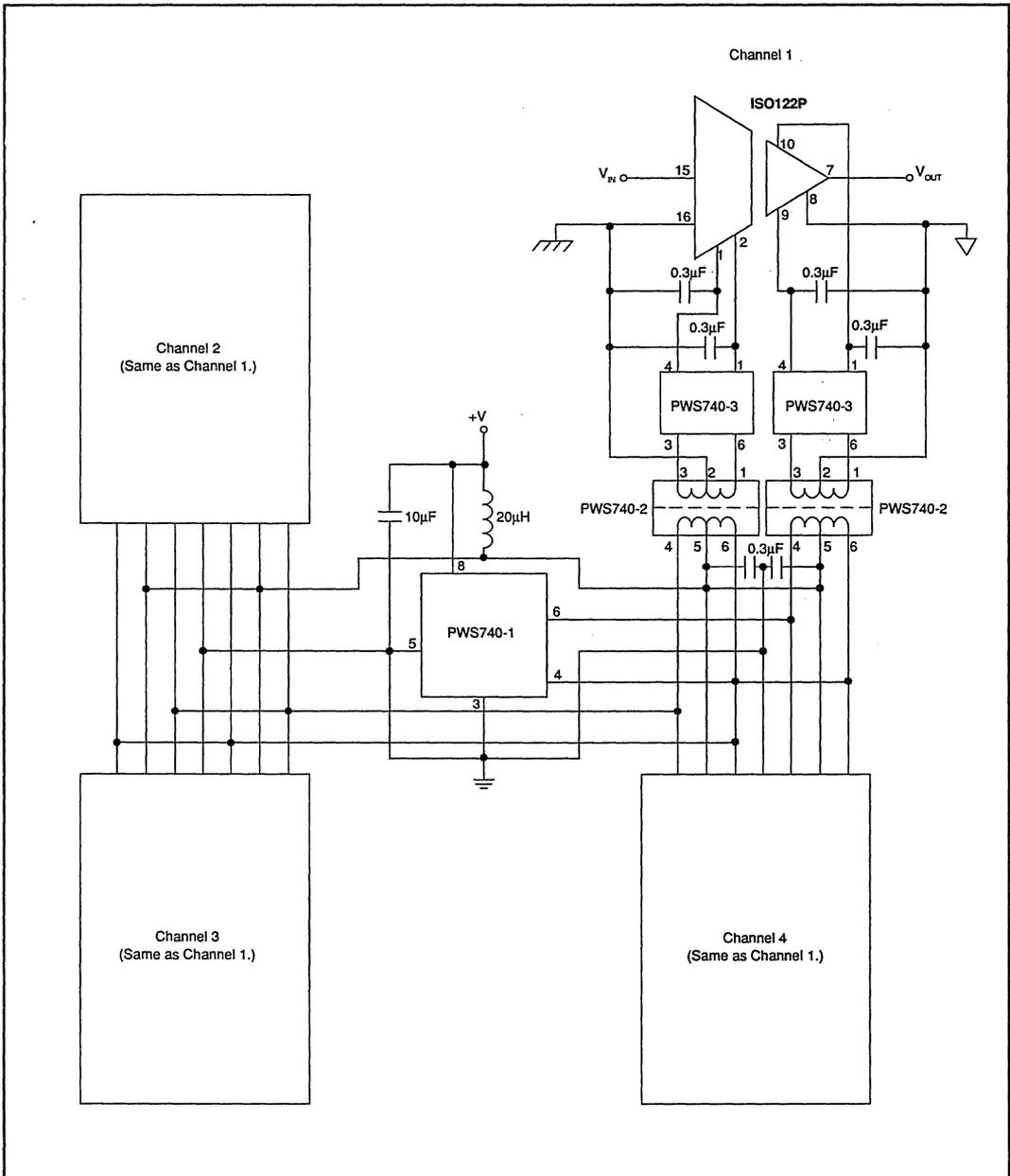
FIGURE 9. Three-Port, Low-Cost, Four-Channel Isolated, Data Acquisition System.
