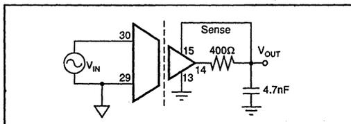
FIGURE 4. Ripple Reduction.
