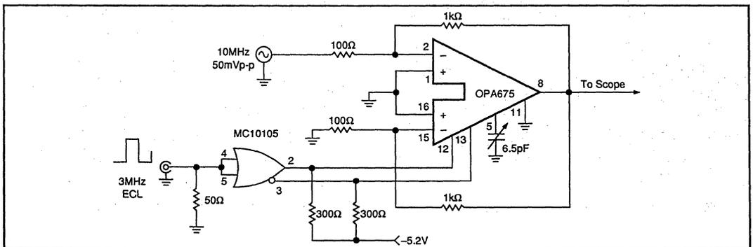
FIGURE 10. OPA675 Input Selection Transition Time Test Circuit.
