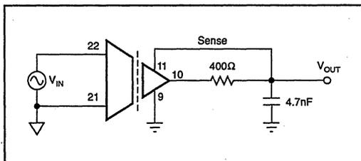
FIGURE 4. Ripple Reduction.
