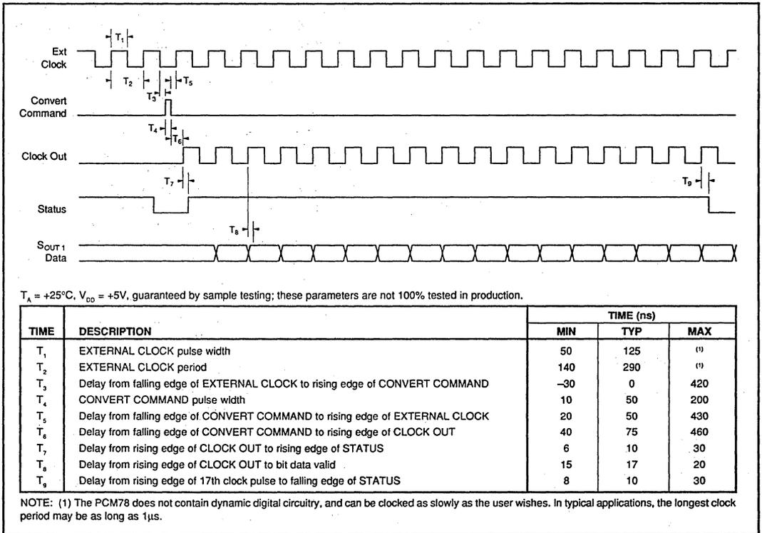
FIGURE 7. Conversion Timing when using External Clock.
