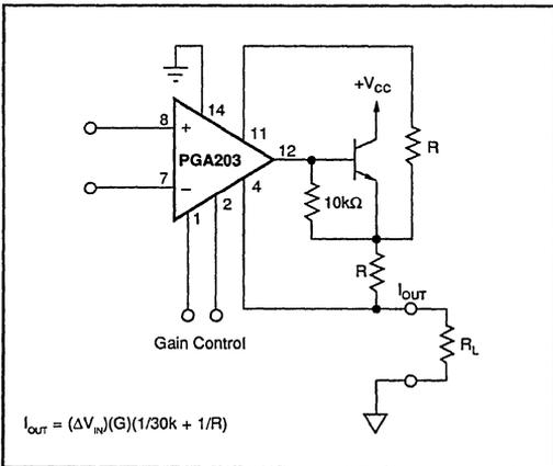
FIGURE 10. Programmable Current Source.
