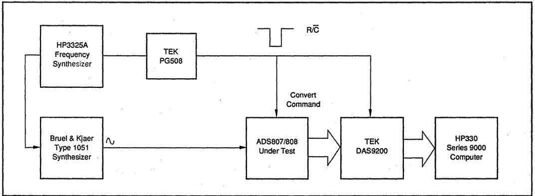
FIGURE 2. Equipment Configuration for Single-Tone Spectral Characterization.
