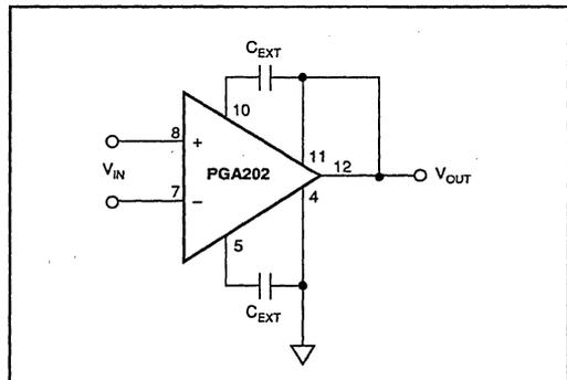
FIGURE 5. Output Filtering.
