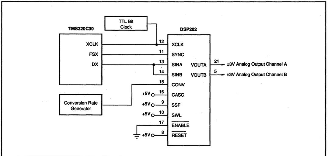
FIGURE 5. Using DSP202 with TMS320C30 in Cascade Mode.
