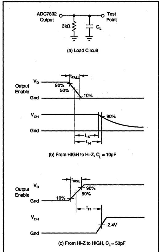
FIGURE 8. Measuring Active HIGH to/from Hi-Z State.
