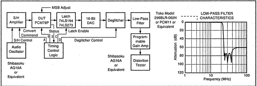
FIGURE 4. Production Distortion + Noise Test System Block Diagram.
