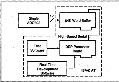
FIGURE 1. Single Channel Analog Input System.
