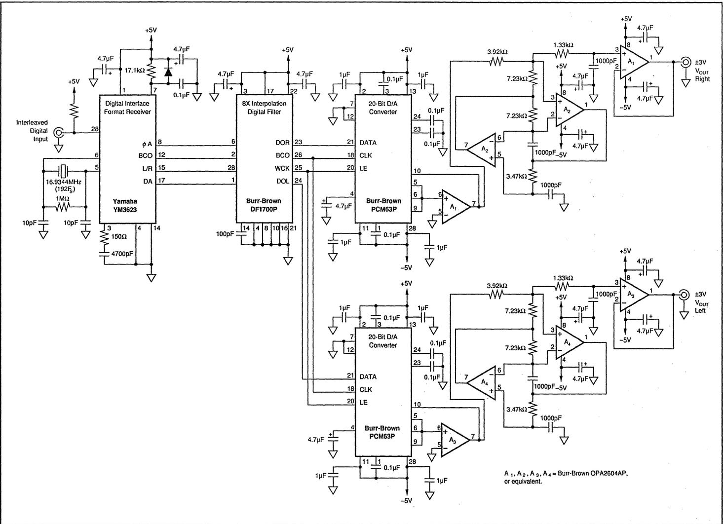
A<sub>1</sub>, A<sub>2</sub>, A<sub>3</sub>, A<sub>4</sub> = Burr-Brown OPA2604AP, or equivalent.
