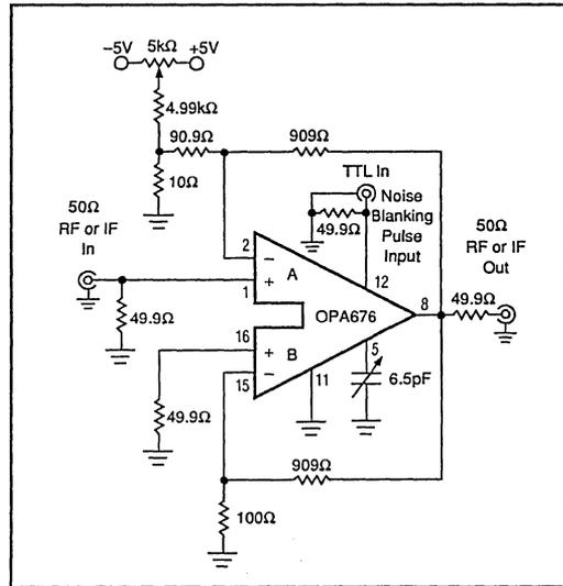
FIGURE 20. Receiver Noise Blanker: A Wideband Gated Video Amplifier.
