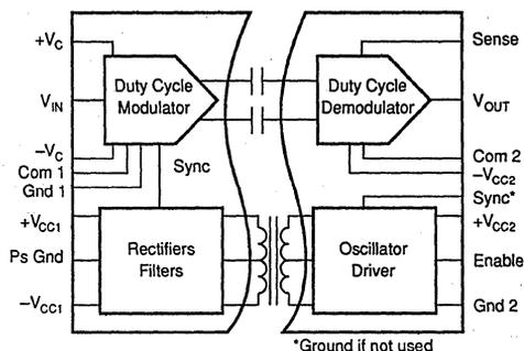
rol is used to turn off transformer drive while keeping the signal channel demodulator active. This feature provides a convenient way to reduce quiescent current for low power applications.
