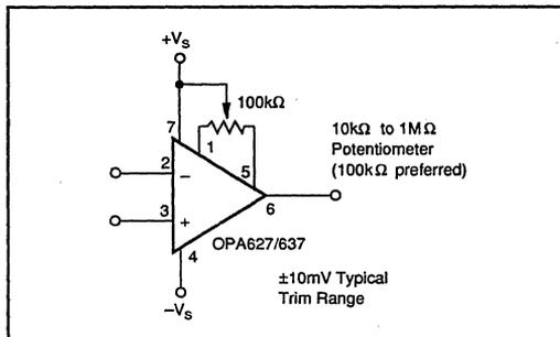
FIGURE 3. Optional Offset Voltage Trim Circuit.
