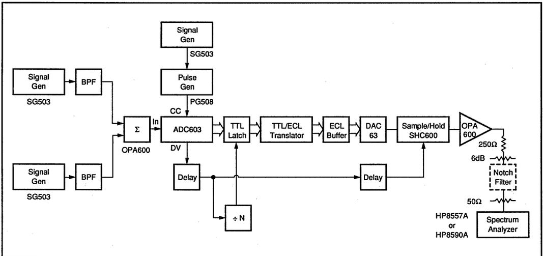
FIGURE 17. Analog-to-Analog Spectral Analysis by Beat-Frequency Techniques.
