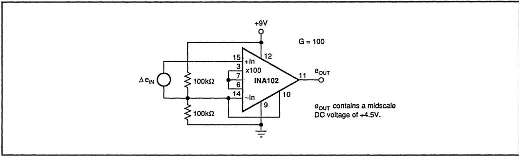
FIGURE 9. Single Supply Low Power Instrumentation Amplifier.
