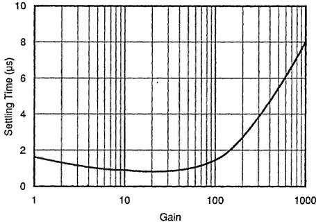
SETTLING TIME vs GAIN
