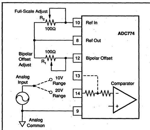
FIGURE 3. Bipolar Configuration.
