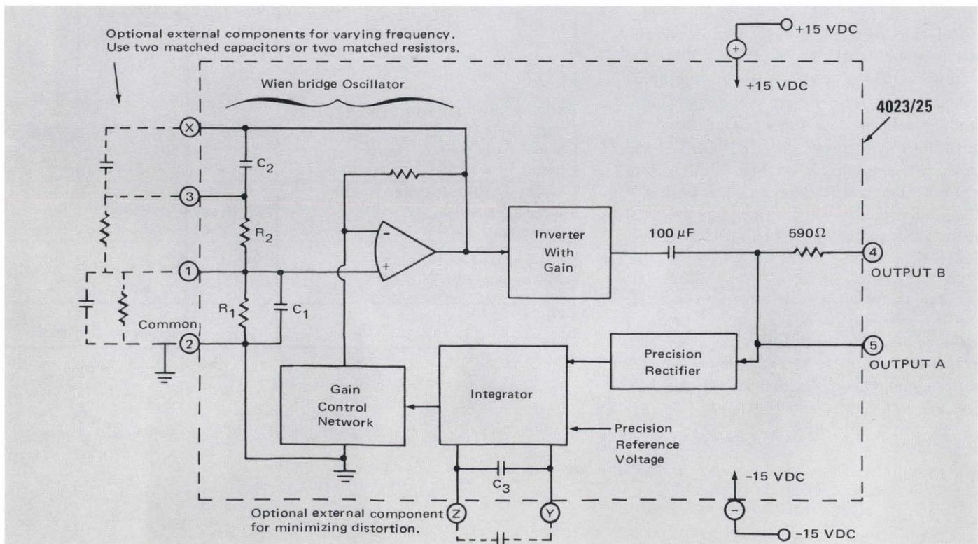
**SIMPLIFIED SCHEMATIC DIAGRAM OF MODEL 4023/25**
