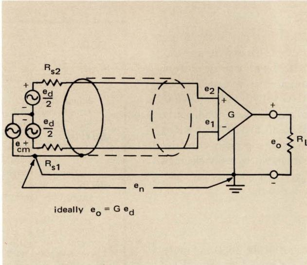
FIGURE 3. Typical Application of Instrumentation Amplifier.
