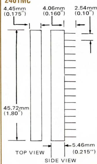
A set of four 18-pin connector strips for PC board mounting.
