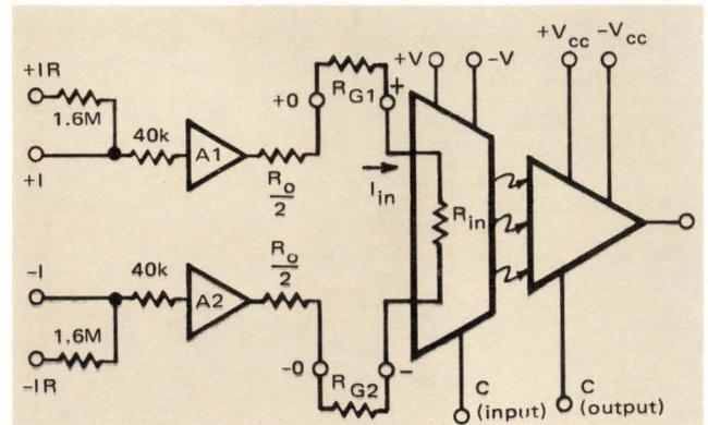
FIGURE 5. Simple Model of 3652.
