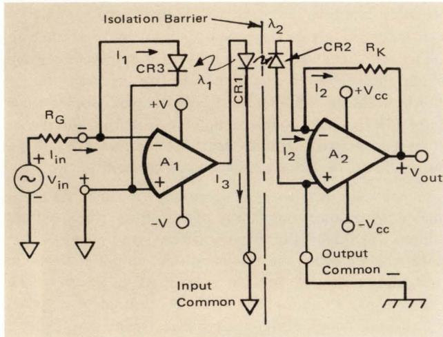
FIGURE 3. Improved Linear Isolator.
