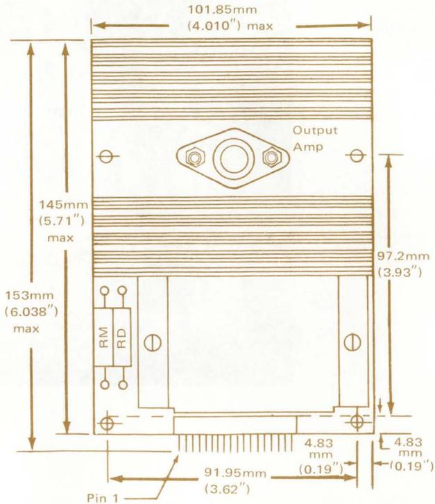
Material: Extruded, black-anodized, aluminum heat sink and discrete components mounted on glass epoxy printed circuit board.
