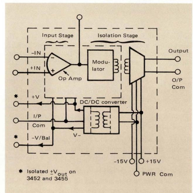
FIGURE 2. Simplified Block Diagram of Transformer Coupled Isolation Amplifiers.
