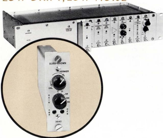
The 3640 offers excellent performance at a surprisingly low cost. The direct-coupled, differential input stage provides resolution of microvolt signals through the use of a low noise, monolithic amplifier. Low DC input drift is assured by proprietary input stage balancing techniques. Linearity of 0.01% and gain accuracy of 0.1% are achieved through the use of heavy negative feedback and precision, high stability resistors.
