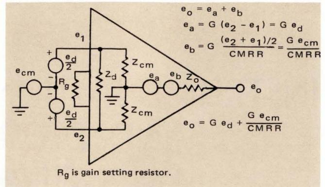
FIGURE 2. Model Of An Instrumentation Amplifier.
