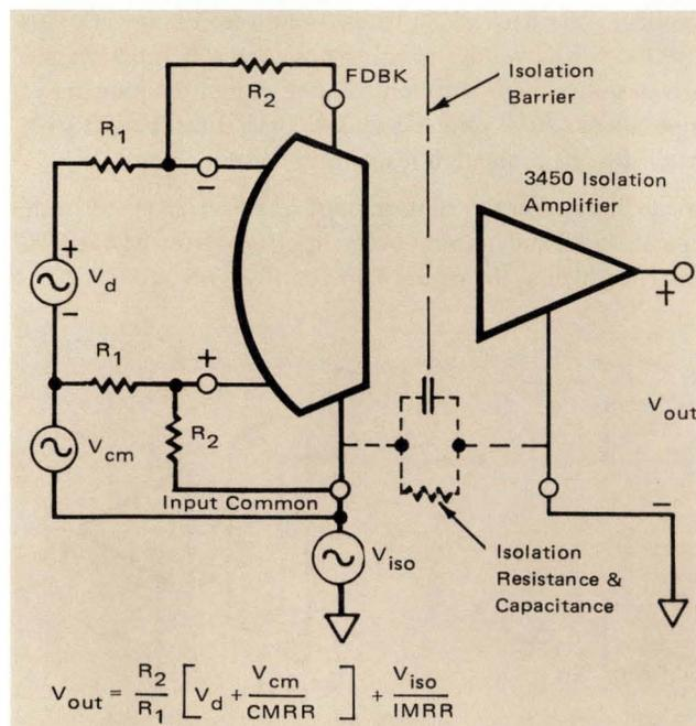
FIGURE 1. Typical Isolation Amplifier Application.
