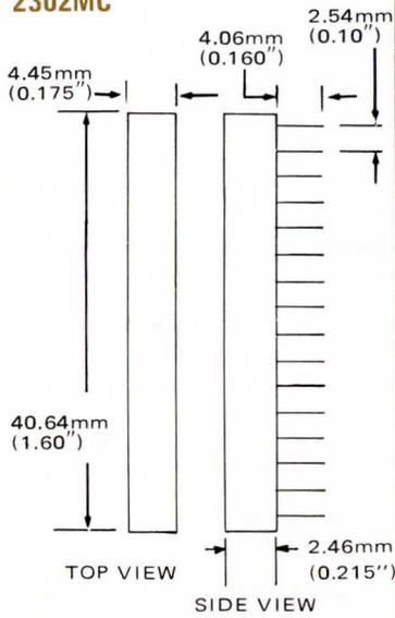
A set of two 16-pin connector strips for PC board mounting.
