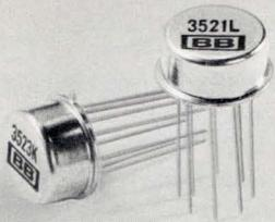
These amplifiers are designed to have high input impedance (approximately  $10^{11}\Omega$ ) and very low bias currents (0.01 to 25 pA). They are especially useful for impedance buffering of high impedance current sources. This group includes varactor, IC, and modular devices. The varactors feature ultra low bias currents and low input noise, but are limited in frequency response. The IC devices have good all-around performance and are low cost.
