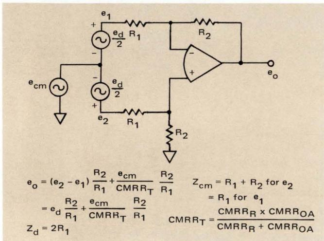
FIGURE 1. Single Op Amp, Differential Input Configuration.
