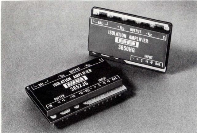
The 3650 and 3652 are the industry's first optically coupled isolation amplifiers. Compared to transformer coupled units they have the advantages of smaller size, lower cost, wider bandwidth and integrated circuit reliability.
