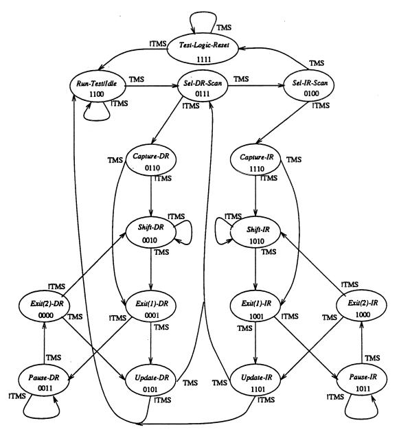
Figure 10-1. TAP Controller State Diagram
