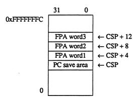
Figure 2-4. Floating-point Accumulator
