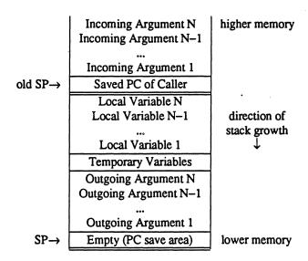
Figure 2-14. Typical Stack-frame
