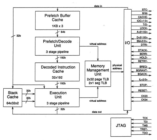
Figure 1-1. ATT2100 Functional Block Diagram
