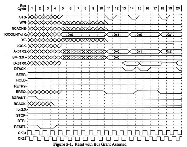
A reset sequence can be internally generated. If there is a bus transaction owned by the ATT2100 in progress when the internal reset is generated, the transaction is allowed to complete prior to execution of the reset sequence. There is no external indication that an internal reset has occured other than the text fetch which occurs at location 0x0 after the internal reset sequence completes. Section 2.13.1 gives details on the internal reset sequence.
