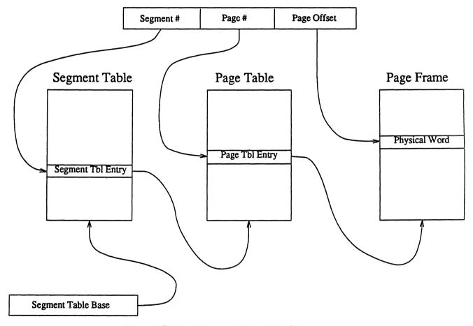
Figure 6-7. Paged Segment Address Mapping
