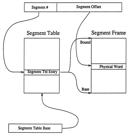
Figure 6-8. Non-paged Segment Address Mapping
