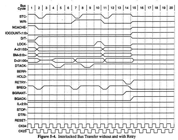
NOTE: The bus transaction may be ended by RESET- or BERR- with DTACK- to signal an exception.
