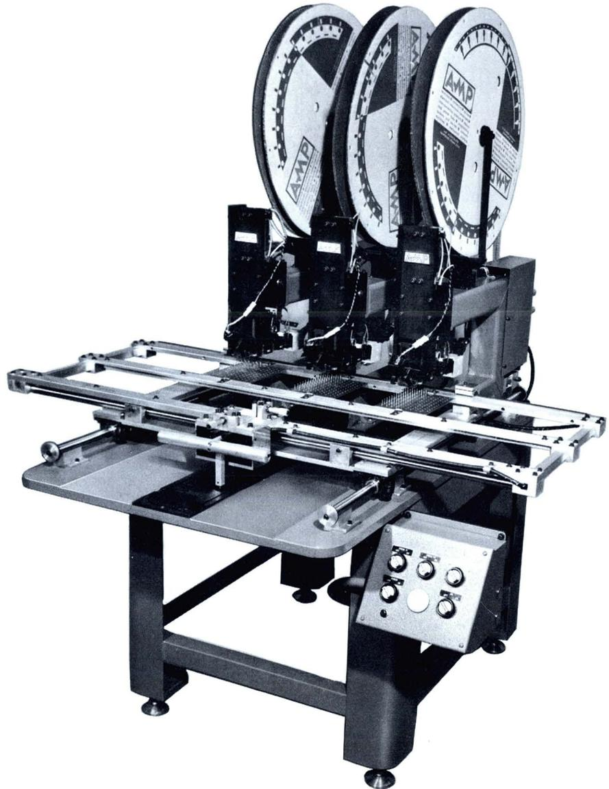
The Multi-Head Insertion Machine is a stand-mounted unit equipped with a movable work table with an adjustable position stylus and a conveniently located control panel and has the ability to accept 1, 2 or 3 presses and miniature inserter applicators. The stylus is template controlled and requires two-hand operation for operator safety. The machine will accept a variety of strip-fed reel-stored AMP pc board posts,
