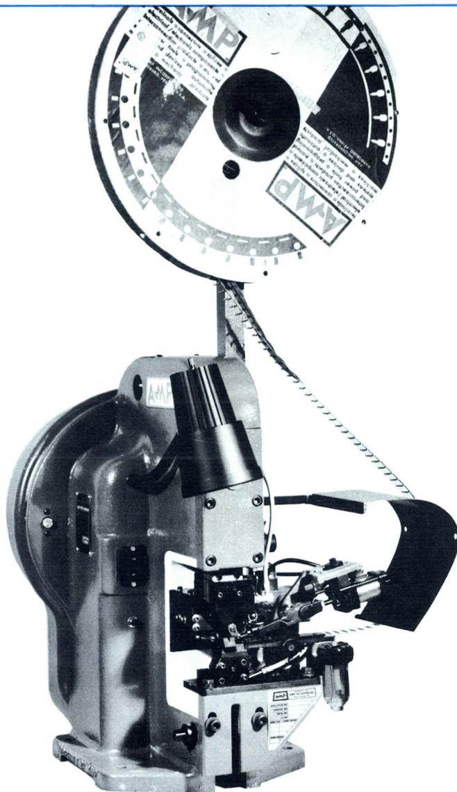
The AMP-O-MATIC Stripper/Crimper Machine is an electro-pneumatic machine consisting of a slightly modified AMP-O-ELECTRIC Press and an almost "standard" side-fed Miniature Applicator. Designed to accommodate wire employing non-metallic insulations, this machine strips wire in the #16 - 26 AWG ranges and terminates the wire with strip-fed, open-barrel terminals. In a single operation, the wire is located then automatically gripped, stripped and terminated.
