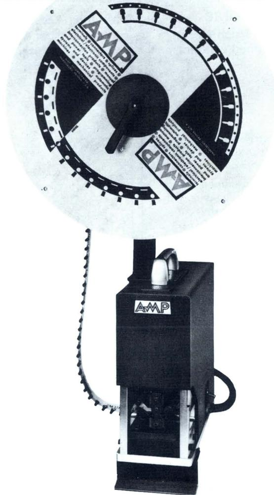
The AMP-TAPEMATIC machine, no. 68075, is designed to terminate a variety of tape-mounted pre-insulated and uninsulated products to pre-stripped solid or stranded wire. It offers a day-in and day-out production of top quality terminations at rates up to 1,800 an hour. The unit itself is extremely compact, completely portable . . . and takes up very little bench space. Only 5" wide x 14" high x 12" deep and weighing a mere 35 lbs., it can be easily transported from one location to another.
