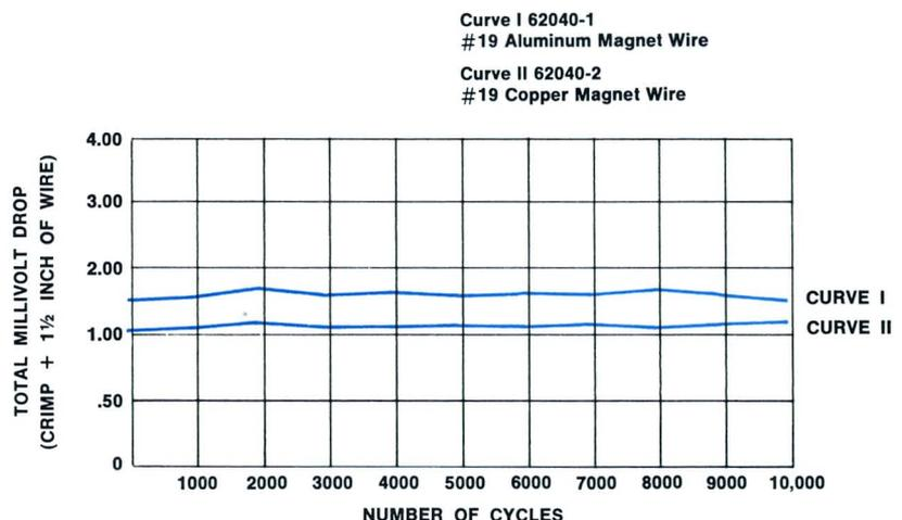
**Current Cycling:** The splices were subjected to 10,000 cycles of current cycling at the current (24 amperes) which established a wire temperature of 150°C. Duration of the cycle was 3 minutes on and 3 minutes off.
