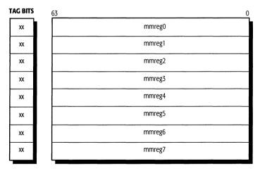
Aliasing the MMX registers onto the floating-point stack registers provides a safe way to introduce this new technology. Instead of needing to modify operating systems, new MMX applications can be supported through device drivers, MMX libraries, or DLL files. See the *Programming Considerations* section of this document for more information.
