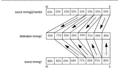
In the functional illustration of the PUNPCKLBW instruction, the 8-bit values from mmreg1 are stored in the low-order 8 bits of the 16-bit result. The mmreg2/mem64 source operand is set to all zero bits so it can provide zero fill in the high-order 8 bits of the 16-bit result. This is a method that can be used to expand unsigned 8-bit values into unsigned 16-bit operands for subsequent processing that requires higher precision.
