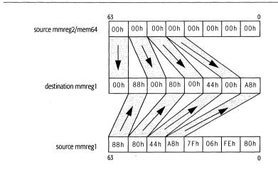
In the functional illustration of the PUNPCKHBW instruction, the 8-bit values from mmreg1 are stored in the low-order 8 bits of the 16-bit result. The mmreg2/mem64 source operand is set to all zero bits so it can provide zero fill in the high-order 8 bits of the 16-bit result. This is a method that can be used to expand unsigned 8-bit values into unsigned 16-bit operands for subsequent processing that requires higher precision.
