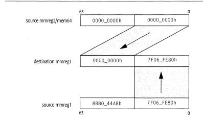
In the functional illustration of the PUNPCKLDQ instruction, the 32-bit value from mmreg1 is stored in the low-order 32 bits of the 64-bit result. The mmreg2/mem64 source operand is set to all zero bits so it can provide zero fill in the high-order 32 bits of the 64-bit result. This is a method that can be used to expand unsigned 32-bit values into unsigned 64-bit operands for subsequent processing that requires higher precision.
