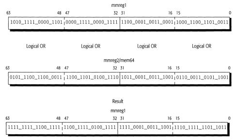
In the functional illustration of the POR instruction, the 64-bit source value is logically OR'd to the 64-bit destination value, and the result is stored in the destination register.
