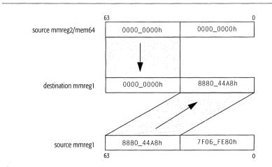
In the functional illustration of the PUNPCKHDQ instruction, the 32-bit value from mmreg1 is stored in the low-order 32 bits of the 64-bit result. The mmreg2/mem64 source operand is set to all zero bits so it can provide zero fill in the high-order 32 bits of the 64-bit result. This is a method that can be used to expand unsigned 32-bit values into unsigned 64-bit operands for subsequent processing that requires higher precision.
