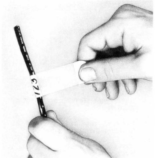
**Fig. 1—♦Placing Self-Laminating Label♦**
