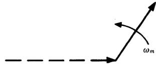
FIG. 5-6. Upper sideband and reference carrier phasors for SSB signal.
