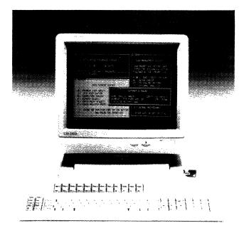
Lee Data's Model 1222 Open Window Display provides users with a choice of four screen capacities, plus windowing capabilities. Up to four windows can be displayed on the screen simultaneously, in any combination of 3270 mode and/or Async mode sessions.
