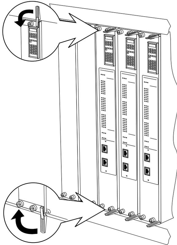
Figure 2-4. Seating Module Connectors
